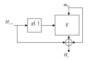
Figure 5: Miyaguchi-Preneel hash construction [10].
