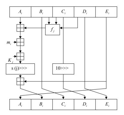
FIGURE 11: Step function of RIPEMD-160 [86].
