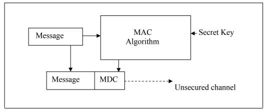
Figure 24: Data integrity using a 'MAC' alone.
