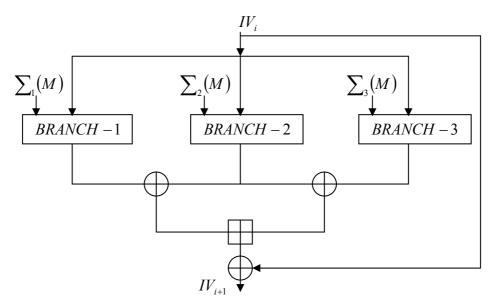
Figure 19: Structure of 3-branch hash function.
