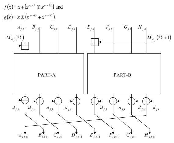
Figure 20: Step function of 3-branch hash function.
