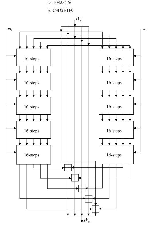
Figure 10: Processing of single 512-bit block in RIPEMD-160 [86]. Step 4: Processing message in 512-bit blocks:
