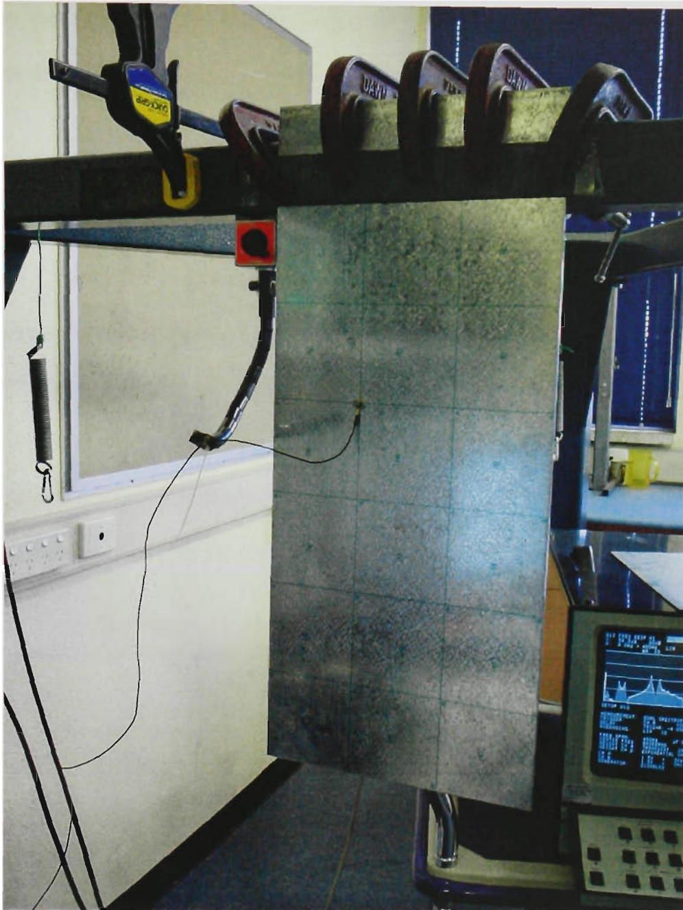
**Figure 6.6** Experimental Setup of Plate28 without Damage
