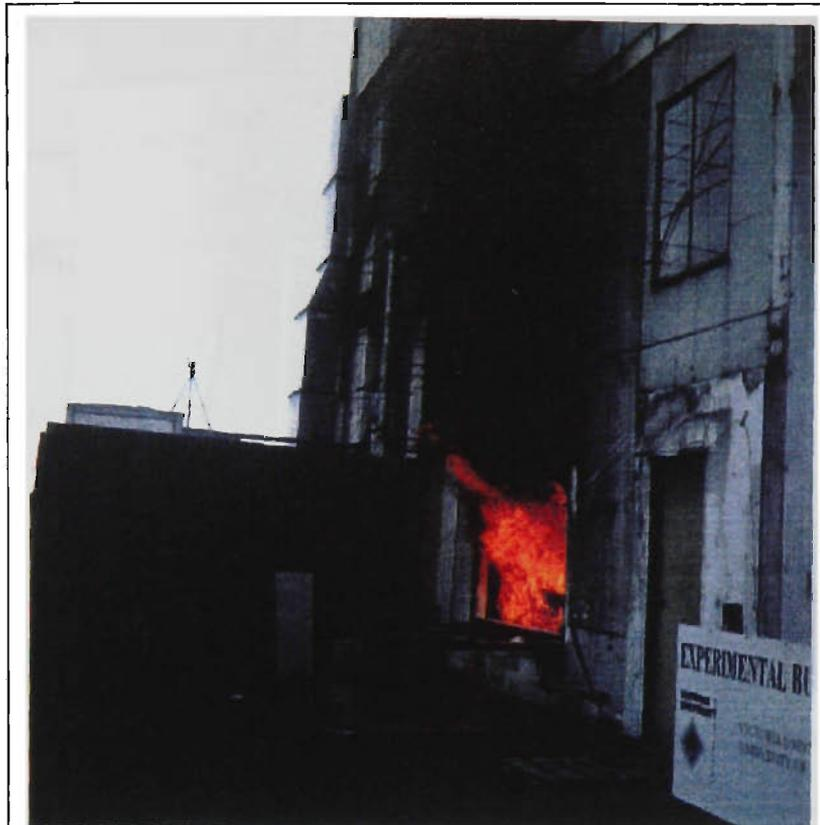
*Figure 5.3:* Growth phase, side view, at approximately 6½ minutes after ignition during Burn 8.
