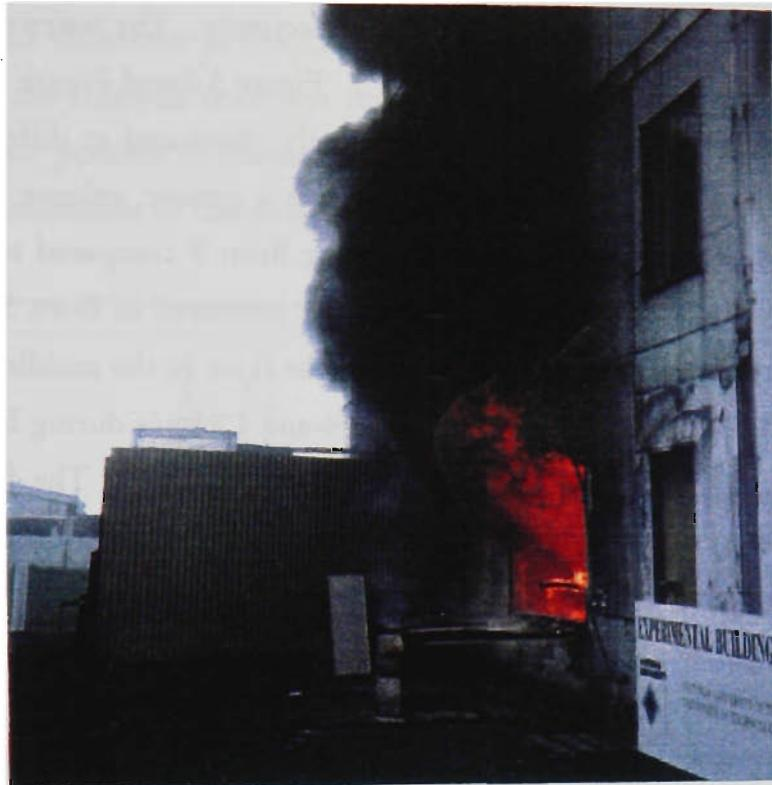
*Figure 5.5:* Fully developed phase, side view, at approximately 8 minutes after ignition during Burn 8.
