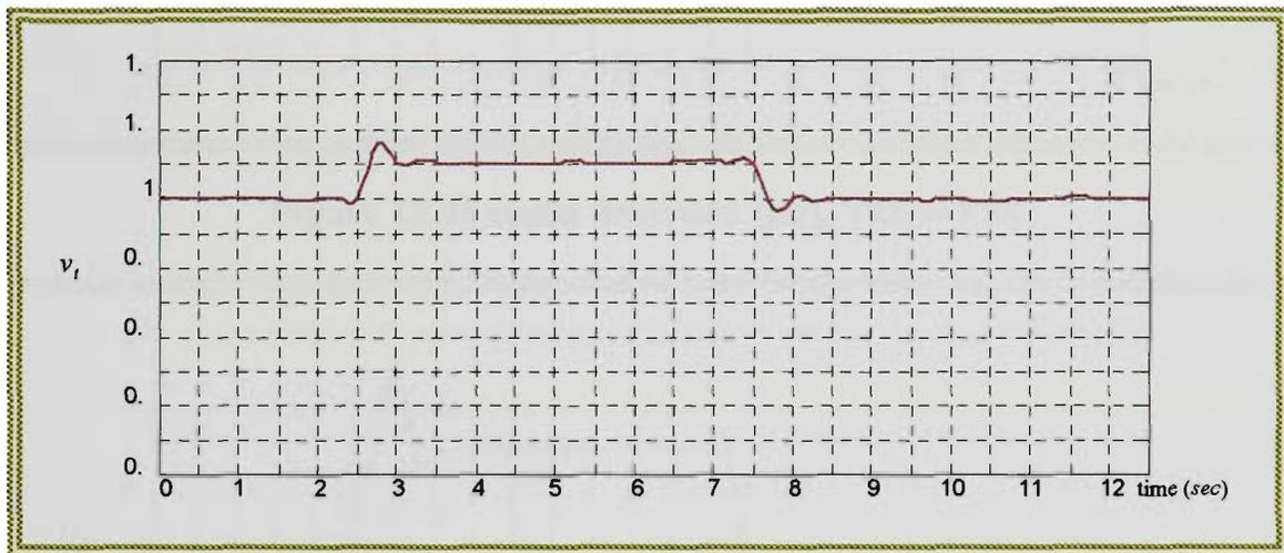
Figure 12.41 terminal voltage (pu), TEST-VS4
