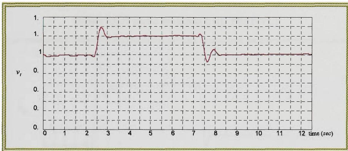
**Figure 12.45 terminal voltage (pu), TEST-VL1**
