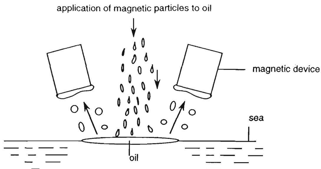
**Figure 1.1** : Schematic diagram of method and device for collecting oil magnetically (Adapted from Wessman, 1981).
