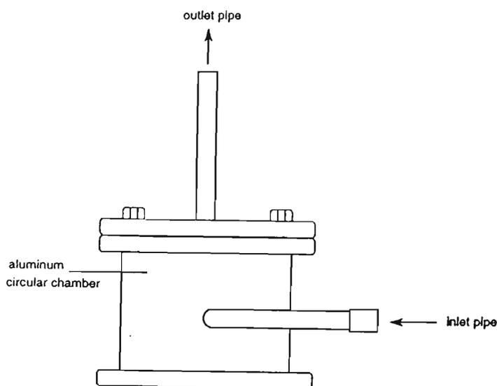
**Figure 2.5 :** Apparatus based on a crystal spherising chamber.
