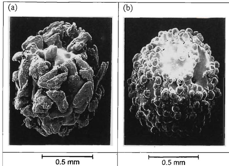
**Figure 2.4** : Scanning electron micrographs of: (a) PE-coated particles and (b) PVC-coated particles.
