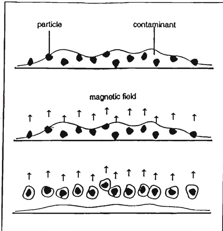
**Figure 1.6 :** Schematic diagram of oil-laden magnetic particles being magnetically harvested.
