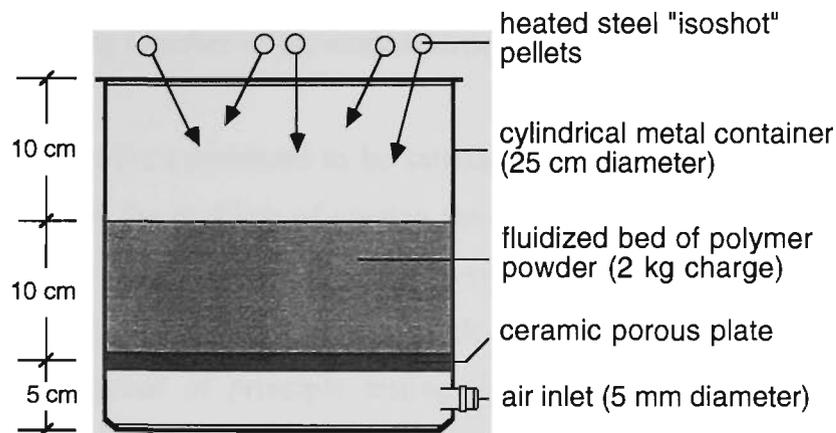
**Figure 2.2** : Schematic diagram of fluidised bed apparatus
