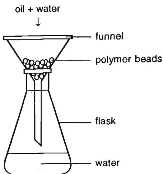
**Figure 1.5 :** Schematic diagram of an apparatus for separating water from oil.
