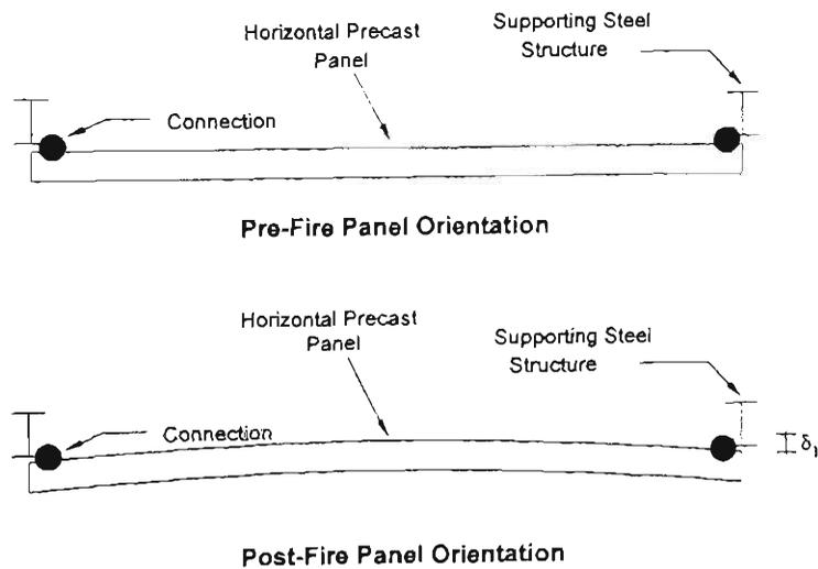
**CASE B Wall Deformation Between Supports - Horizontally**
