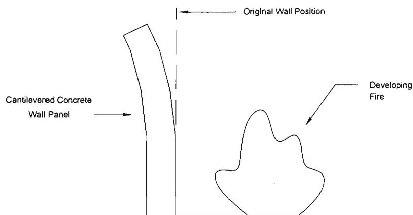
Figure 2.10 Deformation of a Cantilevered Wall
