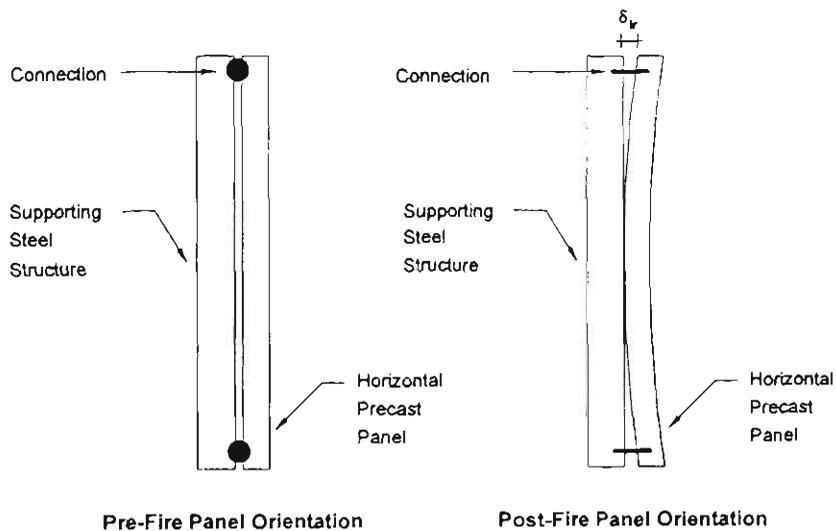
**CASE A Wall Deformation Between Supports - Vertically**
