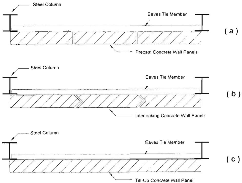
**Figure 2.5** Schematic View of Various Vertical Panel Lateral Support Systems
