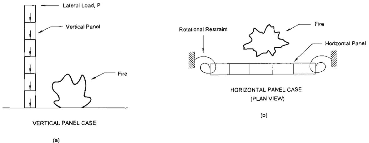
**Figure 3.3** The Two Cases as Modelled for the Analysis
