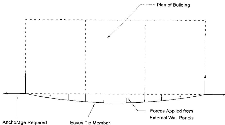
**Figure 2.13** Anchorage of External Eaves Tie Member
