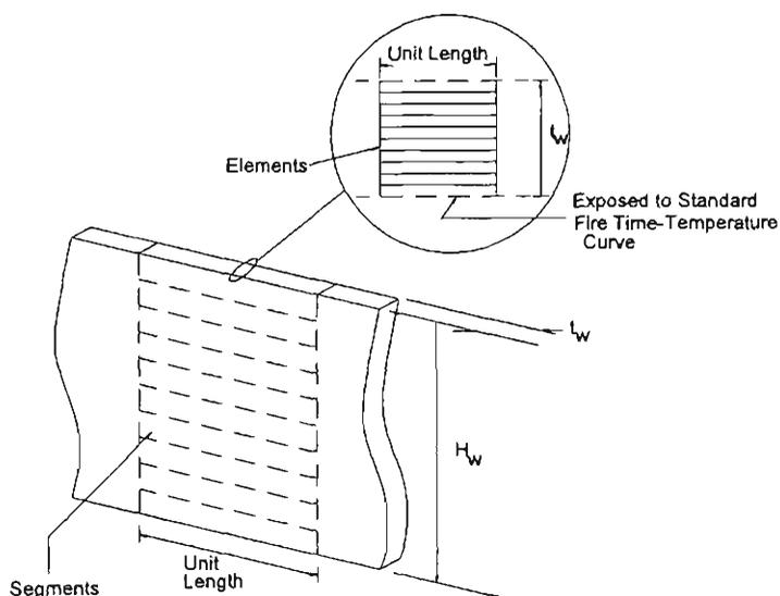
**Figure 3.4** Discretisation of the Cantilevered Concrete Wall
