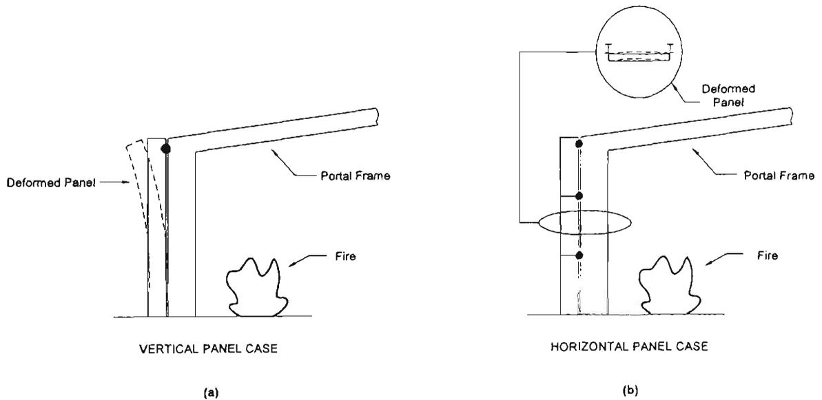
**Figure 3.2** The Two Cases Analysed for the Wall Model Study
