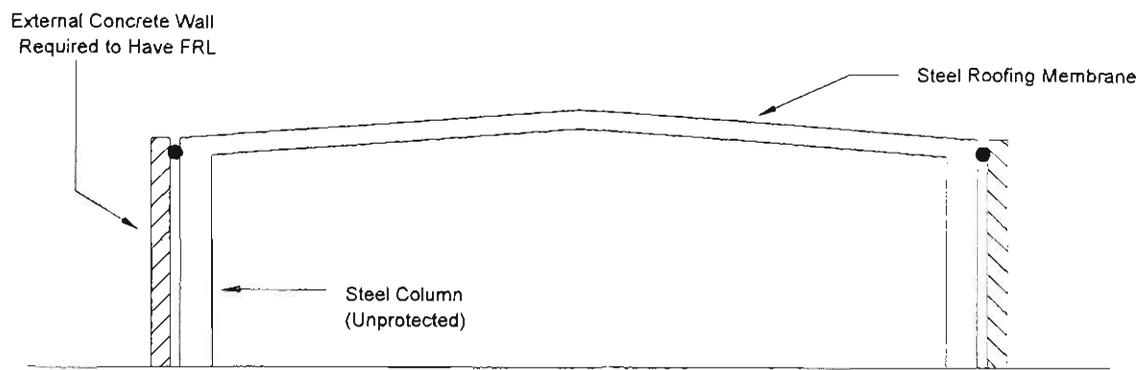
**Figure 2.1** BCA Concession for Steel Columns
