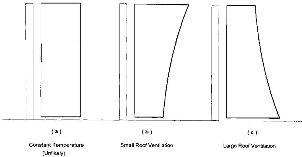
**Figure 4.1** Temperature Distributions of Cases Considered in Modelling
