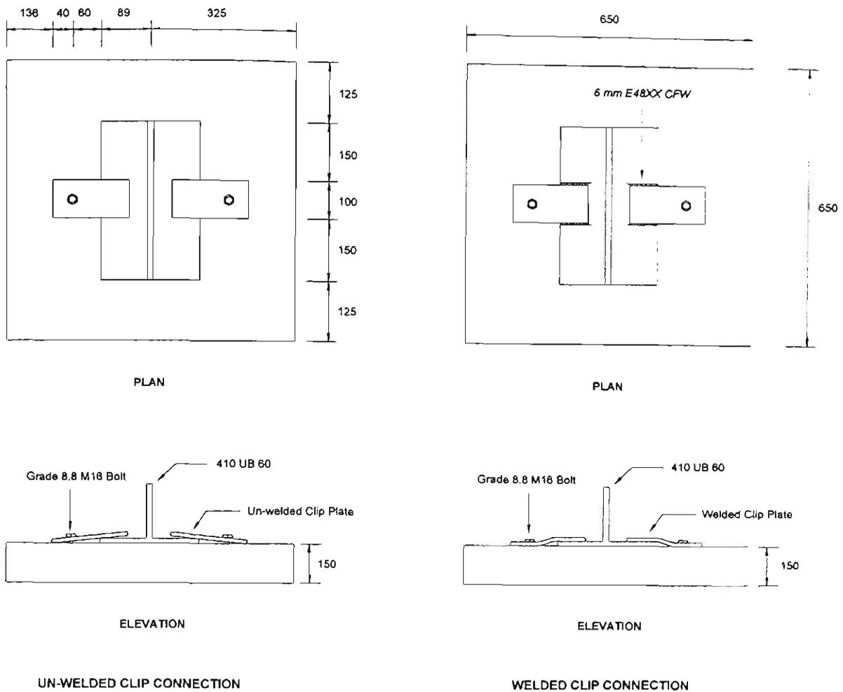
**Figure 5.4** Details of Connection Samples Tested
