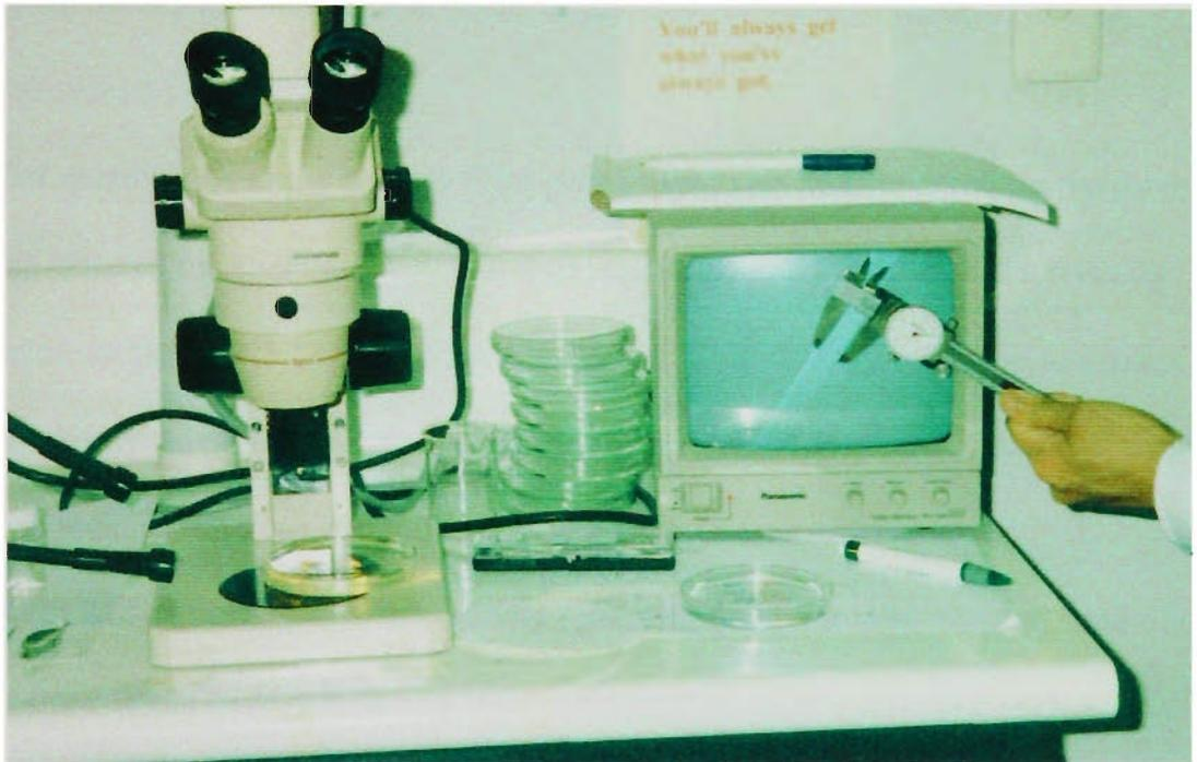
**Figure 2.2** Video camera-monitor system used to measure the size of single fibres with a pair of callipers.
