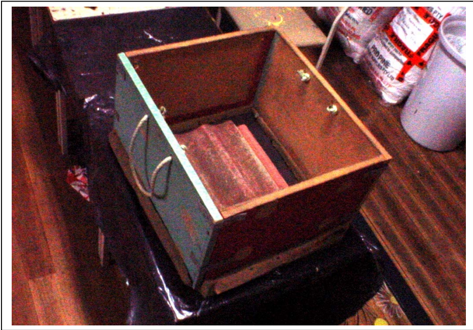
Figure 3.9: The roof tile monitoring box, with sample roof tile inside.
