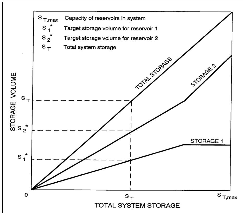
Figure 2-2. Target Storage Curves for a Typical Two-Reservoir System.
