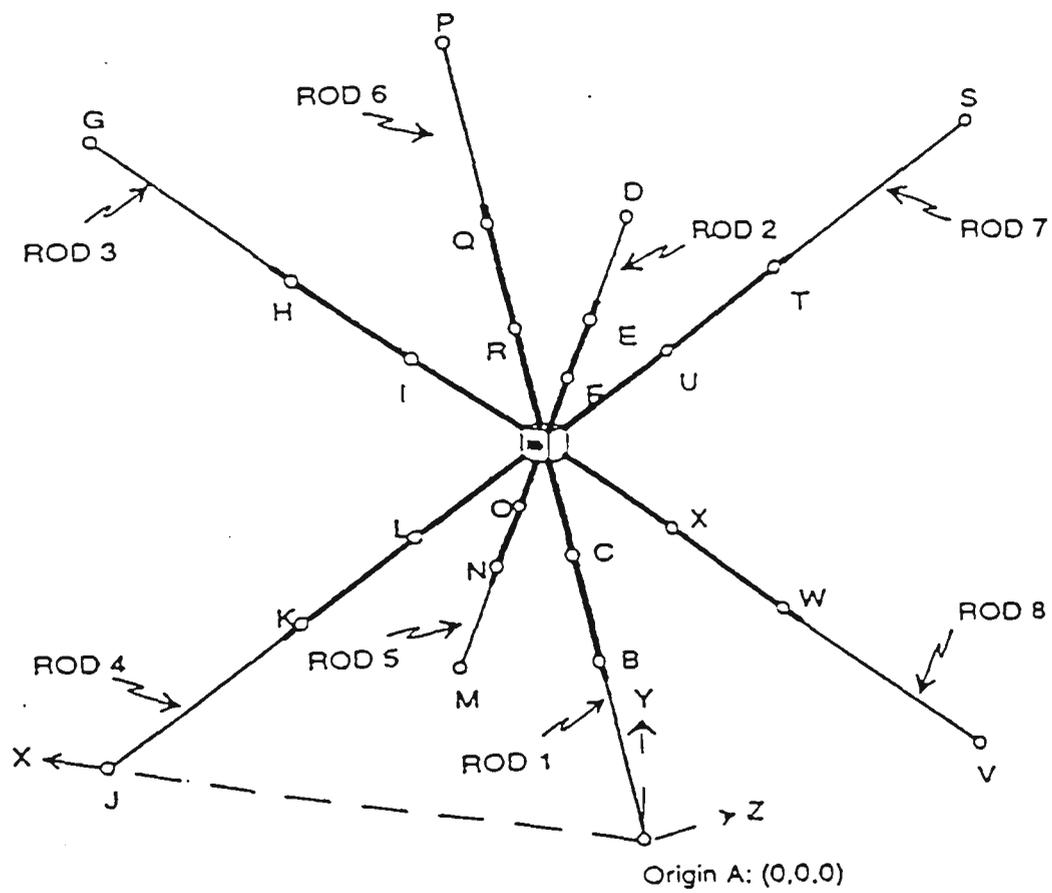
Figure 3.2.2.4.1 PEAK System Calibration Frame (Adapted from PEAK 5, 1993)
