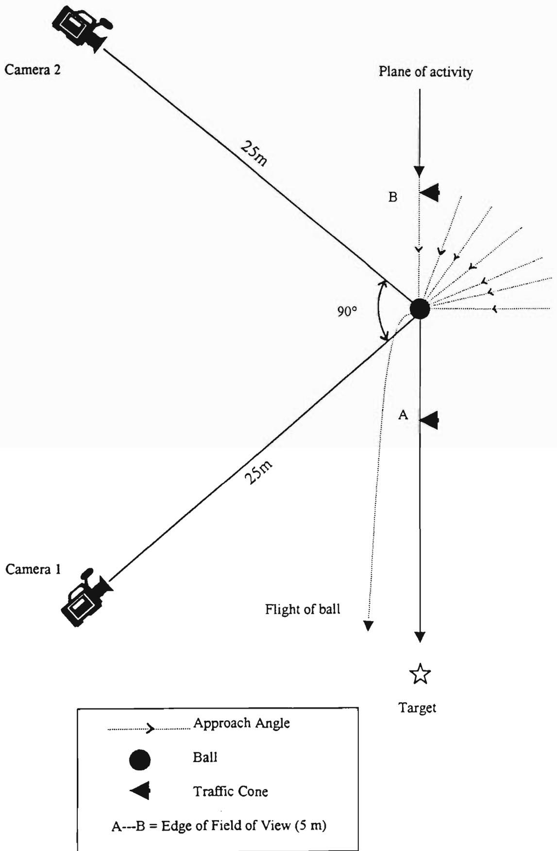
Figure 3.2.2.1.1 Plan View of Equipment Set-Up for the Experiment
