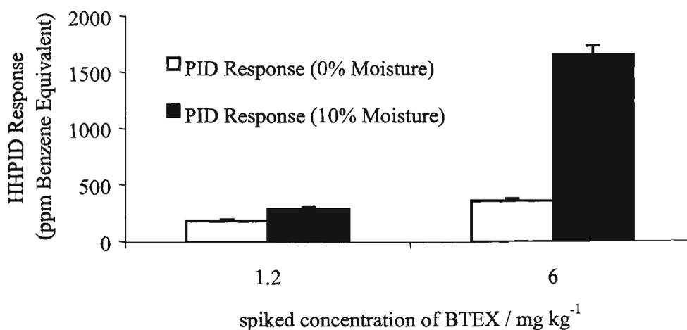
**Figure 2.4:** Comparative HHPID response towards BTEX-spiked silt of different moisture contents.
