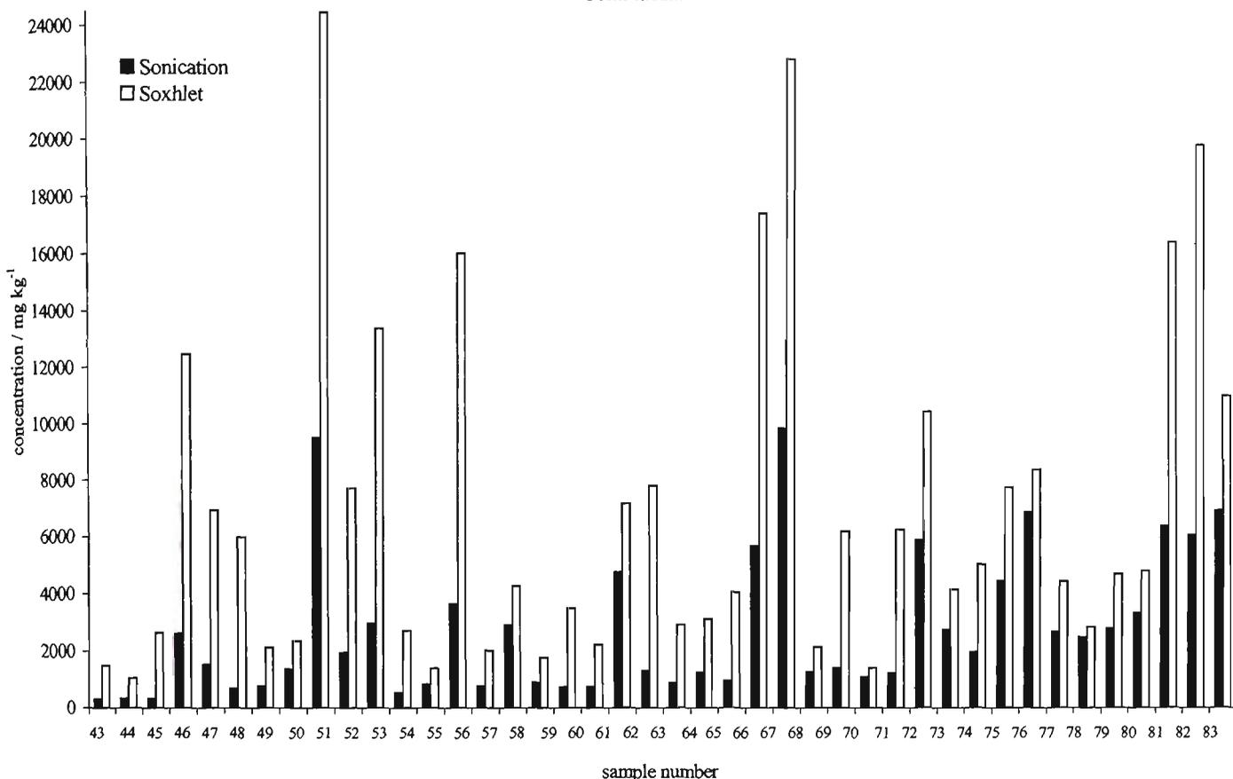
**Figure 4.10b:** Comparison of TPH (C<sub>10</sub>–C<sub>36</sub>) concentrations by sonication and Soxhlet.
