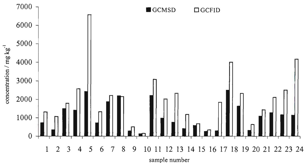
**Figure 6.8:** Comparative TPH (C<sub>10</sub>-C<sub>36</sub>) concentrations using GCFID versus GCMSD.
