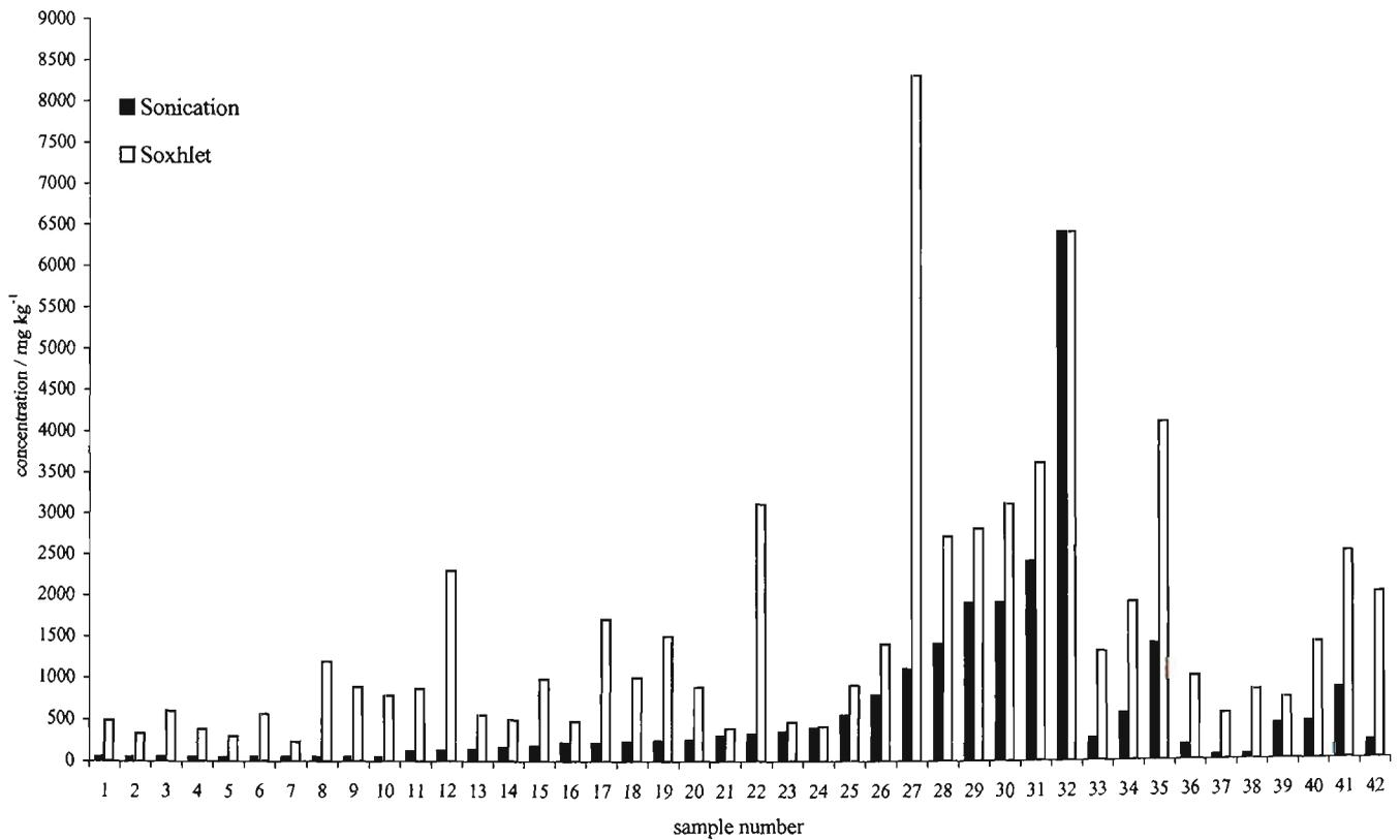
Figure 4.8a: Comparison of TPH (C<sub>15</sub>-C<sub>28</sub>) concentrations by sonication and Soxhlet.
