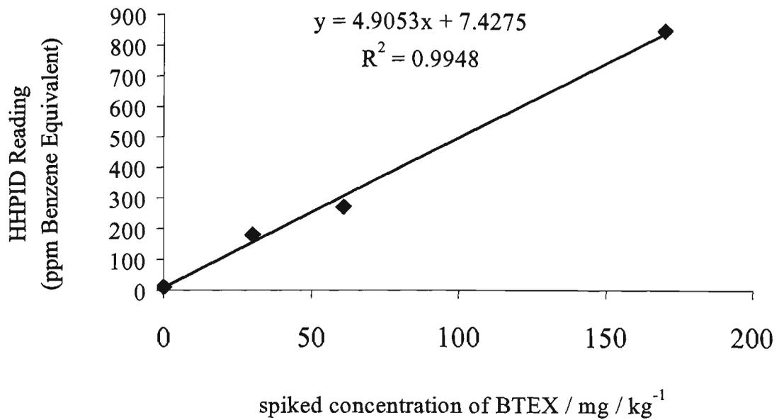
**Figure 2.3:** HHPID Determination of BTEX-spiked Sandy Loam.
