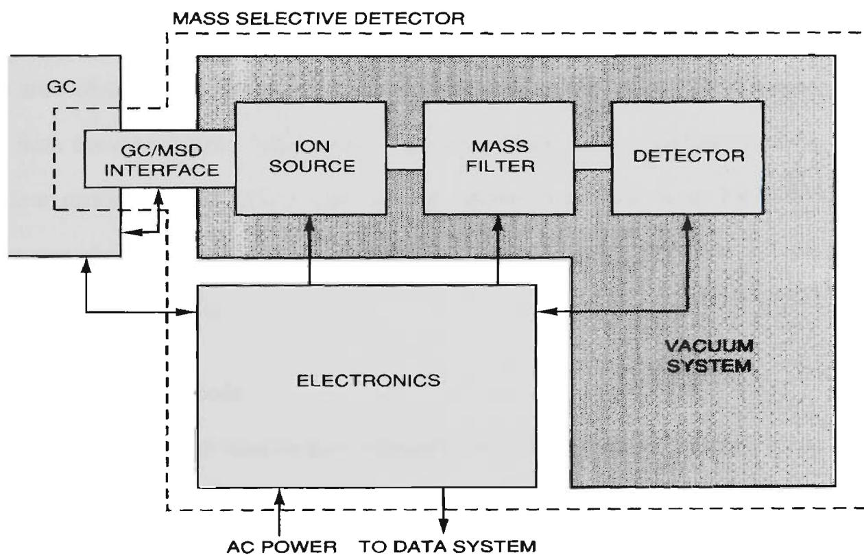
**Figure 6.4:** Components of GCMSD system (by courtesy of Hewlett Packard Australia).
