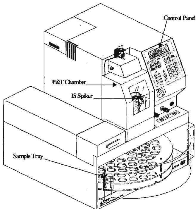
**Figure 7.1:** Example of a purge and trap unit (courtesy of OI Analytical).
