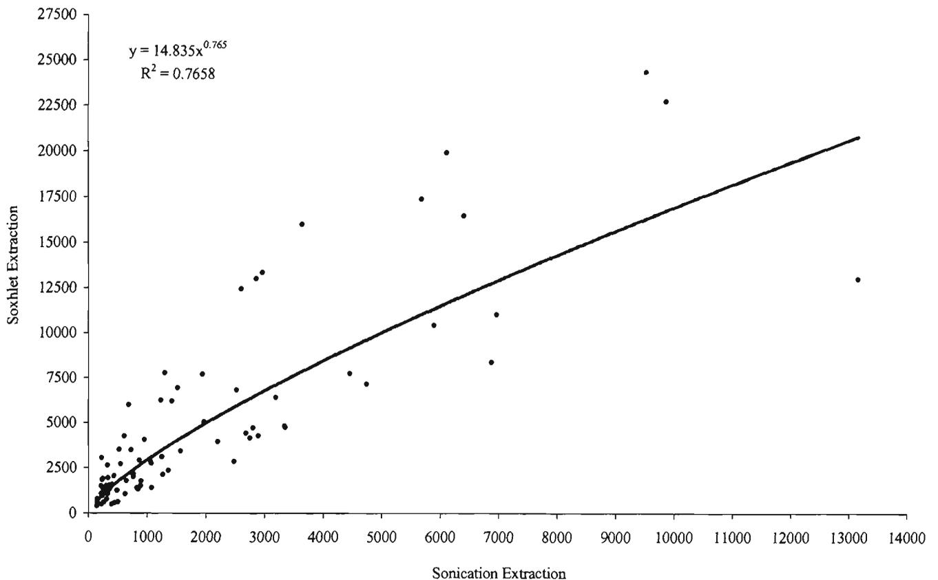
**Figure 4.11:** Scatterplot of TPH ( $C_{10}$ – $C_{36}$ ) concentrations by sonication and Soxhlet extractions.
