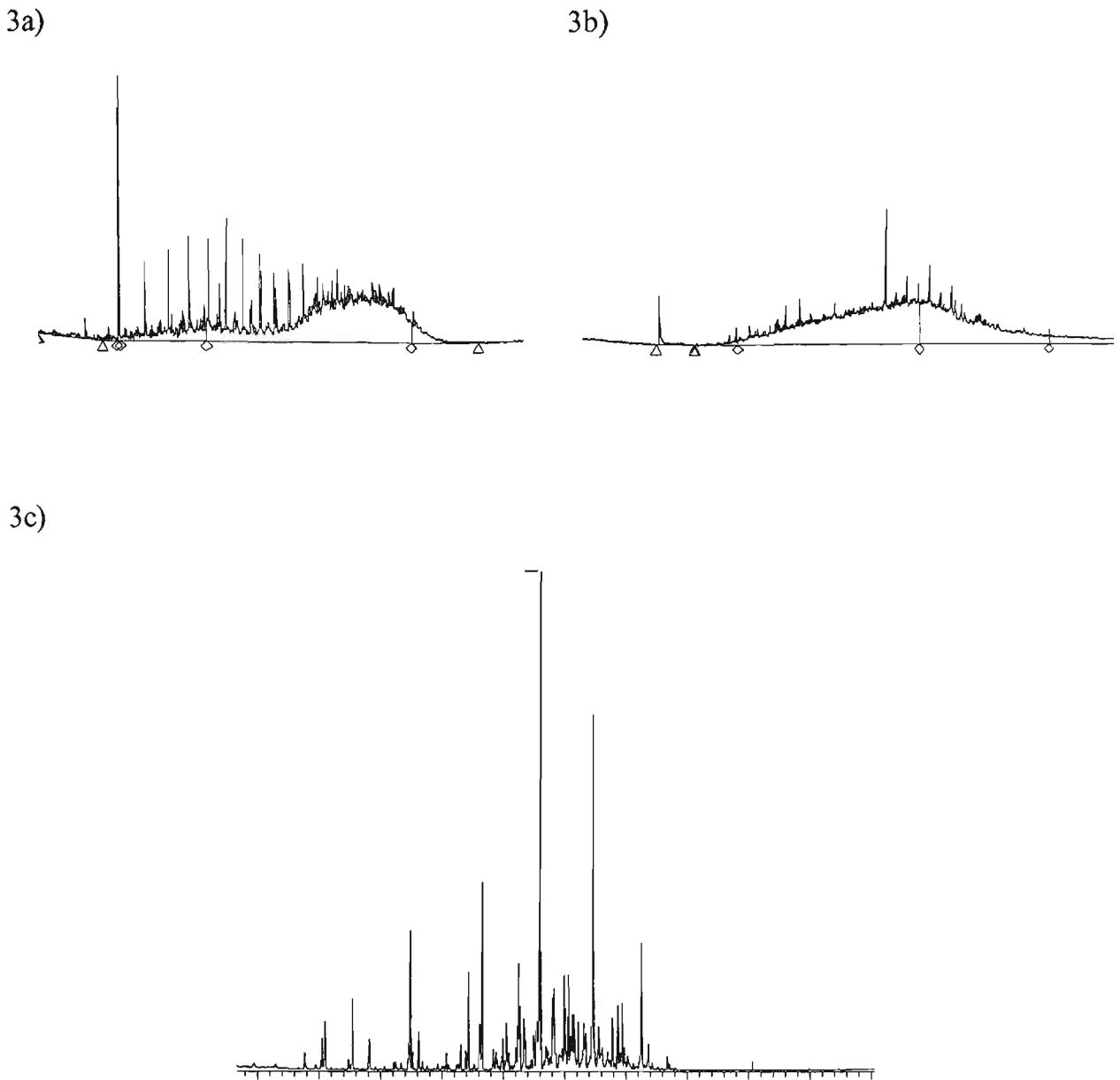
**Figure 4.3 (a-c):** Examples of a typical TPH sample profile at the semi-volatile range.
