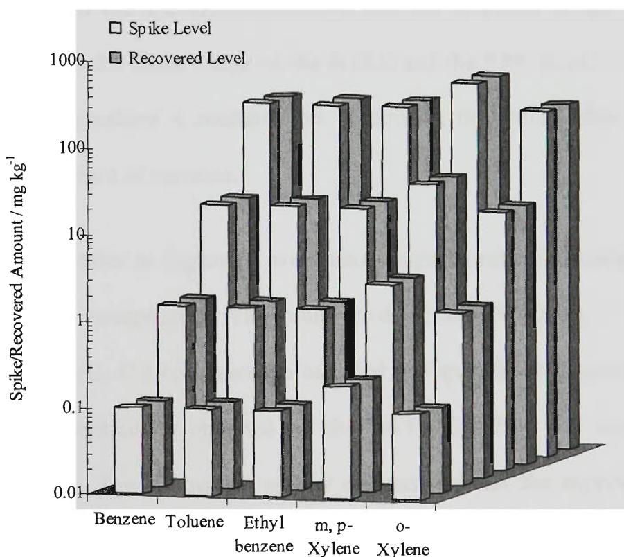
**Figure 8.3:** Comparison of Spiked BTEX concentrations at 0.1, 1.0, 10 and 100 mg/kg, with reference levels. No pair of values was found to be significantly different at the 95% confidence.
