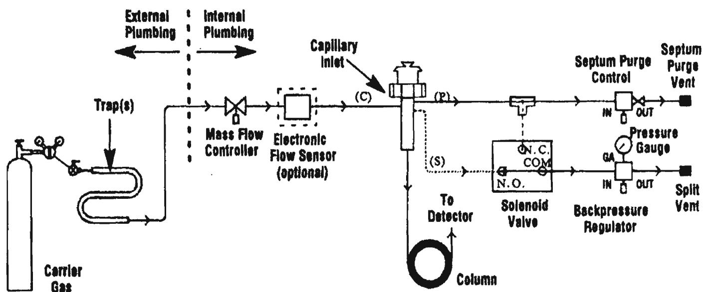
Figure 6.3: Components of a GC system (by courtesy of Hewlett Packard Australia).
