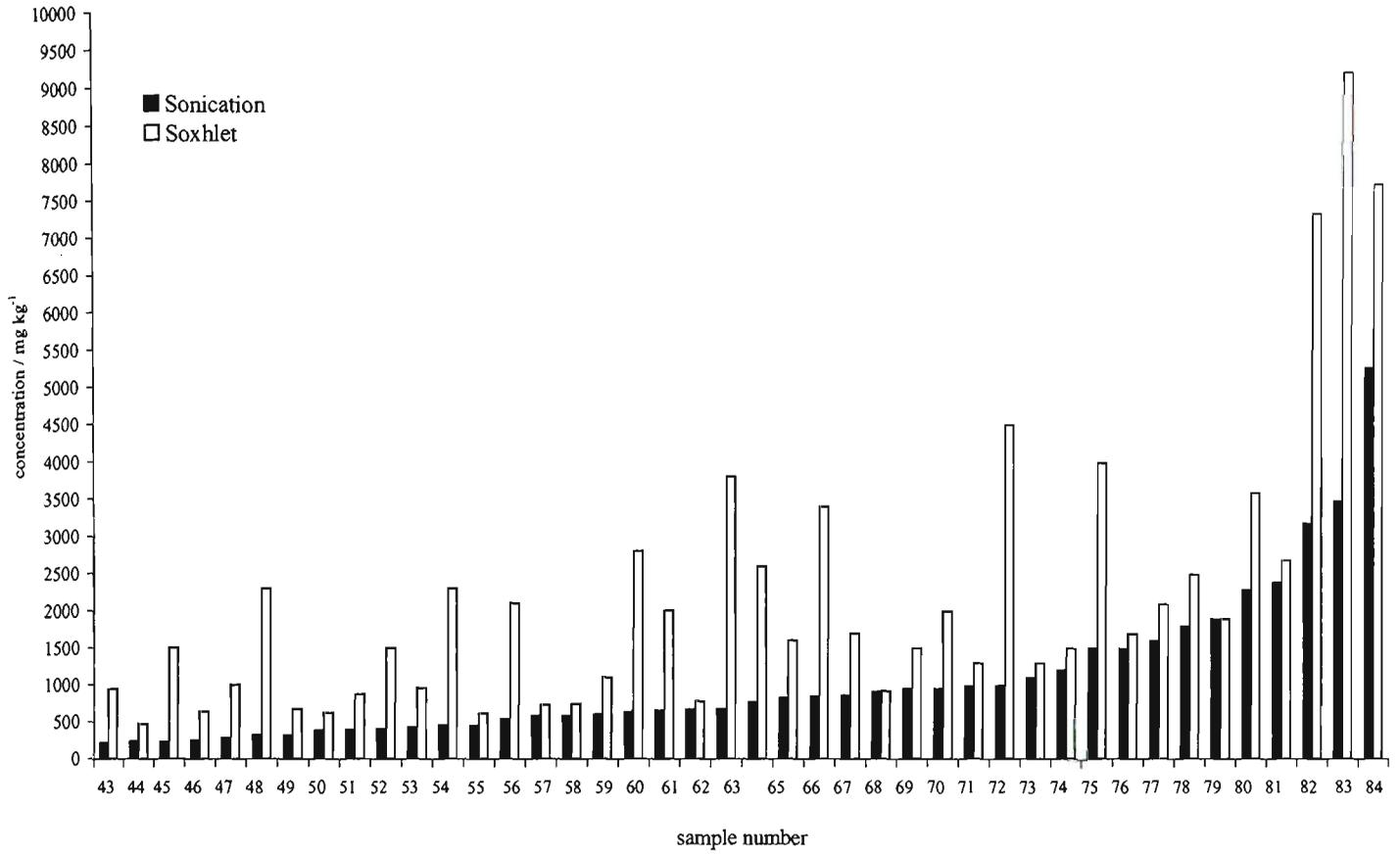
Figure 4.7b: Comparison of TPH (C<sub>10</sub>-C<sub>14</sub>) concentrations by sonication and Soxhlet.
