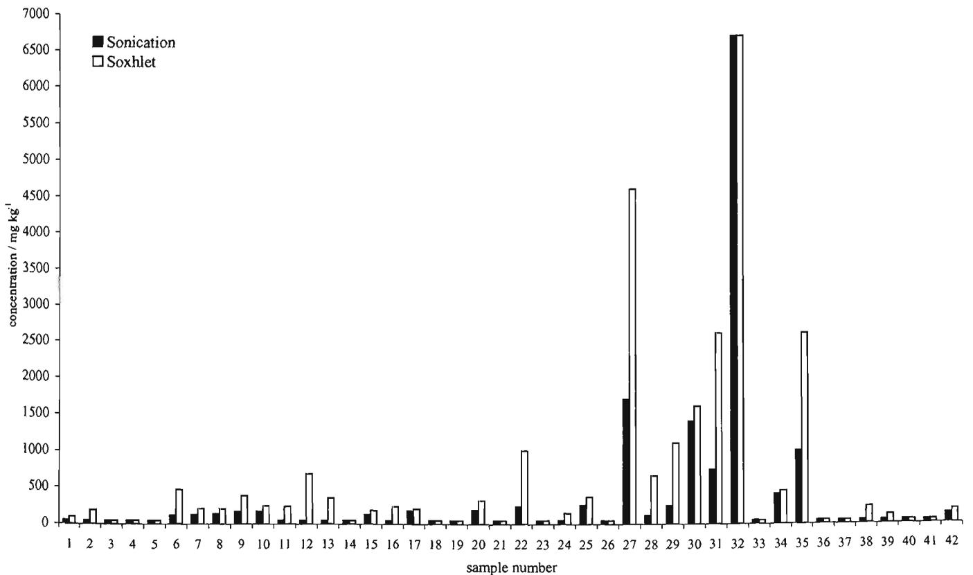
Figure 4.9a: Comparison of TPH (C<sub>29</sub>-C<sub>36</sub>) concentrations by sonication and Soxhlet.
