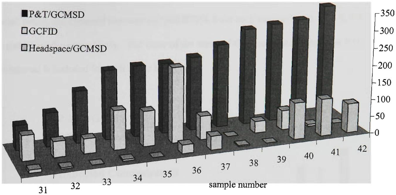
Figure 7.9: BTEX concentrations for sandy soils (higher range).
