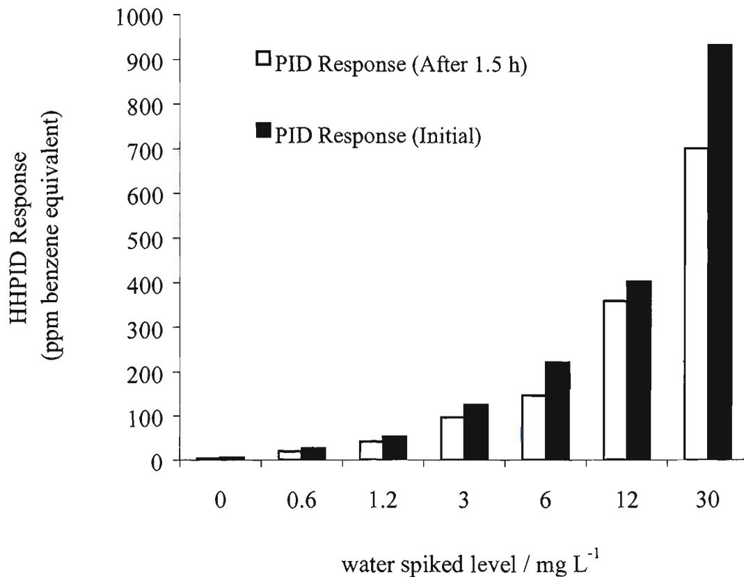
**Figure 2.6:** A comparison between HHPID measurements of BTEX-spiked water samples taken 1.5 h apart.
