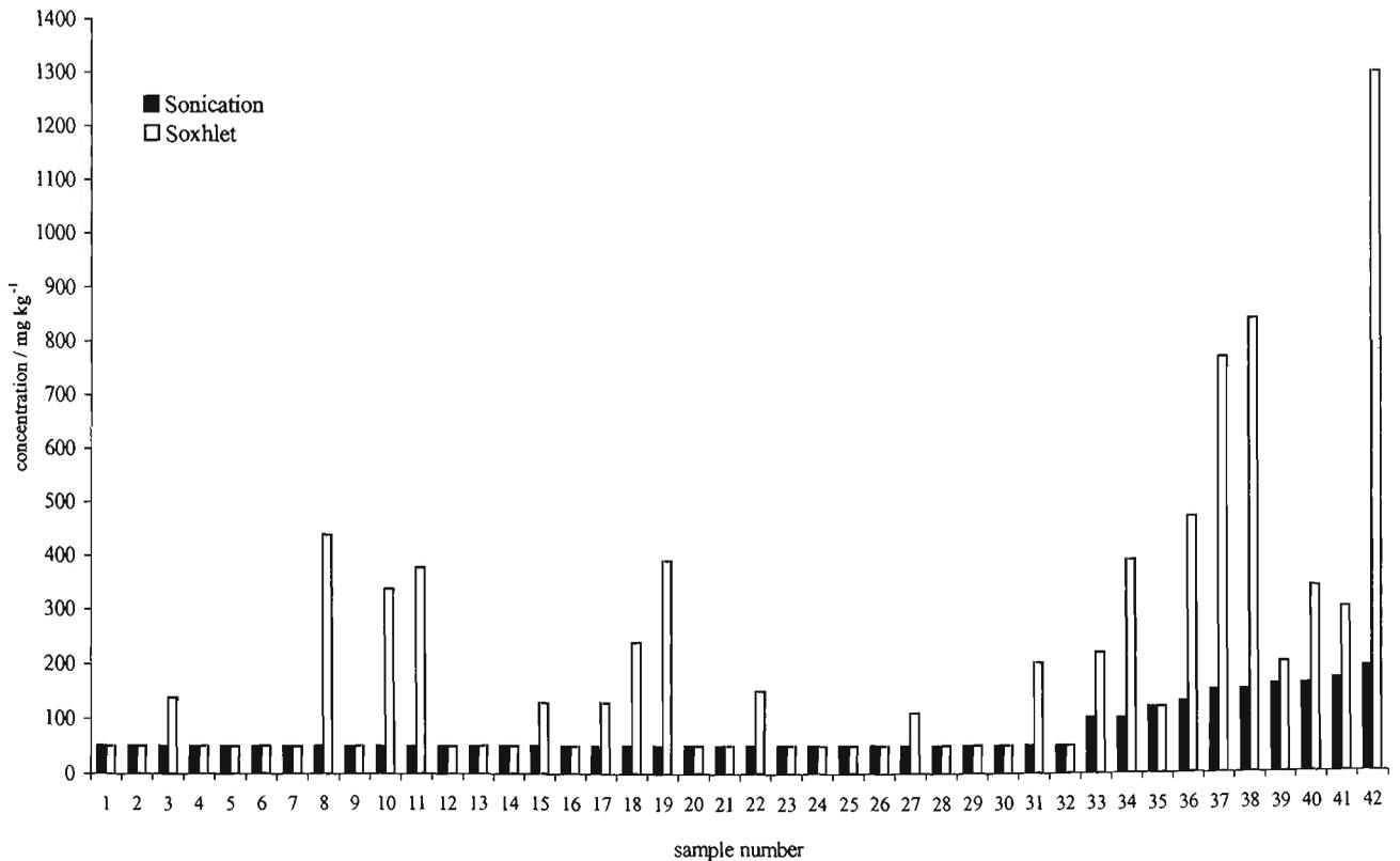
**Figure 4.7a:** Comparison of TPH ( $C_{10}$ - $C_{14}$ ) concentrations by sonication and Soxhlet.
