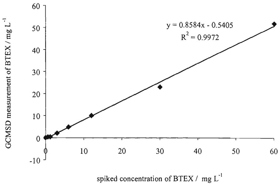
**Figure 2.1:** Headspace/GCMSD determination of BTEX-spiked water samples.
