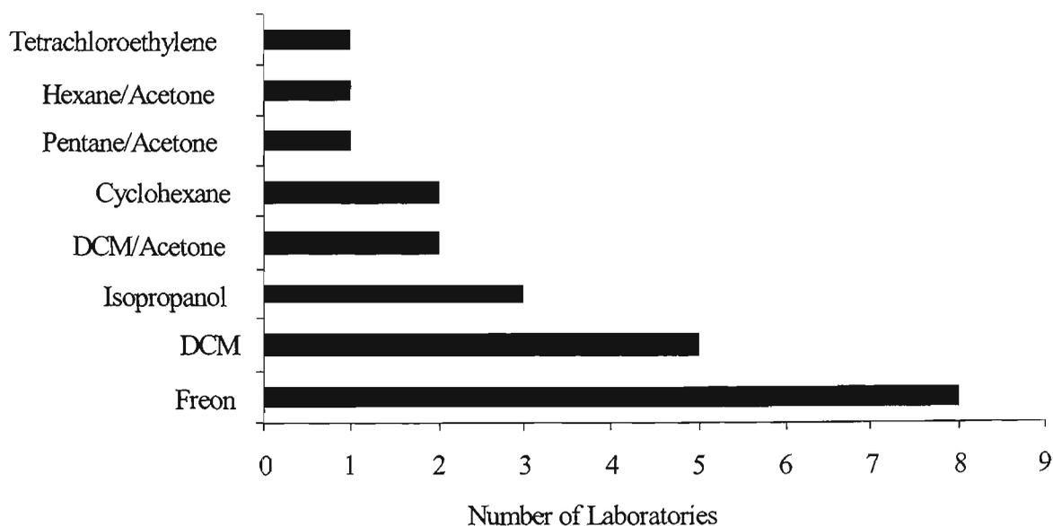
**Figure 3.1:** Solvents used for TPH extractions<sup>7</sup>.
