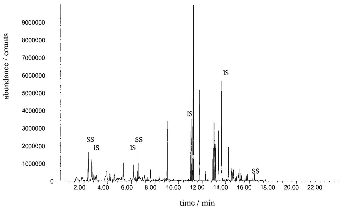
**Figure 6.5:** Typical total ion chromatogram of a representative unleaded petrol sample with the SS/IS.
