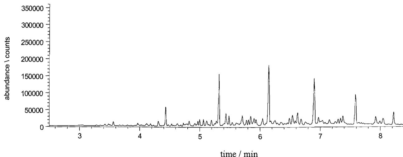
**Figure 3.3:** Sample chromatogram of the above soil extracted by isopropanol.
