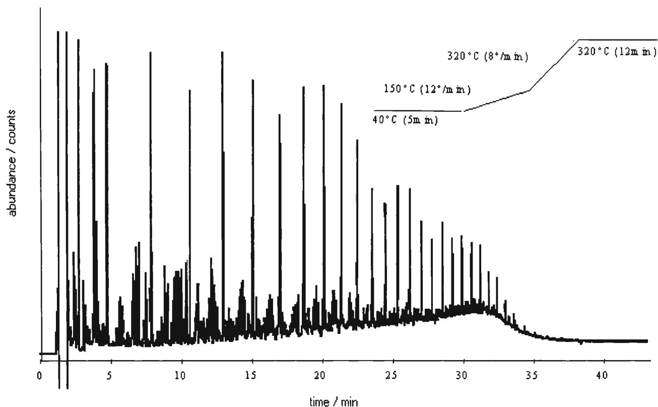
**Figure 1.7:** Example of a crude oil chromatogram with a temperature program (Worrall, 1996)<sup>77</sup>.
