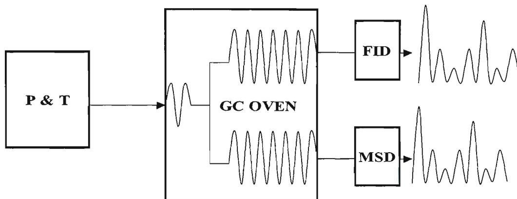
**Figure 6.2:** Instrumental design for diverting samples into the GCFID and the GCMSD.
