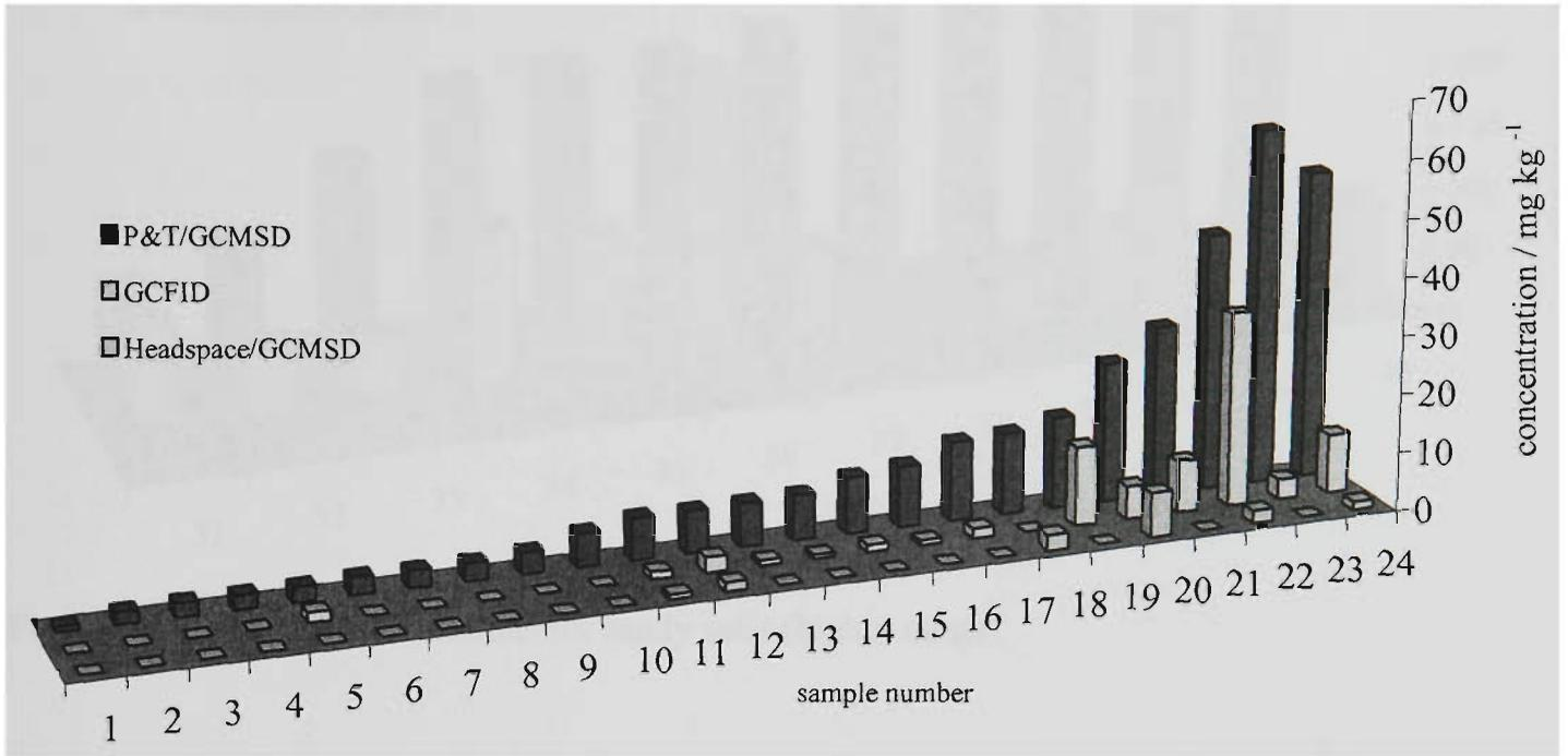
Figure 7.7: BTEX concentrations for sandy soils (lower range).
