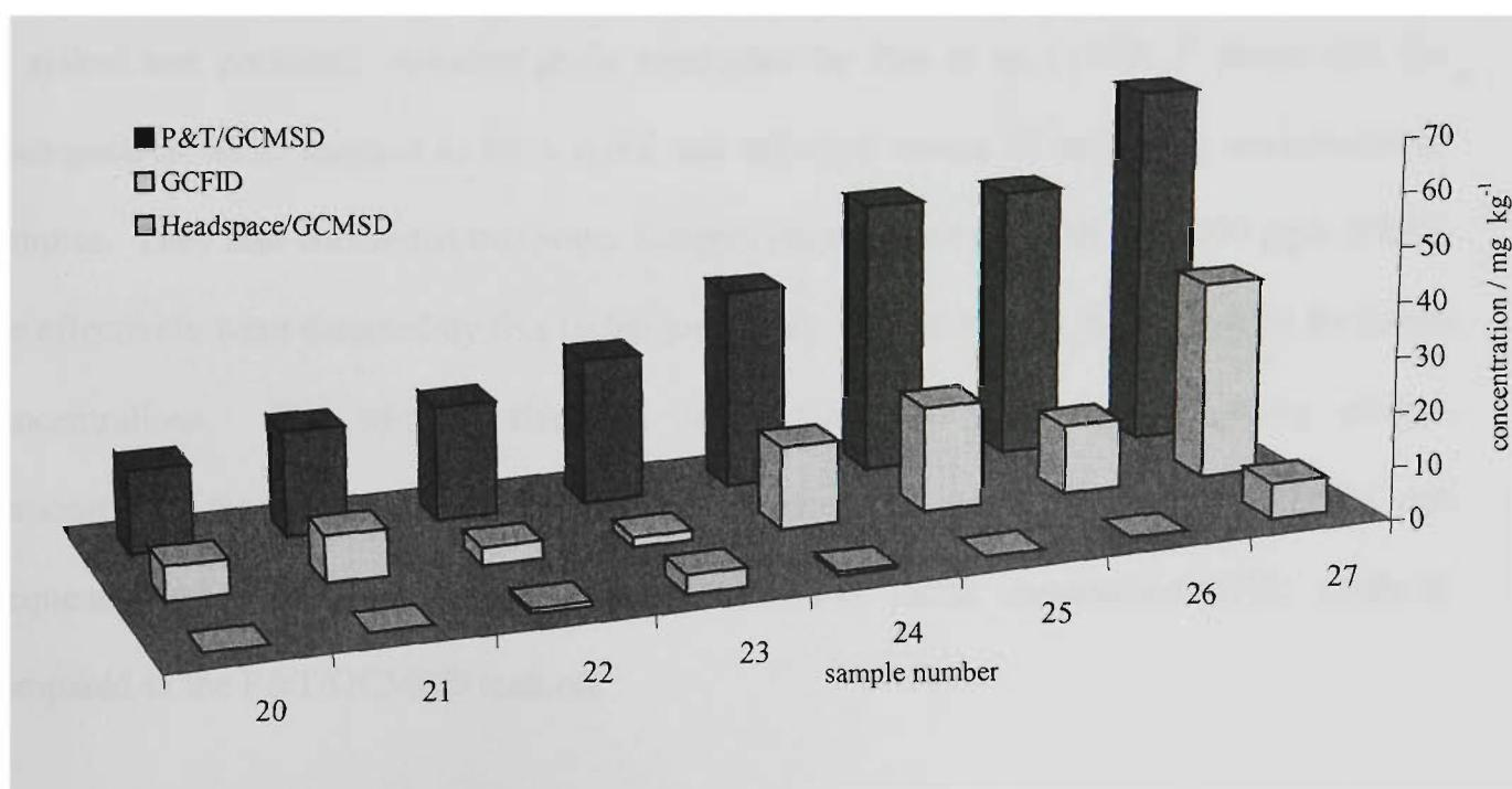
**Figure 7.5:** BTEX concentrations for clay soils (medium range).
