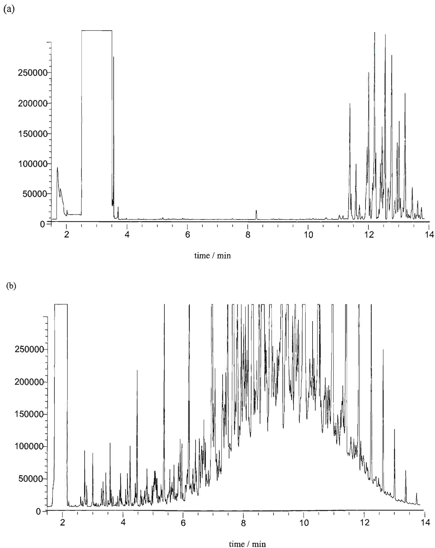
**Figure 6.1:** (a) GCFID profile of Arochlor 1262 (b) GCFID profile of diesel.
