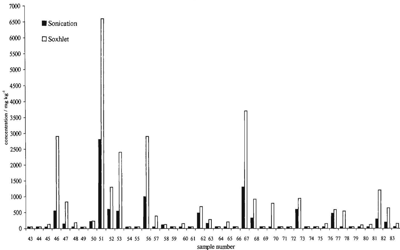
Figure 4.9b: Comparison of TPH (C<sub>29</sub>-C<sub>36</sub>) concentrations by sonication and Soxhlet.
