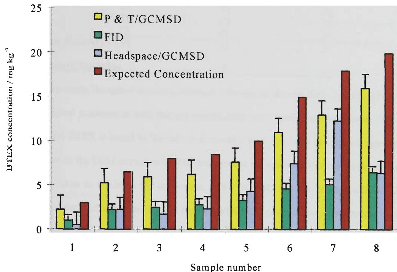
**Figure 7.11:** Recovery of total BTEX by the three methods.
