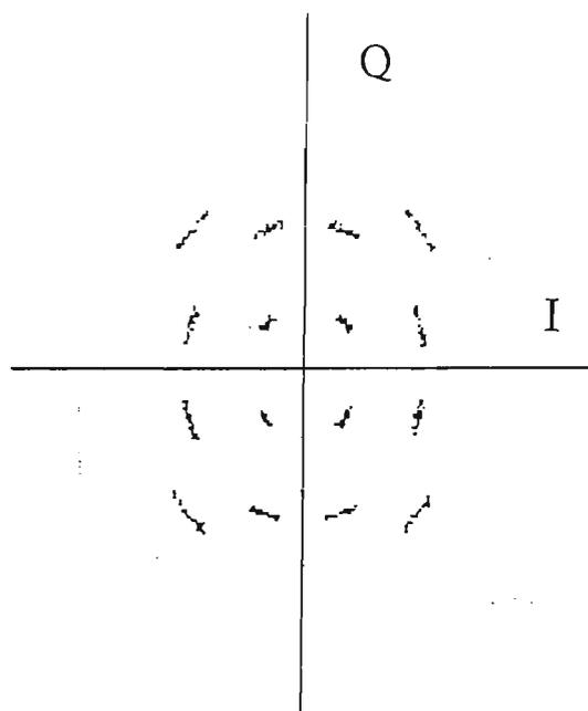
Figure 6.3.1.4 Signal constellation - sinusoidal phase jitter. 14 degree peak to peak - frequency 50 Hz.
