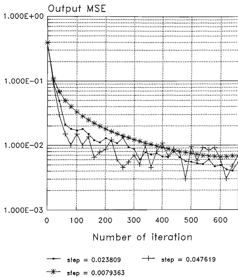
Figure 6.4.3.2 Initial convergence characteristic of the LMS algorithm with different step size for the given channel - normalised output MSE
