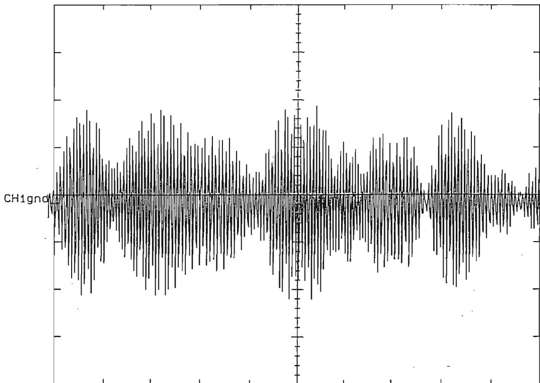
Figure 5.6.2.5 Signal after the summer - modulator side
