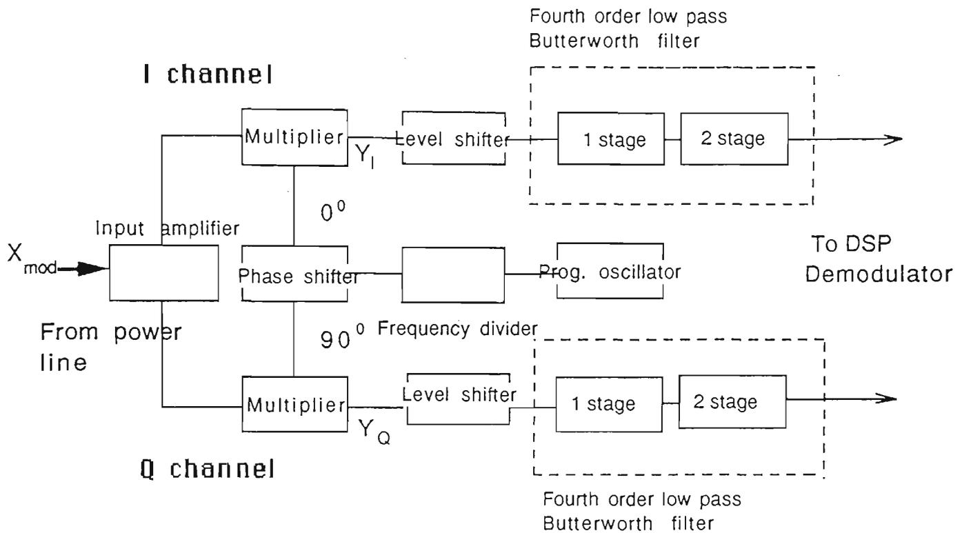
Figure 5.4.3.1 Block diagram - analog section of the demodulator
