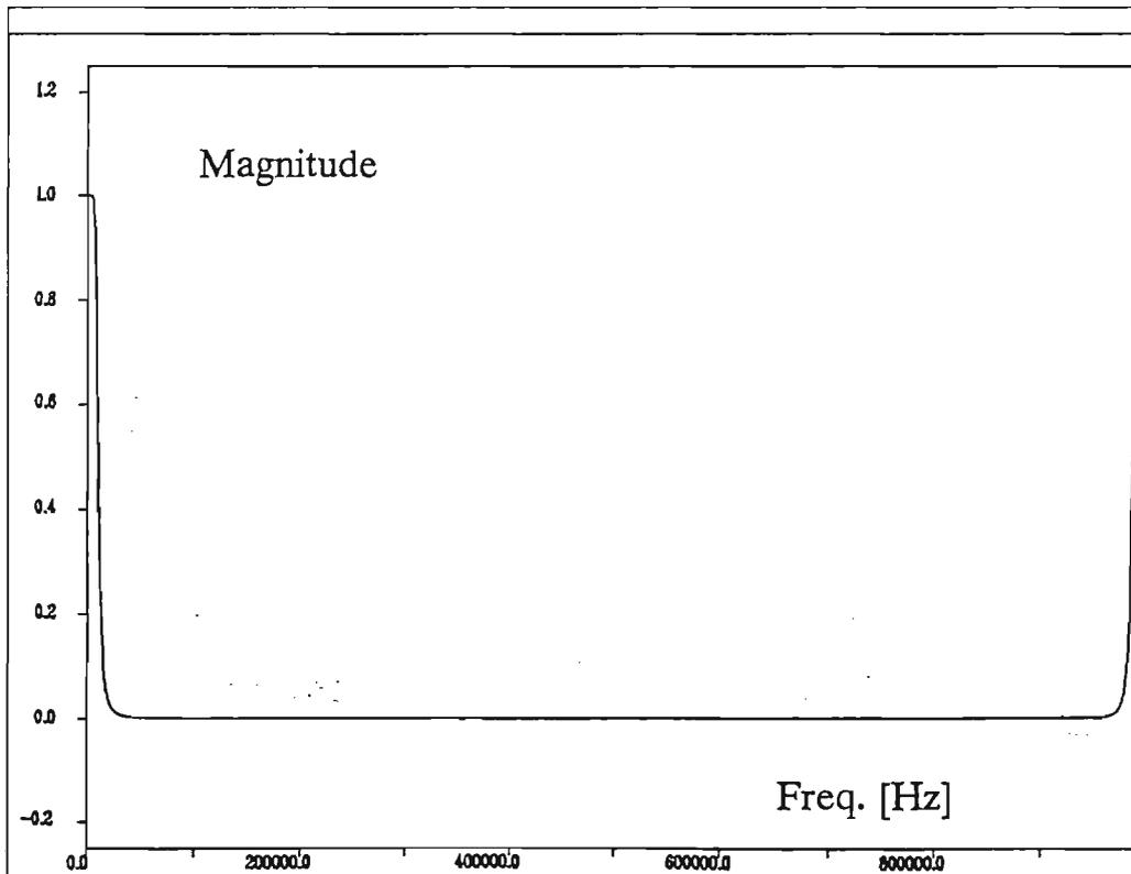
Figure 4.4.2.6 Concatenation - filter frequency response (magnitude) -  $|\tilde{A}_k|$
