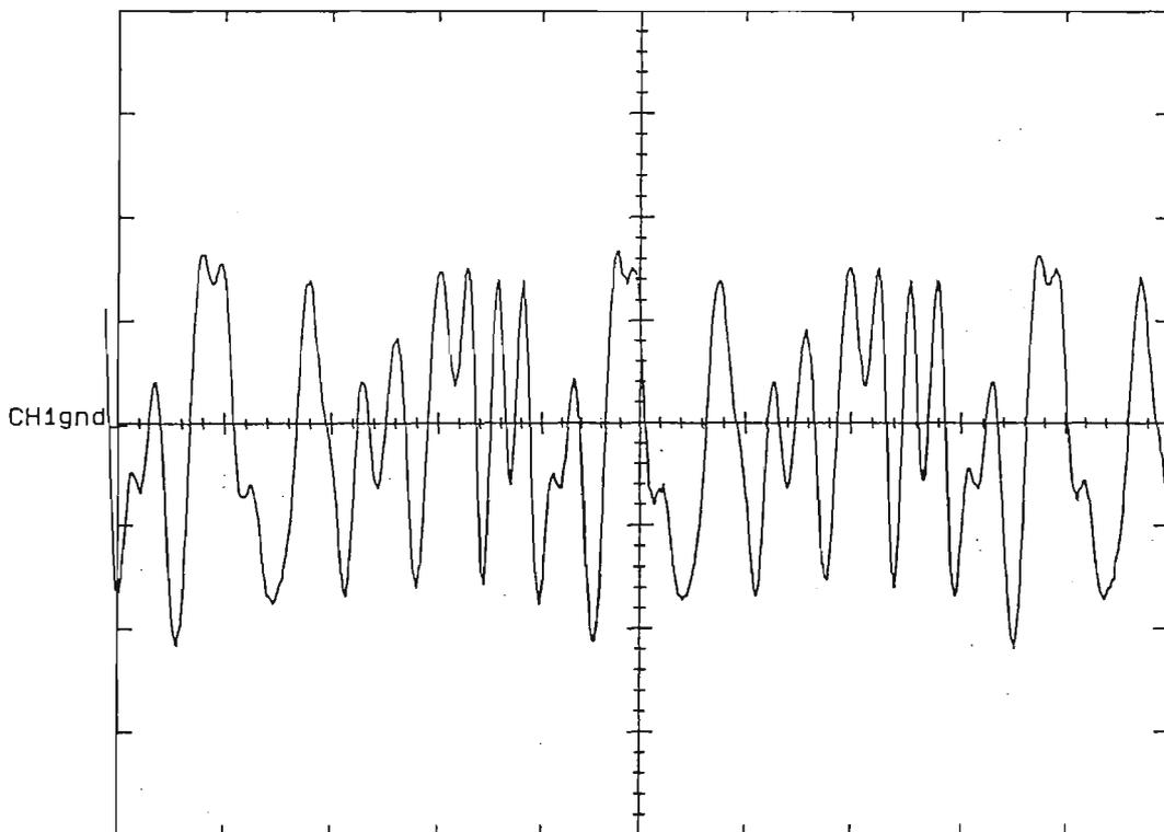
Figure 5.6.2.3 I signal after the low pass (smoothing) filter
