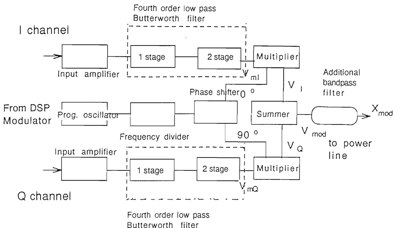
Figure 5.6.1.1 Block diagram - analog section of the modulator
