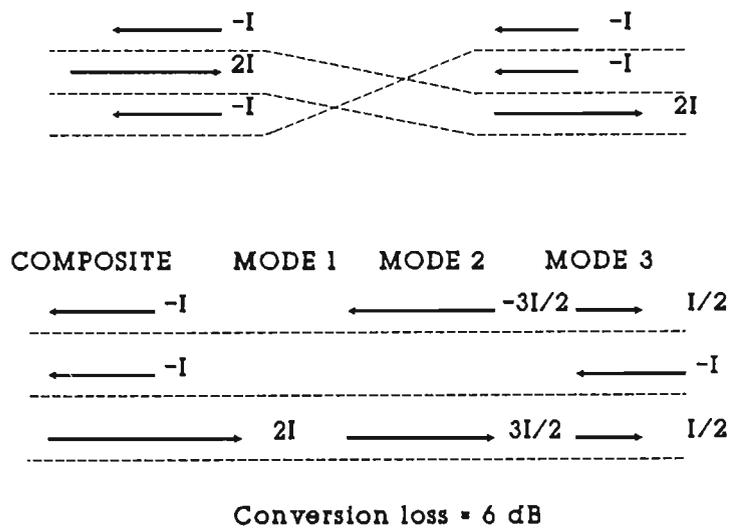
Figure 3.5.4 Transposition losses
