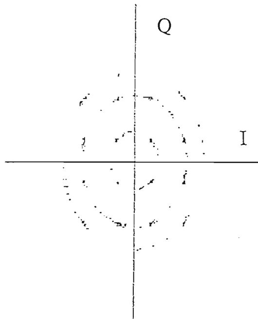
Figure 6.3.2.2 Signal constellation with frequency offset 250 Hz,
