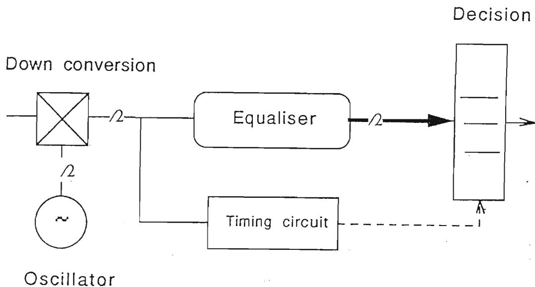
Figure 4.4.1.1 Receiver - simplified block diagram
