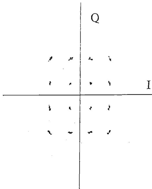
Figure 6.3.1.6 Signal constellation - sinusoidal phase jitter. 14 degree peak to peak
