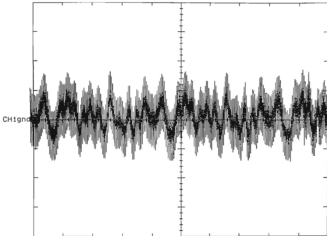
Figure 5.6.2.5 I signal after the multiplier demodulator side
