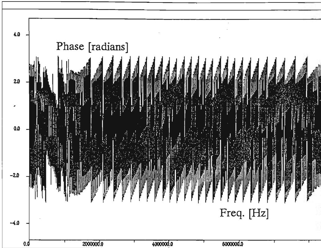
Figure 4.4.2.5 - Circularly shifted - phase response  $\tilde{\theta}_{(k+75\text{KHz})\text{mod } 1000\text{KHz}}$
