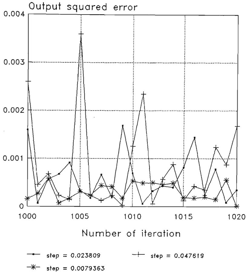
Figure 6.4.3.3 Residual squared error of the LMS algorithm with different step size-normalised output squared error
