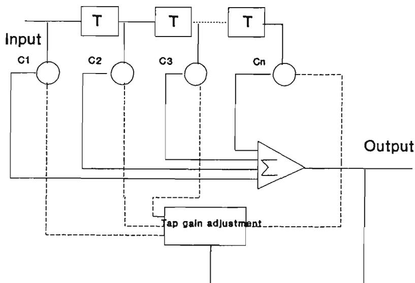
Figure 6.4.1.1 Linear transversal equaliser
