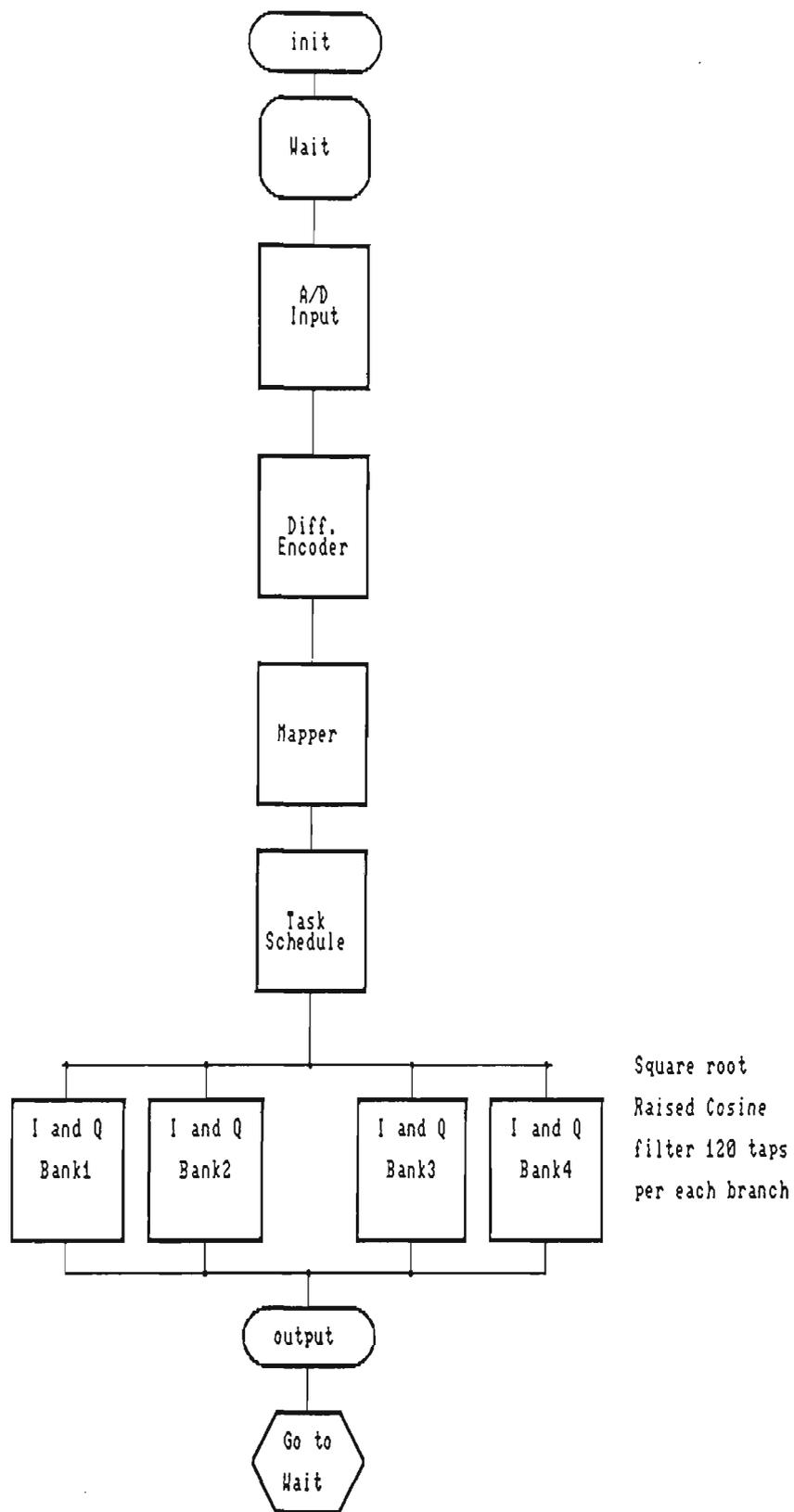
Figure 5.3.4.1 TMS 320C25 assembler modulator program
