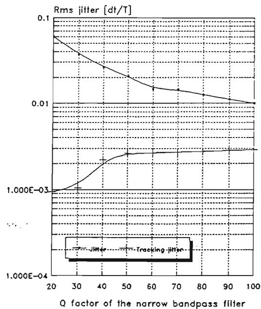
Figure 6.2.4.8 Jitter variance versus Q factor
