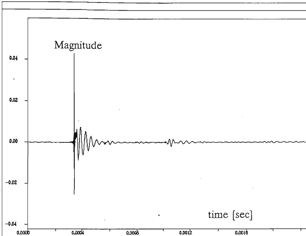
Figure 4.4.2.3 Channel impulse response
