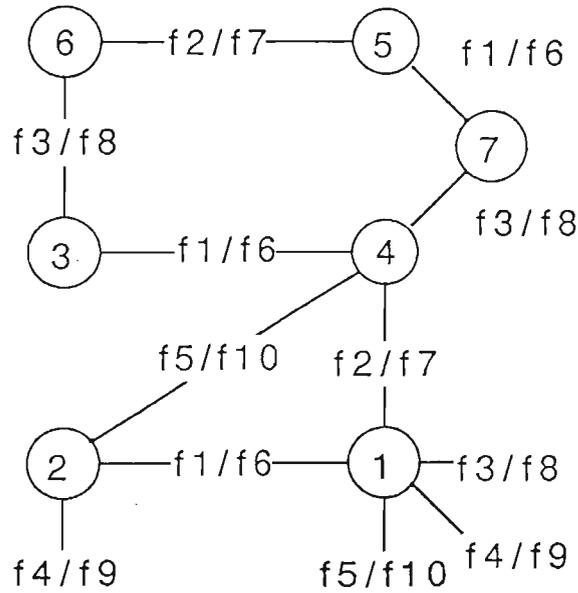
Figure 3.6.3 Grid network - spectrum allocation for analog SSB system
