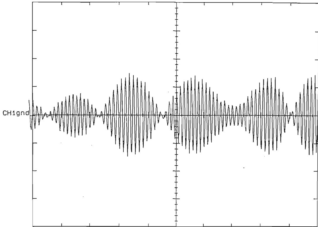
Figure 5.6.2.4 I signal multiplied with the carrier of 75 KHz - modulator side
