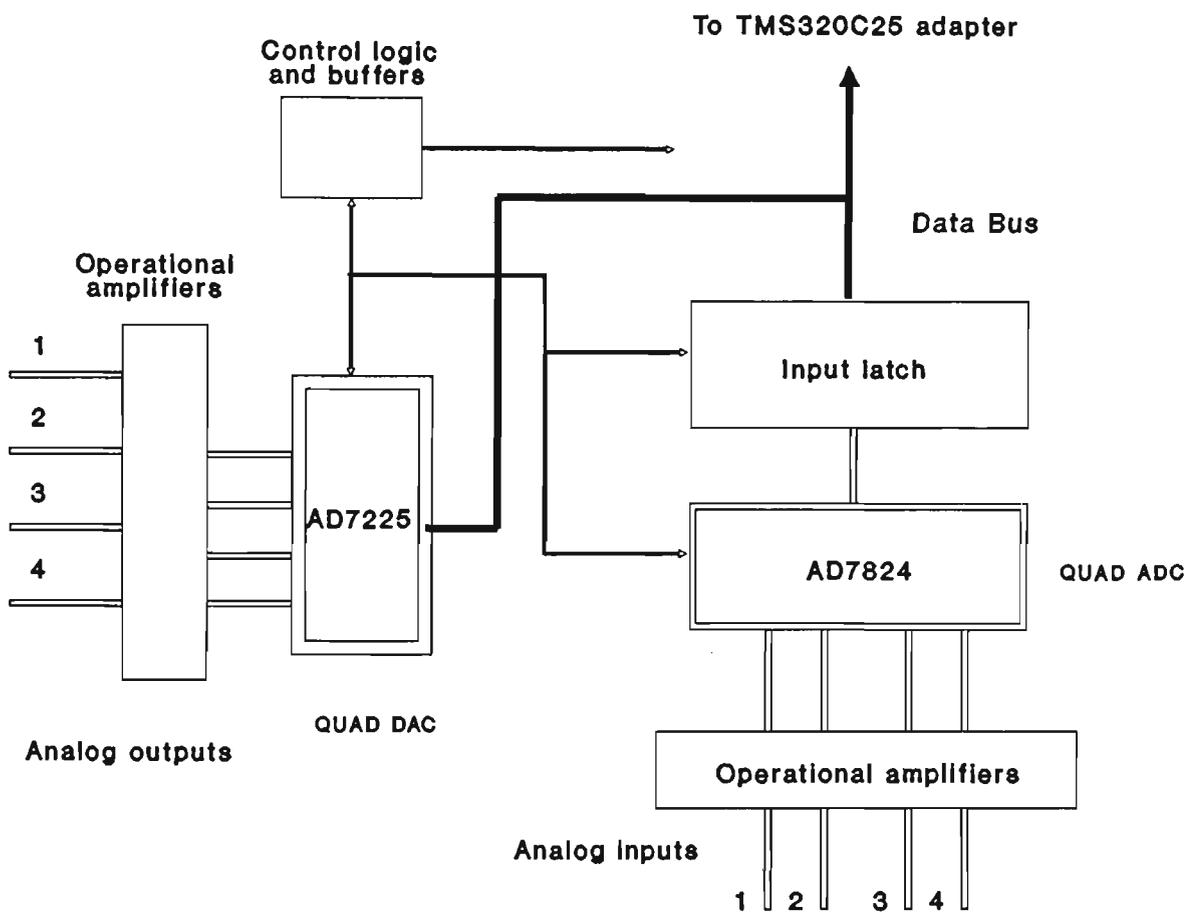
Figure 6.1.1 DSP TMS 320C25 target system - block diagram
