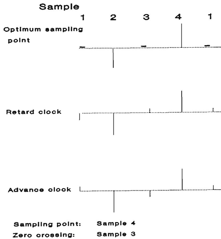
Figure 6.2.2.4 Optimal sampling point
