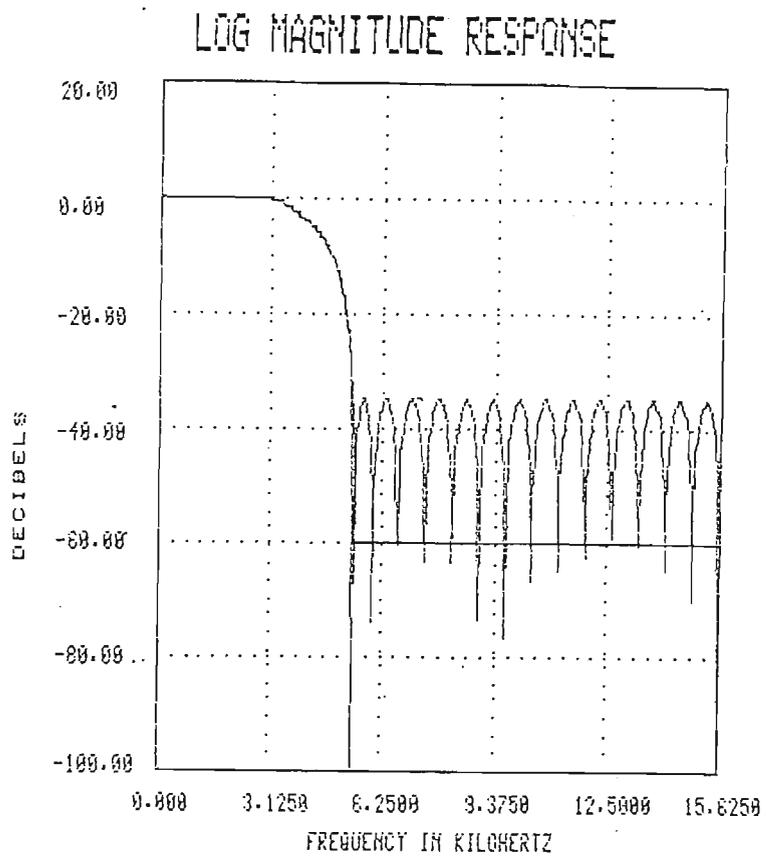
Figure 6.1.1.3 Square root raised cosine filter
