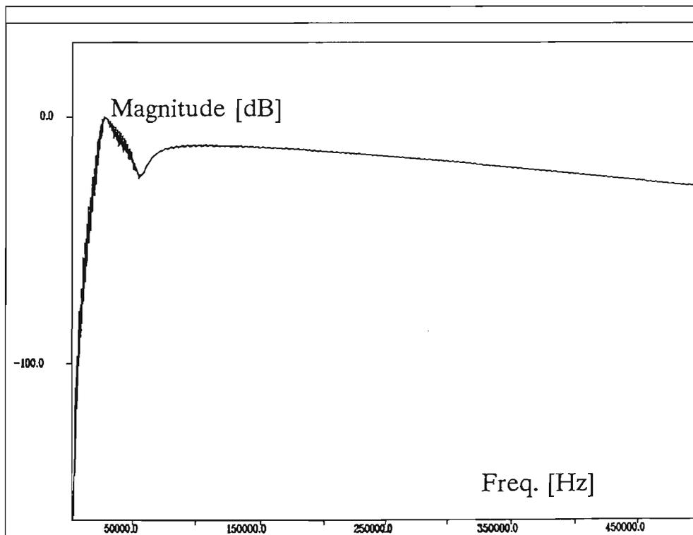
Figure 4.3.4 Channel frequency response (log magnitude),  $R_k$ , obtained from simulation model
