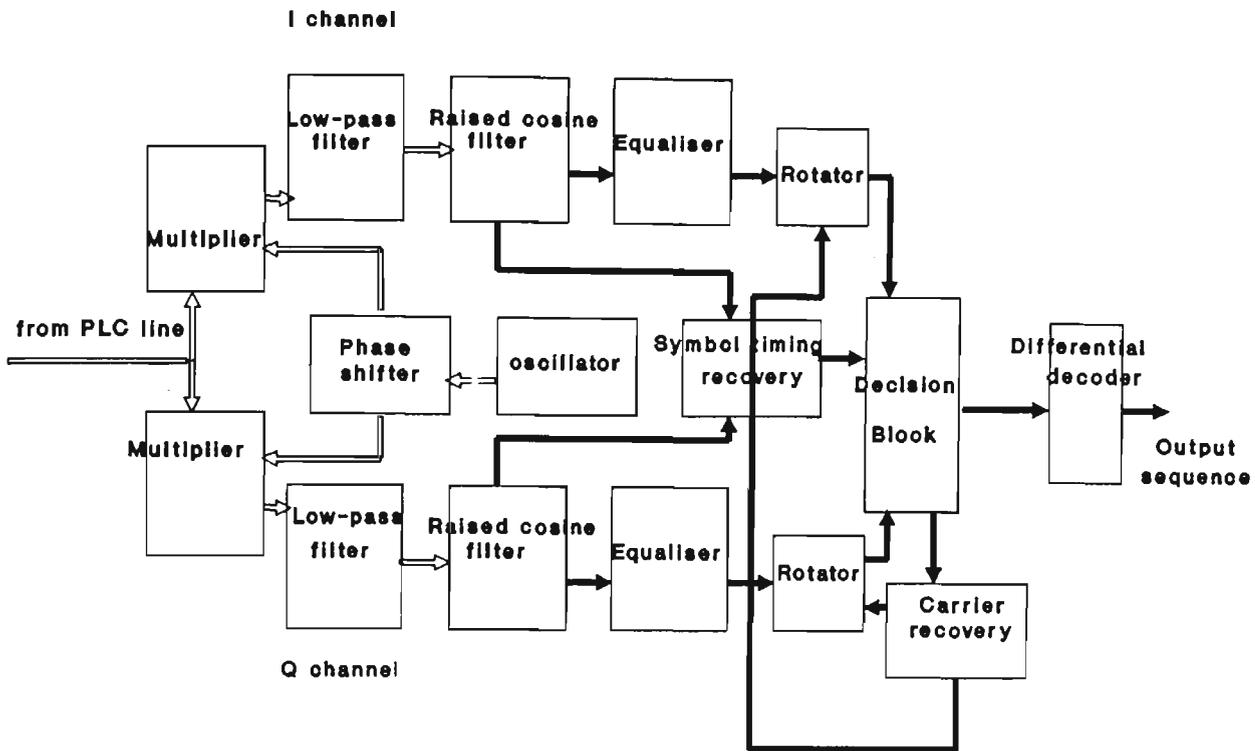
Figure 5.1.3 Demodulator block diagram
