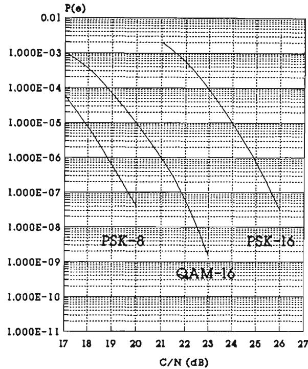
Figure 4.1.2 BER performance of QAM-16 for double-sided Nyquist bandwidth
