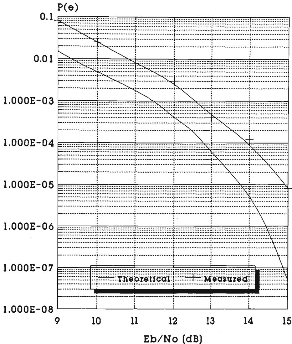
Figure 7.2.3 BER performance for QAM-16. Theoretical and measured curves
