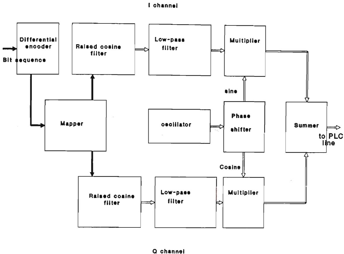
Figure 5.1.2 Modulator block diagram
