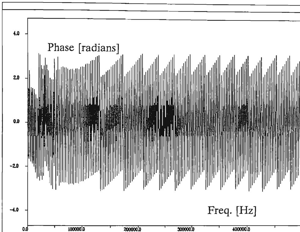
Figure 4.3.5 Channel frequency response (phase),  $\theta_k$  obtained from simulation model
