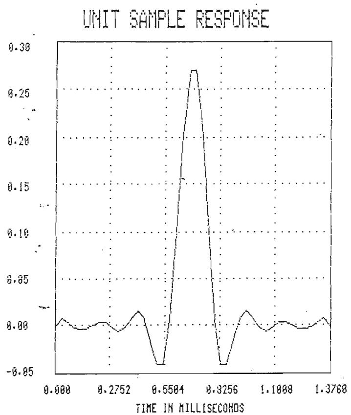
Figure 6.1.1.4 Square root raised cosine filter
