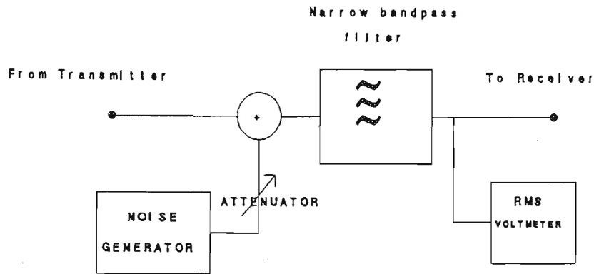
Figure 7.2.1 Setup for performance measurement
