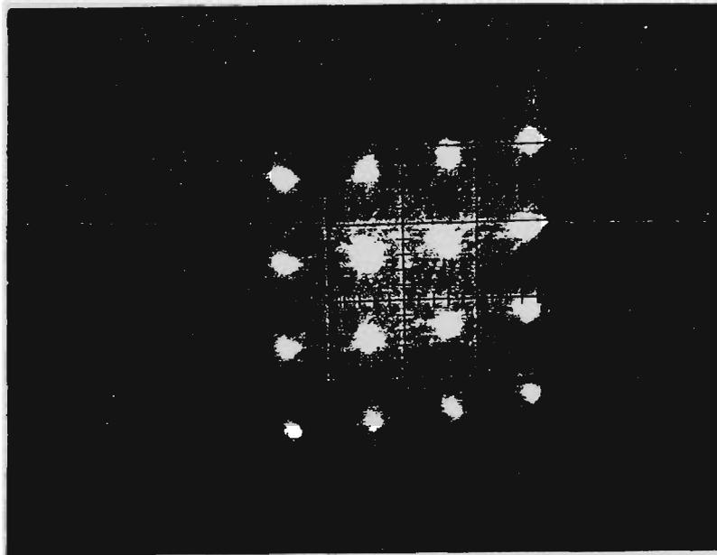
Figure 6.4.4.2 Signal constellation before equalisation
