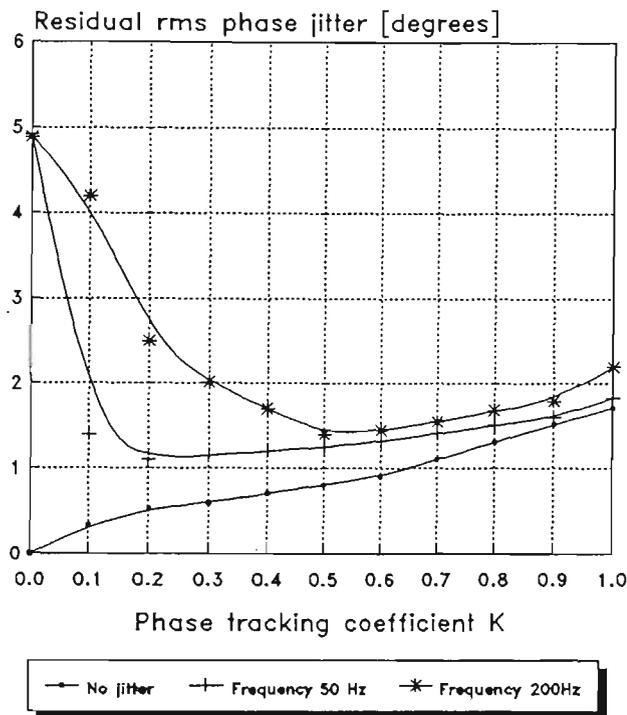
Figure 6.3.1.2 Residual rms phase jitter for channel with S/N = 20 dB
