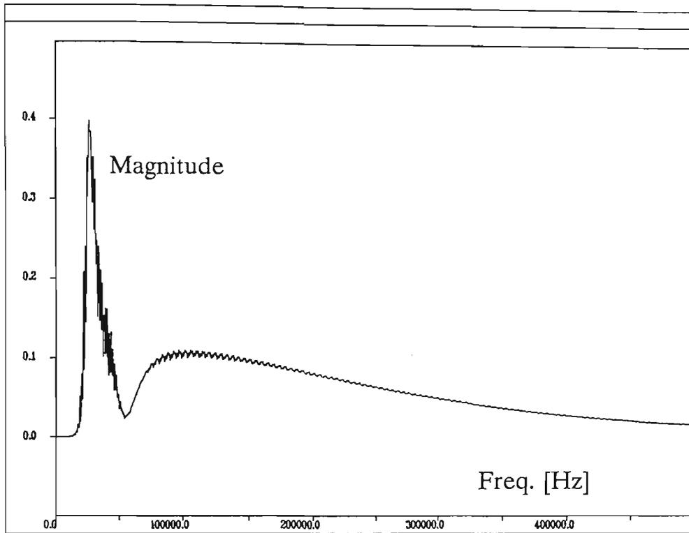
Figure 4.3.3 Channel frequency response (magnitude),  $R_k$ , obtained from simulation model
