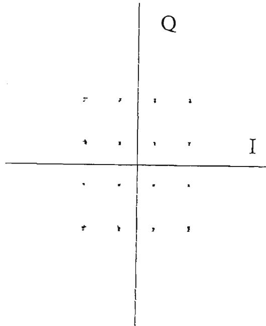
Figure 6.3.1.7 Signal constellation - sinusoidal phase jitter. 14 degree peak to peak - frequency 50 Hz. Receiver  $K = 1$
