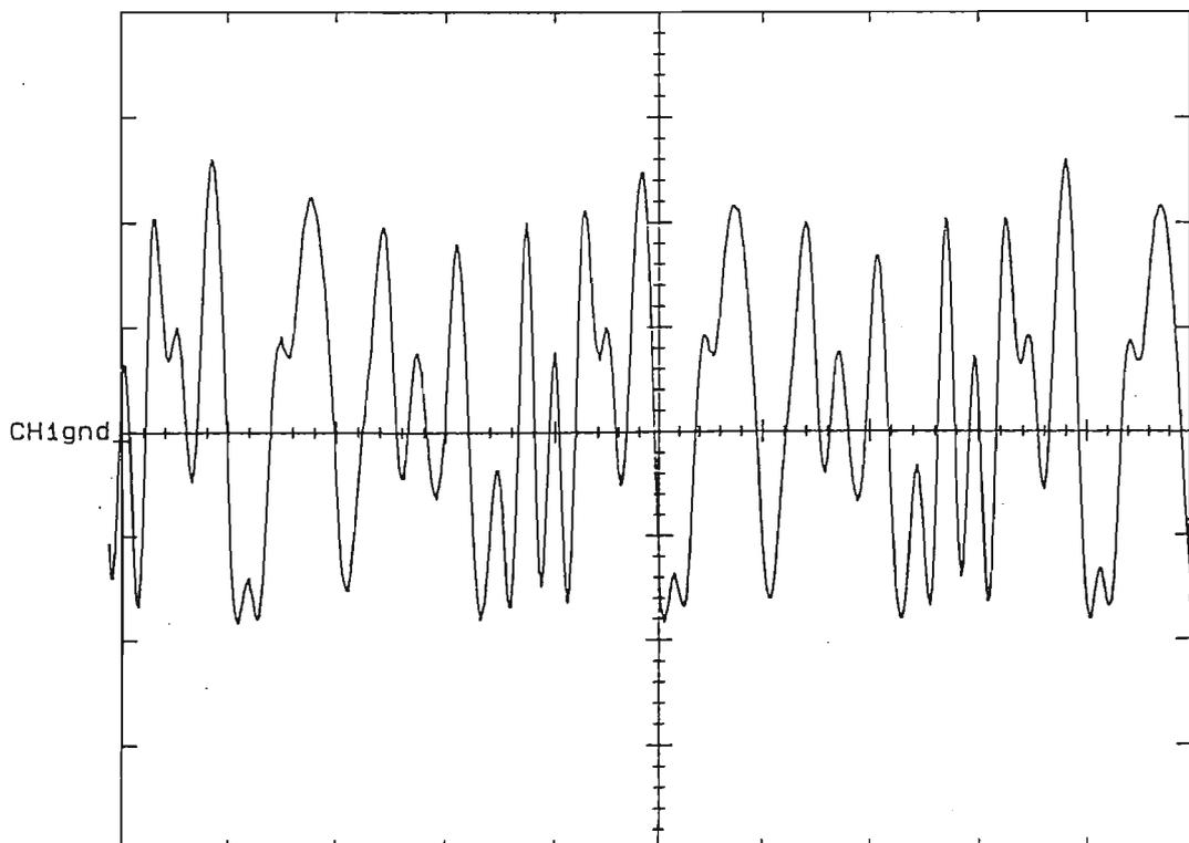
Figure 5.4.3.6 I signal after the low pass filter - demodulator side
