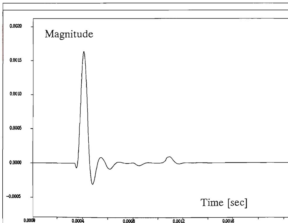
Figure 4.4.2.8 Baseband impulse response of bandlimited system -  $h_n$  (narrow band) - imaginary part
