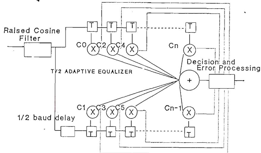
Figure 6.4.3.1 Fractional spaced equaliser
