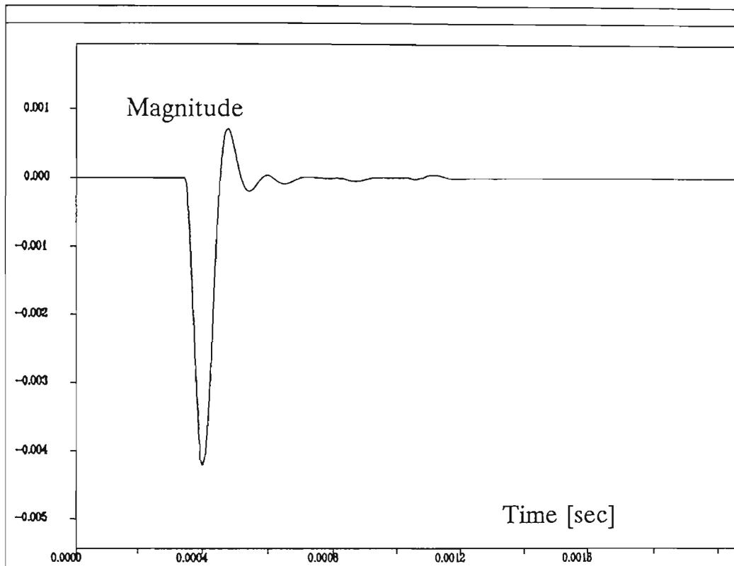
Figure 4.4.2.7 Baseband impulse response of bandlimited system -  $h_n$  (narrow band) - real part
