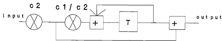
Figure 6.3.3.2. PLL filter configuration
