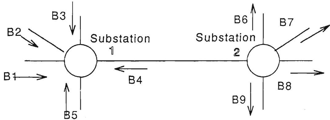
Figure 4.1.1 Interference analysis. Arrows indicate channels using the same frequency. The wanted signal is B4. The others are possible cochannel interferers
