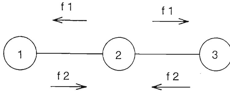
Figure 4.1.3 Cascaded full duplex structure - Dig. modulation
