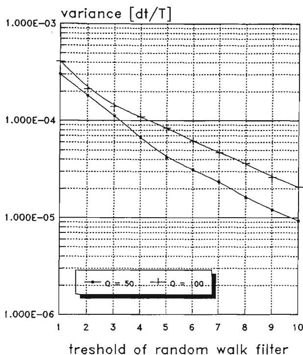
Figure 6.2.4.10 Jitter variance versus threshold
