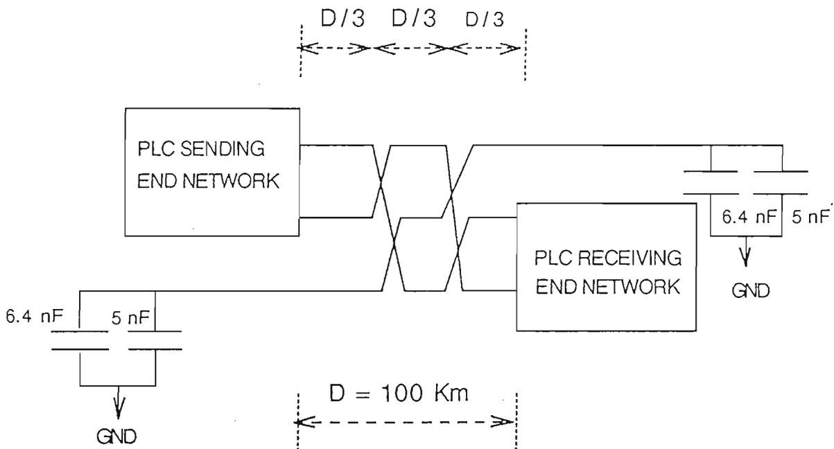
Figure 4.3.2 Line transposition and coupling
