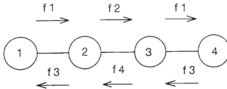
Figure 3.6.2 Cascaded full duplex structure for analog SSB modulation
