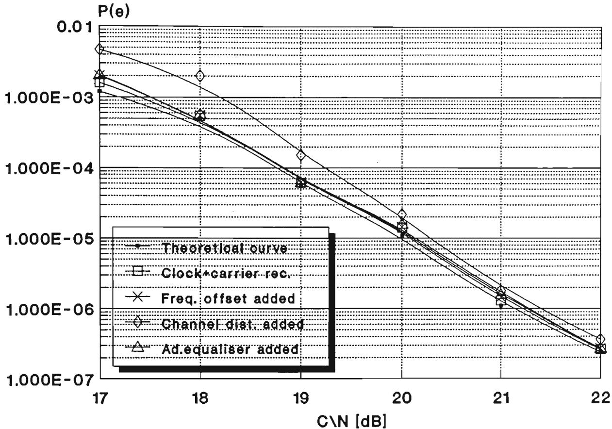
Figure 7.2.2  $P(e)$  performance of QAM-16. The rms C/N specified in double-sided Nyquist bandwidth
