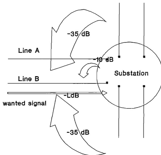
Figure 3.6.1 PLC interference sources into the receiver on the line B
