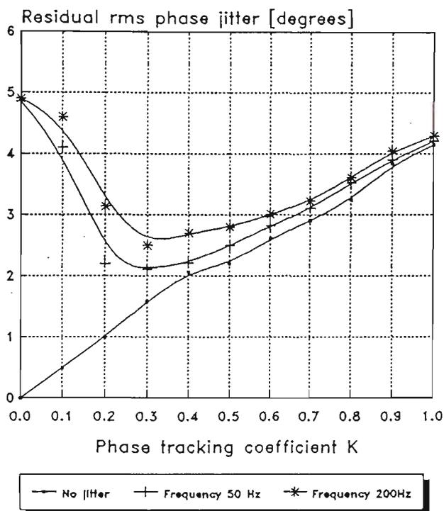
Figure 6.3.1,3 Residual rms phase jitter for the channel with  $S/N = 30$  dB
