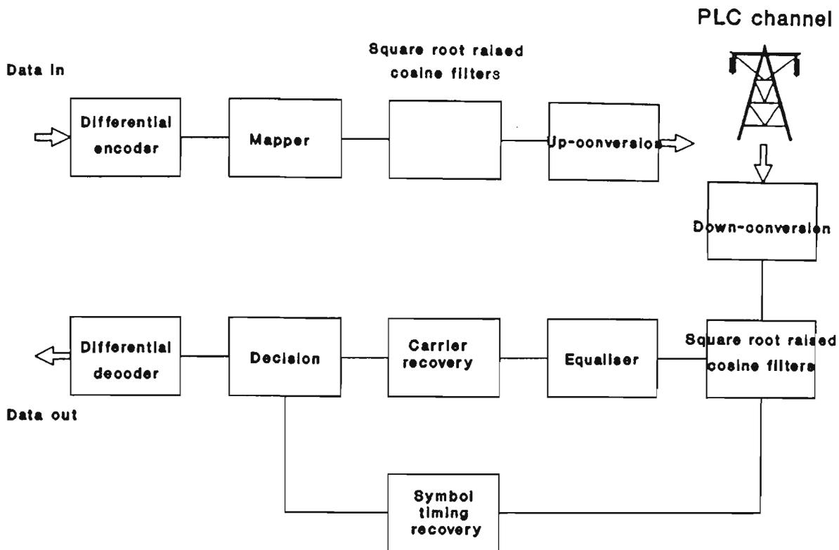
Figure 5.1.1 Modem block diagram
