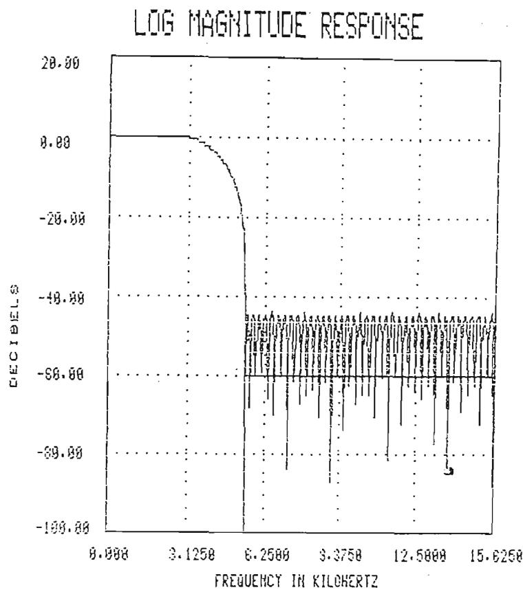
Figure 5.3.4 Log. magnitude response of square root raised cosine filter
