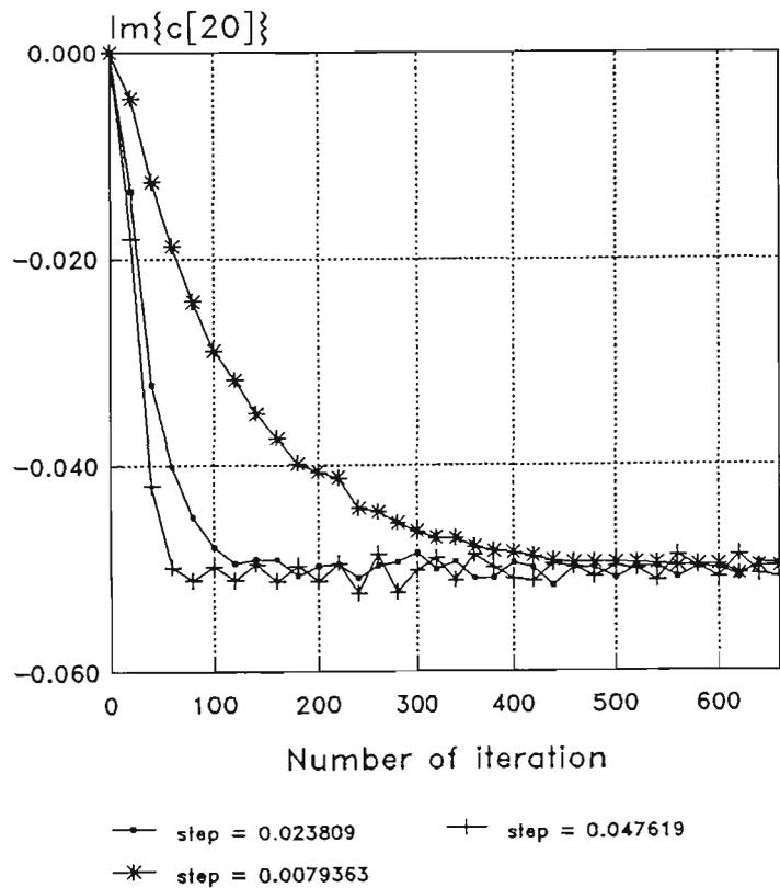
Figure 6.4.3.5 Initial convergence of the LMS algorithm with different step size for given channel - real part of  $c[20]$
