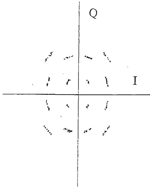
Figure 6.3.1.5 Signal constellation - sinusoidal phase jitter. 14 degree peak to peak
