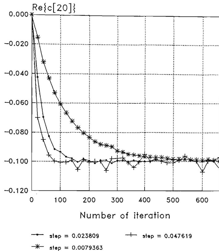
Figure 6.4.3.4 Initial convergence of the LMS algorithm with different step size for the given channel - real part of  $c[20]$
