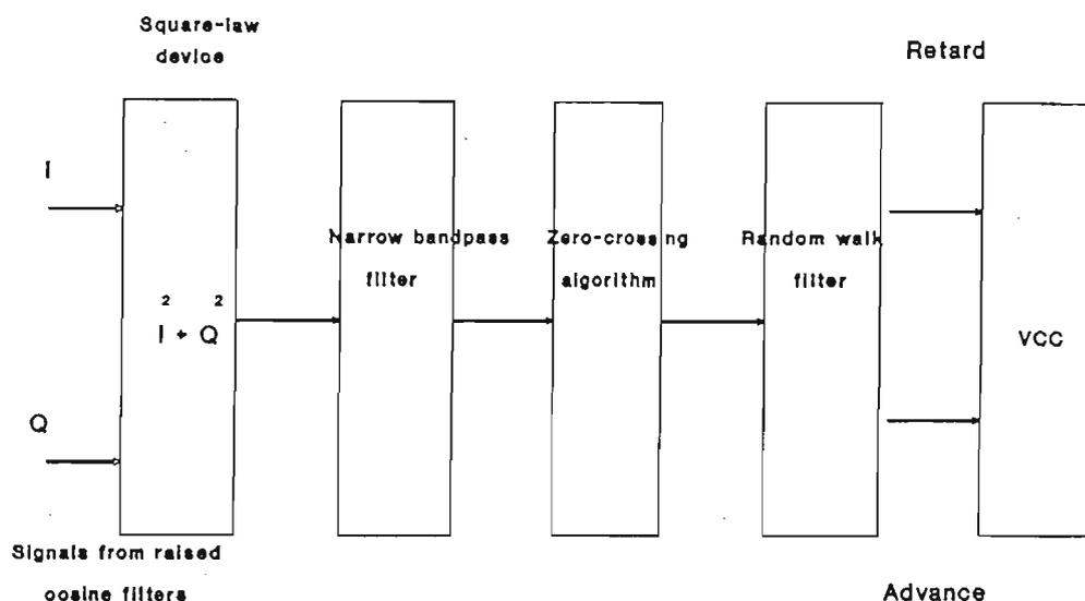
Figure 6.2.2.1 Timing recovery - block diagram
