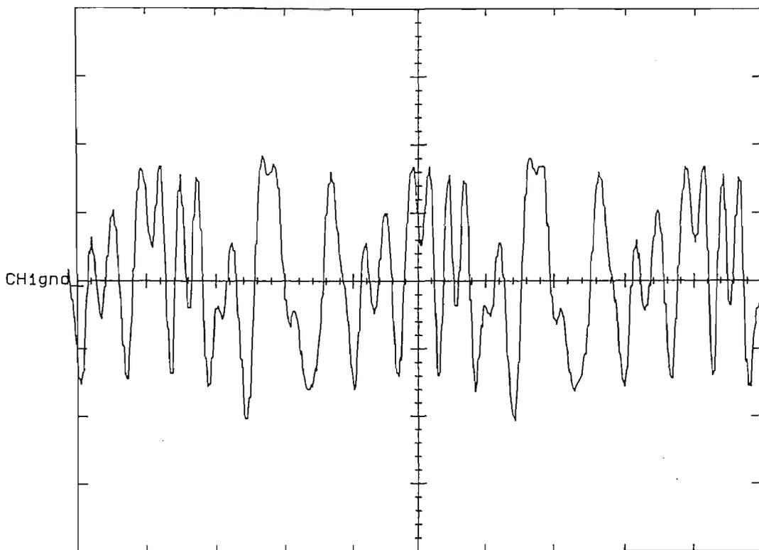
Figure 5.6.2.2 Signal after D/A converter - modulator side
