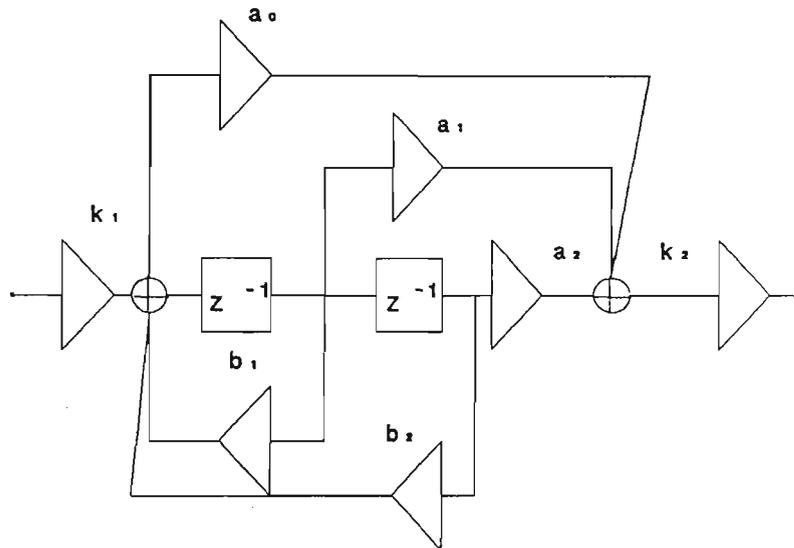
Figure 6.2.2.3 Second order narrow bandpass filter
