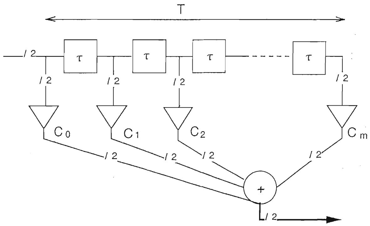
Figure 4.4.1.2 Transversal Filter - complex equaliser for baseband signals
