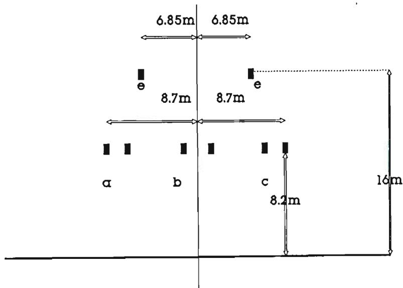
Figure 4.3.1 Line configuration e-earth wires
