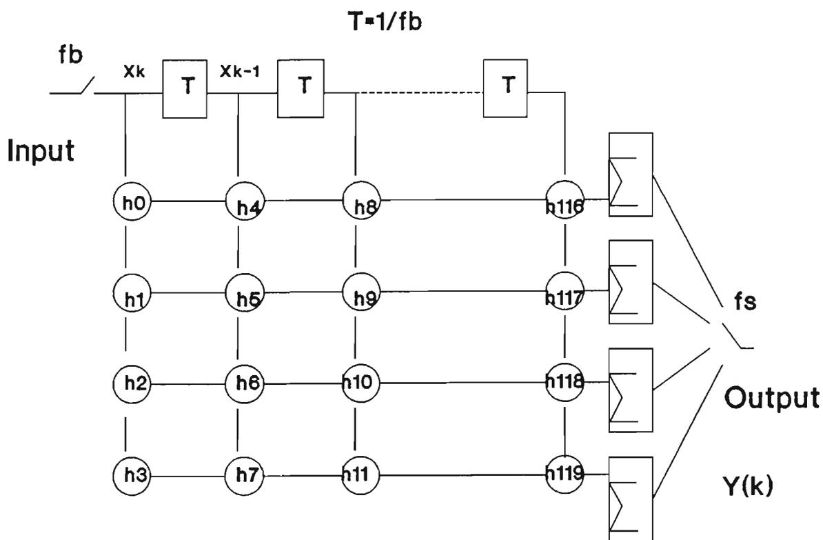
Figure 5.3.3.1 Polyphase interpolation filter
