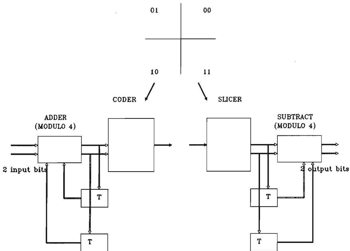
Figure 5.3.2 Differential encoding and decoding
