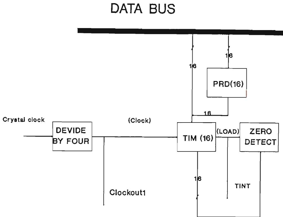
Figure 6.2.5.1 TMS320C25 timer block diagram
