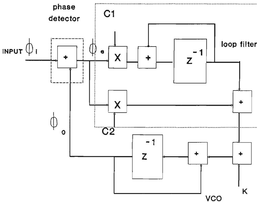
Figure 6.3.2.1 Loop filter incorporated in DPLL
