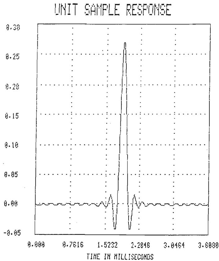
Figure 5.3.5 Unit impulse response of square root raised cosine filter
