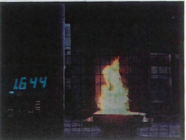
Figure 5.12 Video stills of the oscillating flame 106 seconds after ignition (Test 2)
