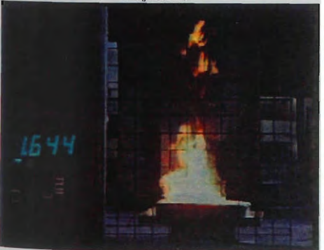
Figure 5.12 Video stills of the oscillating flame 106 seconds after ignition (Test 2)
