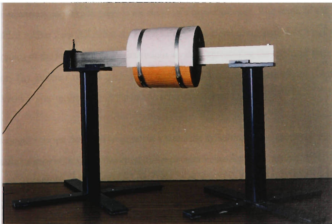
Figure 16. Assembled thigh model attached to support stands.
