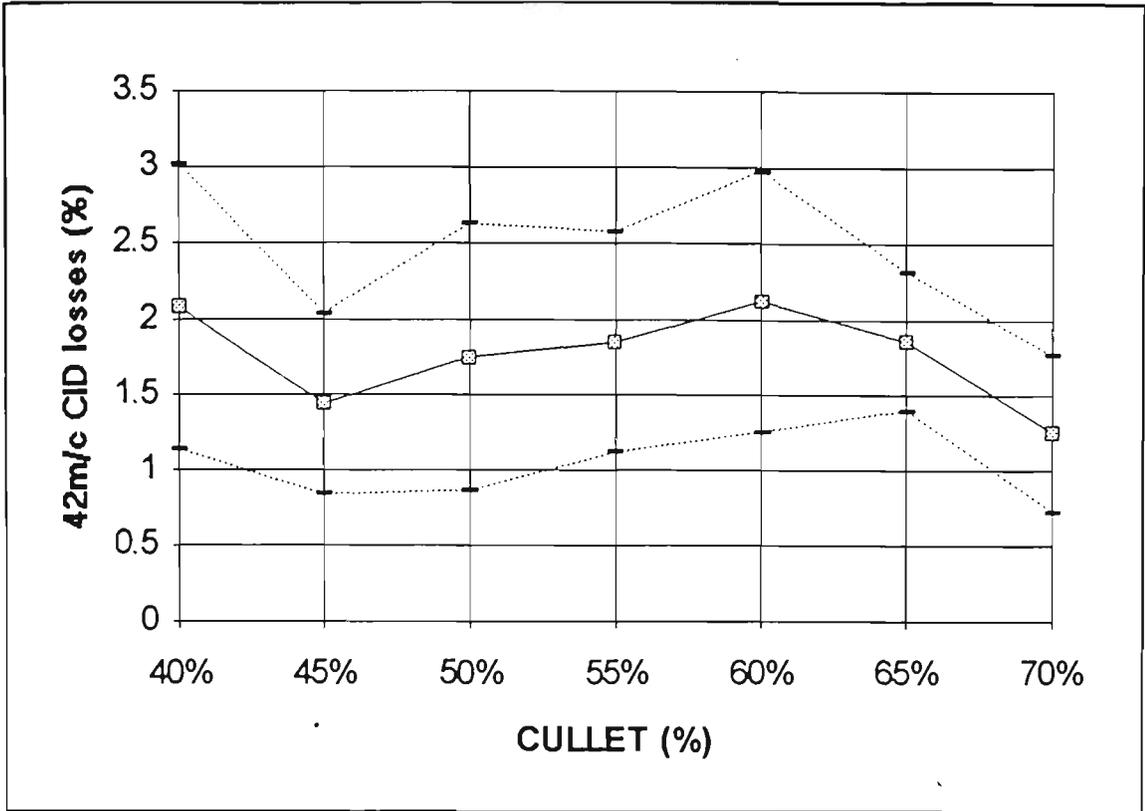
Figure 41. 42m/c CID losses & variance Vs cullet
