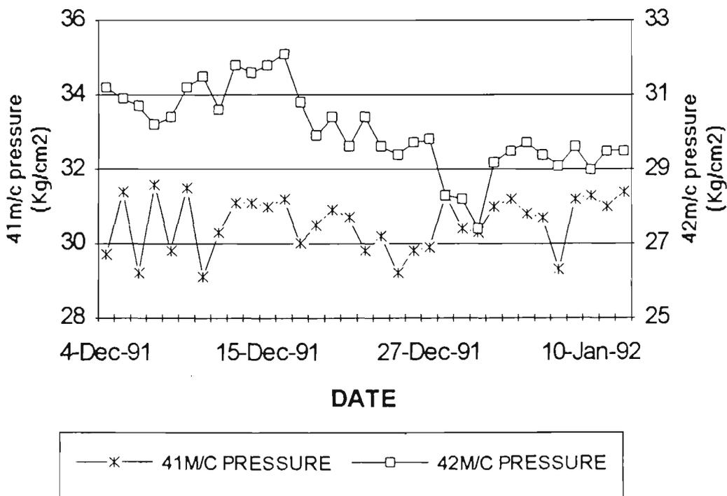
Figure 55. 41m/c & 42m/c breaking pressure at 40% cullet
