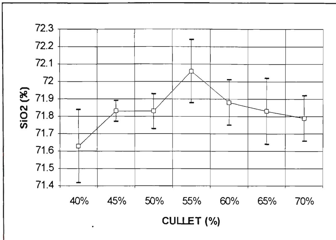
Figure 21. SiO<sub>2</sub> & S.D. Vs cullet, (target = 71.9)
