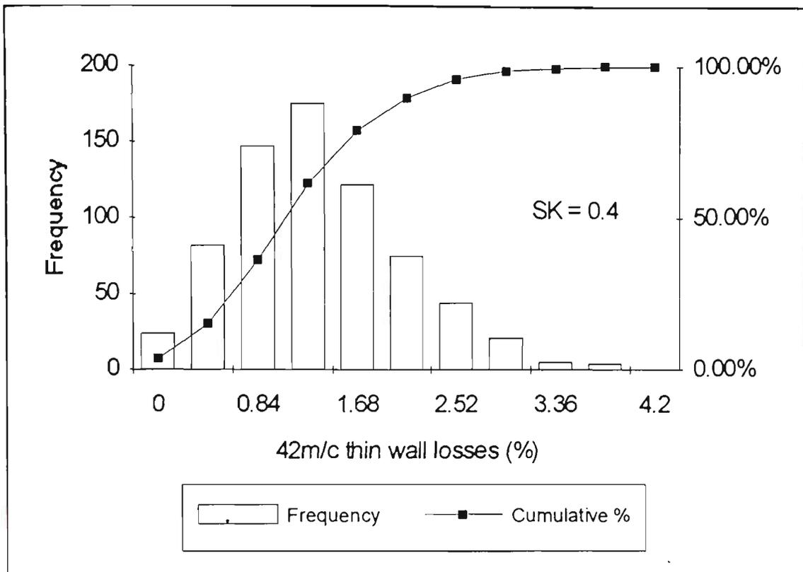
Figure 60. Continuous distribution, 42m/c thin wall losses
