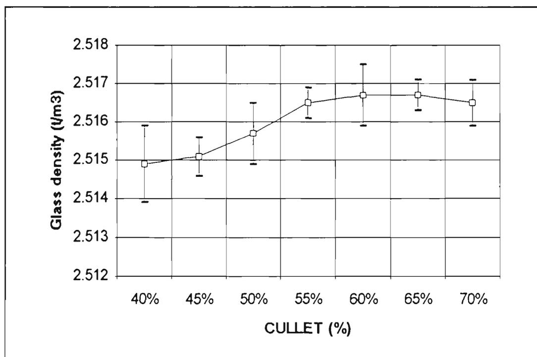
Figure 18. MB4 glass density & S.D. Vs cullet
