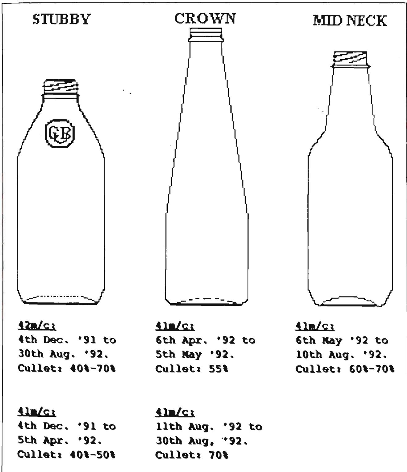
Figure 17. Container profiles and production dates
