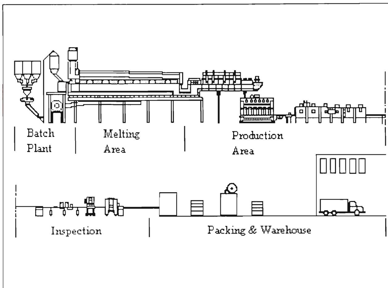
Figure 2. Typical glass plant production line layout
