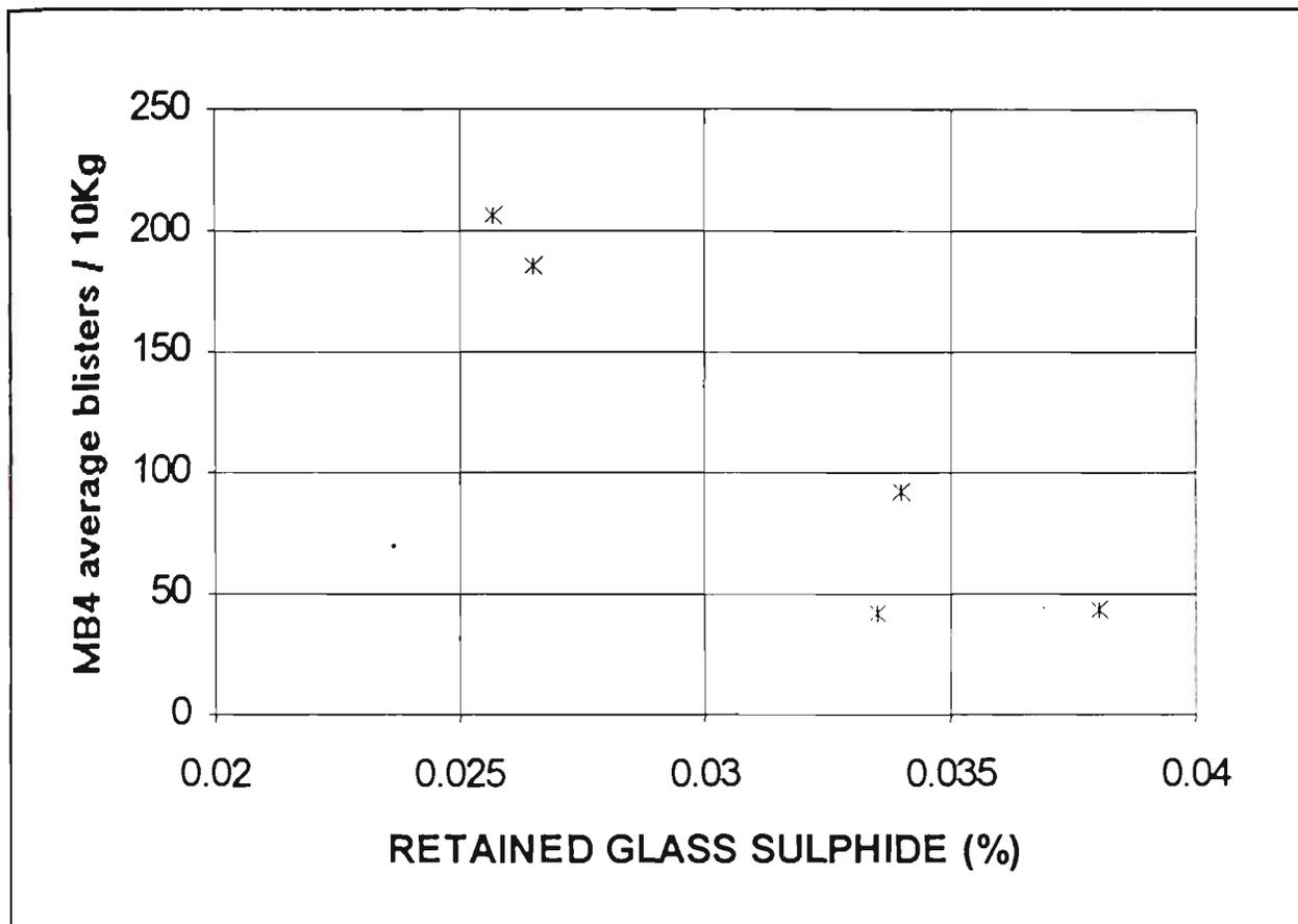
Figure 31. MB4 blister Vs retained sulphide
