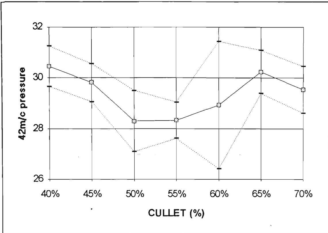
Figure 52. 42m/c breaking pressure & variance Vs cullet
