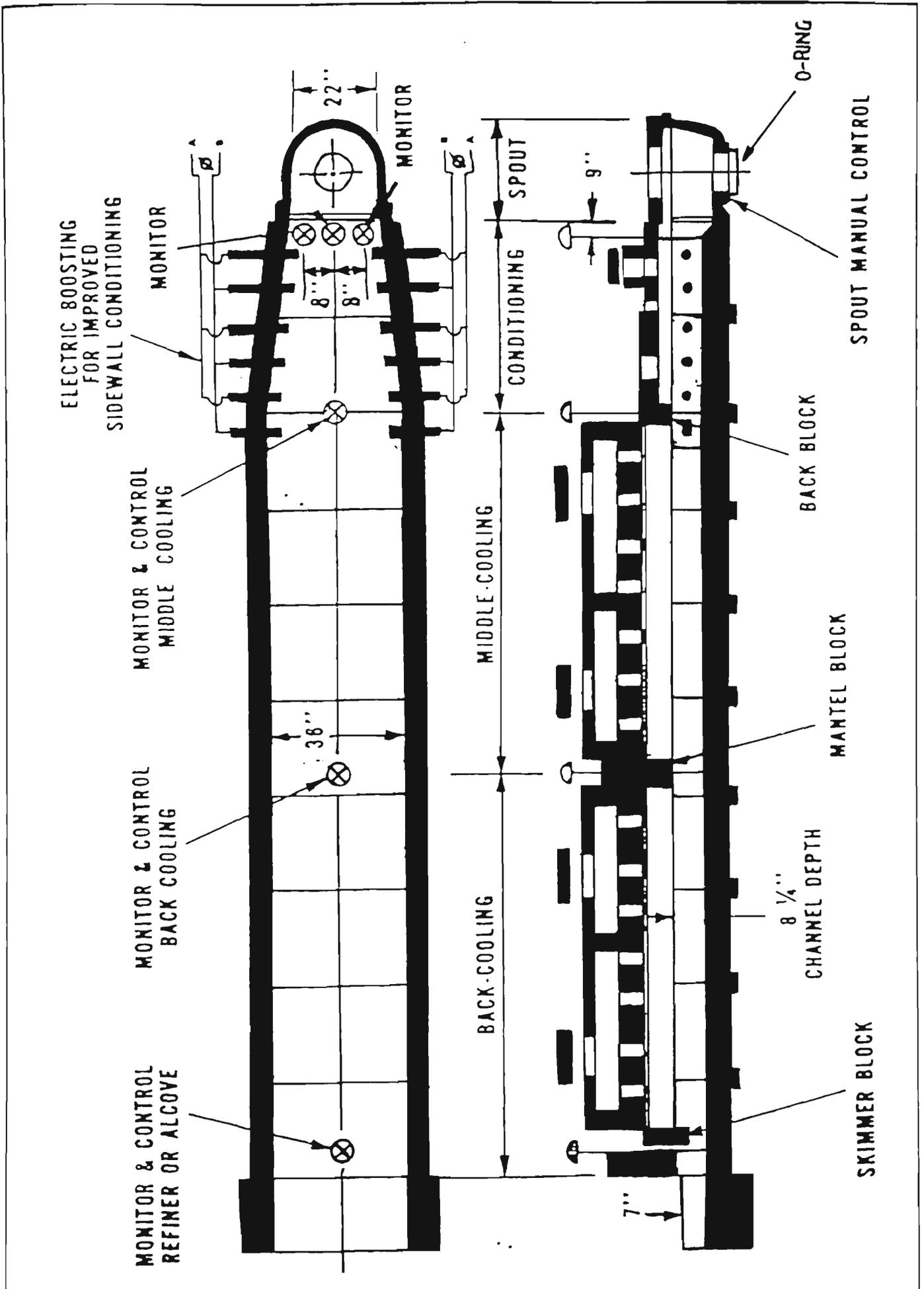
Figure 7. Forehearth schematic diagram (O-B Forehearth training manual)
