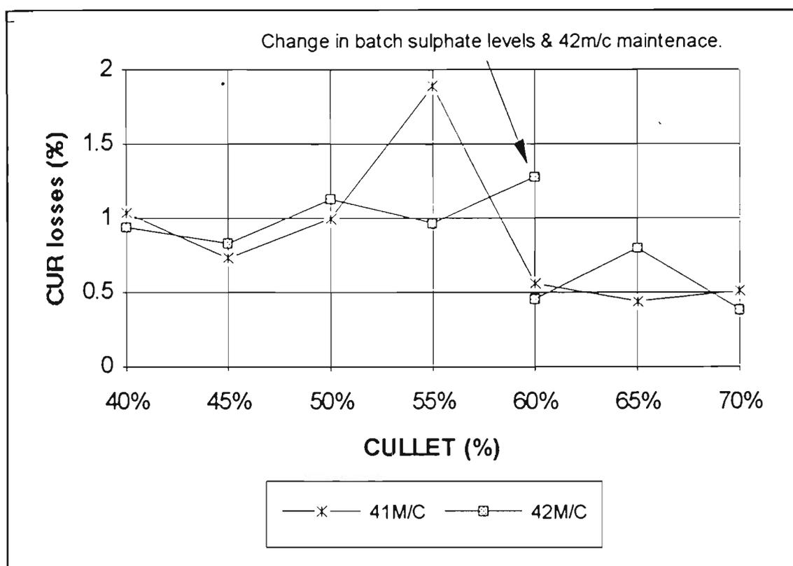
Figure 34. 41m/c & 42m/c CUR losses Vs cullet
