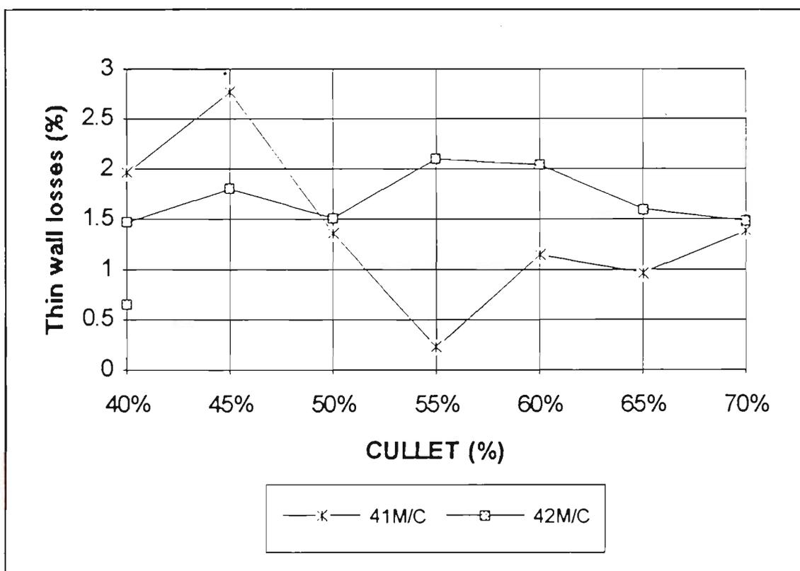
Figure 37. 41m/c & 42m/c thin wall losses Vs cullet
