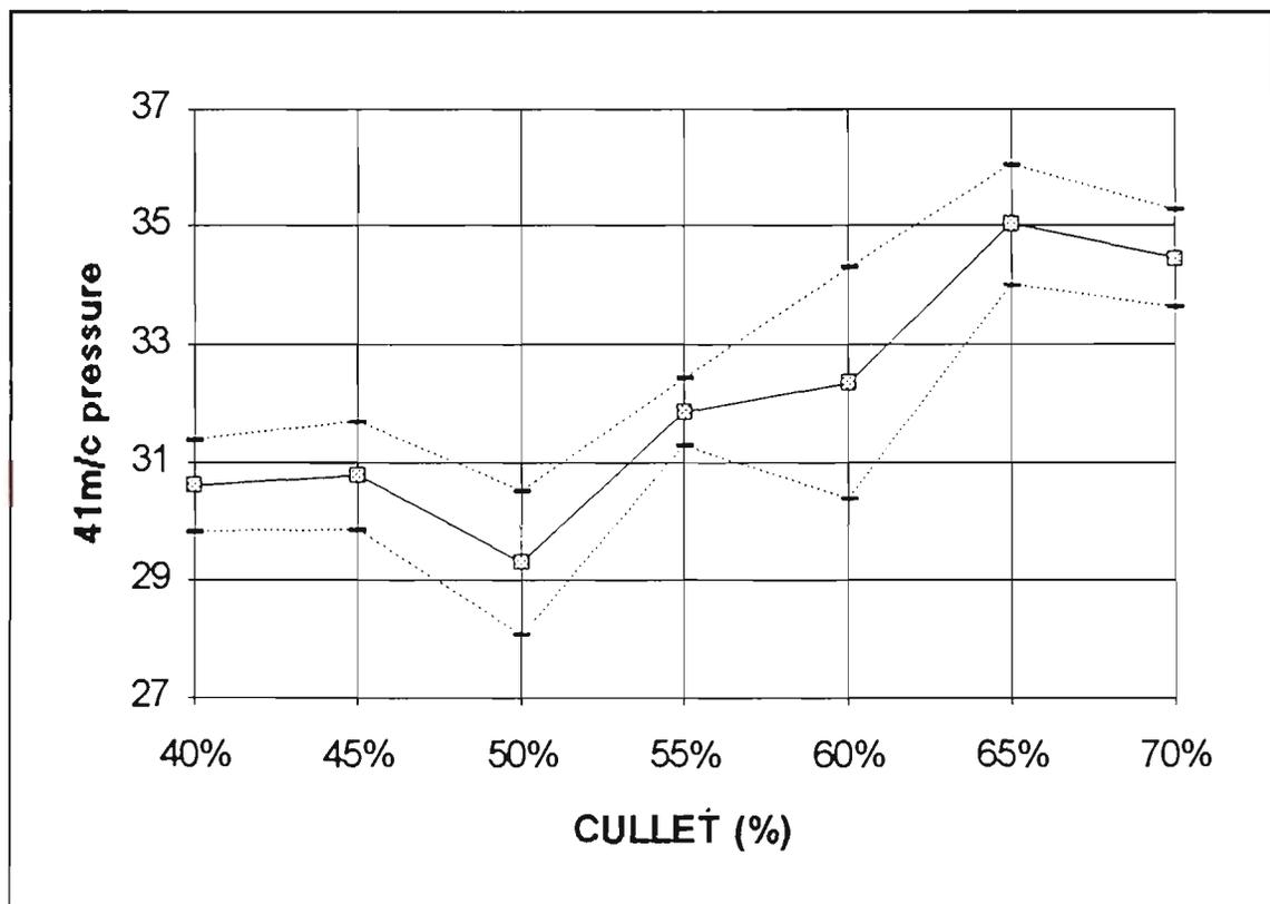
Figure 51. 41m/c breaking pressure & variance Vs cullet
