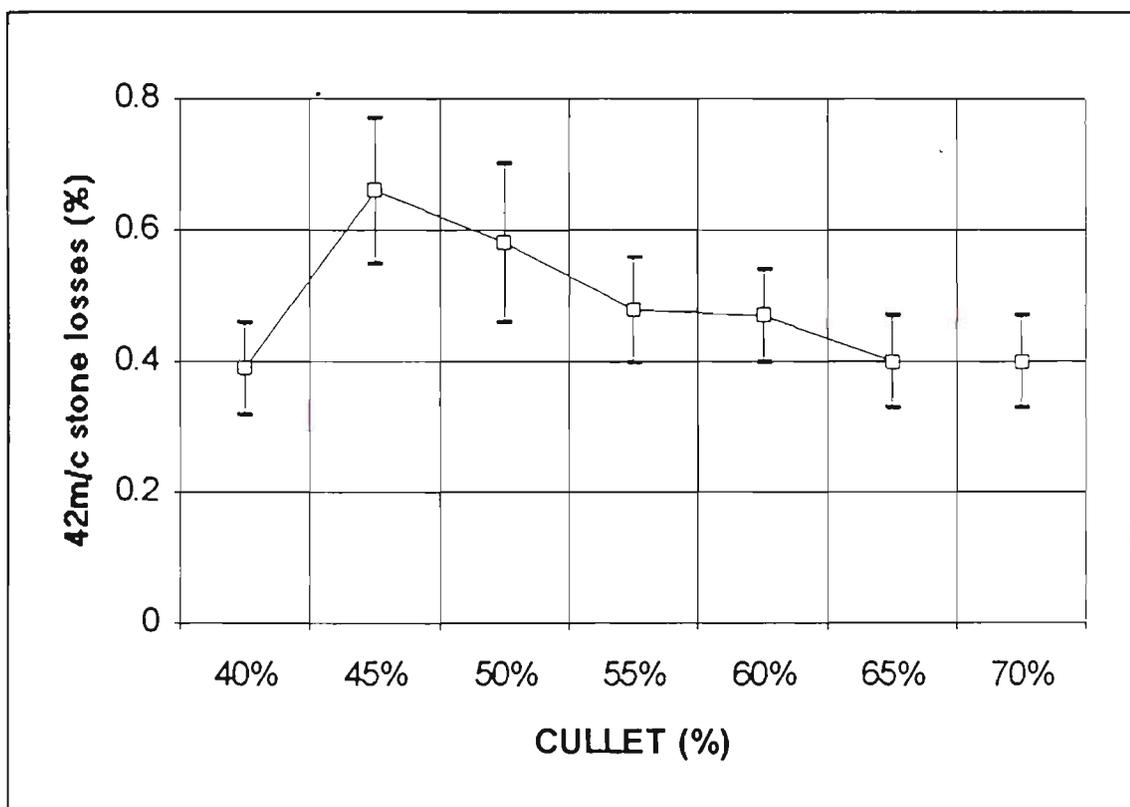
Figure 27. 42m/c stone losses & S.D. Vs cullet
