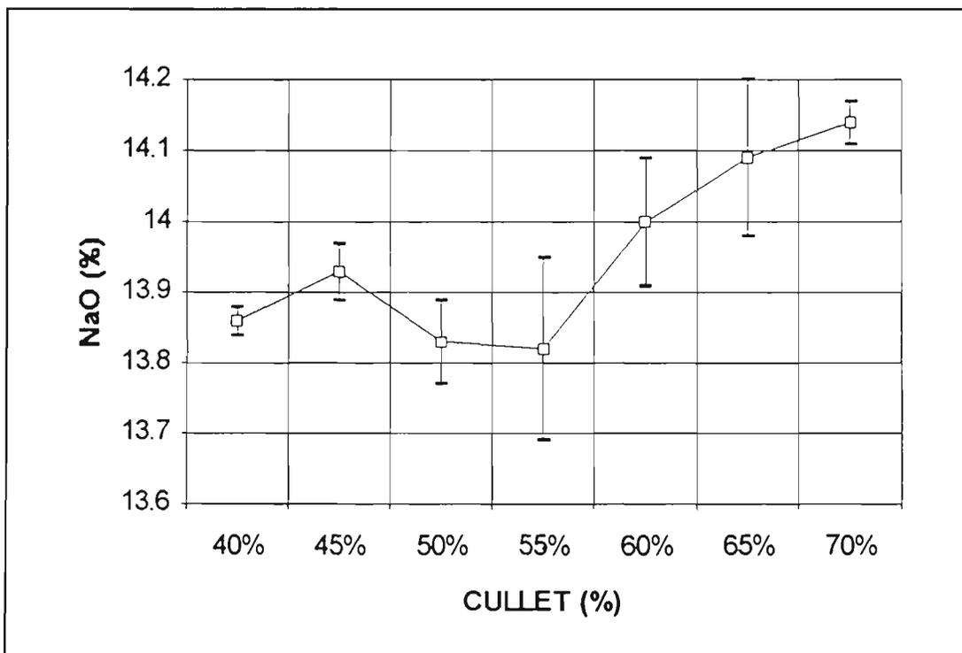
Figure 20. NaO & S.D. Vs cullet, (target = 13.9%)
