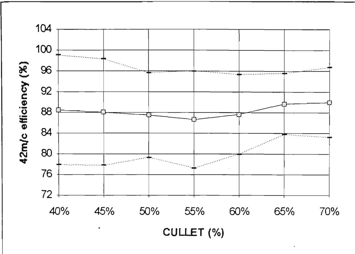
Figure 48. 42m/c efficiency & variance Vs cullet
