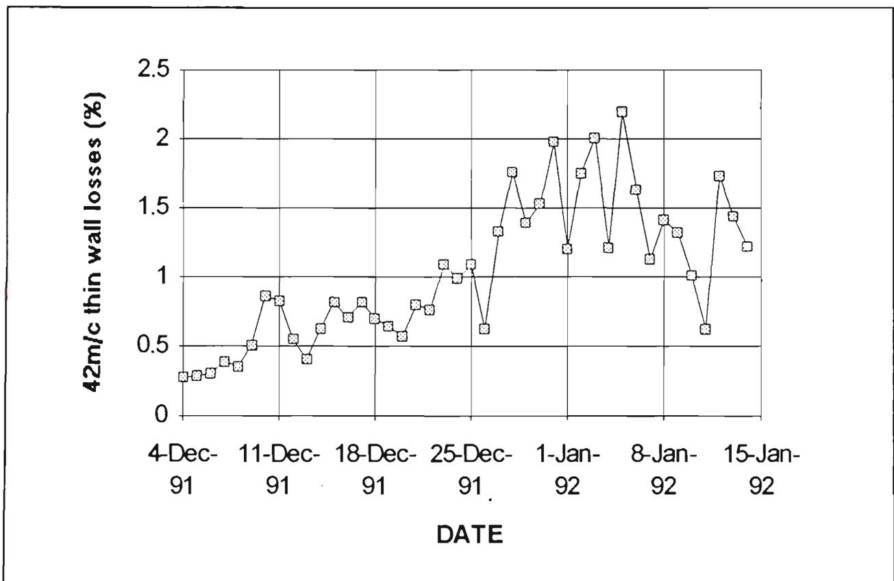
Figure 43. 42m/c thin wall losses at 40% cullet
