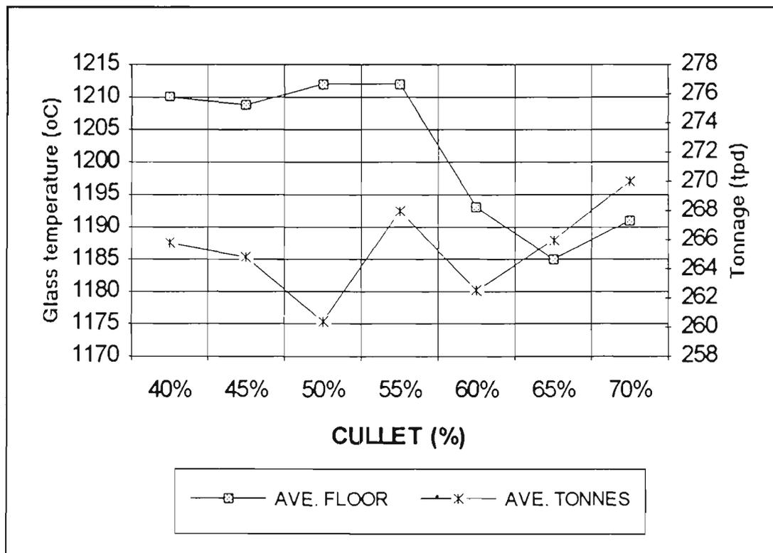
Figure 23. MB4 glass temperature & tonnage Vs cullet
