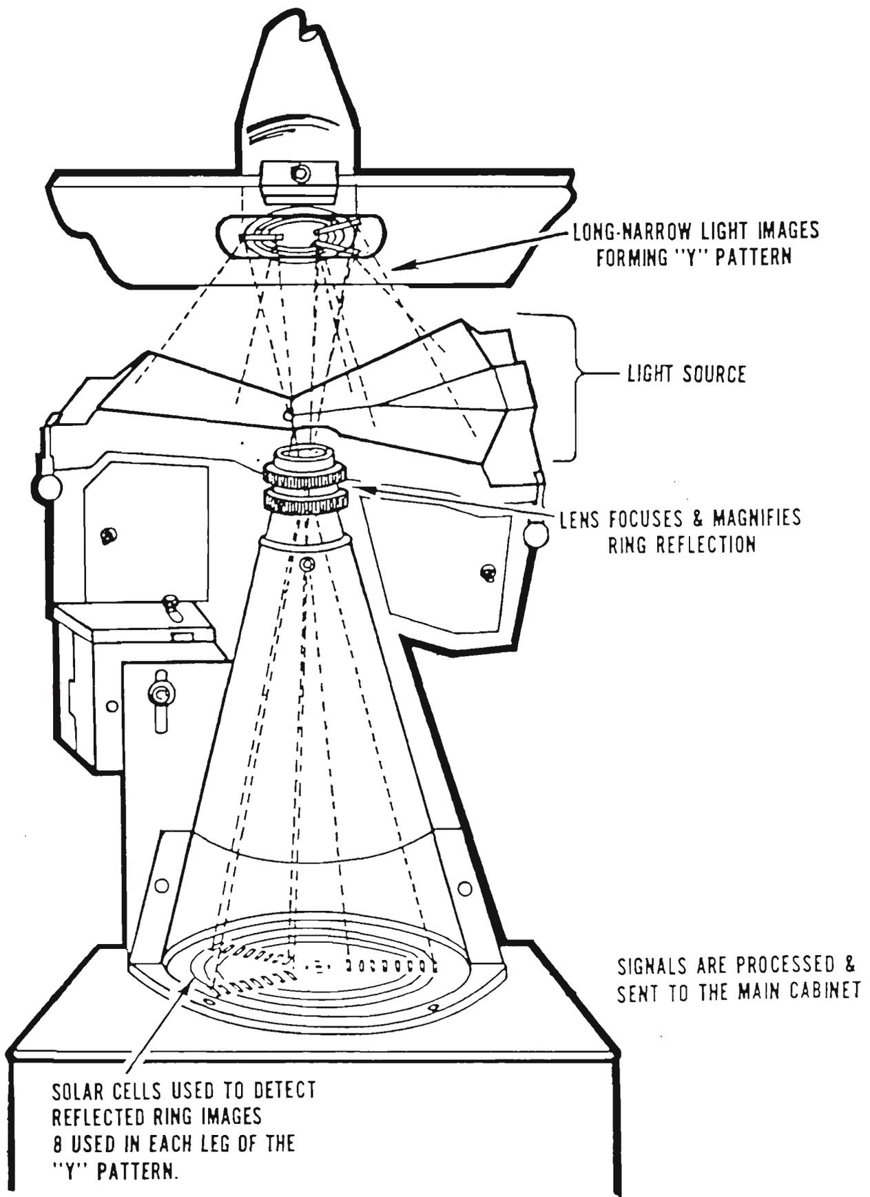
Figure 14. Cavity identification device for CID rejects (O-B technical manual)
