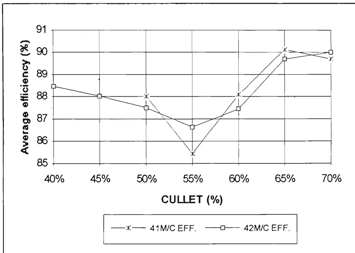
Figure 47. 41m/c & 42m/c efficiency Vs cullet
