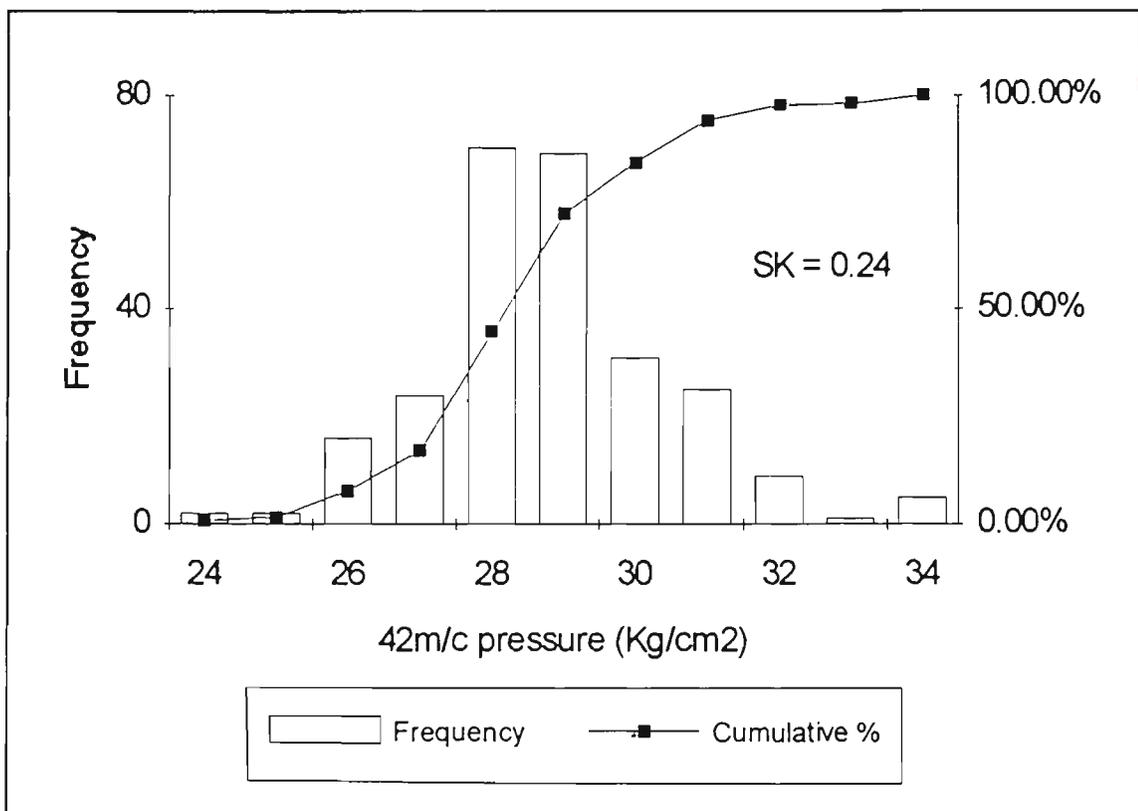
Figure 63. Continuous distribution, 42m/c breaking pressure
