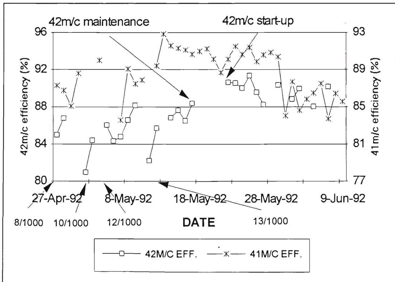
Figure 56. 41m/c & 42m/c efficiency at 60% cullet
