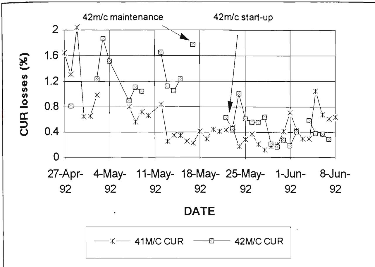
Figure 45. 41m/c & 42m/c CUR losses at 60% cullet
