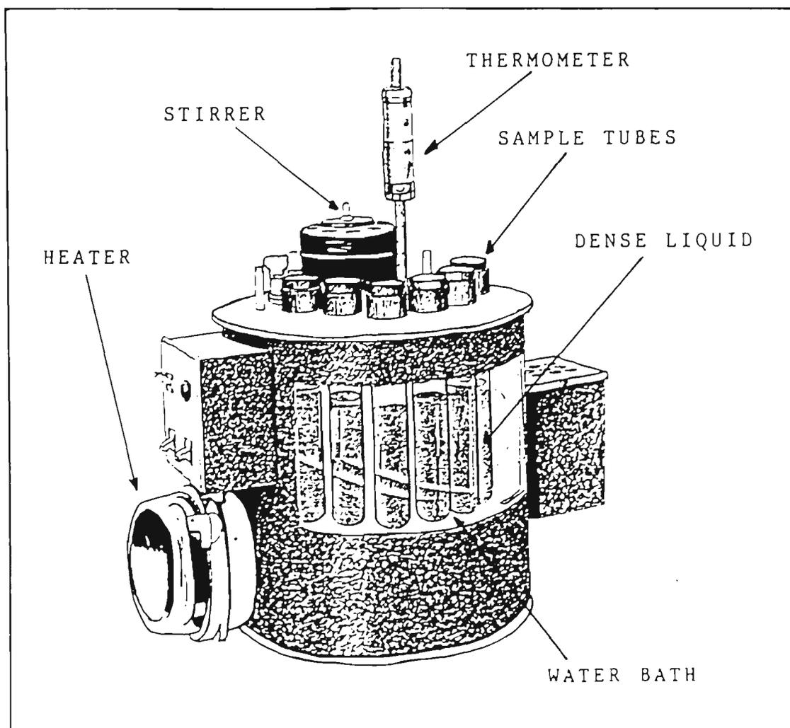
Figure 15. Sink/float glass density comparator
