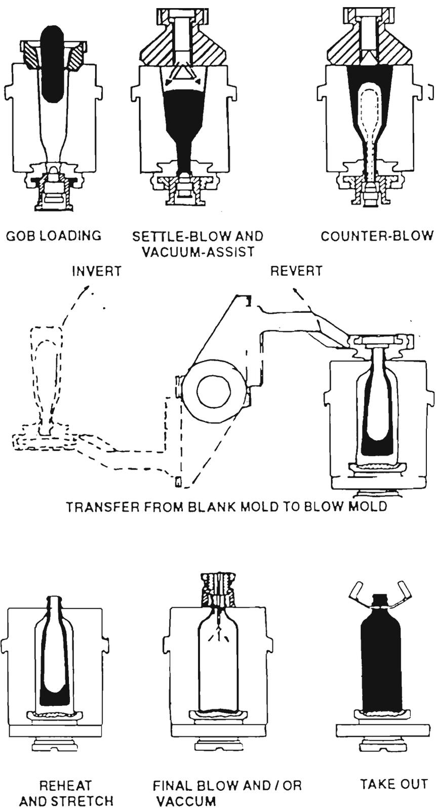
Figure 9. Functional diagram of bottle forming, blow & blow process (Emhart technical training manual)
