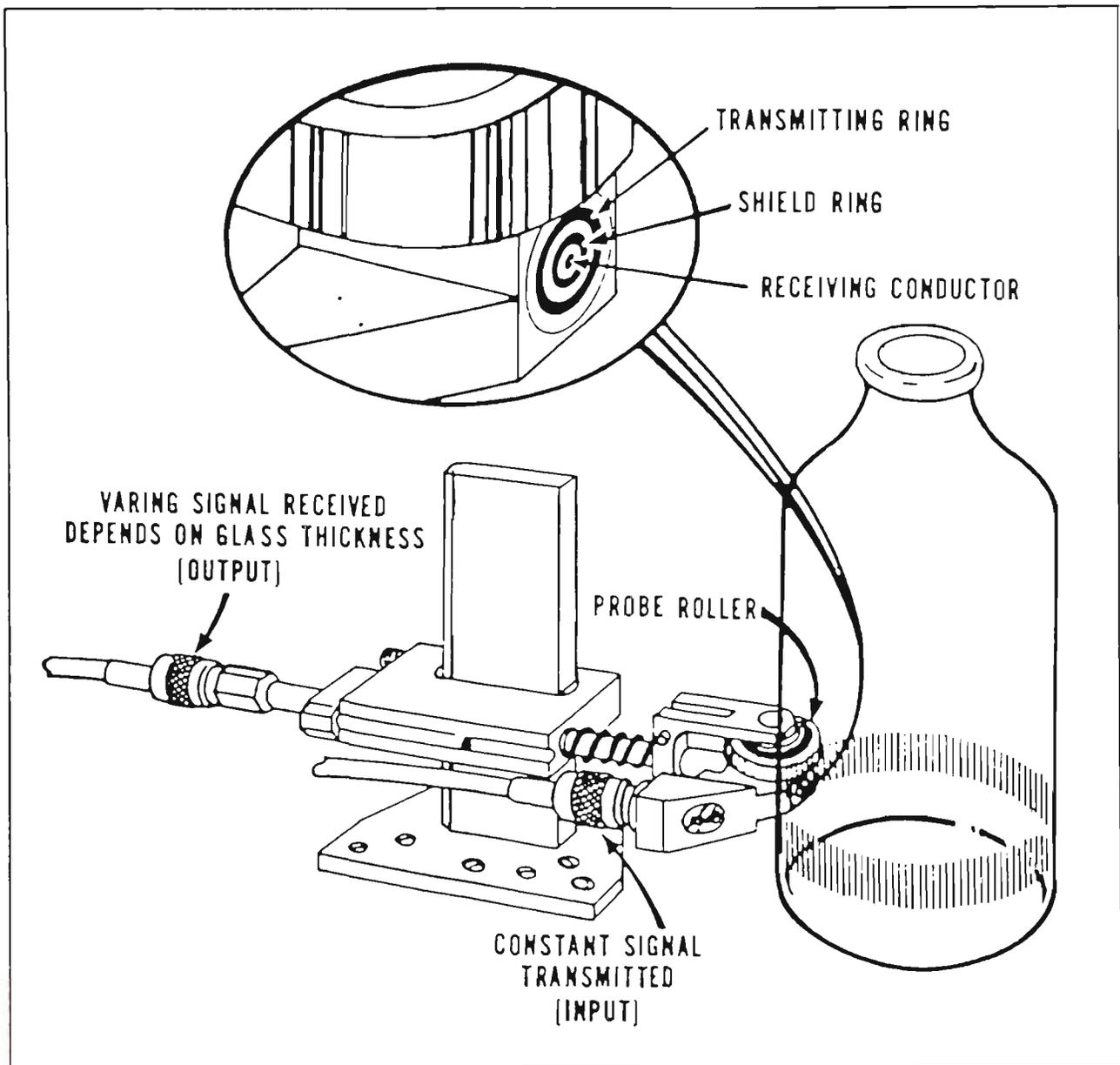
Figure 11. Radio frequency gauge (RF), for thin wall defects (O-B technical manual)
