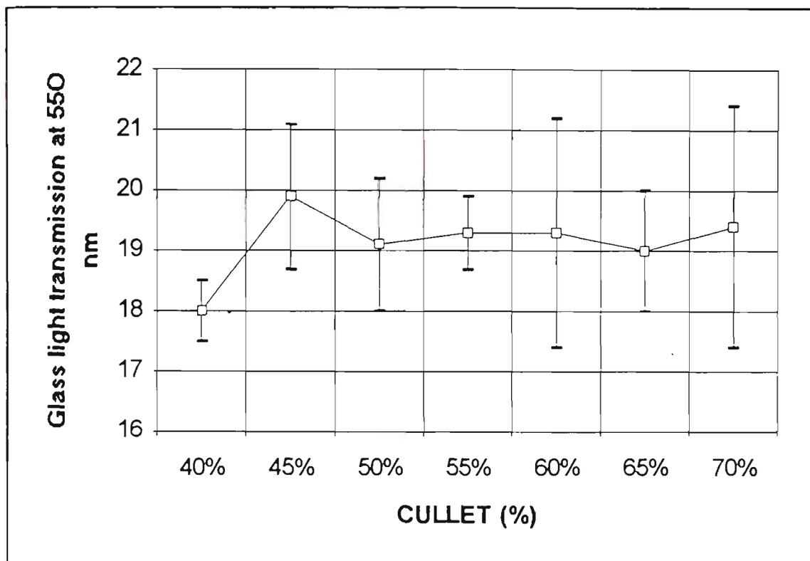
Figure 28. MB4 T550% & S.D. Vs cullet
