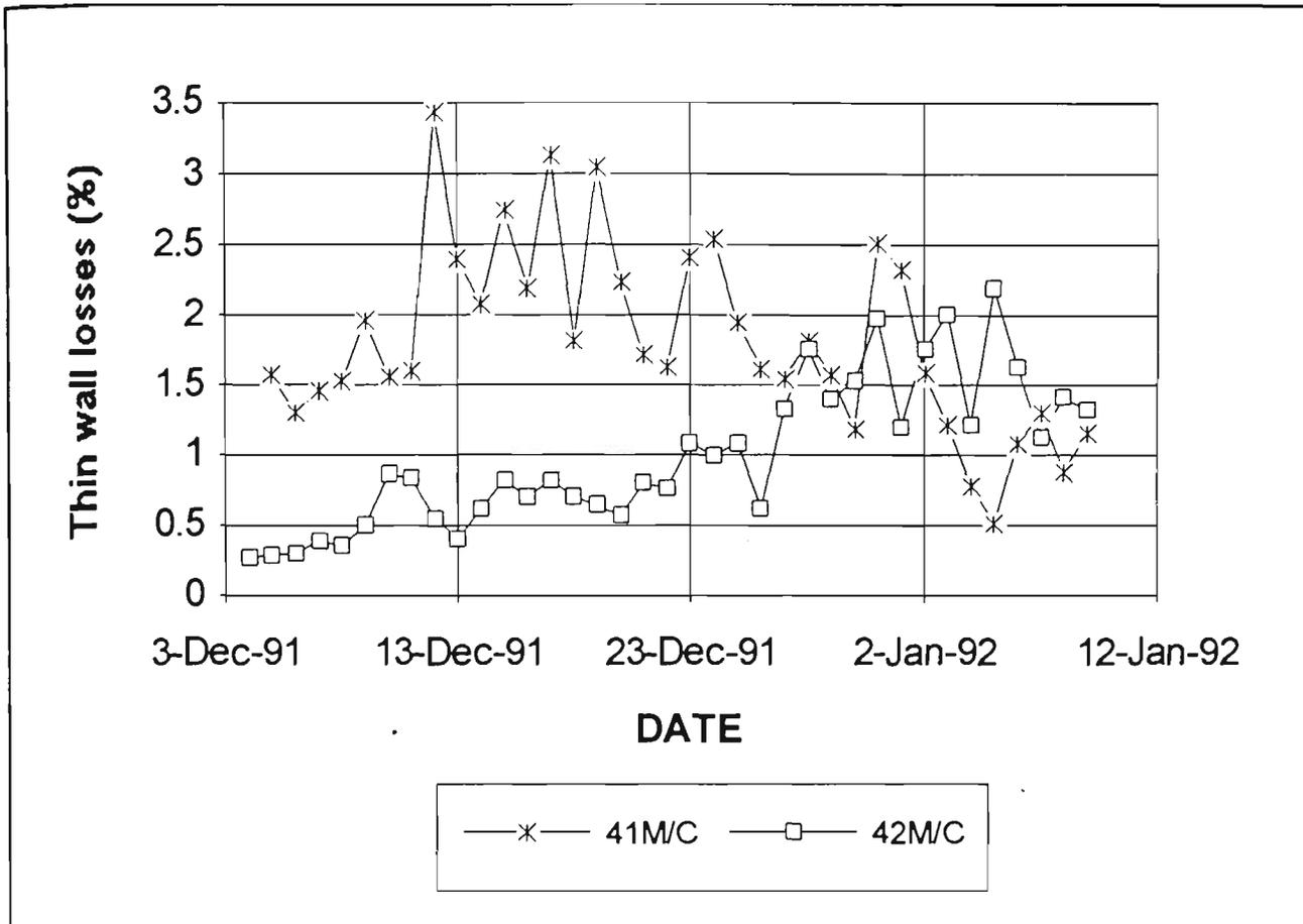
Figure 44. 41m/c & 42m/c thin wall losses at 40% cullet
