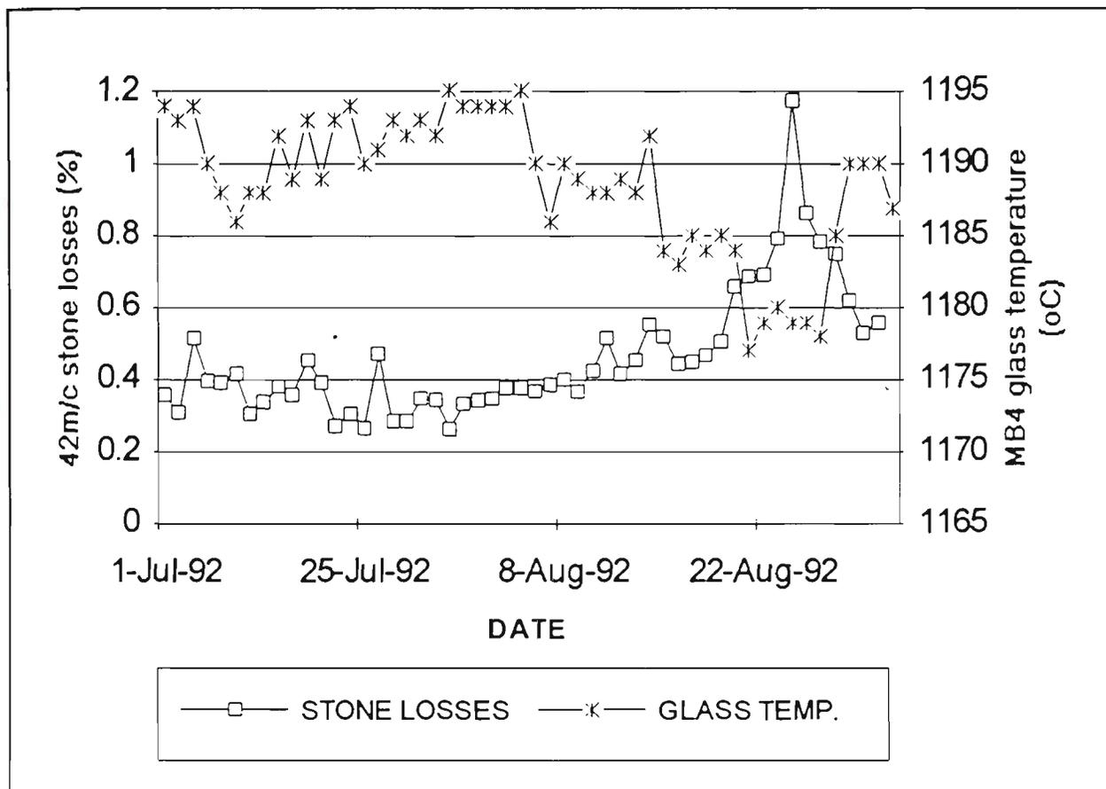
Figure 29. MB4 glass temperature & 42m/c stone losses at 70% cullet
