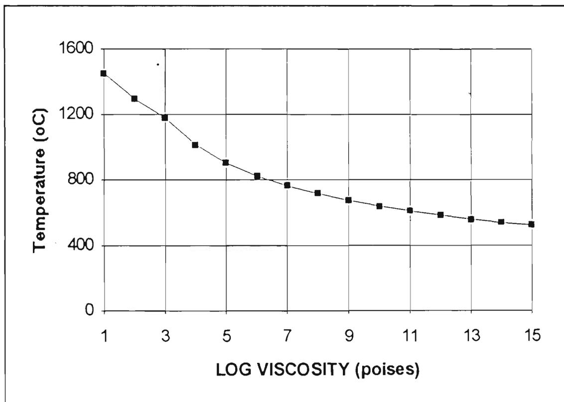
Figure 57. Temperature Vs Log viscosity for commercial soda-lime-silica glass
