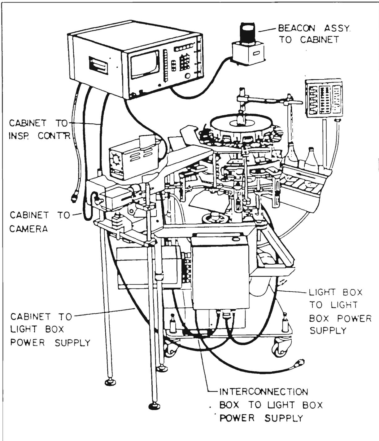
Figure 10. Triple check inspector (O-B technical manual)
