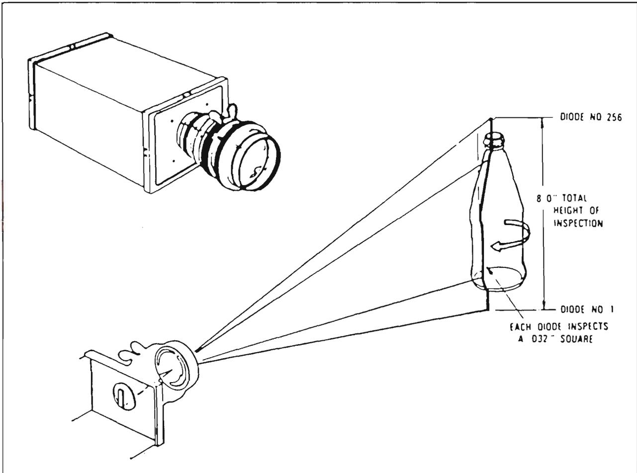
Figure 13. Side wall inspector, for SID faults (O-B technical manual)
