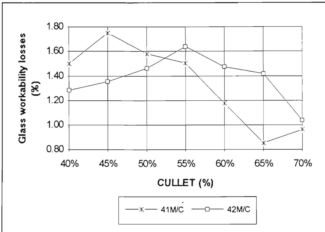
Figure 33. Average workability losses Vs cullet
