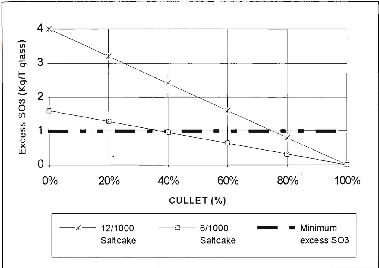
Figure 32. Theoretical glass excess SO<sub>3</sub> % Vs cullet
