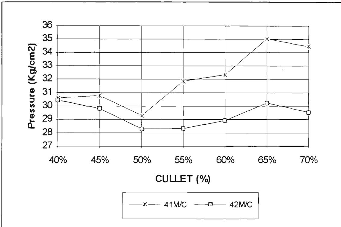
Figure 50. 41m/c & 42m/c breaking pressure Vs cullet
