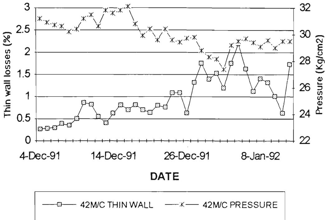
Figure 54. 42m/c thin wall losses & breaking pressure at 40% cullet
