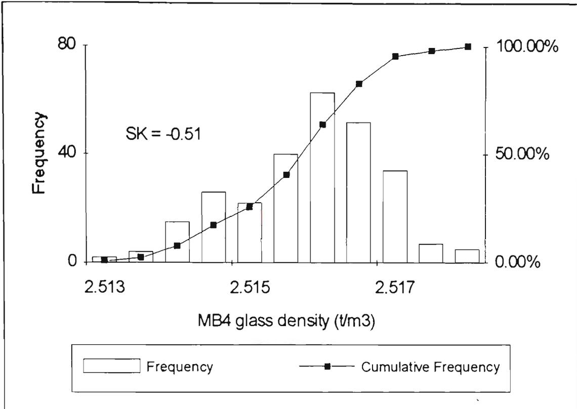
Figure 64. Continuous distribution, MB4 density
