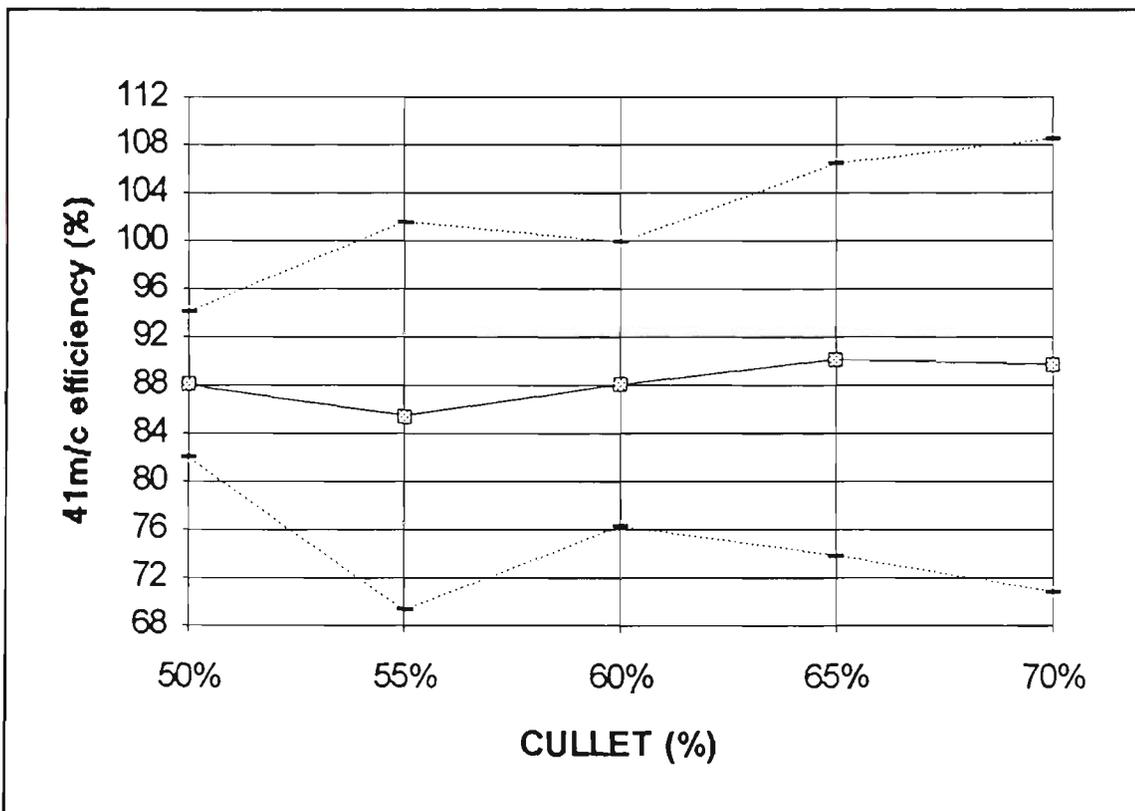
Figure 49. 41m/c efficiency & variance Vs cullet
