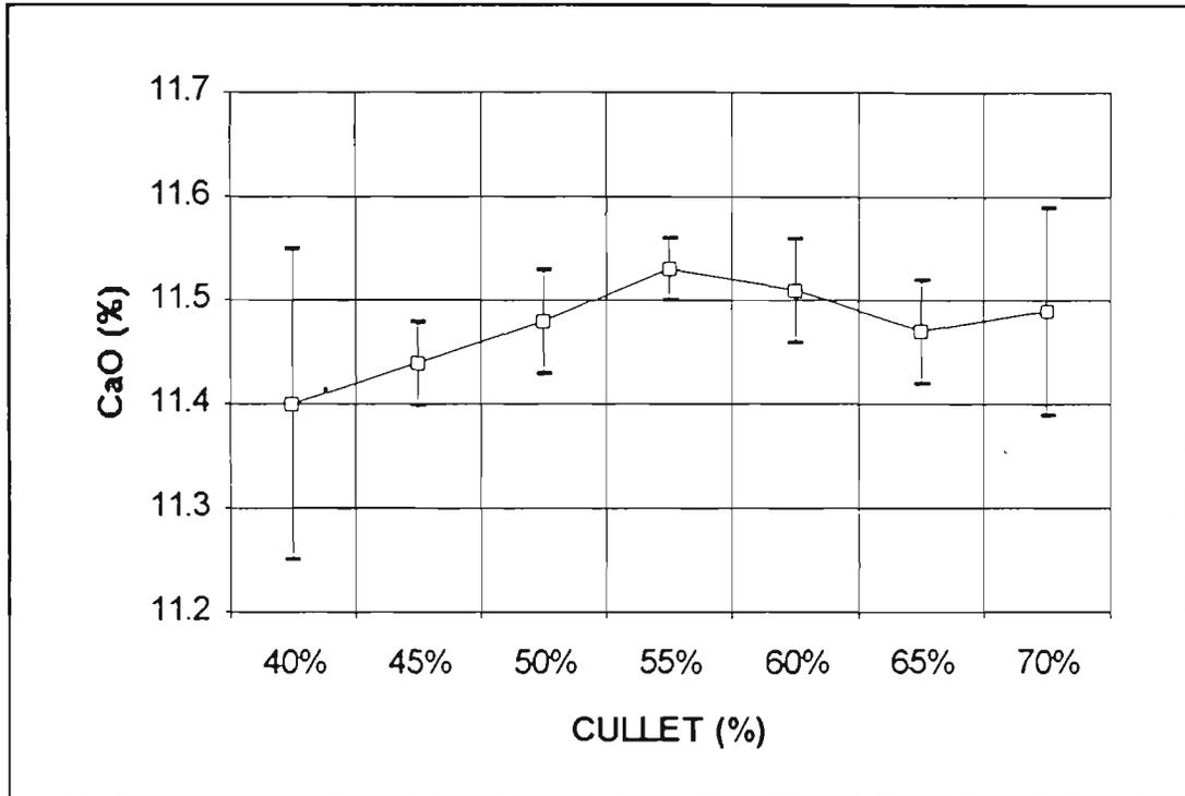
Figure 19. CaO & S.D. Vs cullet, (target = 11.5%)
