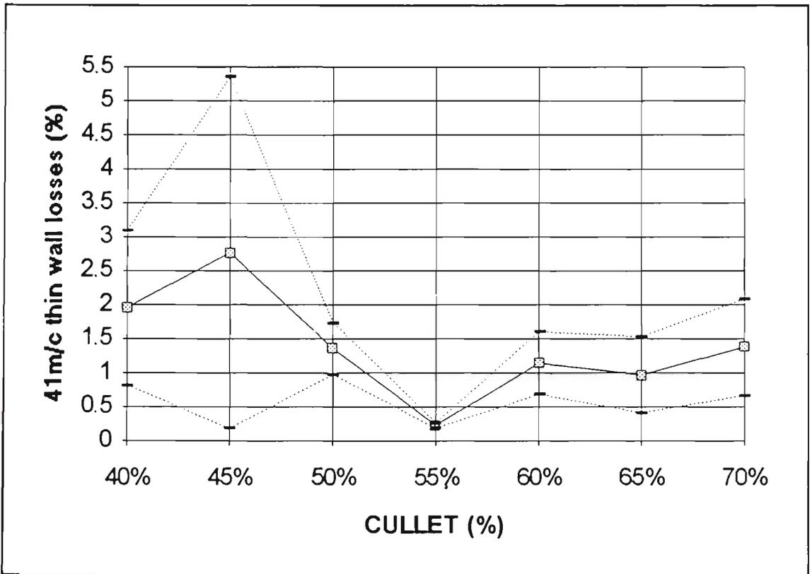
Figure 39. 41m/c thin wall losses & variance Vs cullet
