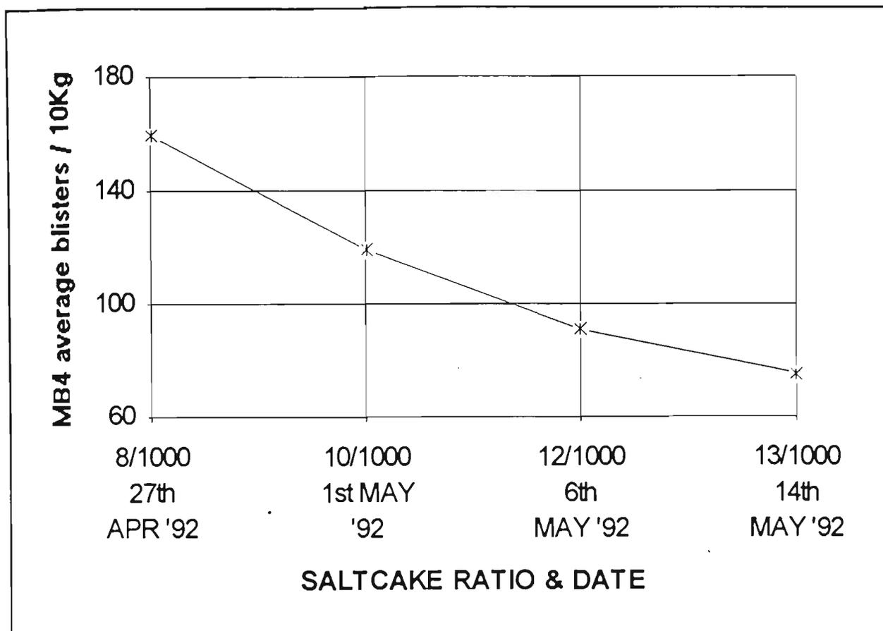
Figure 30. MB4 blister Vs saltcake ratio at 60% cullet
