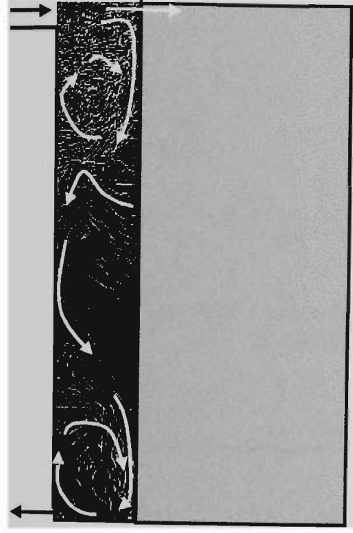
(b) Enhanced image. H=0.05 m, h_p=0.1 m, U_b=1.6 m/s, G10 foam.
