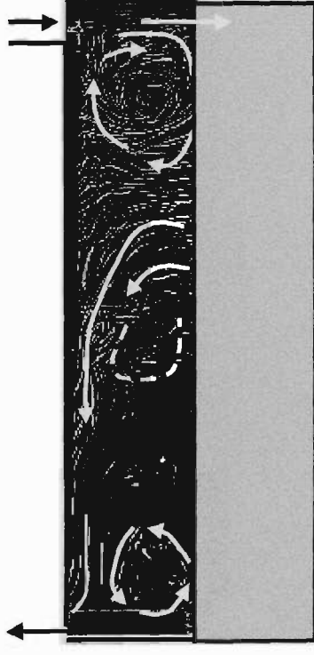
(b) Enhanced image. H=0.05 m, h_p=0.05 m, U_b=1.6 m/s, G10 foam.
