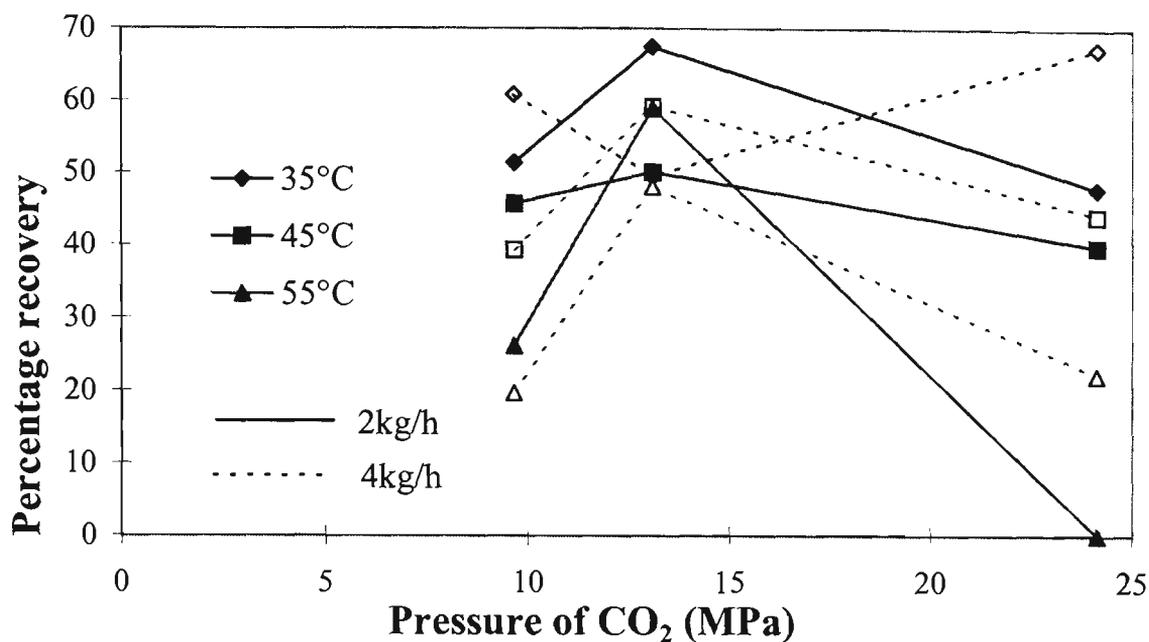
Fig 5.30. Percentage recovery of decanal 10 times concentrated as the feed (dec/lim) (observed), isotherms as functions of pressure.
