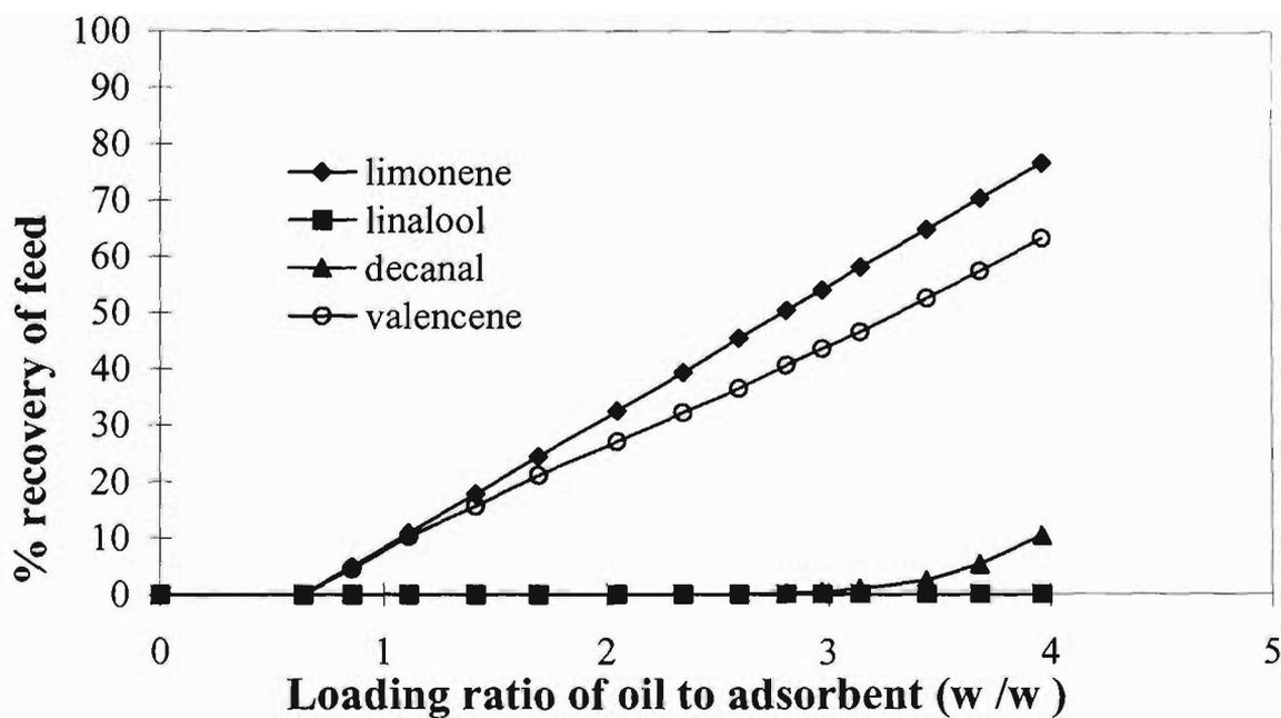
Fig. 4.5. Breakthrough curve of orange oil (25.33 g) on Silica gel (35-70 mesh, 6.39 g).
