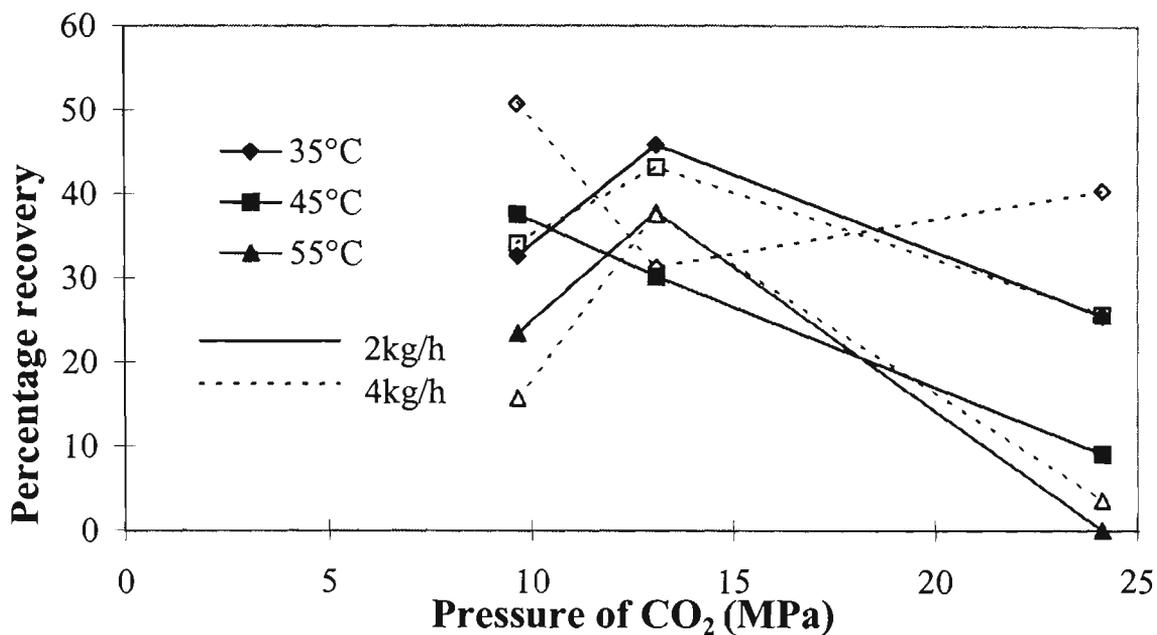
Fig 5.38. Percentage recovery of decanal 15 times concentrated as the feed (dec/lim) (observed), isotherms as functions of pressure.
