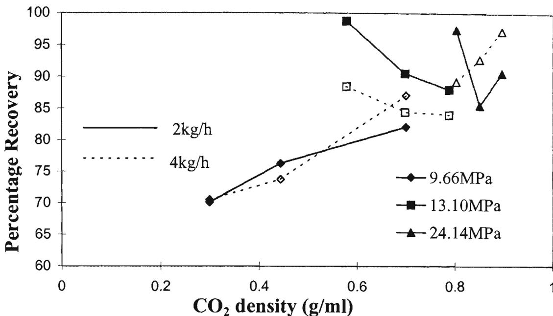
**Fig 5.25. Percentage recovery of total feed alcohols using 5 kg CO<sub>2</sub>, isobars as functions of density (observed).**
