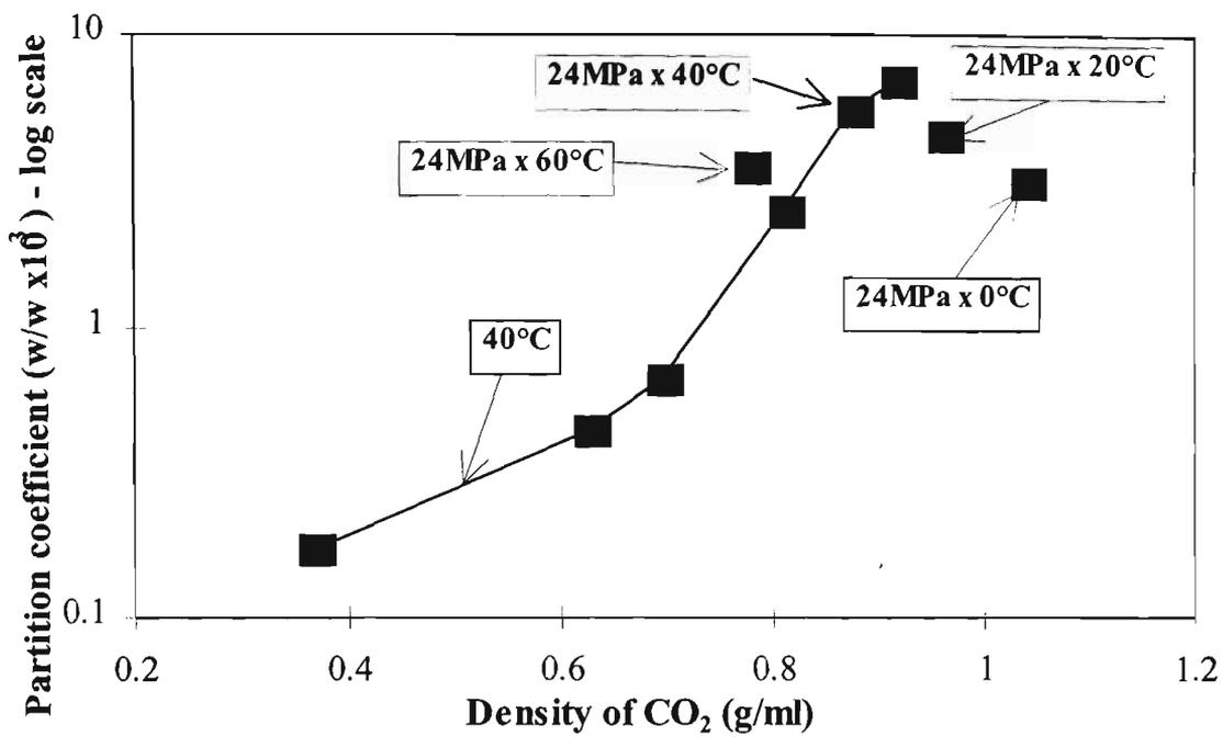
**Fig. 3.3. Partition coefficients of triglycerides in rice bran oil plotted on a logarithmic scale. Single points represent the mean values of data from duplicated experiments.**
