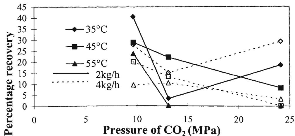
Fig 5.42. Percentage recovery of linalool 15 times concentrated as the feed (lin/lim) (observed), isotherms as functions of pressure of CO<sub>2</sub>.
