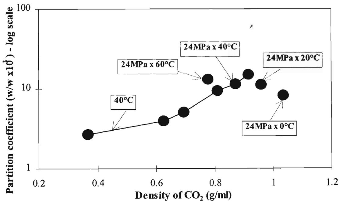
**Figure 3.4. Partition coefficients of FFA in rice bran oil plotted on a logarithmic scale. Single points represent the mean values of data from duplicated experiments.**
