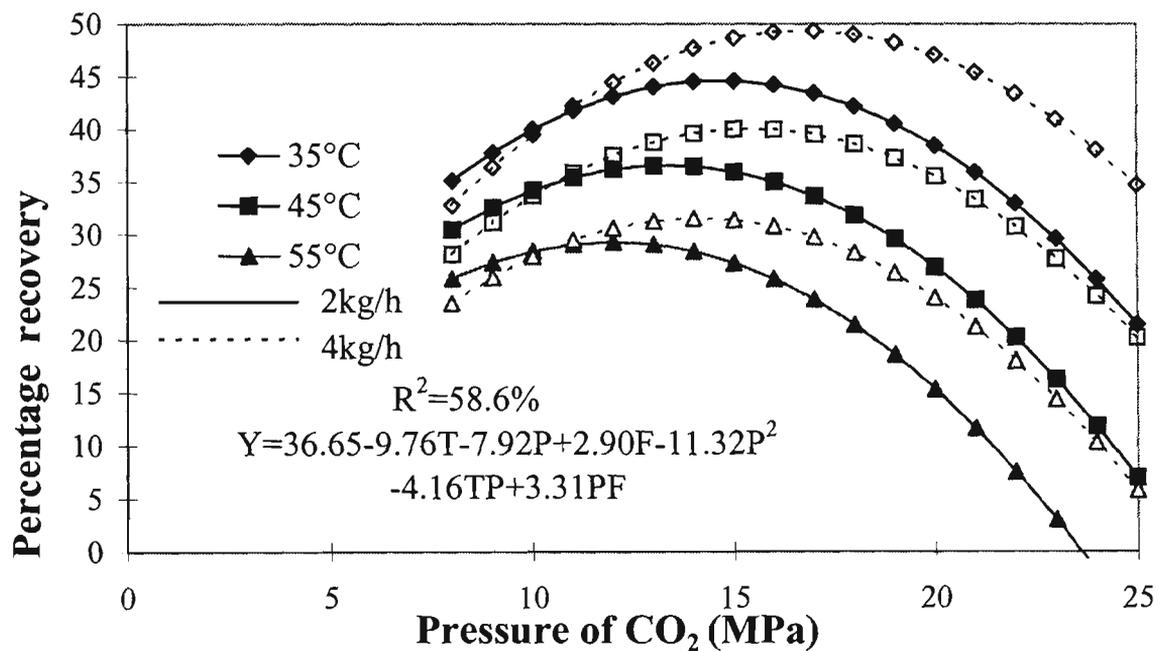
Fig 5.39. Percentage recovery of decanal 15 times concentrated as the feed (dec/lim) (modelled), isotherms as functions of pressure of CO<sub>2</sub>. T, P and F in this model represent the coded value of temperature, pressure and flowrate of CO<sub>2</sub>. R<sup>2</sup> is the percentage of variance accounted for by the model.
