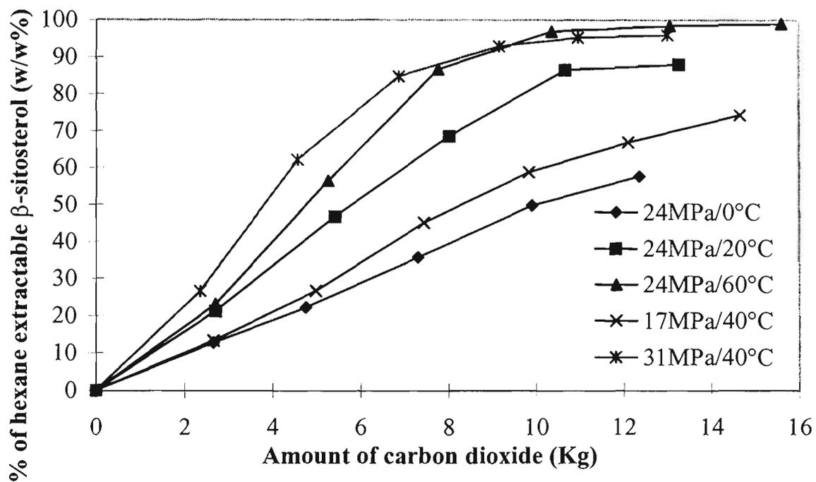
Figure 2.9. Extraction of beta-sitosterol from rice bran by dense CO<sub>2</sub> at different temperatures and pressures (CO<sub>2</sub> flow rate, average of 2.5 Kg/h).
