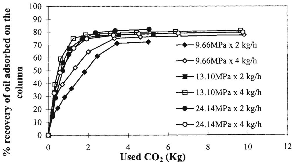
Fig 5.9. Effect of pressure and flowrate on the total orange oil recovery of CO<sub>2</sub> desorption at 55°C.
