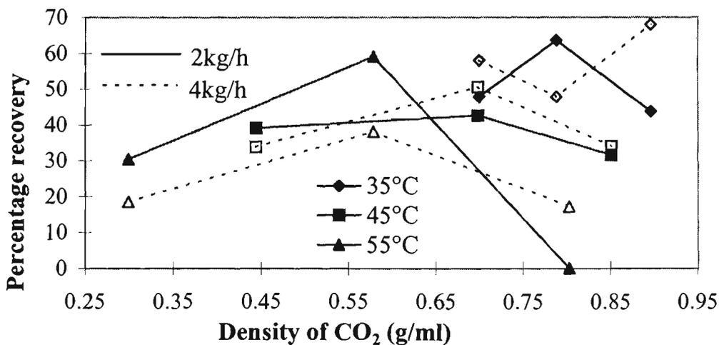
Fig 5.29. Percentage recovery of aldehydes 10 times concentrated as the feed (ald/ter) (observed), isotherms as functions of density.
