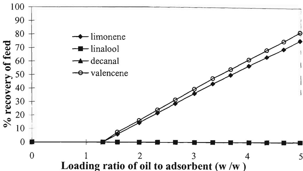
**Fig. 4.12. Breakthrough curve of orange oil (pumping- 0.85g oil/min) on Silica gel (70-230 mesh, 14.95 g). The two curves of decanal and linalool overlap each other.**
