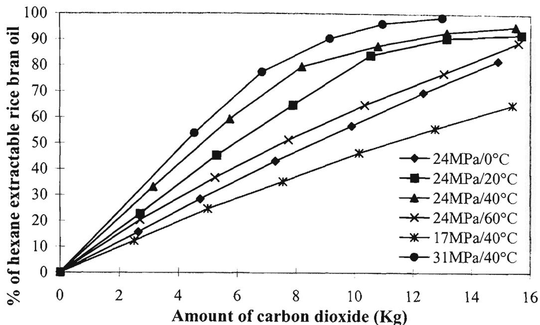
**Figure 2.2.** Extraction of oil from rice bran by dense CO<sub>2</sub> at different pressures and temperatures (CO<sub>2</sub> flow rate, average of 2.5 Kg/h). Single points represent the mean values of data from duplicate or triplicate experiments.
