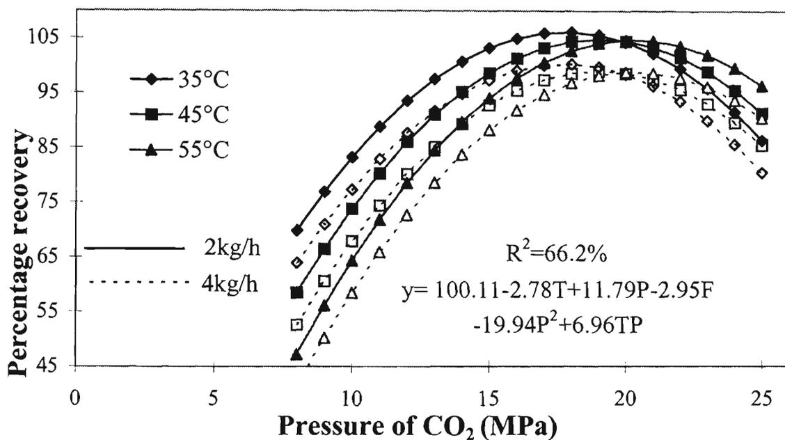
**Fig 5.16. Percentage recovery of total feed decanal using 5 kg CO<sub>2</sub>, isotherms as functions of CO<sub>2</sub> pressure (modelled), T, P and F in this model represent the coded temperature, pressure and flowrate of CO<sub>2</sub>. R<sup>2</sup> is the percentage of variance accounted for by the model.**
