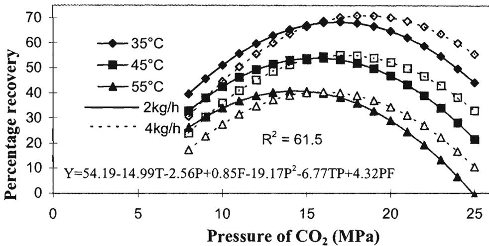
Fig 5.28. Percentage recovery of aldehydes 10 times concentrated as the feed (ald/ter) (modelled), isotherms as functions of pressure. T, P and F in this model represent the coded temperature, pressure and flowrate of CO<sub>2</sub>. R<sup>2</sup> is the percentage of variance accounted for by the model.
