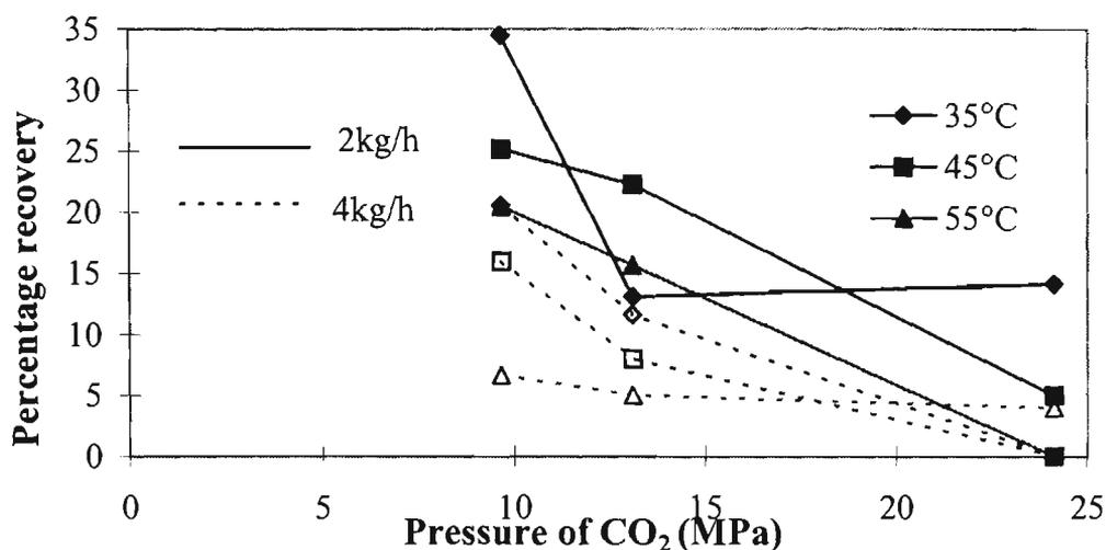
Fig 5.40. Percentage recovery of alcohols 15 times concentrated as the feed (alc/ter) (observed), isotherms as functions of pressure.
