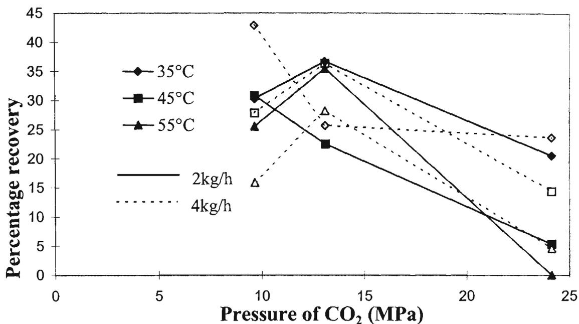
Fig.5.36. Percentage recovery of aldehydes 15 times concentrated as the feed (ald/ter) (observed), isotherms as functions of pressure.
