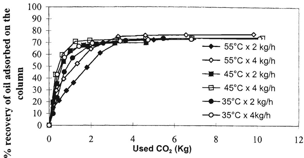
Fig 5.4. Effect of temperature and flowrate on the total orange oil recovery of CO<sub>2</sub> desorption at 9.66 MPa.
