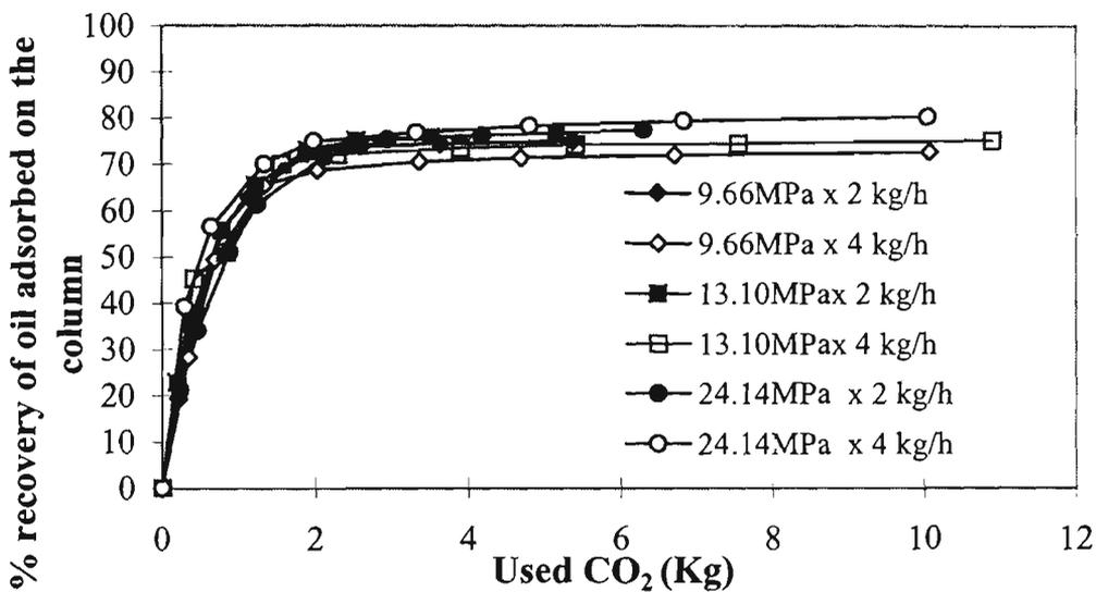
Fig 5.8 Effect of pressure and flowrate on the total orange oil recovery of CO<sub>2</sub> desorption at 45°C
