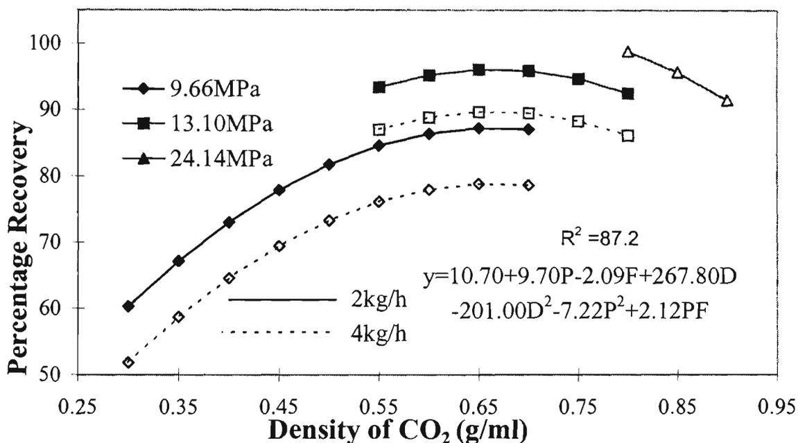
**Fig 5.20. Percentage recovery of total feed aldehydes using 5 kg CO<sub>2</sub>, isobars as functions of CO<sub>2</sub> density (modelled). P and F in this model represent the coded value of pressure and flowrate of CO<sub>2</sub> and D is the density of CO<sub>2</sub>. R<sup>2</sup> is the percentage of variance accounted for by the model. At 24.14 MPa the two recovery curves overlap.**
