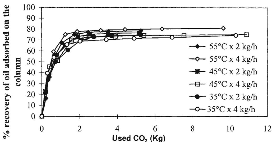
Fig 5.5 Effect of temperature and flowrate on the total orange oil recovery of CO<sub>2</sub> desorption at 13.10 MPa.
