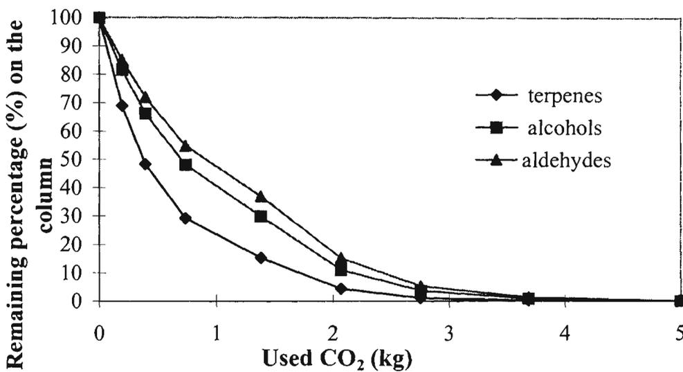
Fig 5.11. Desorption curves of major classes of orange oil constituents at 13.1MPa, 35°C and 2kg/h of CO<sub>2</sub>.
