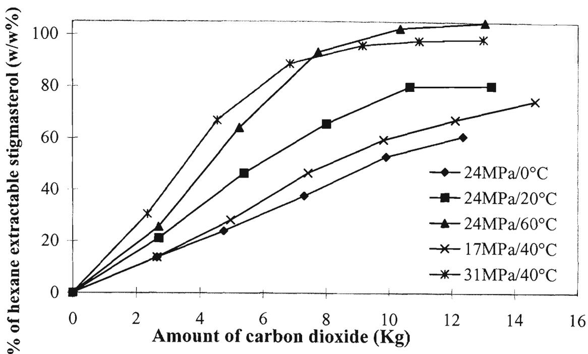
Figure 2.8. Extraction of stigmasterol from rice bran by dense CO<sub>2</sub> at different temperatures and pressures (CO<sub>2</sub> flow rate, average of 2.5 Kg/h).
