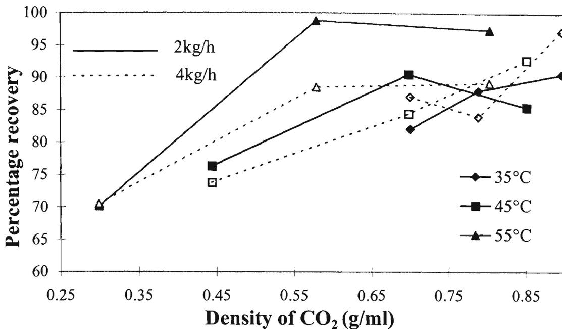
**Fig 5.23. Percentage recovery of total feed alcohols using 5 kg CO<sub>2</sub>, isotherms as functions of CO<sub>2</sub> density (observed).**
