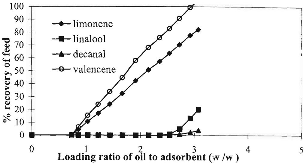
**Fig 4.9. Breakthrough curve of orange oil (pumping - 0.96 g oil/min) on Aluminium Oxide (14.70 g).**
