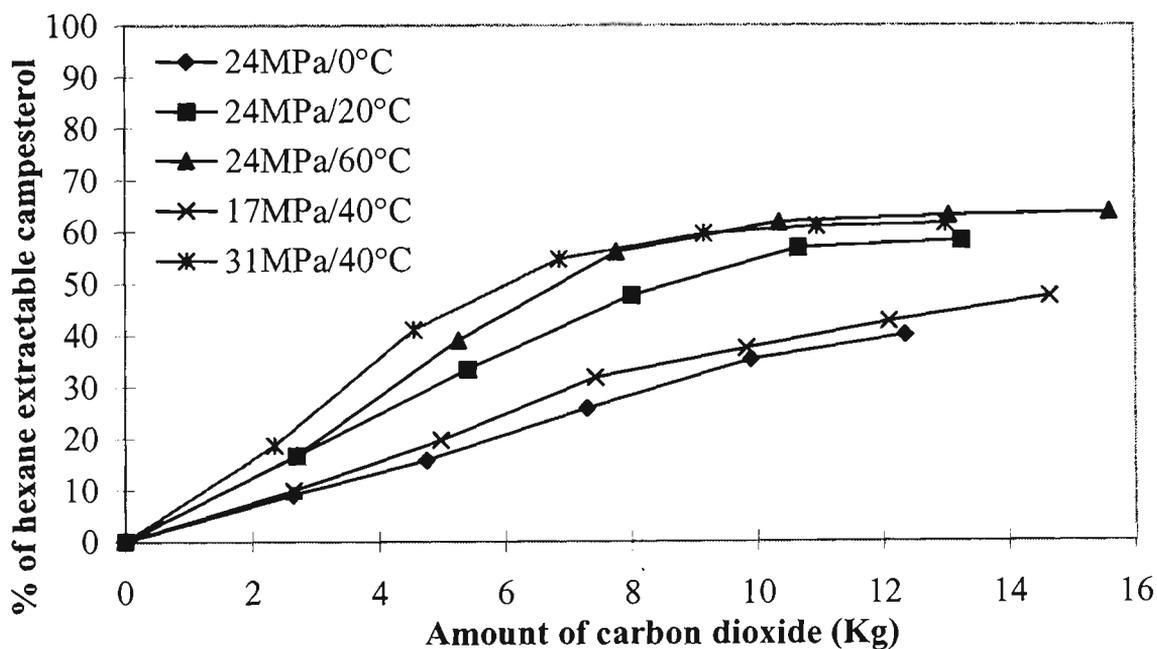
Figure 2.7. Extraction of campesterol from rice bran by dense CO<sub>2</sub> at different temperatures and pressures (CO<sub>2</sub> flow rate, average of 2.5 Kg/h).
