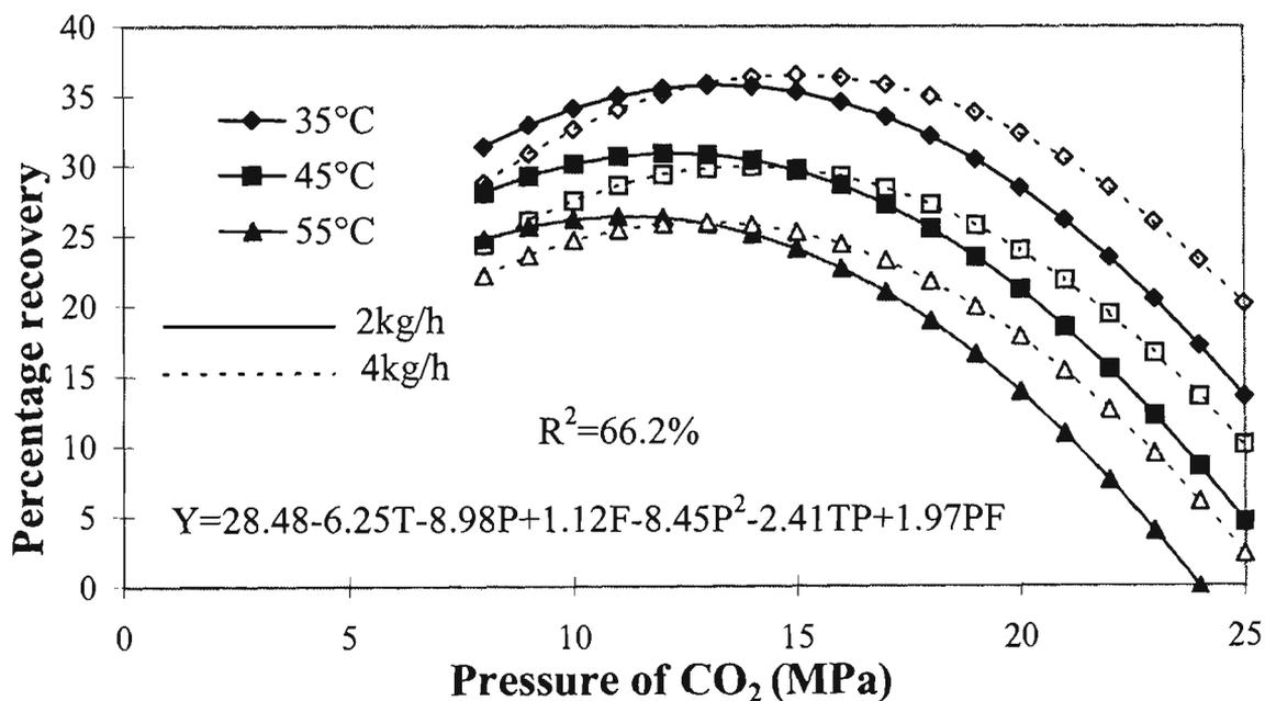
Fig. 5.37. Percentage recovery of aldehydes 15 times concentrated as the feed(ald/ter) (modelled), isotherms as functions of pressure of CO<sub>2</sub>. T, P and F in this model represent the coded temperature, pressure and flowrate of CO<sub>2</sub>. R<sup>2</sup> is the percentage of variance accounted for by the model.
