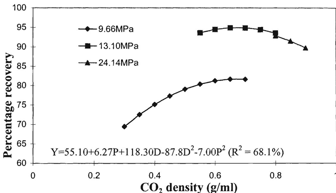
**Fig. 5.26. Percentage recovery of total feed alcohols using 5 kg CO<sub>2</sub>, isobars as functions of density (modelled). P and D in this model represent the coded value of pressure and density of CO<sub>2</sub>. R<sup>2</sup> is the percentage of variance accounted for by the model. Flowrate is not a variable in this model.**
