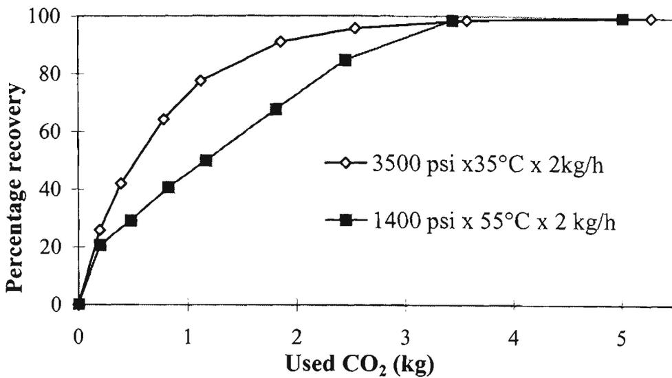
Fig 5.10. Percentage recovery yield of Valencia orange oil refined with CO<sub>2</sub> and Silica gel.
