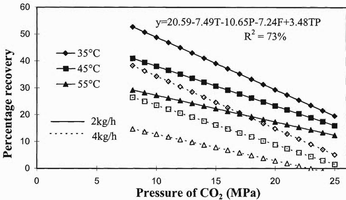
Fig 5.33. Percentage recovery of alcohols 10 times concentrated as the feed (alc/ter, modelled), isotherms as functions of pressure. T, P and F in this model represent the coded temperature, pressure and flowrate of used CO<sub>2</sub>. R<sup>2</sup> is the percentage of variance accounted for by the model.
