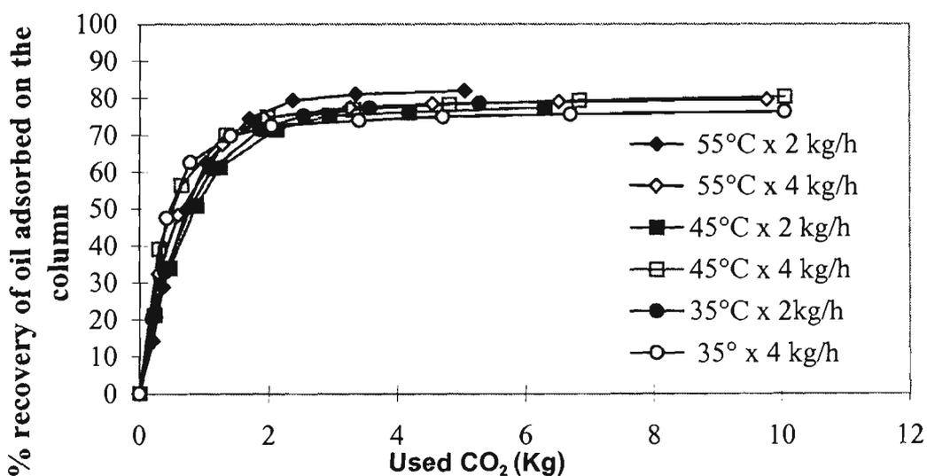
Fig 5.6 Effect of temperature and flowrate on the total orange oil recovery of CO<sub>2</sub> desorption at 24.14 MPa.
