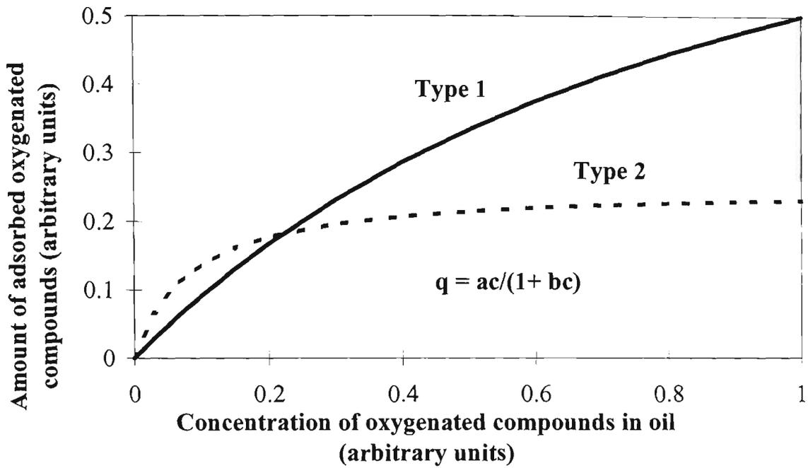
Fig. 4.2. Typical adsorption isotherms,  $q$  is the amount of compound adsorbed,  $c$  is its concentration in the oil phase;  $a$  and  $b$  are constants (Wankat, 1987).
