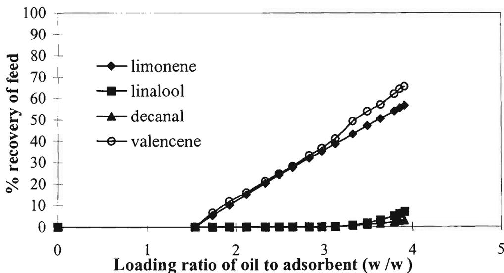
Fig. 4.8. Breakthrough curve of orange oil (20.31g) on Silica gel 60 (70-230 mesh, 5.20 g).
