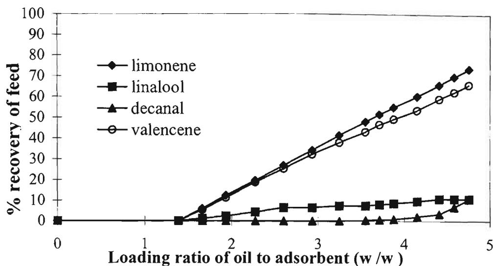
Fig. 4.6. Breakthrough curve of orange oil (31.32 g) on Silica gel (35-70 mesh, 6.59 g).
