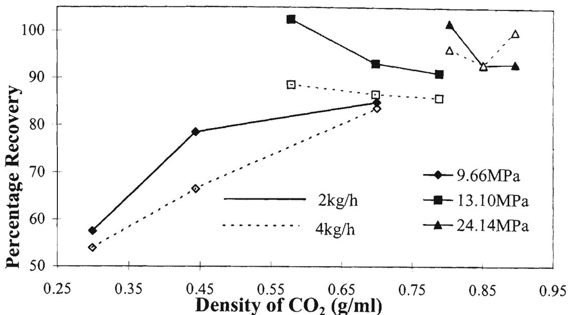
**Fig 5.19. Percentage recovery of total feed aldehydes using 5 kg CO<sub>2</sub>, isobars as functions of CO<sub>2</sub> density (observed).**
