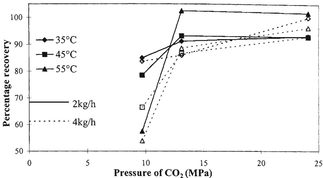
**Fig 5.13. Percentage recovery of total feed aldehydes using 5 kg CO<sub>2</sub>, isotherms as functions of CO<sub>2</sub> pressure (observed).**
