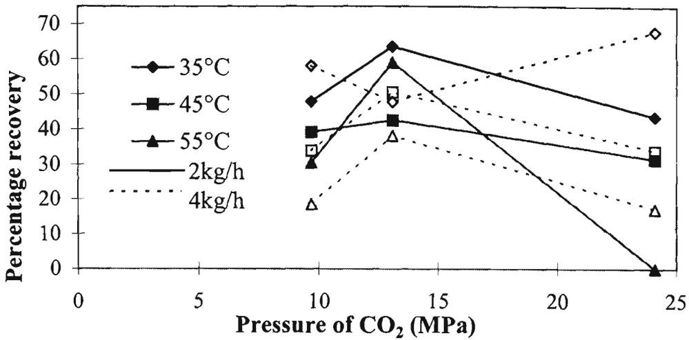
Fig 5.27. Percentage recovery of aldehydes 10 times concentrated as the feed (ald/ter) (observed), isotherms as functions of pressure.
