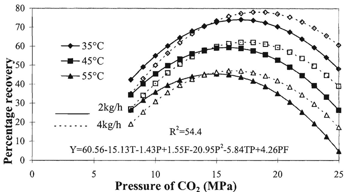
Fig 5.31. Percentage recovery of decanal 10 times concentrated as the feed (dec/lim) (modelled), isotherms as functions of pressure of CO<sub>2</sub>. T, P and F in this model represent the coded temperature, pressure and flowrate of CO<sub>2</sub>. R<sup>2</sup> is the percentage of variance accounted for by the model.
