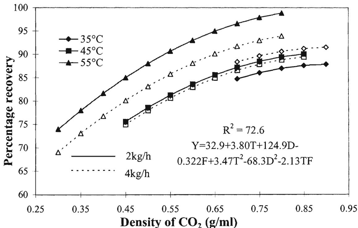
**Fig 5.24. Percentage recovery of total feed alcohols using 5 kg CO<sub>2</sub>, isotherms as functions of density (modelled). P and F in this model represent the coded pressure and flowrate of CO<sub>2</sub> and D is the density of CO<sub>2</sub>. R<sup>2</sup> is the percentage of variance accounted for by the model.**
