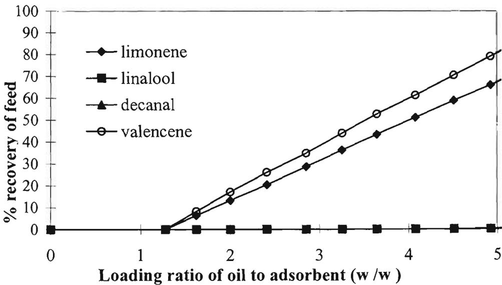
**Fig. 4.11. Breakthrough curve of orange oil (pumping- 0.65 g/min) on Silica gel (70-230 mesh, 14.82 g). The two breakthrough curves of decanal and linalool overlap each other.**
