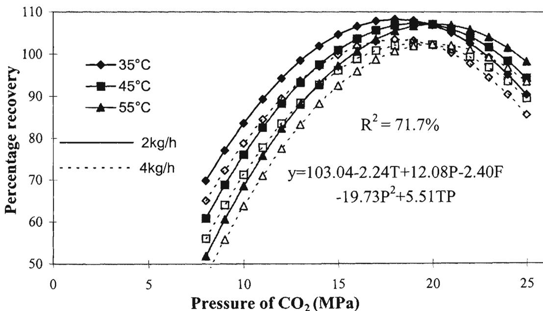
**Fig 5.14. Percentage recovery of total feed aldehydes using 5 kg CO<sub>2</sub>, isotherms as functions of CO<sub>2</sub> pressure (modelled). T, P and F in this model represent the coded temperature, pressure and flowrate of CO<sub>2</sub>. R<sup>2</sup> is the percentage of variance accounted for by the model.**
