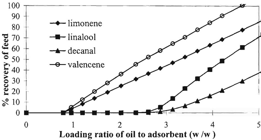
**Fig. 4.10 Breakthrough curve of orange oil (pumping - 0.70g oil/min) on Aluminium Oxide (14.84g).**
