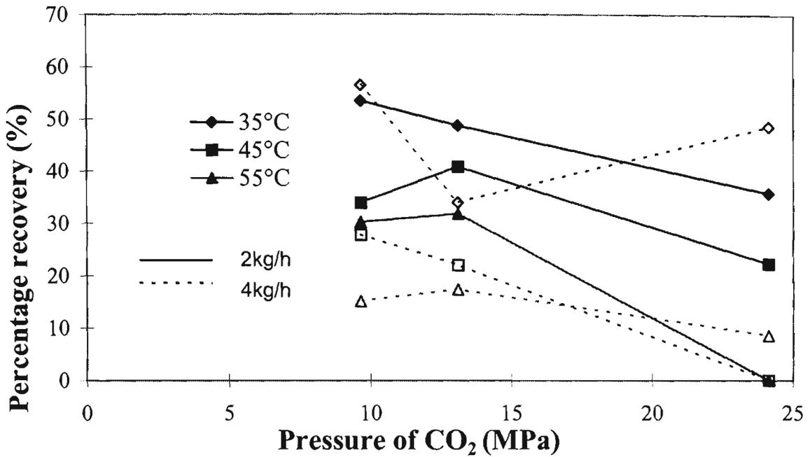
Fig. 5.34. Percentage recovery of linalool 10 times concentrated as the feed (lin/lim, observed), isotherms as functions of pressure.
