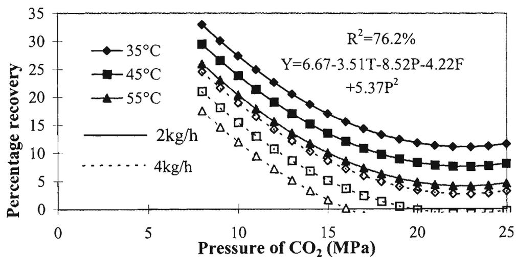
Fig 5.41. Percentage recovery of alcohols 15 times concentrated as the feed (alc/ter) (modelled), isotherms as functions of pressure of CO<sub>2</sub>. T, P and F in this model represent the coded temperature, pressure and flowrate of CO<sub>2</sub>. R<sup>2</sup> is the percentage of variance accounted for by the model.
