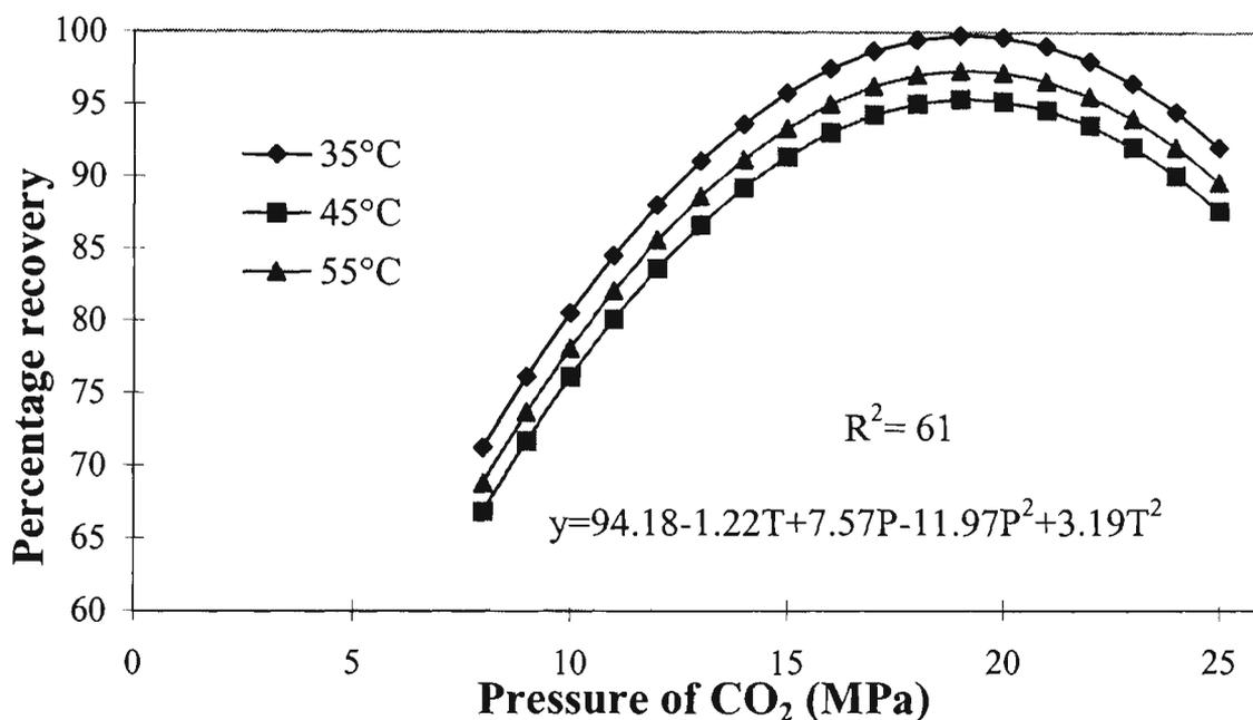
**Fig 5.22. Percentage recovery of total feed alcohols using 5 kg CO<sub>2</sub>, isotherms as functions of pressure (modelled). P and T in this model represent the coded pressure and temperature of CO<sub>2</sub>. Flowrate is not a variable in this model. R<sup>2</sup> is the percentage of variance accounted for by the model.**
