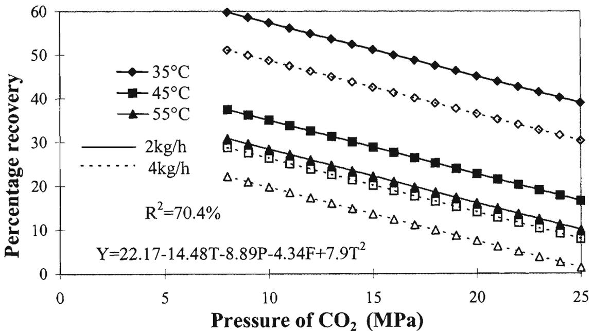
Fig. 5.35. Percentage recovery of linalool 10 times concentrated as the feed (lin/lim)(modelled), isotherms as functions of pressure of CO<sub>2</sub>. T, P and F in this model represent the coded temperature, pressure and flowrate of CO<sub>2</sub>. R<sup>2</sup> is the percentage of variance accounted for by the model.
