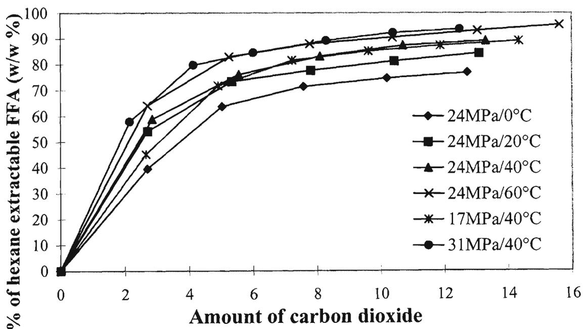
Figure 2.4. Extraction of total FFA from rice bran by dense CO<sub>2</sub> at different temperatures and pressures (CO<sub>2</sub> flow rate, average of 2.5 Kg/h). Single points represent the mean values of data from duplicate or triplicate experiments.
