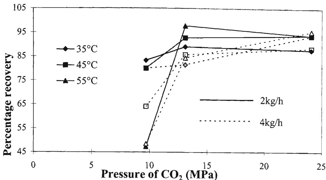
**Fig. 5.15. Percentage recovery of total feed decanal using 5 kg CO<sub>2</sub>, isotherms as functions of CO<sub>2</sub> pressure (observed).**
