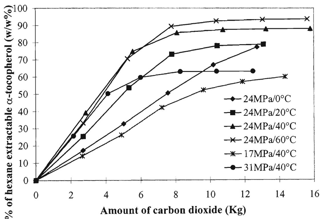
**Figure 2.5. Extraction of  $\alpha$ -tocopherol from rice bran by dense CO<sub>2</sub> at different temperatures and pressures (CO<sub>2</sub> flow rate, average of 2.5 Kg/h). Single points represent the mean values of data from duplicate or triplicate experiments.**
