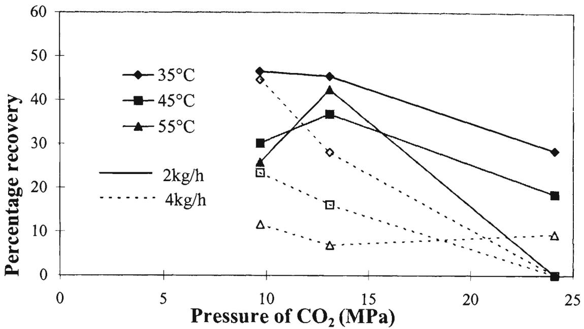
Fig 5.32. Percentage recovery of alcohols 10 times concentrated as the feed (alc/ter) (observed), isotherms as functions of pressure.
