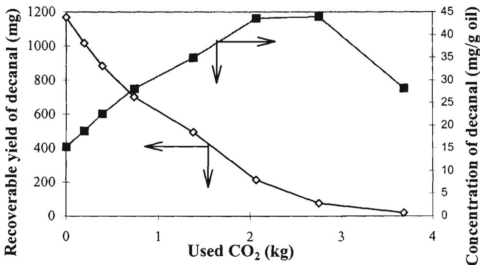
Fig. 5.12. Decanal in remaining adsorbate during extraction at 13.1MPa, 35°C and 2kg/h of CO<sub>2</sub>.
