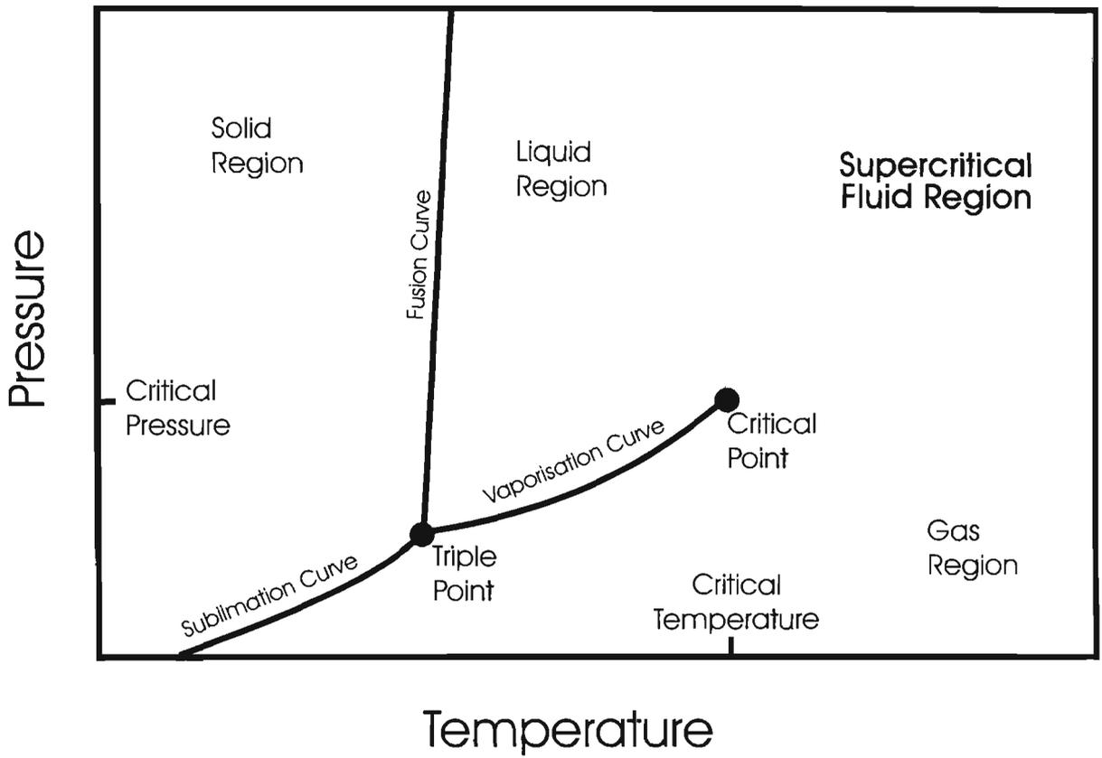
Figure 1.1 Theoretical pressure-temperature phase diagram for a pure compound
