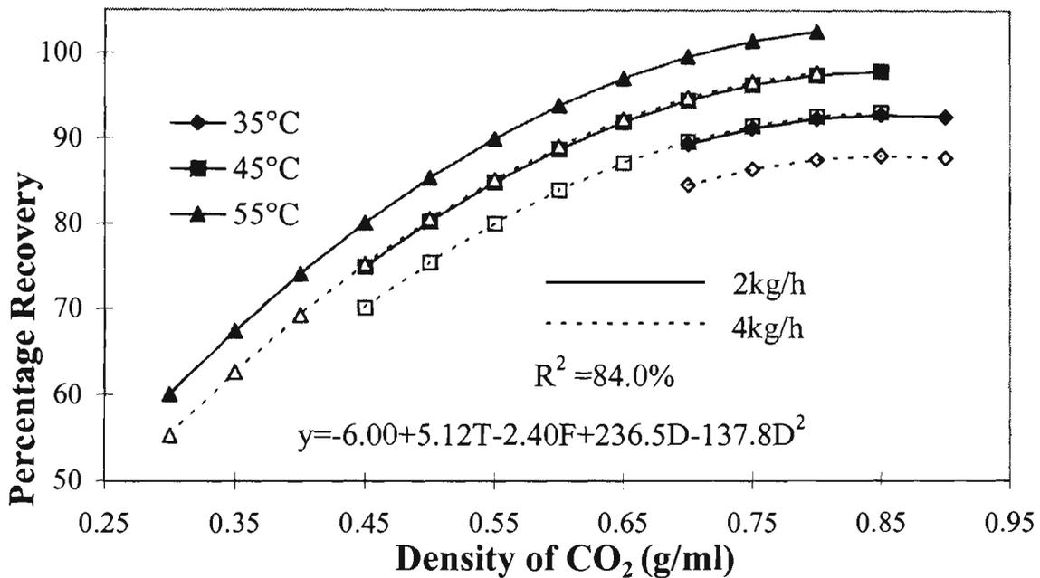
**Fig 5.18. Percentage recovery of total feed aldehydes using 5 kg CO<sub>2</sub>, isotherms as functions of CO<sub>2</sub> density (modelled), T, and F in this model represent the coded temperature and flowrate of CO<sub>2</sub> and D is the density of CO<sub>2</sub>. R<sup>2</sup> is the percentage of variance accounted for by the model.**
