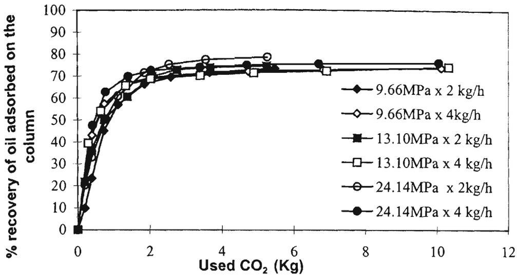
Fig 5.7. Effect of pressure and flowrate on the total orange oil recovery of CO<sub>2</sub> desorption at 35°C.
