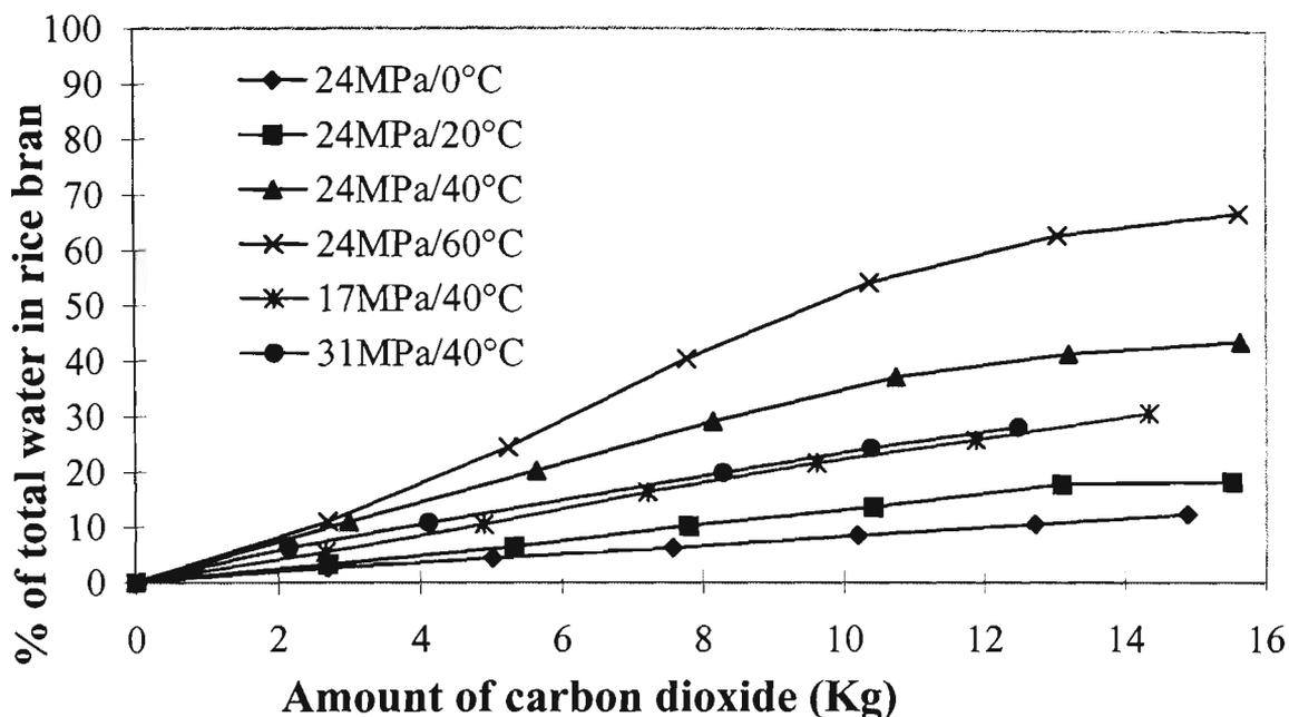
Figure 2.3. Extraction of water from rice bran by dense CO<sub>2</sub> at different temperatures and pressures (CO<sub>2</sub> flow rate, average of 2.5 Kg/h). Single points represent the mean values of data from duplicate or triplicate experiments.
