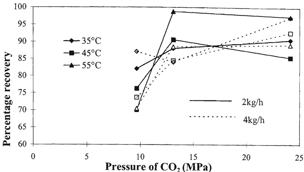
**Fig 5.21. Percentage recovery of total feed alcohols using 5 kg CO<sub>2</sub>, isotherms as functions of pressure (observed).**
