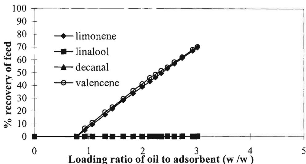
Fig. 4.7. Breakthrough curve of orange oil (16.25 g) on Aluminium Oxide (5.39 g). The two breakthrough curves of decanal and linalool overlap each other.
