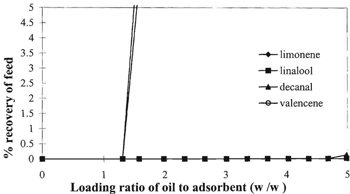
**Fig.4.13. Breakthrough curve of orange oil (pumping- 0.85g oil/min) on Silica gel (70-230 mesh, 14.95 g), magnified, the two steeply rising lines represent breakthrough curves of limonene and valencene.**
