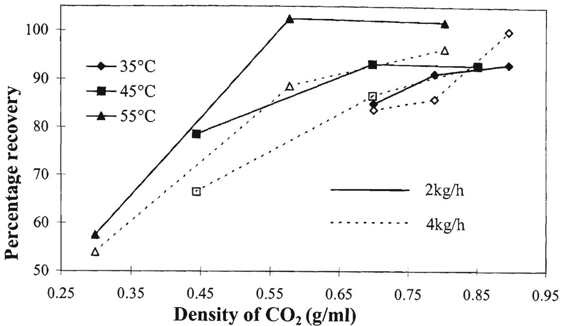
**Fig. 5.17. Percentage recovery of total feed aldehydes using 5 kg CO<sub>2</sub>, isotherms as functions of CO<sub>2</sub> density (observed).**
