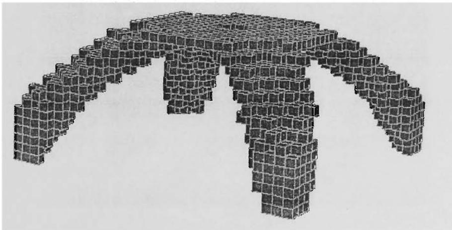
Fig. 4.16. Topology design (stress-based optimisation).
