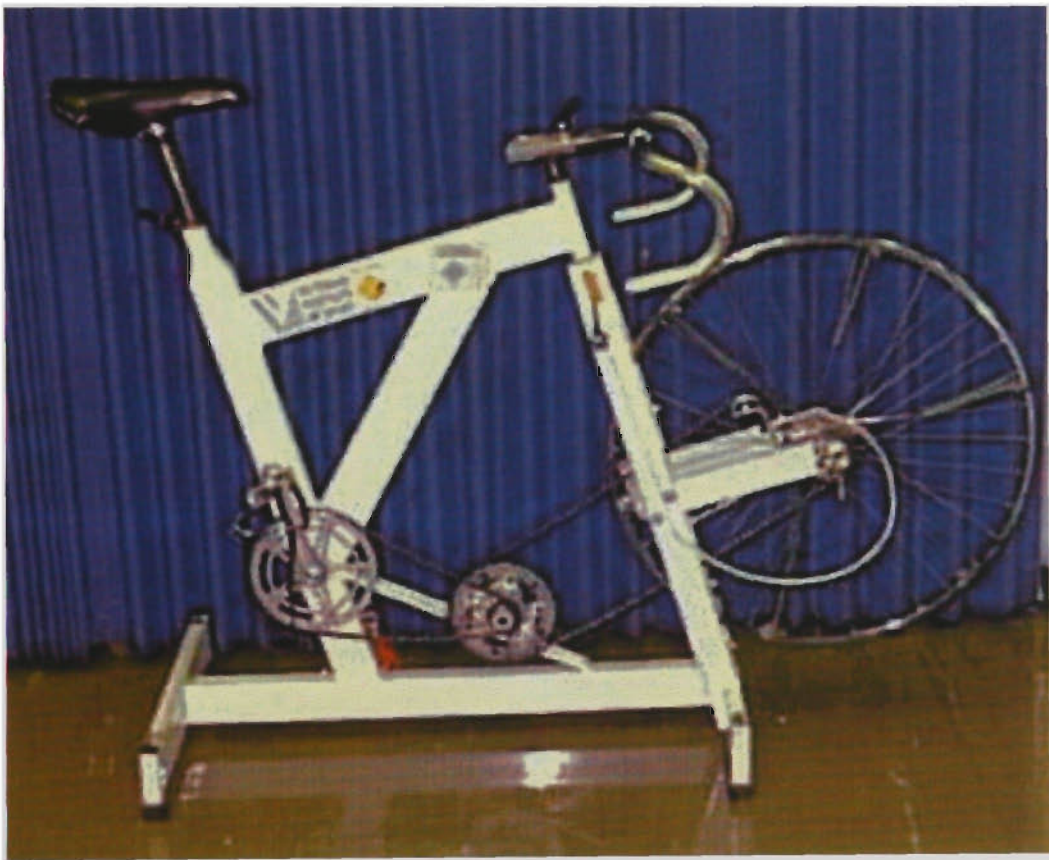
Figure 5.2 A locally manufactured air-braked ergometer used by the Victorian Institute of Sport
