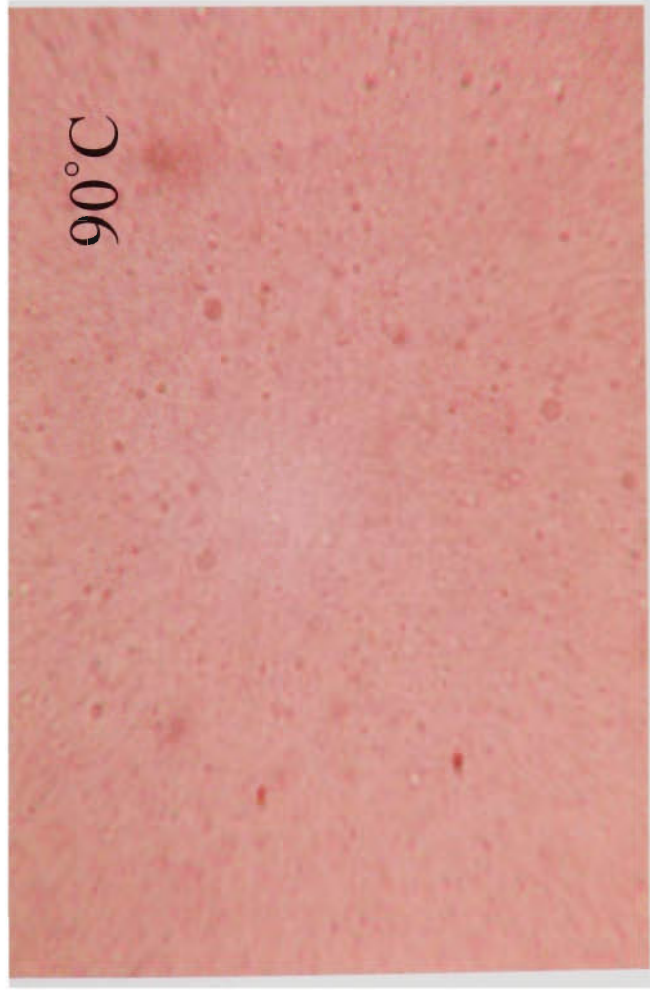
Figure 11.4.12 The effect of heating temperature on maltodextrin Maltrin M040 starch granules as observed under a light microscope.
