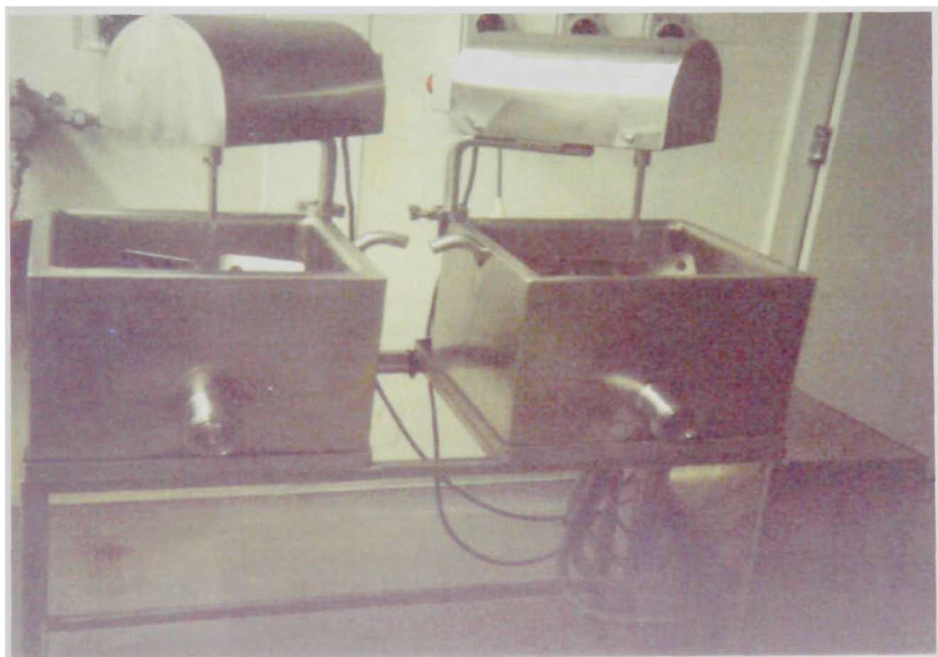
Figure 3.4 Two laboratory scale cheese vats used for making mozzarella cheese.
