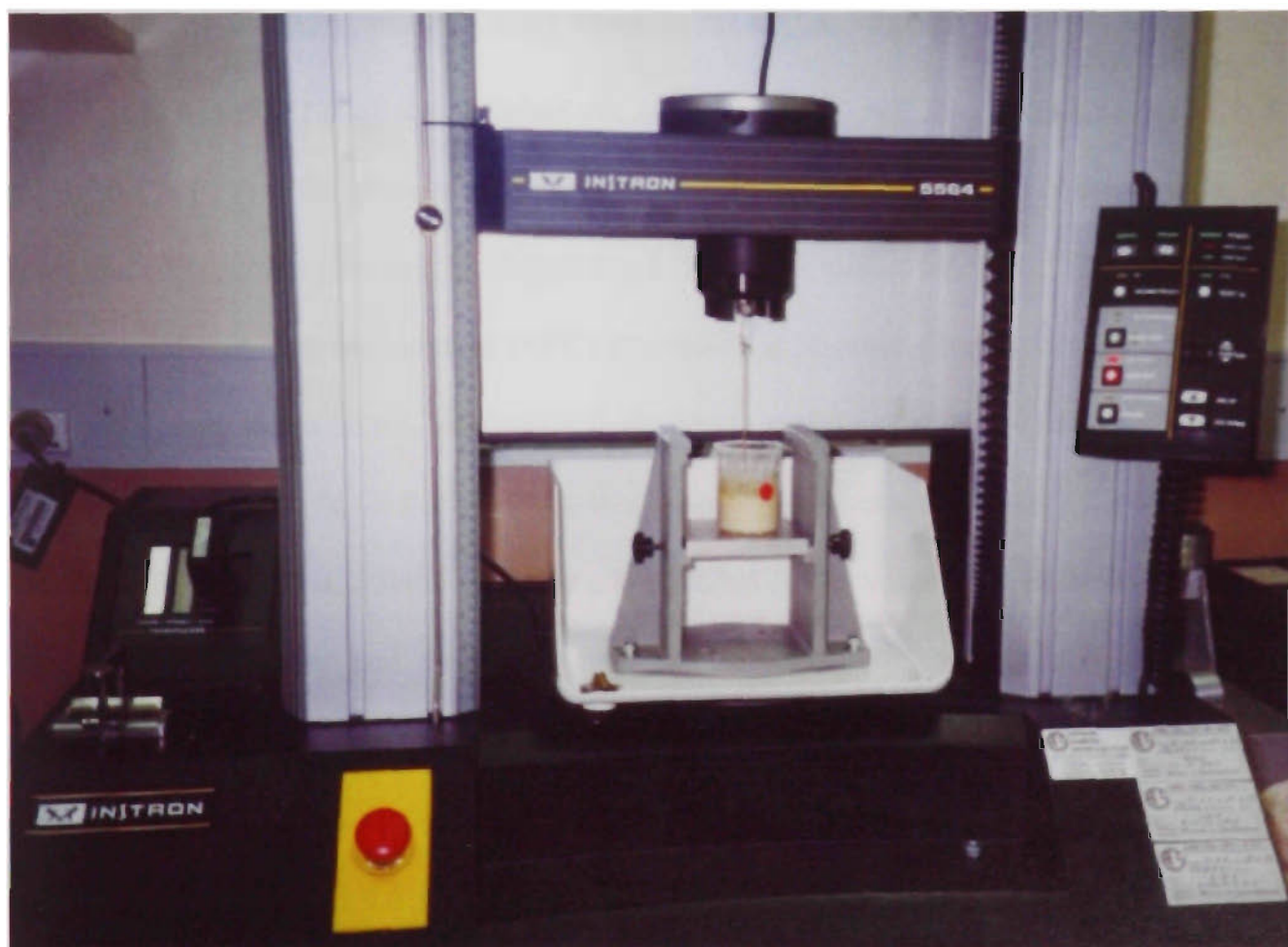
Figure 3.10 Set-up of an experimental mozzarella cheese sample tempered to 60°C for conducting the stretch test.
