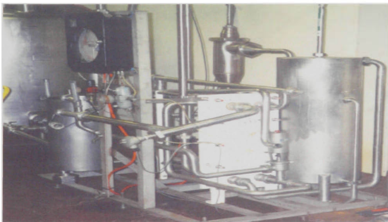
Figure 3.3 A pilot scale HTST pasteuriser used for pasteurising milk.
