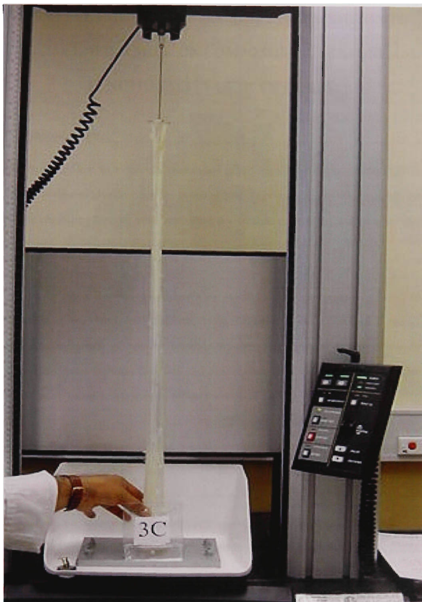
Figure 10.4.13 A typical image of stretched Versagel based cheese stored for 40 d analysed using the stretch test.
