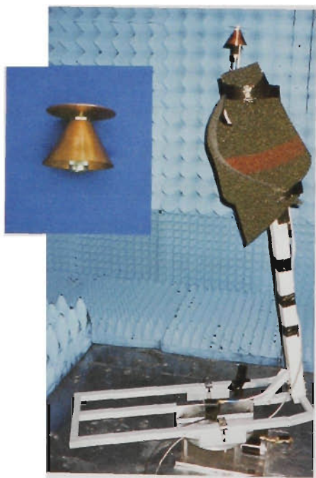
FIGURE C.5 Discone on test in the anechoic chamber at the University of Bristol
