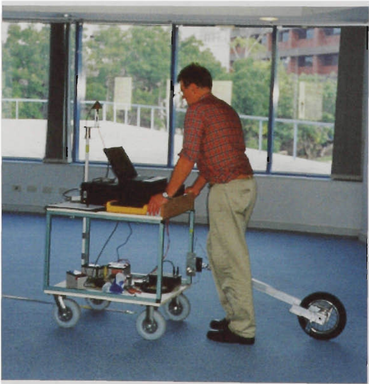
FIGURE B.45 Receiver on a trolley - with wheel trigger
