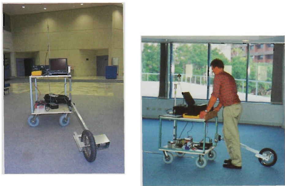
FIGURE 3.32. Receiver on trolley with distance triggering wheel
