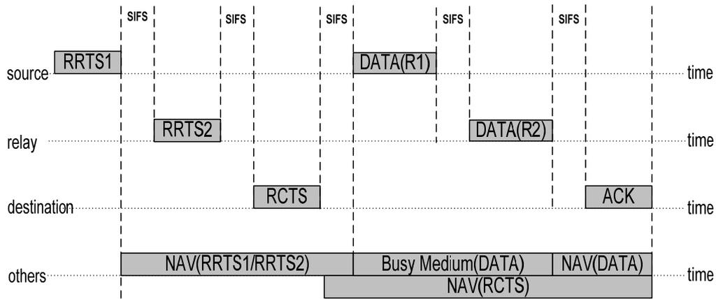
Figure 3.4: Carrier sensing scheme of rDCF.
