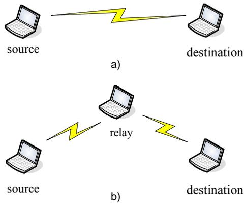
Figure 3.1: a) Slow Single hop direct transmission, b) Fast Dual-hop transmission via relay.
