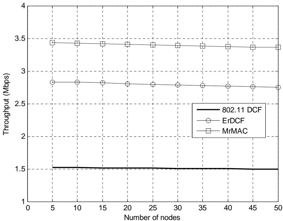
Figure 5.6: Saturation Throughput of MrMAC, ErDCF and 802.11 DCF.
