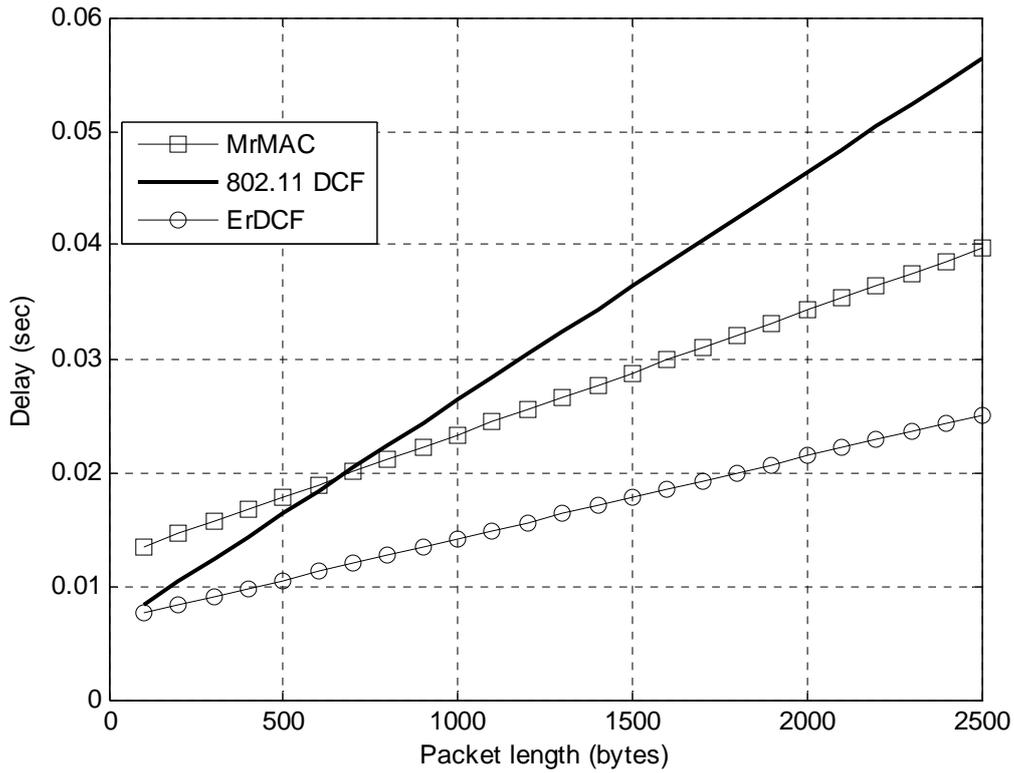
Figure 5.8: Delay of MrMAC, ErDCF802.11 DCF and 802.11 DCF for different packet lengths.
