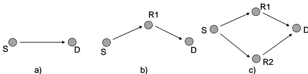
Figure 5.2: Modes of transmission: a) Direct transmission, b) Single relay transmission and c) Multiple relay transmission.
