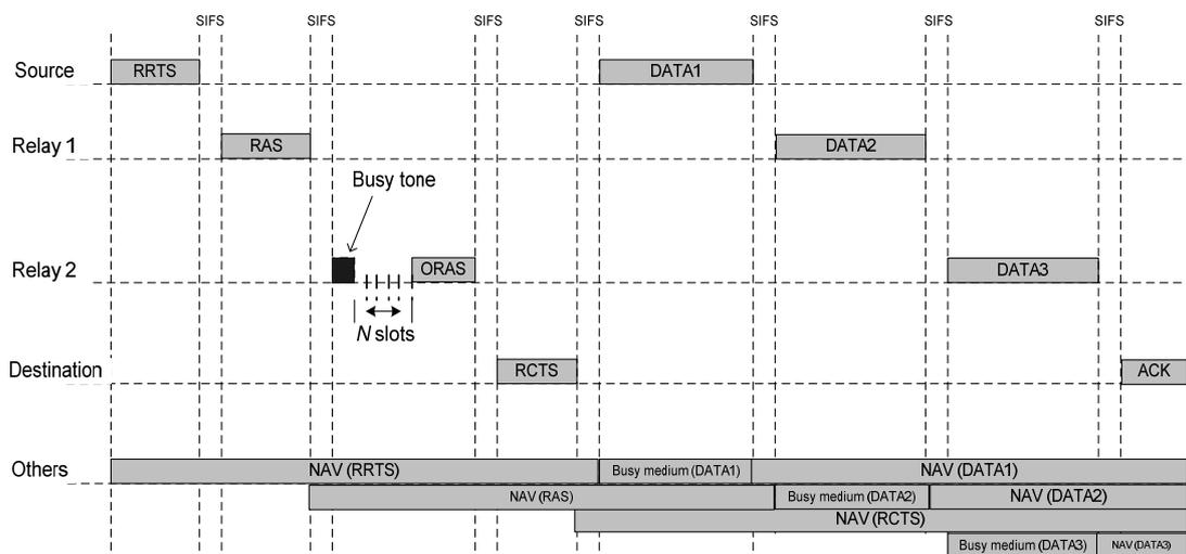
Figure 5.4: MrMAC carrier sensing scheme.
