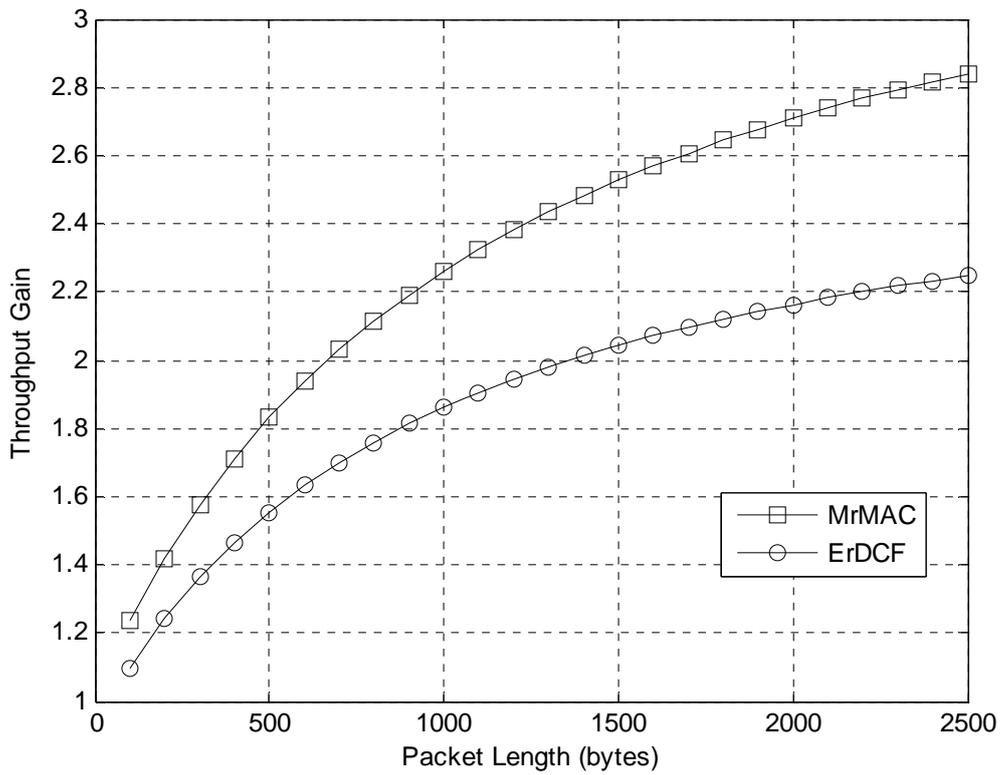
Figure 5.7: Throughput gain of MrMAC and ErDCF over 802.11 DCF for different packet lengths.
