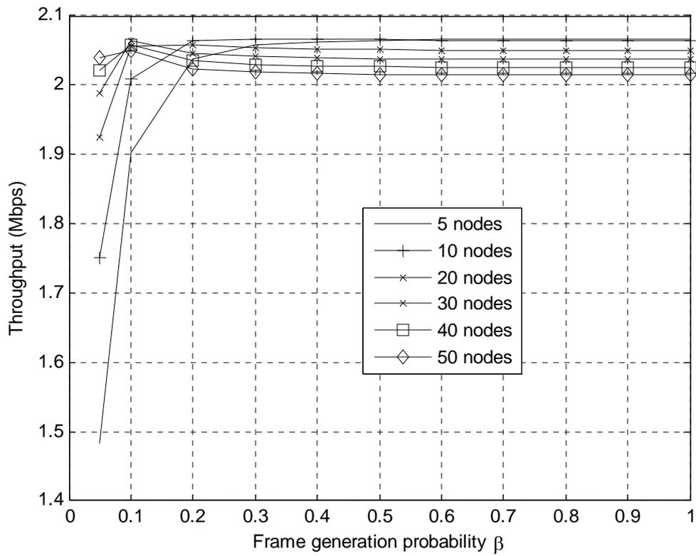
Figure 4.21: Non-saturated throughput of ErDCF(11, 5.5) in an ideal channel.
