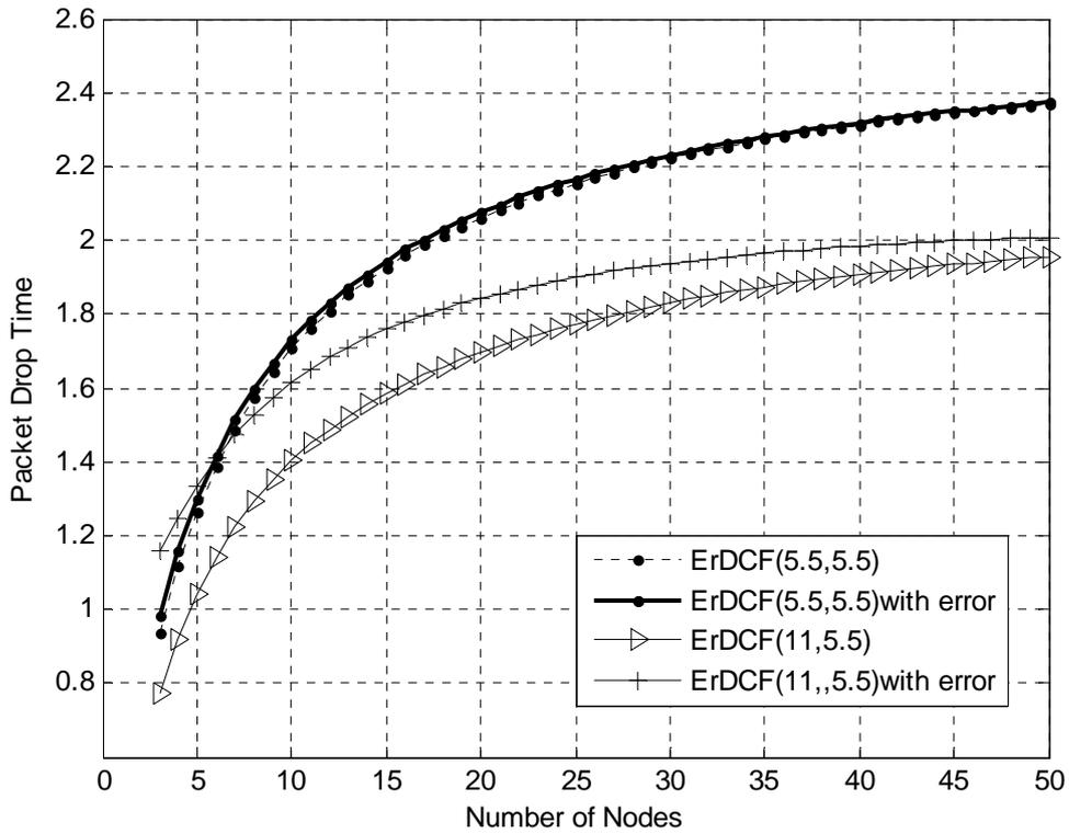
Figure 4.14: Comparing Packet drop time ErDCF ( $R_1, R_2$ ) in an ideal channel and with transmission errors.
