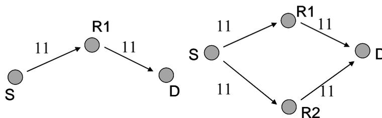
Figure 5.1: Single and Two relay (with 11 Mbps links) scenario in an ideal environment.
