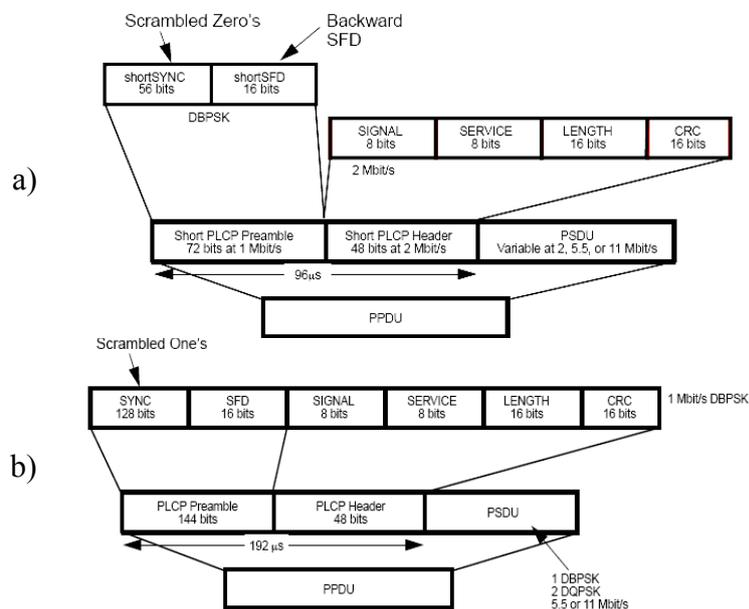
Figure 4.2: a) Short preamble format, and b) Long preamble format [14].
