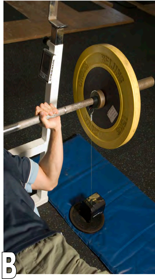
Figure 3.6: The Gymaware Set-up on a Weight Stack (left) and Free Barbell Bench Press (right). The Gymaware cord connected to the floor unit is attached to either the weight stack (A) or barbell (B). The floor unit is wired to an infrared transceiver, which sends the time and position data to the personal digital assistant via an infrared signal.
