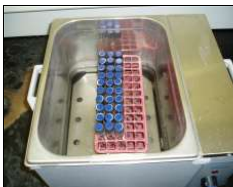
Figure 2.11: Photograph of leaf samples being digested in 17.5% (v/v) hydrogen peroxide in a water bath at 84°C.
