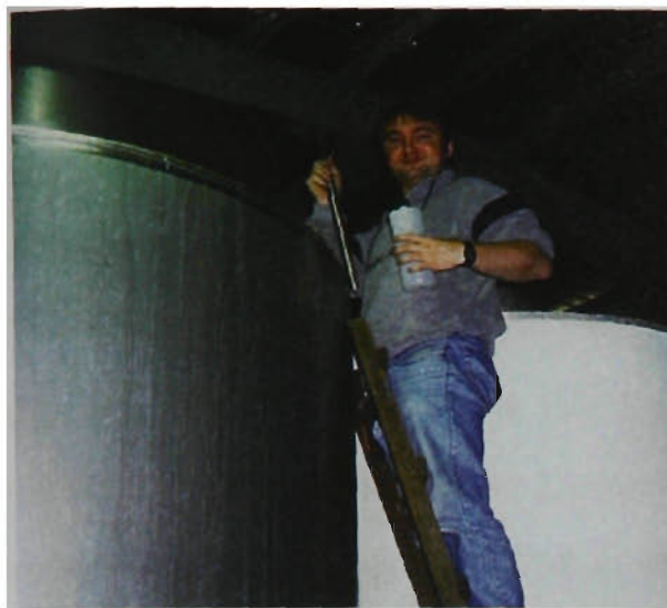
Figure 3.7 Sampling ferment from tank using washed stainless steel fife to decant into clean polyethylene bottle.
