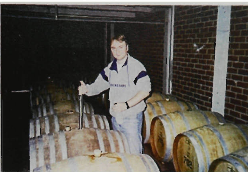
Figure 3.8 Sampling unfinished wine from barrel using washed stainless steel fife and collecting into clean polyethylene bottle.
