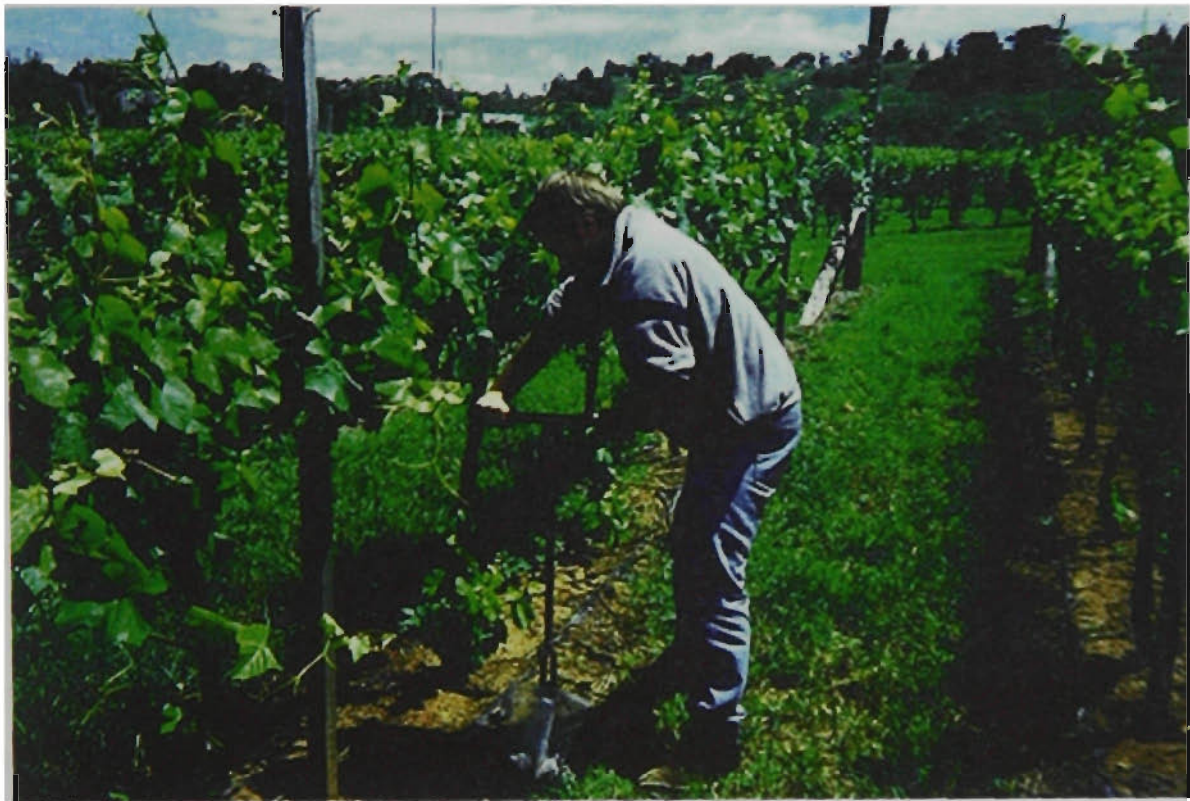
Figure 3.5 Photograph of the author showing use of stainless steel auger and sampling position relative to vine rows. Polyethylene sample bags appear at the author’s feet in the foreground.
