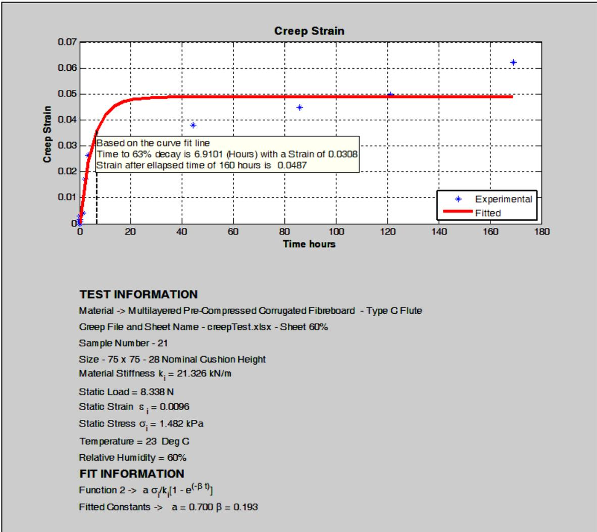
Figure 4.15 Creep Experimental and Simulation sample 21 at 60% RH using Equation 4.6
