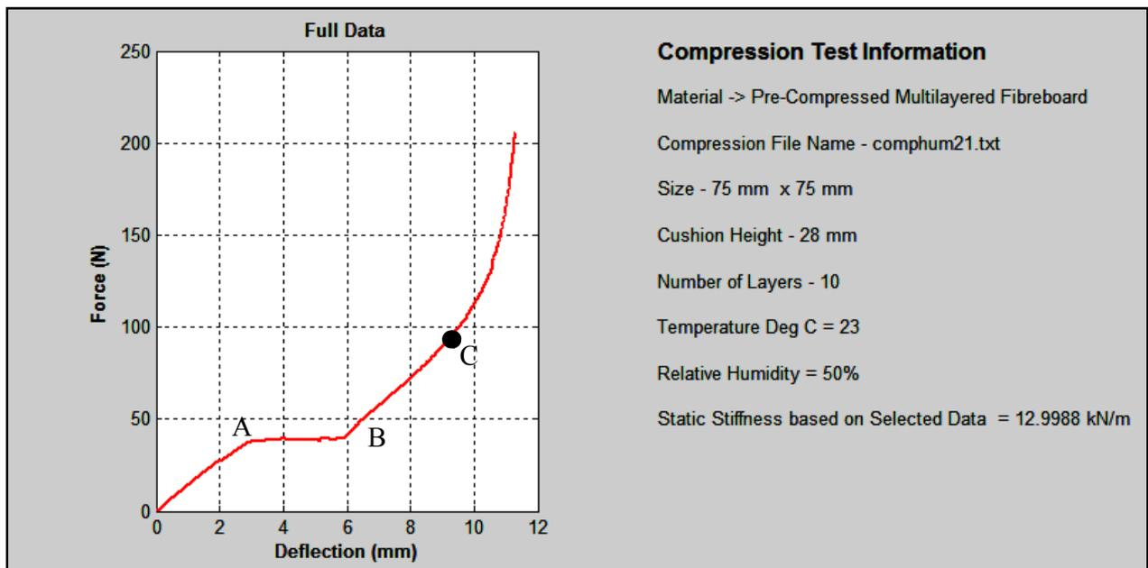
Figure 4.3 Typical Static Strain Test
