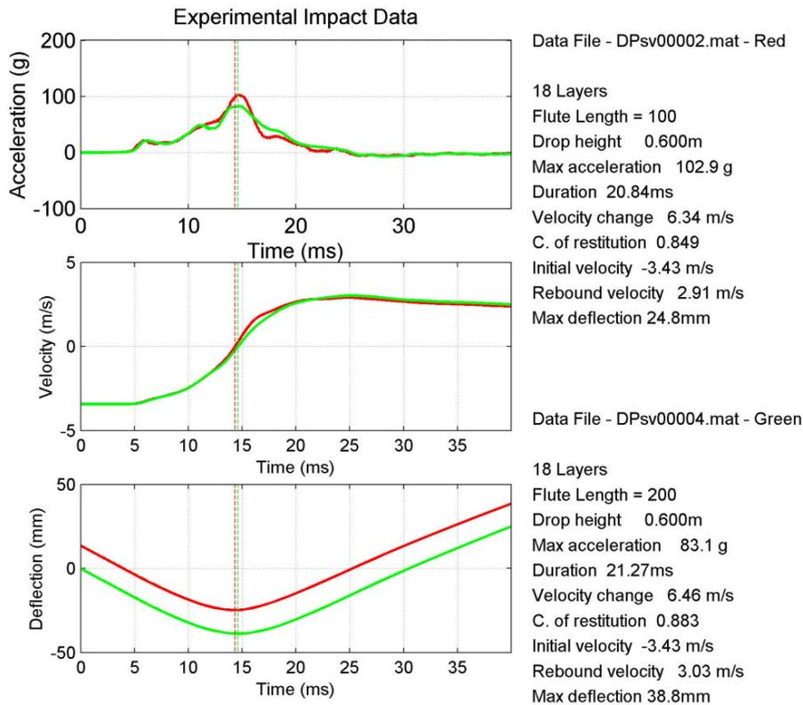
**Figure 1.2 Impact Behaviour of Pre-compressed Multilayered Fibreboard**
