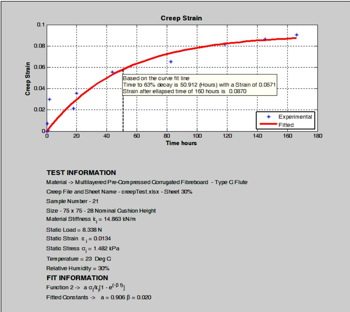
Figure 4.13 Creep Experimental and Simulation sample 21 at 30% RH using Equation 4.6
