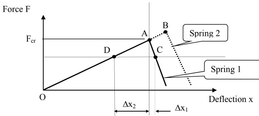
**Figure 2.2 Representation of two springs compressed to failure**
