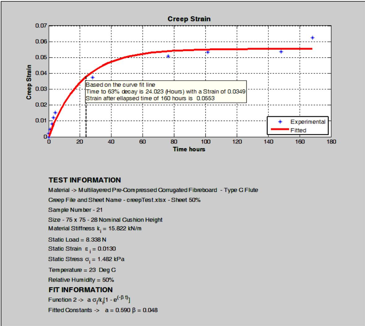
Figure 4.14 Creep Experimental and Simulation sample 21 at 50% RH using Equation 4.6
