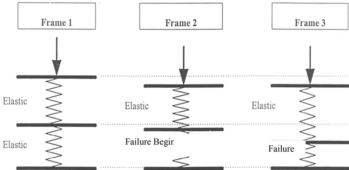
**Figure 2.1 Spring model representing two layers of corrugated fibreboard**
