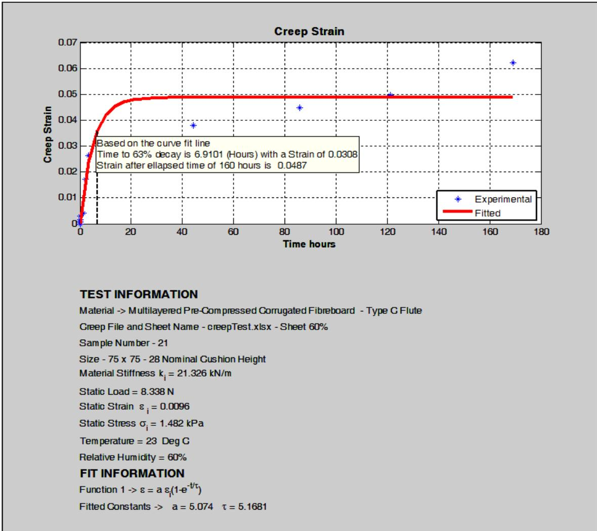
Figure 4.11 Creep Experimental and Simulation sample 21 at 60% RH using Equation 4.5
