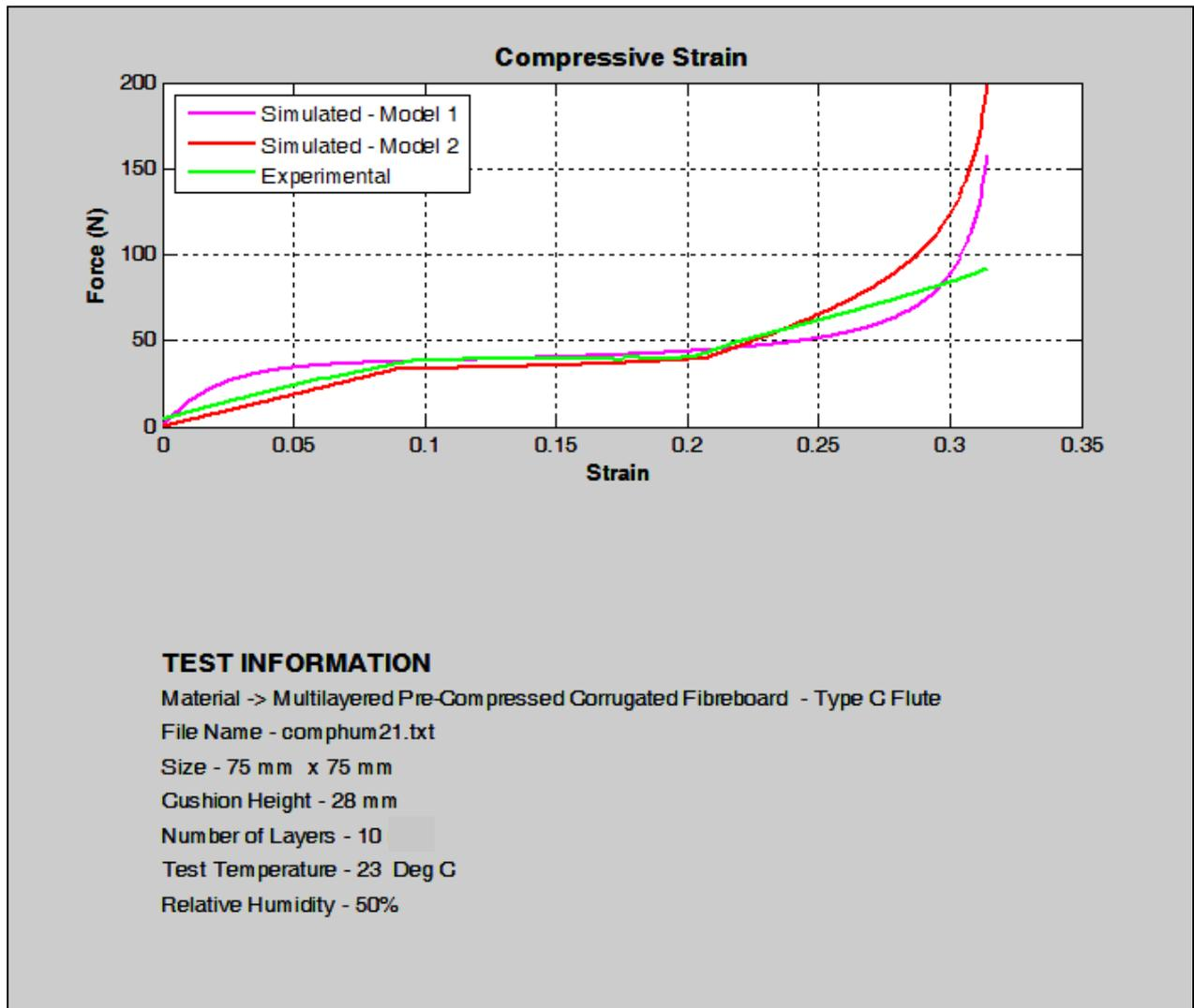
Figure 4.5 Compression and Simulation at 50% Humidity based on Equations 4.2 and 4.3
