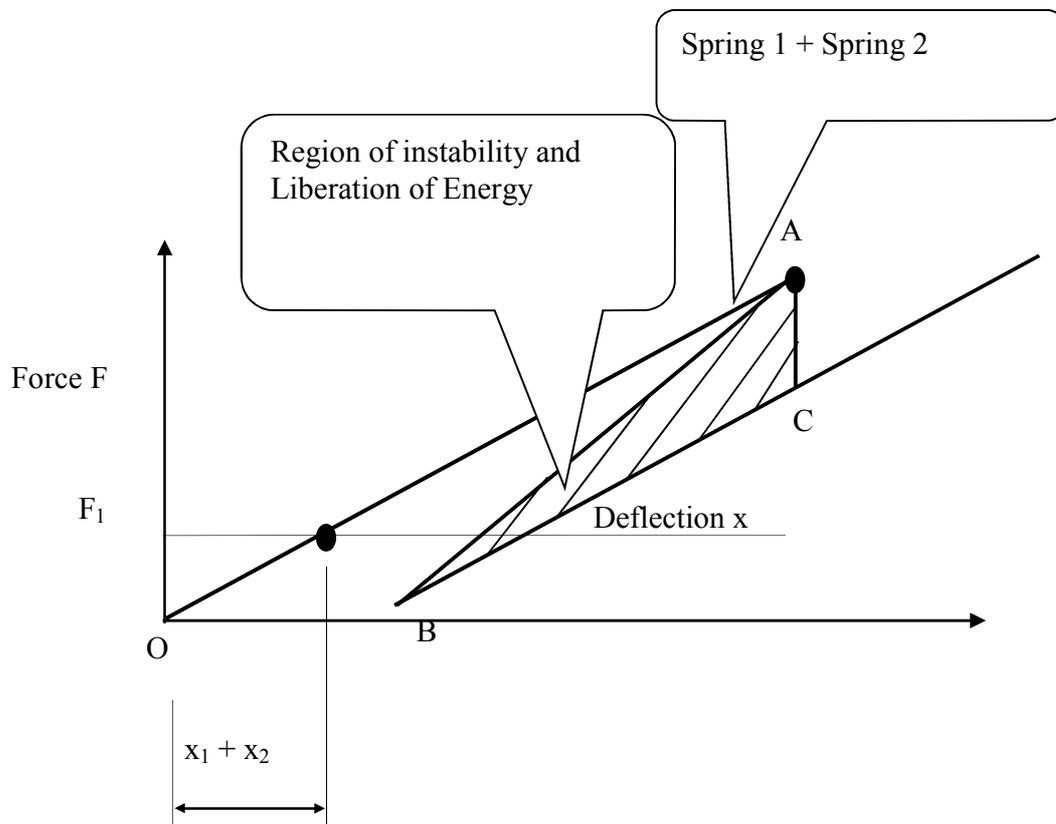
**Figure 2.3 The resulting Force v Deflection after failure of spring 1**
