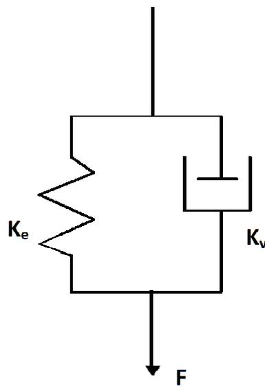
Figure 4.8 Voigt Model of Viscoelasticity
