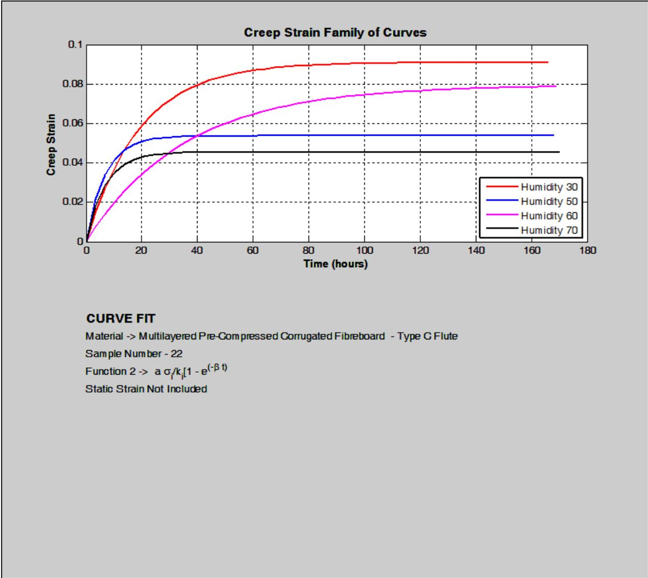
Figure 4.19 Simulated Curve Family for Sample 22 over the experimental Humidity Range, no Static Strain
