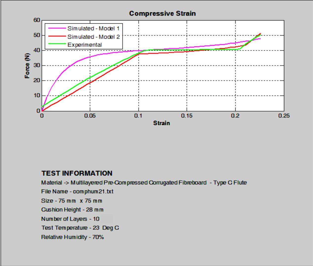
Figure 4.7 Compression and Simulation at 70% Humidity based on Equations 4.2 and 4.3
