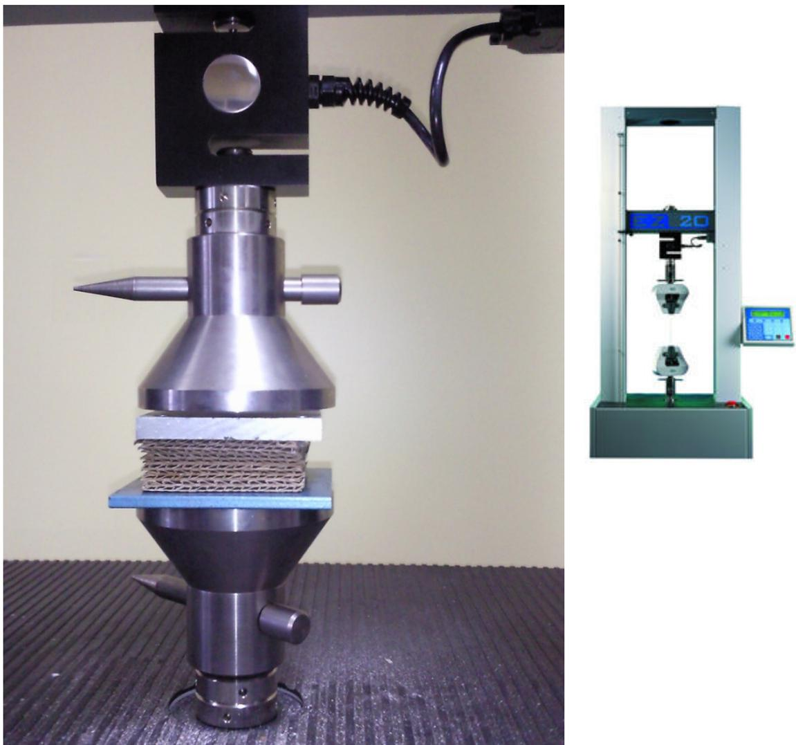
**Figure 3.1 Lloyd Universal Tensile Testing Machine Compressing Cushion**
