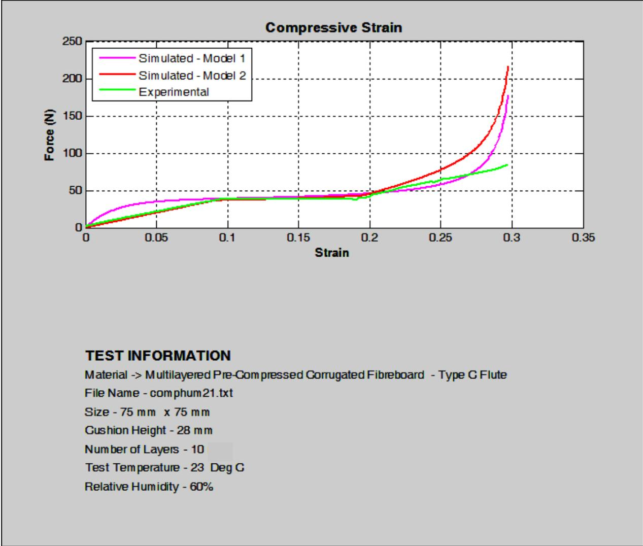
Figure 4.6 Compression and Simulation at 60% Humidity based on Equations 4.2 and 4.3
