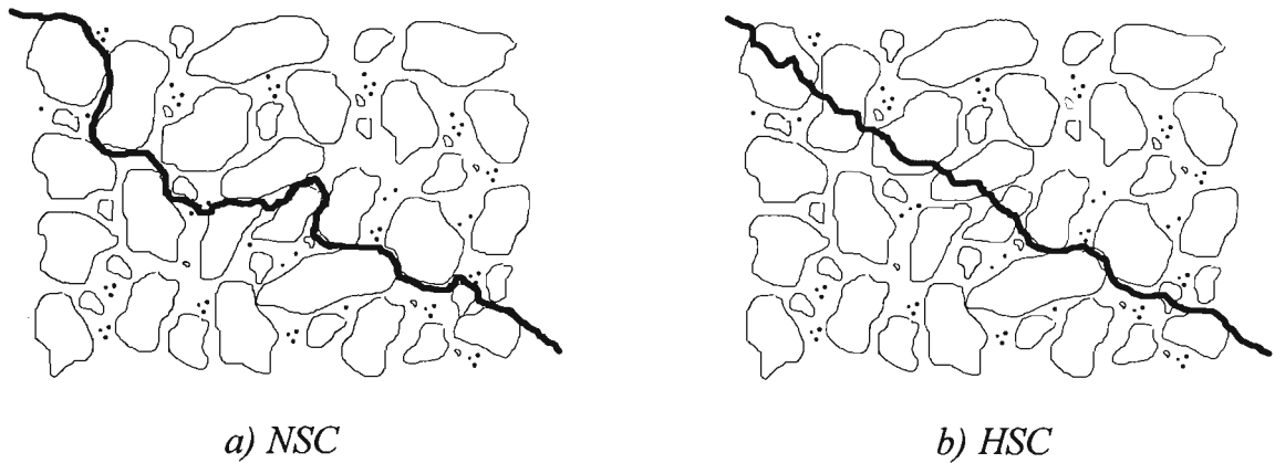
Figure 2.7: Shear crack patterns in normal strength and high strength concretes.
