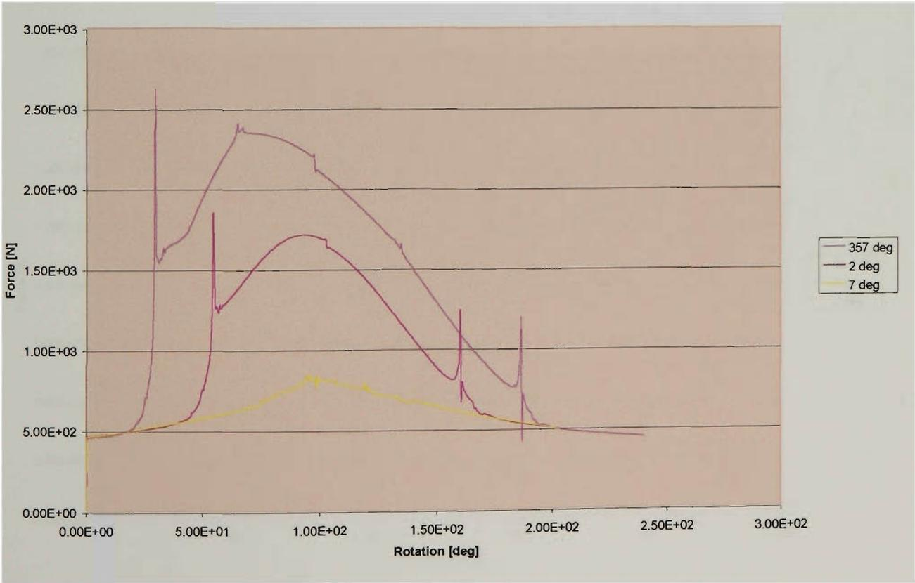
Figure 4.54 – Gudgeon Pin to Guideshaft Force at 9000 degrees/sec
