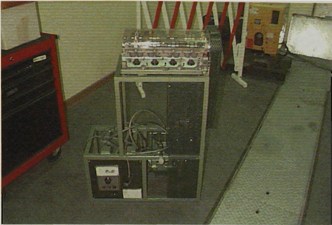
Figure 3.1 – Cylinder head test rig.
