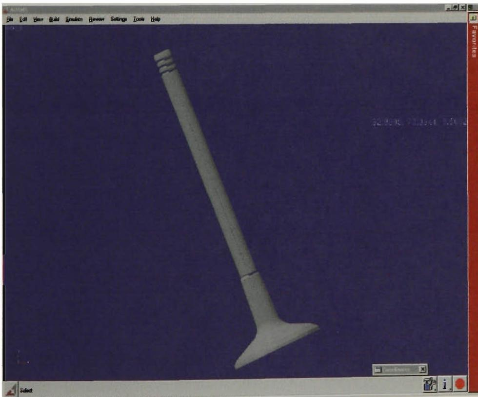
Figure 4.1 – DVC valve as modeled using ADAMS
