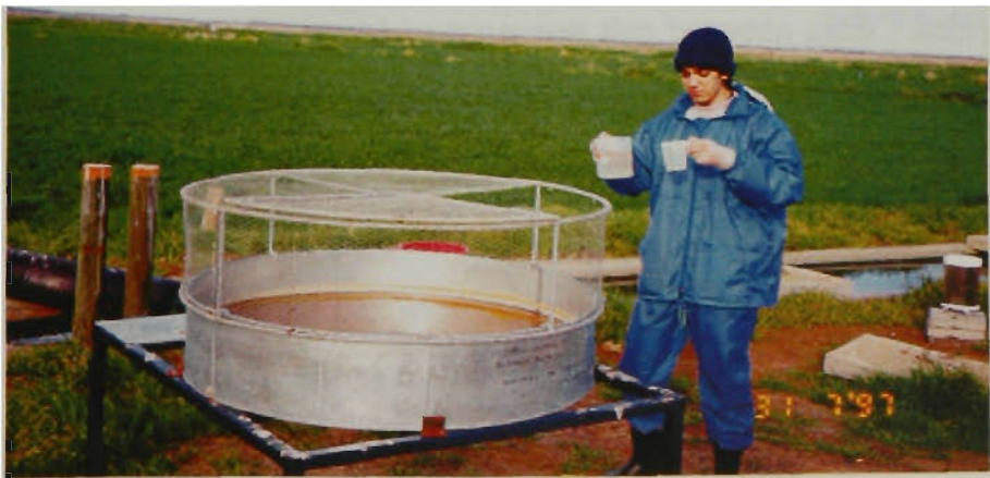
Figure 4.9 Class A Evaporation Pan and Pluviometer (Edge Right)
