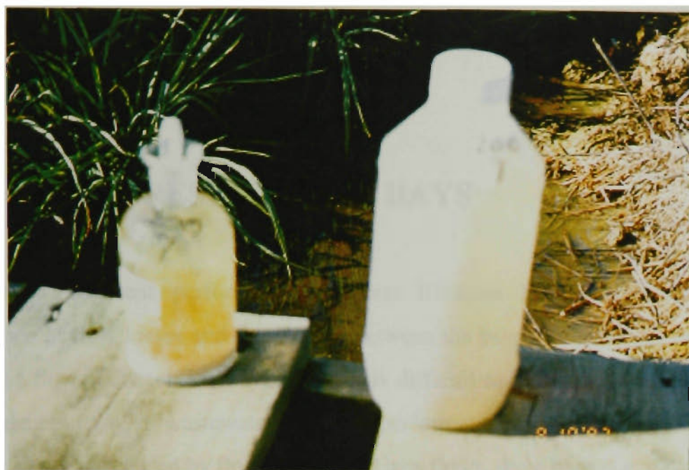
Figure 5.2 300 ml Glass Bottle and 1 Litre Plastic Bottle used in Sampling
