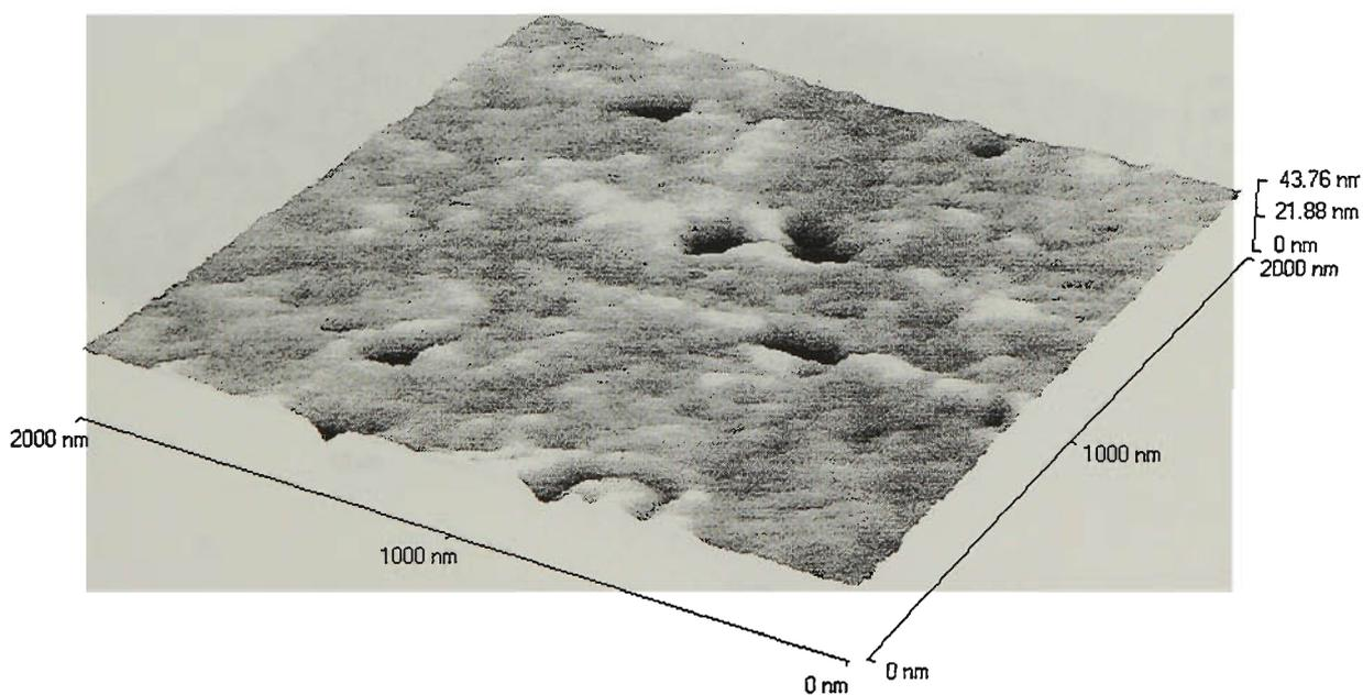
Figure 4.20 AFM image ( $2 \times 2 \mu\text{m}^2$ ) of the air-facing surface of the membrane containing 30% Aliquat 336.
