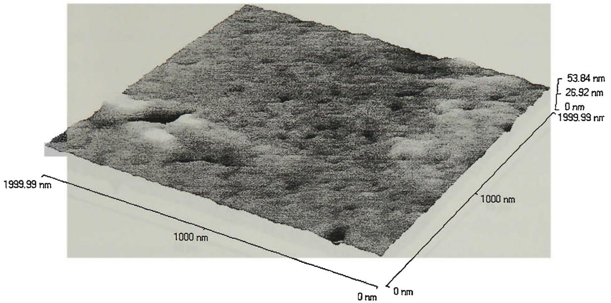
Figure 4.21 AFM image ( $2 \times 2 \mu\text{m}^2$ ) of the glass-facing surface of the membrane containing 30% Aliquat 336.
