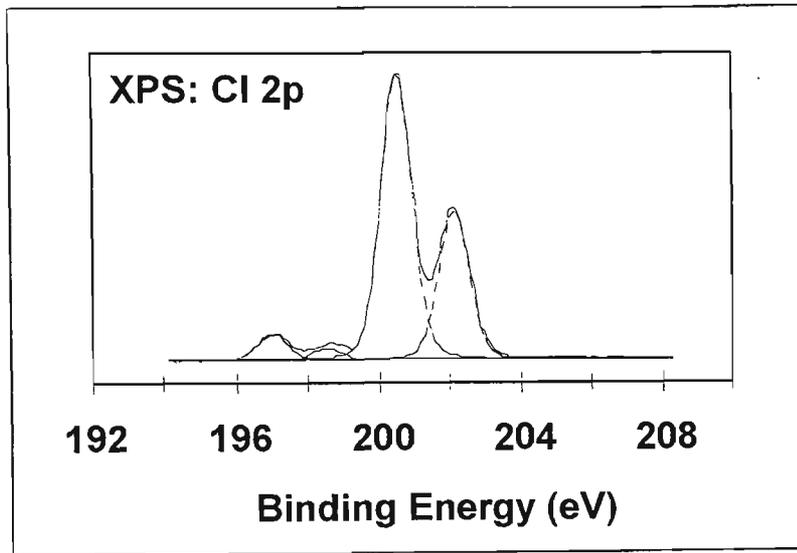
Figure 4.17 Cl 2p XP spectrum acquired from the air-facing surface of a 30% Aliquat 336/PVC membrane before extraction. The solid line is the photoelectron signal and broken lines are the deconvoluted components of the spectral envelope.
