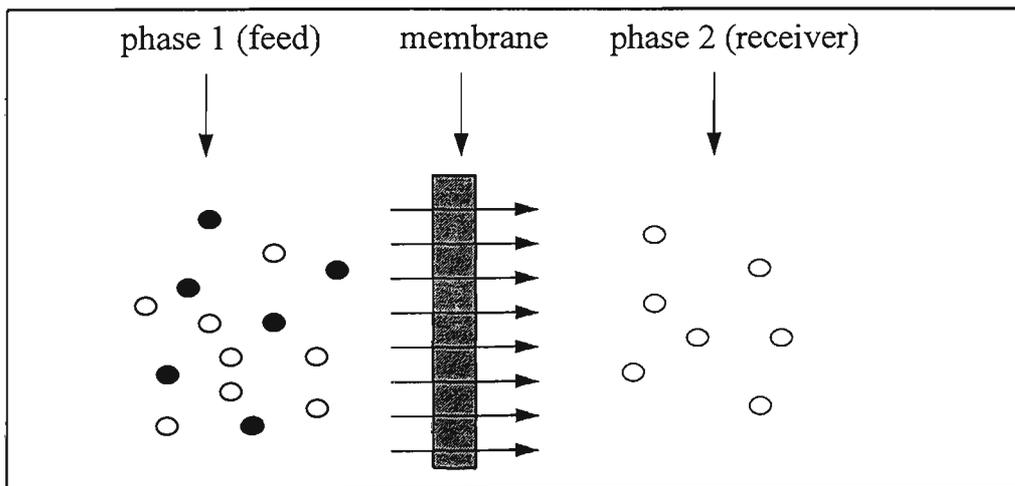
Figure 3.1. Schematic representation of membrane separation process (○ is component A, ● is component B and → is the driving force.)
