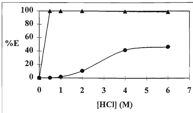
Figure 2.3. Effect of HCl concentrations on the extraction of Cd(II) and Cu(II) from hydrochloric acid solution by Aliquat 336 in Shellsol AB (▲ Cd(II) and ● Cu(II)). The initial aqueous phase Cd(II) and Cu(II) concentration were 200 mg/L and 140 mg/L, respectively. The initial Aliquat 336 concentration of the organic phase was 0.04M.)
