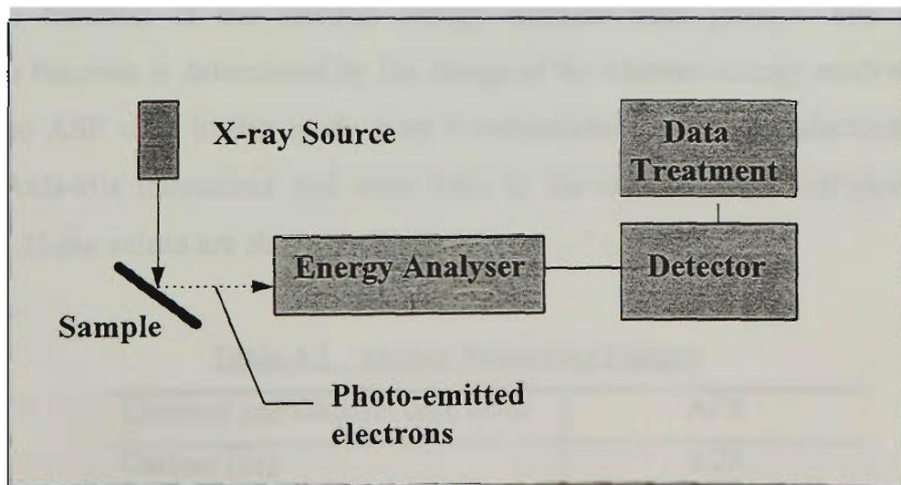
Figure 4.3 A schematic experimental set-up of XPS
