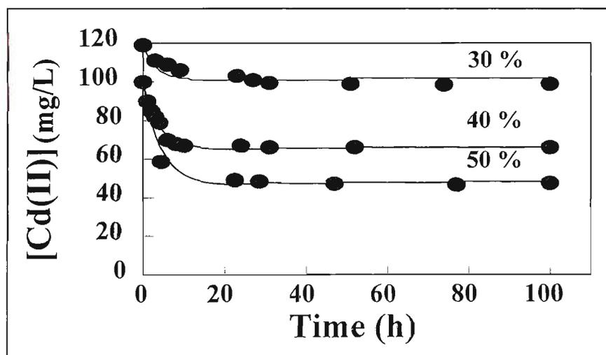
Figure 3.13. Aqueous Cd(II) concentrations vs. the extraction time for various membrane compositions (Initial aqueous Cd(II) concentration in 2M HCl solution - 120mg/L for 30% Aliquat 336/PVC membrane and 100mg/L for 40% and 50% Aliquat 336/PVC membranes. The solid dots are experiment data and the solid lines are mathematical fitting curves)
