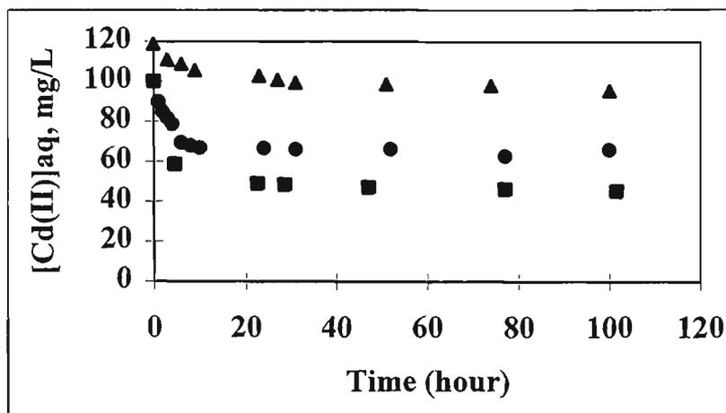
Figure 3.4. Aqueous Cd(II) concentrations vs. the extraction time for various membrane compositions ( $\blacktriangle$  30% Aliquat 336/PVC membrane;  $\bullet$  40% Aliquat 336/PVC membrane and  $\blacksquare$  50% Aliquat 336/PVC membrane ) Initial aqueous Cd(II) concentration in 2M HCl solution - 120mg/L for 30% Aliquat 336/PVC membrane and 100mg/L for 40% and 50% Aliquat 336/PVC membranes.
