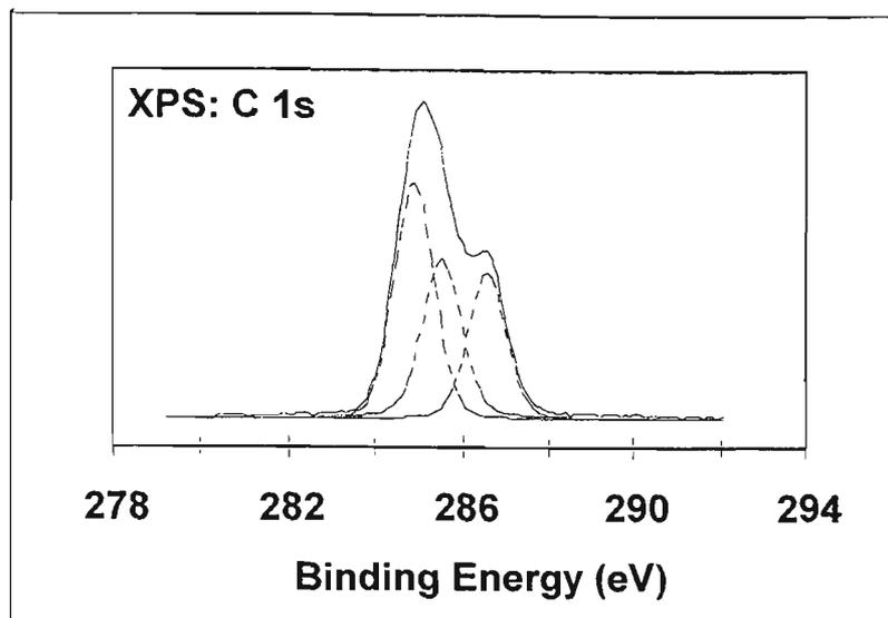
Figure 4.16 C 1s XP spectrum acquired from the air-facing surface of a 30% Aliquat 336/PVC membrane before extraction. The solid line is the photoelectron signal and broken lines are the deconvoluted components of the spectral envelope.
