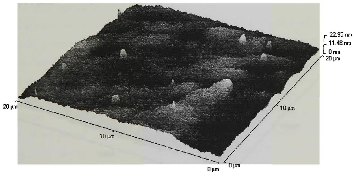
Figure 4.12 AFM image ( $20 \times 20 \mu\text{m}^2$ ) of the air-facing surface of 40% Aliquat 336/PVC membrane.
