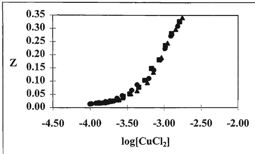
Figure 2.5. Equilibrium data for the extraction of Cu(II) from 3M hydrochloric acid solution using Aliquat 336 in Shellsol AB (▲ 0.04M Aliquat 336; ● 0.08M Aliquat 336; ■ 0.12M Aliquat 336). The aqueous phase Cu(II) concentration range was 0.003-0.25M)
