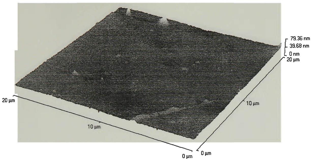
Figure 4.11 AFM image ( $20 \times 20 \mu\text{m}^2$ ) of the glass-facing surface of 30% Aliquat 336/PVC membrane.
