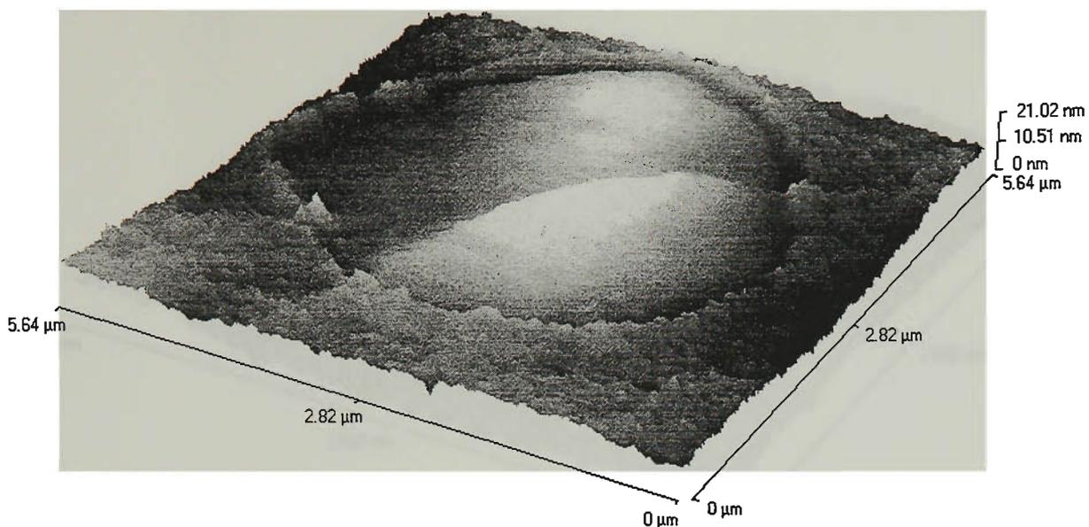
Figure 4.7 AFM image ( $5.6 \times 5.6 \mu\text{m}^2$ ) of a “blister” like spot on the air-facing surface of 1% Aliquat 336/PVC membrane.
