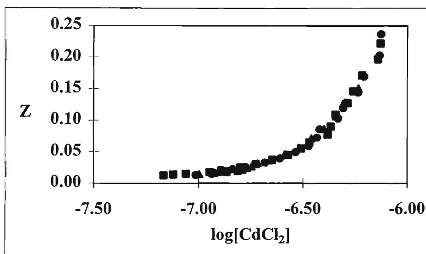
Figure 2.4 Equilibrium data for the extraction of Cd(II) from 2M hydrochloric acid solution using Aliquat 336 in Shellsol AB solvent ( $\blacktriangle$  0.04M Aliquat 336;  $\bullet$  0.06M Aliquat 336;  $\blacksquare$  0.08M Aliquat 336. The aqueous phase Cd(II) concentration range was 0.0006 to 0.02M)
