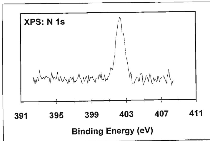
Figure 4.18 N 1s XP spectrum acquired from the air-facing surface of a 30% Aliquat 336/PVC membrane before extraction.
