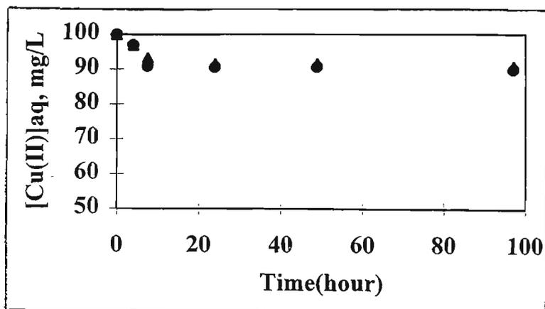
Figure 3.12. Extraction of Cu(II) using 40% Aliquat 336/PVC membrane formed facing air (▲) and facing glass (●) (The thickness of the membrane was 147 $\mu$ m)
