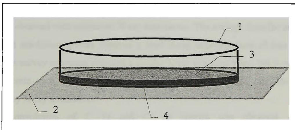
Figure 4.4. Schematic diagram of the membrane surfaces formed under different conditions. ( 1. glass ring, 2. The glass plate, 3. the air-facing surface and 4. the glass-facing surface)
