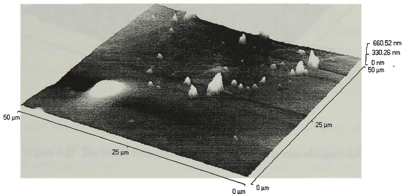
Figure 4.25 AFM image ( $50 \times 50 \mu\text{m}^2$ ) of the glass-facing surface of the membrane containing 40% Aliquat 336 after extracting Cd(II).
