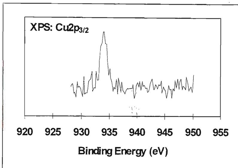
Figure 4.19 Cu 2p XP spectrum acquired from the air-facing surface of a 30% Aliquat 336/PVC membrane after extraction.
