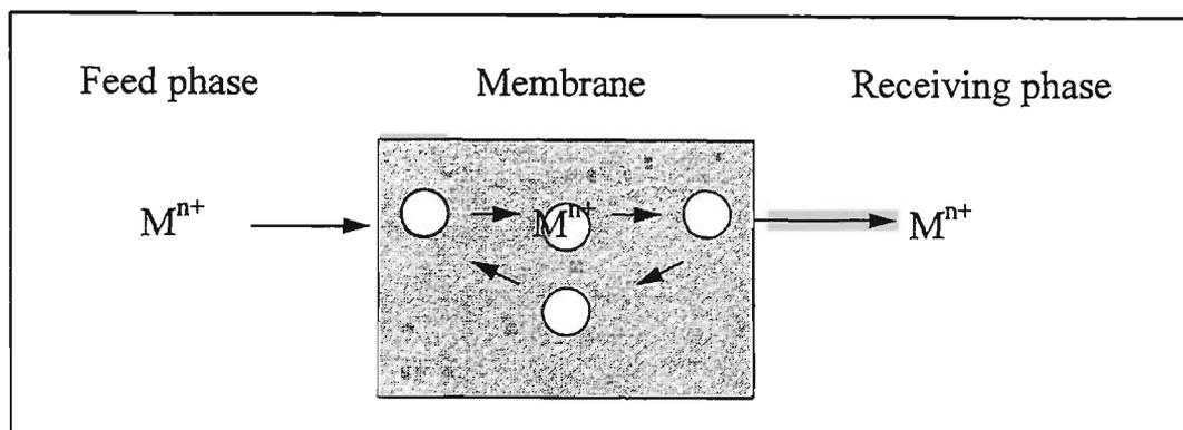
Figure 3.2. The transport mechanism of metal ions in the Aliquat 336/PVC membrane extraction system ( $M^{n+}$  = the metal ions and  $\bigcirc$  = extractant molecules)
