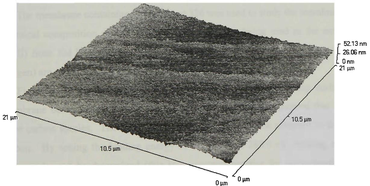
Figure 4.14 AFM image ( $21 \times 21 \mu\text{m}^2$ ) of the air-facing surface of 50% Aliquat 336/PVC membrane.
