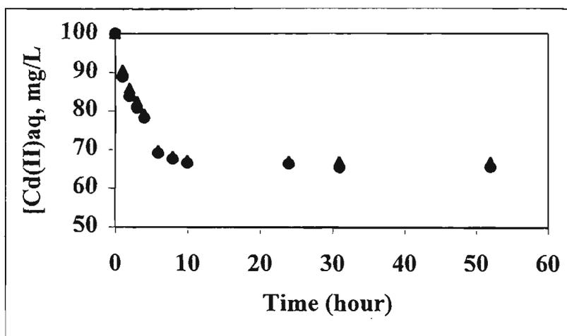
Figure 3.10. Extraction of Cd(II) using 40% Aliquat 336/PVC membrane formed facing air (▲) and facing glass (●)(The thickness of the membrane was 138 $\mu$ m)
