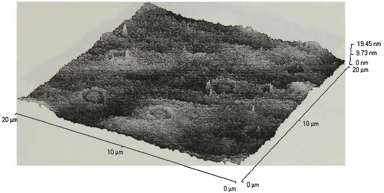
Figure 4.5 AFM image ( $20 \times 20 \mu\text{m}^2$ ) of the air-facing surface of 1% Aliquat 336/PVC membrane.
