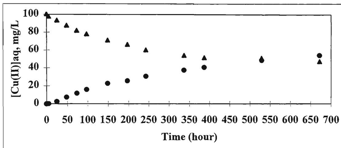
Figure 3.15. The extraction of Cu(II) from the feed phase to the receiver phase by 40% Aliquat 336/PVC membrane. (Initial Cu(II) concentration were 100mg/L in the feed phase and 0 mg/L in the receiver phase. Initial HCl concentration were 3M in the feed and 0.1M in the receiver. ▲ feed phase and ● receiver phase)
