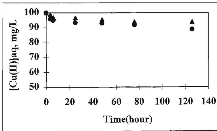
Figure 3.9. Extraction of Cu(II) using 30% Aliquat 336/PVC membrane formed facing air (▲) and facing glass (●) (The thickness of the membrane was 113 $\mu$ m)
