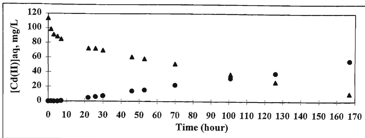
Figure 3.14. The extraction of Cd(II) from the feed phase to the receiver phase by 40% Aliquat 336/PVC membrane. (Initial Cd(II) concentration were 114mg/L in the feed phase and 0 mg/L in the receiver phase. Initial HCl concentration were 2M in the feed and 0.05M in the receiver. ▲ feed phase and ● receiver phase)
