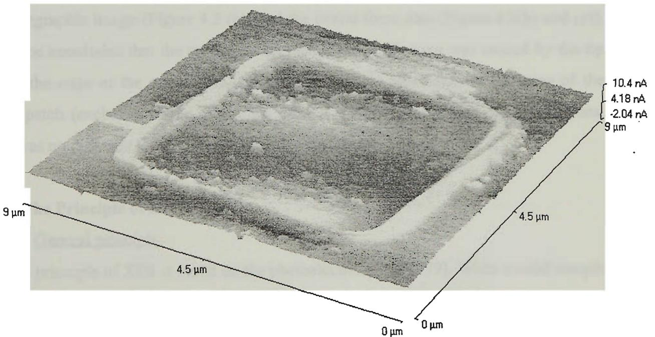
Figure 4.2 (a) The topographic image of the raised patch of SiO<sub>2</sub> on the semiconductor grid. (b) The lateral force map obtained when the tip was scanned in the forward direction. (c) The lateral force map obtained when the tip was scanned in the backward (reverse) direction.
