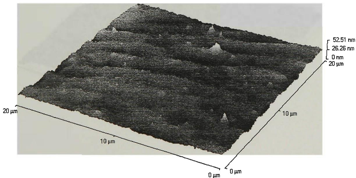
Figure 4.10 AFM image ( $20 \times 20 \mu\text{m}^2$ ) of the air-facing surface of 30% Aliquat 336/PVC membrane.
