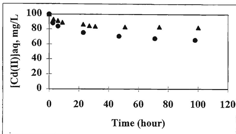
Figure 3.6. The effect of membrane thickness on the extraction of Cd(II). (the membrane composition was 30% Aliquat 336 in PVC, the initial Cd(II) concentration are 100mg/L for both 82 $\mu\text{m}$  membrane thickness ( $\blacktriangle$ ) and 279 $\mu\text{m}$  membrane thickness( $\bullet$ ).)
