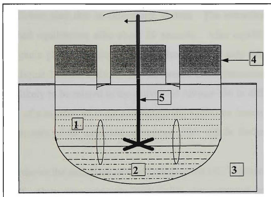
Figure 2.1. Schematic diagram of the two-phase titration apparatus. (1) Organic phase, (2) Aqueous phase, (3) Thermostated water bath, (4) Three-neck round bottomed flask with indentations to facilitate mixing and (5) Stirrer
