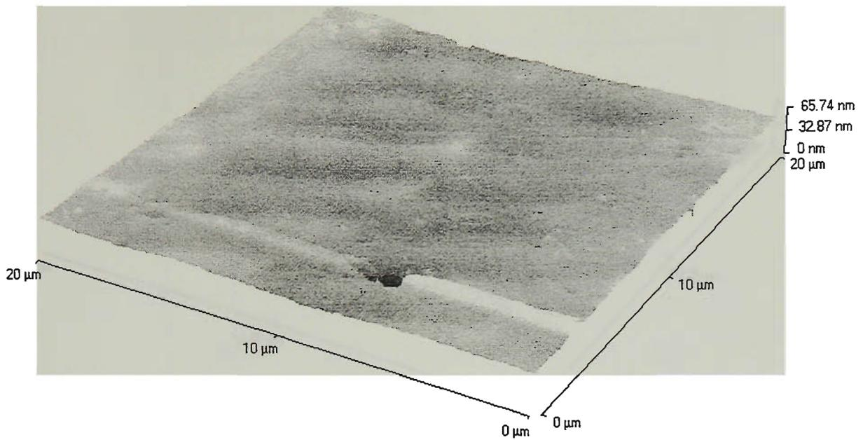
Figure 4.13 AFM image ( $20 \times 20 \mu\text{m}^2$ ) of the glass-facing surface of 40% Aliquat 336/PVC membrane.
