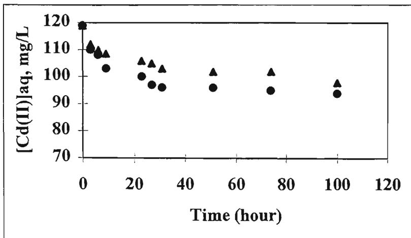
Figure 3.8. Extraction of Cd(II) using 30% Aliquat 336/PVC membrane formed facing air (▲) and facing glass (●) (The thickness of the membrane was 82 $\mu$ m)
