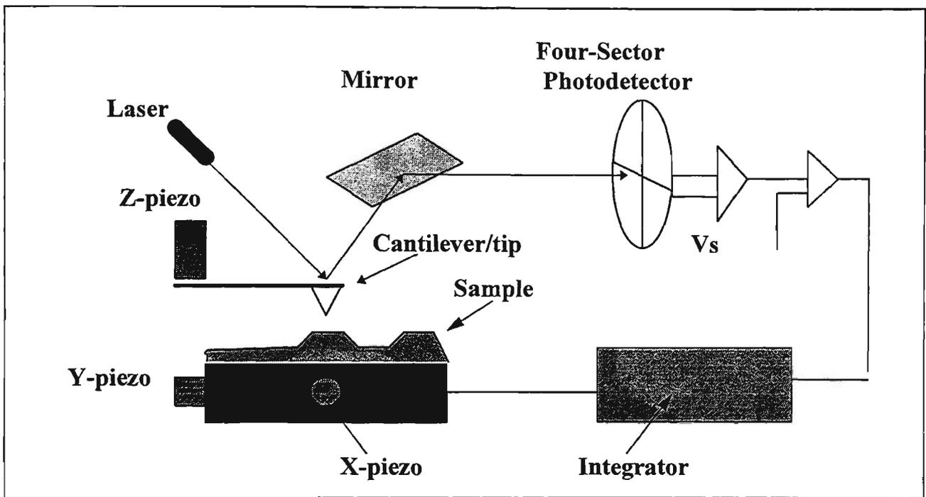
Figure 4.1 Schematic diagram of an atomic force microscope
