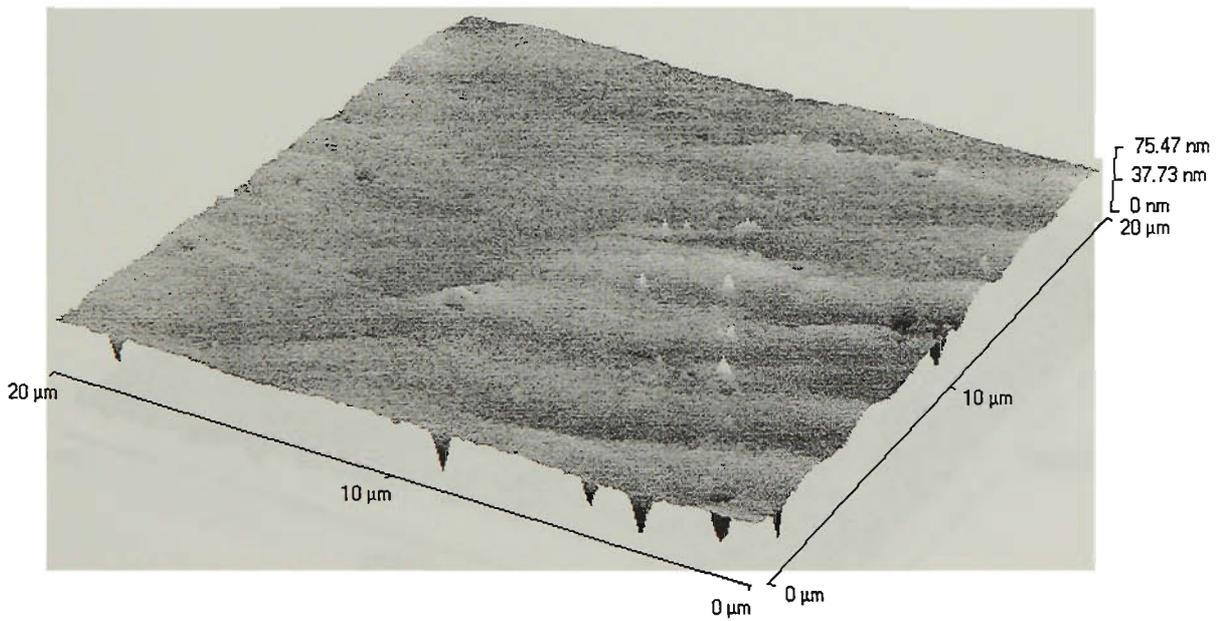
Figure 4.6 AFM image ( $20 \times 20 \mu\text{m}^2$ ) of the glass-facing surface of 1% Aliquat 336/PVC membrane.
