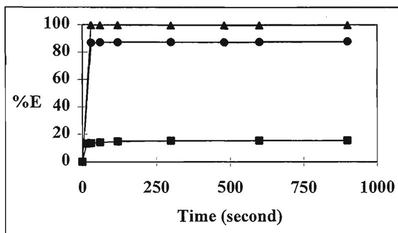
Figure 2.2 Effect of organic-aqueous phase contact time on the extraction of Cd(II) and Cu(II) from 3M hydrochloric acid solutions by Aliquat 336. ( $\blacktriangle$  Cd(II)/Shellsol AB,  $\bullet$  Cd(II)/Chloroform,  $\blacksquare$  Cu(II)/Shellsol AB. The initial aqueous phase Cd(II) and Cu(II) concentration were 200 mg/L and 140mg/L, respectively. The Aliquat 336 concentration in the organic phase was 0.04M.)
