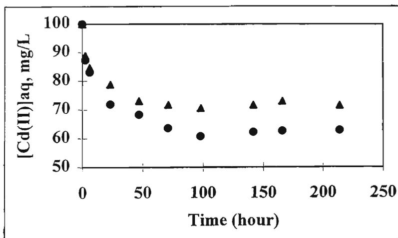
Figure 3.7. Extraction of Cd(II) using 30% Aliquat 336/PVC membrane formed facing air (▲) and facing glass (●) (The thickness of the membrane was 279 $\mu$ m)
