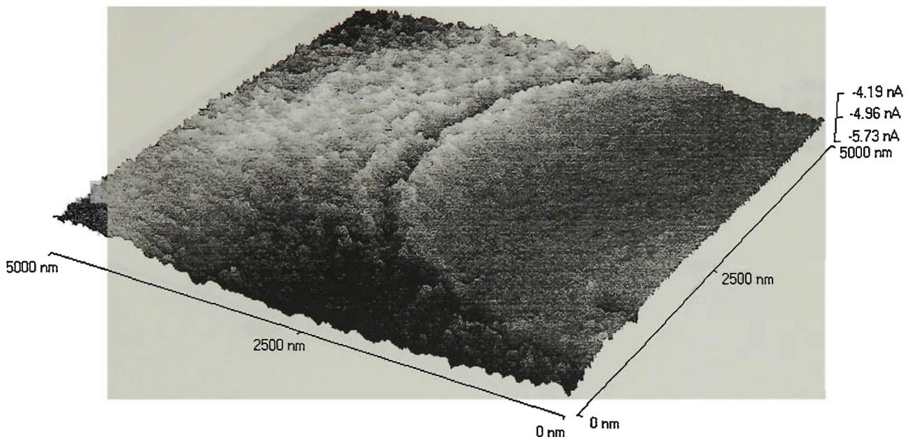
Figure 4.9 Lateral force (backward) map ( $5 \times 5 \mu\text{m}^2$ ) of the “blister” like spot and its surrounding areas on the air-facing surface of 1% Aliquat 336/PVC membrane.
