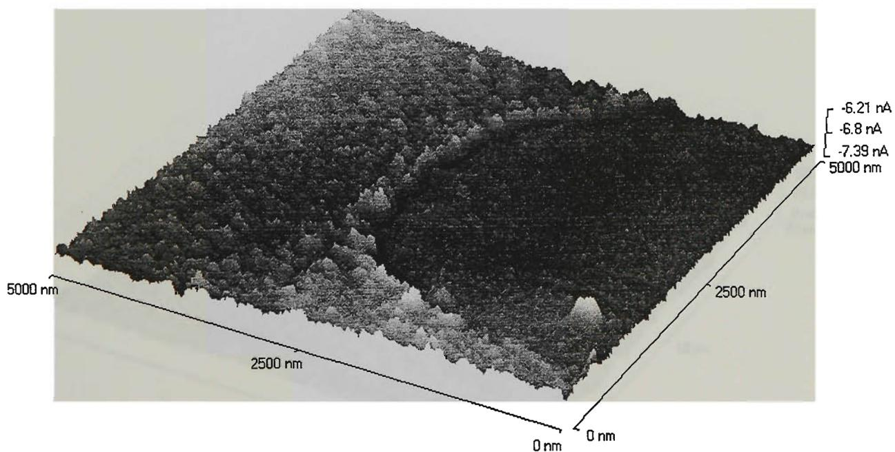
Figure 4.8 Lateral force (forward) map ( $5 \times 5 \mu\text{m}^2$ ) of the “blister” like spot and its surrounding areas on the air-facing surface of 1% Aliquat 336/PVC membrane.
