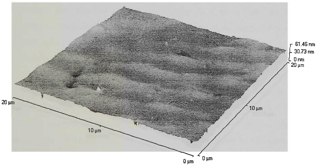
Figure 4.22 AFM image ( $20 \times 20 \mu\text{m}^2$ ) of the air-facing surface of the membrane containing 30% Aliquat 336 after extracting Cu(II).
