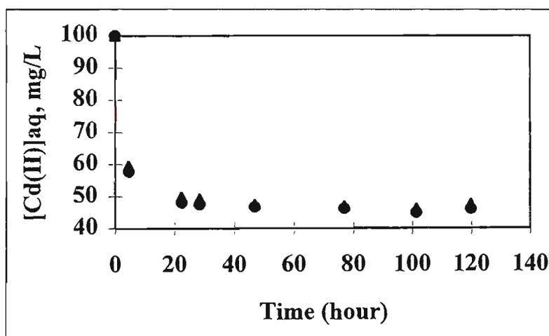
Figure 3.11. Extraction of Cd(II) using 50% Aliquat 336/PVC membrane formed facing air (▲) and facing glass (●) (The thickness of the membrane was 133 $\mu$ m)
