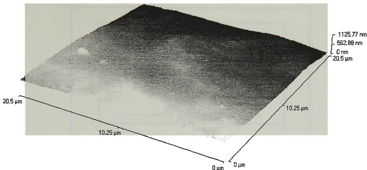
Figure 4.15 AFM image ( $20 \times 20 \mu\text{m}^2$ ) of the glass-facing surface of 50% Aliquat 336/PVC membrane.
