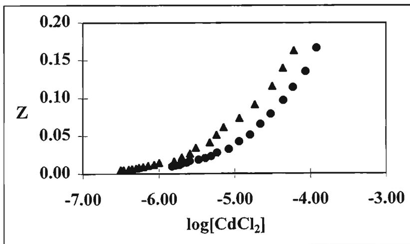
Figure 2.6 Equilibrium data for the extraction of Cd(II) from 2M hydrochloric acid solution using Aliquat 336 in chloroform (▲ 0.04M Aliquat 336; ● 0.06M Aliquat 336). The aqueous phase Cd(II) concentration range was 0.0006 to 0.02M)
