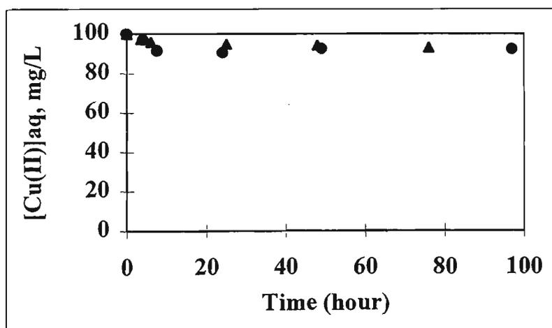
Figure 3.5. Aqueous Cu(II) concentrations vs. extraction time for various membrane compositions ( $\blacktriangle$  30% Aliquat 336/PVC membrane;  $\bullet$  40% Aliquat 336/PVC membrane). The initial Cu(II) concentration of the feed solution was 100mg/L
