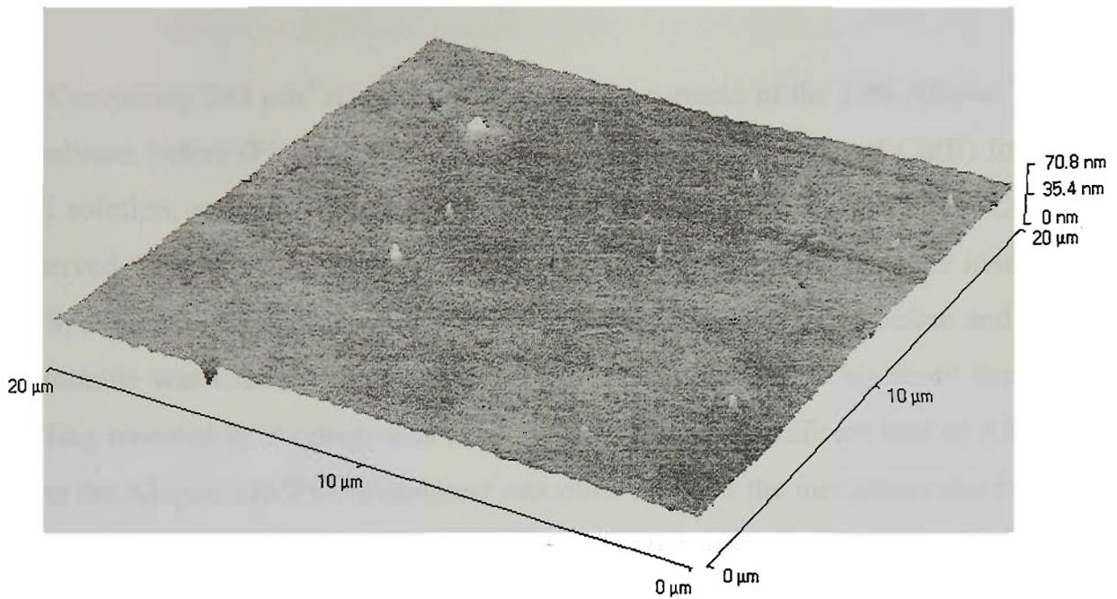
Figure 4.23 AFM image ( $20 \times 20 \mu\text{m}^2$ ) of the glass-facing surface of the membrane containing 30% Aliquat 336 after extracting Cu(II).
