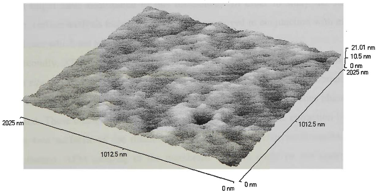
Figure 4.24 AFM image ( $2 \times 2 \mu\text{m}^2$ ) of the glass-facing surface of the membrane containing 30% Aliquat 336 after extracting Cu(II).
