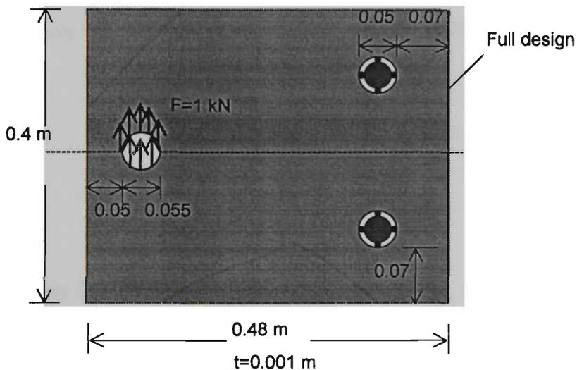
Fig. 5.6: Design domain of an angle piece.
