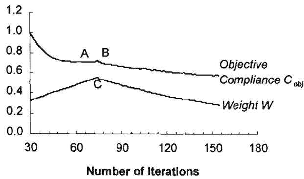
Fig. 5.3: Evolutionary history of objective compliance and structural weight.
