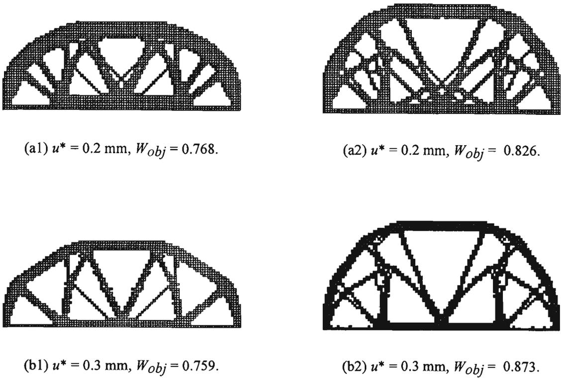
Fig. 5.26: Optimal topologies: BESO:(a1)~(b1); ESO: (a2)~(b2).
