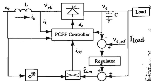
Fig.2 The block diagram of the PCFF controlled power converter
