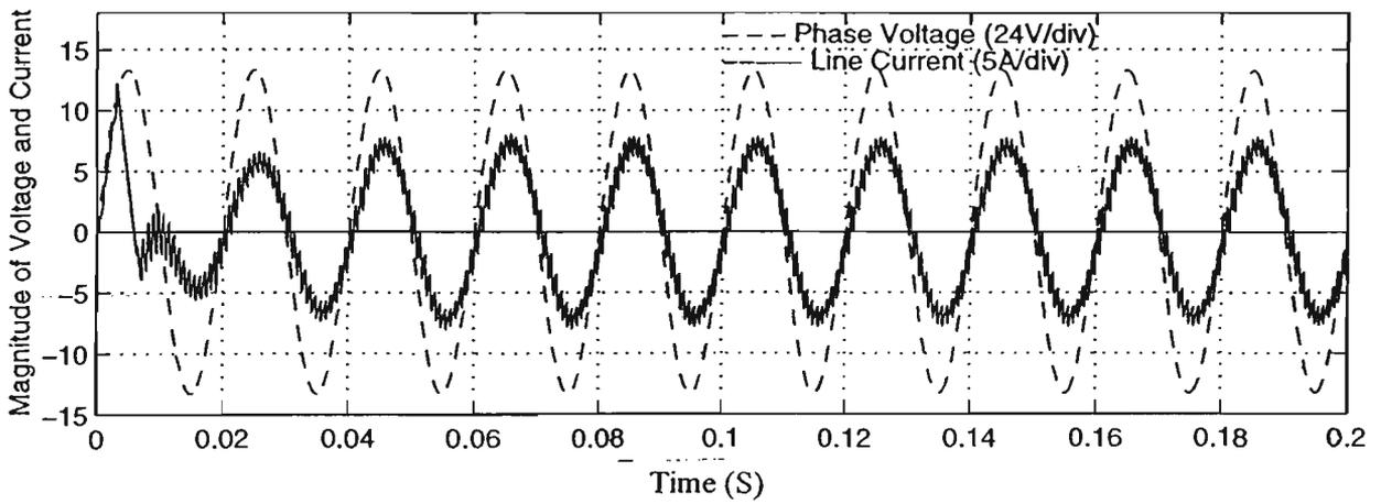
Fig. 4.12 Step Response of Line Current and Line-to-Neutral Voltage in the Rectifying Mode
