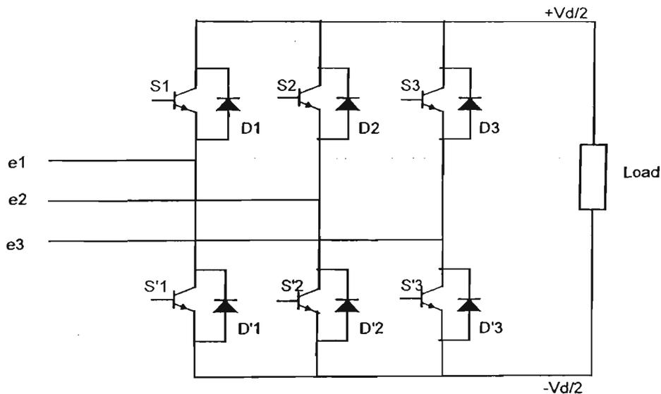
Fig. 5.1 Circuit Diagram of the Three Phase Voltage Source Converter
