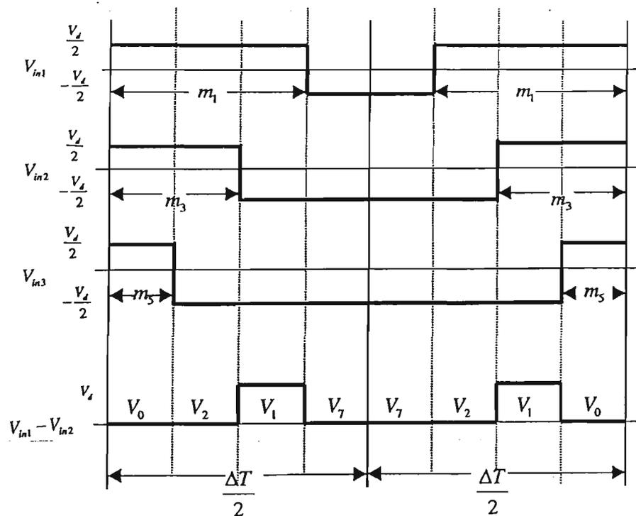
Fig. 5.8 Space Vector PWM Switching Patterns
