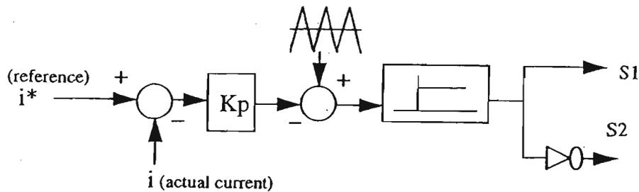
Fig. 1.3 Phase SFRC Current Regulator Structure
