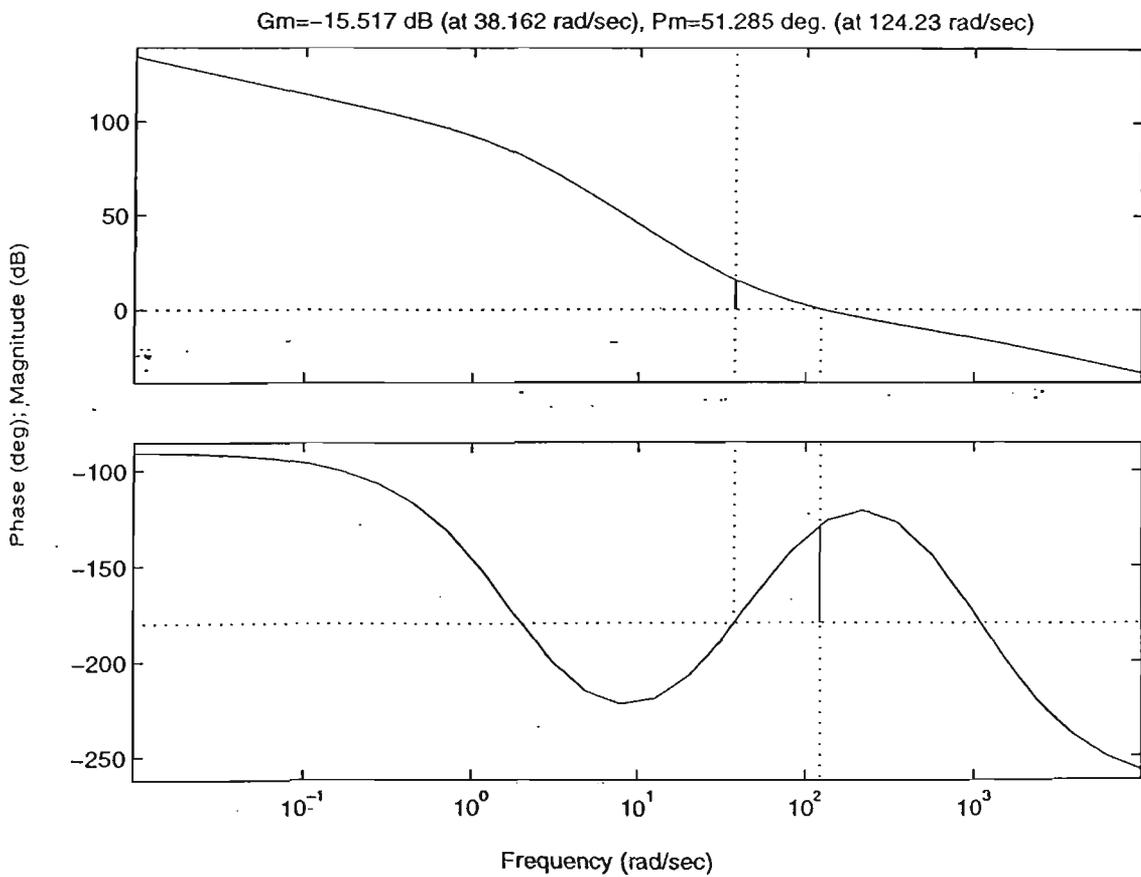
Fig. 3.8 Determination of Gain Margin and Phase Margin on the Bode Plot of  $L_{02}(s)$
