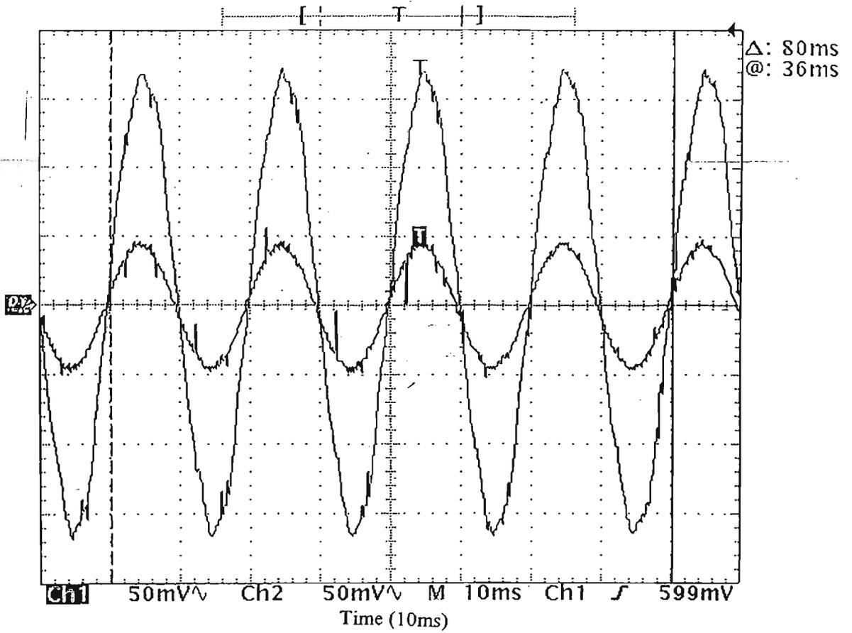
Fig. 6.9 Experimental Results of Line Current and Line-to-Neutral Voltage
