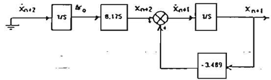
Figure 4: Modelling the load disturbance  $\Delta r_o$ .
