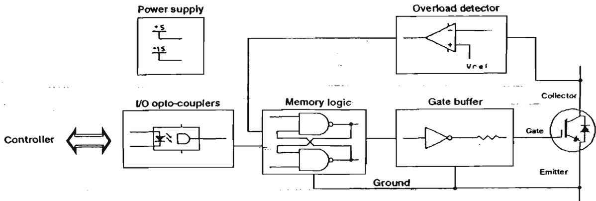
Fig. 5.4 Block Diagram of IGBT Gate Driver
