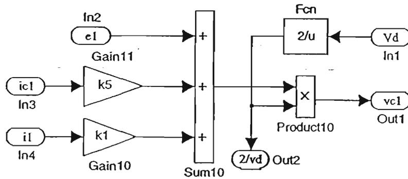
Fig. 4.3 The Configuration of the PCFF Controller Subroutine
