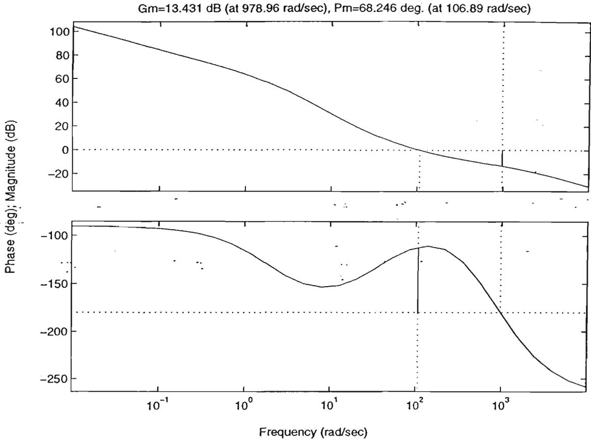
Fig. 3.7 Determination of Gain Margin and Phase Margin on the Bode Plot of  $L_{01}(s)$
