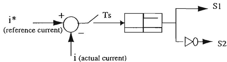
Fig. 1.1 Per Phase Delta Current Regulator Structure
