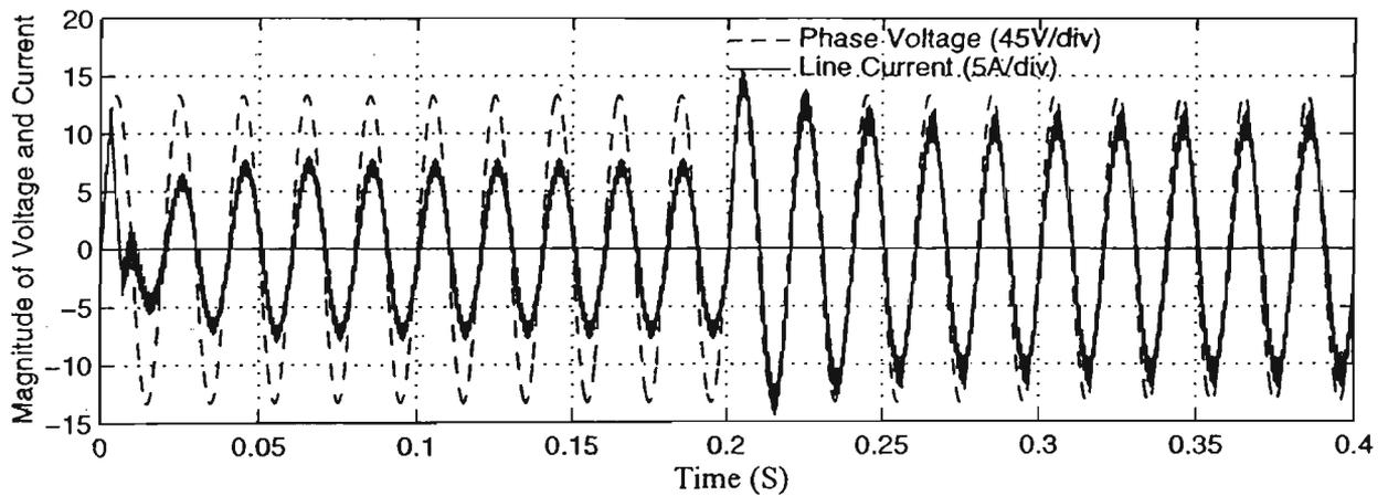
Fig. 4.20 Transient Performance of Line Current and Phase Voltage in Input Change
