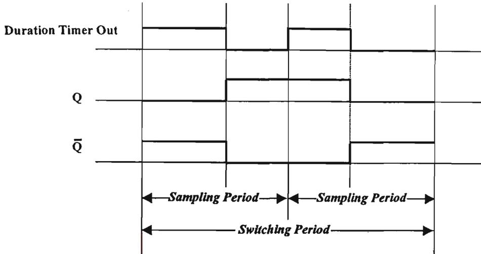
*Fig.5.12 Waveforms of Timer Output and J-K Flip-Flop Outputs*
