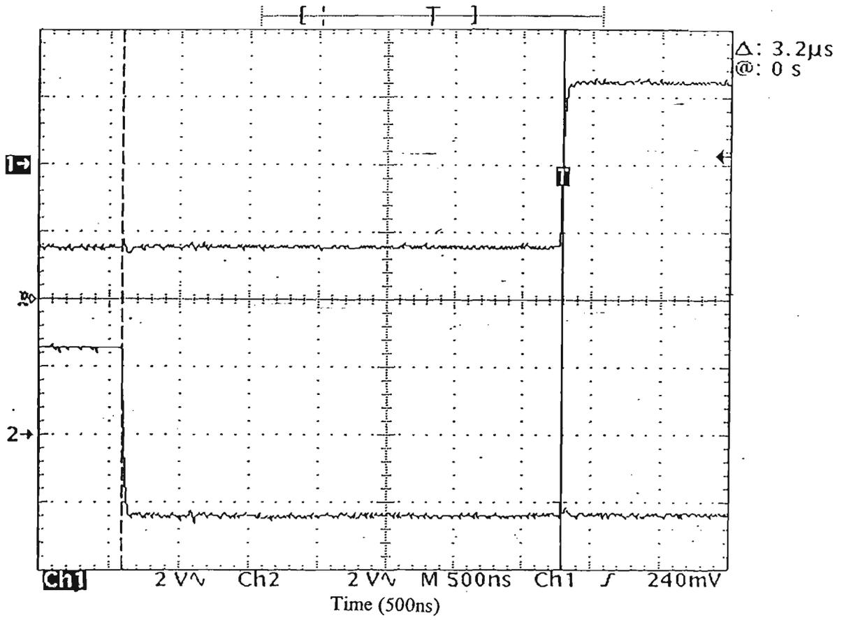
Fig. 6.5 Experimental Result of Crossover Delay
