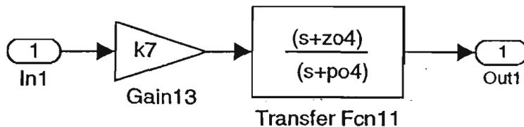
Fig. 4.8 The Configuration of Phase Lead Subroutine
