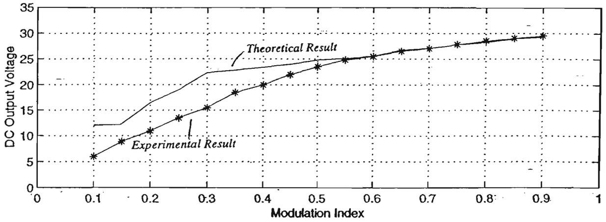
Fig.6.6 DC Output Voltage of Converter
