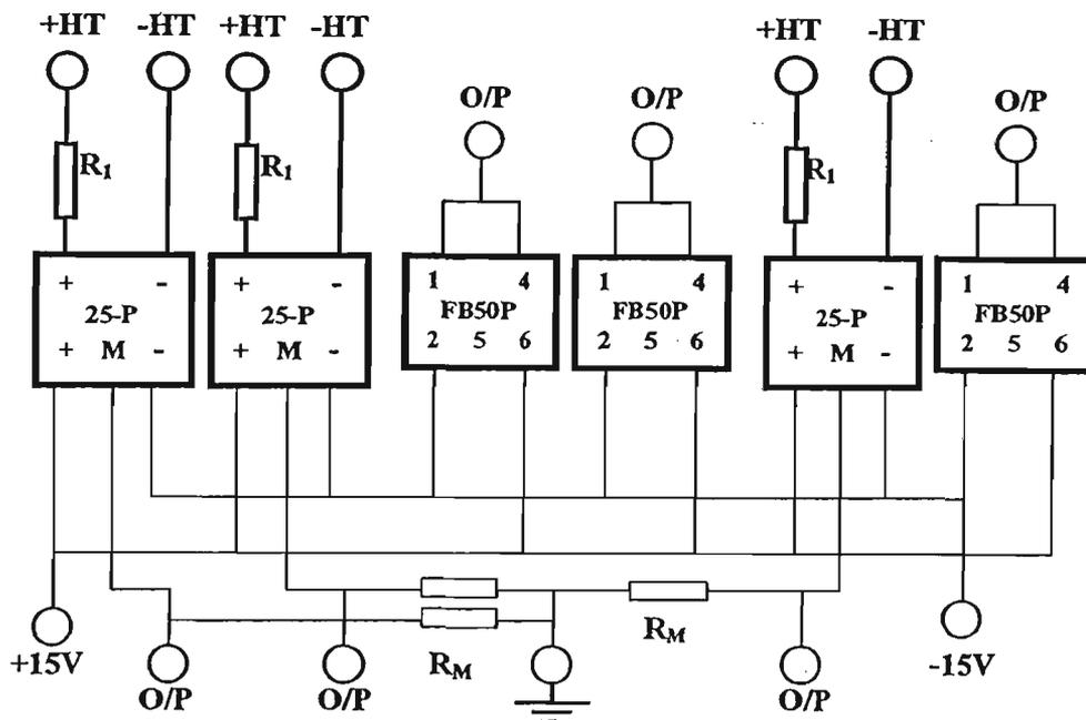
Fig. 5.16 Circuit Connection of Three Current Transducers and Three Voltage Transducers
