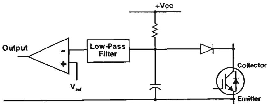
Fig. 5.5 Overload Detection for IGBT Devices
