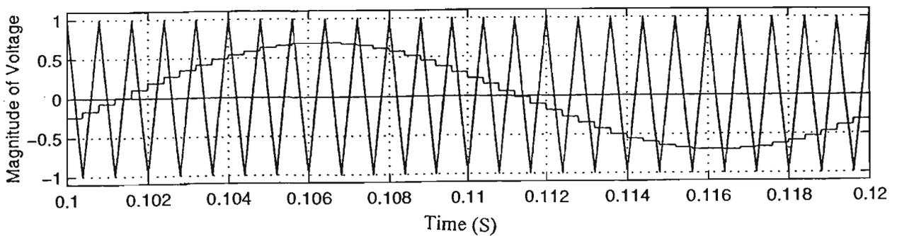
Fig. 4.13 Sample-and-hold Modulating Waveform and Carrier Waveform in the Rectifying Mode
