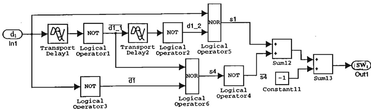
Fig. 4.5 The Simulation Structure of Crossover Delay Subroutine
