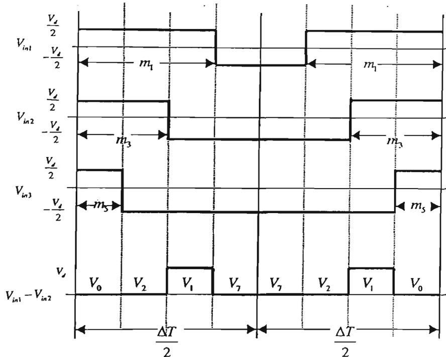
Fig. 1.7 Space Vector PWM Waveform in One Switching Period
