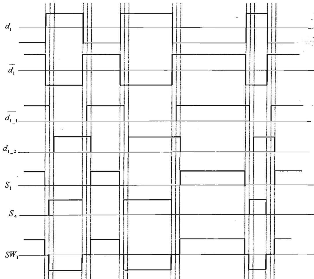
Fig. 4.6 The Simulation Results of Gating Signals.
