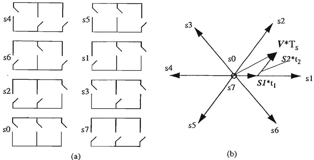
Fig. 1.6 Switch configuration and Target Phase from Space Vector
