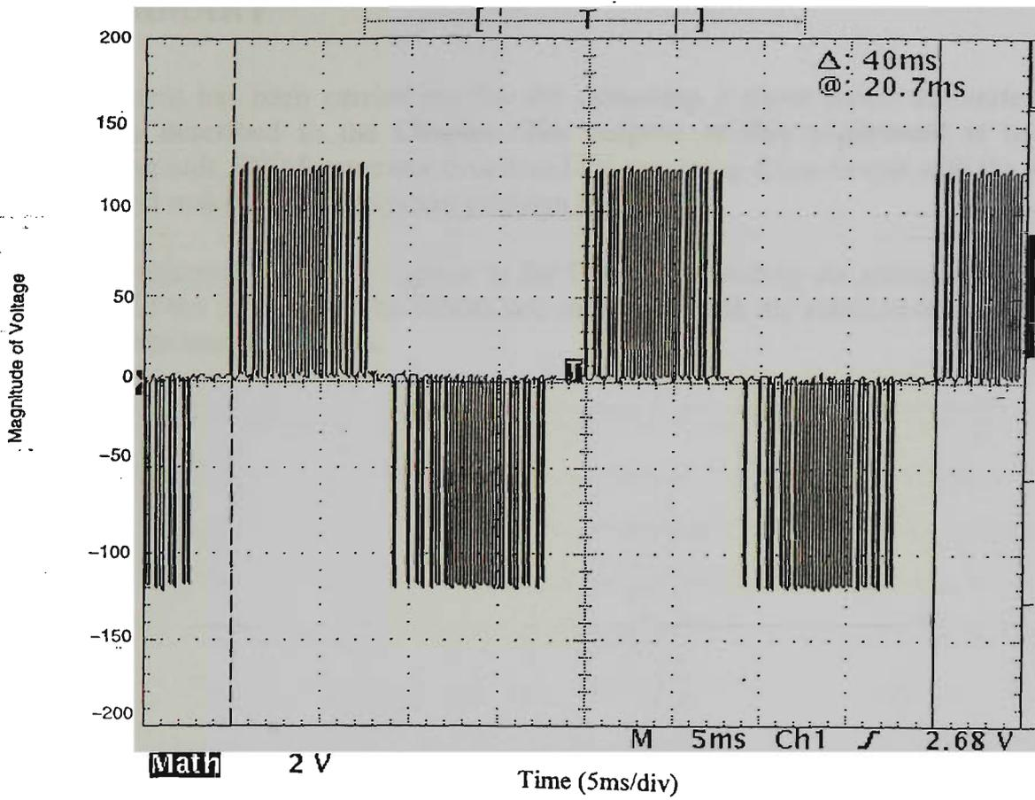
Fig. 6.11 Experimental Results of Line-to-Line Voltage of the Converter.
