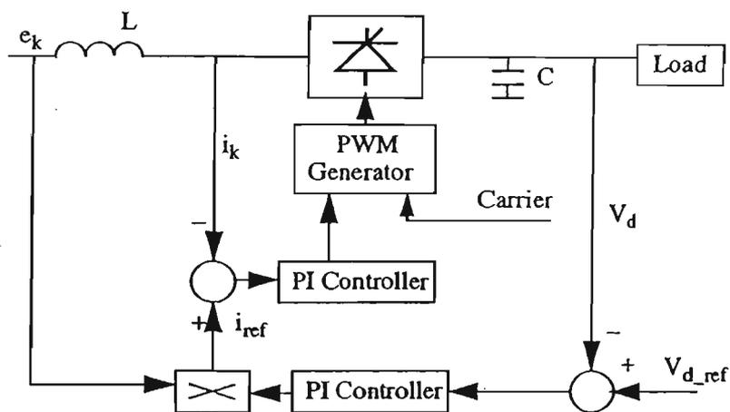
Fig. 1.9 Current Control in Stationary Frame
