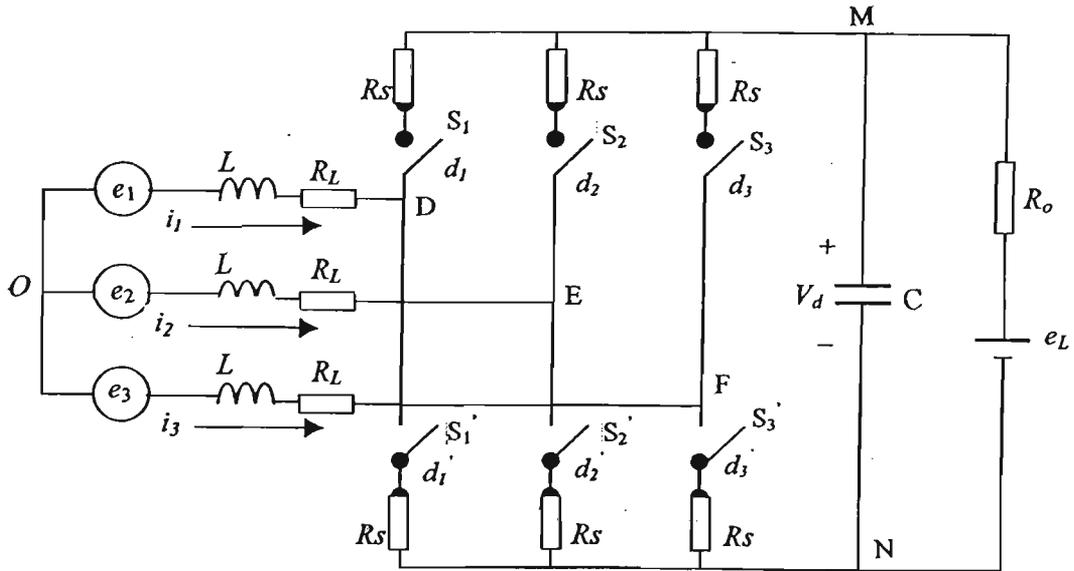
Fig. 2.1 The Circuit of PWM AC/DC Converter
