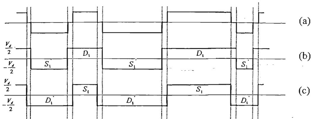
Fig. 5.3 The Waveforms of Driving Signal and Phase Leg Voltage
