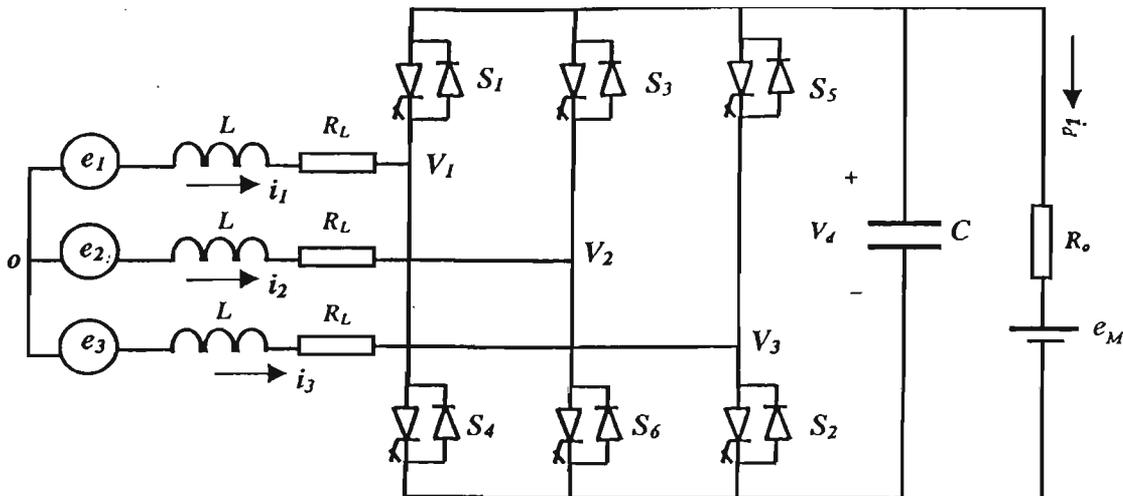
Fig. 4.1 Three Phase PWM AC/DC Power Converter
