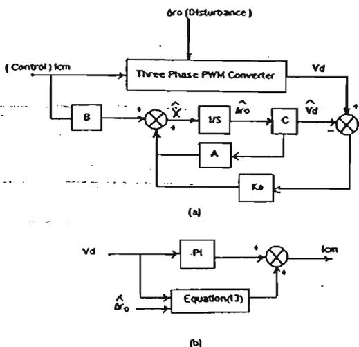
Figure 5: Block schematic of the state observer
