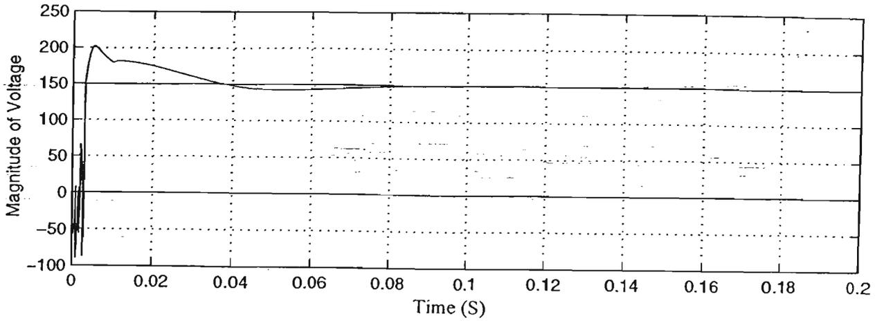
Fig. 4.15 Step Response of DC Output Voltage in the Regenerating Mode
