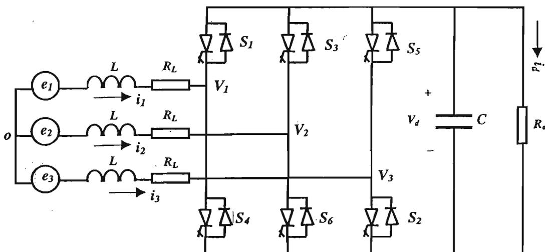
Fig. 6.1 The Circuit of Three Phase PWM AC/DC Power Converter
