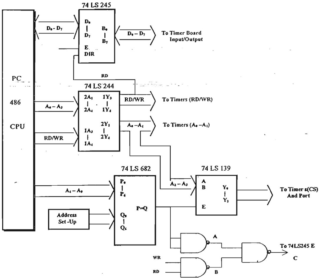
Fig. 5.10 Block Diagram of the Control Block
