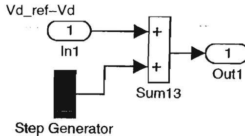
*Fig. 4.9 The Configuration of the Step Signal Generator Subroutine*
