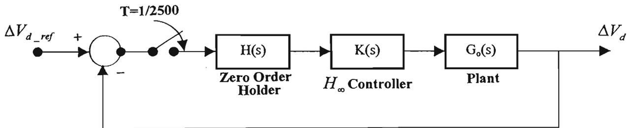
Fig. 3.9 The Discrete-Time PCFF Control System with  $H_\infty$  Controller
