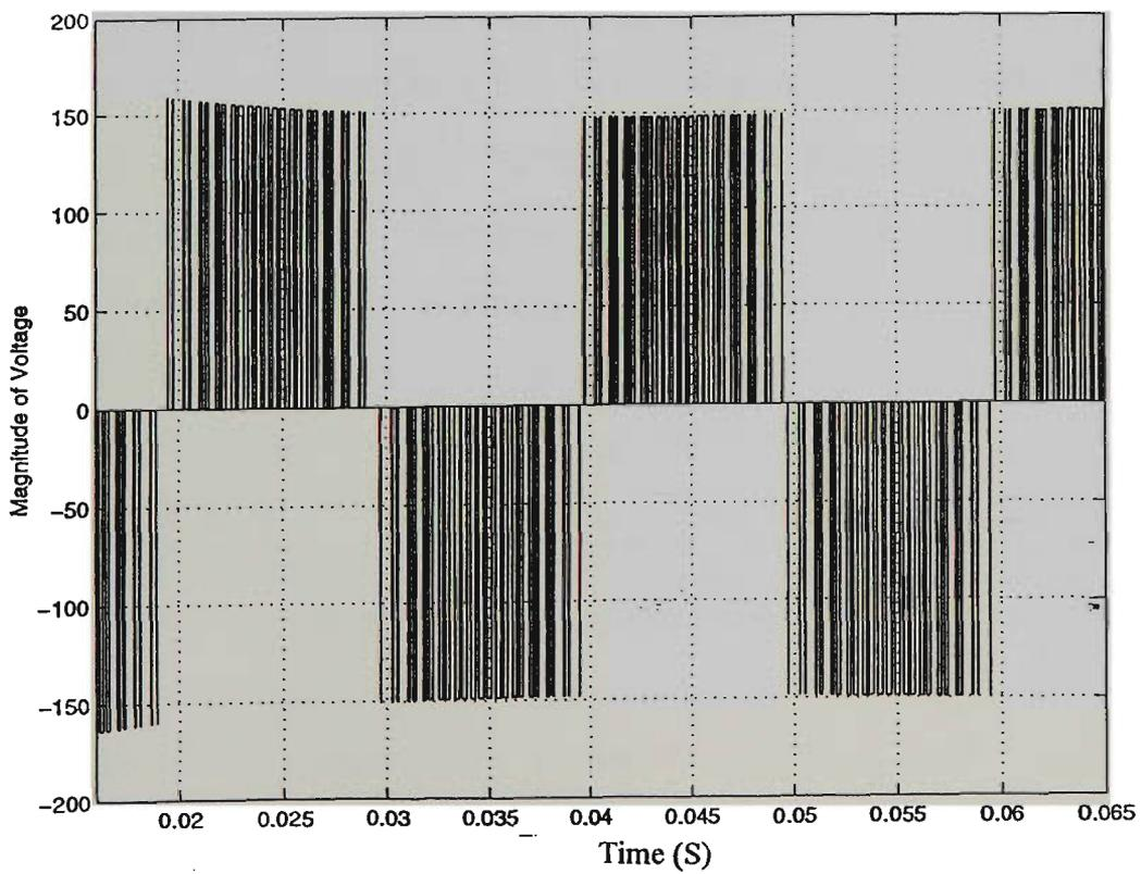
Fig. 6.12 Simulation Result of Line-to-Line Voltage at the AC Terminal of the Converter
