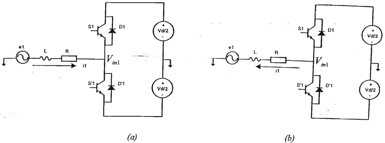
*Fig. 5.2 Three Phase Leg Voltage Source Converter (with One Phase shown Only)*
