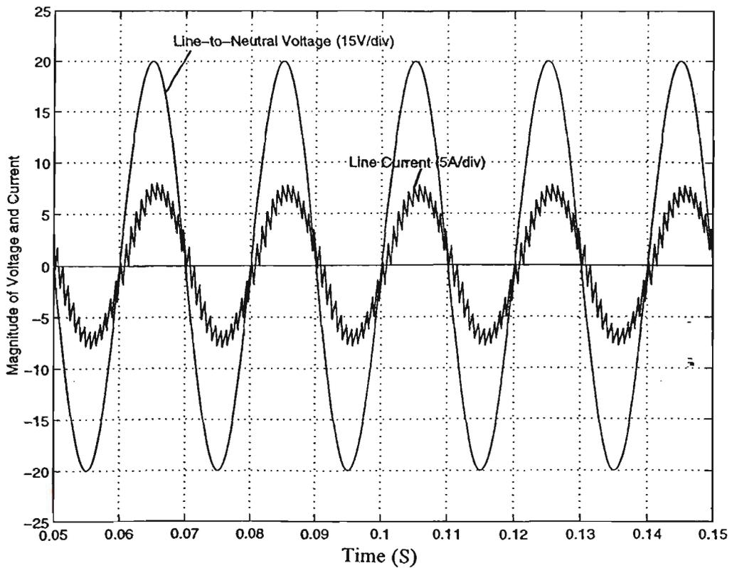
Fig. 6.10 Simulation Results of Line Current and Line-to-Neutral Voltage
