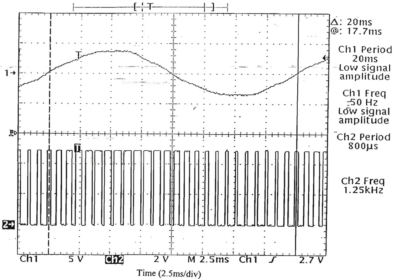
Fig. 6.4 Experimental Results of Utility Phase Voltage and PWM Firing Signal
