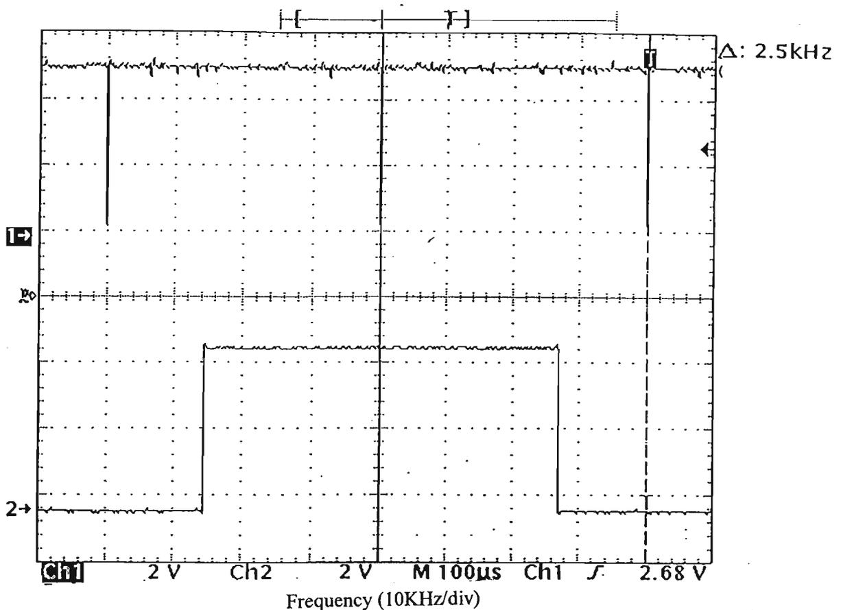
Fig. 6.3 Experimental Results of Sampling Signal and PWM Firing Signal
