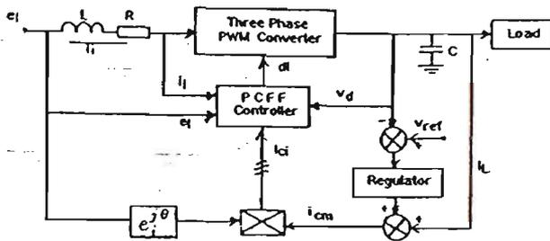
Figure 2: Block diagram of the PCFF control
