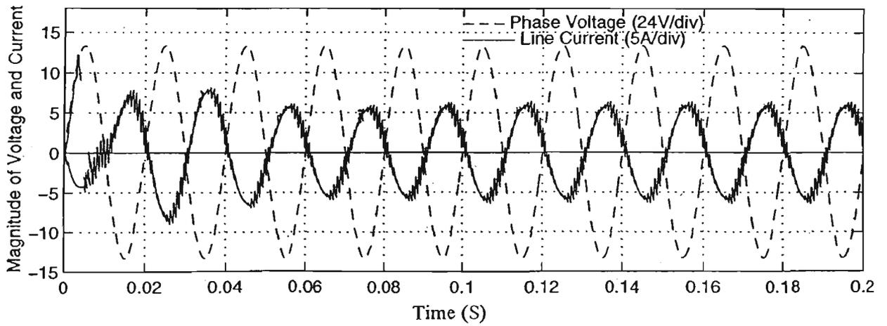
Fig. 4.17 Step Response of Line Current and Line-to-Neutral Voltage in the Regenerating Mode
