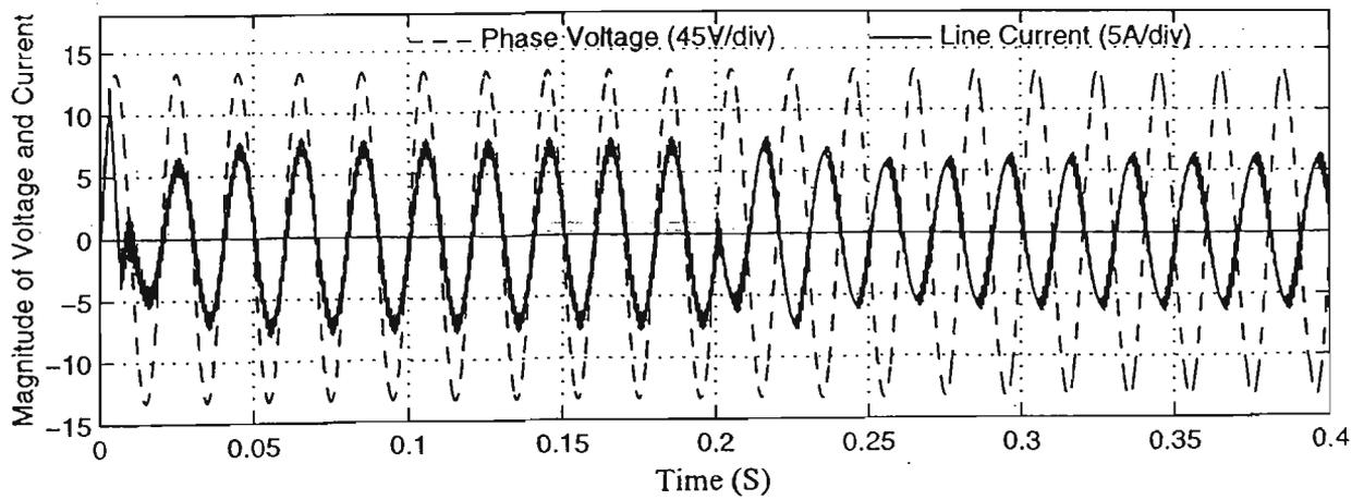
Fig. 4.23 Transient Performance of Line Current and Phase Voltage in the Load Change
