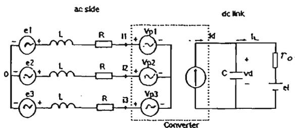
Figure 3: The equivalent circuit of the PWM converter
