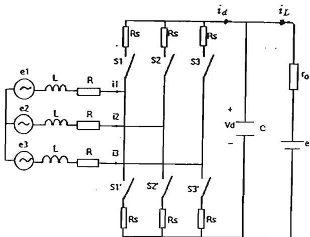
Figure 1: Schematic of an ac/dc PWM converter
