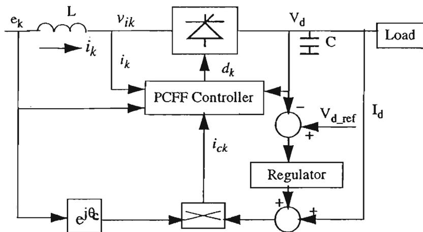
Fig. 1.11 Block Diagram of the PCFF Control
