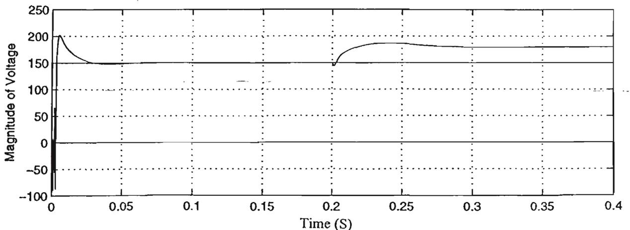
Fig. 4.18 Transient Performance of DC Output Voltage for an Input Change of 20% in  $V_{d-ref}$
