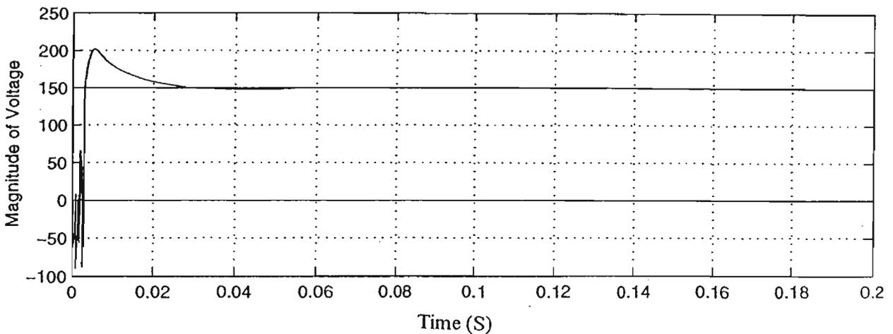
Fig. 4.10 Step Response of DC Output Voltage in the Rectifying mode
