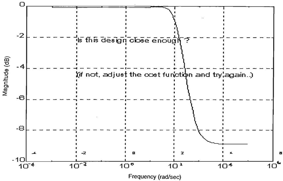
Fig. 3.6 The Gain Plot of the Optimal  $M(s)$
