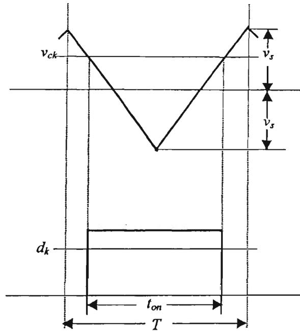
Fig. 2.3 The Waveform of Voltage Trigger Converter
