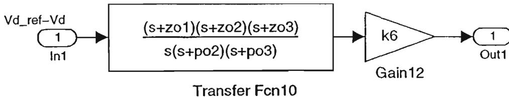
Fig. 4.7 The Configuration of the  $H_\infty$  Controller Subroutine
