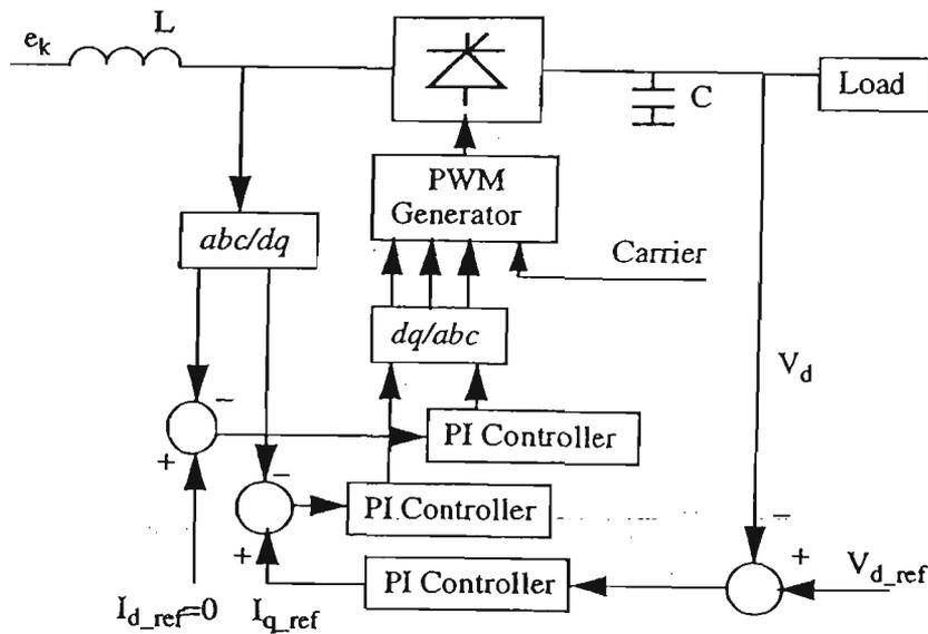
Fig. 1.10 Current Control in Rotating Frame
