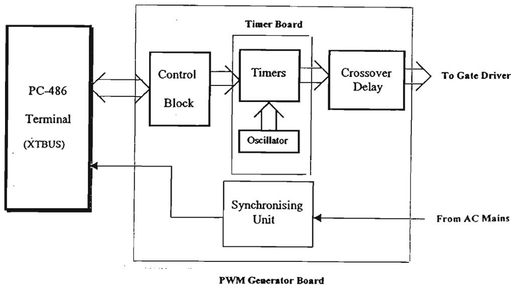
Fig. 5.9 Structure of PWM Generator Board
