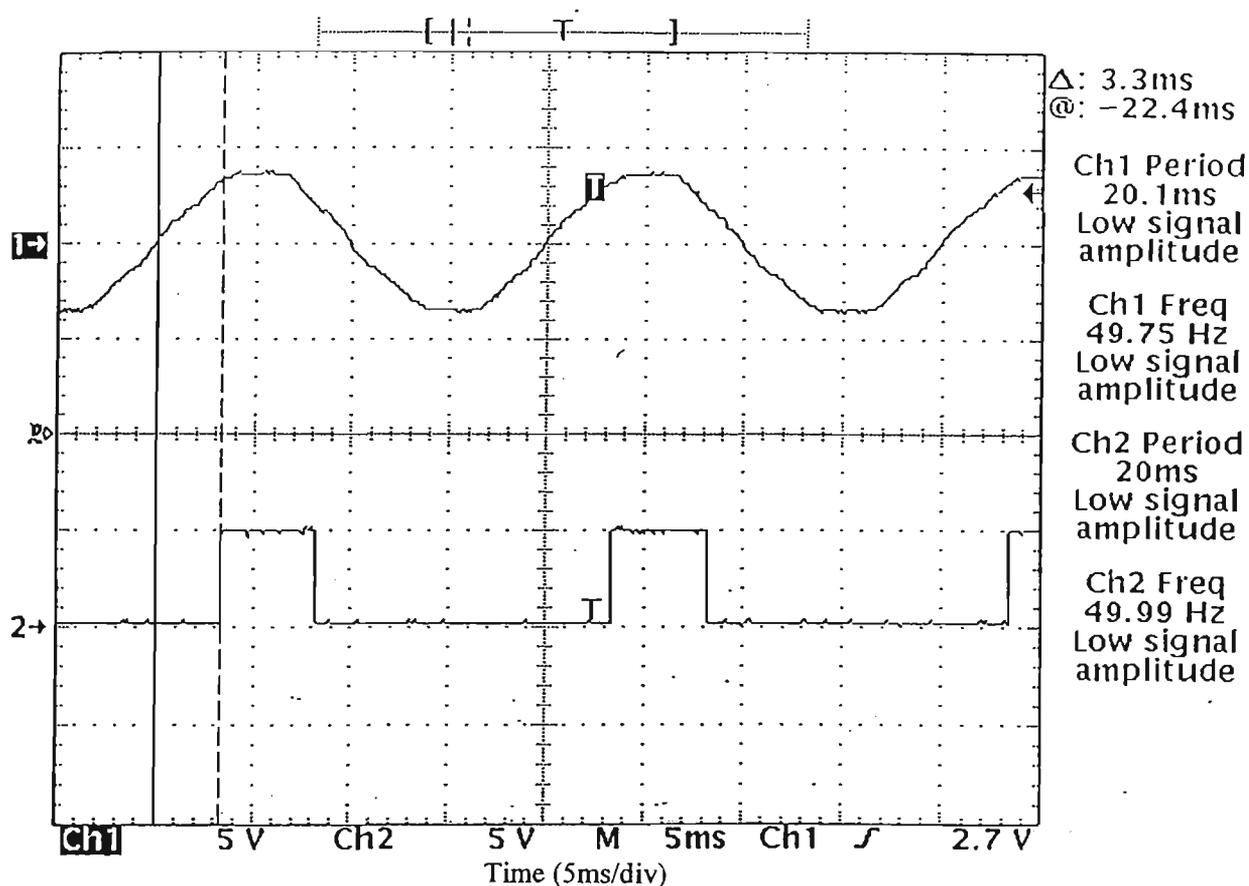
Fig. 6.2 Experimental Result of Synchronising Unit
