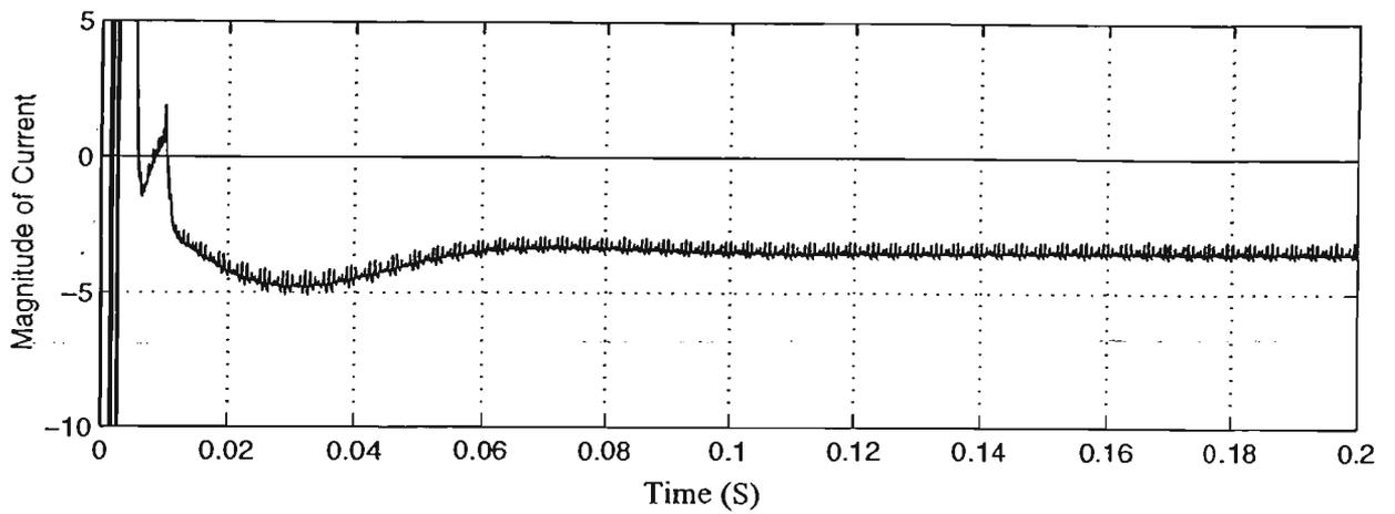
Fig. 4.16 Step Response of DC Output Current in the Regenerating Mode
