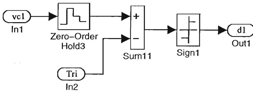
Fig. 4.4 The Configuration of the PWM Modulator Subroutine
