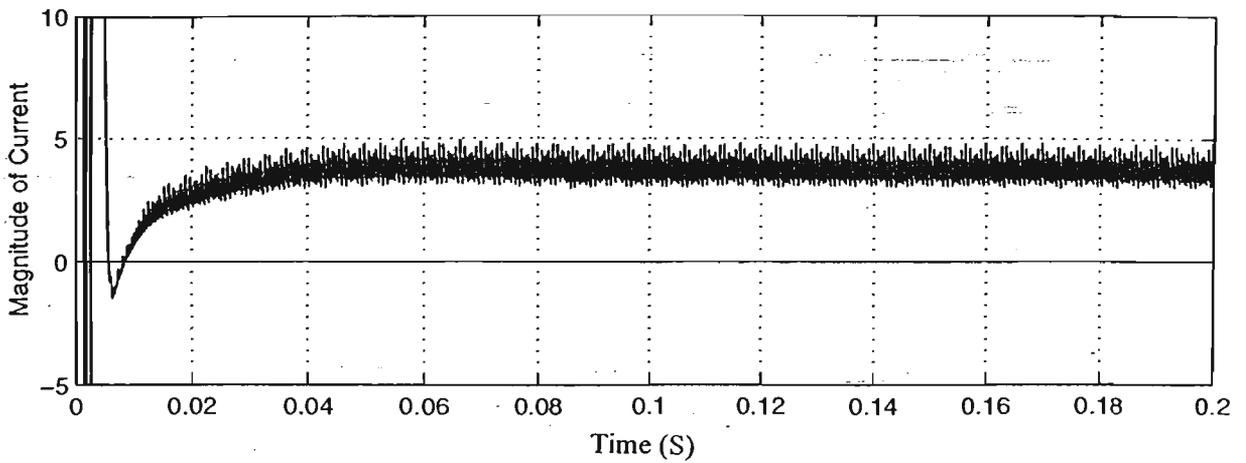
Fig. 4.11 Step Response of DC Output Current in the Rectifying Mode
