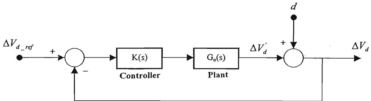
Fig. 3.4 The  $H_\infty$  Controlled PCFF Converter
