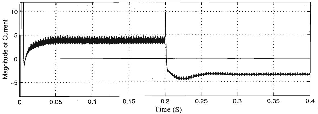
Fig. 4.22 Transient Performance of DC Output Current in the Load Change
