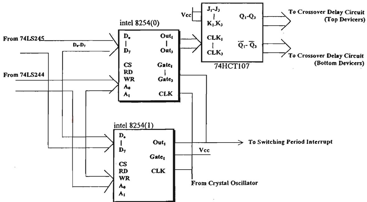
Fig. 5.11 Block Diagram of Timer board
