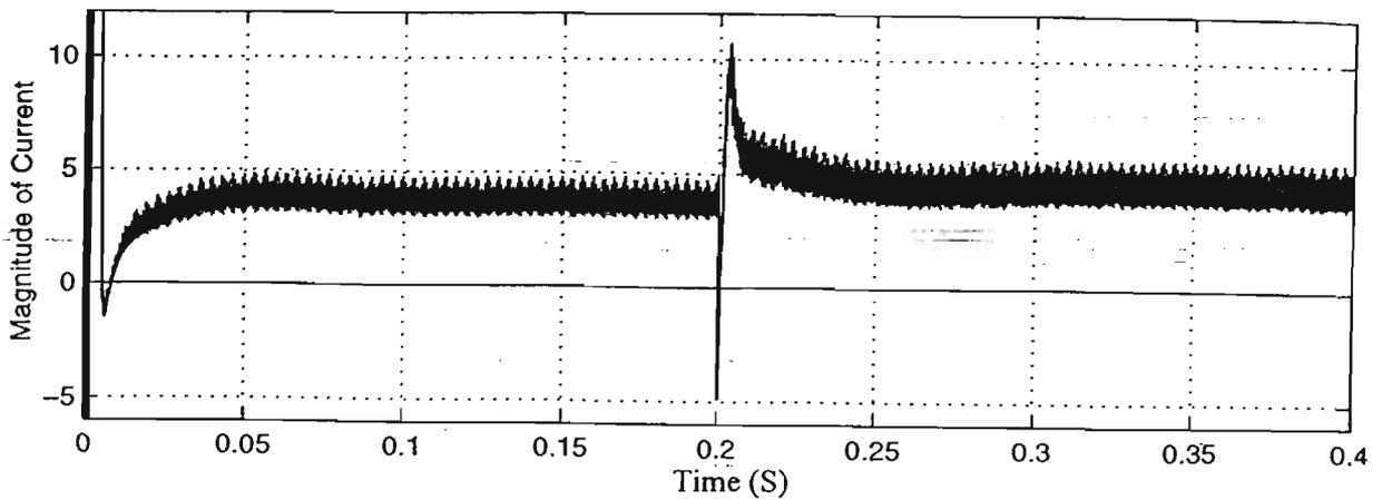
Fig. 4.19 Transient Performance of DC Output Current in the Input Change
