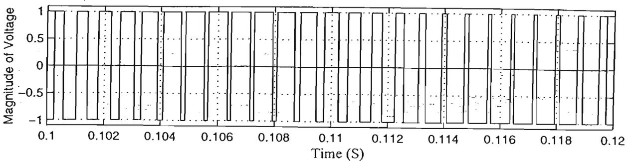
*Fig. 4.14 Steady-State Pulse Width Modulated Waveform in the Rectifying Mode*
