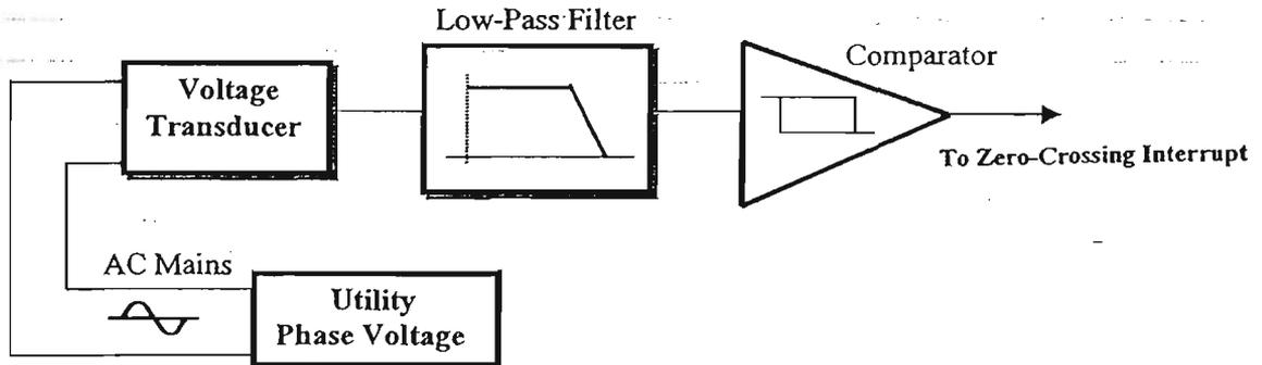
*Fig. 5.13 Block Diagram of Synchronising Unit*
