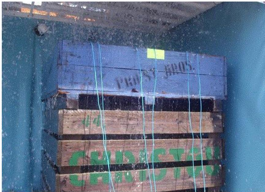
**Figure 6.16.** The box in which the instrumented pieces of broccoli were placed to measure their rate of cooling.
