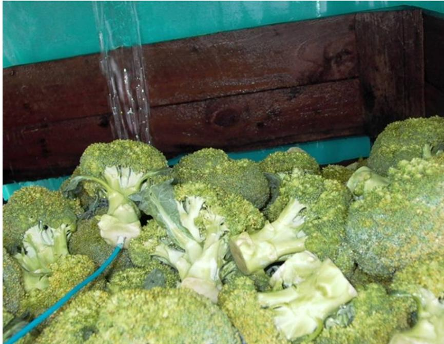
**Figure 6.17.** The instrumented broccoli in the hydrocooler.
