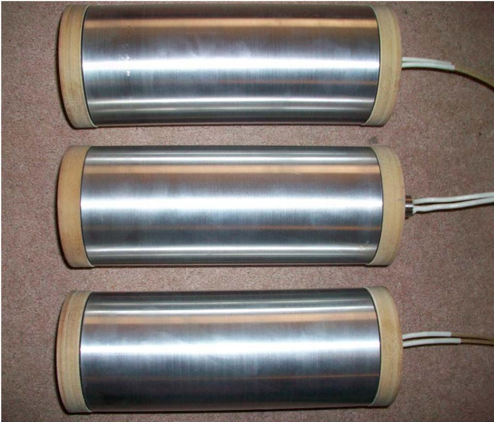
**Figure 2.18.** Photograph of the three cylinders with element heaters inside and Bakelite at both ends of each cylinder.
