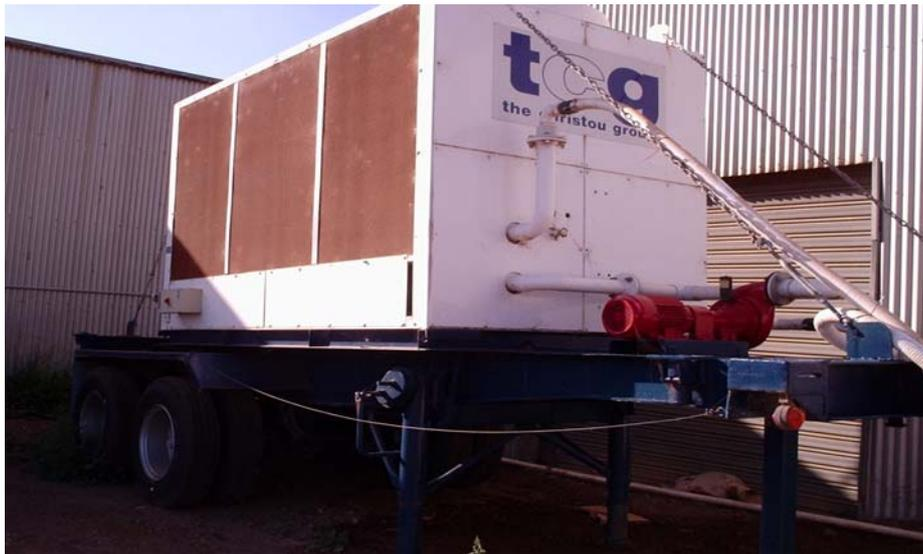
**Figure 6.7.** Water chilling unit supplies the hydrocooler with chilled water, and it is transported separately from the hydrocooler.
