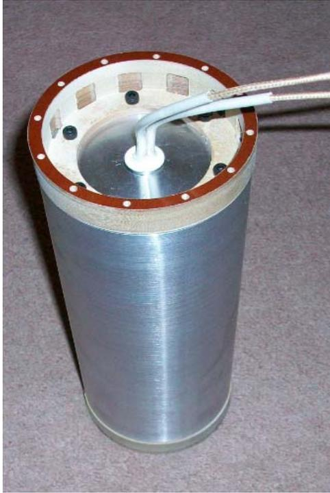
**Figure 2.16.** Photograph of one cylinder with element heater and inner part of the Bakelite insulation cap.
