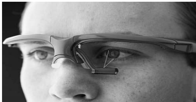
Figure 2.01: Optalert glasses (without prescription lenses) with IR emitters in the arm attached to the frame, showing the direction of the IR light pulses directed up at the eye (adapted from Johns, 2007 with permission).
