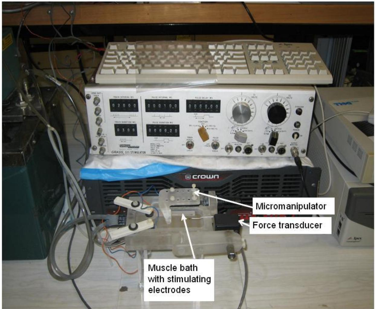
**Figure 3.1 Contractile machine setup used for stimulation protocols**
