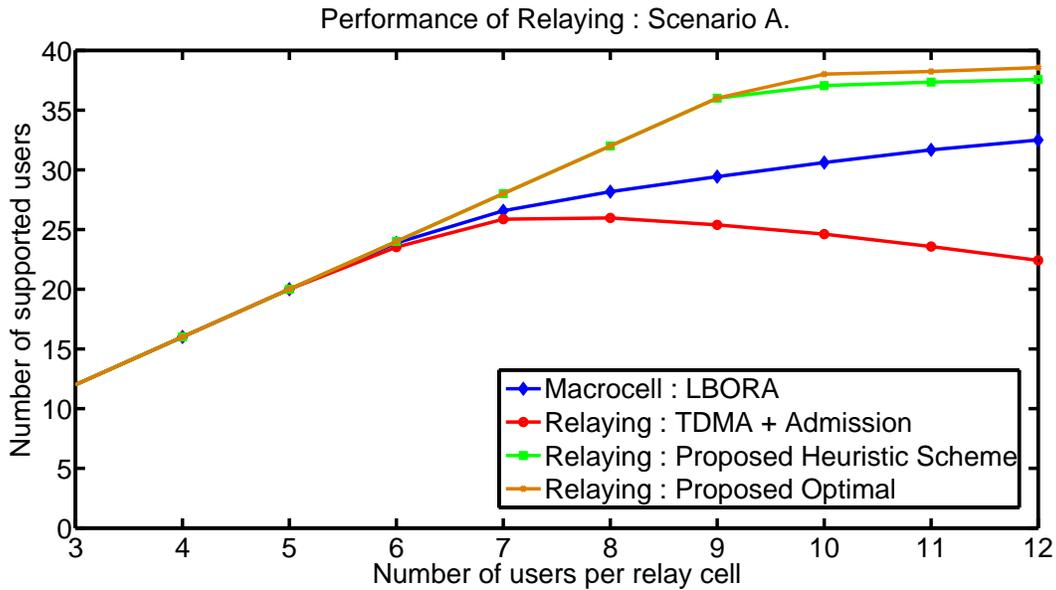
(a) Scenario A. Dense relay cell along with low link QoS constraints. Up to 12 users per relay, high PER of  $10^{-2}$  and 26 MCS values. There are 4 relays
