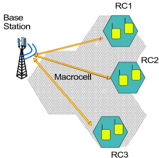
Figure 6.1: A set-up of multiple relays in a macrocell
