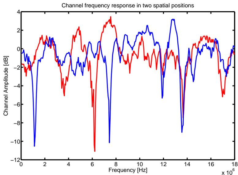
Figure 4.2: Normalised channel frequency response at two spatial positions. Obtained from a measurement outdoors in 18 MHz bandwidth and using 336 downlink reference symbols
