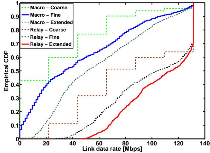
Figure 5.8: Performance comparison of various feedback schemes in distribution of data rate using 20 MHz bandwidth. The better performing curves are to the right.
