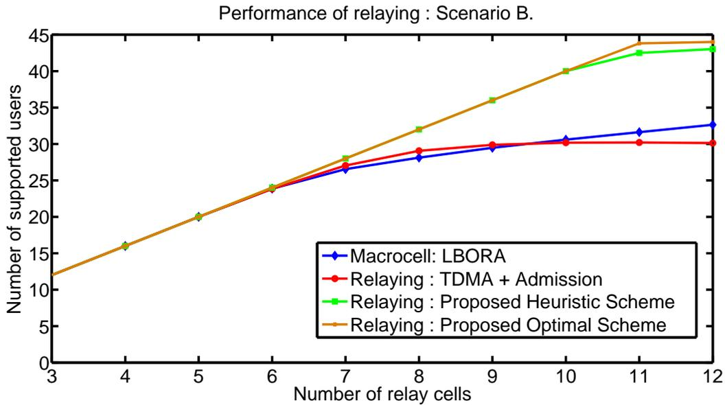
(b) Scenario B. Thin relay cells along with low QoS constraints. It has only 4 users per relay, high PER of  $10^{-2}$  and 26 MCS values. There are 4 users per relay
