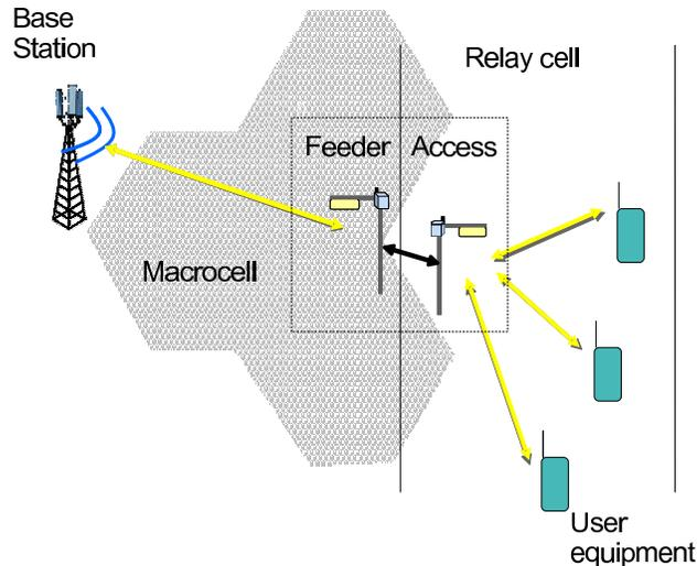
Figure 5.1: A cellular three terminal relay set-up
