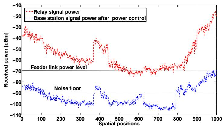
Figure 6.4: Results showing suppression of interference in indoor locations from the base station
