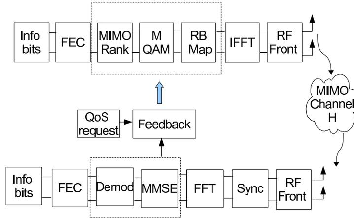
Figure 5.3: Functional blocks of OFDM air interface transceiver
