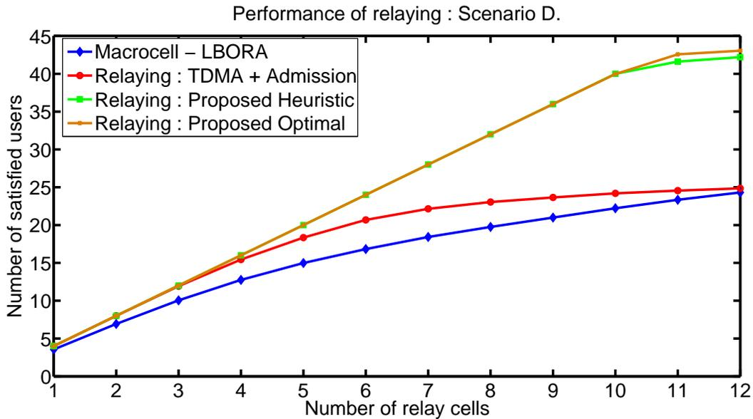
(b) Scenario D. Thin relay cells along with high link QoS constraints. It has only 4 users per relay but low PER of  $10^{-6}$  and only 4 MCS values. There are 4 users per relay
