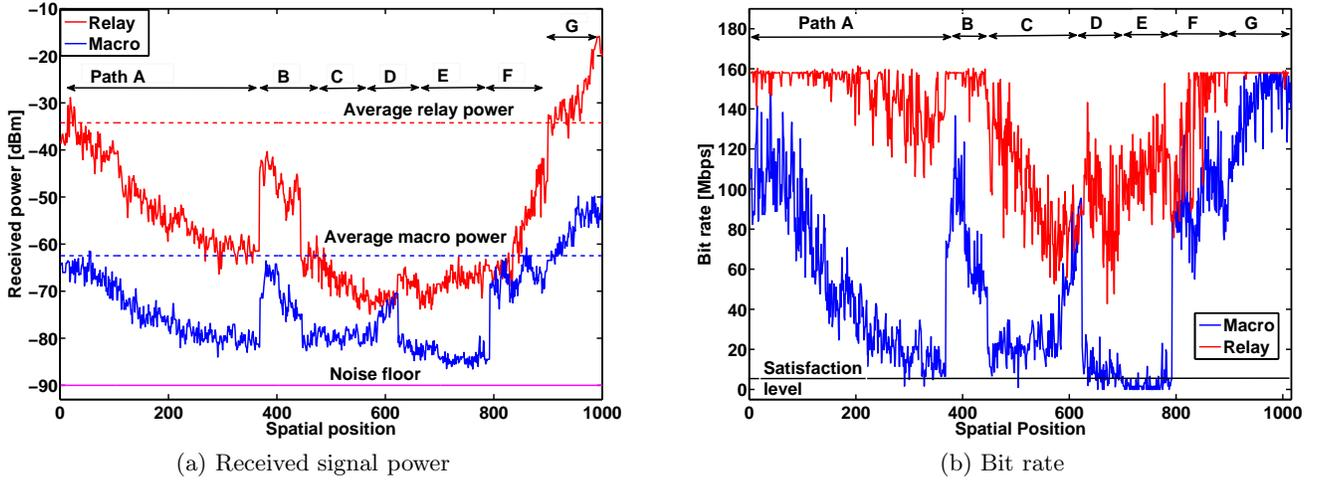
Figure 5.6: Measurements comparing coverage with and without a relay using  $2 \times 2$  MIMO in OFDM for 20 MHz bandwidth
