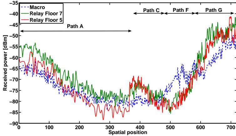
Figure 5.7: Relay coverage in different floors
