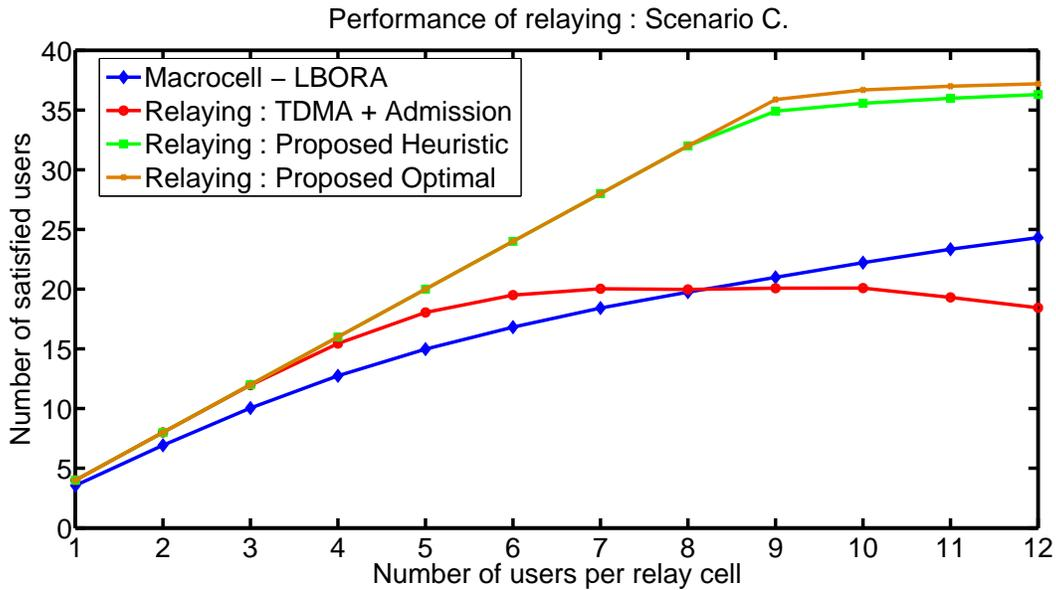
(a) Scenario C. Dense relay cell along with high link QoS constraints. Up to 12 users per relay but low PER of  $10^{-6}$  and only 4 MCS values. There are 4 relays
