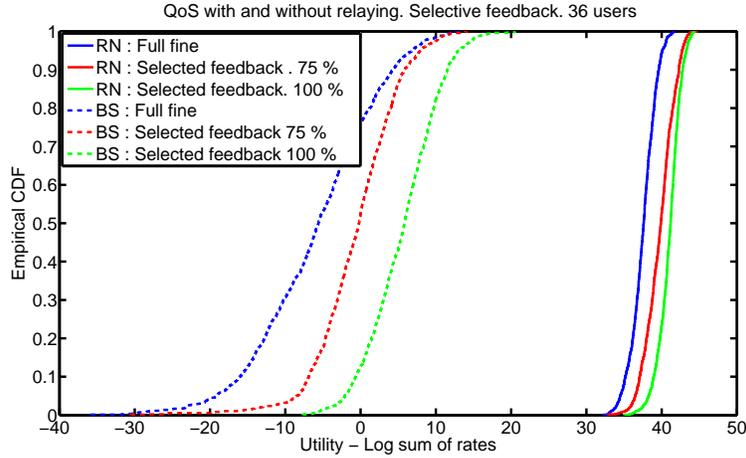
Figure 5.10: Performance of user selective feedback for proportional fairness, shown with and without relaying. The results demonstrate the effectiveness of feedback allocation based on user location.
