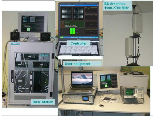
Figure 2.4: Main units of the experimental real-time test-bed
