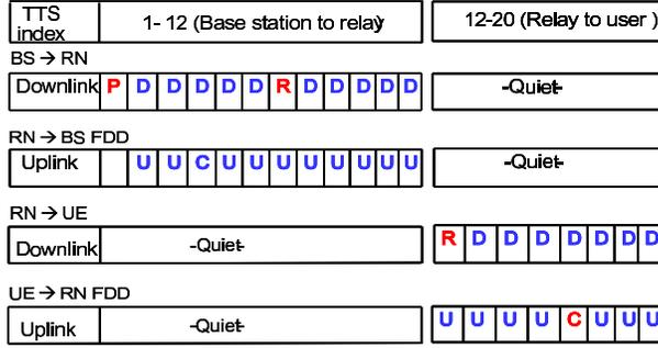
Figure 5.2: Timing diagram of decode and forward FDD relaying. D-downlink data, U- uplink data, R- radio resource management, P- AB/TA preambles, C-channel quality indicator, TTS - transmit time slot.
