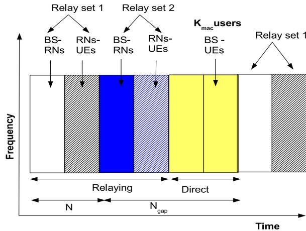
Figure 6.2: Frame diagram showing dedicated time slots for relaying
