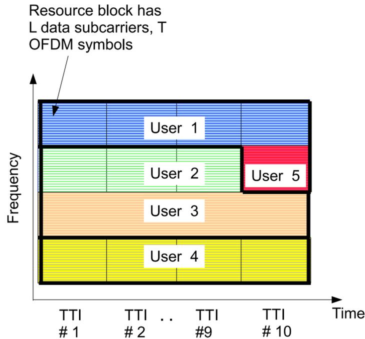
Figure 2.1: Illustration of resource allocation in OFDMA. Resource blocks and transmit time intervals (TTIs) are allocated to different users.
