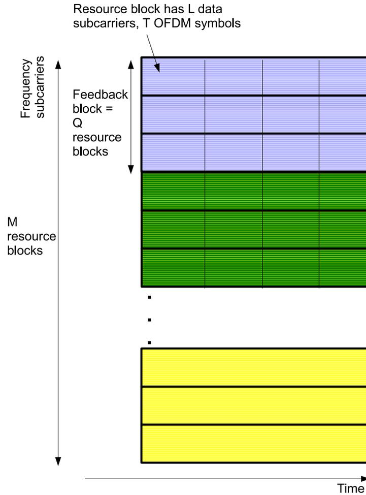
Figure 5.4: Description of feedback block. The example shows 3 resource blocks to make a feedback block.
