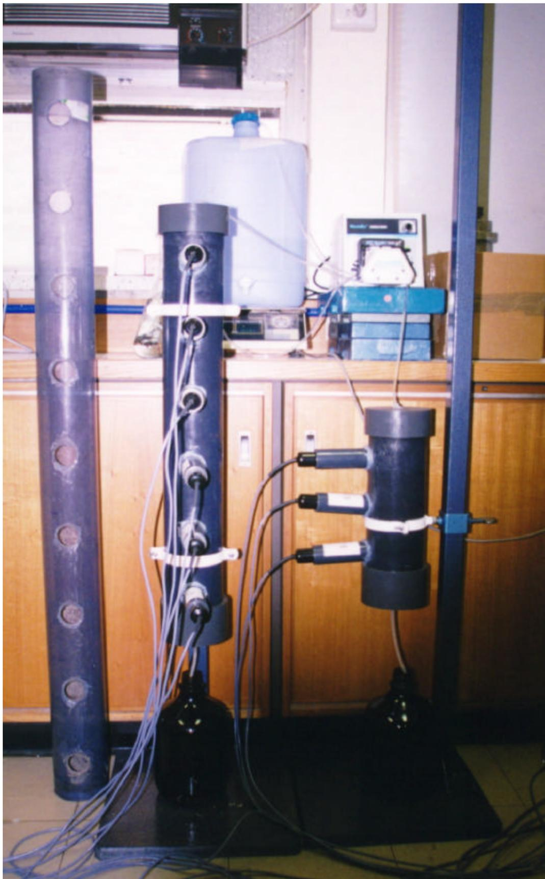
Figure 6.2 - Laboratory Setup of Ash Leaching Columns (Large, Medium & Small; L-R)
