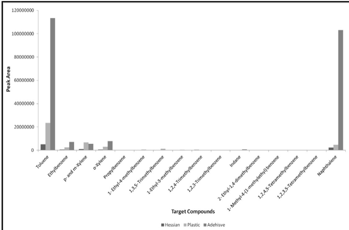
**Figures J1.14: Target Compound Chromatogram for Carpet Backing Components pyrolysed at 900°C**
