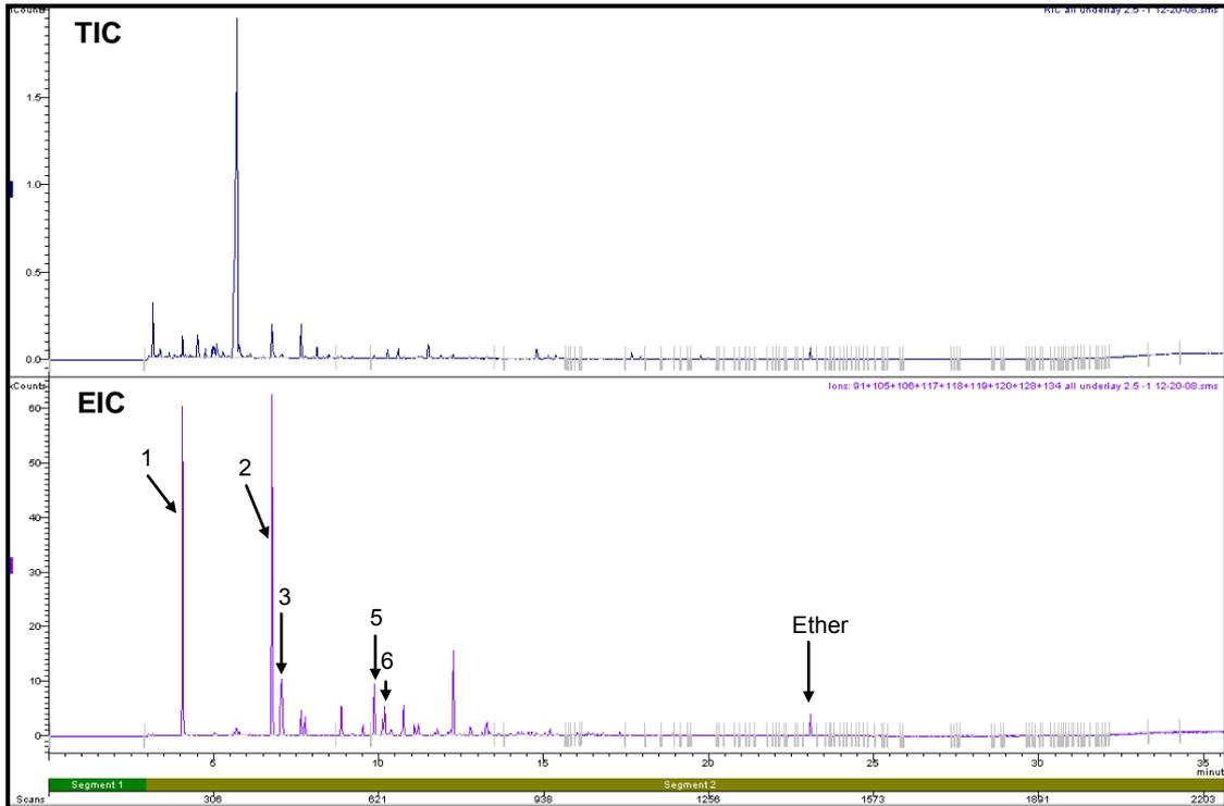
**Figure F2.2: Total Ion Chromatogram and Extracted Ion Chromatogram of Underlay Burnt in a Can with Lid On for 2.5 minutes**
