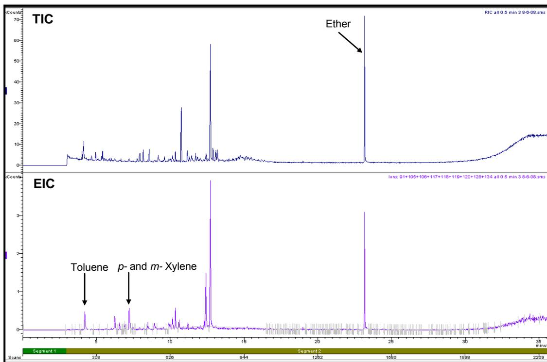
**Figure C1.2: Target Ion Chromatogram and Extracted Ion Chromatogram of a Nylon Carpet Swatch burnt in a Can with Lid On for 30 Seconds**
