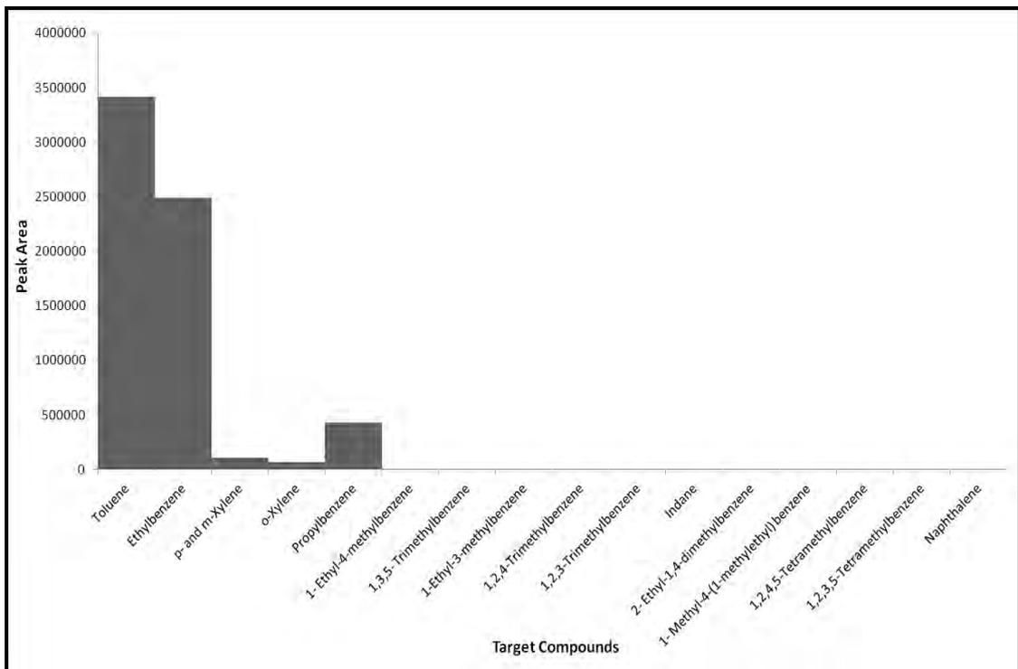
**Figure 4.45: Target Compound Chromatogram of a Polypropylene Carpet Swatch burnt in a Can with Lid On for 2.5 minutes**
