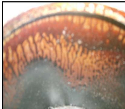
**Figure C1.17 (c): Inside of Can after Burning**
