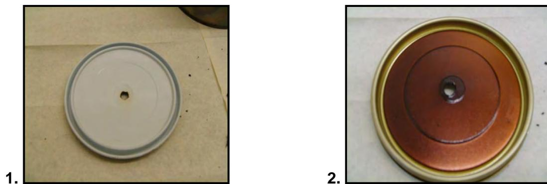
**Figure D3.1 (a): 1. Top and 2. Underside of Lid after Burning**
