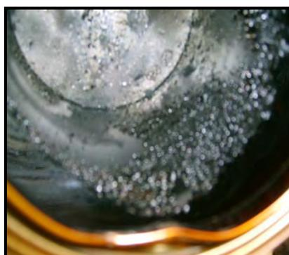
**Figure F1.3 (c): Inside of Can after Burning**
