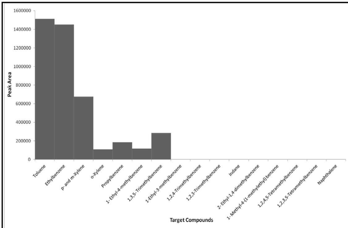
**Figure D1.12: Target Compound Chromatogram of a Polypropylene Carpet Switch burnt in a Can with Lid On for 10 minutes**
