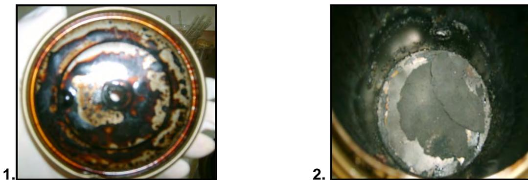
**Figure C1.29 (a): 1. Underside of Lid and 2. Sample in Bottom of Can after Burning**
