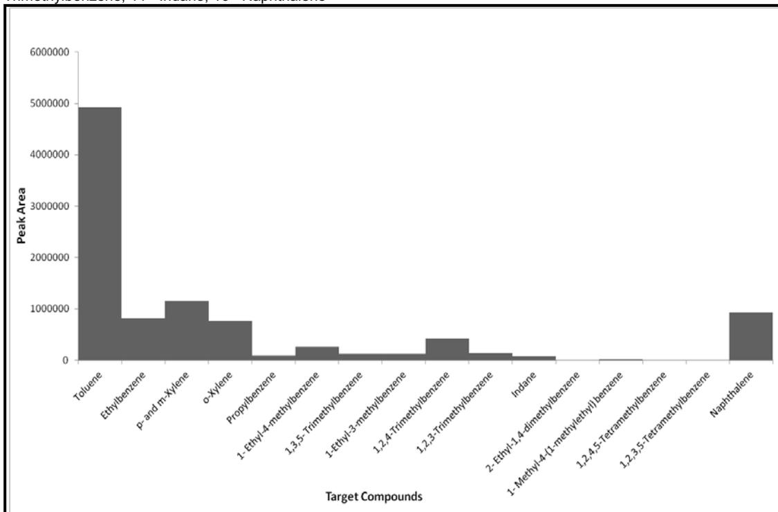
**Figure H2.4: Target Compound Chromatogram of Hessian Carpet Backing Pyrolysed at 750°C**
