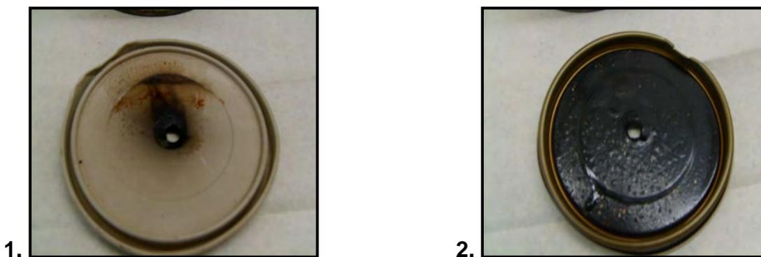
**Figure D3.10 (a): 1. Top of Lid and 2. Underside of Lid after Burning**
