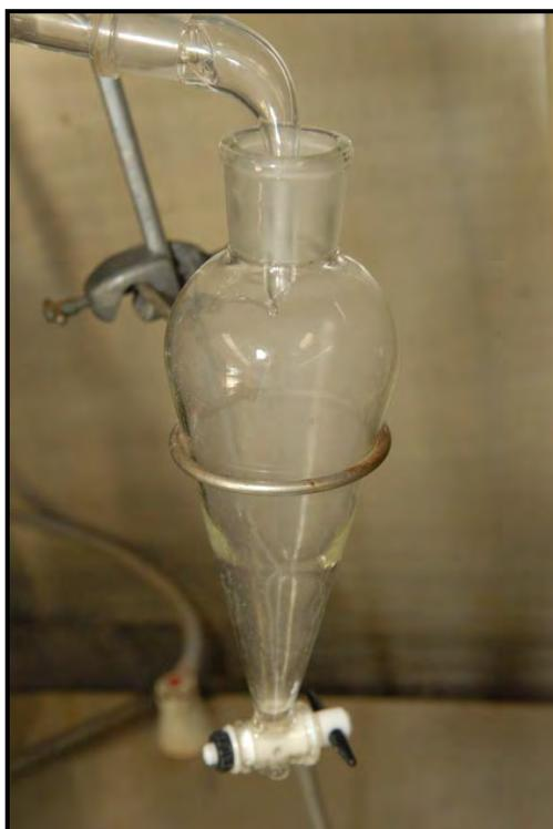
**Figure A1.1(e): Condensation of Steam and Volatiles in Separatory Funnel**
