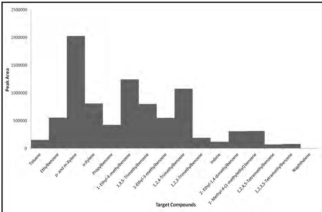
**Figure 3.41: Target Compound Chromatogram of KimWipe spiked with 100µL of 95% Evaporated Petrol**
