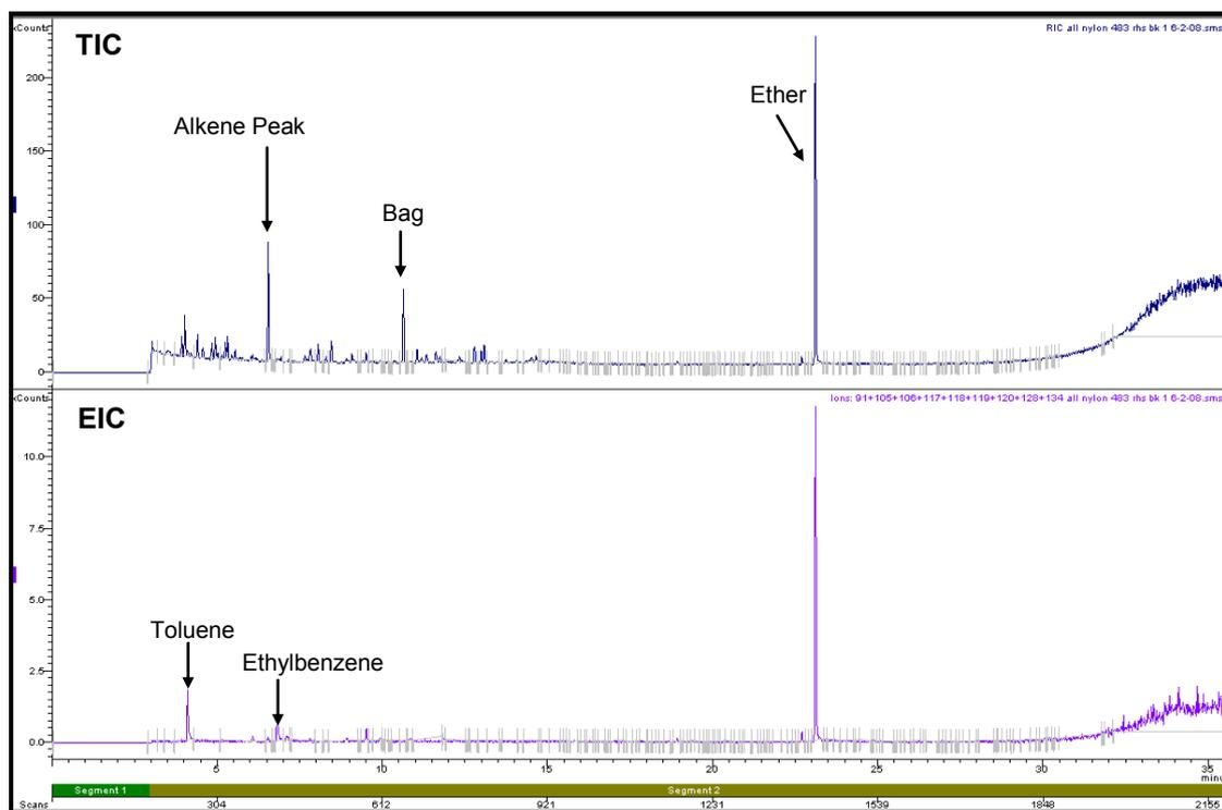
**Figure 4.17(c): Total Ion Chromatogram and Extracted Ion Chromatogram of Right Side-Back of the Nylon Carpet after Furnace Burn at 483°C (Refer to Section 2.5.1 for GC/MS conditions)**
