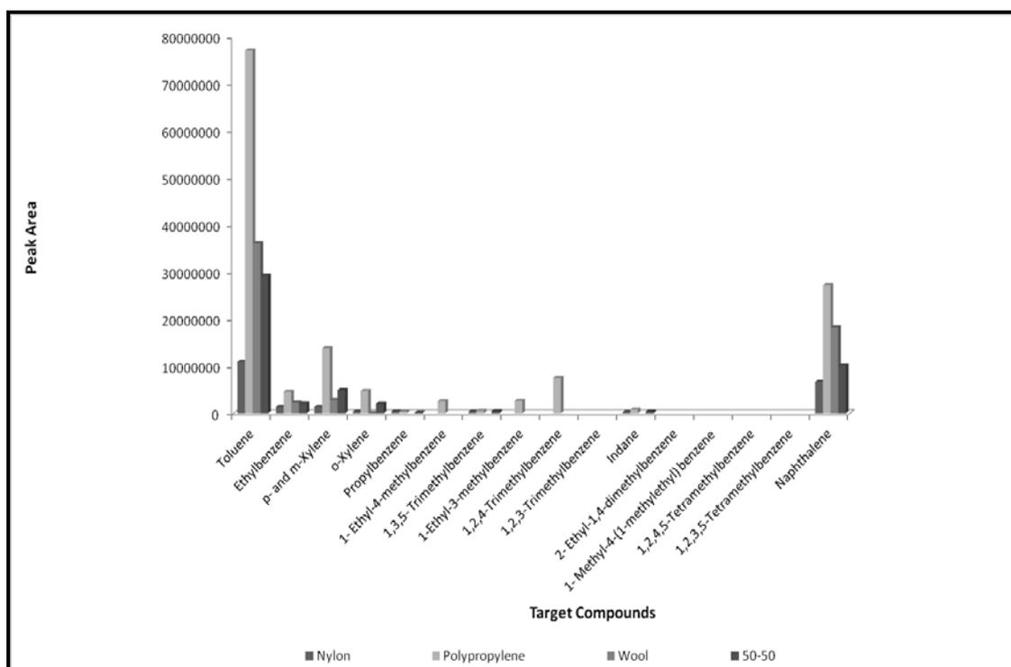
**Figures J1.10: Target Compound Chromatogram for all Carpet Fibres pyrolysed at 900°C**
