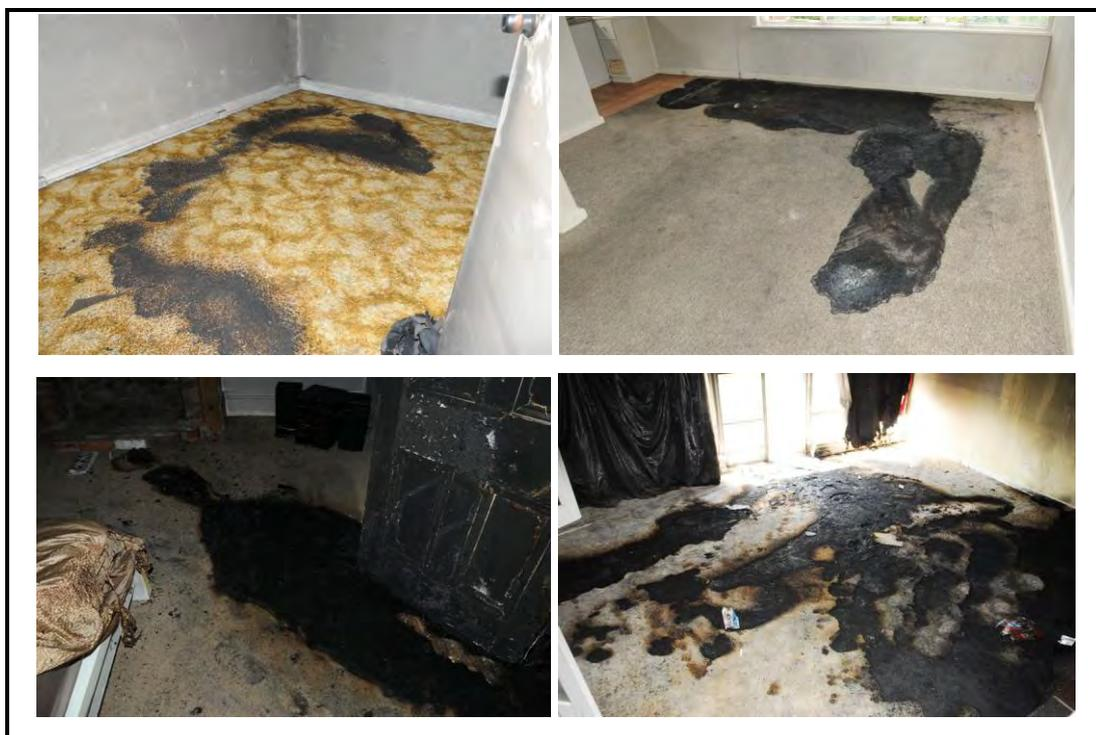
**Figure 1.2: Examples of Ignitable Liquid Trailers** (Courtesy of the Fire Investigation Unit at VPFSC)
