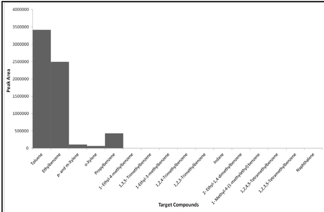
**Figure D1.3: Target Compound Chromatogram of a Polypropylene Carpet Swatch burnt in a Can with Lid On for 2.5 minutes**
