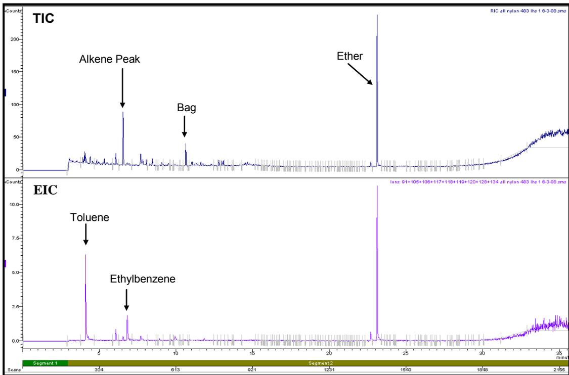
**Figure 4.17(a): Total Ion Chromatogram and Extracted Ion Chromatogram of Left Side of the Nylon Carpet after Furnace Burn at 483°C (Refer to Section 2.5.1 for GC/MS conditions)**
