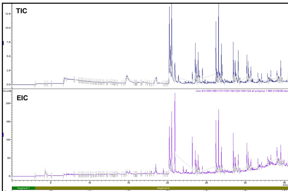
**Figure H7.6: Total Ion Chromatogram and EIC of 50-50 Polypropylene-Wool Fibres Pyrolysed at 450°C**
