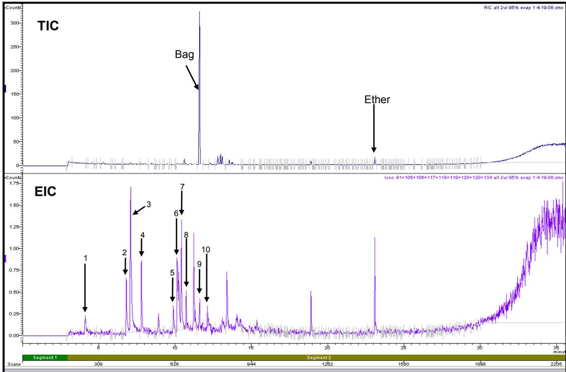
**Figure 3.52: Total Ion Chromatogram and Extracted Ion Chromatogram of KimWipe spiked with 2µL of 95% Evaporated Petrol (Refer to Section 2.5.1 for GC/MS conditions)**
