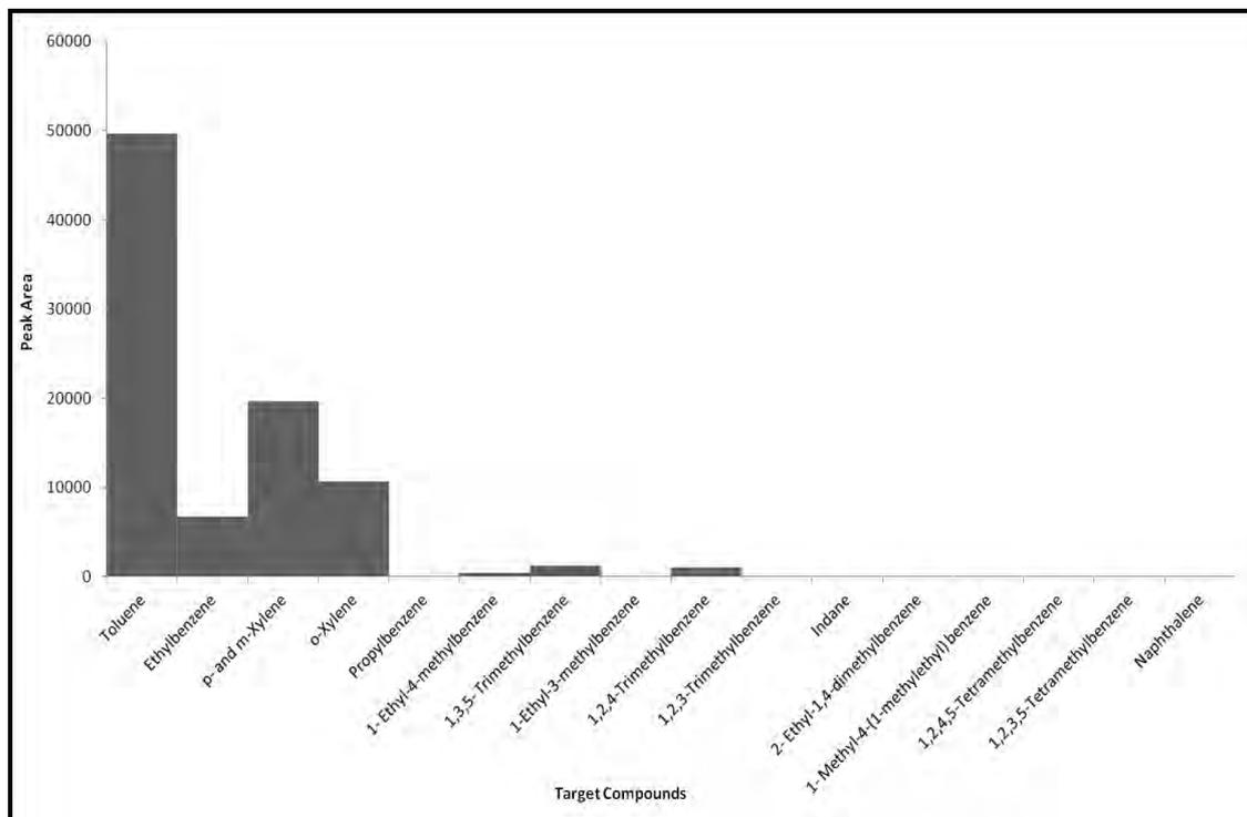
**Figure 3.49: Target Compound Chromatogram of KimWipe spiked with 2 $\mu$ L of Unevaporated Petrol**
