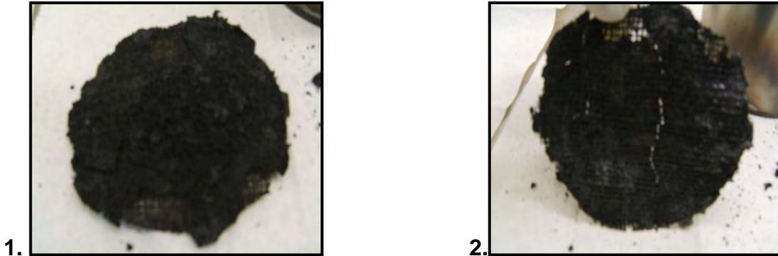
**Figure D2.10 (b): 1. Top and 2. Underside of Sample after Burning**
