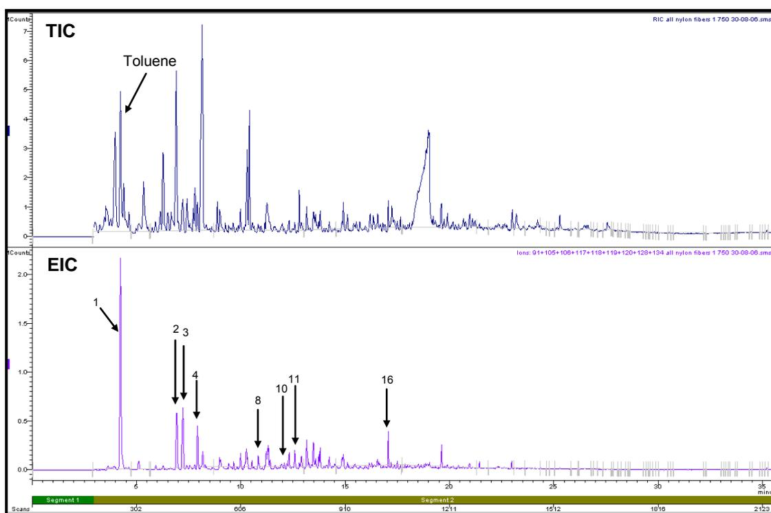
**Figure H1.3: Total Ion Chromatogram and Extracted Ion Chromatogram Nylon Fibres Pyrolysed at 750°C**
