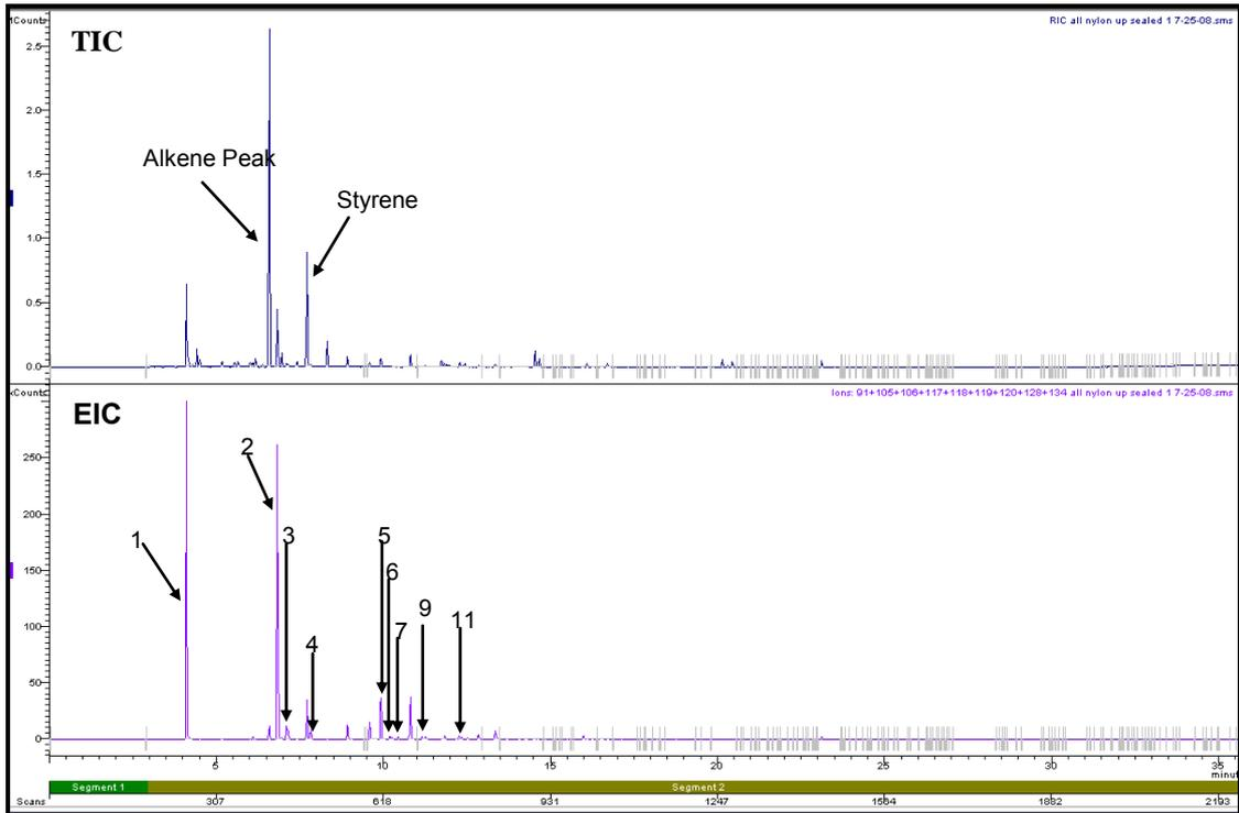
**Figure 4.35: Total Ion Chromatogram and Extracted Ion Chromatogram of Nylon Swatch placed in the Bottom of a Can burnt with Lid On (Refer to Section 2.5.1 for GC/MS conditions)**
