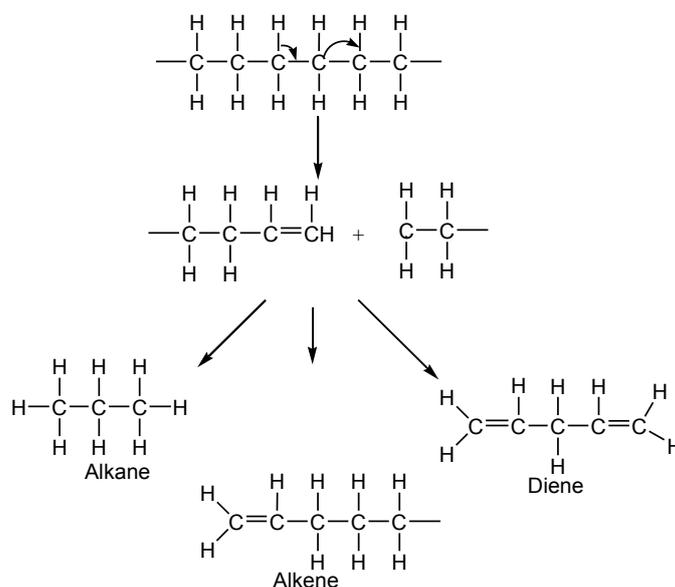
**Figure 1.10: Random Scission of Polyethylene**
