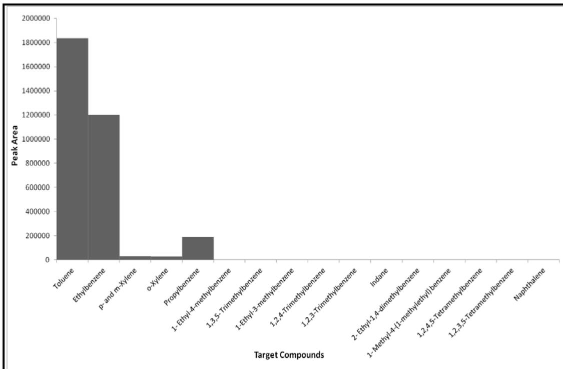
**Figure D2.3: Target Compound Chromatogram of a Wool Carpet Swatch burnt in a Can with Lid On for 2.5 minutes**
