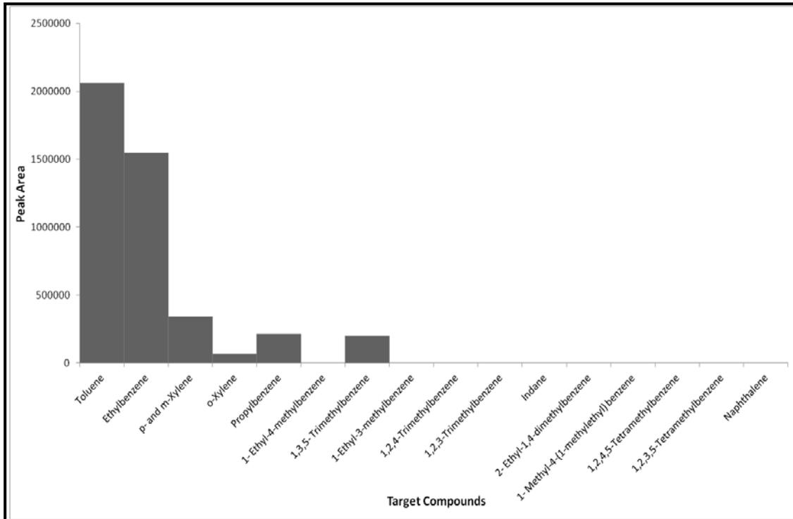
**Figure D1.9: Target Compound Chromatogram of a Polypropylene Carpet Swatch burnt in a Can with Lid On for 7.5 minutes**
