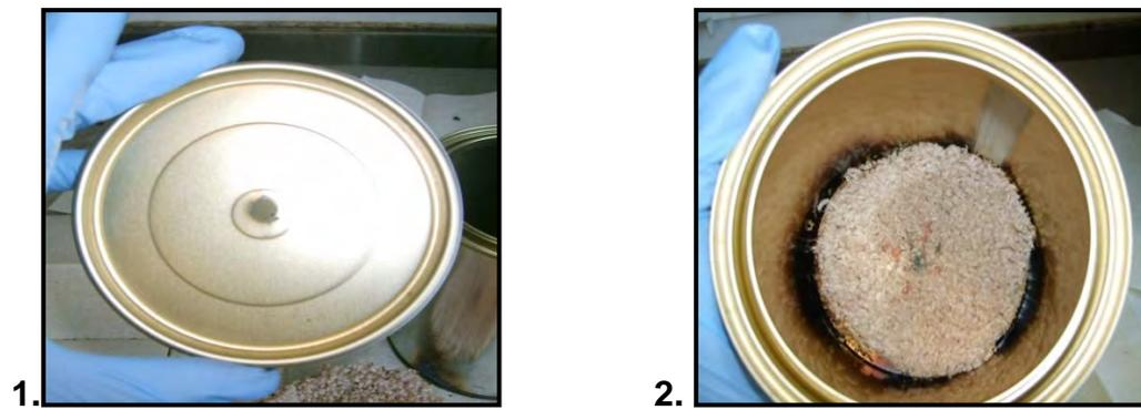
Figure C1.1 (a): 1. Underside of Lid and 2. Nylon Carpet in Bottom of Can after Burning
