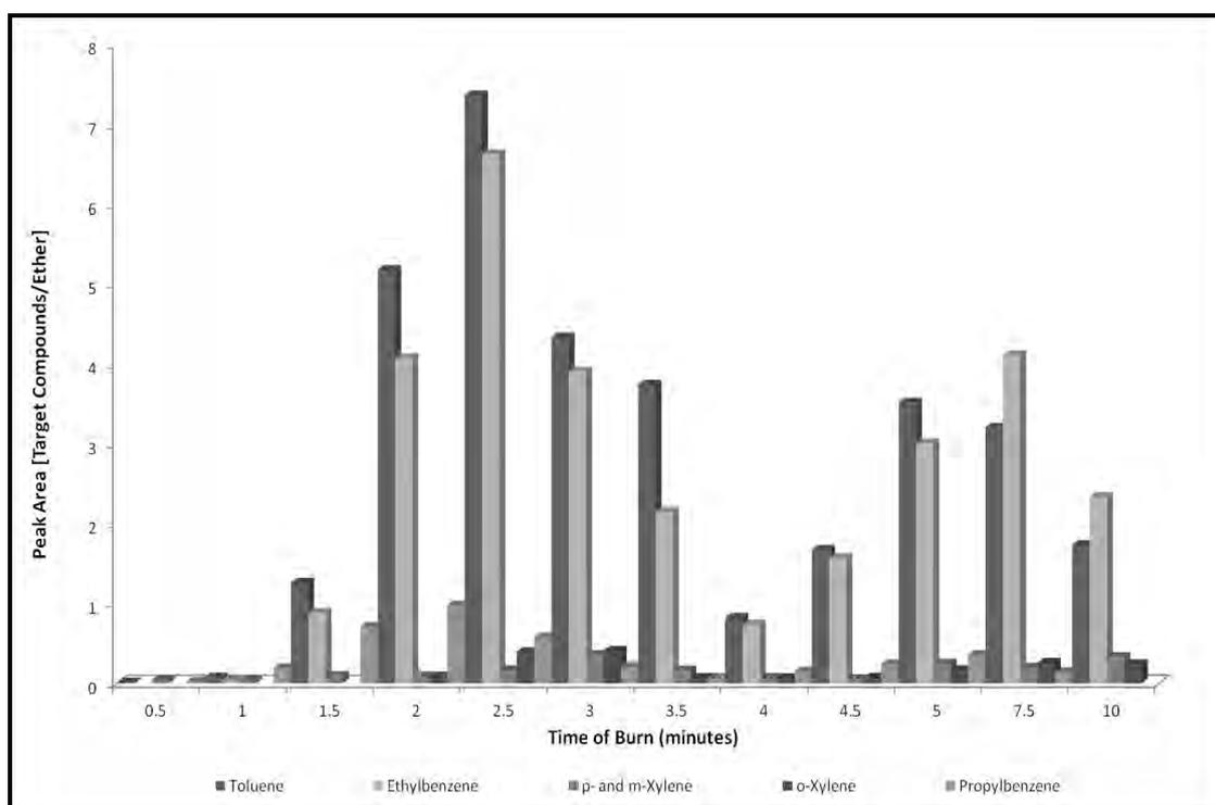
**Figure 4.40: Graph of Peak Area of Target Compounds with Butylated Hydroxytoluene vs. Burn Time**
