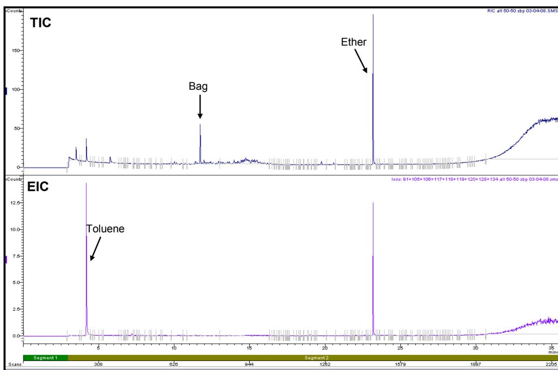
**Figure 4.1: Total Ion Chromatogram and Extracted Ion Chromatogram of the Substrate Background Products recovered from the 50-50 Polypropylene-Wool Carpet (Refer to Section 2.5.1 for GC/MS conditions)**
