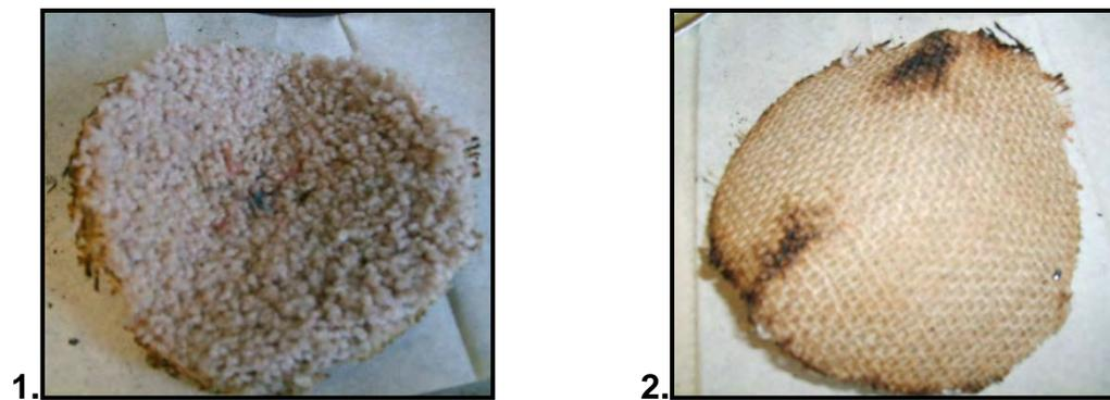
Figure C1.1 (b): 1. Top and 2. Underside of Sample after Burning
