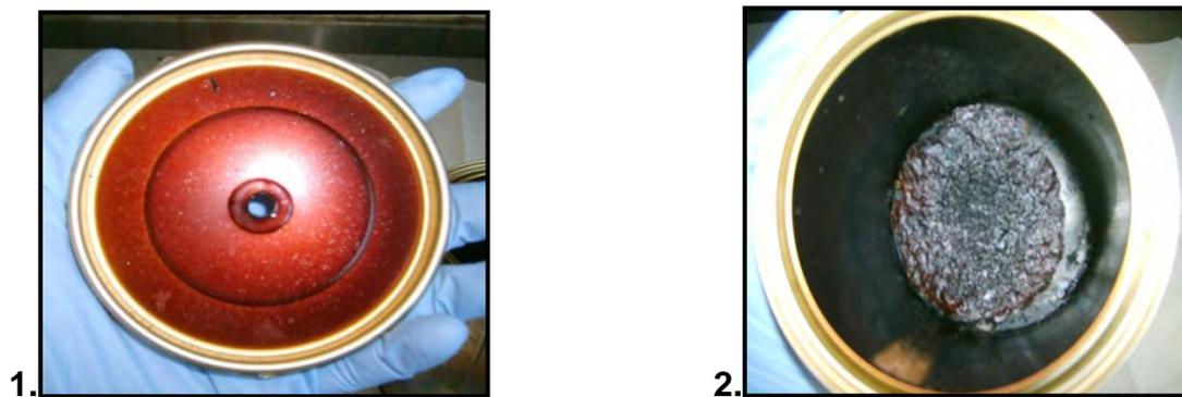
**Figure C1.9 (a): 1. Underside of Lid and 2. Sample in Bottom of Can after Burning**
