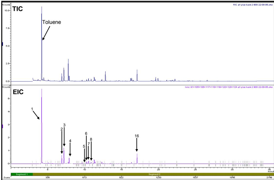
**Figure H3.1: Total Ion Chromatogram and Extracted Ion Chromatogram of Plastic Carpet Backing Pyrolysed at 900°C**
