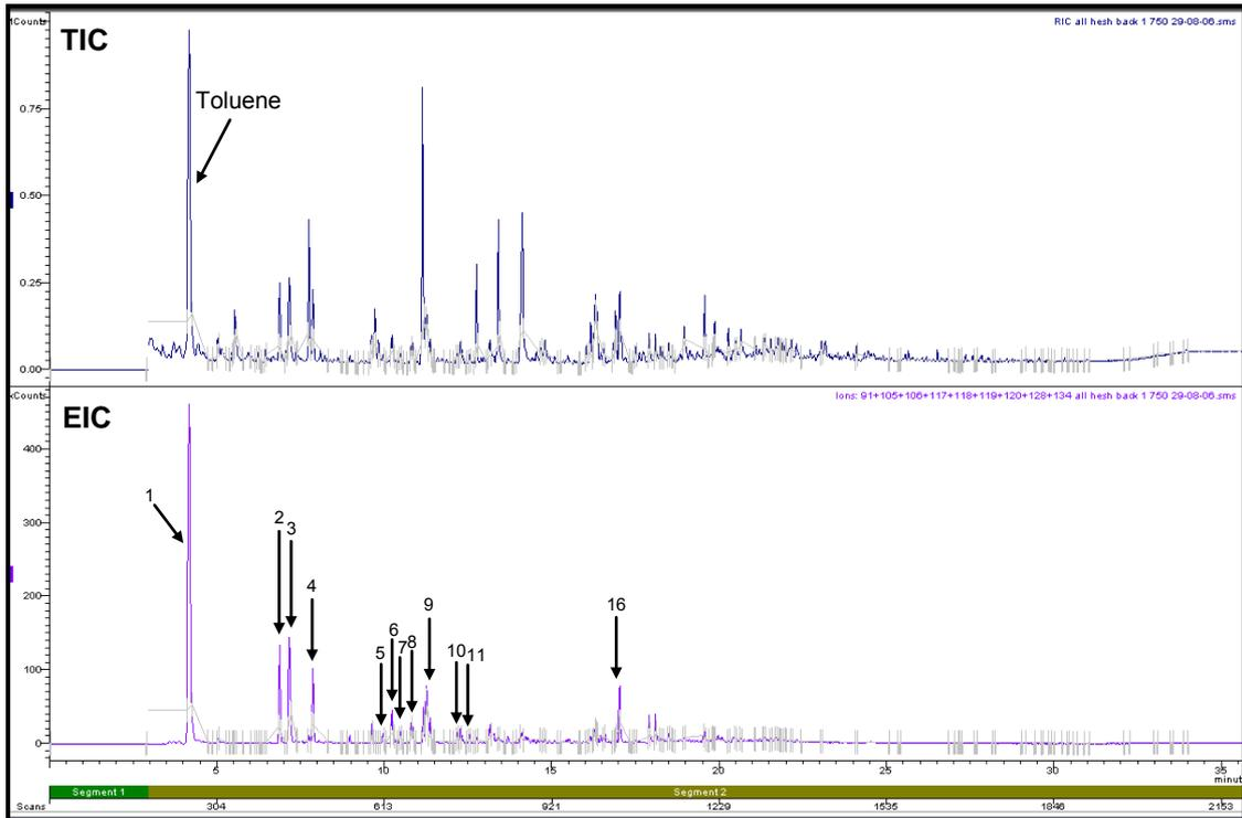
**Figure H2.3: Total Ion Chromatogram and Extracted Ion Chromatogram of Hessian Carpet Backing Pyrolysed at 750°C**
