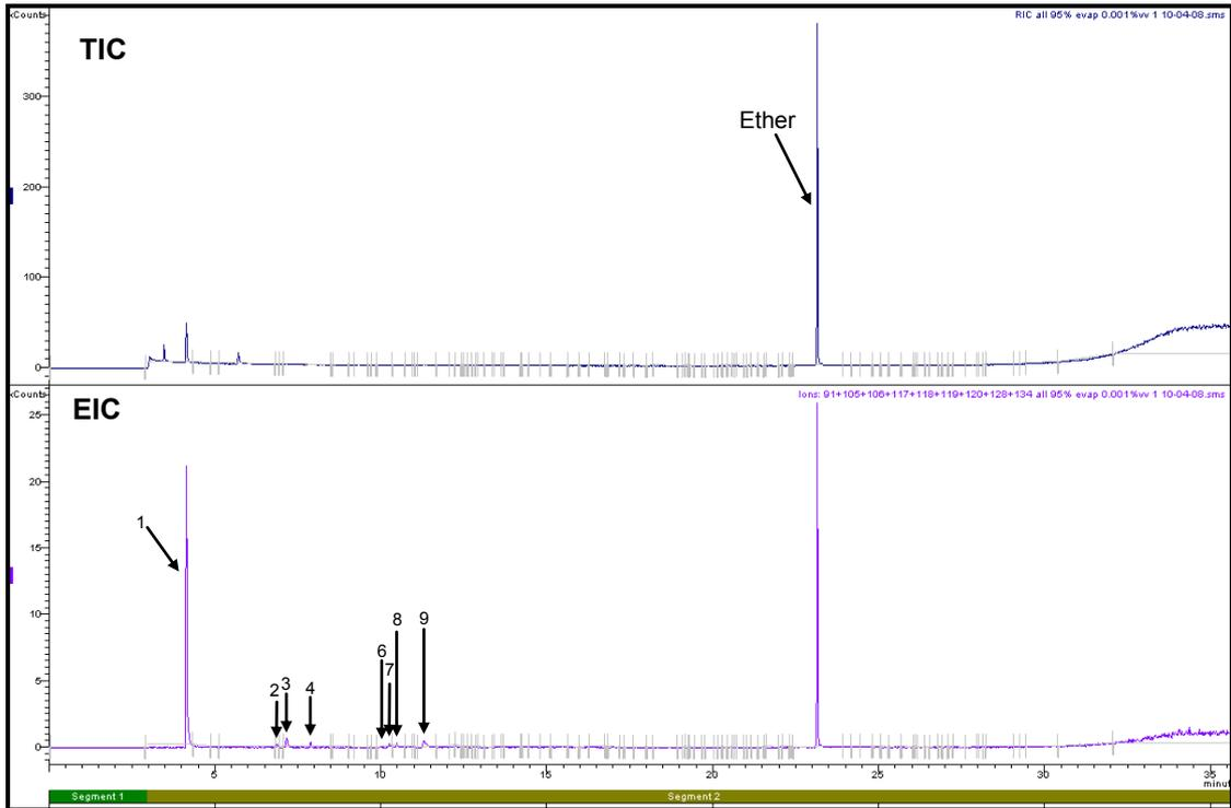
**Figure 3.32: Total Ion Chromatogram and Extracted Ion Chromatogram for 95% Evaporated Petrol Diluted to 0.001% (v/v) (Refer to Section 2.5.1 for GC/MS conditions)**
