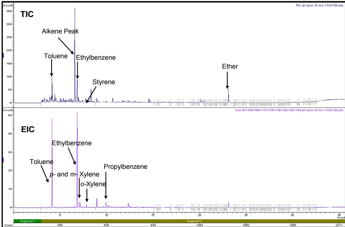
**Figure C1.30: Target Ion Chromatogram and Extracted Ion Chromatogram of a Nylon Carpet Swatch burnt in a Can with Lid On for 10 minutes**
