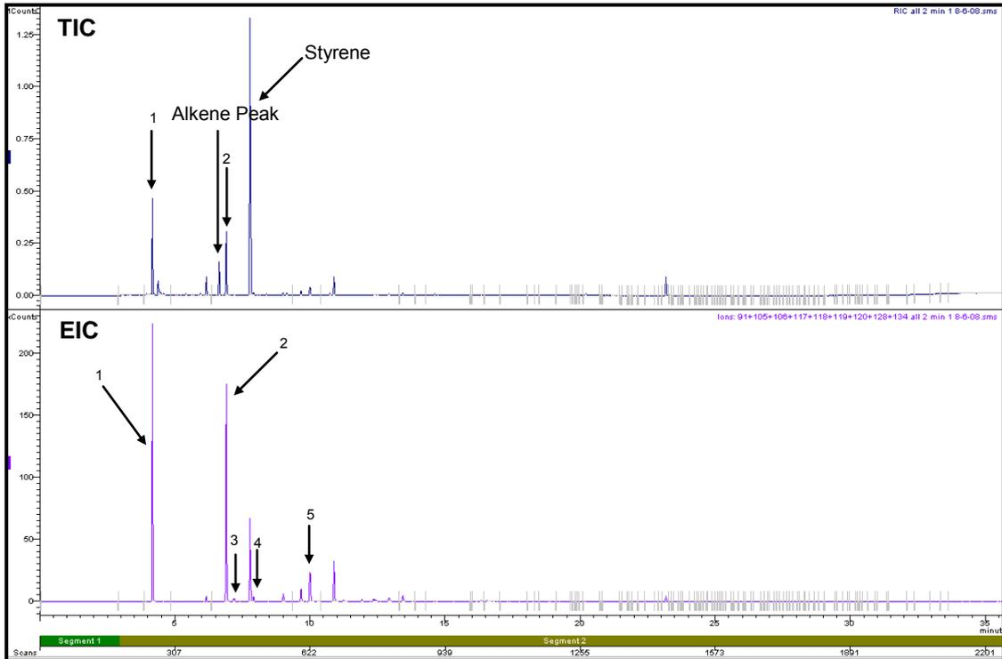
**Figure C1.8: Target Ion Chromatogram and Extracted Ion Chromatogram of a Nylon Carpet Swatch burnt in a Can with Lid On for 2 minutes**
