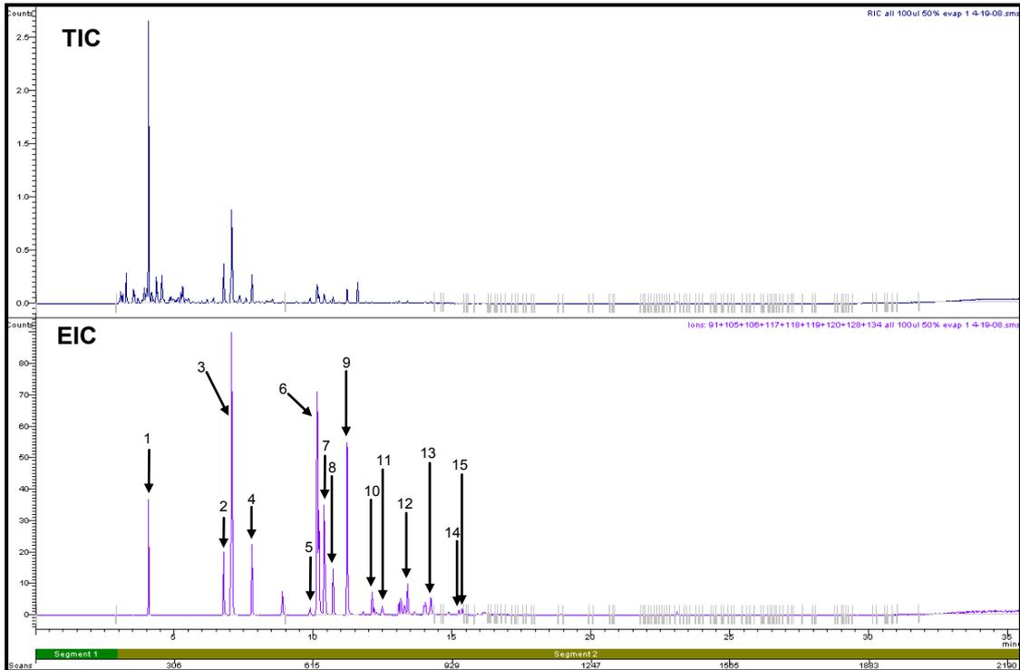
**Figure 3.38: Total Ion Chromatogram and Extracted Ion Chromatogram of KimWipe spiked with 100µL of 50% Evaporated Petrol (Refer to Section 2.5.1 for GC/MS conditions)**
