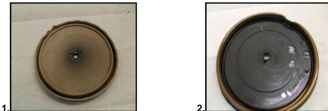
**Figure F2.12 (a): 1. Top and 2. Underside of Lid after Burning**
