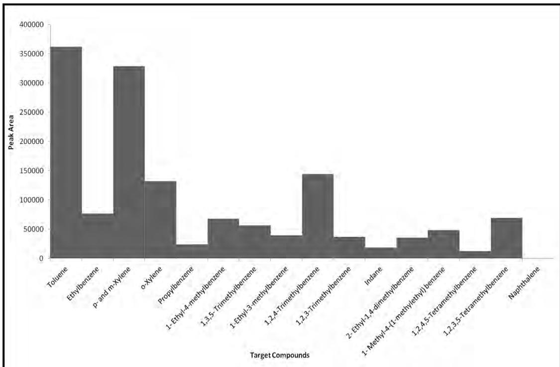
**Figure 3.19: Target Compound Chromatogram for 50% Evaporated Petrol Diluted to 0.1% (v/v)**
