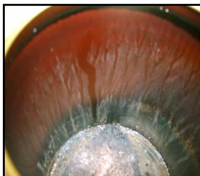
**Figure D1.4 (c): Inside of Can after Burning**
