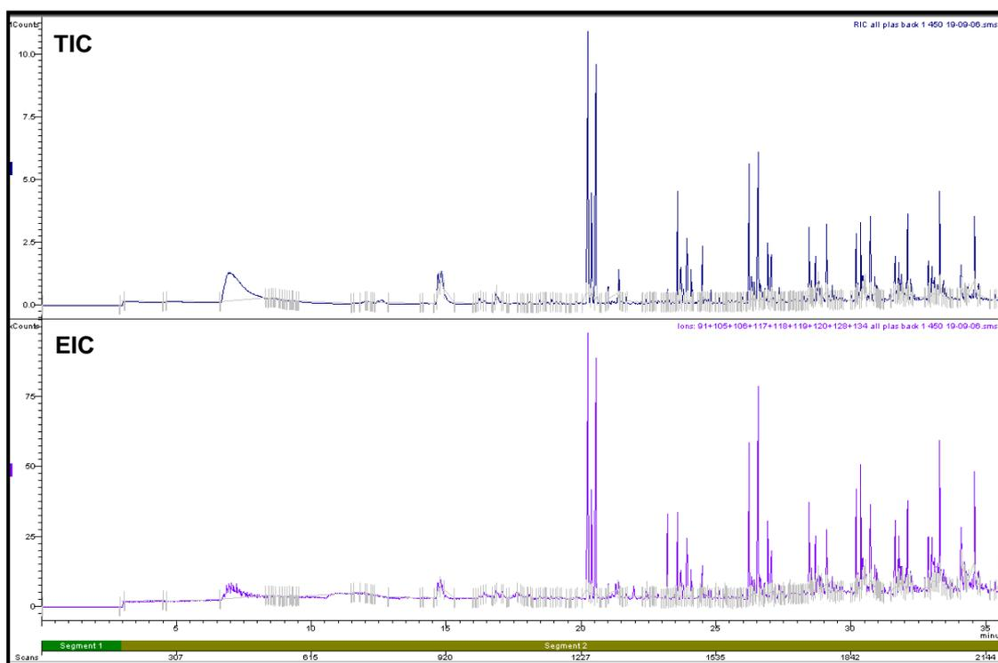
**Figure H3.7: Total Ion Chromatogram and Extracted Ion Chromatogram of Plastic Carpet Backing Pyrolysed at 450°C**
