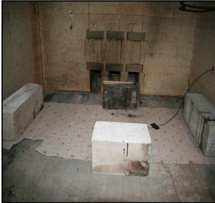
**Figure 2.6: Nylon Carpet Swatch placed on Bottom of Furnace with Hebel Bricks**
