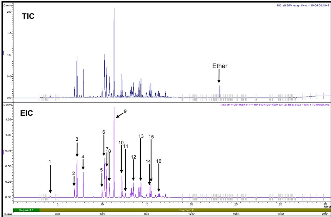
**Figure 3.14: Total Ion Chromatogram and Extracted Ion Chromatogram for 95% Evaporated Petrol Diluted to 1% (v/v) (Refer to Section 2.5.1 for GC/MS conditions)**
