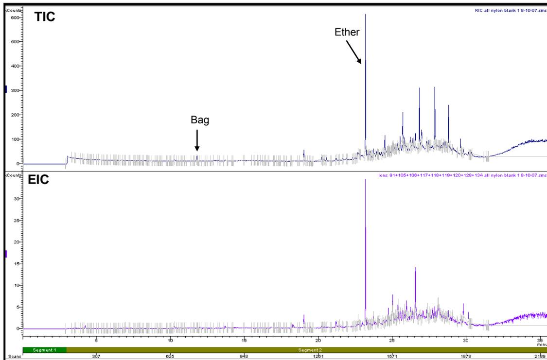
**Figure A1.2(a): Target Ion Chromatogram and Extracted Ion Chromatogram of Nylon Carpet burnt in Room 1**
