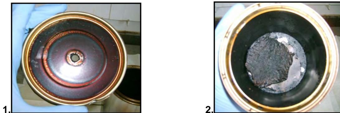
**Figure C1.11 (a): 1. Underside of Lid and 2. Sample in Bottom of Can after Burning**
