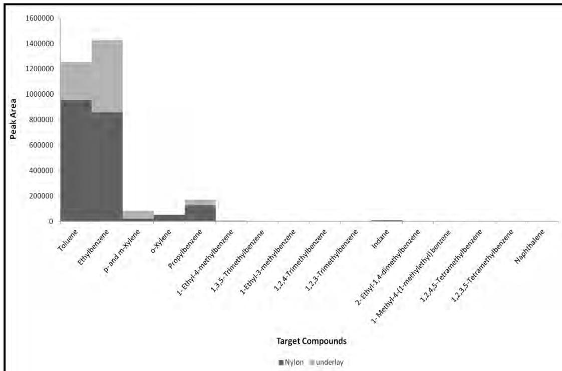
**Figure 5.6: Target Compound Chromatogram of Nylon Carpet superimposed with Underlay burnt in a Small Can with Lid On for 2.5 minutes**
