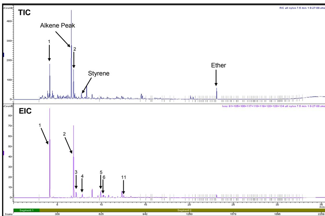
**Figure C1.27: Target Ion Chromatogram and Extracted Ion Chromatogram of a Nylon Carpet Swatch burnt in a Can with Lid On for 7.5 minutes**
