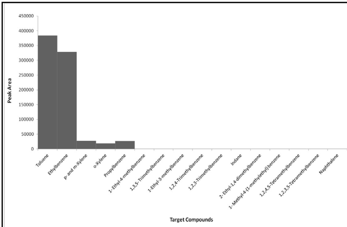
**Figure C1.25: Target Compound Chromatogram of a Nylon Carpet Swatch burnt in a Can with Lid On for 5 minutes**
