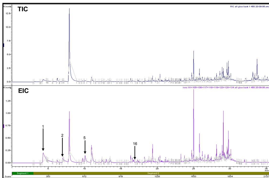
**Figure H4.7: Total Ion Chromatogram and Extracted Ion Chromatogram of Adhesive from Carpet Backing Pyrolysed at 450°C**
