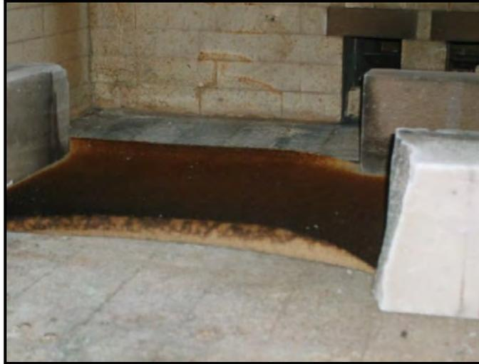
**Figure 4.24: Wool Carpet after the Furnace Burn at 230°C**
