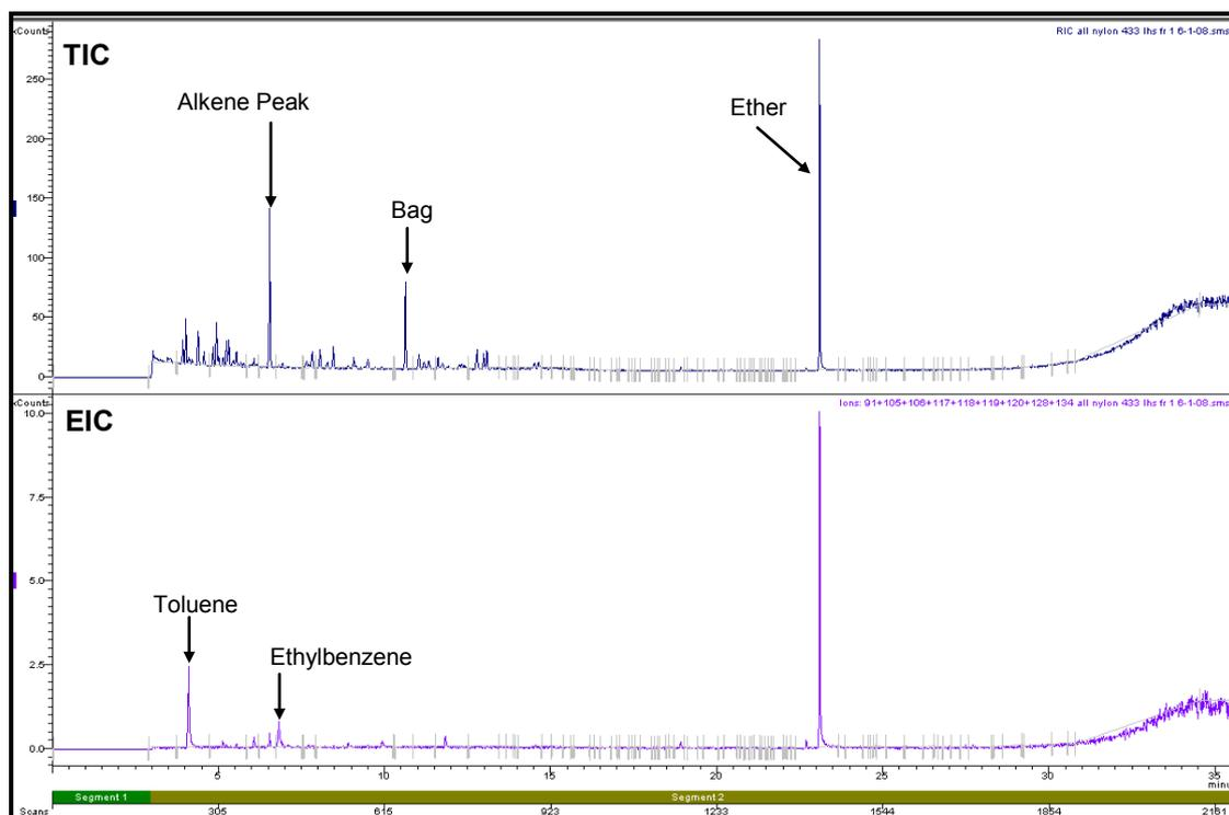
**Figure 4.18: Total Ion Chromatogram and Extracted Ion Chromatogram of the Left Side-Front of the Nylon Carpet after Furnace Burn at 433°C (Refer to Section 2.5.1 for GC/MS conditions)**
