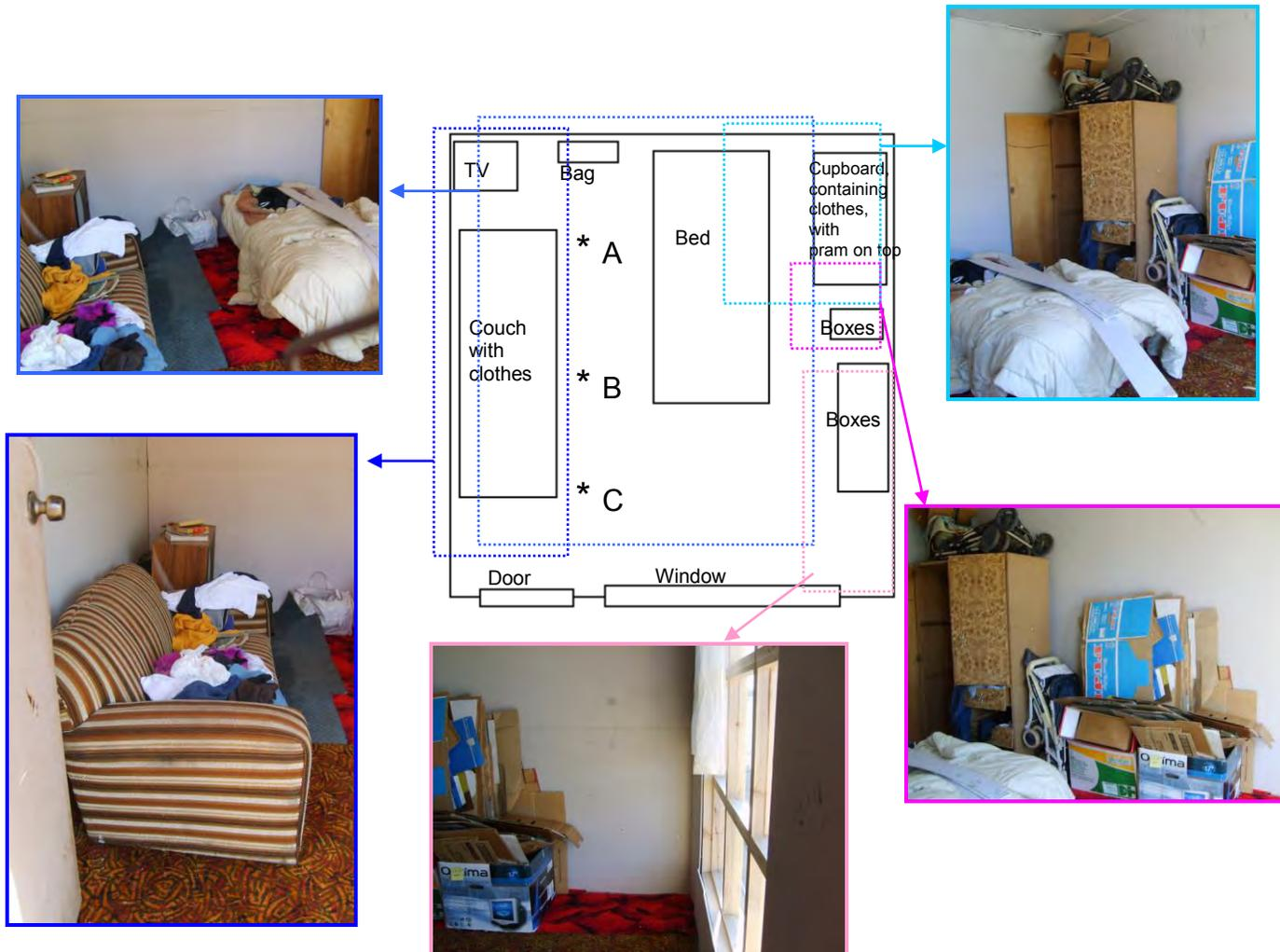
Figure 3.82: Layout of Room 3 with asterisks showing where each group of three Thermocouples were placed
