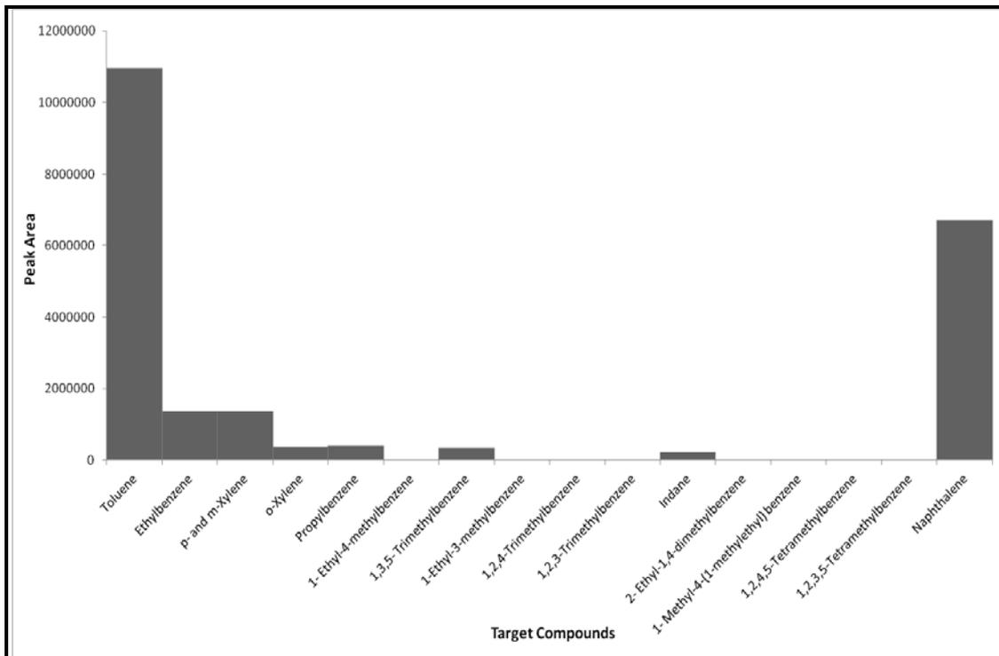
**Figure H1.2: Target Compound Chromatogram of Nylon Fibres Pyrolysed at 900°C**
