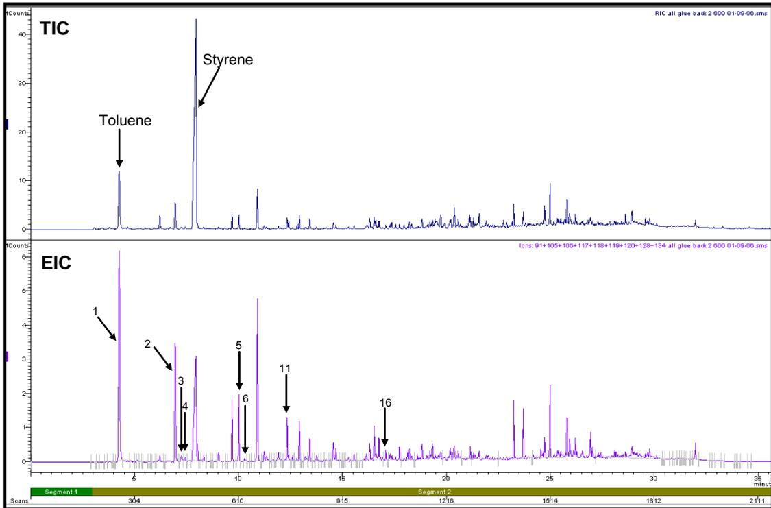
**Figure H4.5: Total Ion Chromatogram and Extracted Ion Chromatogram of Adhesive from Carpet Backing Pyrolysed at 600°C**
