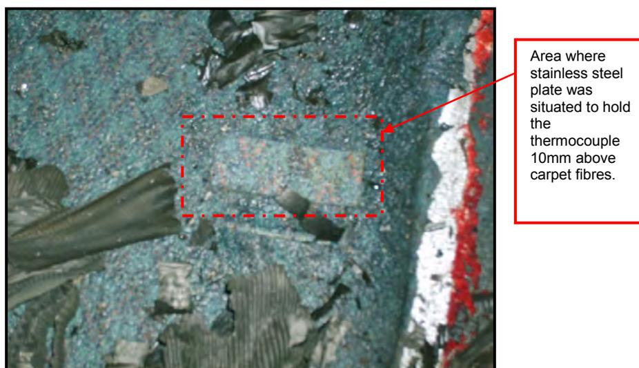
**Figure 3.84: Carpet at centre of Petrol Spill after the Fire (where group A Thermocouples were located)**
