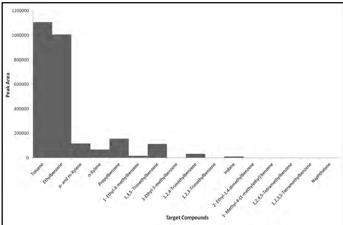
**Figure 4.36: Target Compound Chromatogram of Nylon Swatch placed in the Bottom of a Can burnt with Lid On**
