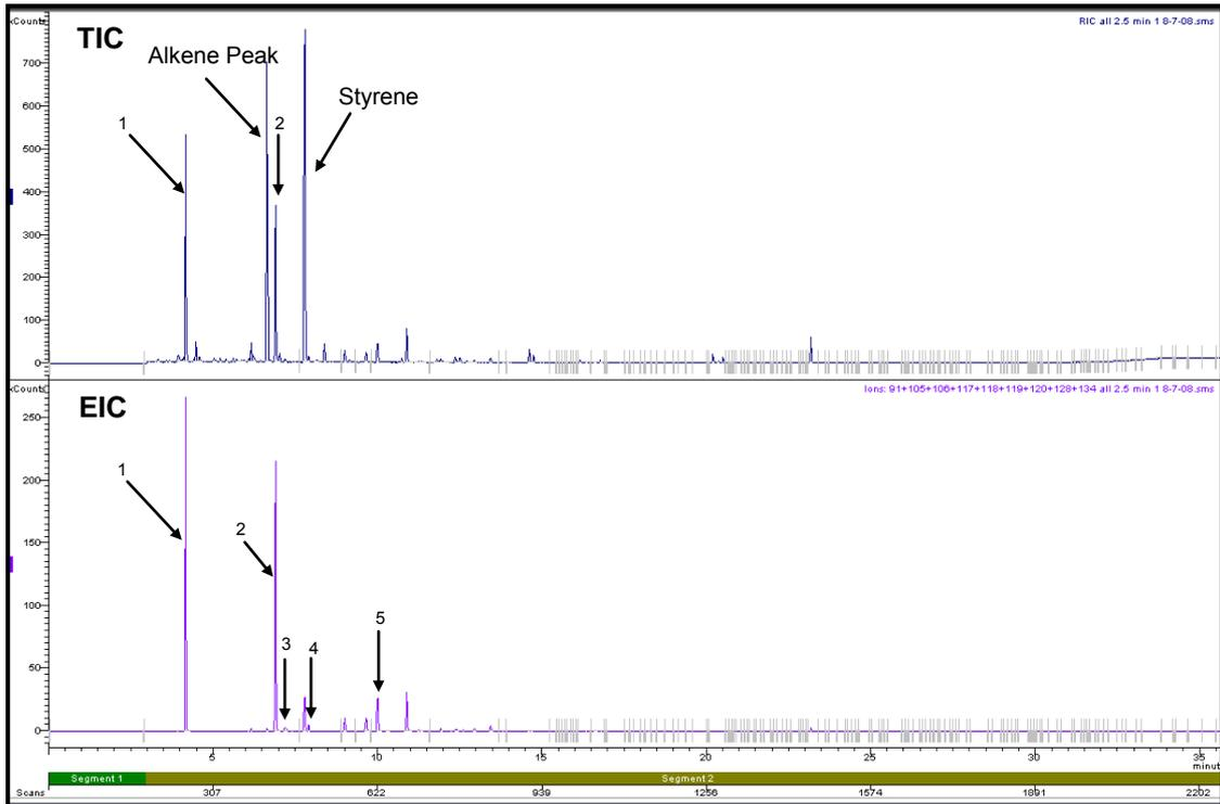
**Figure C1.10: Target Ion Chromatogram and Extracted Ion Chromatogram of a Nylon Carpet Swatch burnt in a Can with Lid On for 2.5 minutes**
