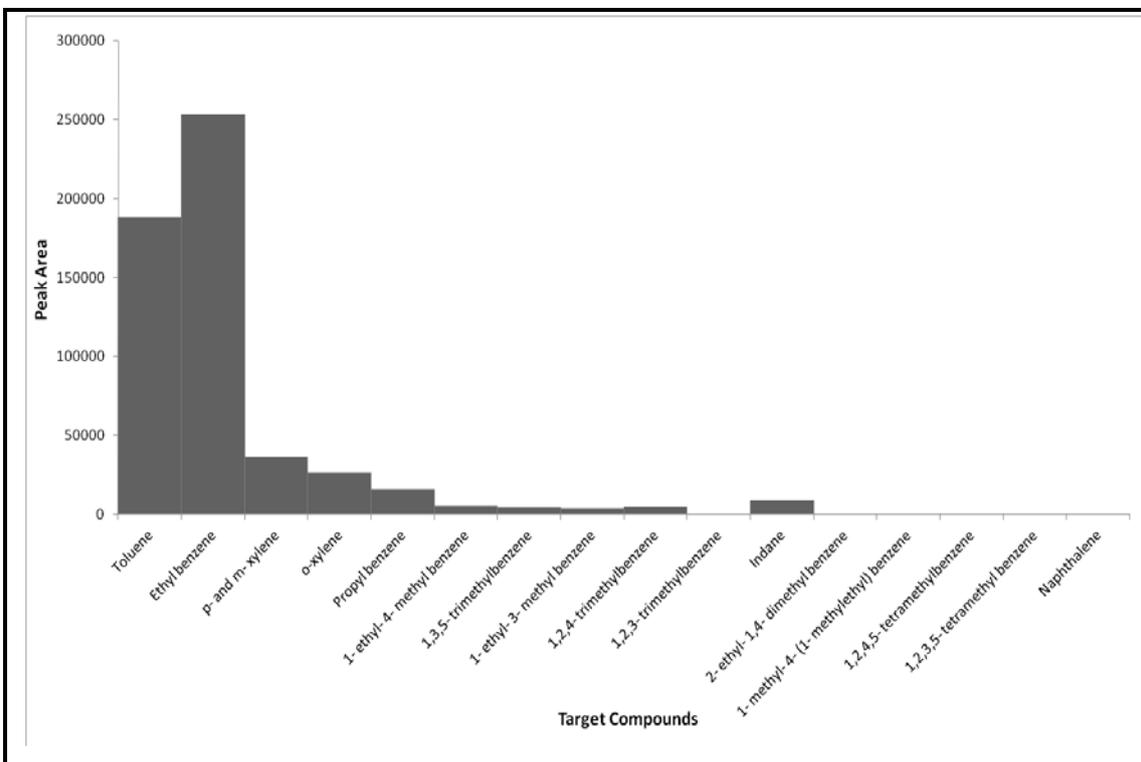
**Figure C1.31: Target Compound Chromatogram of a Nylon Carpet Swatch burnt in a Can with Lid On for 10 minutes**
