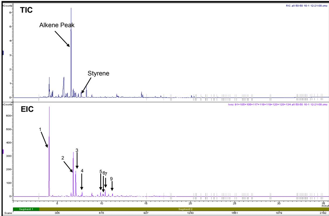
**FigureD3.11: Total Ion Chromatogram and Extracted Ion Chromatogram of a 50-50 Polypropylene-Wool Carpet Swatch burnt in a Can with Lid On for 10 minutes**
