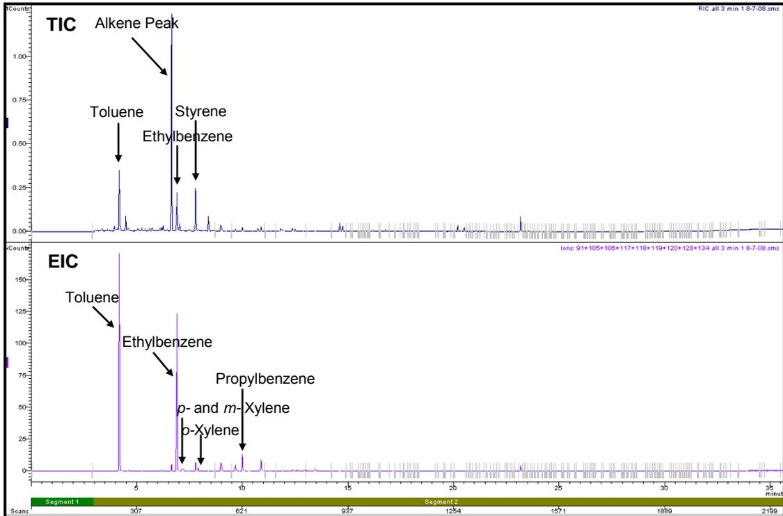
**Figure C1.12: Target Ion Chromatogram and Extracted Ion Chromatogram of a Nylon Carpet Swatch burnt in a Can with Lid On for 3 minutes**
