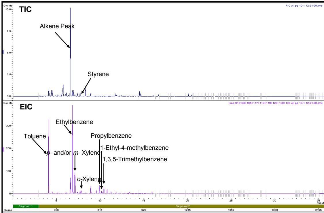
**Figure D1.11: Total Ion Chromatogram and Extracted Ion Chromatogram of a Polypropylene Carpet Switch burnt in a Can with Lid On for 10 minutes**
