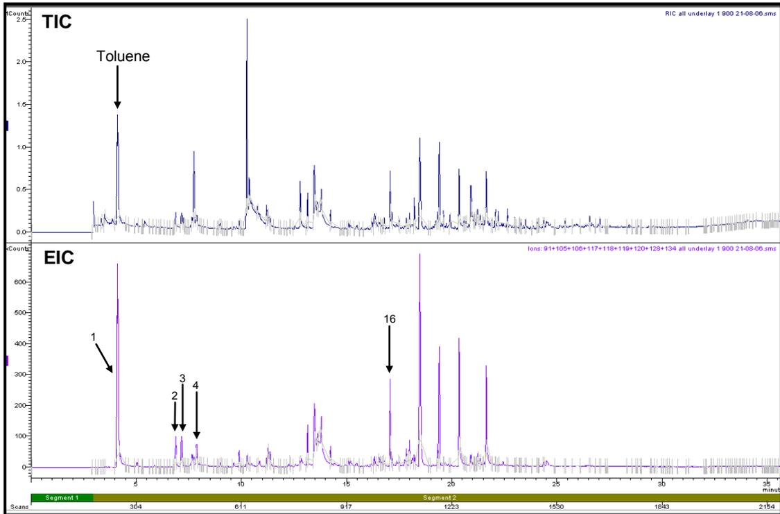
**Figure H9.1: Total Ion Chromatogram and Extryacted Ion Chromatogram of Underlay Pyrolysed at 900°C**
