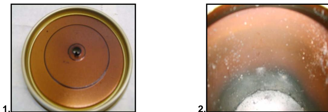
Figure D1.1 (a): 1. Underside of Lid and 2. Side of Can after Burning
