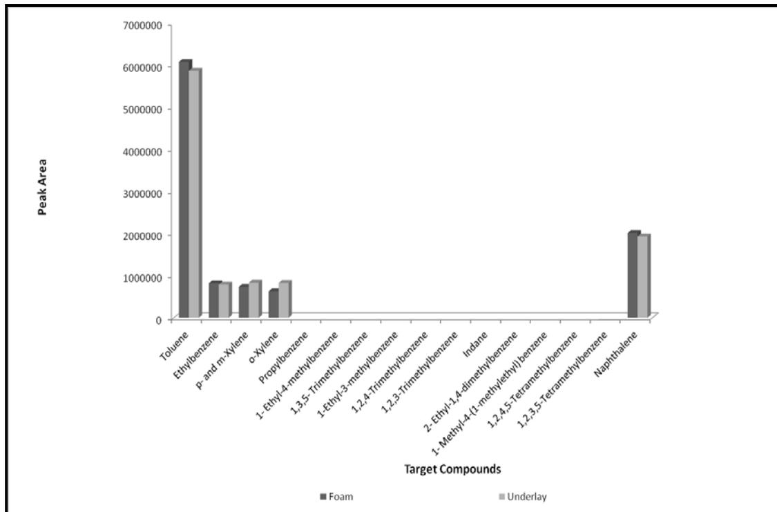
**Figures J1.18: Target Compound Chromatogram for Foam and Underlay pyrolysed at 900°C**
