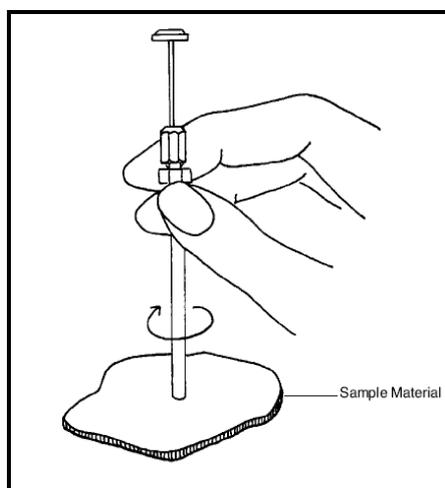
**Figure 2.2: Tubular Cutter Obtaining Sample<sup>148</sup>**
