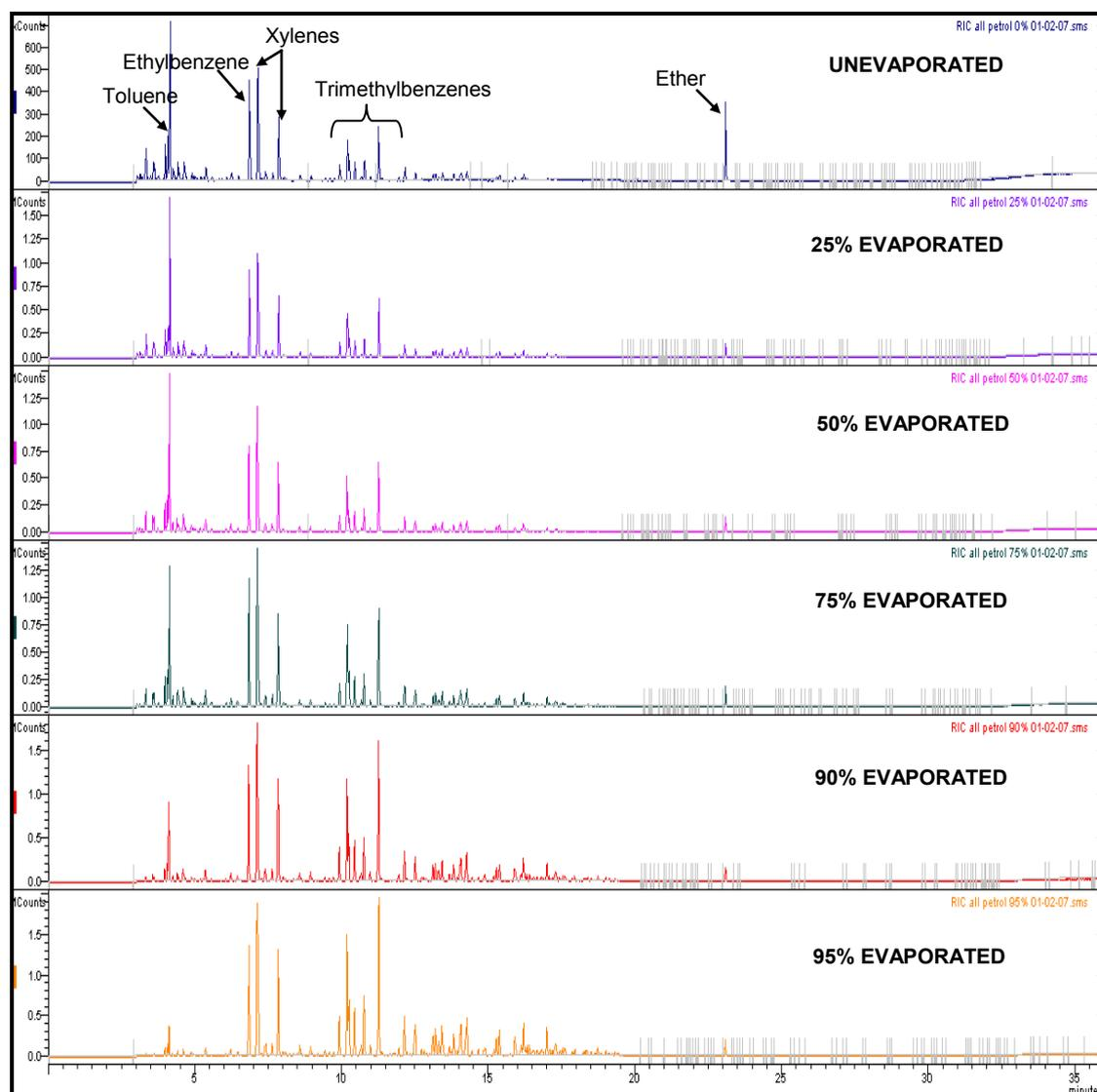
**Figure 3.2: Total Ion Chromatograms of Unevaporated Petrol (blue), 25% Evaporated (purple), 50% Evaporated (pink), 75% Evaporated (green), 90% Evaporated (red) and 95% Evaporated Petrol (orange), respectively (Refer to Section 2.5.1 for GC/MS conditions)**
