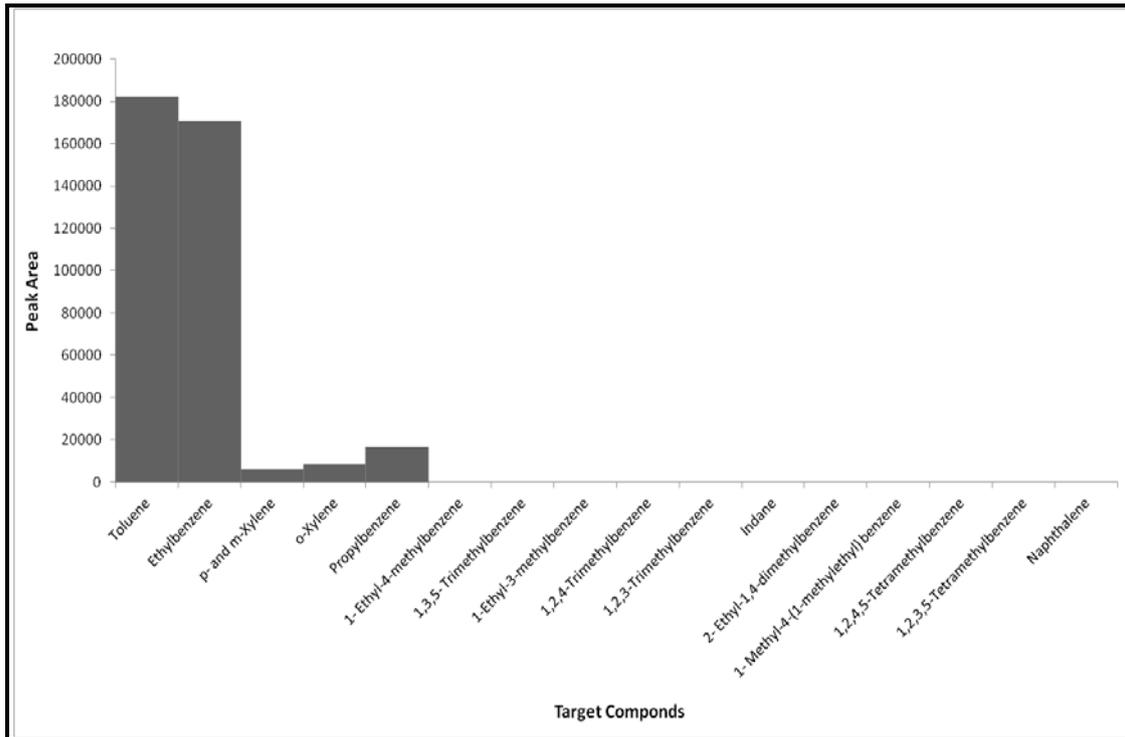
**Figure C1.22: Target Compound Chromatogram of a Nylon Carpet Swatch burnt in a Can with Lid On for 4.5 minutes**
