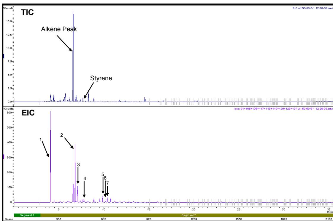
**Figure D3.5: Total Ion Chromatogram and Extracted Ion Chromatogram of a 50-50 Polypropylene-Wool Carpet Swatch burnt in a Can with Lid On for 5 minutes**
