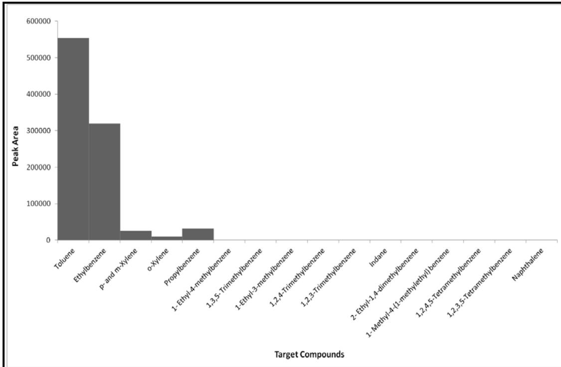
**Figure C1.16: Target Compound Chromatogram of a Nylon Carpet Swatch burnt in a Can with Lid On for 3.5 minutes**
