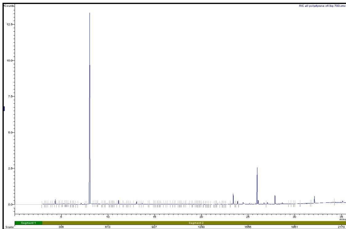
**Figure 3.67: Pyrogram of Thin Piece of Polystyrene Pyrolysed at 700°C with Split Ratio Increased to 100:1 (Refer to Section 2.5.1 for GC/MS conditions)**
