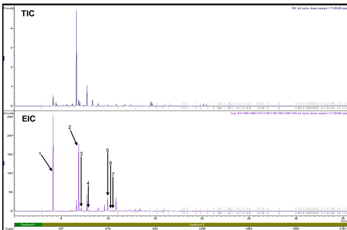
**Figure B1.1: Target Ion Chromatogram and Extracted Ion Chromatogram of Nylon Swatch placed Face Down in the Bottom of a Can burnt with Lid On**
