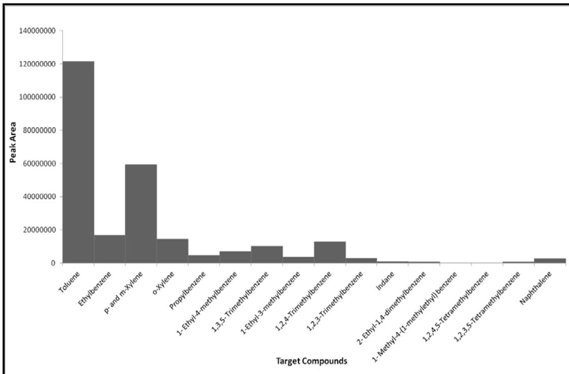
**Figure H5.4: Target Compound Chromatogram of Polypropylene Fibres Pyrolysed at 750°C**
