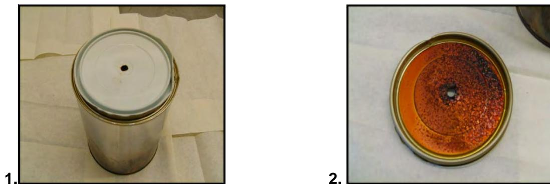
Figure F1.1 (a): 1. Top and 2. Underside of Lid after Burning
