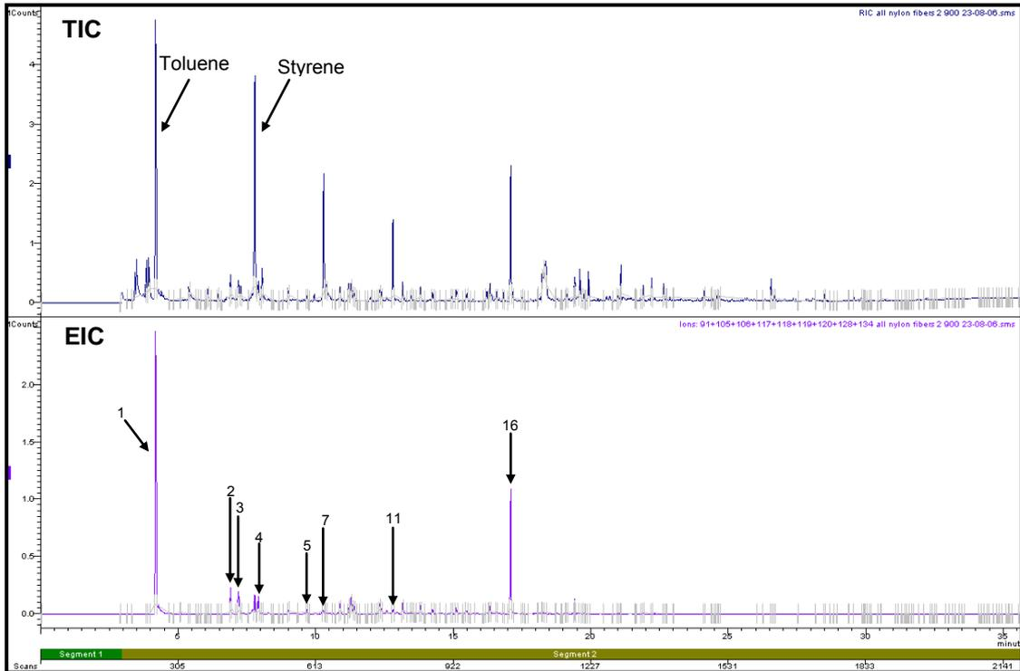
**Figure H1.1: Total Ion Chromatogram and Extracted Ion Chromatogram of Nylon Fibres Pyrolysed at 900°C**
