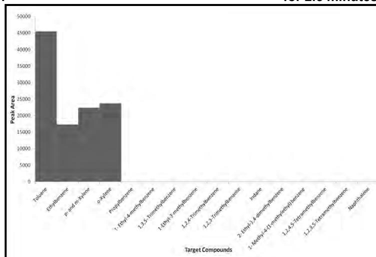
**Target Compound Chromatogram of a foam swatch burnt for 7.5 minutes in a can**
