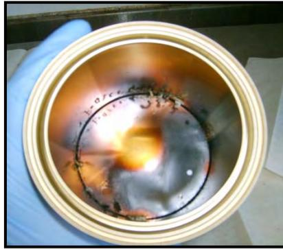
**Figure C1.1 (c): Inside of Can after Burning**
