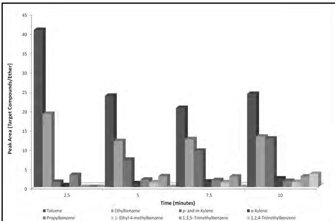
**Figure 4.53: Graph of Peak Area of Target Compounds with Butylated Hydroxytoluene vs. Burn Time for 50-50 Polypropylene-Wool Carpet**
