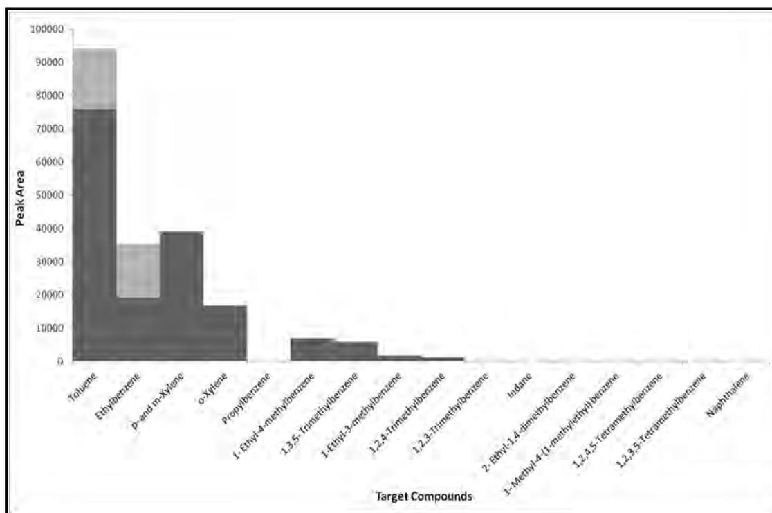
**Figure 5.1: Hypothetical Target Compound Chromatogram of Fire Debris containing Petrol Residue (dark grey) superimposed with Interferences from Carpet and Foam (light grey)**
