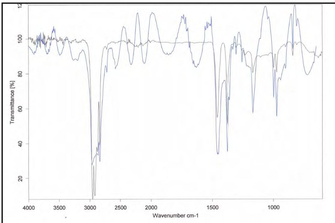
**Figure 3.66: FTIR Spectra of Beige Carpet Fibre (blue) compared with the Polypropylene from Library (black)**
