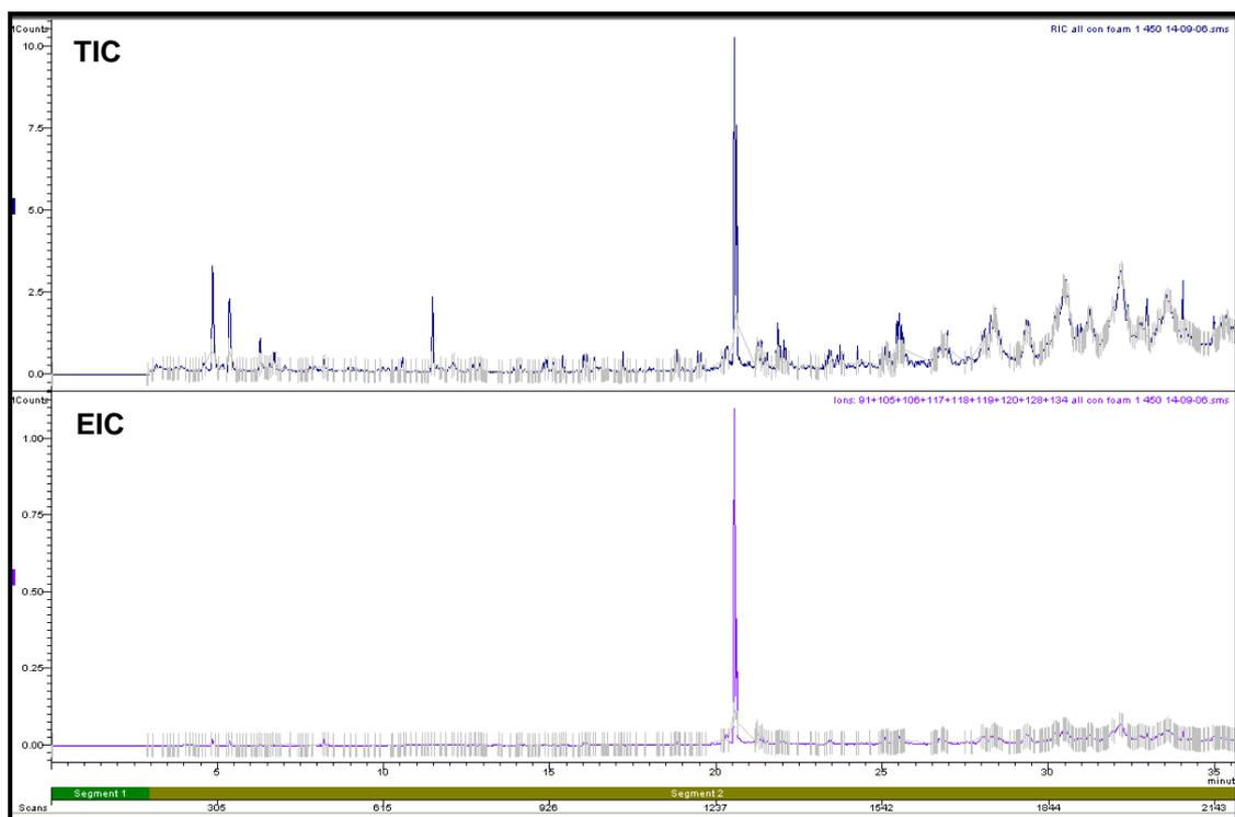
**Figure H8.6: Total Ion Chromatogram and Extracted Ion Chromatogram of Foam Pyrolysed at 450°C**
