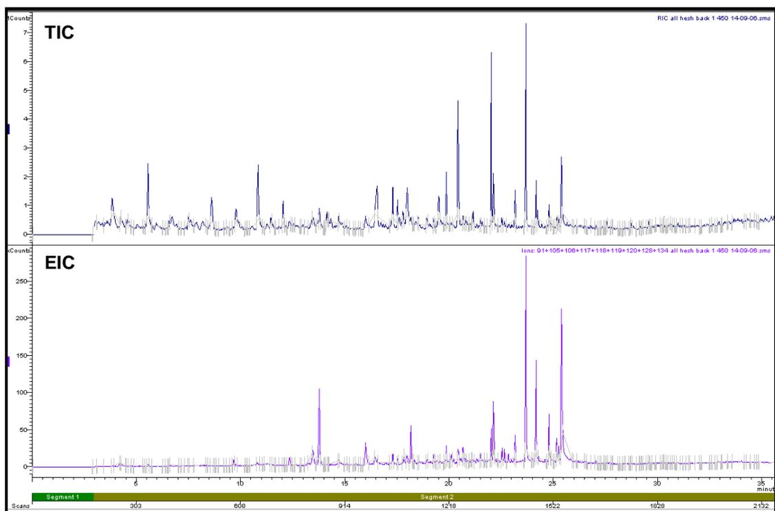
**Figure H2.7: Total Ion Chromatogram and Extracted Ion Chromatogram of Hessian Carpet Backing Pyrolysed at 450°C**
