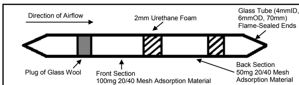
**Figure 2.1: Solvent Desorption Adsorption Charcoal Tube**
