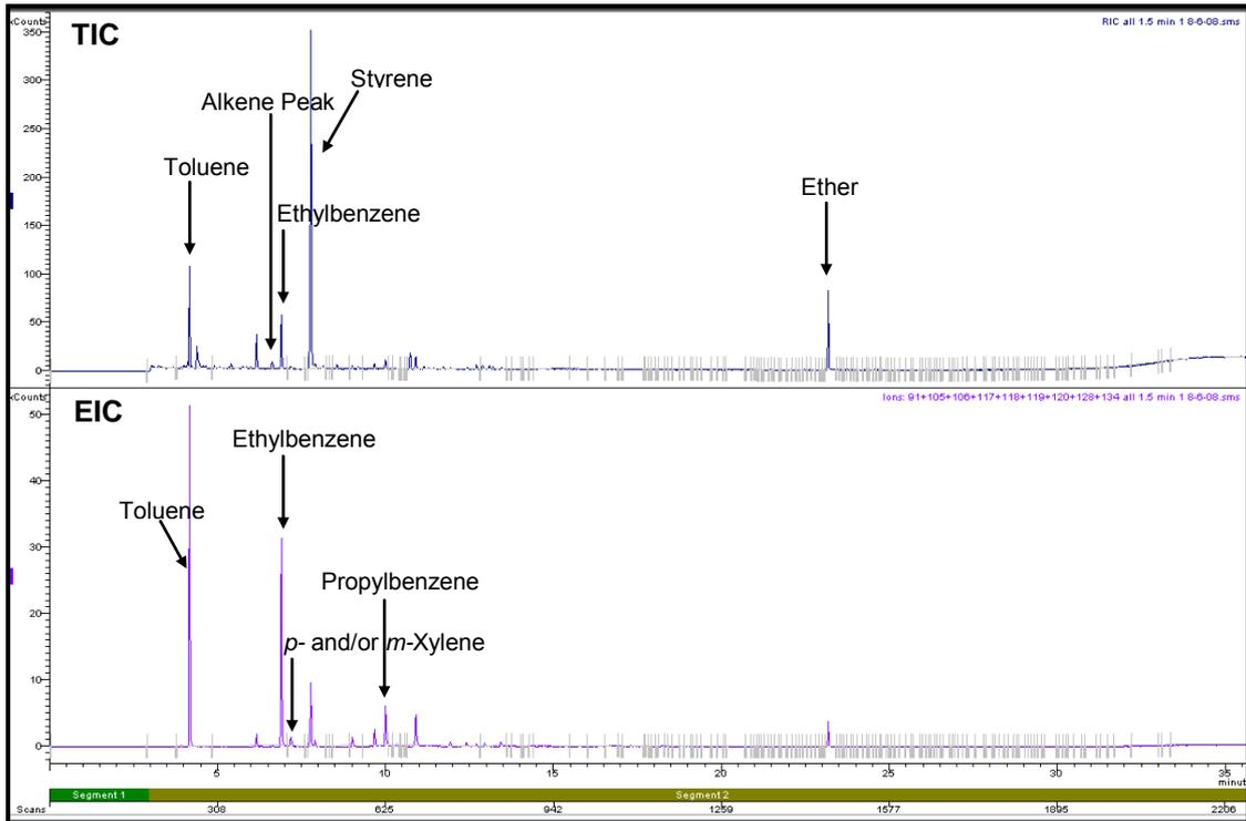
**Figure C1.6: Target Ion Chromatogram and Extracted Ion Chromatogram of a Nylon Carpet Swatch burnt in a Can with Lid On for 1.5 minutes**
