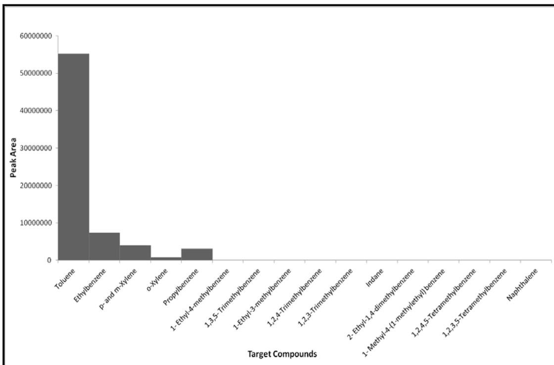
**Figure H6.4: Target Compound Chromatogram of Wool Fibres Pyrolysed at 750°C**
