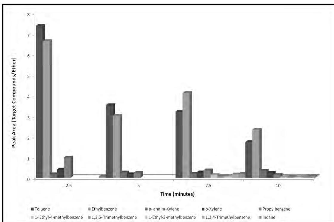
**Figure 4.50: Graph of Peak Area of Target Compounds with Butylated Hydroxytoluene vs. Burn Time for Nylon Carpet**
