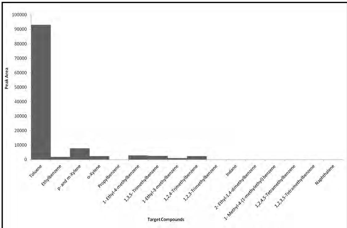
**Figure 3.33: Target Compound Chromatogram for 95% Evaporated Petrol Diluted to 0.001% (v/v)**
