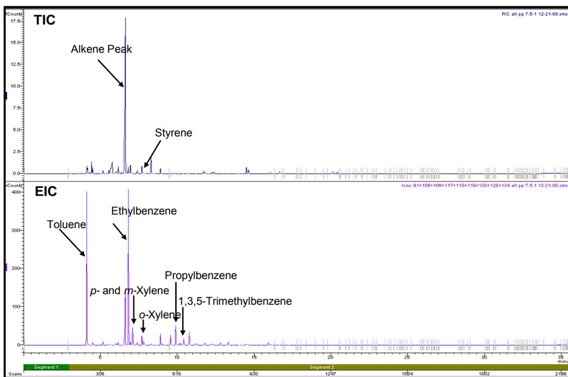
**Figure D1.8: Total Ion Chromatogram and Extracted Ion Chromatogram of a Polypropylene Carpet Swatch burnt in a Can with Lid On for 7.5 minutes**
