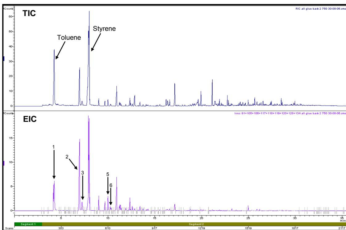
**Figure H4.3: Total Ion Chromatogram and Extracted Ion Chromatogram Adhesive from Carpet Backing Pyrolysed at 750°C**
