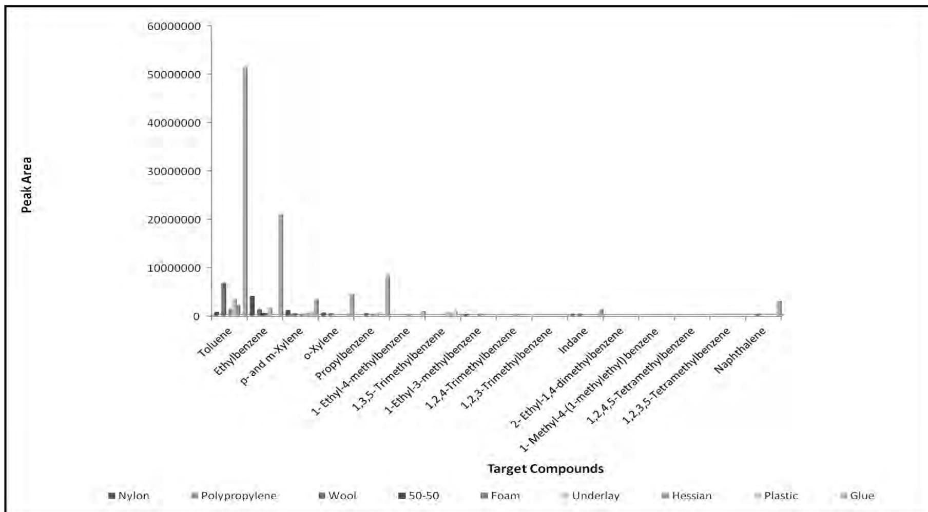
**Figure 4.65: Target Compound Chromatograms incorporating Carpet Fibres and Carpet Backing Components Pyrolysed at 600°C**
