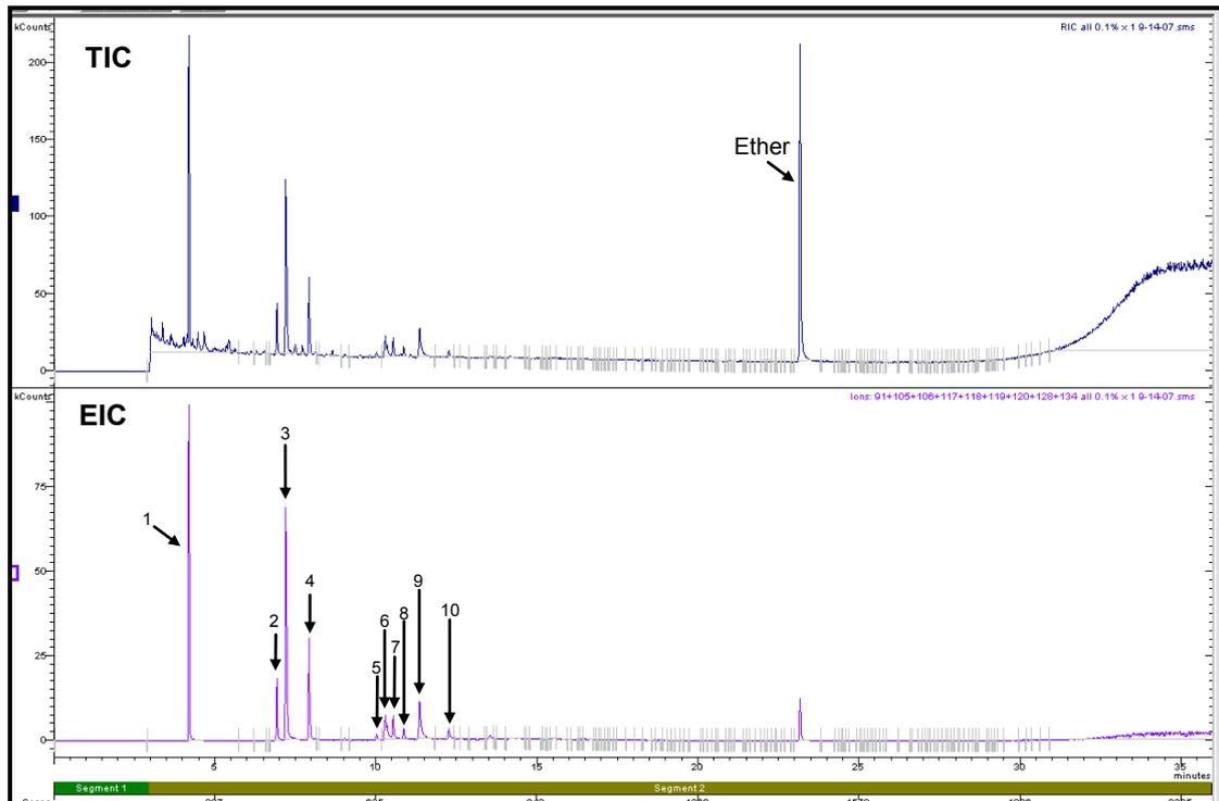
**Figure 3.16: Total Ion Chromatogram and Extracted Ion Chromatogram for Unevaporated Petrol Diluted to 0.1% (v/v) (Refer to Section 2.5.1 for GC/MS conditions)**
