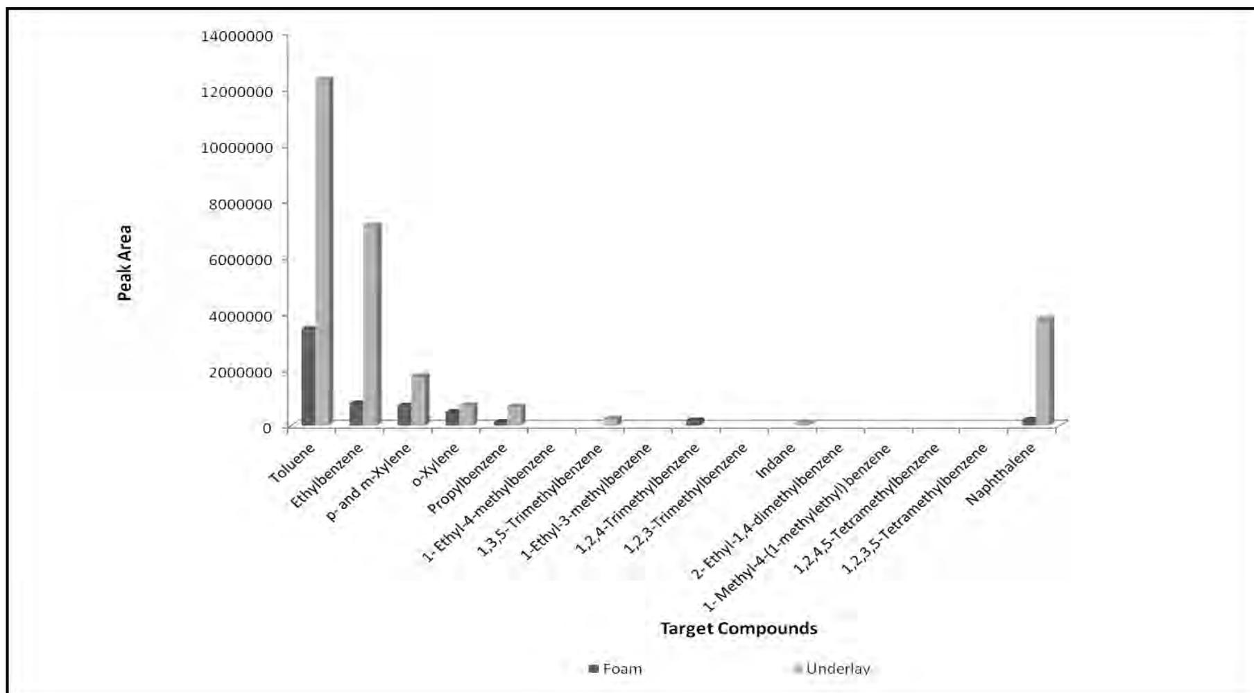
Figure 4.60: Target Compound Chromatograms incorporating Foam and Underlay Pyrolysed at 750°C
