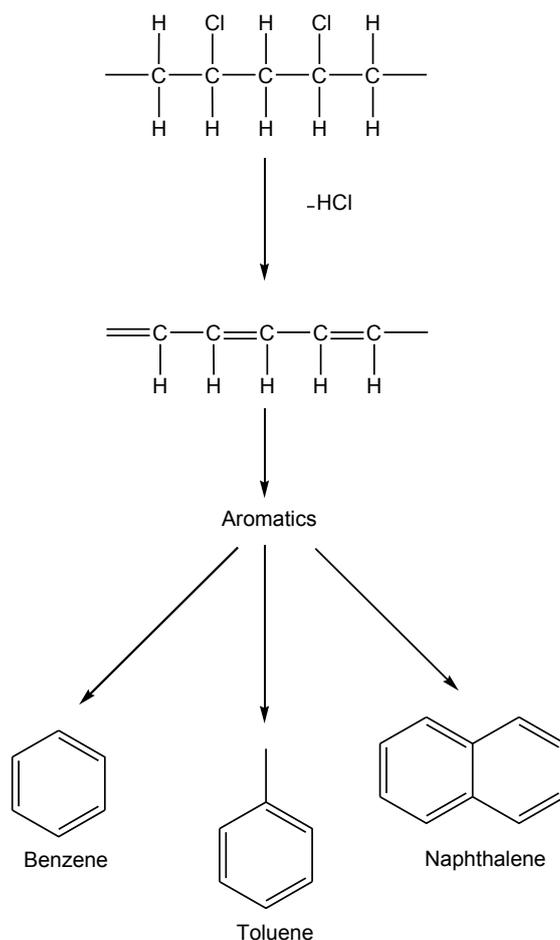
**Figure 1.11: Side Group Scission of Polyvinylchloride**
