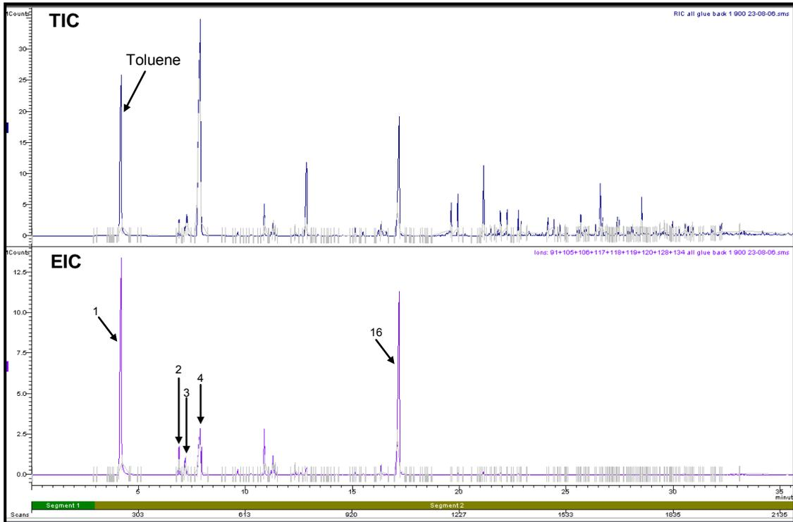
**Figure H4.1: Total Ion Chromatogram and Extracted Ion Chromatogram of Adhesive from Carpet Backing Pyrolysed at 900°C**
