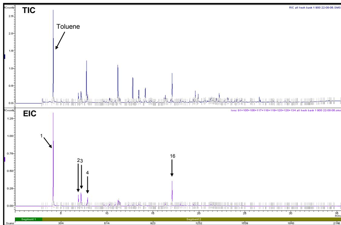
**Figure H2.1: Total Ion Chromatogram and Extracted Ion Chromatograms of Hessian Carpet Backing Pyrolysed at 900°C**
