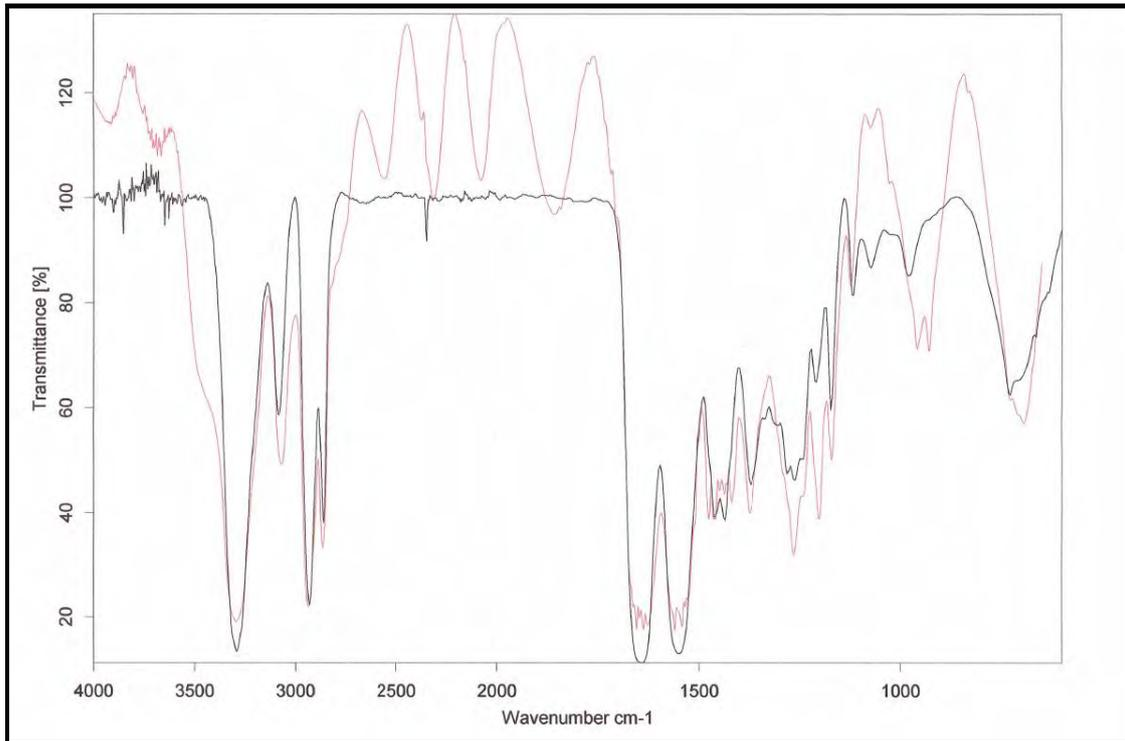
**Figure 3.56: FTIR Spectra of the Carpet Sample (red) compared with Library Spectra of Nylon (black)**
