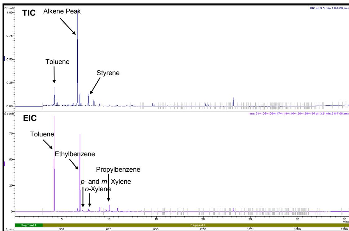
**Figure C1.15: Target Ion Chromatogram and Extracted Ion Chromatogram of a Nylon Carpet Swatch burnt in a Can with Lid On for 3.5 minutes**
