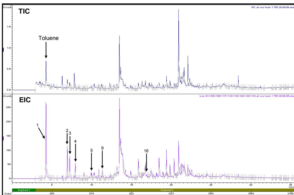
**Figure H8.3: Total Ion Chromatogram and Extracted Ion Chromatogram of Foam Pyrolysed at 750°C**
