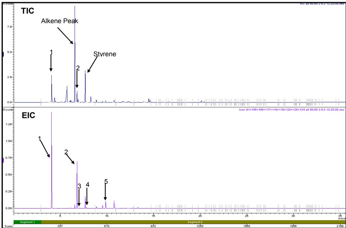
**Figure 4.48: Total Ion Chromatogram and Extracted Ion Chromatogram of a 50-50 Polypropylene-Wool Carpet Swatch burnt in a Can with Lid On for 2.5 minutes (Refer to Section 2.5.1 for GC/MS conditions)**
