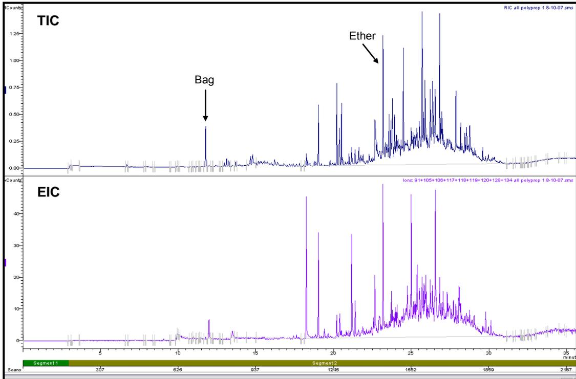
**Figure A1.2(b): Target Ion Chromatogram and Extracted Ion Chromatogram of Polypropylene Carpet burnt in Room 1**
