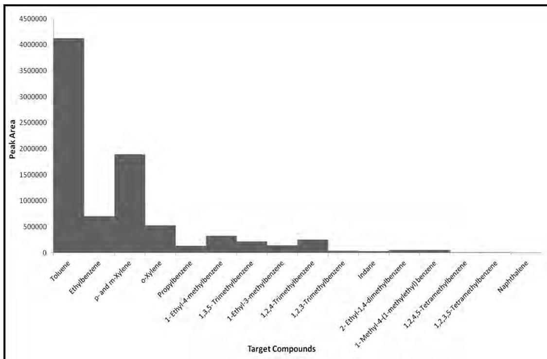
**Figure 3.37: Target Compound Chromatogram of KimWipe spiked with 100 $\mu$ L of Unevaporated Petrol**
