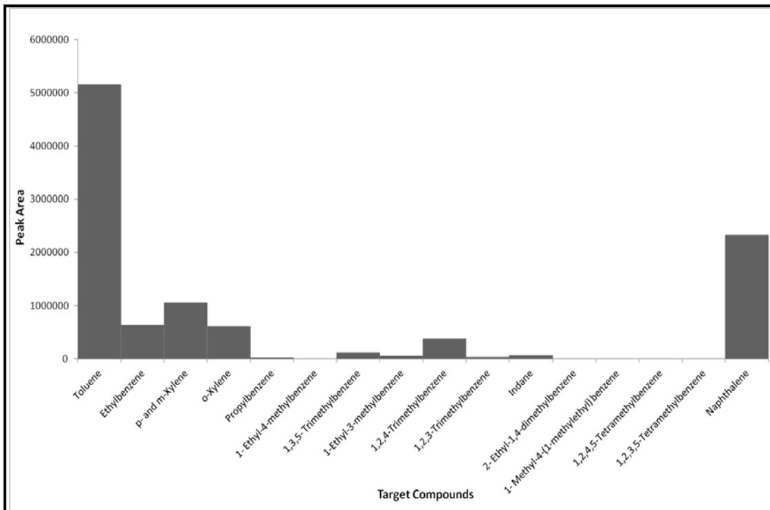
**Figure H2.2: Target Compound Chromatogram of Hessian Carpet Backing Pyrolysed at 900°C**
