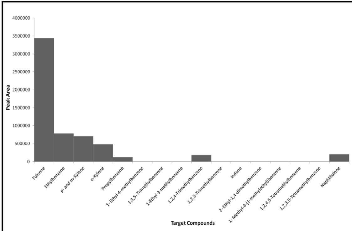
**Figure H8.4: Target Compound Chromatogram of Foam Pyrolysed at 750°C**
