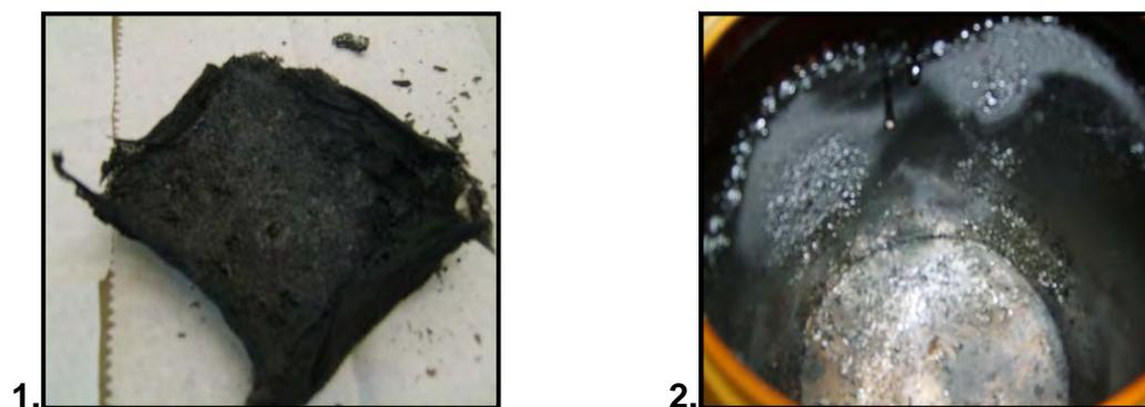
**Figure F1.6 (b): 1. Sample after Burning 2. Inside of Can after Burning**
