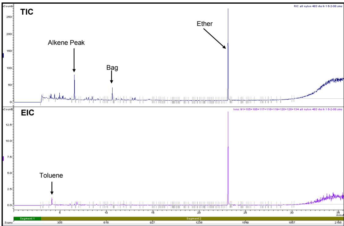
**Figure 4.17(b): Total Ion Chromatogram and Extracted Ion Chromatogram of the Right Side-Front of the Nylon Carpet after Furnace Burn at 483°C (Refer to Section 2.5.1 for GC/MS conditions)**
