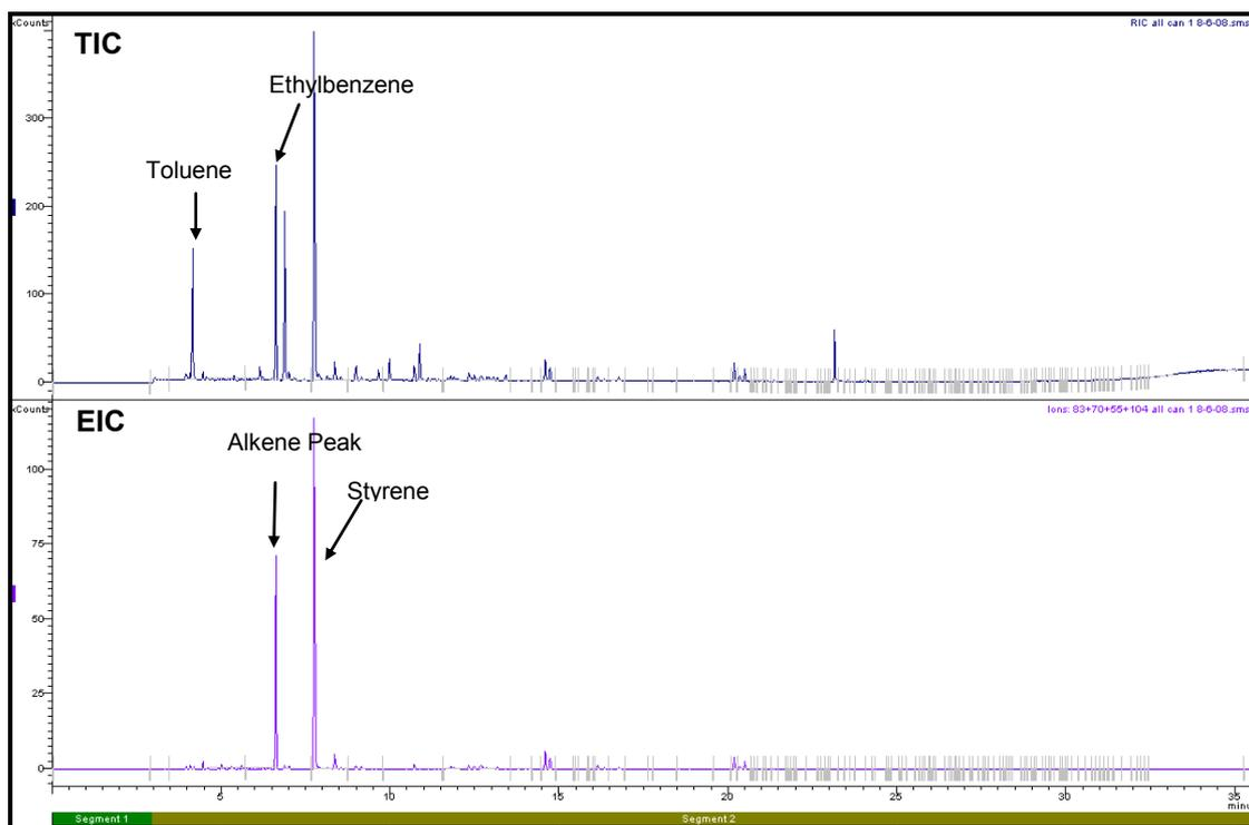
**Figure 4.67: Total Ion Chromatogram and Extracted Ion Chromatogram showing Alkene Peak and Styrene (Refer to Section 2.5.1 for GC/MS conditions)**
