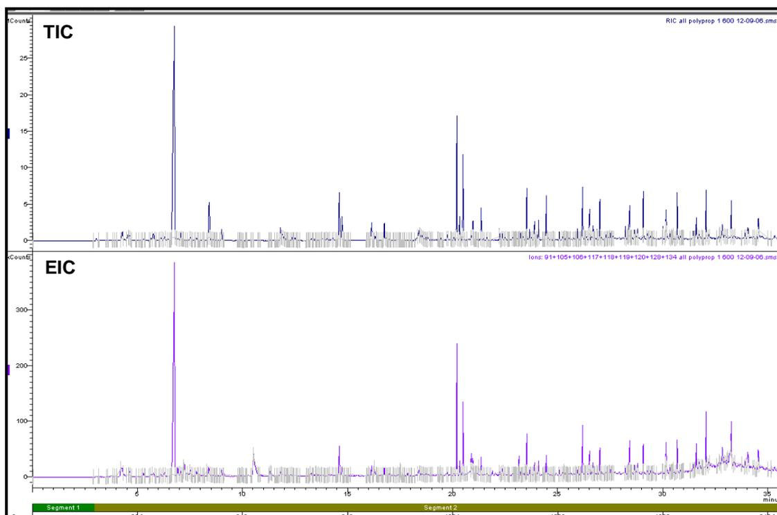
**Figure H5.5: Total Ion Chromatogram and Extracted Ion Chromatogram of Polypropylene Fibres Pyrolysed at 600°C**
