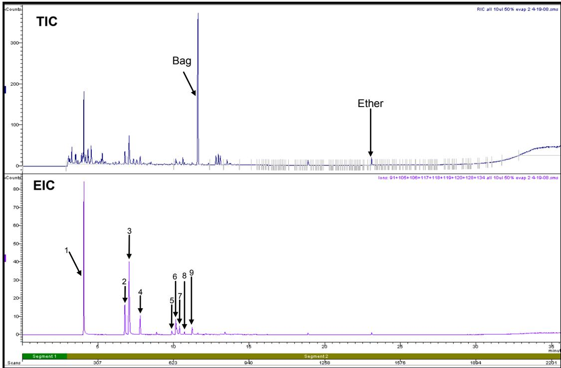
**Figure 3.44: Total Ion Chromatogram and Extracted Ion Chromatogram of KimWipe spiked with 10 $\mu$ L of 50% Evaporated Petrol (Refer to Section 2.5.1 for GC/MS conditions)**
