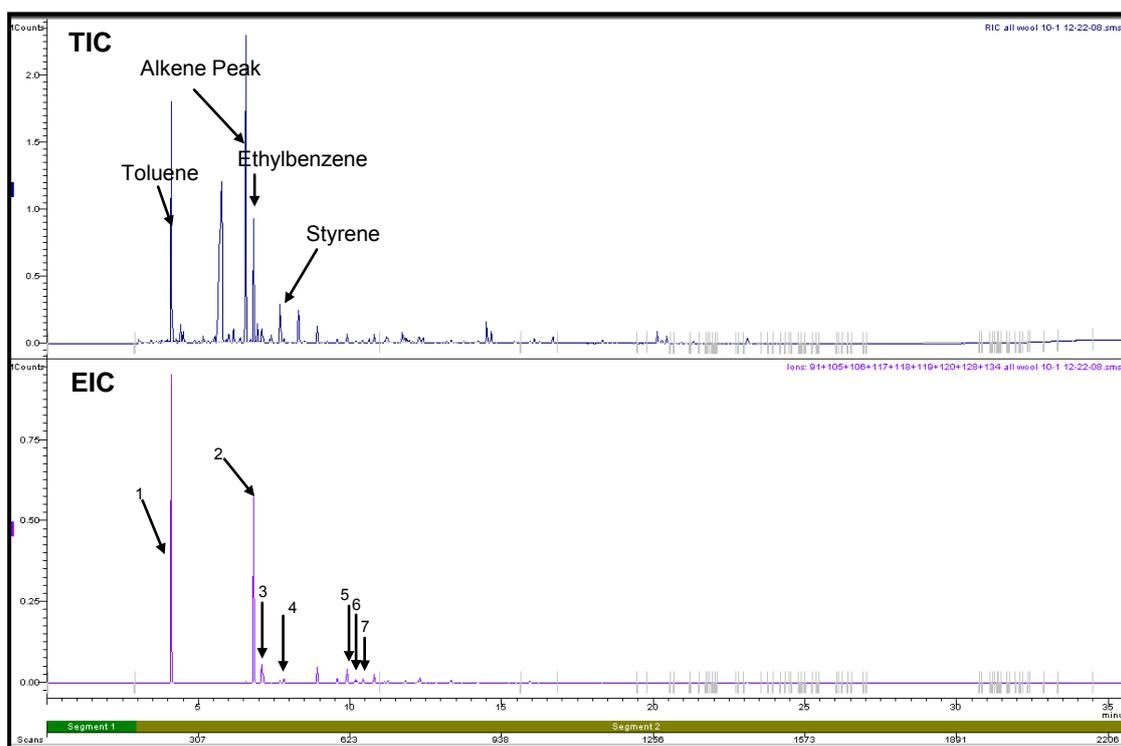
**Figure D2.11: Total Ion Chromatogram and Extracted Ion Chromatogram of a Wool Carpet Swatch burnt in a Can with Lid On for 10 minutes**
