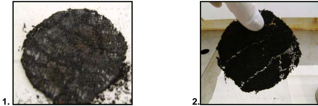
**Figure D3.10 (b): 1. Top and 2. Underside of Sample after Burning**
