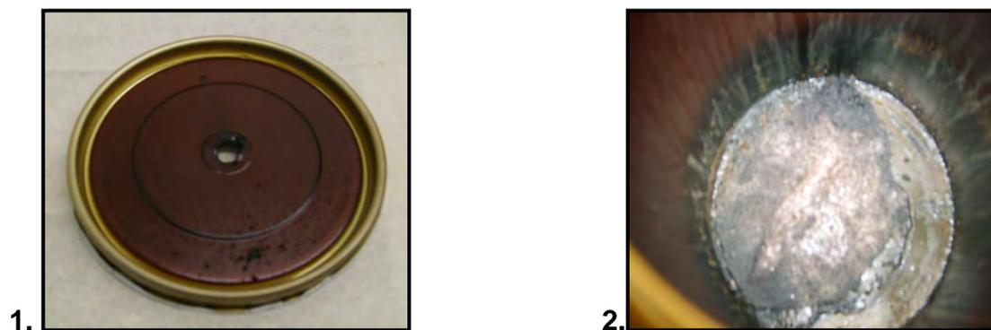
**Figure D1.4 (a): 1. Underside of Lid and 2. Sample in Bottom of Can after Burning**
