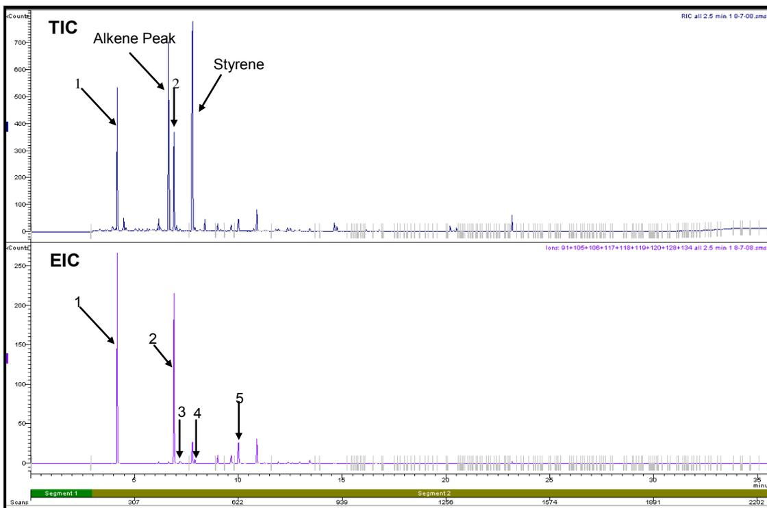
**Figure 4.42: Total Ion Chromatogram and Extracted Ion Chromatogram of a Nylon Carpet Swatch burnt in a Can with Lid On for 2.5 minutes (Refer to Section 2.5.1 for GC/MS conditions)**
