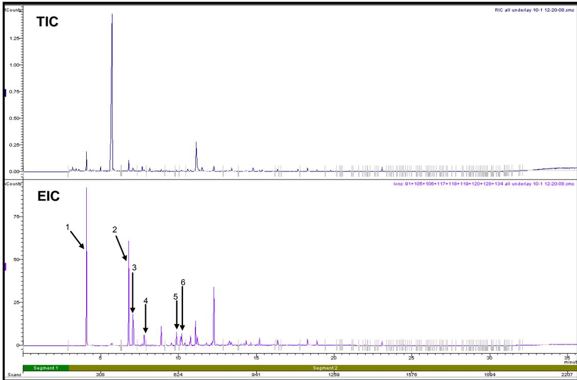
**Figure F2.13: Total Ion Chromatogram and Extracted Ion Chromatogram of Underlay Burnt in a Can with Lid On for 10 minutes**
