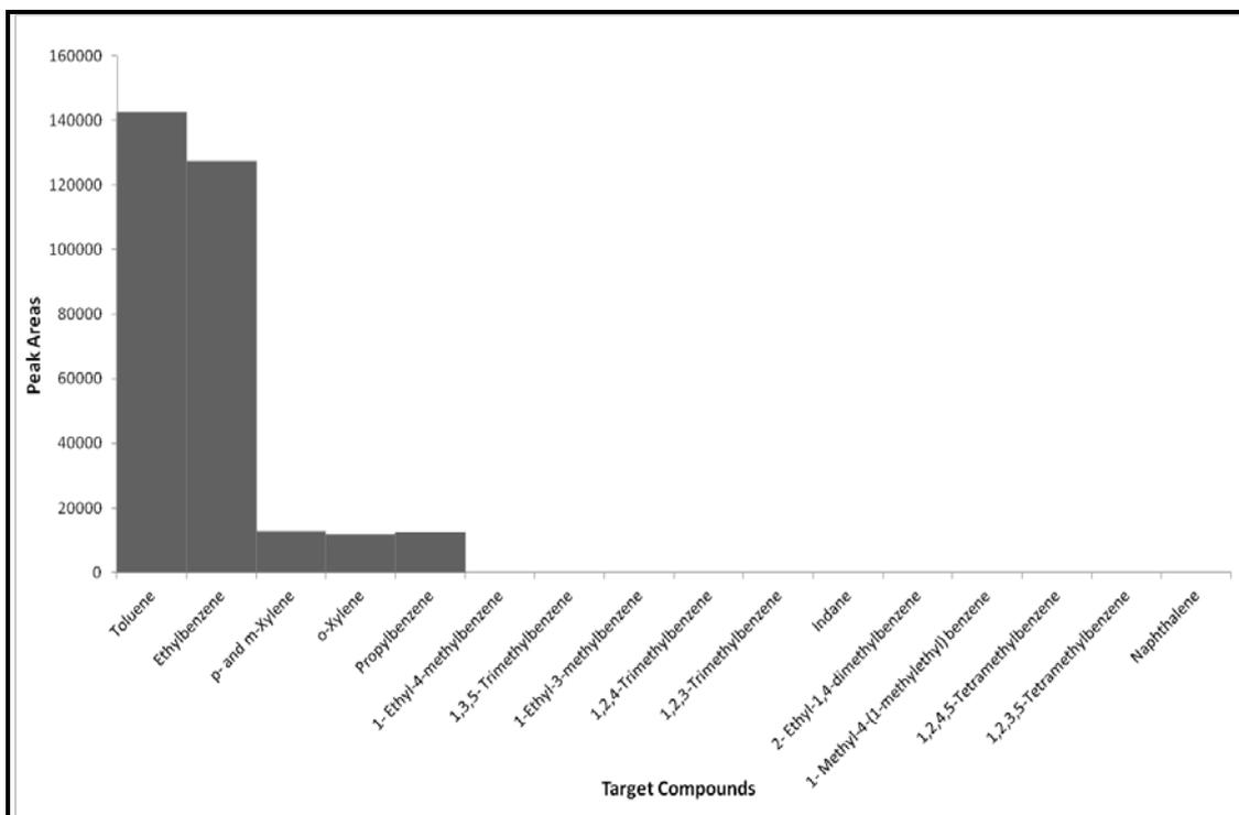
**Figure C1.19: Target Compound Chromatogram of a Nylon Carpet Swatch burnt in a Can with Lid On for 4 minutes**
