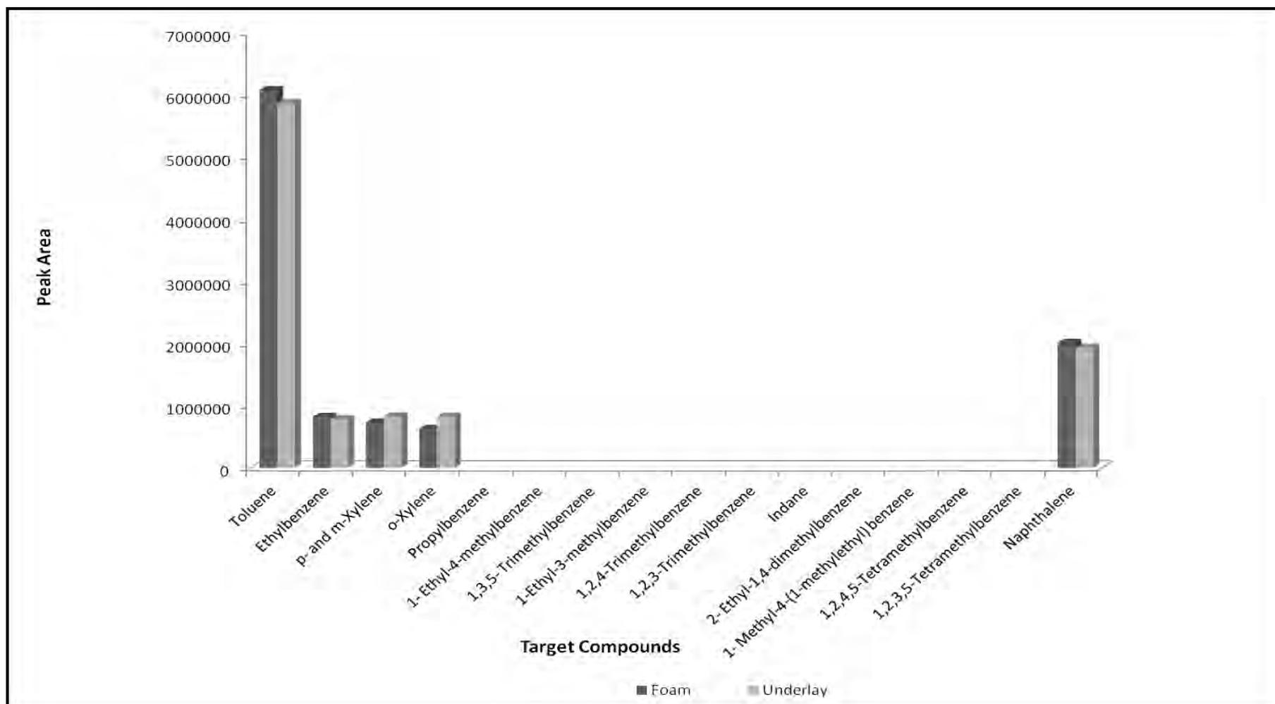
Figure 4.64: Target Compound Chromatograms incorporating Foam and Underlay Pyrolysed at 900°C
