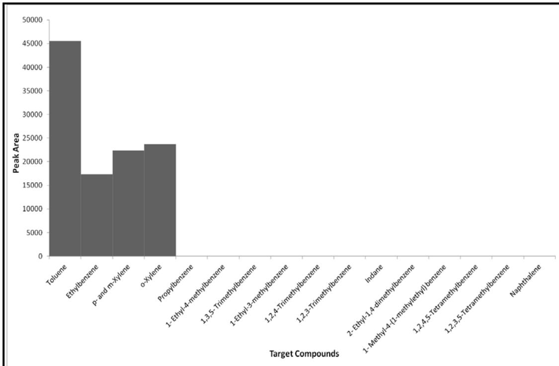
**Figure F1.8: Target Compound Chromatogram of Foam Burnt in a Can with Lid On for 7.5 minutes**
