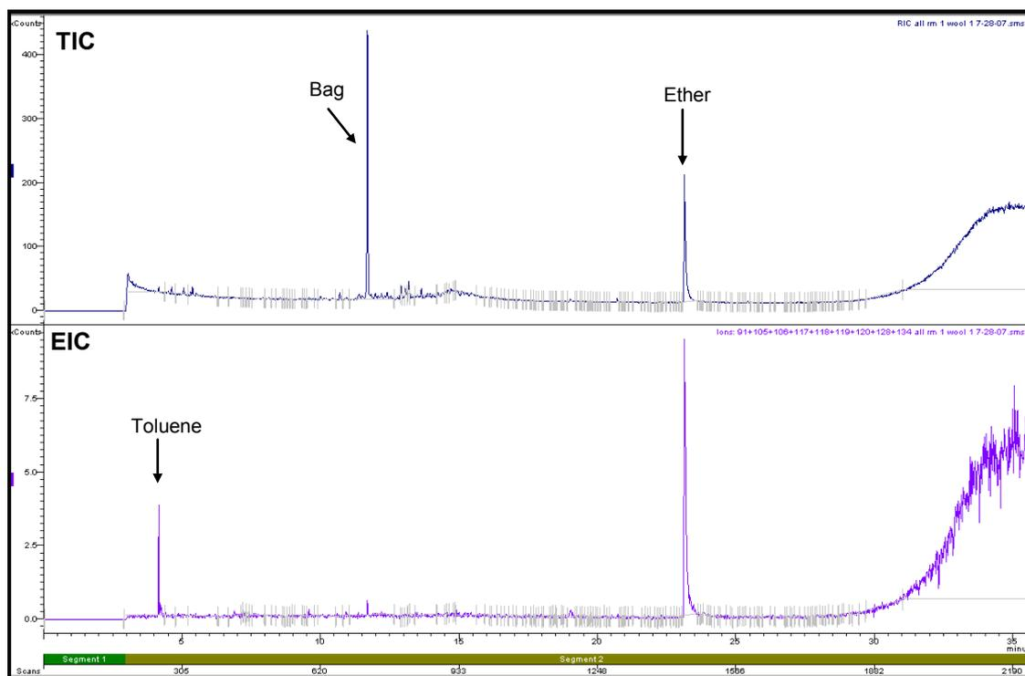
**Figure 4.10: Total Ion Chromatogram and Extracted Ion Chromatogram of Wool Carpet burnt in Room 1 (Refer to Section 2.5.1 for GC/MS conditions)**
