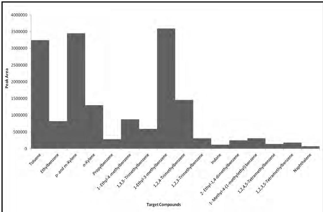
**Figure 3.13: Target Compound Chromatogram for 50% Evaporated Petrol Diluted to 1% (v/v)**
