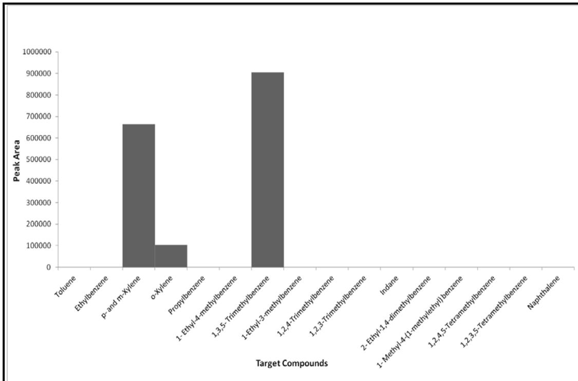
**Figure H3.6: Target Compound Chromatogram of Plastic Carpet Backing Pyrolysed at 600°C**
