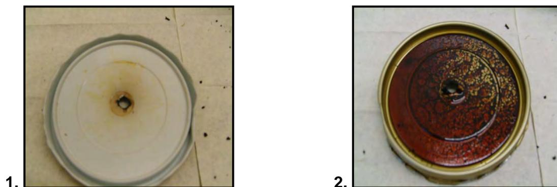
**Figure D3.4 (a): 1. Top and 2. Underside of Lid after Burning**
