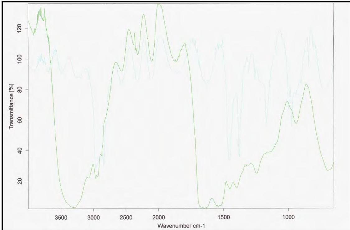
**Figure 3.64: FTIR Spectra of Black Carpet Fibre (green) compared with Beige Carpet Fibre (blue)**
