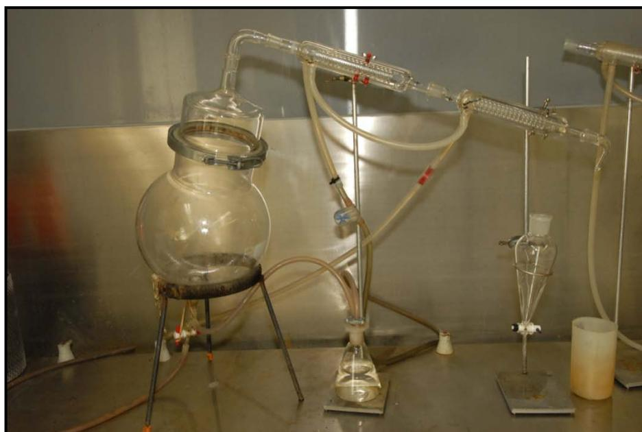
**Figure A1.1(a): Steam Distillation set up at VPFSC Laboratories**
