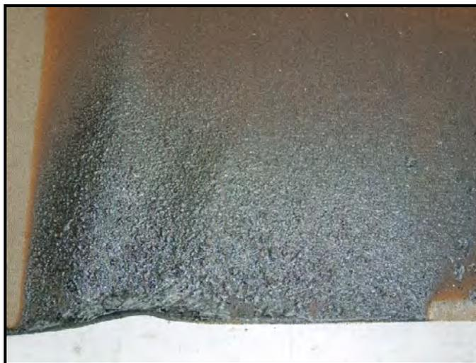
**Figure 4.26: Wool Carpet after the Furnace Burn at 330°C**
