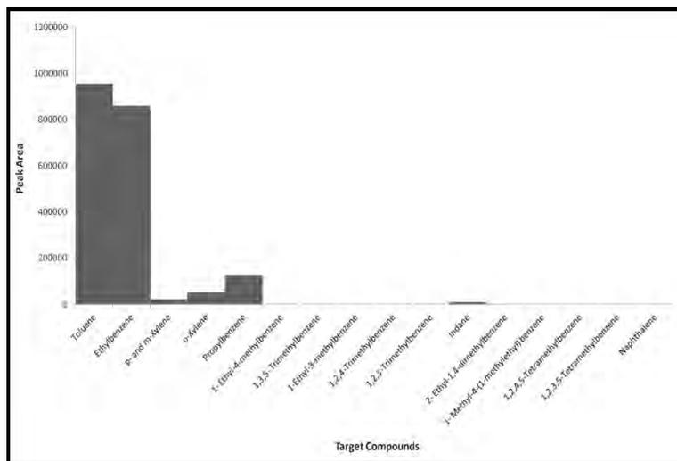
**Target Compound chromatogram of a nylon carpet swatch burnt for 2.5 minutes in a can**
