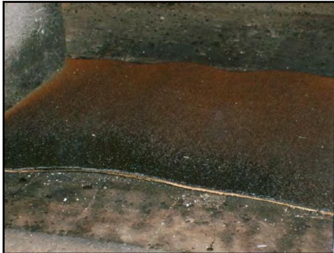
**Figure 4.25: Wool Carpet after the Furnace Burn at 280°C**
