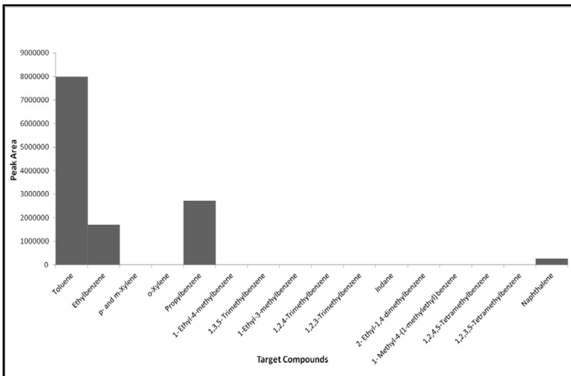
**Figure H4.8: Target Compound Chromatogram of Adhesive from Carpet Backing Pyrolysed at 450°C**
