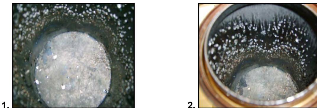
**Figure F2.12 (b): 1. Bottom and 2. Sides of Can after Burning**
