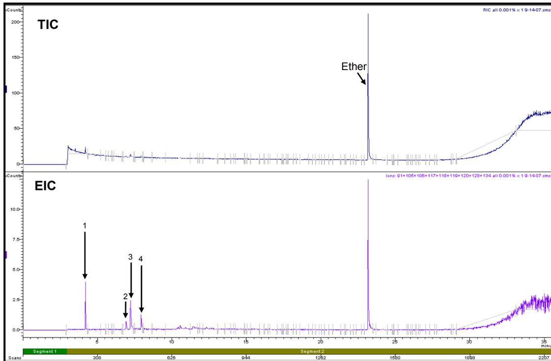
**Figure 3.28: Total Ion Chromatogram and Extracted Ion Chromatogram for Unevaporated Petrol Diluted to 0.001% (v/v) (Refer to Section 2.5.1 for GC/MS conditions)**
