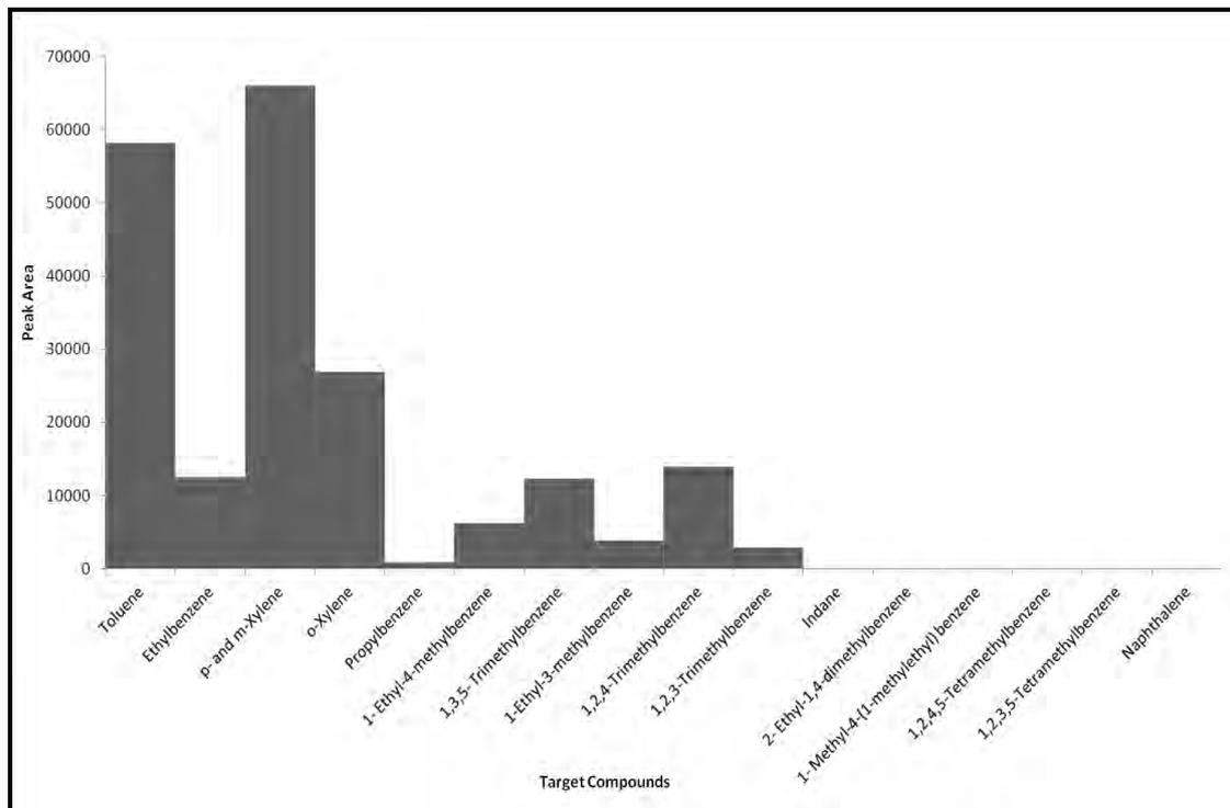
**Figure 3.23: Target Compound Chromatogram for Unevaporated Petrol Diluted to 0.01% (v/v)**
