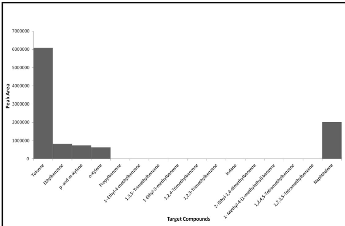
**Figure H8.2: Target Compound Chromatogram of Foam Pyrolysed at 900°C**
