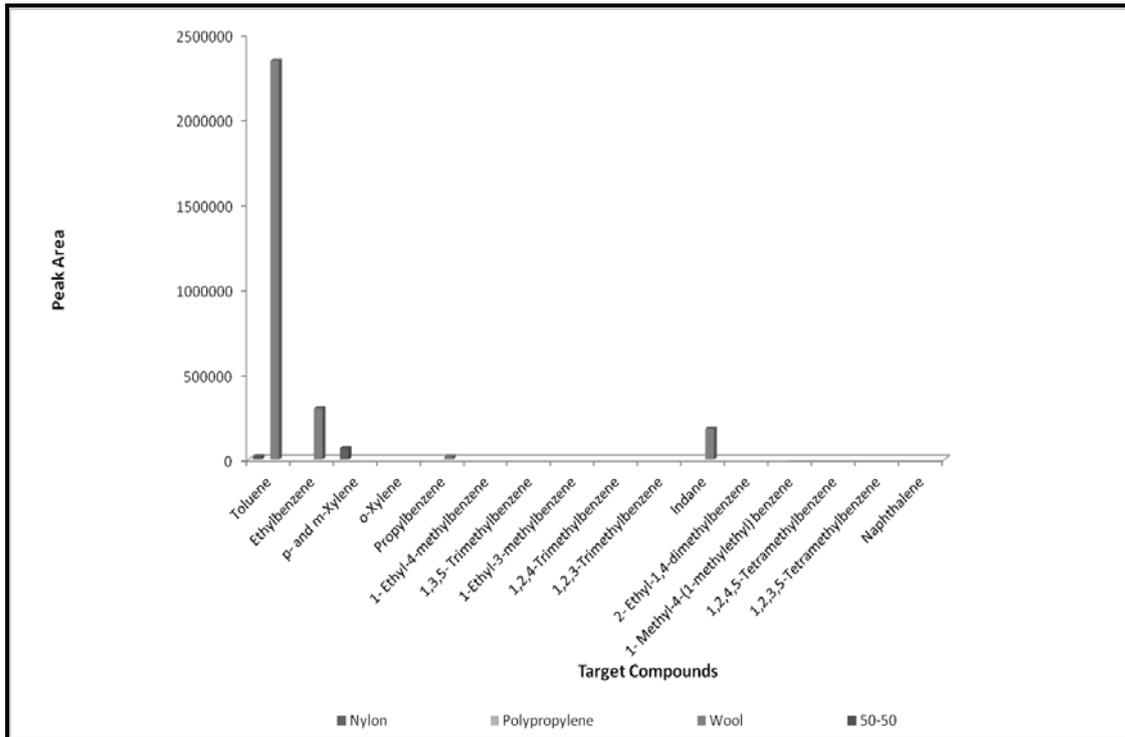
**Figures J1.13: Target Compound Chromatogram for all Carpet Fibres pyrolysed at 450°C**
