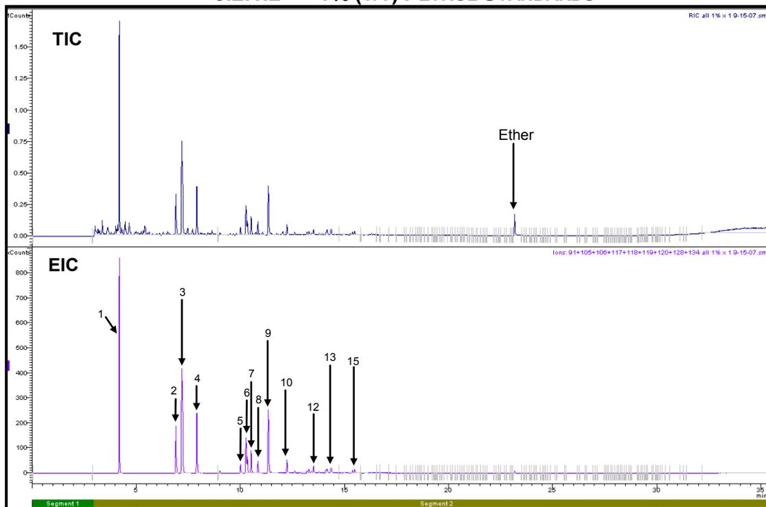
**Figure 3.10: Total Ion Chromatogram and Extracted Ion Chromatogram for Unevaporated Petrol Diluted to 1% (v/v) (Refer to Section 2.5.1 for GC/MS conditions)**
