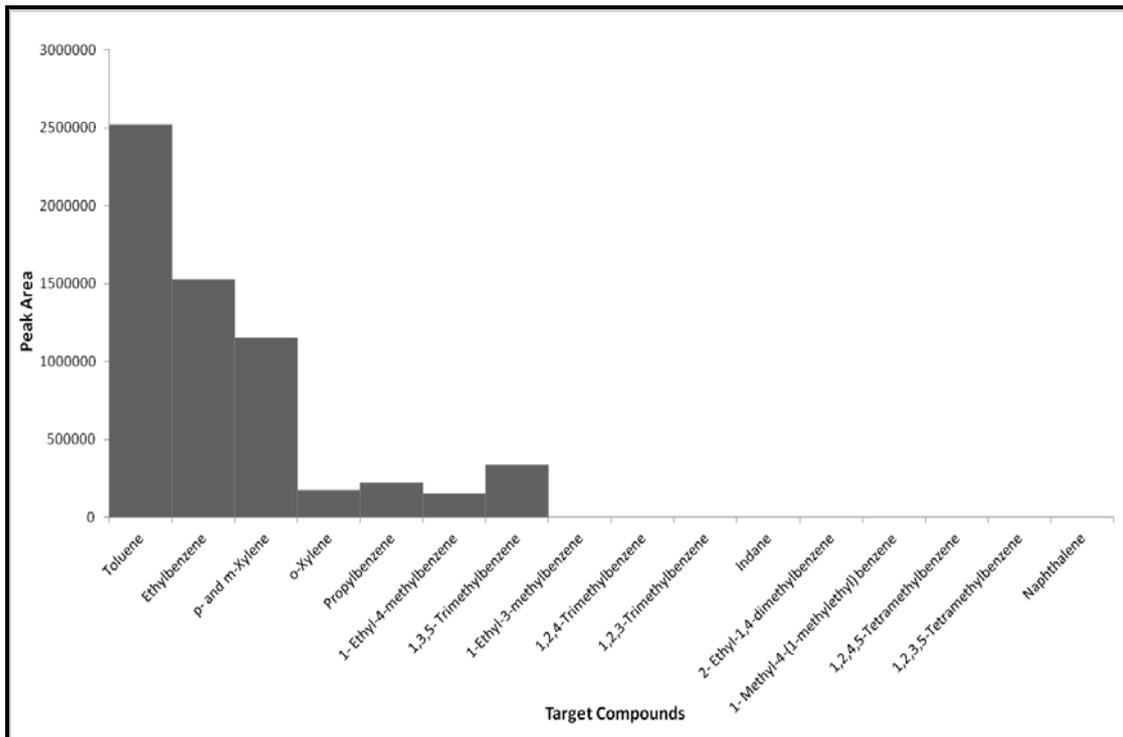
**Figure D3.9: Target Compound Chromatogram of a 50-50 Polypropylene-Wool Carpet Swatch burnt in a Can with Lid On for 7.5 minutes**
