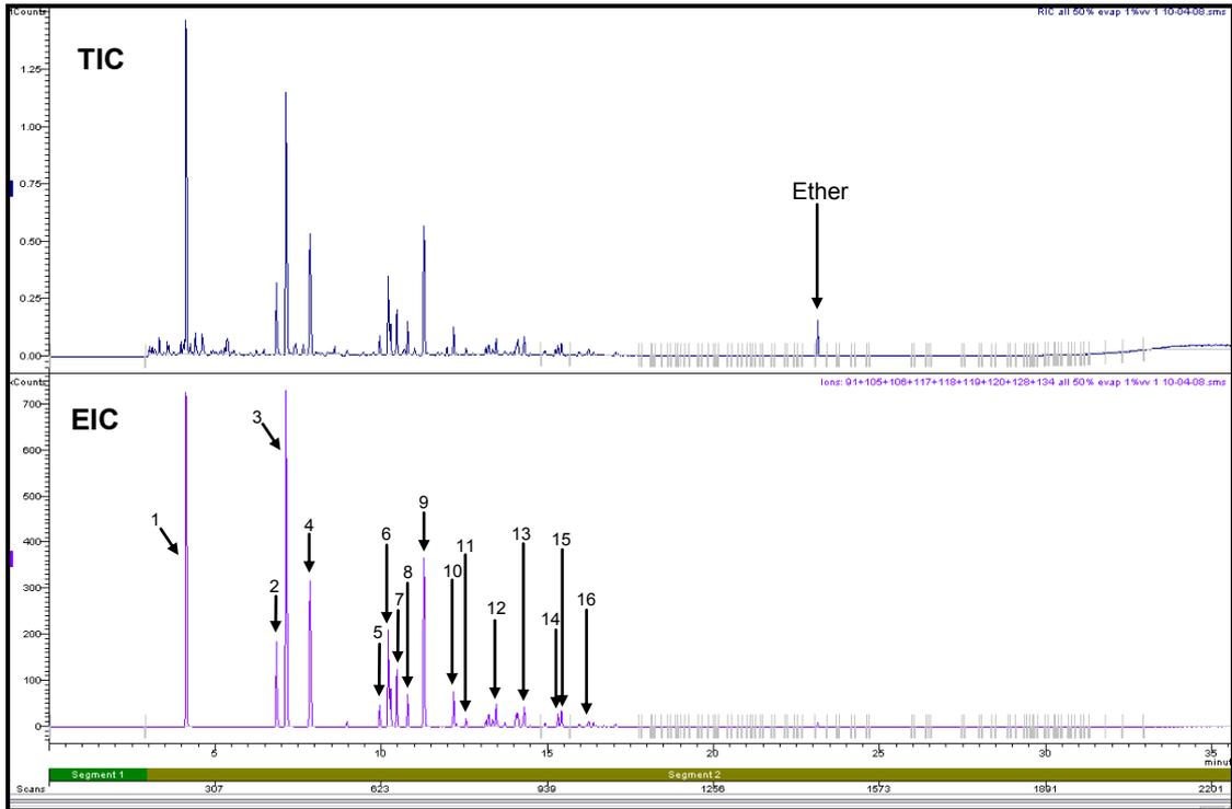
**Figure 3.12: Total Ion Chromatogram and Extracted Ion Chromatogram for 50% Evaporated Petrol Diluted to 1% (v/v) (Refer to Section 2.5.1 for GC/MS conditions)**
