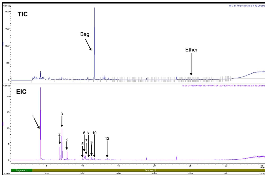
**Figure 3.42: Total Ion Chromatogram and Extracted Ion Chromatogram of KimWipe spiked with 10 $\mu$ L of Unevaporated Petrol (Refer to Section 2.5.1 for GC/MS conditions)**
