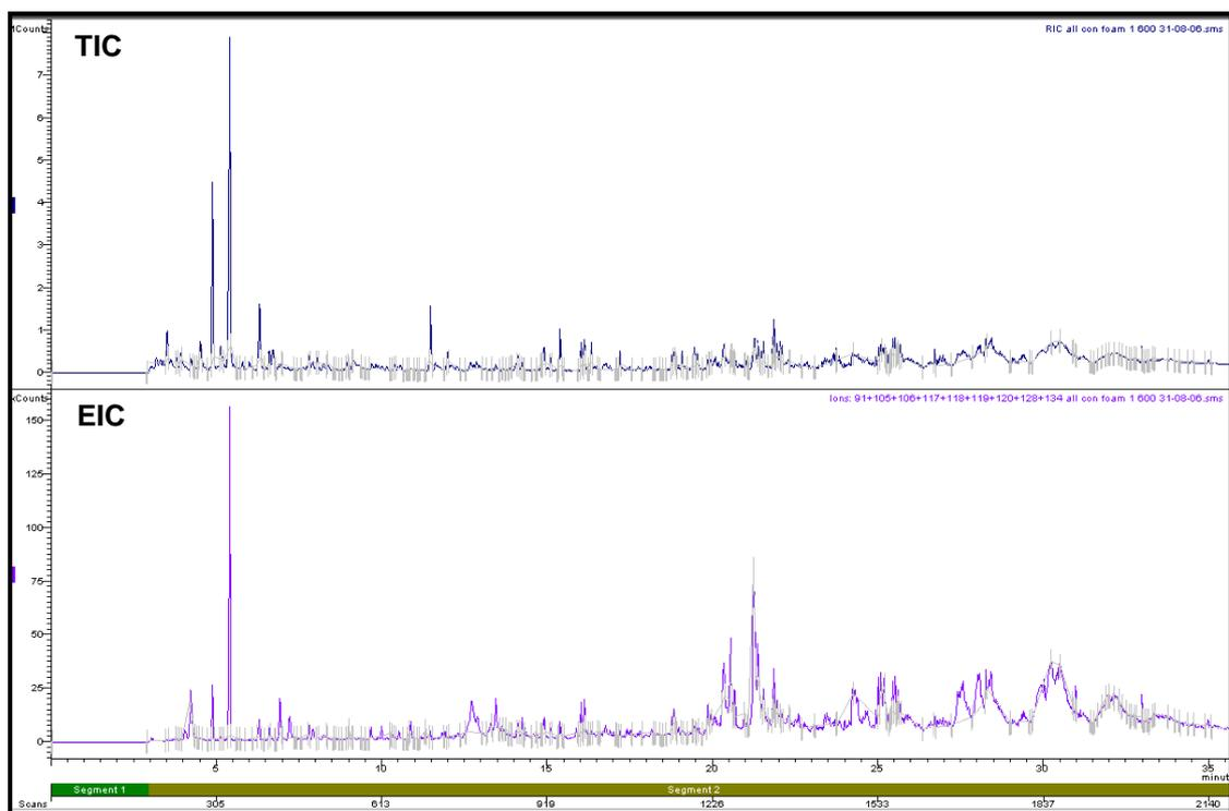
**Figure H8.5: Total Ion Chromatogram and Extracted Ion Chromatogram of Foam Pyrolysed at 600°C**
