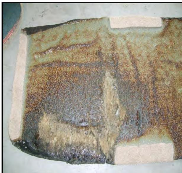
**Figure 4.15: Nylon Carpet after Furnace Burn at 433°C**
