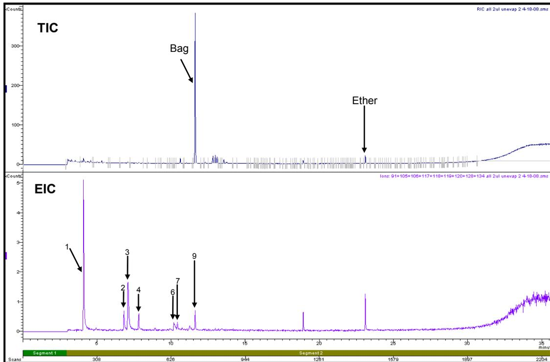
**Figure 3.48: Total Ion Chromatogram and Extracted Ion Chromatogram of KimWipe spiked with 2 $\mu$ L of Unevaporated Petrol (Refer to Section 2.5.1 for GC/MS conditions)**
