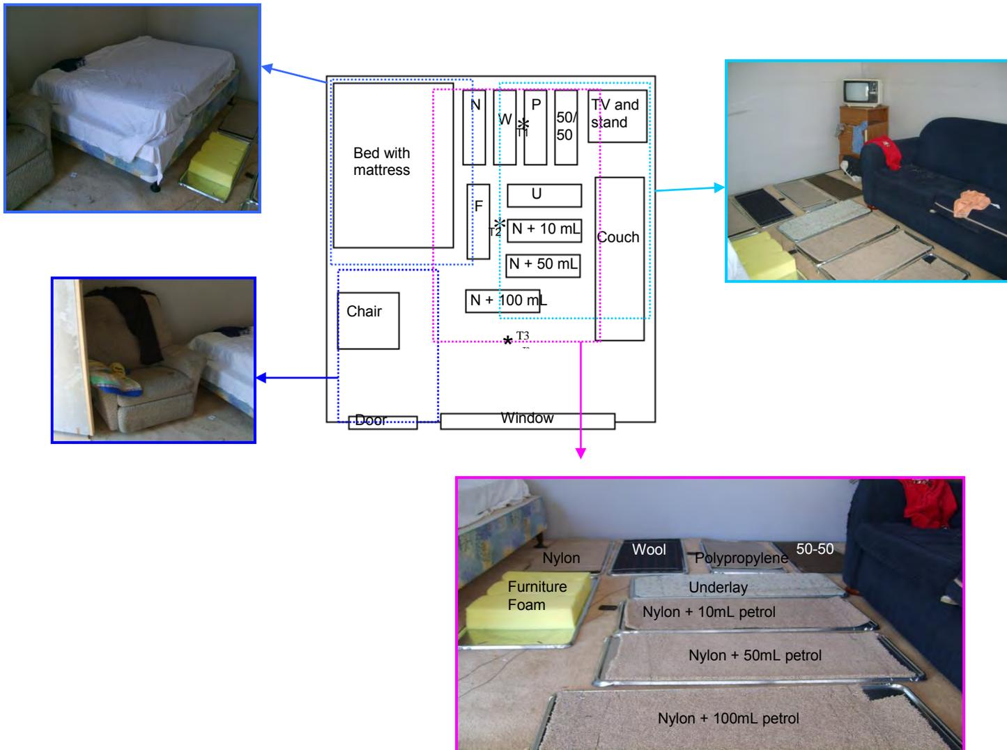
Figure 4.3: Layout of Room 3, with asterisk showing placement of the Thermocouples
