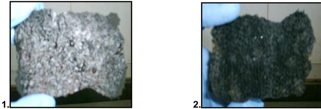
**Figure C1.17 (b): 1. Top and 2. Underside of Sample after Burning**
