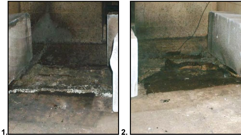
**Figure 4.20(b): Polypropylene Carpet after Extinguishment following the Furnace Burn at 470°C 1. Left Side and 2. Right Side of the Furnace**
