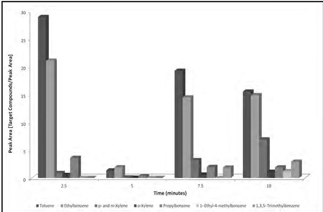
**Figure 4.51: Graph of Peak Area of Target Compounds with Butylated Hydroxytoluene vs. Burn Time for Polypropylene Carpet**
