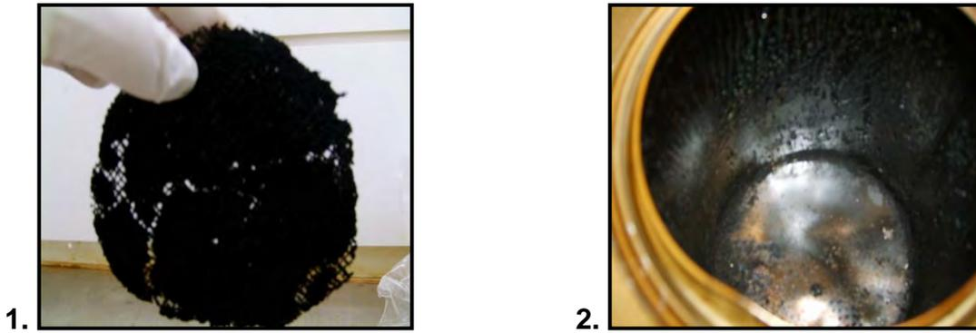
**Figure D3.7 (b): 1. Underside of Sample and 2. Side of Can after Burning**
