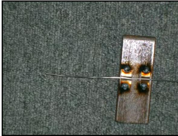
**Figure 3.71: Thermocouple placed 10mm above Carpet Fibres**
