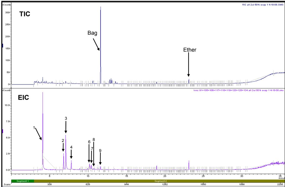
**Figure 3.50: Total Ion Chromatogram and Extracted Ion Chromatogram of KimWipe spiked with 2 $\mu$ L of 50% Evaporated Petrol (Refer to Section 2.5.1 for GC/MS conditions)**
