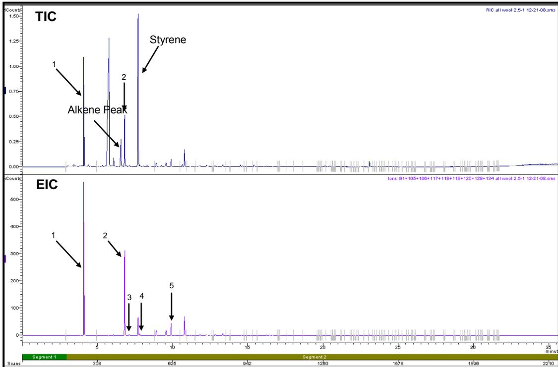
**Figure D2.2: Total Ion Chromatogram and Extracted Ion Chromatogram of a Wool Carpet Swatch burnt in a Can with Lid On for 2.5 minutes**
