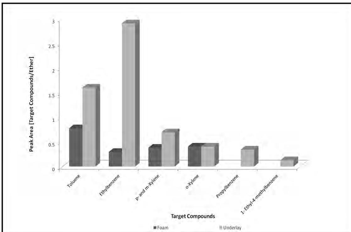
**Figure 4.57: Target Compound Chromatogram for Furniture Foam and Underlay burnt in a Small Can with Lid On for 7.5 minutes**
