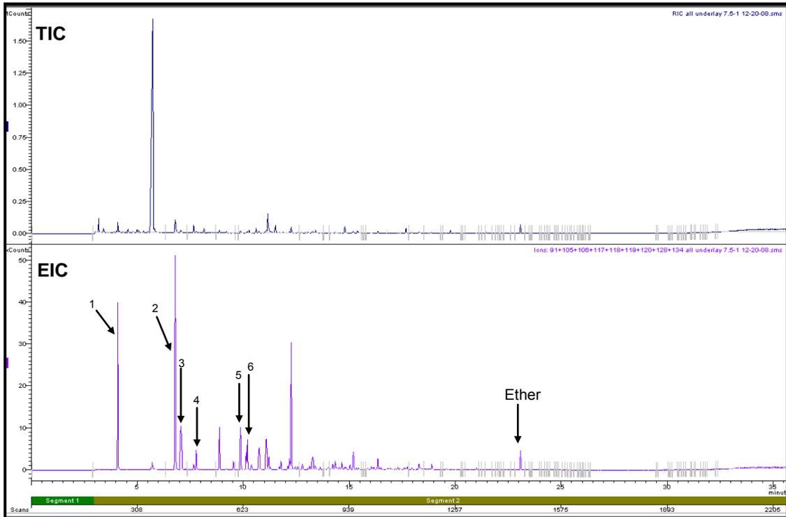
**Figure F2.10: Total Ion Chromatogram and Extracted Ion Chromatogram of Underlay Burnt in a Can with Lid On for 7.5 minutes**
