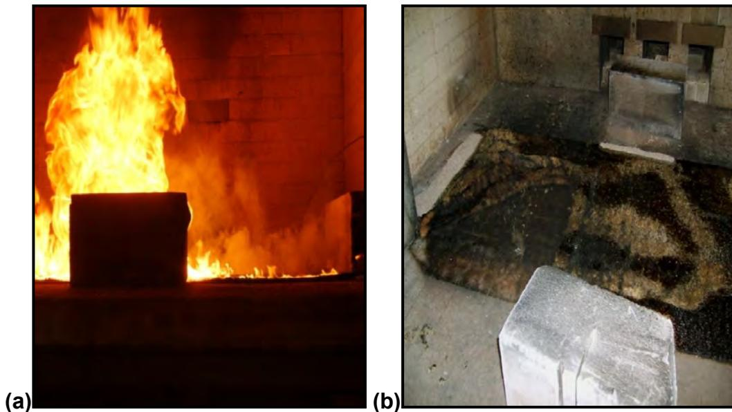
**Figure 4.14: Nylon Carpet after Furnace Burn at 483°C (a) When Doors were Opened (b) After Extinguishment**
