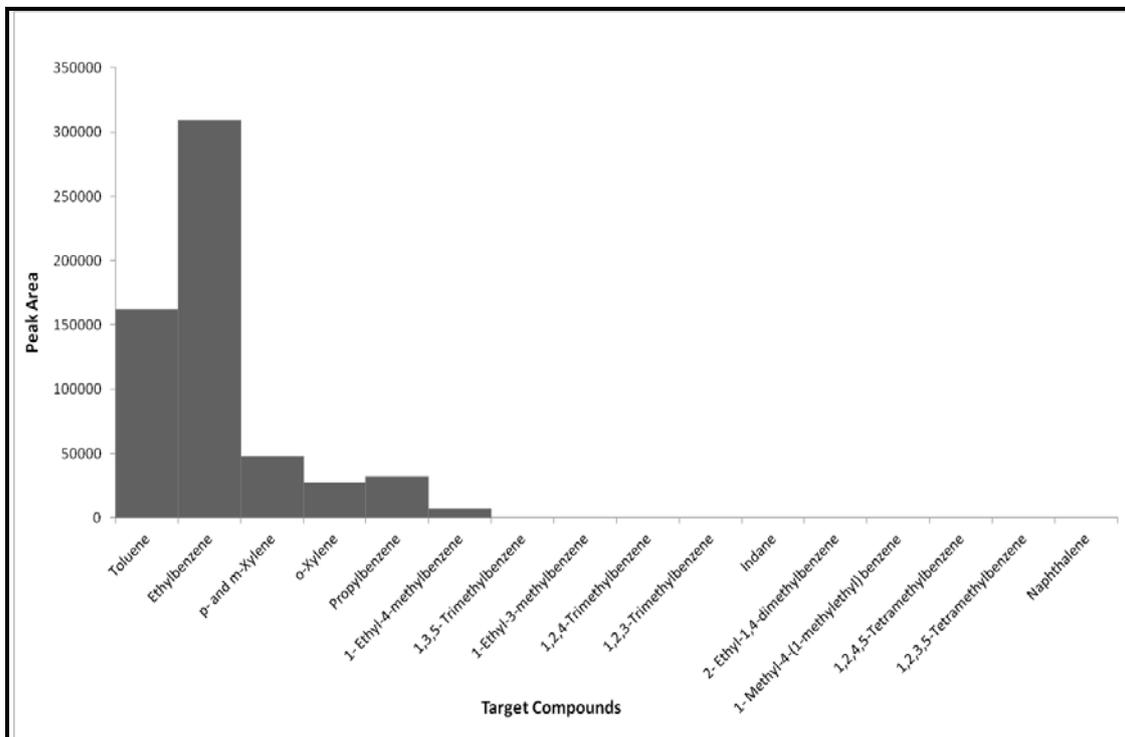
**Figure F2.8: Target Compound Chromatogram of Underlay Burnt in a Can with Lid On for 5 minutes**
