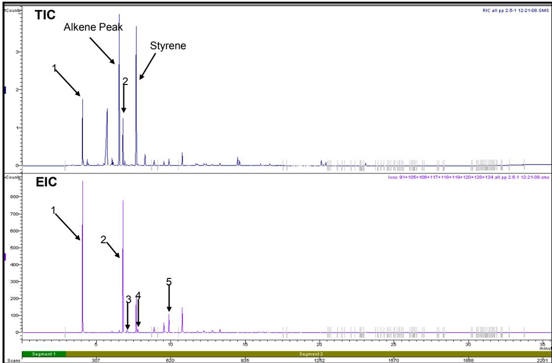
**Figure 4.44: Total Ion Chromatogram and Extracted Ion Chromatogram of a Polypropylene Carpet Swatch burnt in a Can with Lid On for 2.5 minutes (Refer to Section 2.5.1 for GC/MS conditions)**
