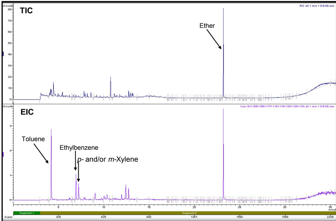
**Figure C1.4: Target Ion Chromatogram and Extracted Ion Chromatogram of a Nylon Carpet Swatch burnt in a Can with Lid On for 1 minute**
