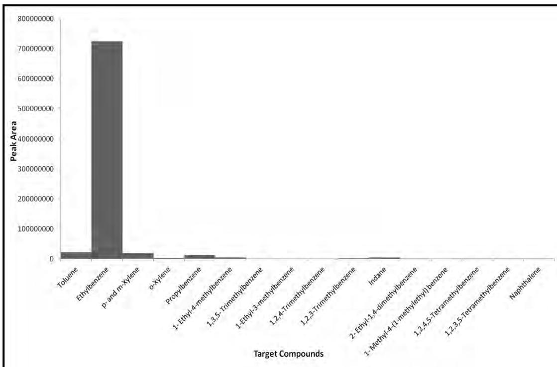
**Figure 4.61: Target Compound Chromatogram for Adhesive Pyrolysed at 750°C**
