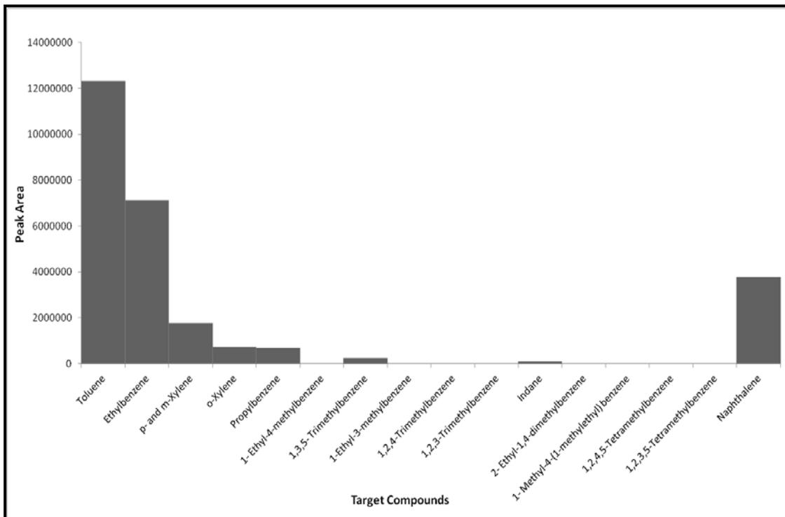
**Figure H9.4: Target Compound Chromatogram of Underlay Pyrolysed at 750°C**
