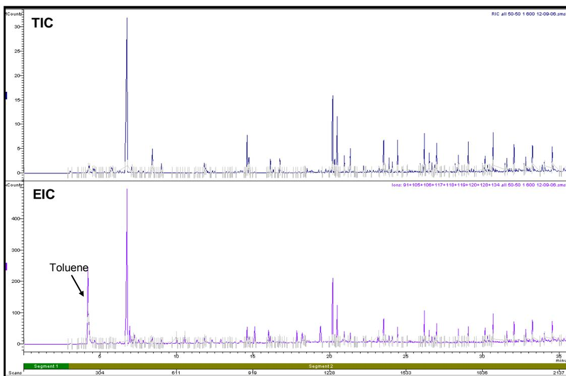
**Figure H7.5: Total Ion Chromatogram and Extracted Ion Chromatogram of 50-50 Polypropylene-Wool Fibres Pyrolysed at 600°C**
