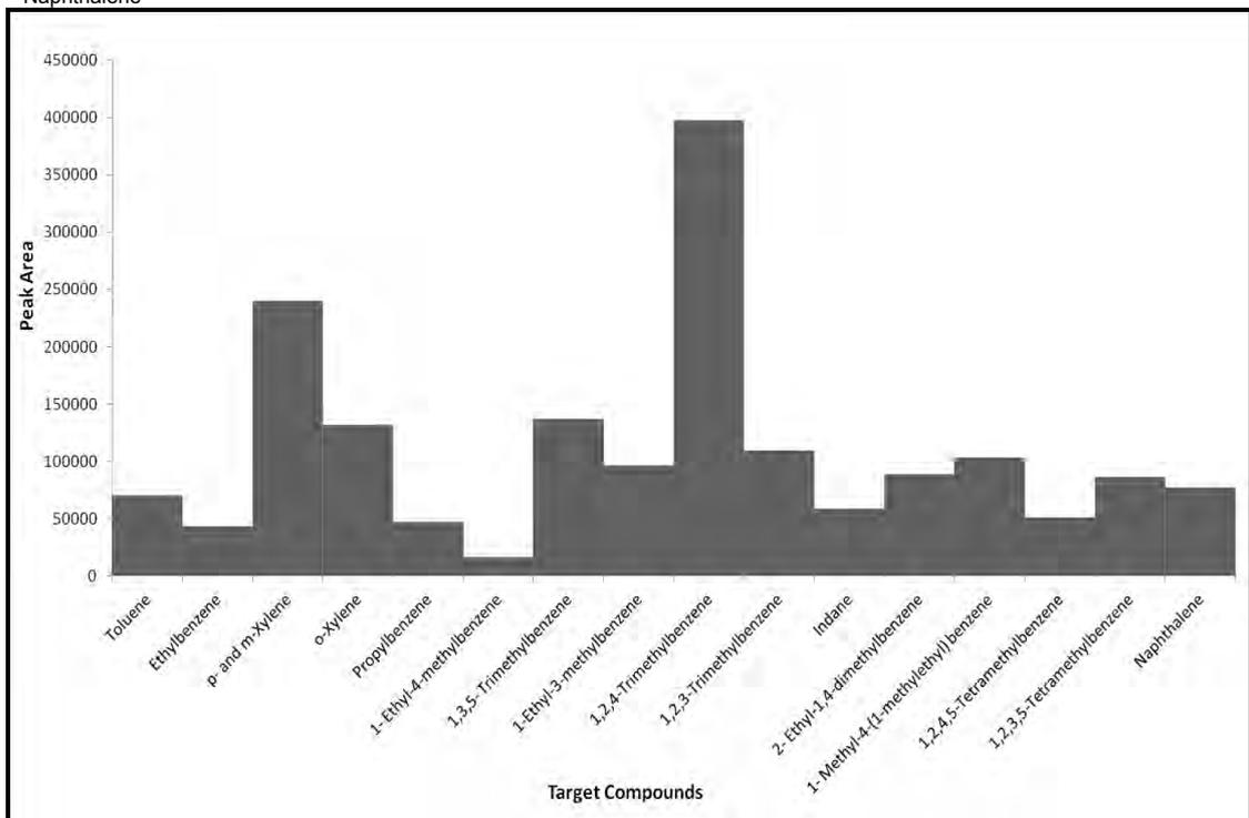
**Figure 3.21: Target Compound Chromatogram for 95% Evaporated Petrol Diluted to 0.1% (v/v)**
