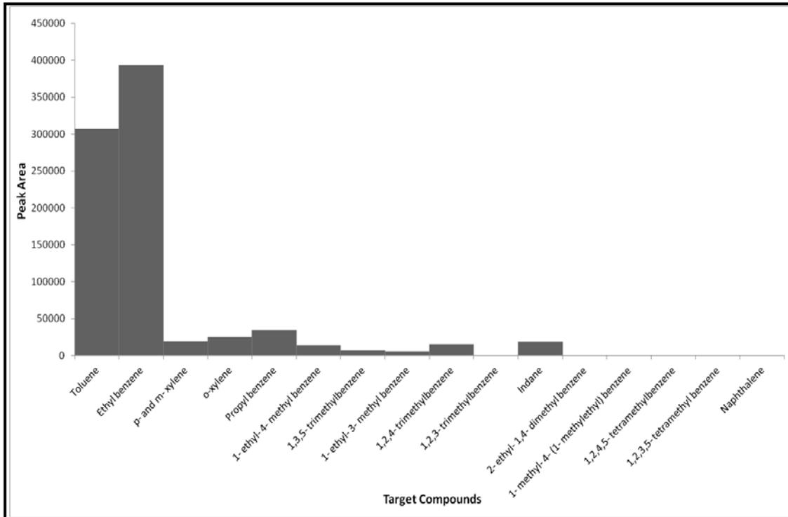
**Figure C1.28: Target Compound Chromatogram of a Nylon Carpet Swatch burnt in a Can with Lid On for 7.5 minutes**
