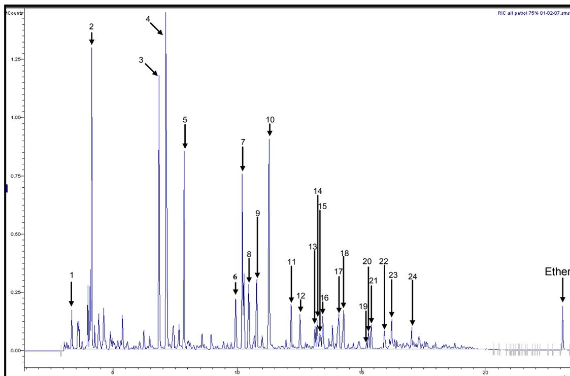
**Figure 3.3: Total Ion Chromatogram of Petrol Indicating Peak Numbers for Identification (Refer to Section 2.5.1 for GC/MS conditions)**
