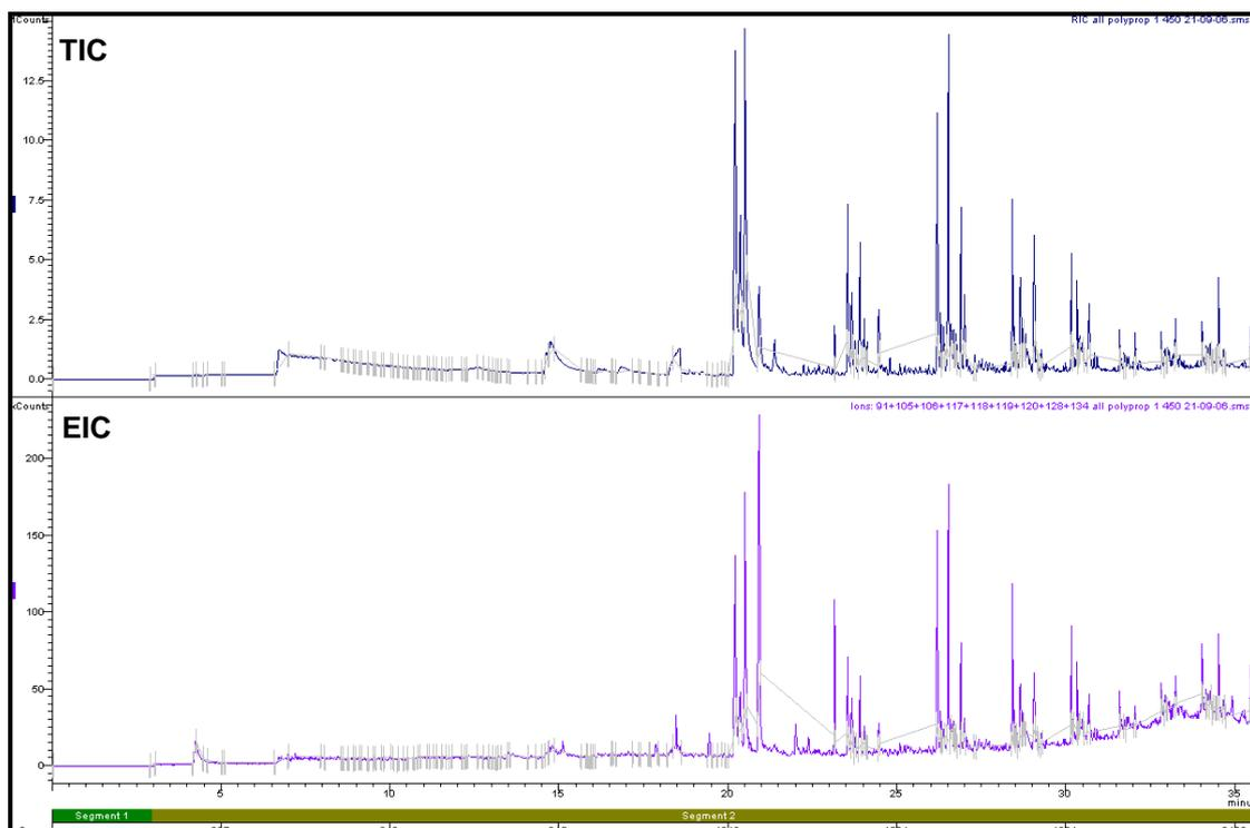
**Figure H5.6: Total Ion Chromatogram and Extracted Ion Chromatogram of Polypropylene Fibres Pyrolysed at 450°C**
