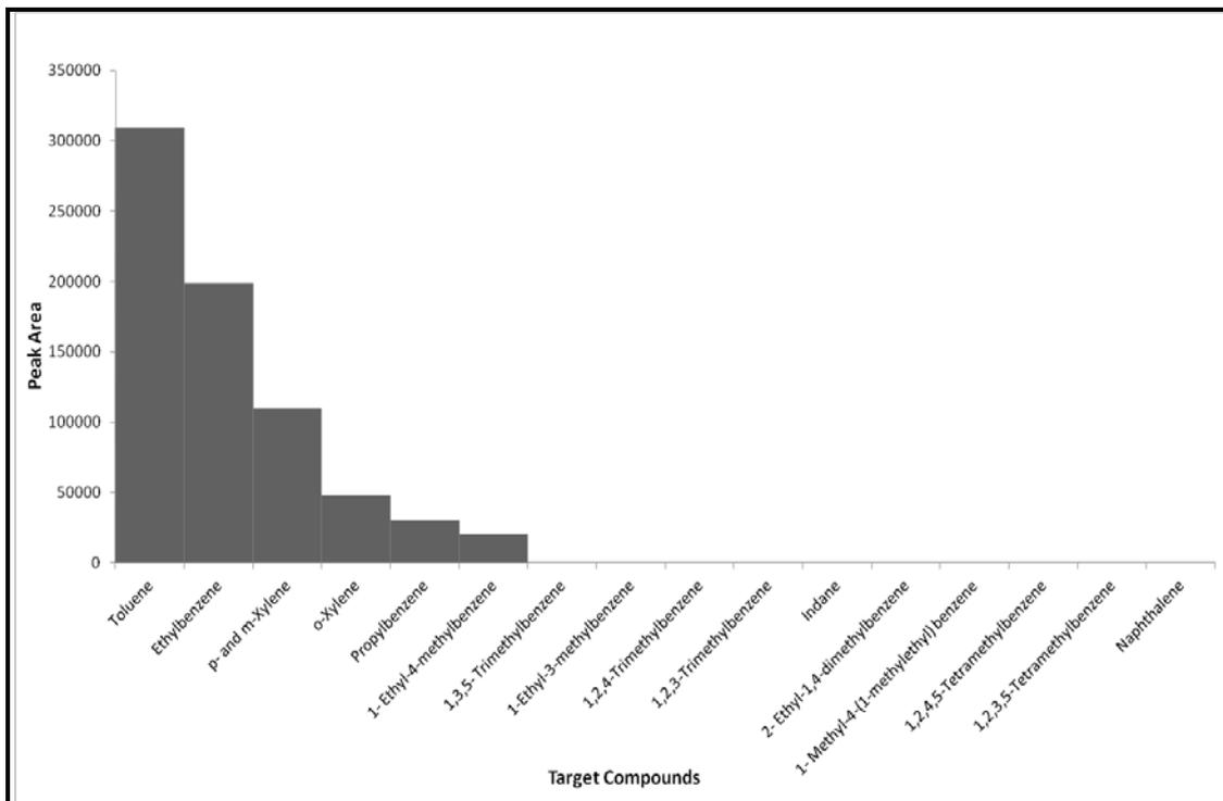
**Figure F2.14: Target Compound Chromatogram of Underlay Burnt in a Can with Lid On for 10 minutes**
