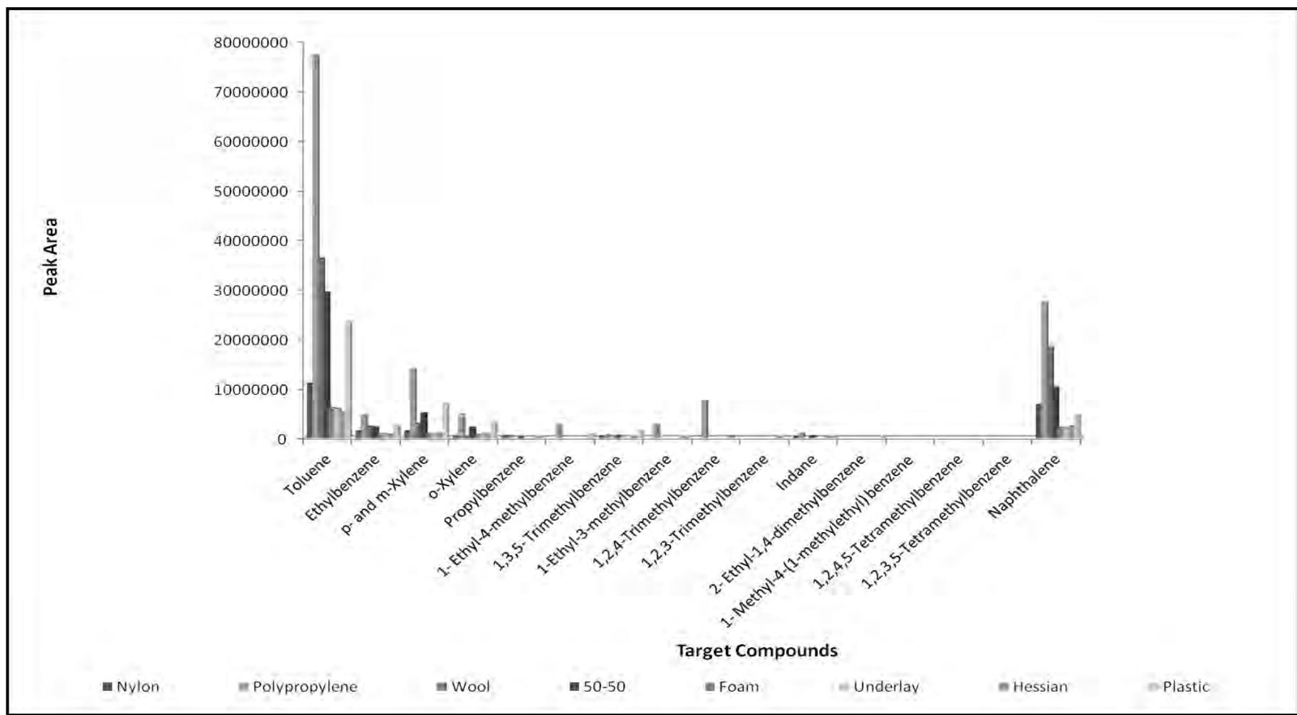
**Figure 4.63: Target Compound Chromatograms incorporating Carpet Fibres and Carpet Backing Components Pyrolysed at 900°C**
