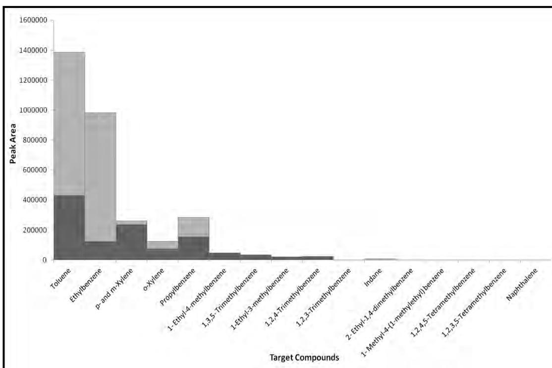
**Figure 5.2: Hypothetical Target Compound Chromatogram of Fire Debris containing Petrol Residue (dark grey) superimposed with Interferences from Carpet and Foam (light grey)**
