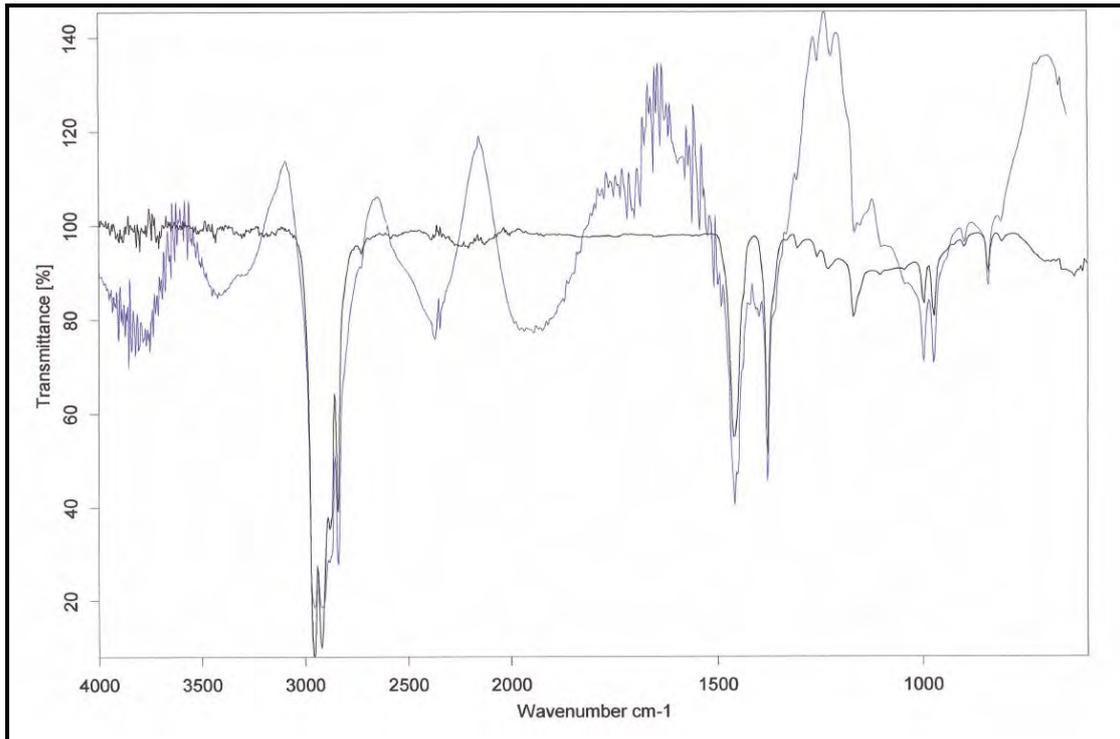
**Figure 3.63: FTIR Spectra of 1 ply 100% Polypropylene Standard (blue) compared with Polypropylene from Library (black)**
