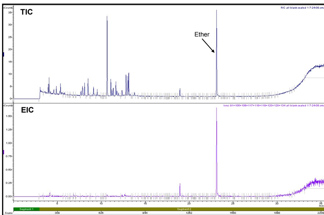
**Figure 4.33: Total Ion Chromatogram and Extracted Ion Chromatogram of burnt 'Can Blank with Lid On' (Refer to Section 2.5.1 for GC/MS conditions)**
