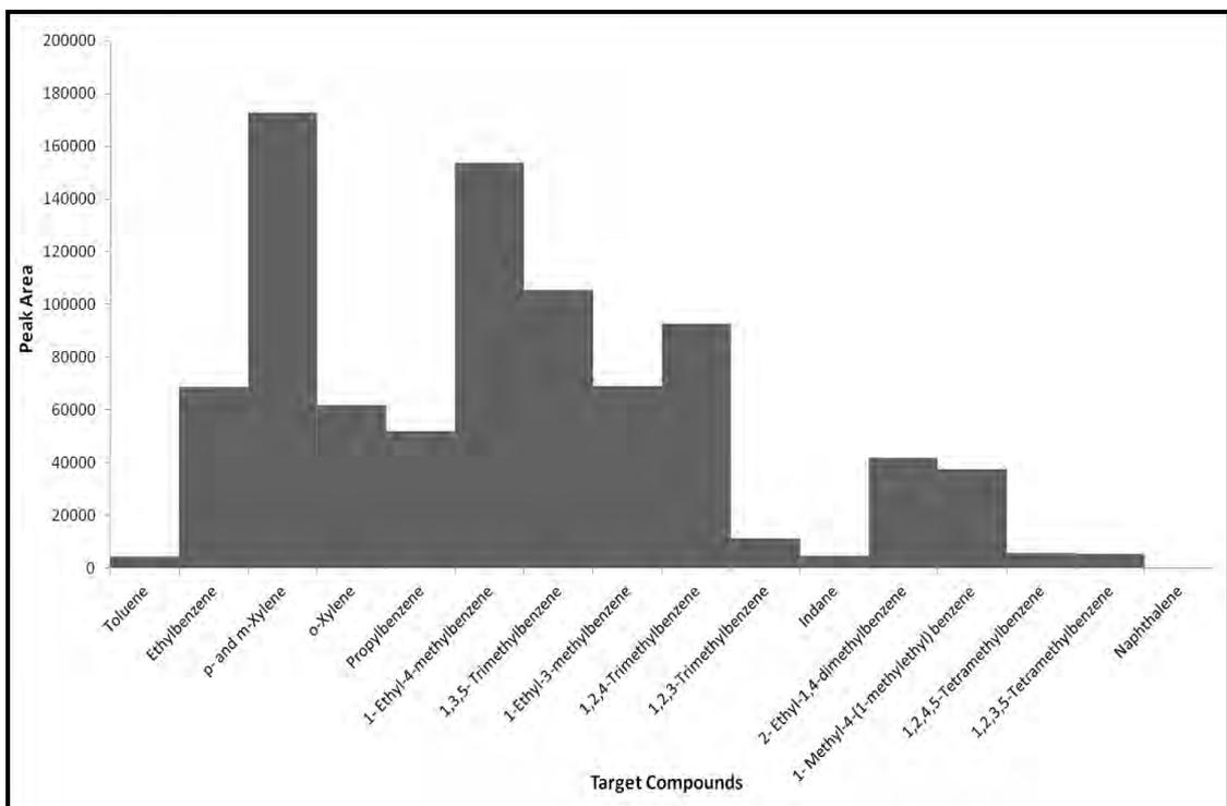
**Figure 3.47: Target Compound Chromatogram of KimWipe spiked with 10 $\mu$ L of 95% Evaporated Petrol**
