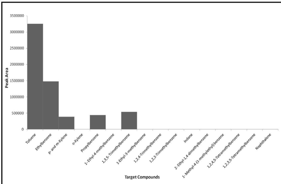
**Figure H9.6: Target Compound Chromatogram of Underlay Pyrolysed at 600°C**
