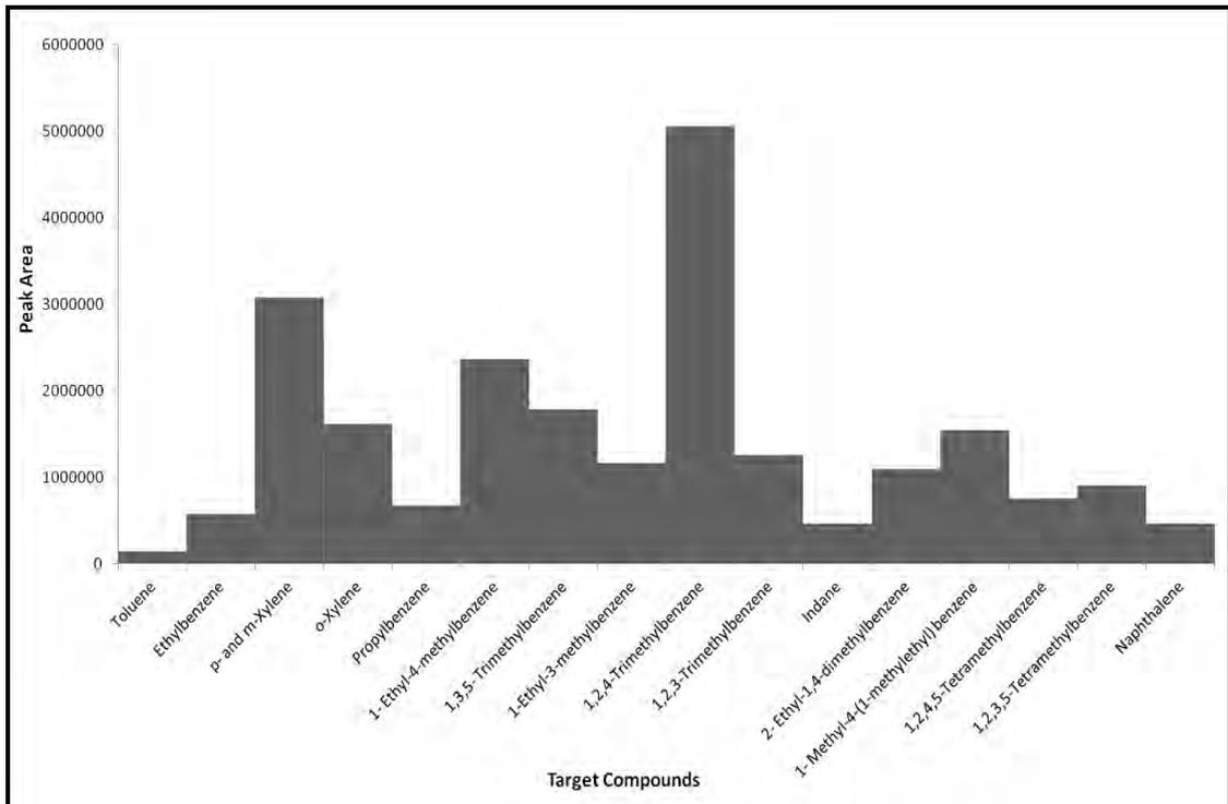
**Figure 3.15: Target Compound Chromatogram for 95% Evaporated Petrol Diluted to 1% (v/v)**
