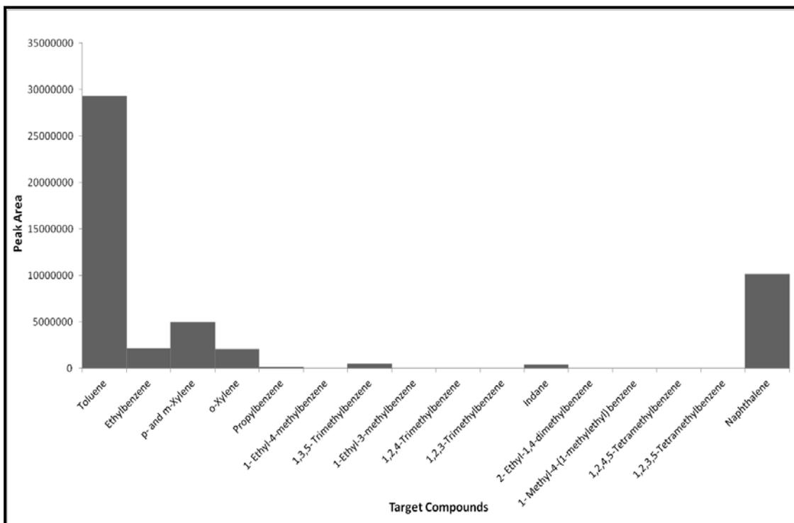
**Figure H7.2: Target Compound Chromatogram of 50-50 Polypropylene-Wool Fibres Pyrolysed at 900°C**
