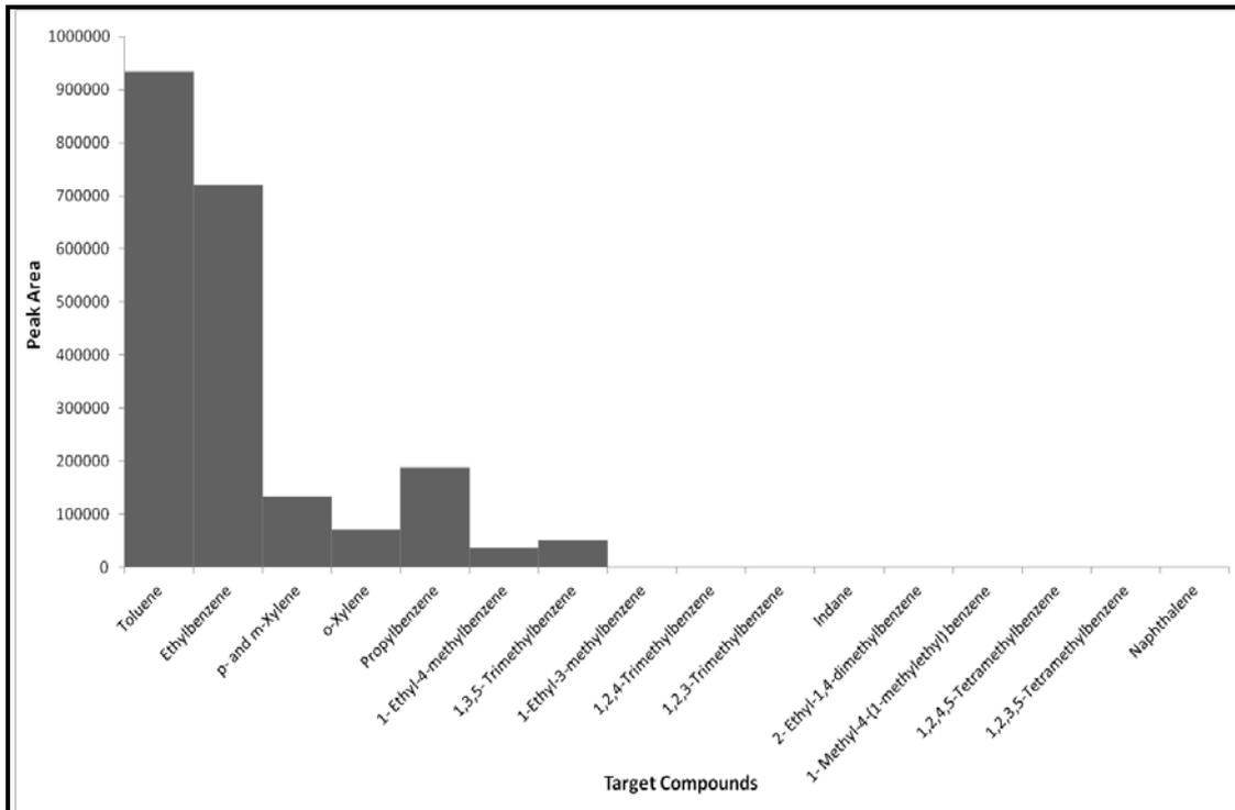
**Figure B1.2: Target Compound Chromatogram of Nylon Swatch placed Face Down in the Bottom of a Can burnt with Lid On**
