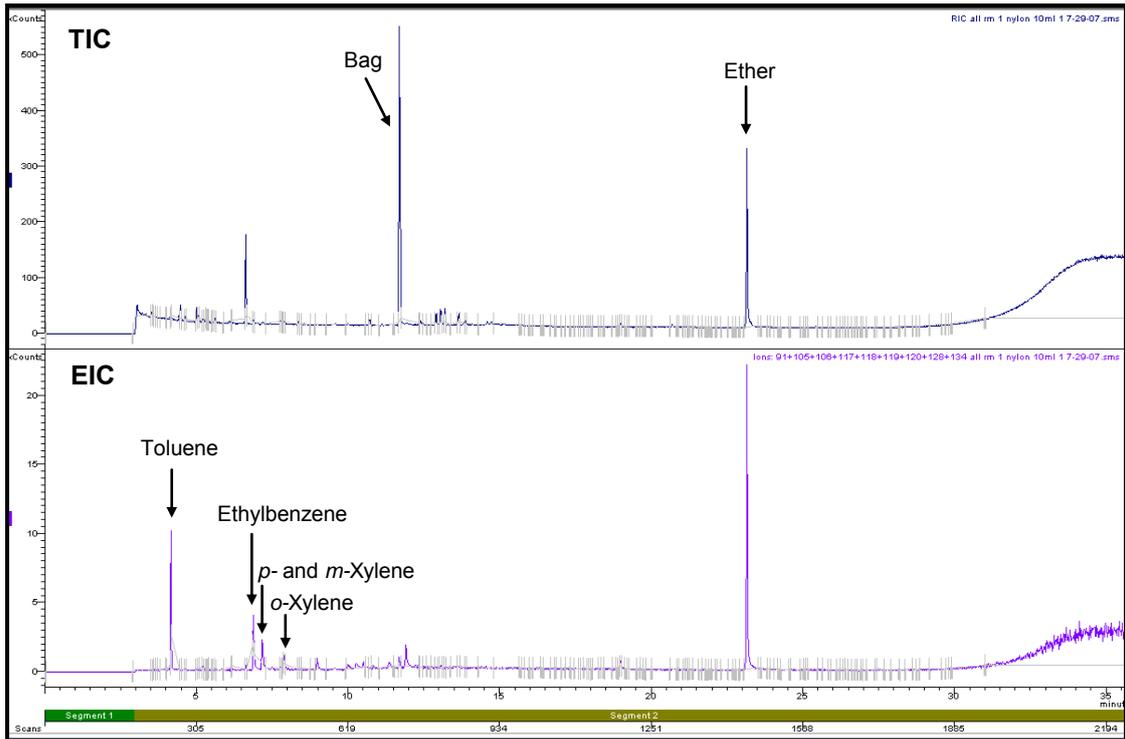
**Figure 4.6: Total Ion Chromatogram and Extracted Ion Chromatogram of Nylon Carpet spiked with 10mL Petrol burnt in Room 1 (Refer to Section 2.5.1 for GC/MS conditions)**
