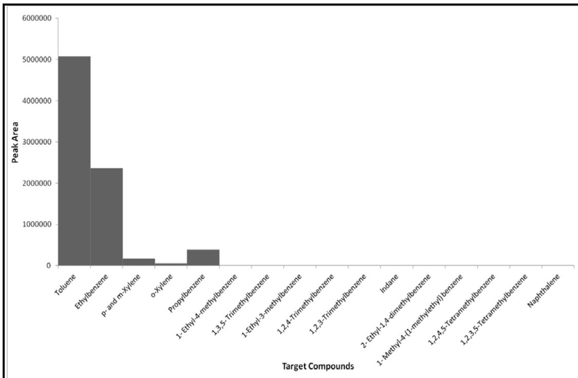
**Figure D3.3: Target Compound Chromatogram of a 50-50 Polypropylene-Wool Carpet Swatch burnt in a Can with Lid On for 2.5 minutes**
