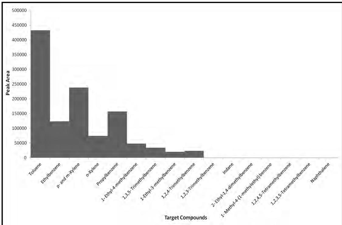
**Figure 3.45: Target Compound Chromatogram of KimWipe spiked with 10 $\mu$ L of 50% Evaporated Petrol**
