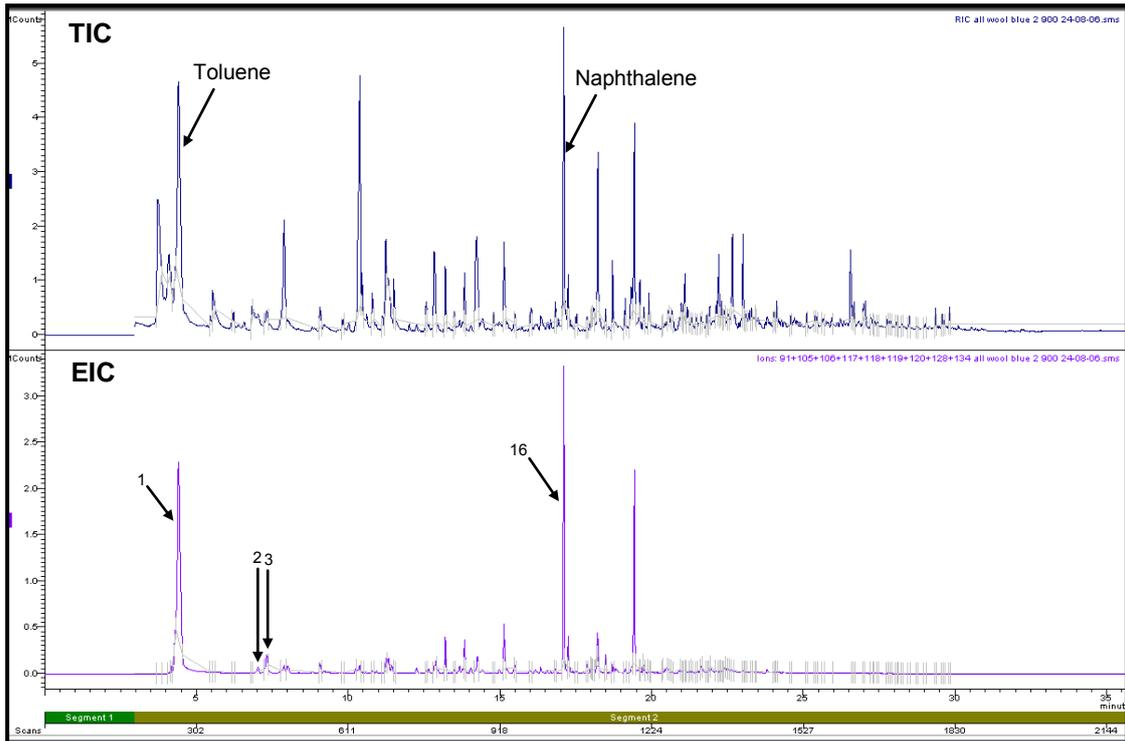
**Figure H6.1: Total Ion Chromatogram and Extracted Ion Chromatogram of Wool Fibres Pyrolysed at 900°C**
