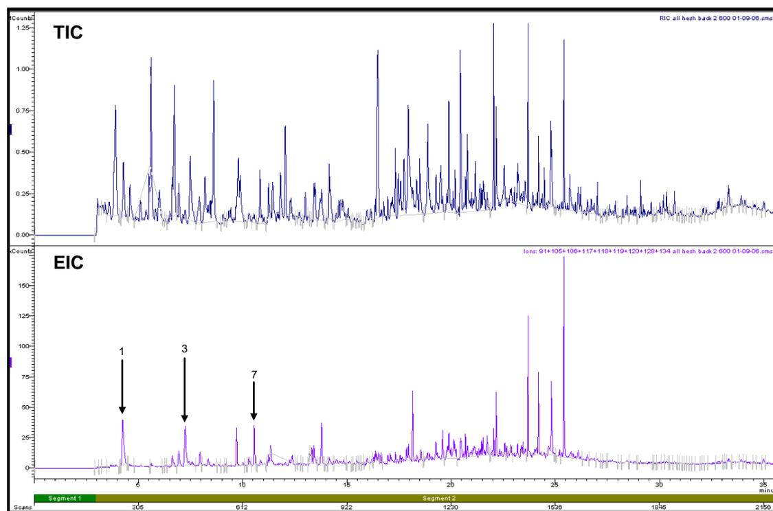
**Figure H2.5: Total Ion Chromatogram and Extracted Ion Chromatogram of Hessian Carpet Backing Pyrolysed at 600°C**
