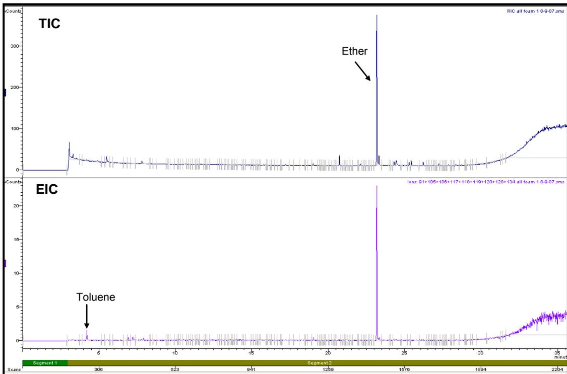
**Figure A1.2(e): Target Ion Chromatogram and Extracted Ion Chromatogram of Foam burnt in Room 1**
