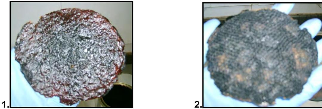
**Figure C1.9 (b): 1. Top and 2. Underside of Sample after Burning**
