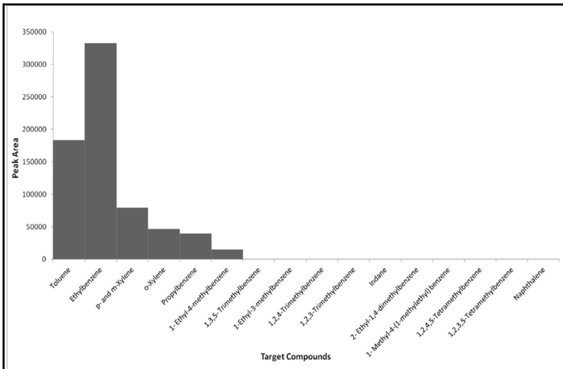
**Figure F2.11: Target Compound Chromatogram of Underlay Burnt in a Can with Lid On for 7.5 minutes**
