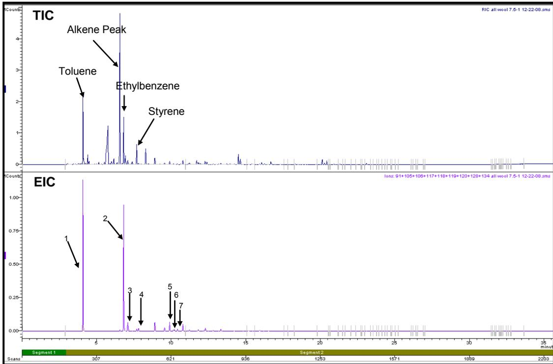
**Figure D2.8: Total Ion Chromatogram and Extracted Ion Chromatogram of a Wool Carpet Swatch burnt in a Can with Lid On for 7.5 minutes**
