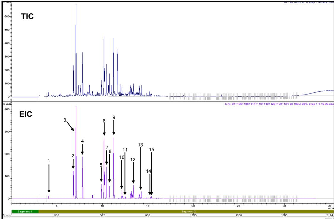
**Figure 3.40: Total Ion Chromatogram and Extracted Ion Chromatogram of KimWipe spiked with 100µL of 95% Evaporated Petrol (Refer to Section 2.5.1 for GC/MS conditions)**
