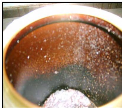
**Figure C1.9 (c): Inside of Can after Burning**
