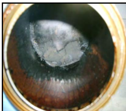
**Figure C1.23 (c): Inside of Can after Burning**
