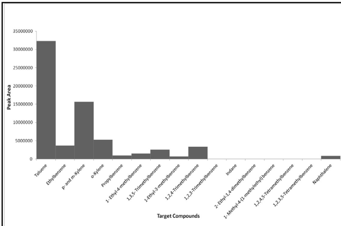
**Figure H3.4: Target Compound Chromatogram of Plastic Carpet Backing Pyrolysed at 750°C**
