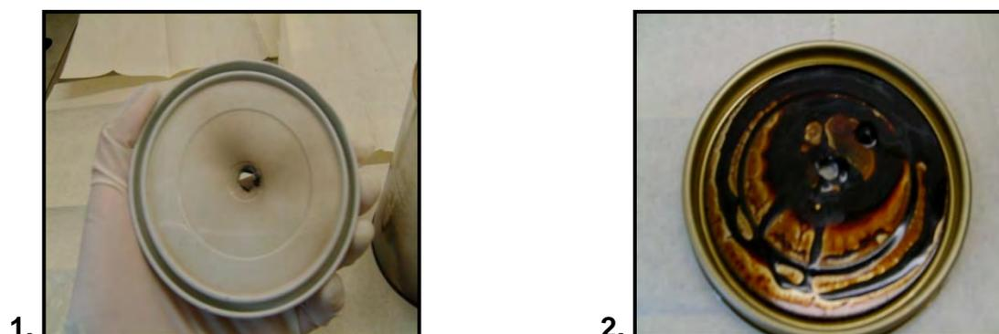
**Figure D2.4 (a): 1. Top and 2. Underside of Lid after Burning**
