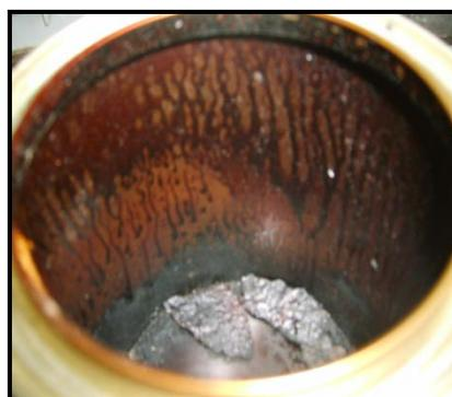
**Figure C1.20 (c): Inside of Can after Burning**
