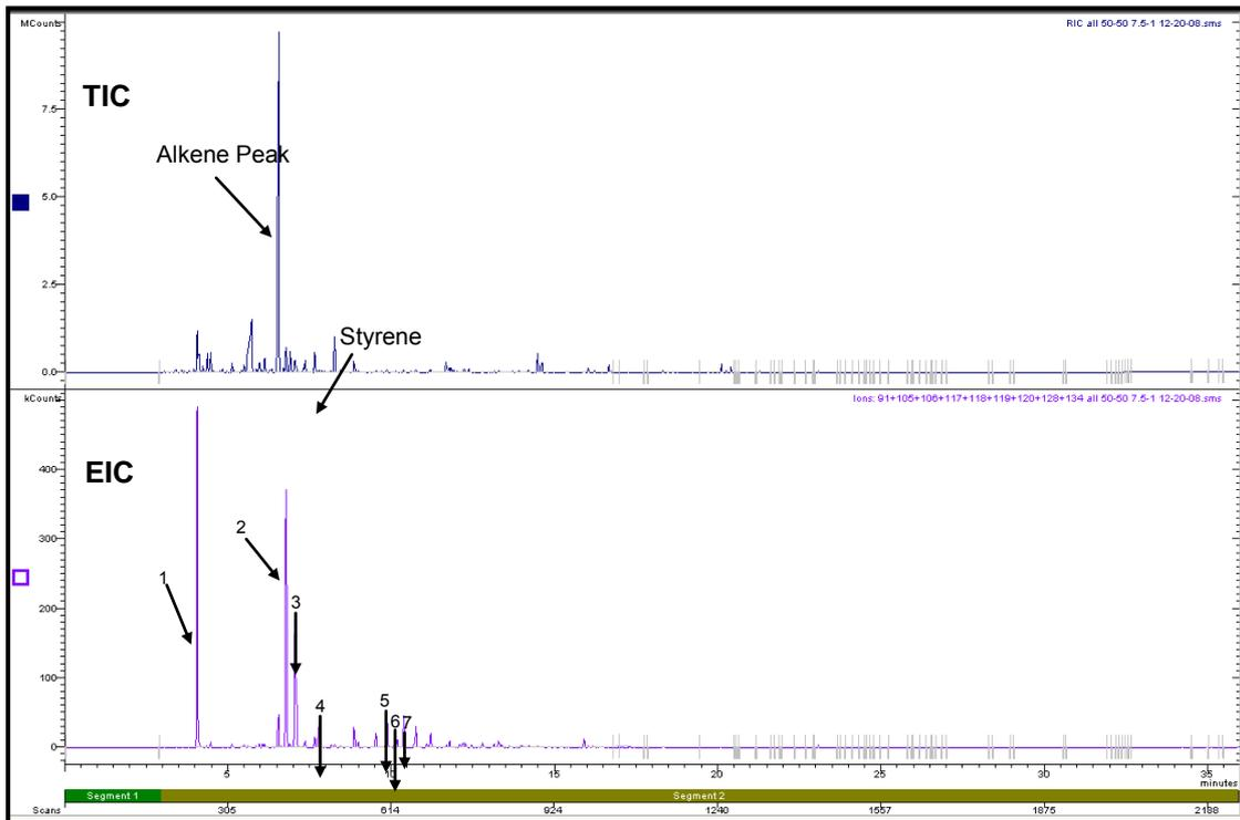
**Figure D3.8: Total Ion Chromatogram and Extracted Ion Chromatogram of a 50-50 Polypropylene-Wool Carpet Swatch burnt in a Can with Lid On for 7.5 minutes** Key: 1= Toluene, 2= Ethylbenzene, 3= *p*- and *m*-Xylene, 4= *o*-Xylene, 5= Propylbenzene, 6= 1-Ethyl-4-methylbenzene, 7= 1,3,5-Trimethylbenzene
