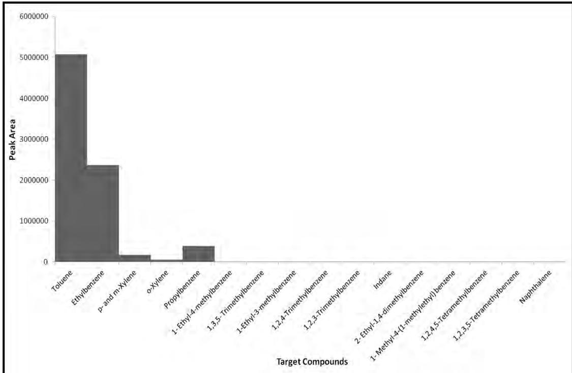
**Figure 4.49: Target Compound Chromatogram of a 50-50 Polypropylene-Wool Carpet Swatch burnt in a Can with Lid On for 2.5 minutes**
