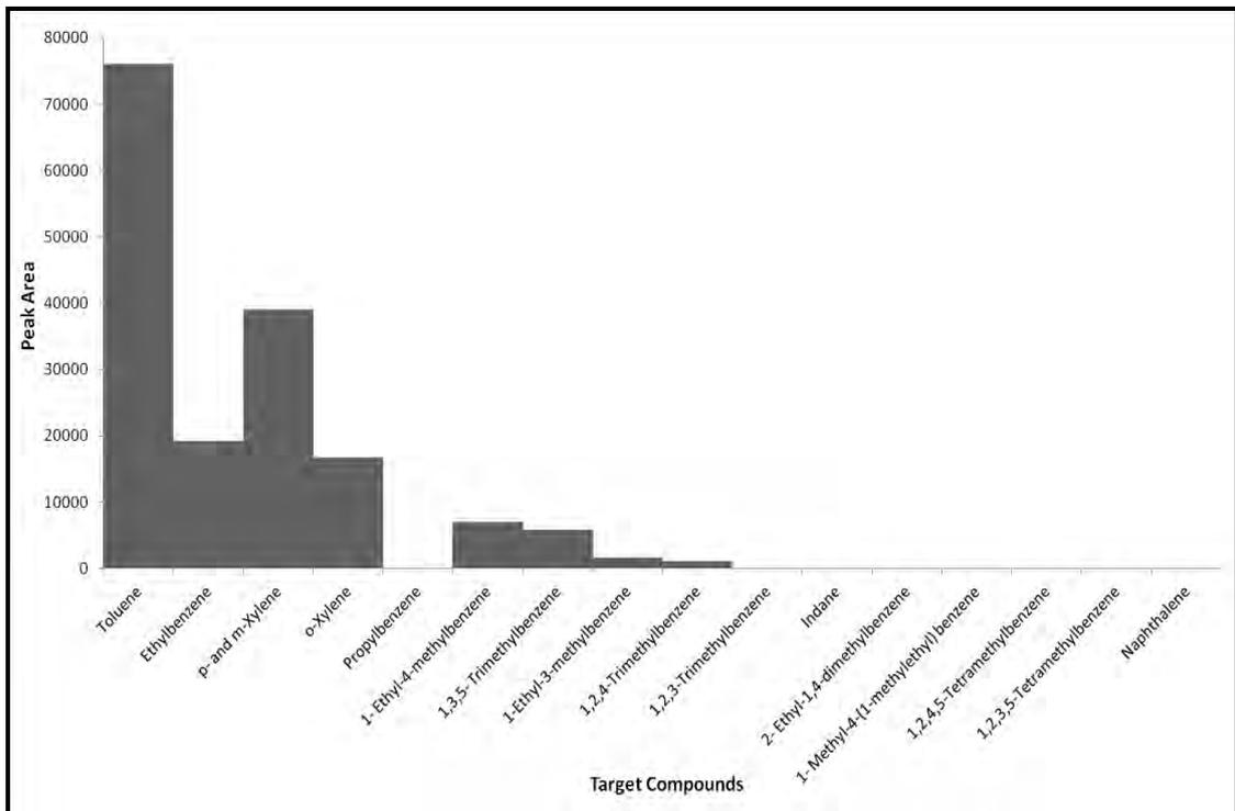
**Figure 3.51: Target Compound Chromatogram of KimWipe spiked with 2 $\mu$ L of 50% Evaporated Petrol**
