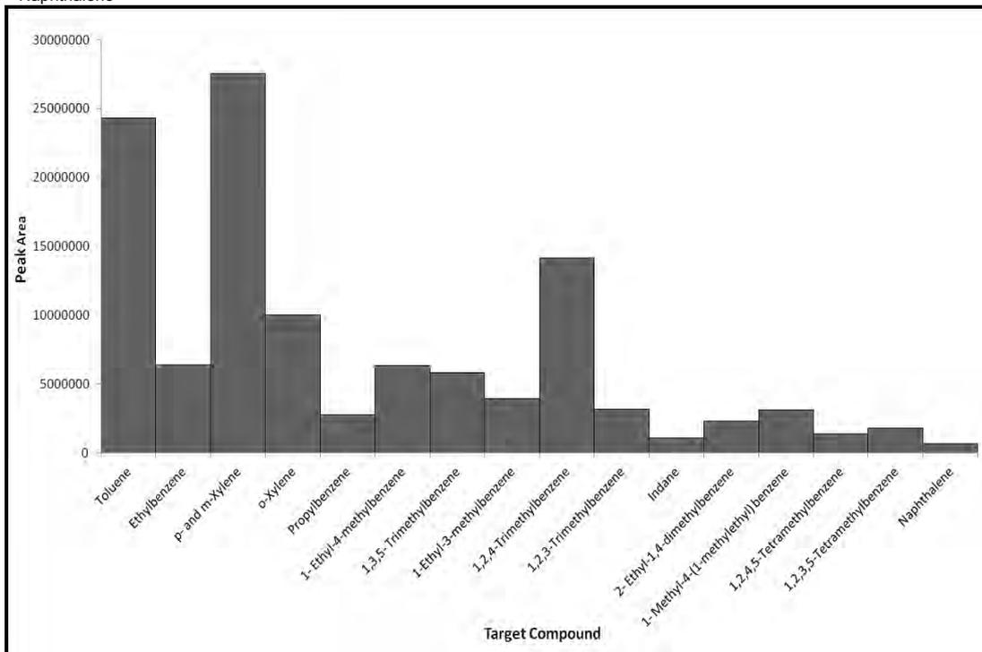
**Figure 3.5: Target Compound Chromatogram for Unevaporated Petrol Diluted to 10% (v/v)**
