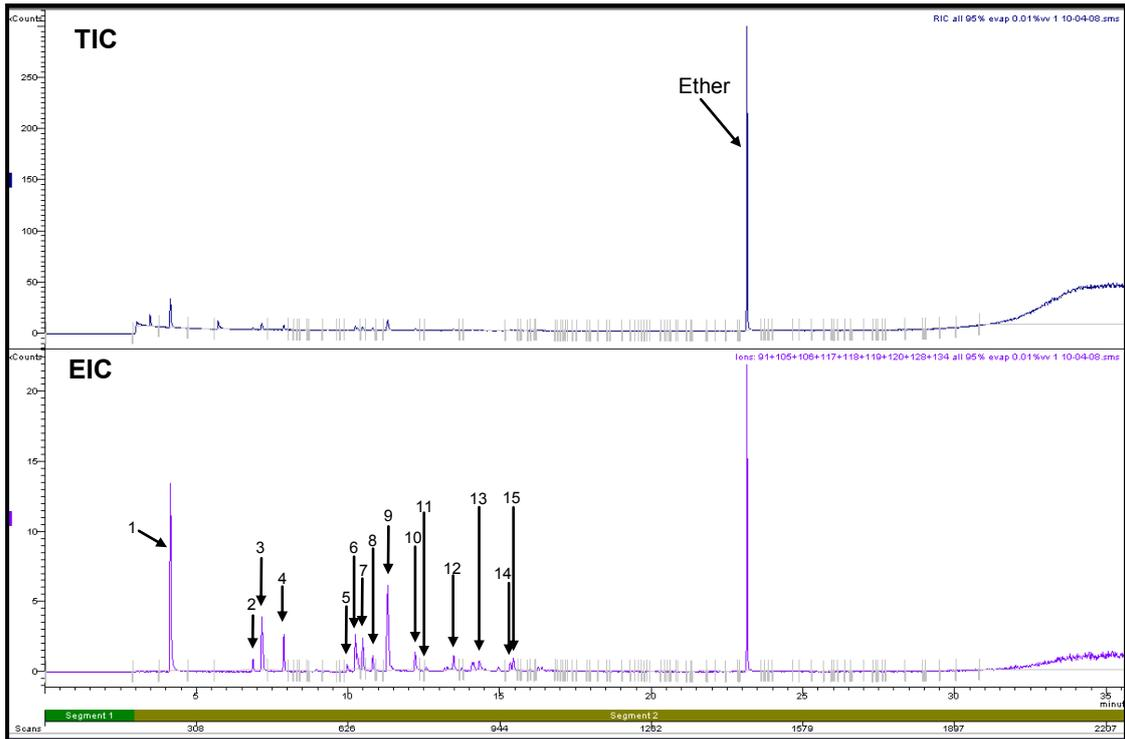
**Figure 3.26: Total Ion Chromatogram and Extracted Ion Chromatogram for 95% Evaporated Petrol Diluted to 0.01% (v/v) (Refer to Section 2.5.1 for GC/MS conditions)**
