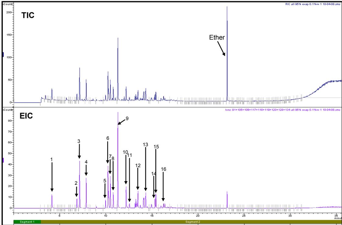
**Figure 3.20: Total Ion Chromatogram and Extracted Ion Chromatogram for 95% Evaporated Petrol Diluted to 0.1% (v/v) (Refer to Section 2.5.1 for GC/MS conditions)**
