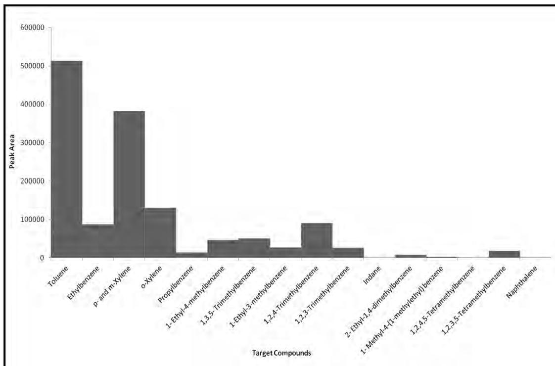
**Figure 3.17: Target Compound Chromatogram for Unevaporated Petrol Diluted to 0.1% (v/v)**
