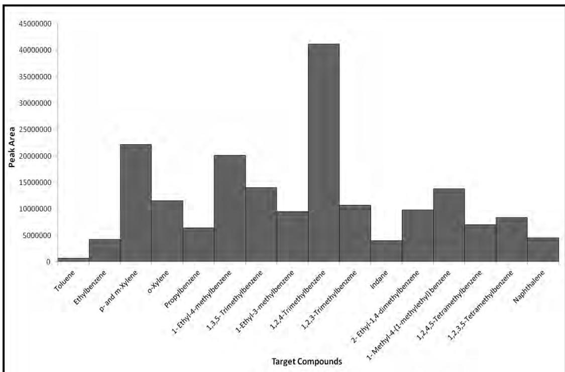
**Figure 3.9: Target Compound Chromatogram for 95% Evaporated Petrol Diluted to 10% (v/v)**
