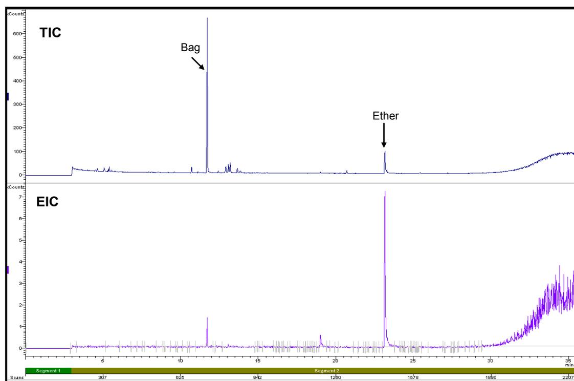
**Figure 3.35: Total Ion Chromatogram and Extracted Ion Chromatogram of blank KimWipe (Refer to Section 2.5.1 for GC/MS conditions)**
