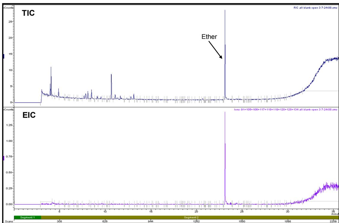
**Figure 4.27: Total Ion Chromatogram and Extracted Ion Chromatogram of 'Can Blank' (Refer to Section 2.5.1 for GC/MS conditions)**
