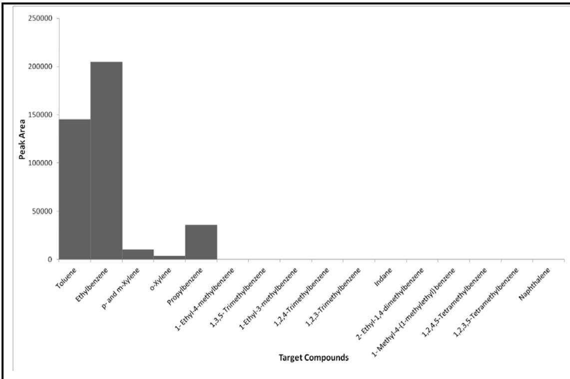
**Figure D1.6: Target Compound Chromatogram of a Polypropylene Carpet Swatch burnt in a Can with Lid On for 5 minutes**
