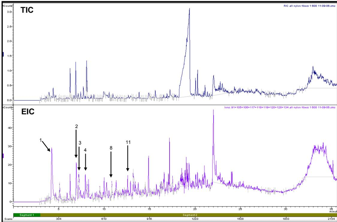
**Figure H1.5: Total Ion Chromatogram and Extracted Ion Chromatogram of Nylon Fibres Pyrolysed at 600°C**
