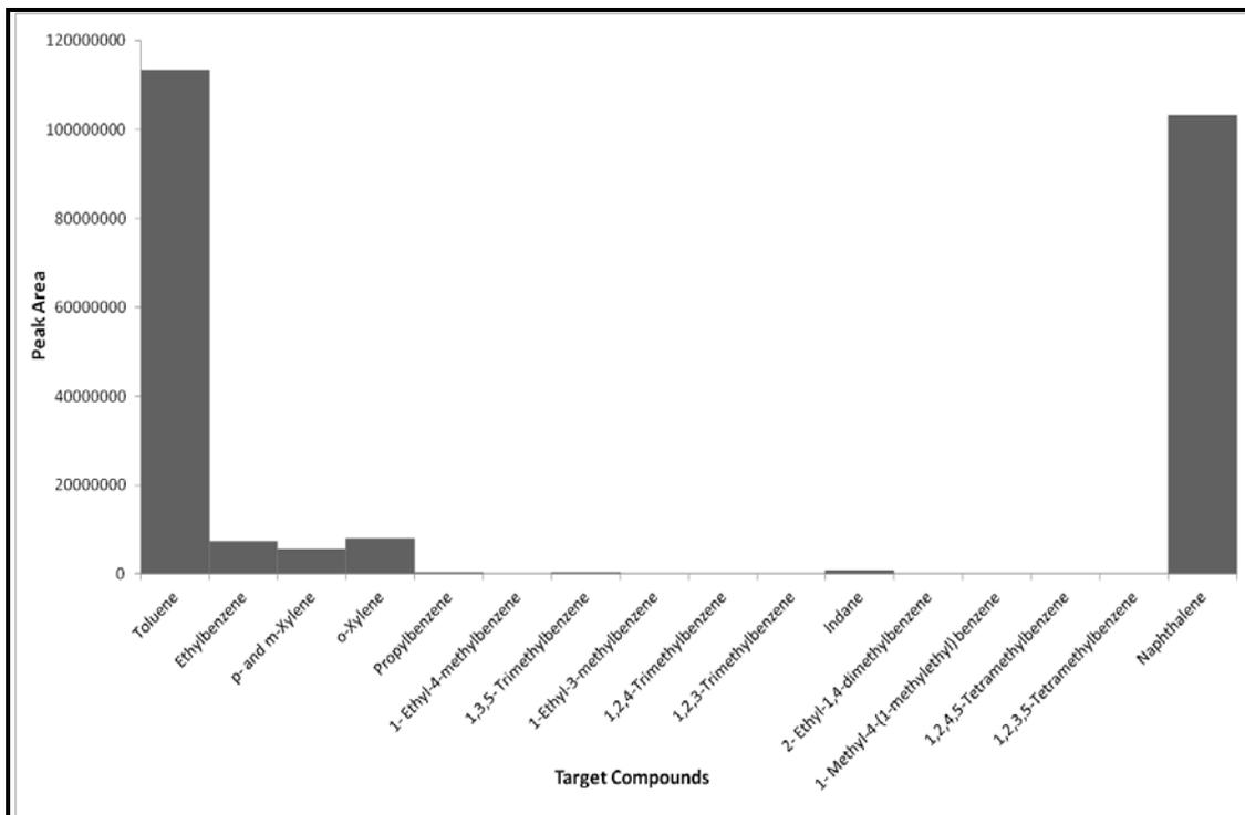
**Figure H4.2: Target Compound Chromatogram of Adhesive from Carpet Backing Pyrolysed at 900°C**
