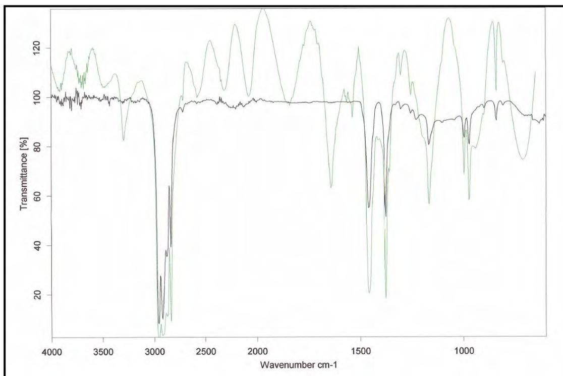
**Figure 3.62: FTIR Spectra of Polypropylene Carpet Sample (green) compared with Polypropylene from Library (black)**
