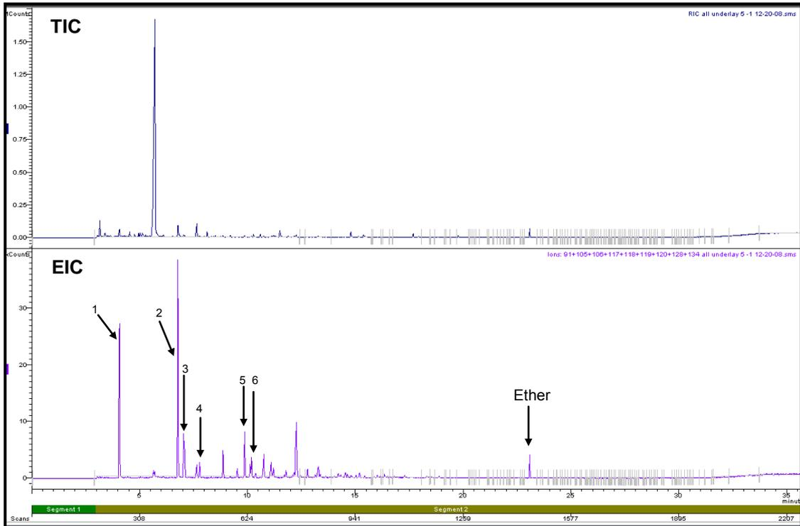
**Figure F2.7: Total Ion Chromatogram and Extracted Ion Chromatogram of Underlay Burnt in a Can with Lid On for 5 minutes**
