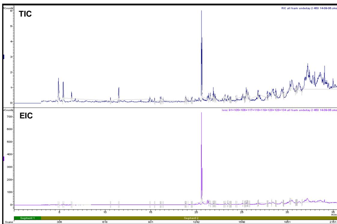
**Figure H9.7: Total Ion Chromatogram and Extracted Ion Chromatogram of Underlay Pyrolysed at 450°C**
