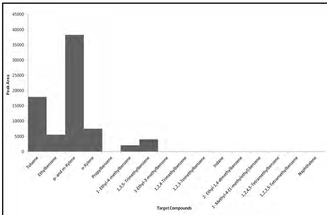
**Figure 3.29: Target Compound Chromatogram for Unevaporated Petrol Diluted to 0.001% (v/v)**
