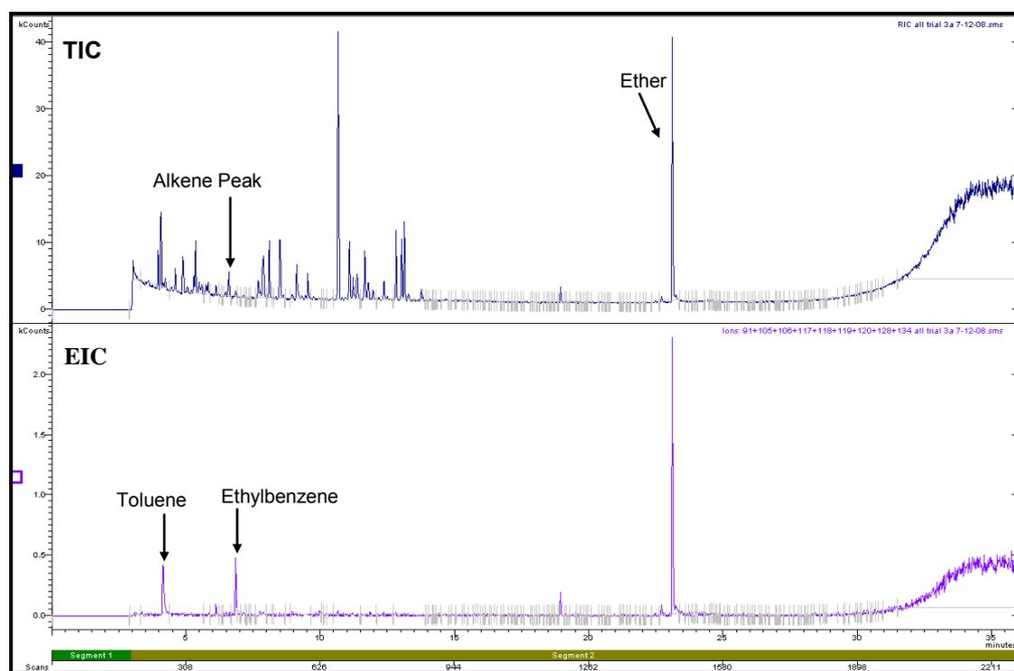
**Figure 4.31: Total Ion Chromatogram and Extracted Ion Chromatogram of Nylon burnt in a Small Can with Lid Off (Refer to Section 2.5.1 for GC/MS conditions)**
