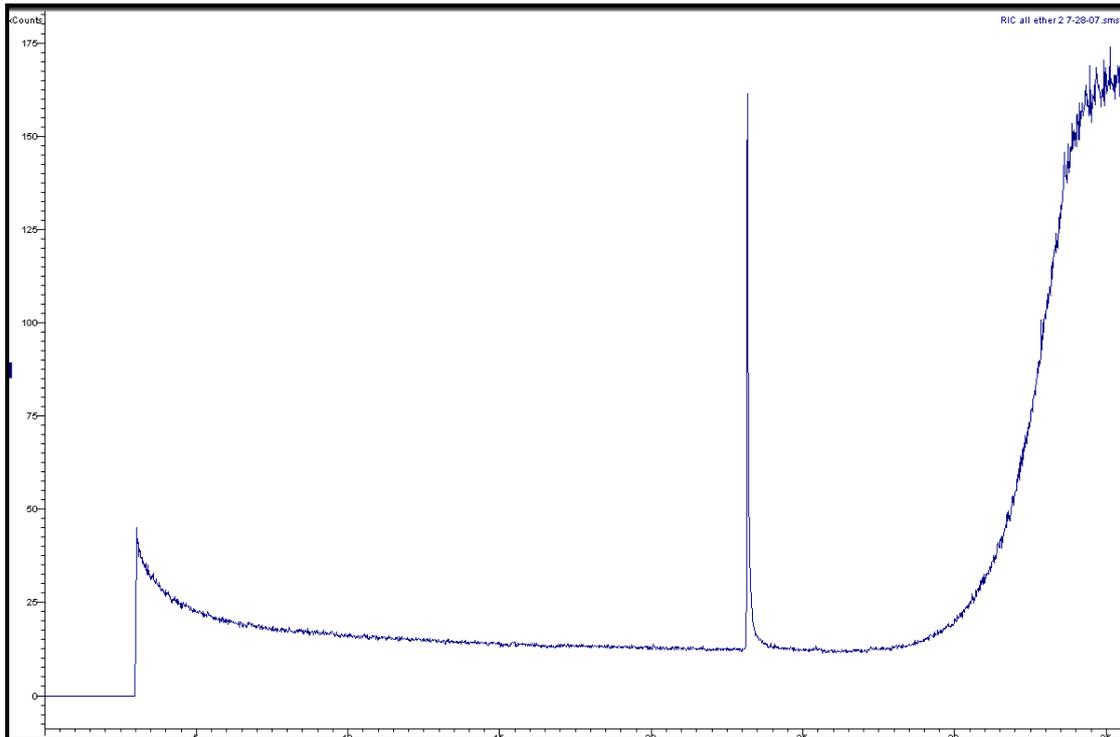
**Figure 3.1: Total Ion Chromatogram of Diethyl ether (Refer to Section 2.5.1 for GC/MS conditions)**
