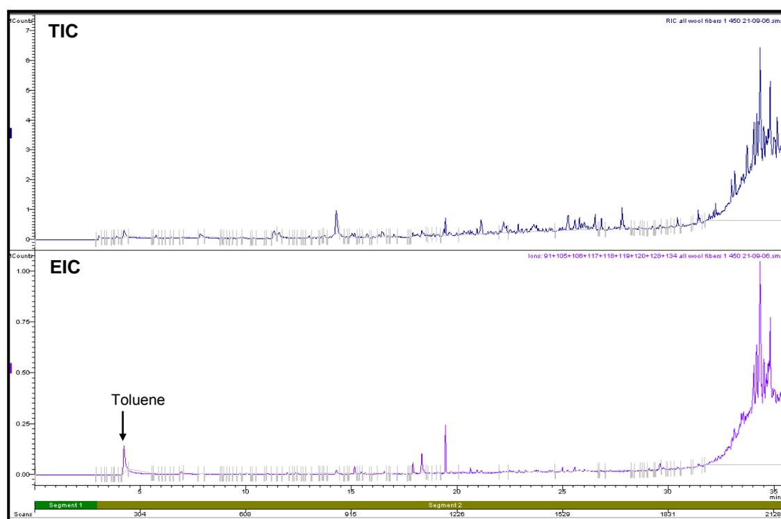
**Figure H6.7: Total Ion Chromatogram and Extracted Ion Chromatogram of Wool Fibres Pyrolysed at 450°C**
