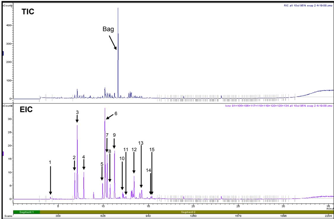
**Figure 3.46: Total Ion Chromatogram and Extracted Ion Chromatogram of KimWipe spiked with 10 $\mu$ L of 95% Evaporated Petrol (Refer to Section 2.5.1 for GC/MS conditions)**
