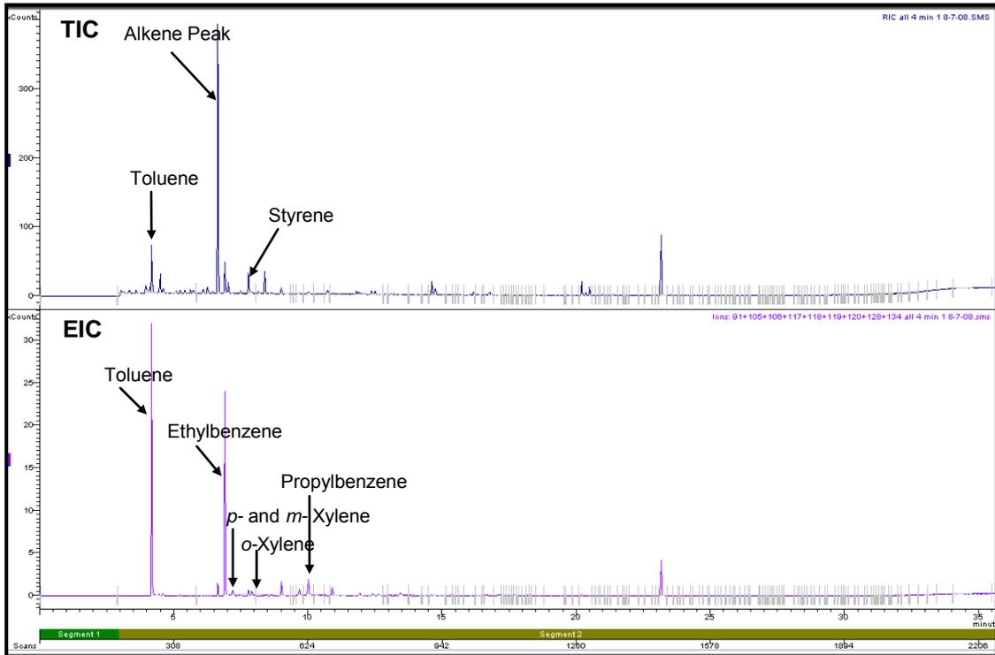
**Figure C1.18: Target Ion Chromatogram and Extracted Ion Chromatogram of a Nylon Carpet Swatch burnt in a Can with Lid On for 4 minutes**
