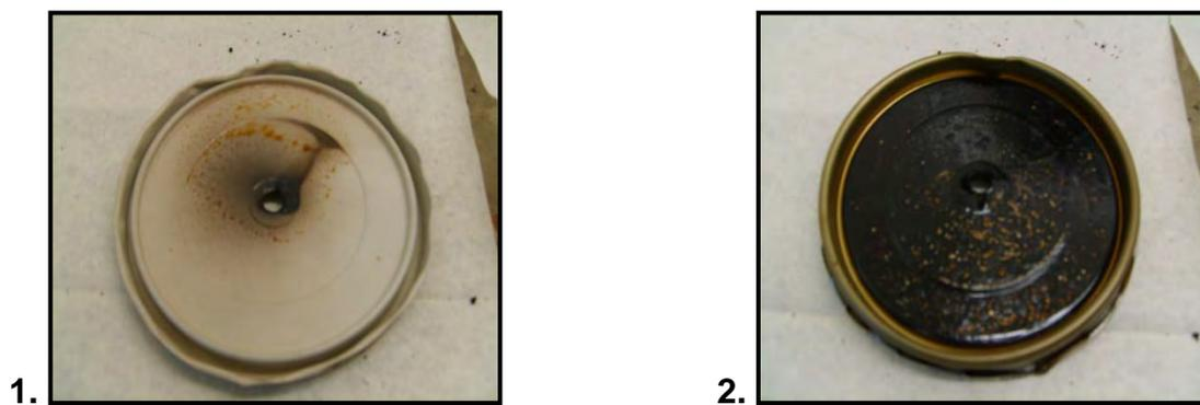
**Figure D3.7 (a): 1. Top and 2. Underside of Lid after Burning**
