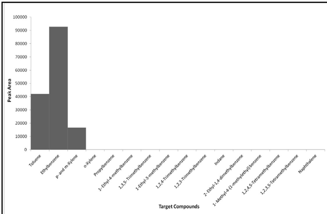
**Figure F1.5: Target Compound Chromatogram of Foam Burnt in a Can with Lid On for 5 minutes**
