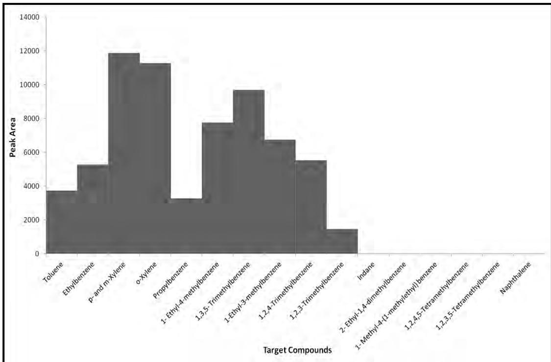
**Figure 3.53: Target Compound Chromatogram of KimWipe spiked with 2µL of 95% Evaporated Petrol**
