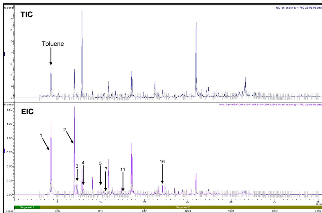
**Figure H9.3: Total Ion Chromatogram and Extracted Ion Chromatogram of Underlay Pyrolysed at 750°C**
