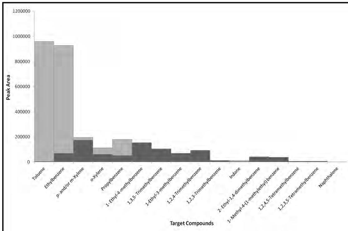
**Figure 5.3: Hypothetical Target Compound Chromatogram of Fire Debris containing Heavily Evaporated Petrol Residue (dark grey) superimposed with Interferences from Carpet and Foam (light grey)**
