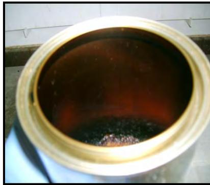
**Figure C1.7 (c): Inside of Can after Burning**
