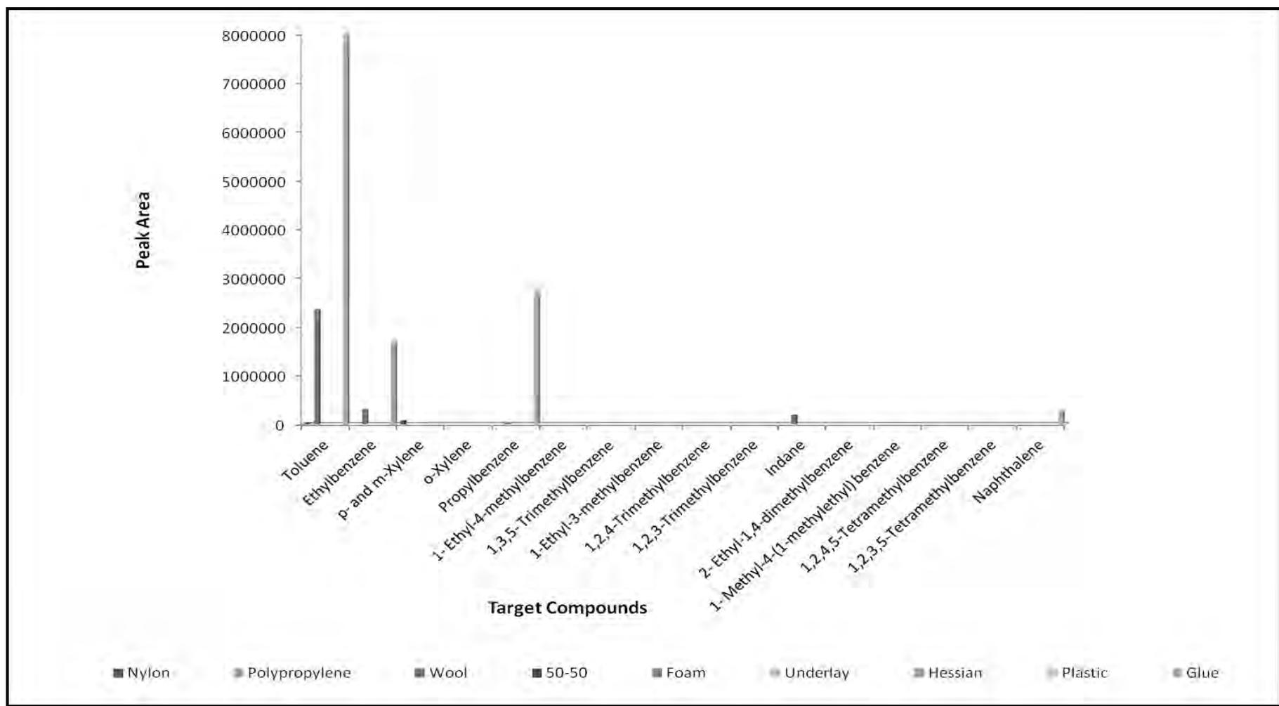
**Figure 4.66: Target Compound Chromatograms incorporating Carpet Fibres and Carpet Backing Components Pyrolysed at 450°C**
