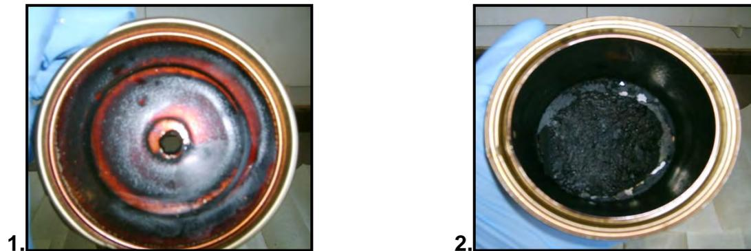
**Figure C1.14 (a): 1. Underside of Lid and 2. Sample in Bottom of Can after Burning**
