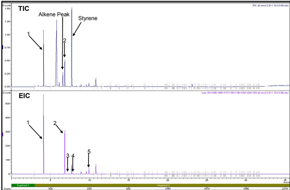
**Figure 4.46: Total Ion Chromatogram and Extracted Ion Chromatogram of a Wool Carpet Swatch burnt in a Can with Lid On for 2.5 minutes (Refer to Section 2.5.1 for GC/MS conditions)**
