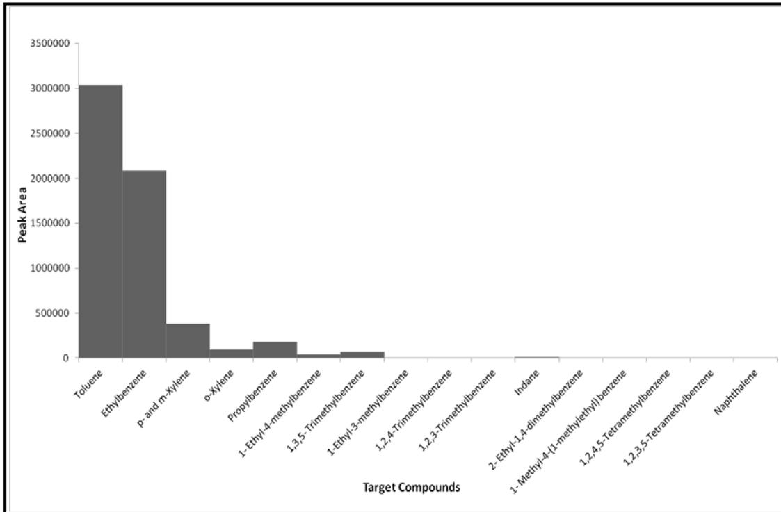
**Figure D2.12: Target Compound Chromatogram of a Wool Carpet Swatch burnt in a Can with Lid On for 10 minutes**
