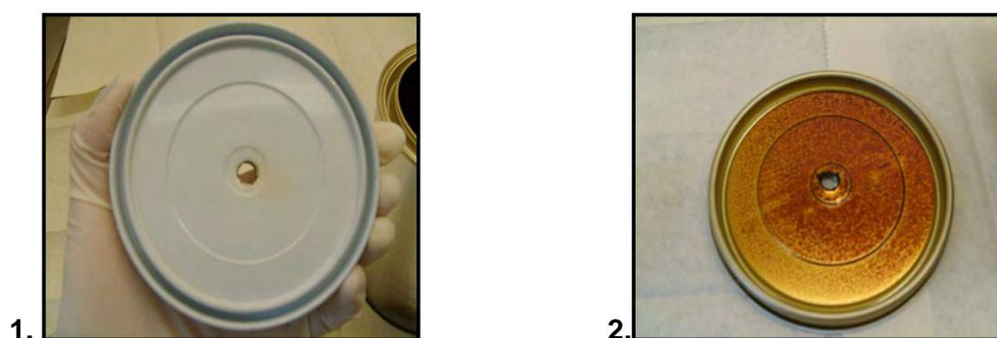
**Figure D2.1 (a): 1. Top and 2. Underside of Lid after Burning**
