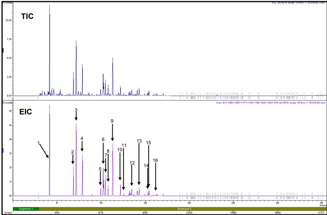
**Figure 3.6: Total Ion Chromatogram and Extracted Ion Chromatogram for 50% Evaporated Petrol Diluted to 10% (v/v) (Refer to Section 2.5.1 for GC/MS conditions)**
