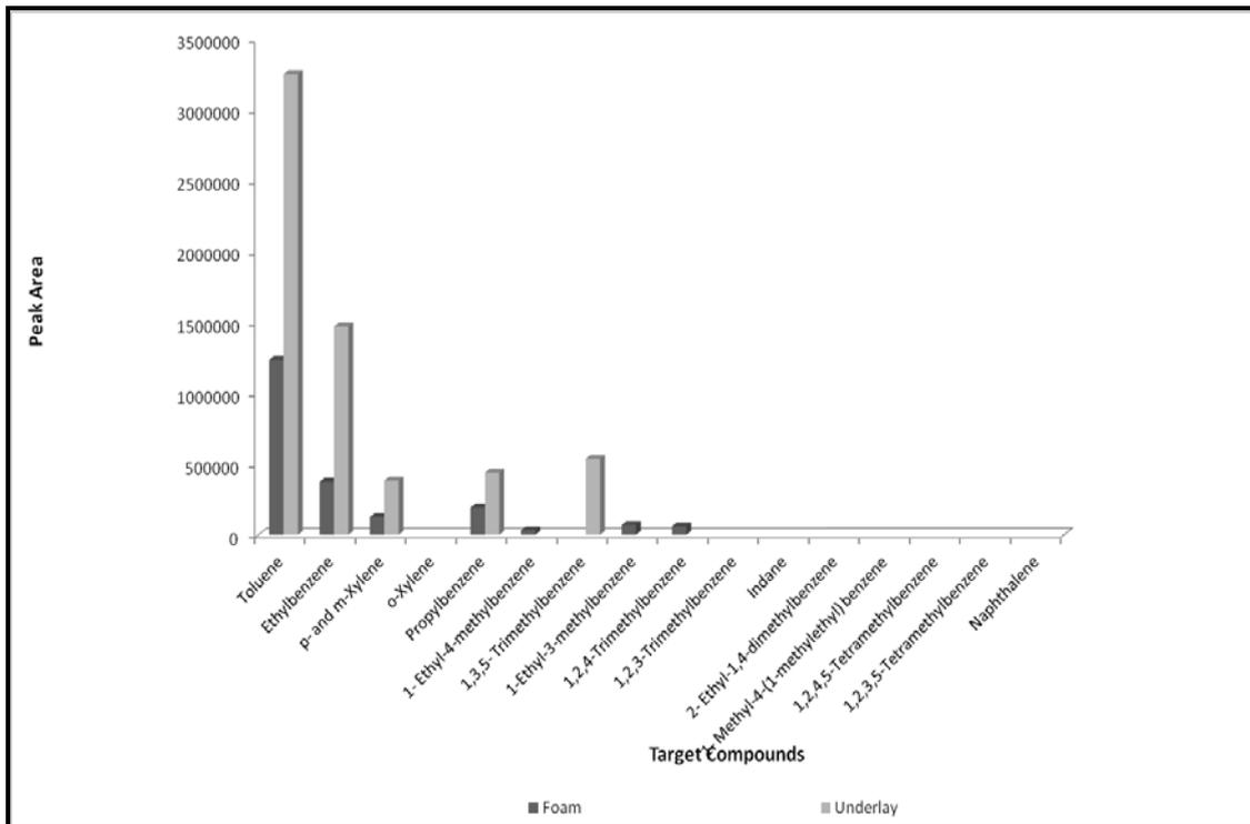
**Figures J1.20: Target Compound Chromatogram for Foam and Underlay pyrolysed at 600°C**
