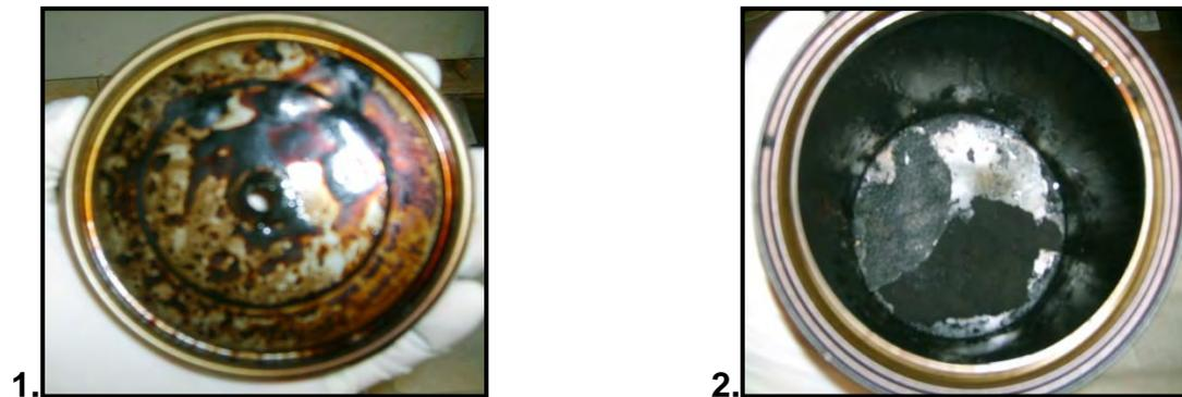
**Figure C1.26 (a): 1. Underside of Lid and 2. Sample in Bottom of Can after Burning**
