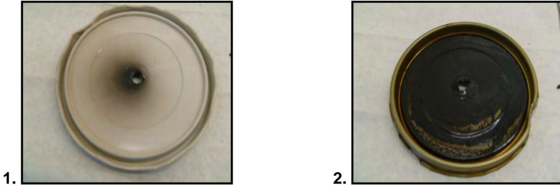
**Figure D2.10 (a): 1. Top of Lid and 2. Underside of Lid after Burning**
