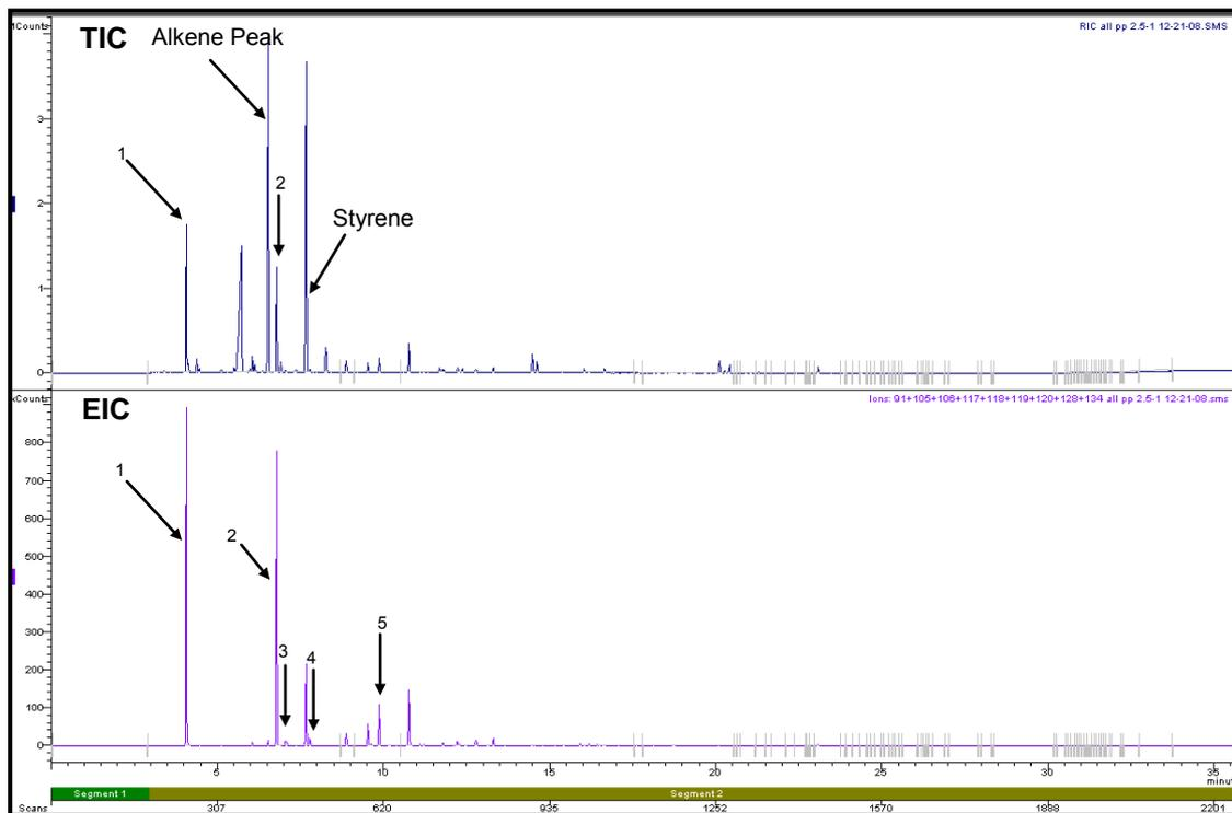
**Figure D1.2: Total Ion Chromatogram and Extracted Ion Chromatogram of a Polypropylene Carpet Swatch burnt in a Can with Lid On for 2.5 minutes**
