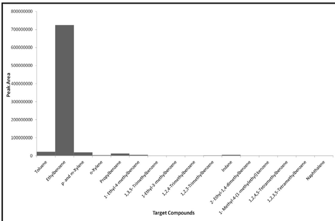
**Figure H4.4: Target Compound Chromatogram of Adhesive from Carpet Backing Pyrolysed at 750°C**
