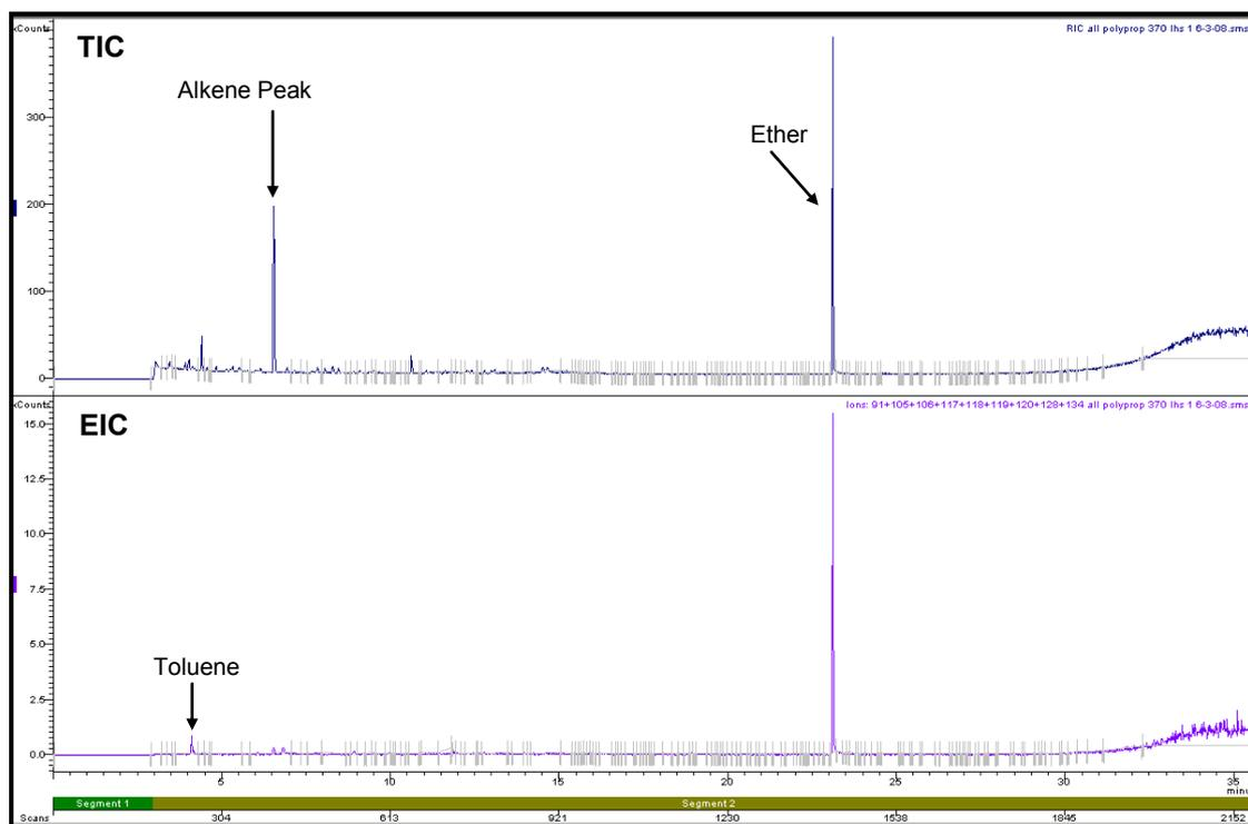
**Figure 4.23: Total Ion Chromatogram and Extracted Ion Chromatogram of the Left Side of the Polypropylene Carpet after Furnace Burn at 370°C (Refer to Section 2.5.1 for GC/MS conditions)**
