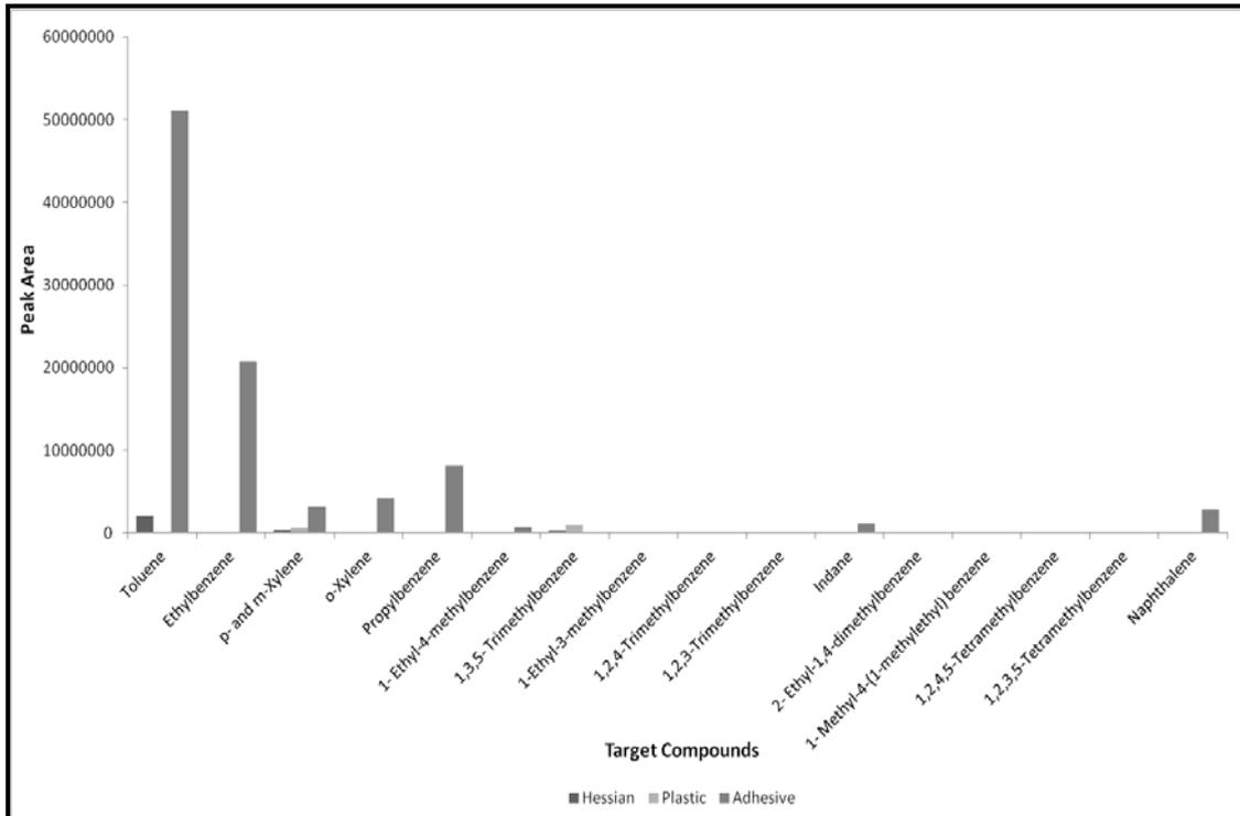
**Figures J1.16: Target Compound Chromatogram for Carpet Backing Components pyrolysed at 600°C**
