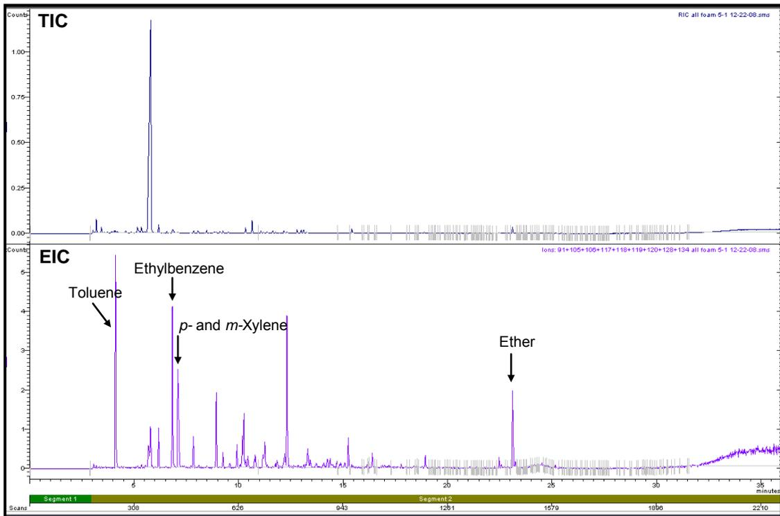
**Figure F1.4: Total Ion Chromatogram and Extracted Ion Chromatogram of Foam Burnt in a Can with Lid On for 5 minutes**
