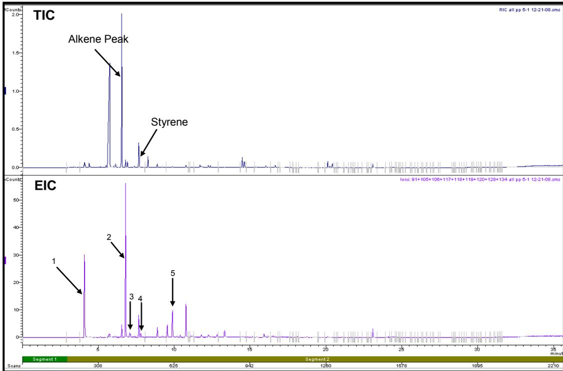
**Figure D1.5: Total Ion Chromatogram and Extracted Ion Chromatogram of a Polypropylene Carpet Swatch burnt in a Can with Lid On for 5 minutes**
