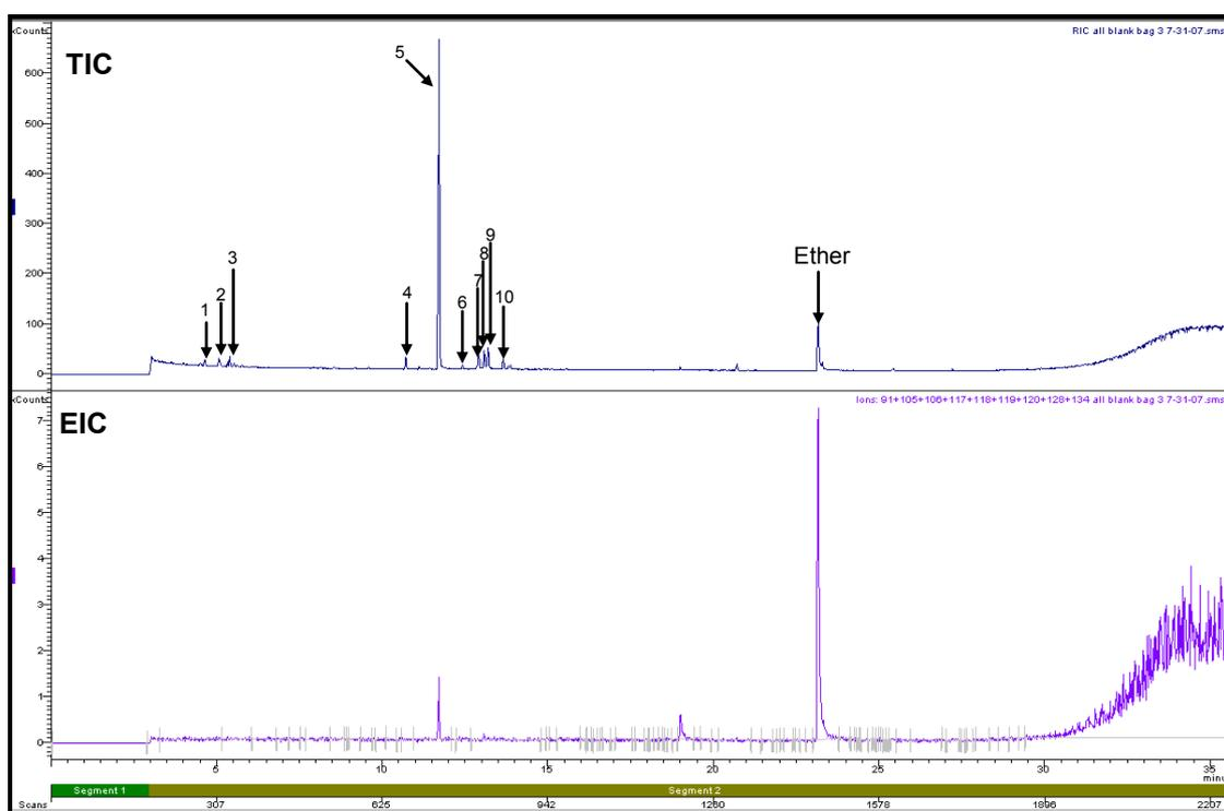
**Figure 3.34: Total Ion Chromatogram and Extracted Ion Chromatogram of Evidence Bag with Charcoal Tube (Refer to Section 2.5.1 for GC/MS conditions)**
