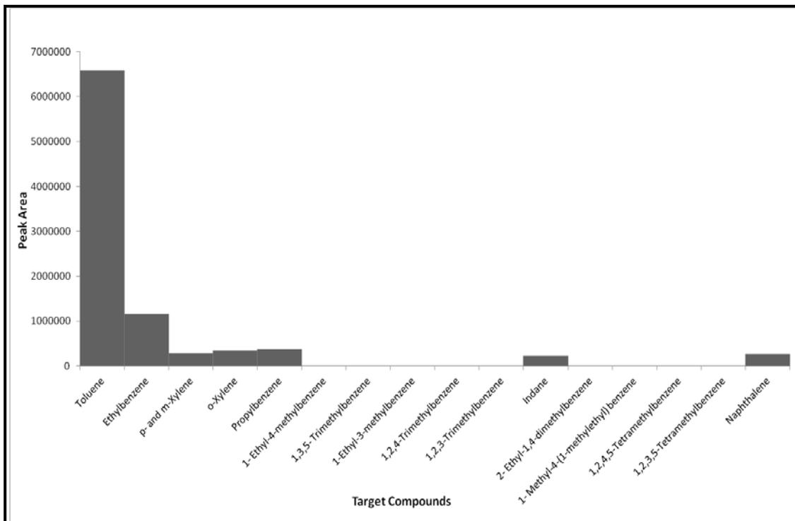
**Figure H6.6: Target Compound Chromatogram of Wool Fibres Pyrolysed at 600°C**
