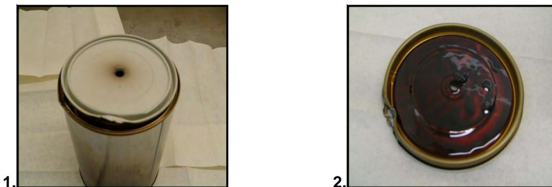
**Figure F1.3 (a): 1. Top and 2. Underside of Lid after Burning**
