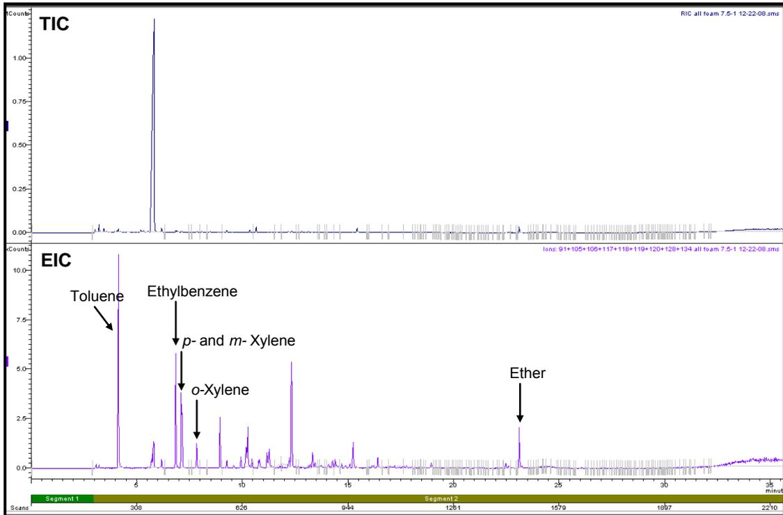
**Figure F1.7: Total Ion Chromatogram and Extracted Ion Chromatogram of Foam Burnt in a Can with Lid On for 7.5 minutes**
