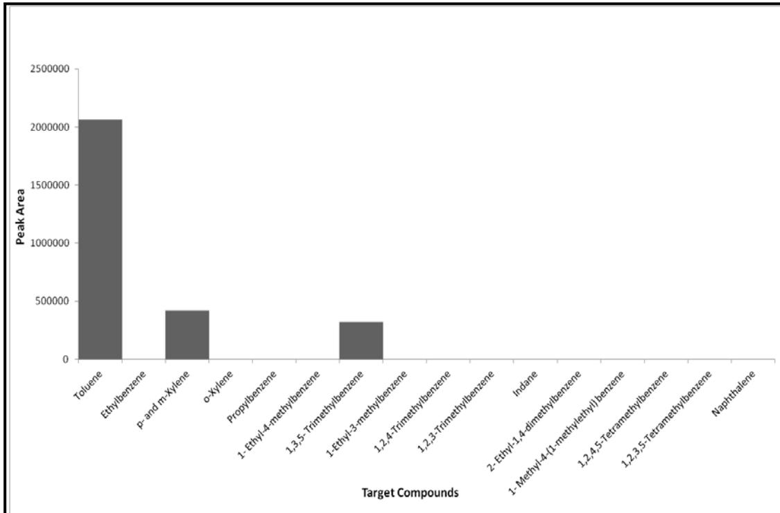
**Figure H2.6: Target Compound Chromatogram of Hessian Carpet Backing Pyrolysed at 600°C**
