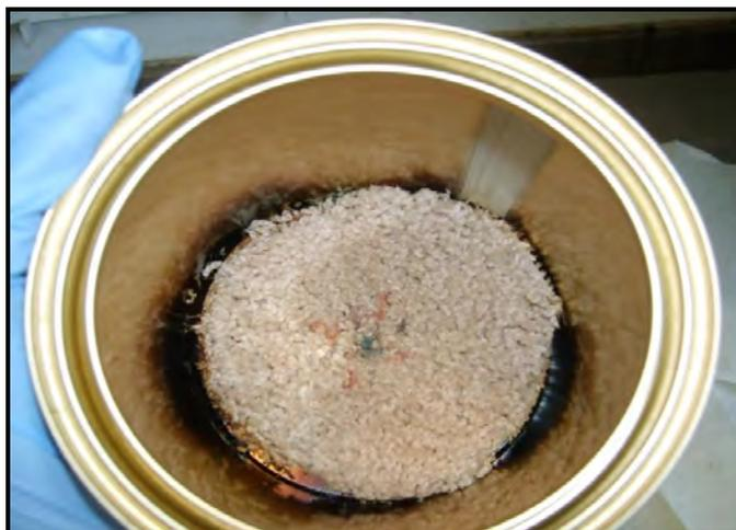
**Figure 4.29: Nylon Carpet Cut to Fit Flat in the Bottom of the Can**
