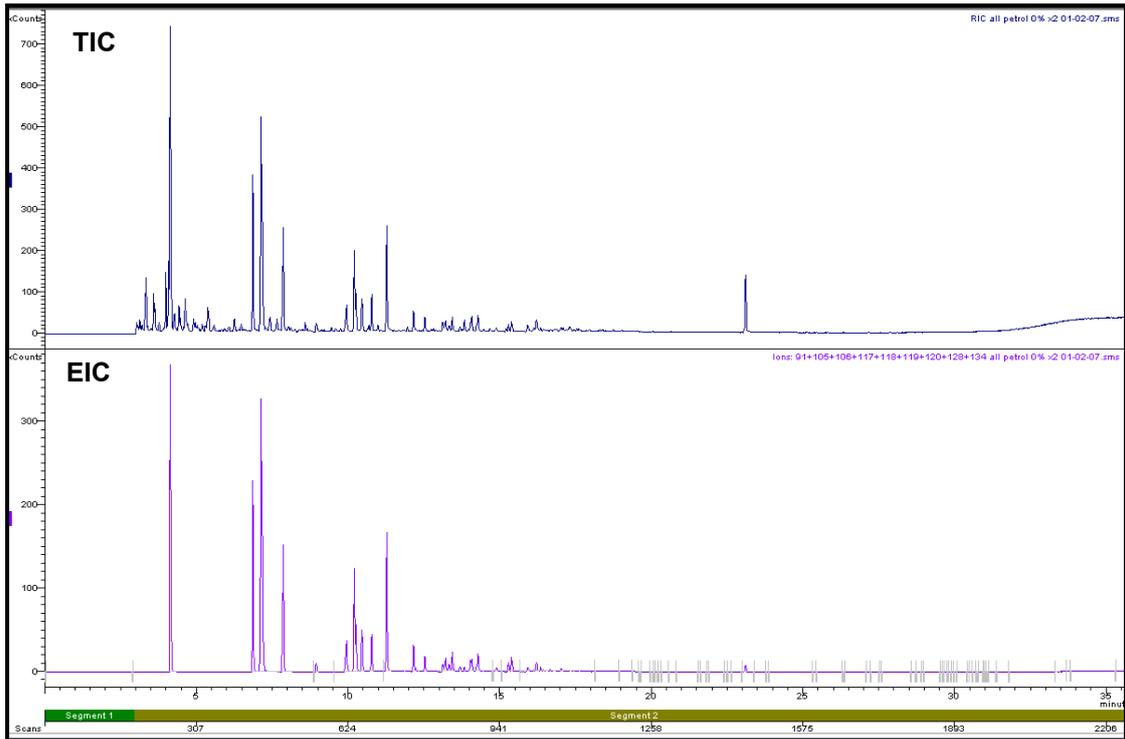
**Figure 1.7: Total Ion Chromatogram and Extracted Ion Chromatogram of Unleaded Petrol (Refer to Section 2.5.1 for GC/MS conditions)**
