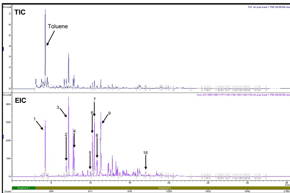
**Figure H3.3: Total Ion Chromatogram and Extracted Ion Chromatogram of Plastic Carpet Backing Pyrolysed at 750°C**
