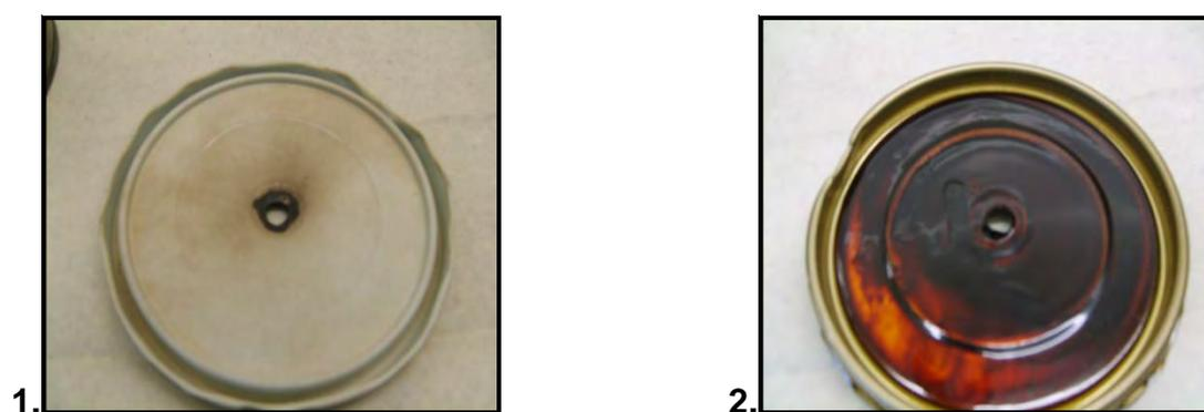
**Figure F2.1 (a): 1. Top and 2. Underside of Lid after Burning**
