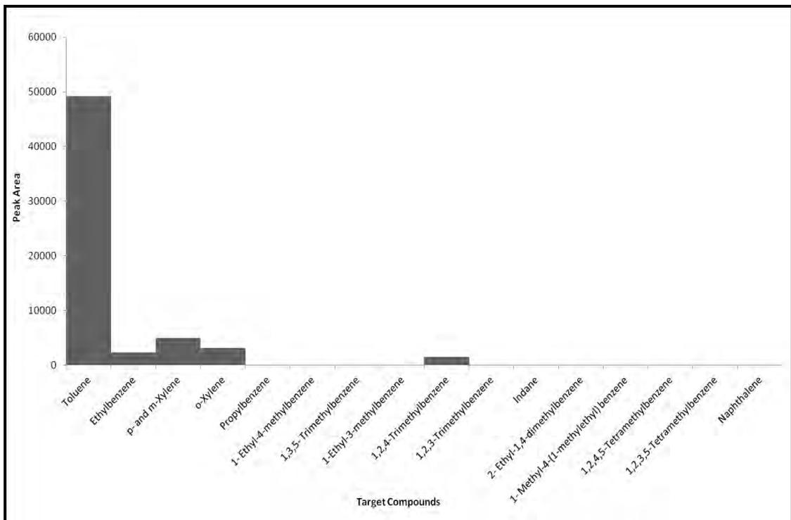
**Figure 3.31: Target Compound Chromatogram for 50% Evaporated Petrol Diluted to 0.001% (v/v)**
