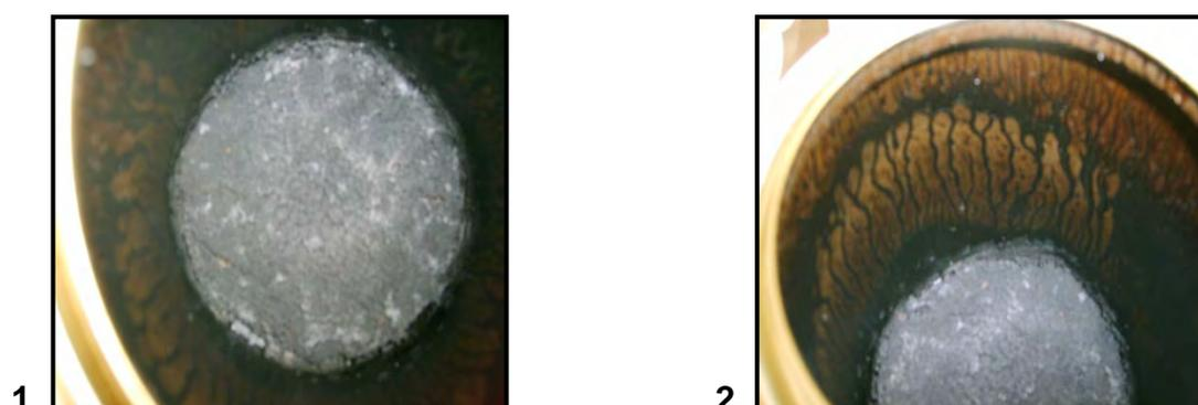
**Figure D2.4 (b): 1. Top of Sample and 2. Side of Can after Burning**
