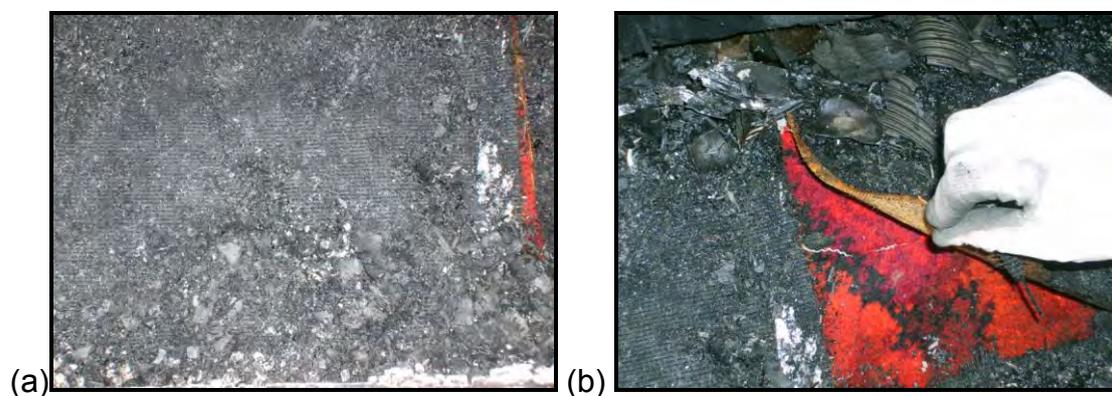
**Figure 3.86: (a) Top of Carpet and (b) Underneath the Carpet in the Area located away from the Petrol Spill after the Fire (where group C Thermocouples were located)**
