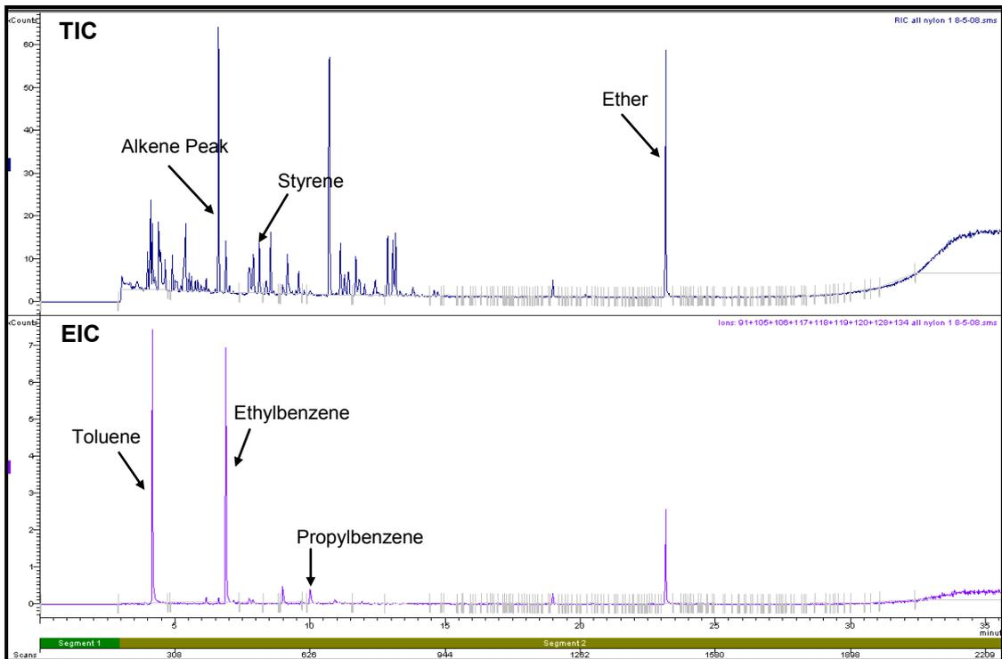
**Figure 4.38: Total Ion Chromatogram and Extracted Ion Chromatogram of Nylon Carpet (Refer to Section 2.5.1 for GC/MS conditions)**
