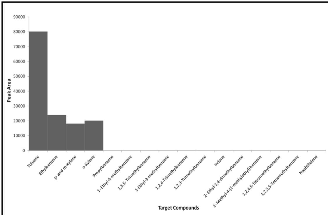
**Figure F1.11: Target Compound Chromatogram of Foam Burnt in a Can with Lid On for 10 minutes**
