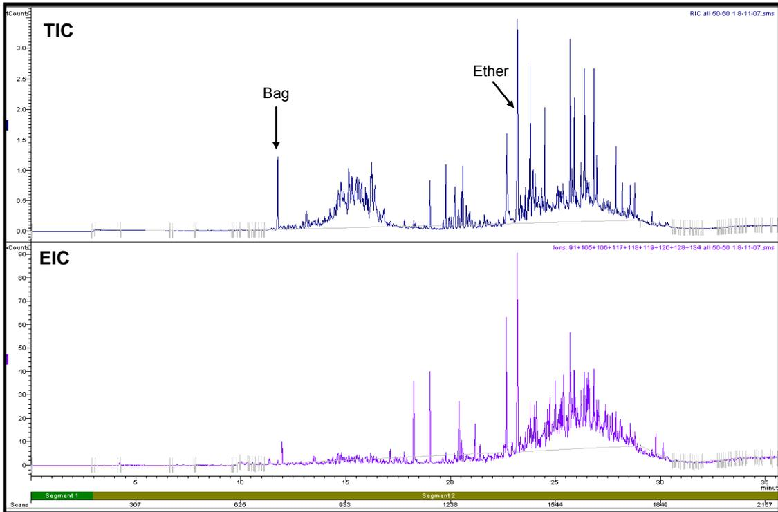
**Figure A1.2(d): Target Ion Chromatogram and Extracted Ion Chromatogram of 50-50 Polypropylene-Wool Carpet burnt in Room 1**
