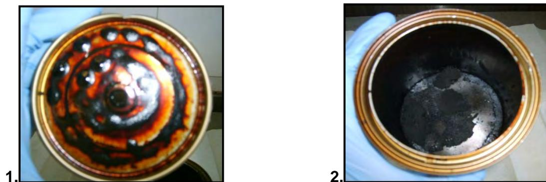
**Figure C1.23 (a): 1. Underside of Lid and 2. Sample in Bottom of Can after Burning**
