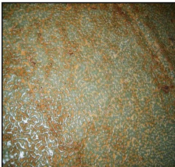
**Figure 4.16: Nylon Carpet after Furnace Burn at 383°C**
