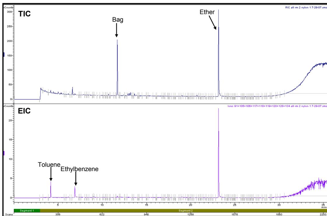
**Figure 4.13: Total Ion Chromatogram and Extracted Ion Chromatogram of Nylon Carpet burnt in Room 3 (Refer to Section 2.5.1 for GC/MS conditions)**
