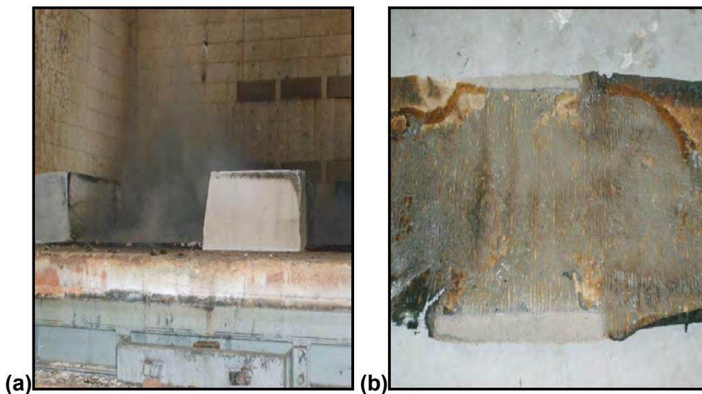
**Figure 4.21: Polypropylene Carpet after Furnace Burn at 370°C (a) When Doors were Opened (b) After Burning**
