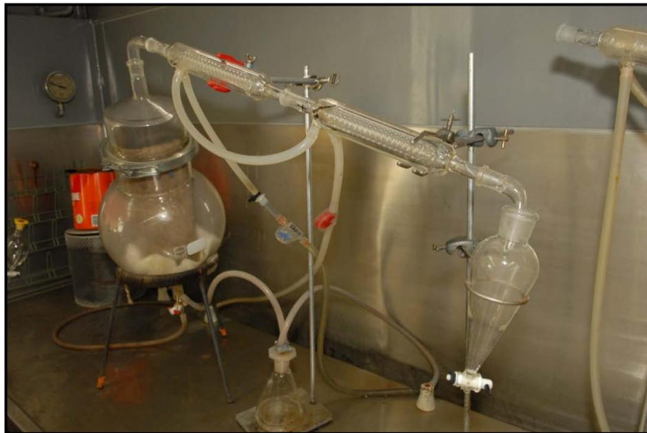
**Figure A1.1(c): Steam Distillation set up at VPFSC Laboratories with Sample of Burnt Nylon Carpet, During Distillation**
