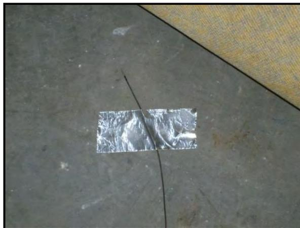
**Figure 3.69: Thermocouple placed on Concrete**
