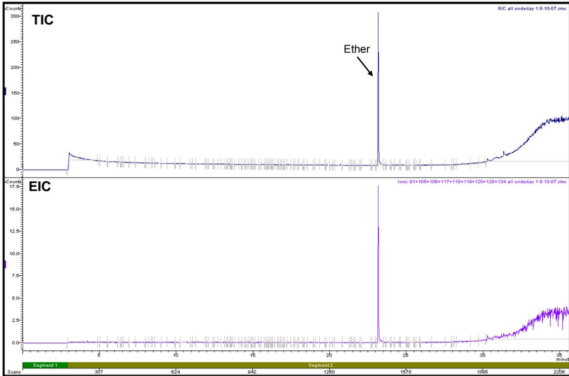
**Figure A1.2(e): Target Ion Chromatogram and Extracted Ion Chromatogram of Underlay burnt in Room 1**
