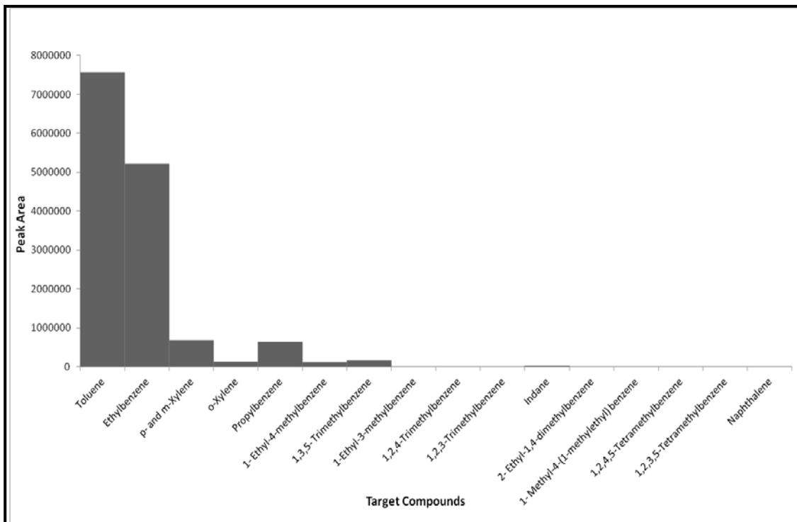
**Figure D2.6: Target Compound Chromatogram of a Wool Carpet Swatch burnt in a Can with Lid On for 5 minutes**
