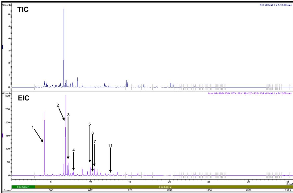
**Figure B1.3: Target Ion Chromatogram and Extracted Ion Chromatogram of Nylon (10cm x10cm swatch) burnt in a Can with Lid On**
