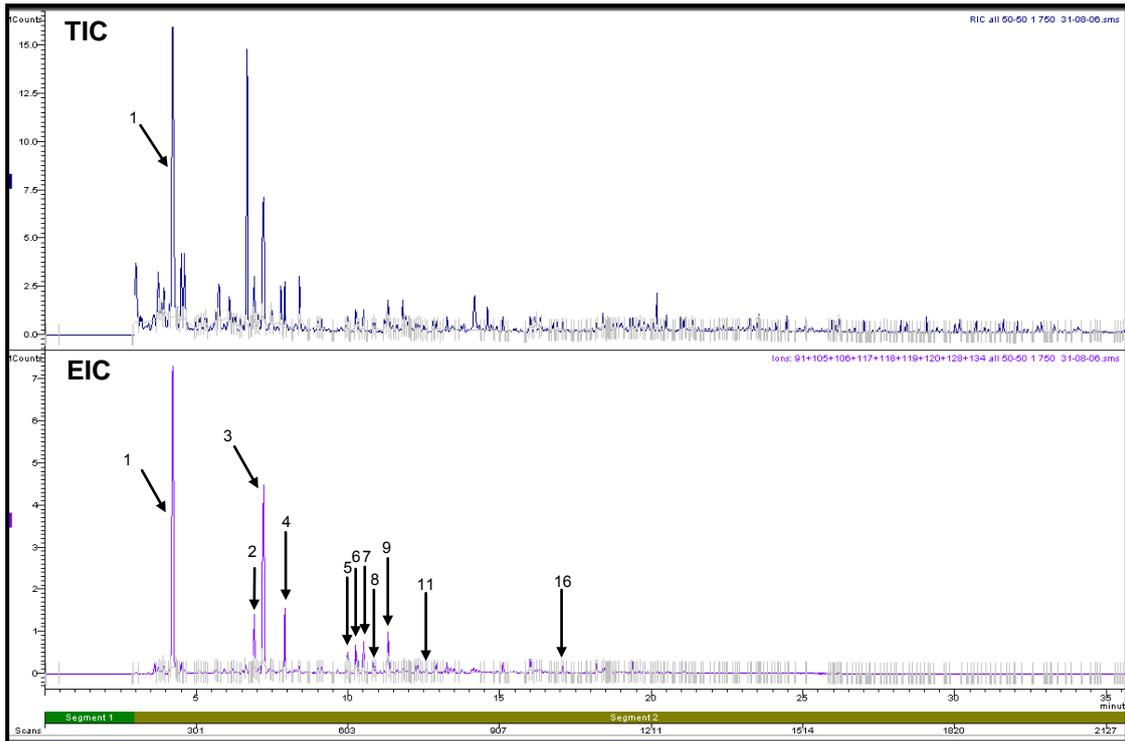
**Figure H7.3: Total Ion Chromatogram and Extracted Ion Chromatogram of 50-50 Polypropylene-Wool Fibres Pyrolysed at 750°C**
