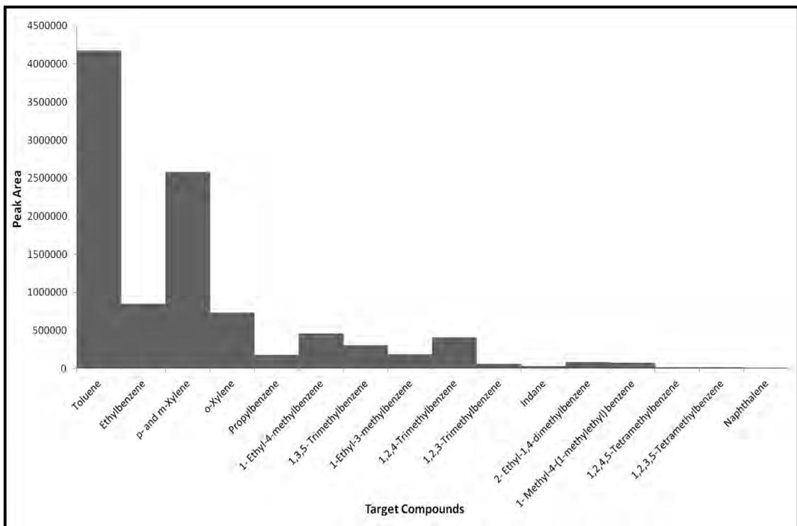
**Figure 3.39: Target Compound Chromatogram of KimWipe spiked with 100µL of 50% Evaporated Petrol**
