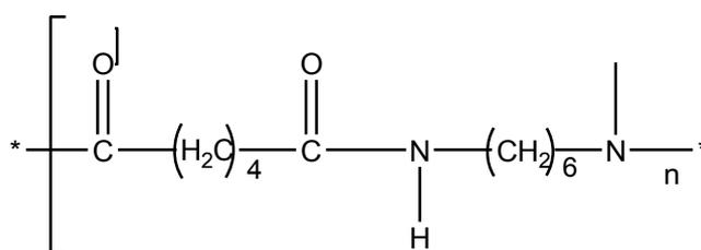
**Figure 3.55: Structure of Nylon 6,6**
