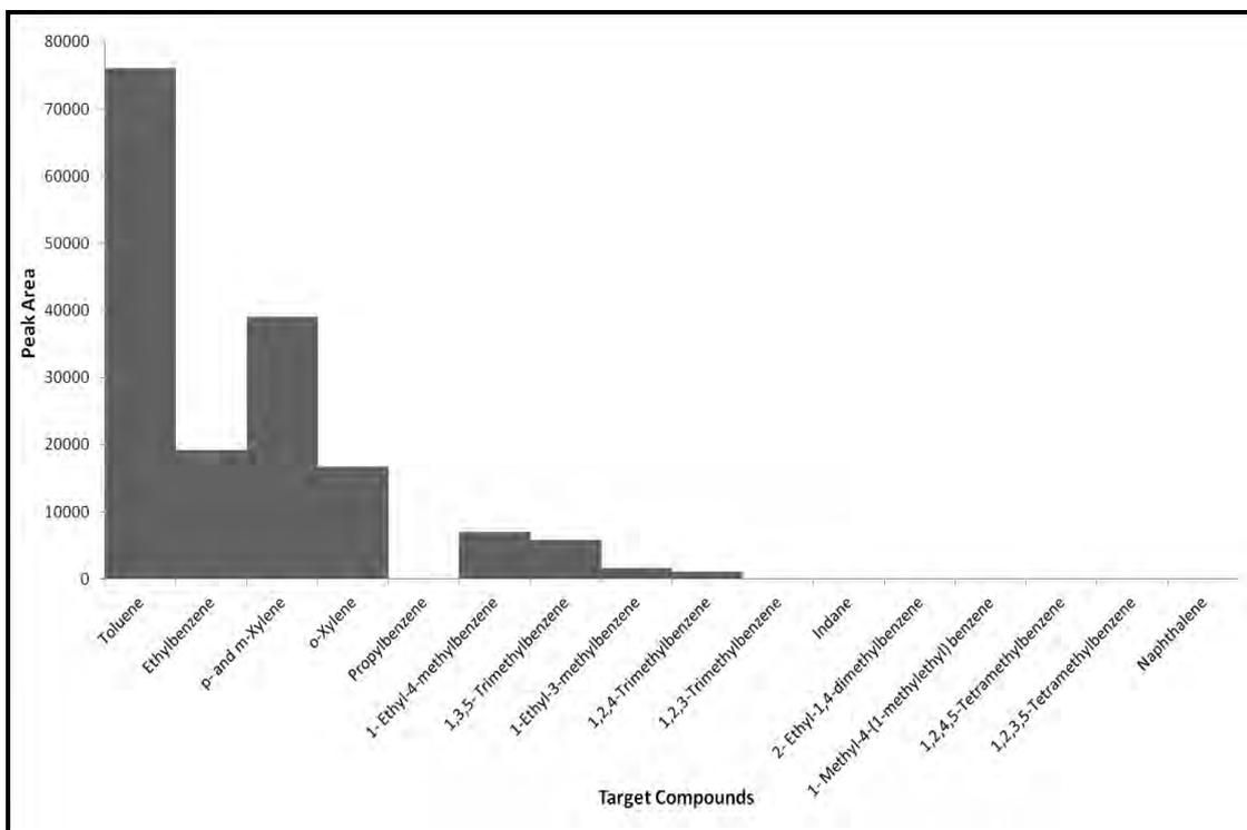
**Figure 4.9: Target Compound Chromatogram of KimWipe spiked with 2µL 50% Evaporated Petrol**
