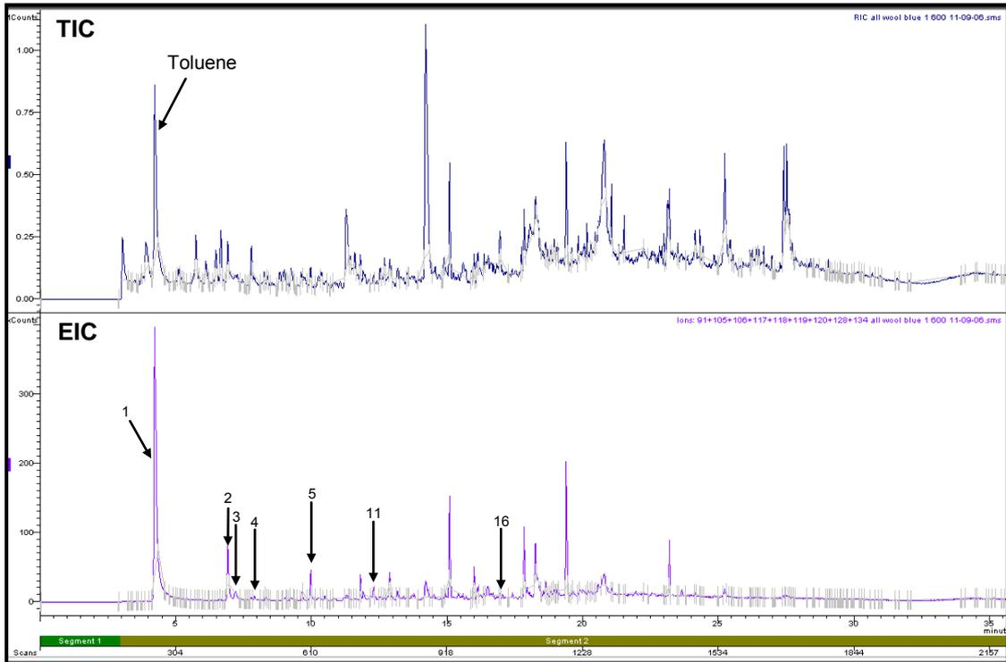
**Figure H6.5: Total Ion Chromatogram and Extracted Ion Chromatogram of Wool Fibres Pyrolysed at 600°C**
