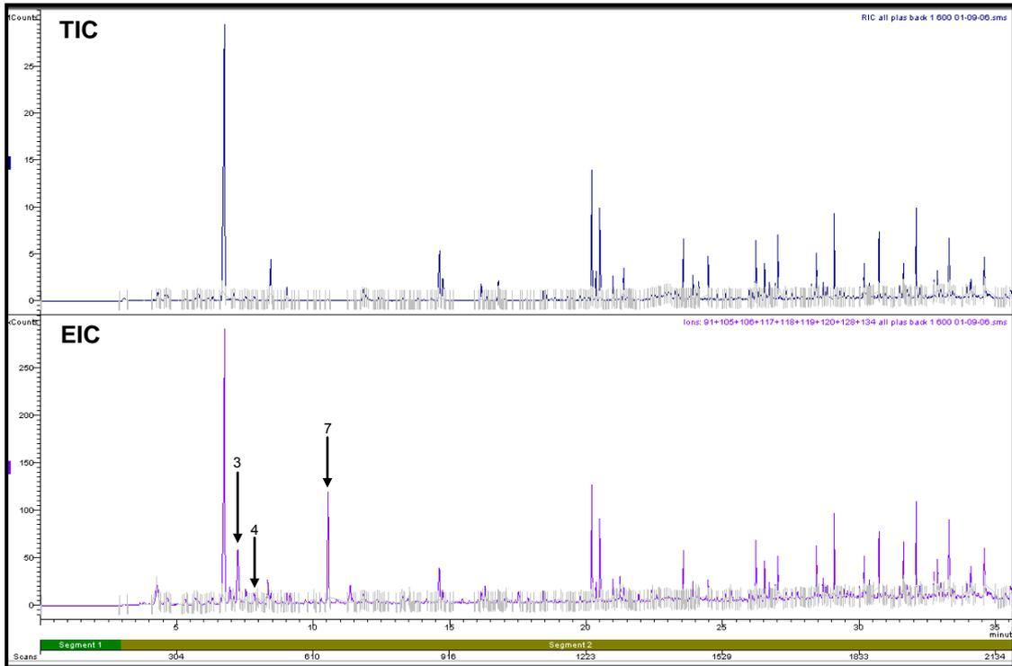
**Figure H3.5: Total Ion Chromatogram and Extracted Ion Chromatogram of Plastic Carpet Backing Pyrolysed at 600°C**
