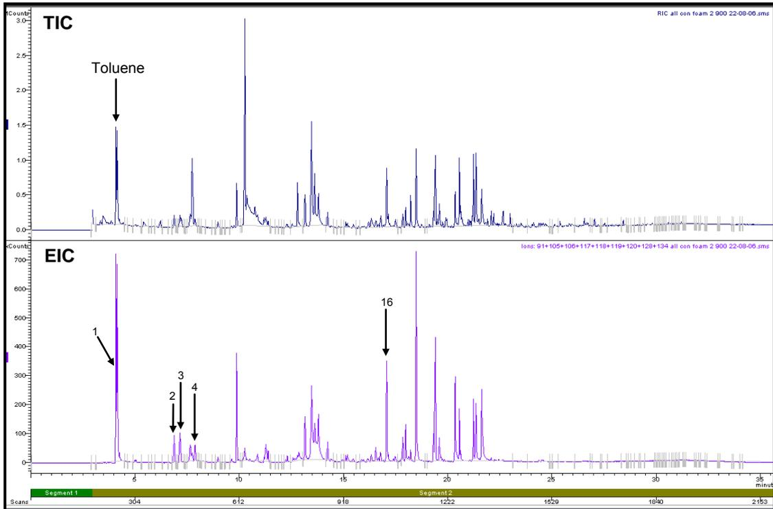
**Figure H8.1: Total Ion Chromatogram and Extracted Ion Chromatogram of Foam Pyrolysed at 900°C**
