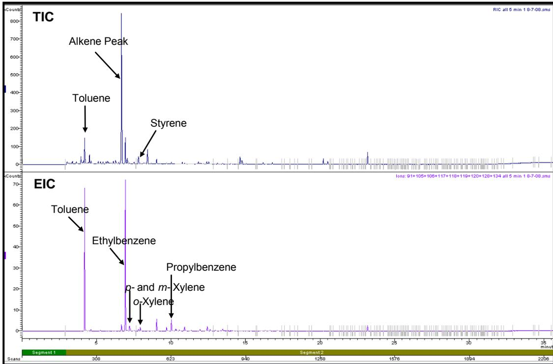
**Figure C1.24: Target Ion Chromatogram and Extracted Ion Chromatogram of a Nylon Carpet Swatch burnt in a Can with Lid On for 5 minutes**
