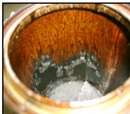
**Figure C1.26 (c): Inside of Can after Burning**
