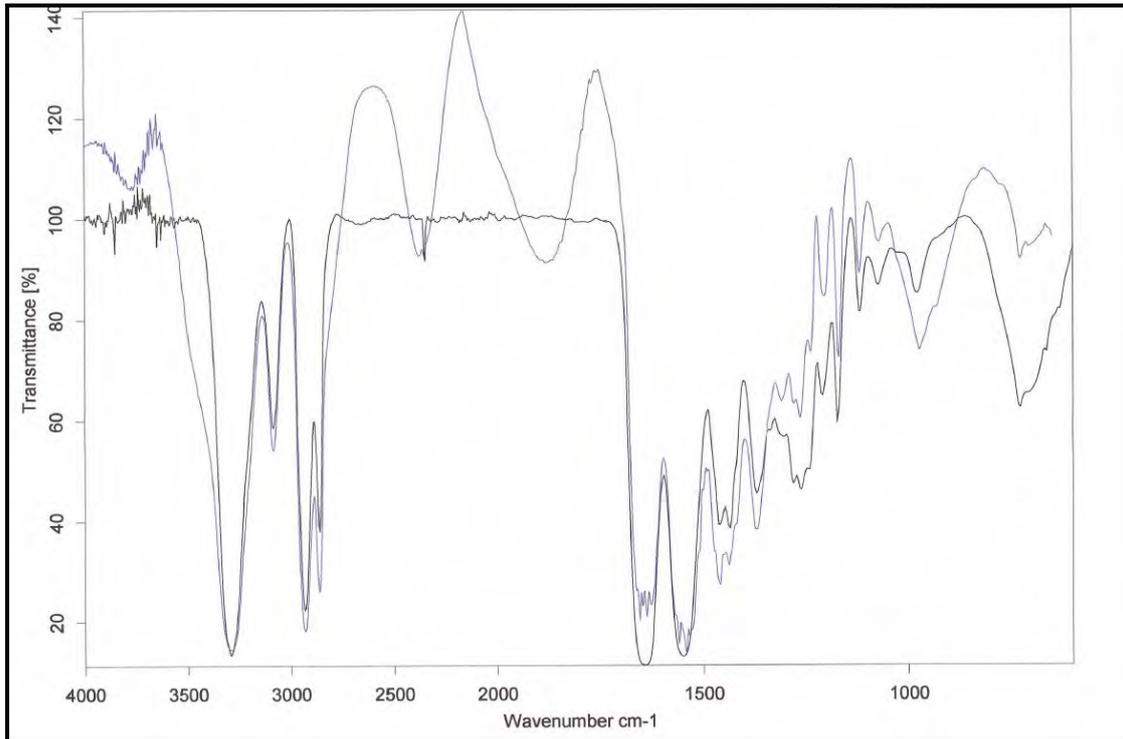
**Figure 3.58: FTIR Spectra of the 1 ply 100% Dyed Nylon Standard (dark blue) compared with Library Spectra of Nylon (black)**
