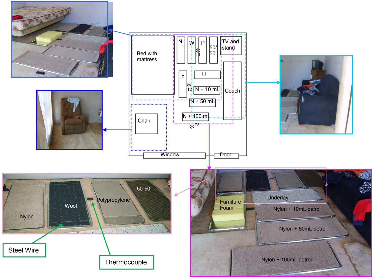
Figure 4.2: Layout of Room 1, with asterisk showing placement of the Thermocouples
