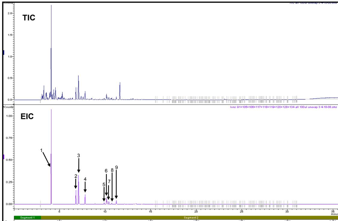
**Figure 3.36: Total Ion Chromatogram and Extracted Ion Chromatogram of KimWipe spiked with 100 $\mu$ L of Unevaporated Petrol (Refer to Section 2.5.1 for GC/MS conditions)**
