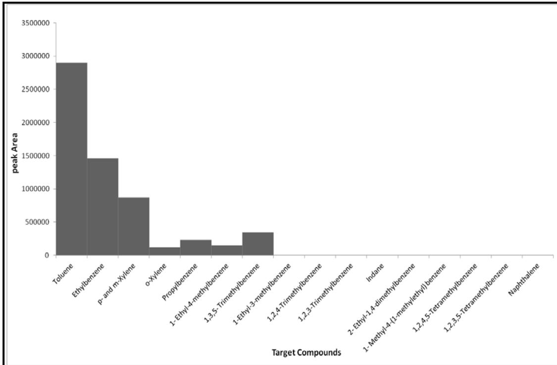
**Figure D3.6: Target Compound Chromatogram of a 50-50 Polypropylene-Wool Carpet Swatch burnt in a Can with Lid On for 2.5 minutes**
