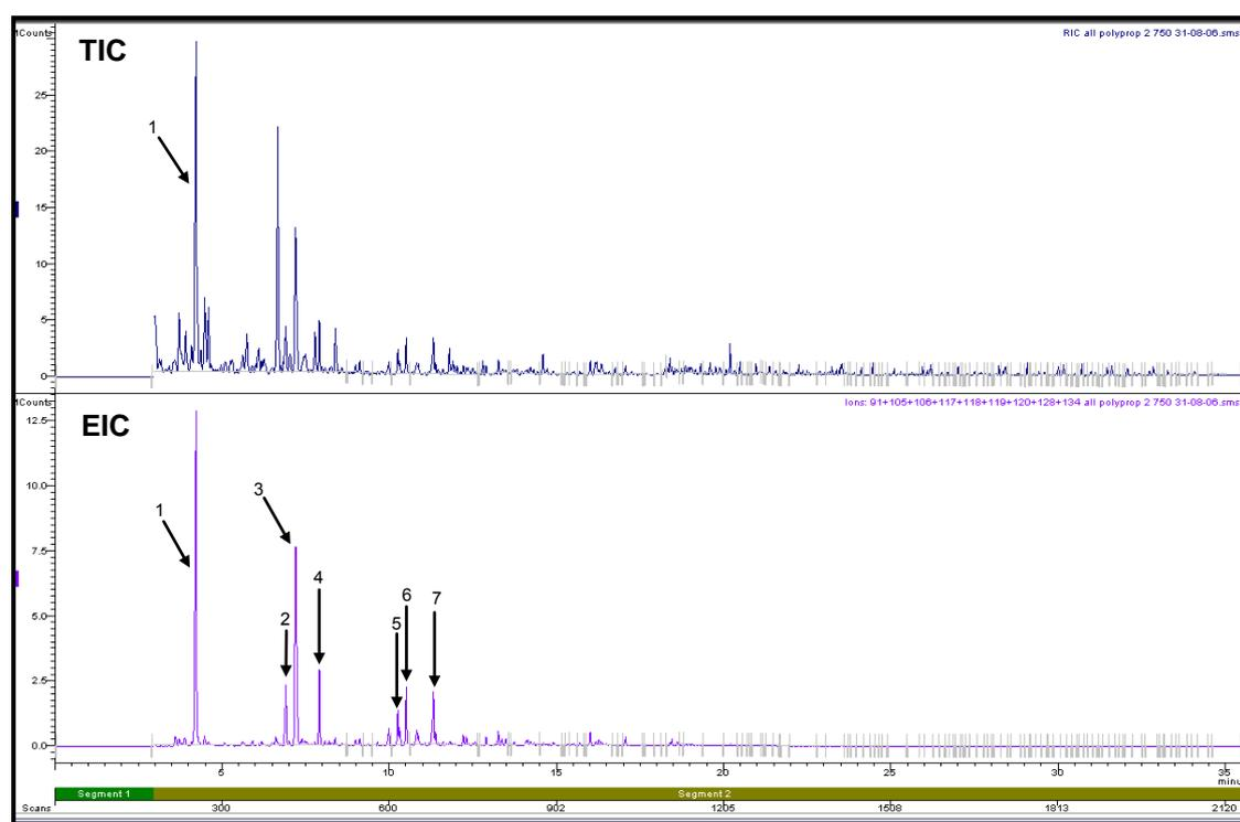
**Figure H5.3: Total Ion Chromatogram and Extracted Ion Chromatogram of Polypropylene Fibres Pyrolysed at 750°C**
