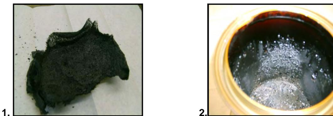
Figure F1.9 (b): 1. Sample after Burning 2. Inside of Can after Burning
