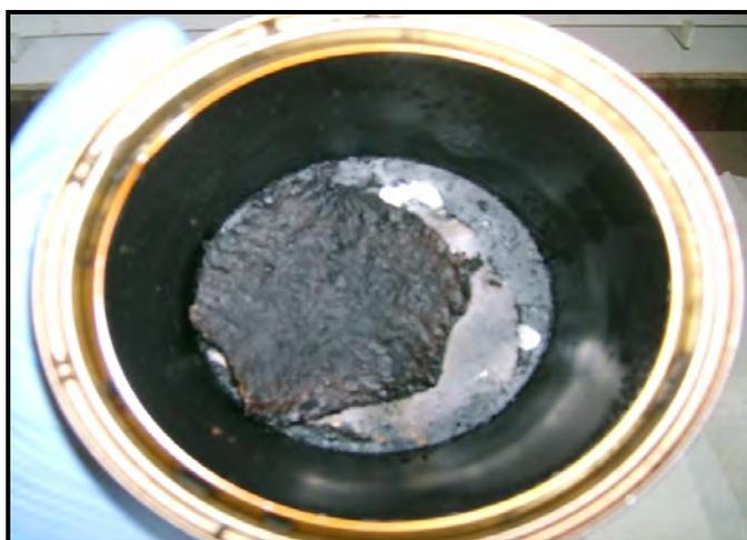
**Figure 4.30: Nylon Carpet after Burning for approximately 2 minutes**
