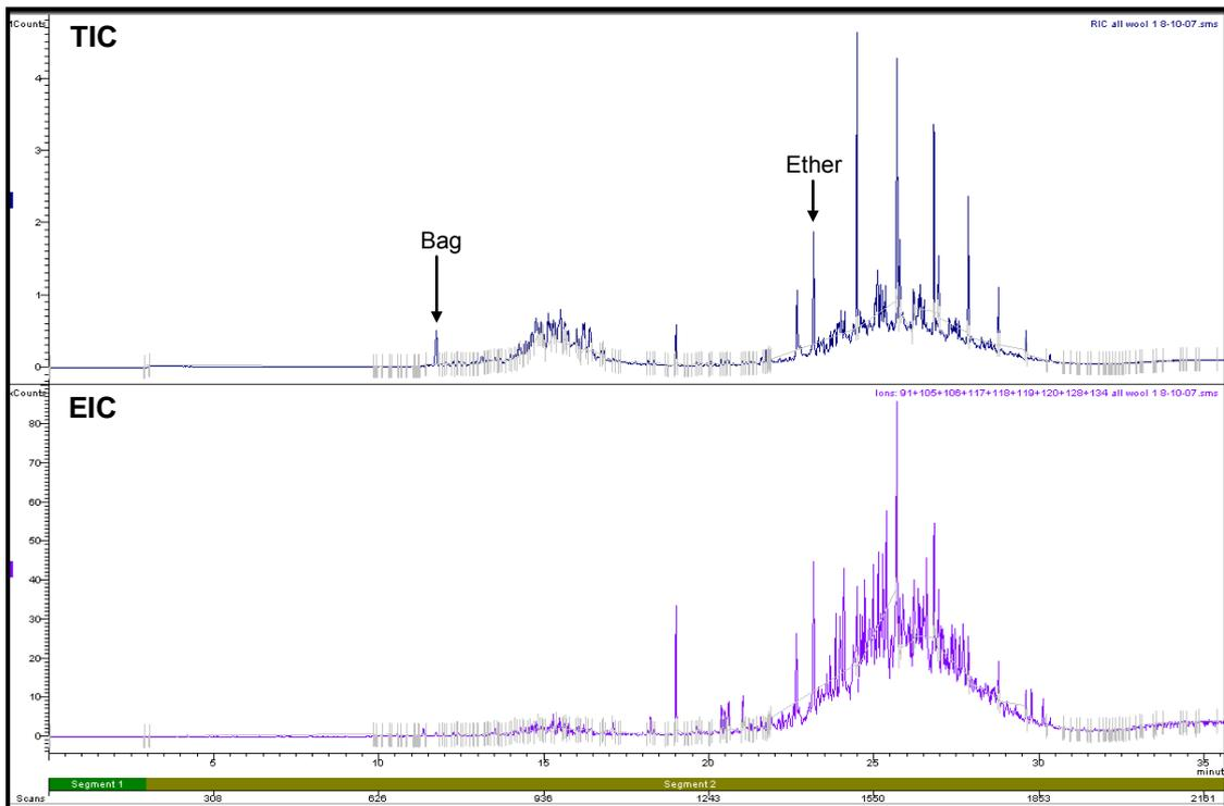
**Figure A1.2(c): Target Ion Chromatogram and Extracted Ion Chromatogram of Wool Carpet burnt in Room 1**
