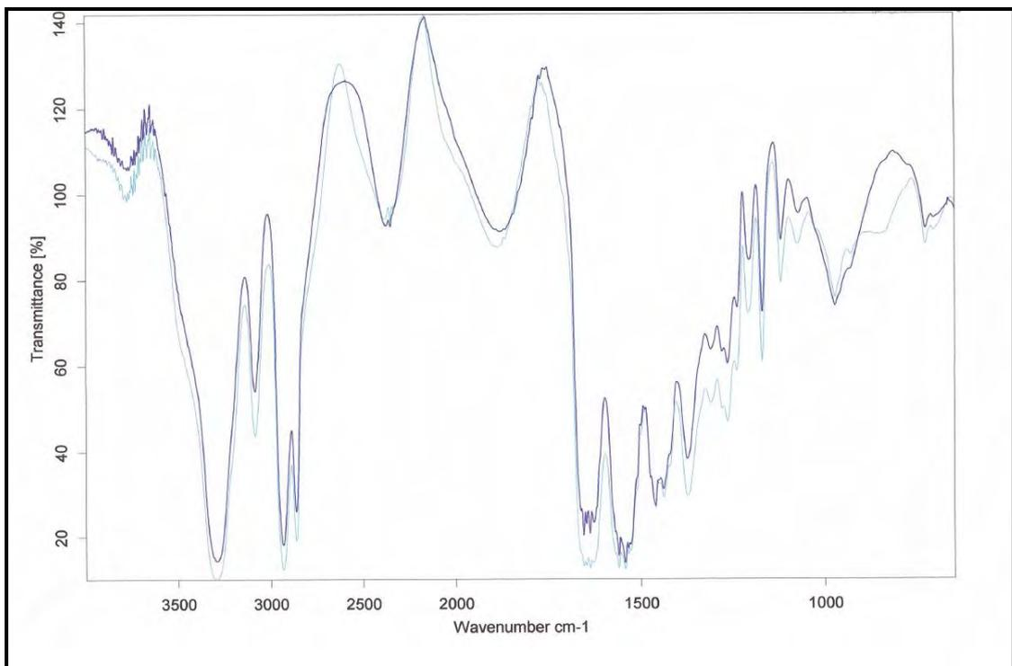
**Figure 3.57: FTIR Spectra of 1 ply 100% Dyed Nylon Standard (dark blue) compared with 2 ply 100% Dyed Nylon Standard (light blue)**
