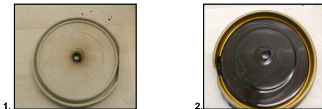
**Figure F2.6 (a): 1. Top and 2. Underside of Lid after Burning**
