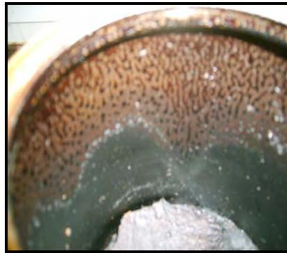
**Figure C1.11(c): Inside of Can after Burning**
