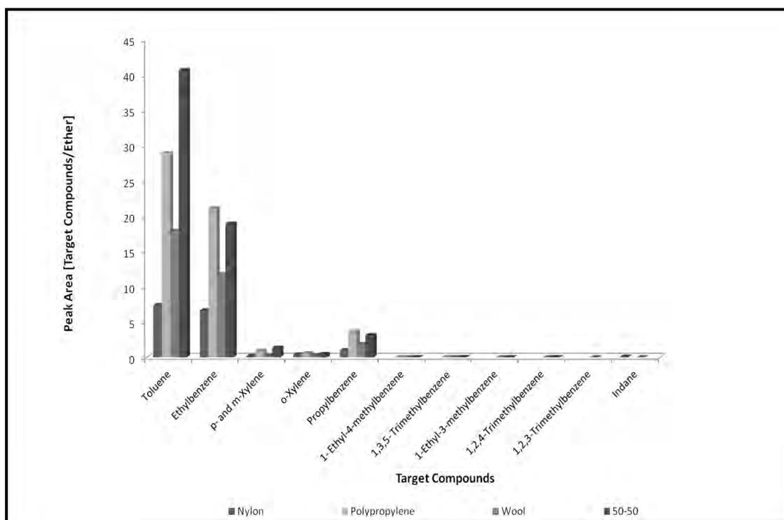
**Figure 4.54: Target Compound Chromatogram for all Carpets when Burnt in the Small Can with Lid On for 2.5 minutes**
