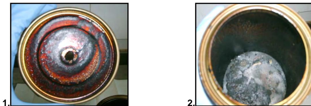
**Figure C1.17 (a): 1. Underside of Lid and 2. Sample in Bottom of Can after Burning**
