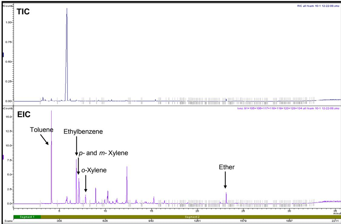
**Figure F1.10: Total Ion Chromatogram and Extracted Ion Chromatogram of Foam Burnt in a Can with Lid On for 10 minutes**
