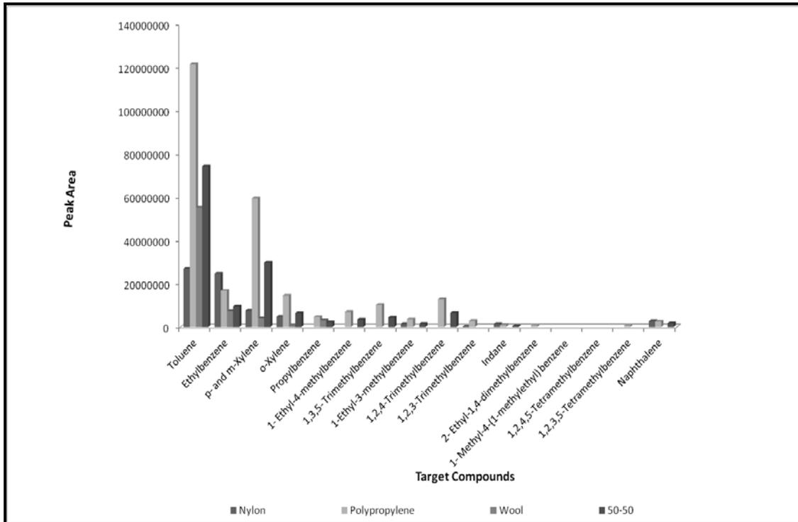
Figures J1.11: Target Compound Chromatogram for all Carpet Fibres pyrolysed at 750°C
