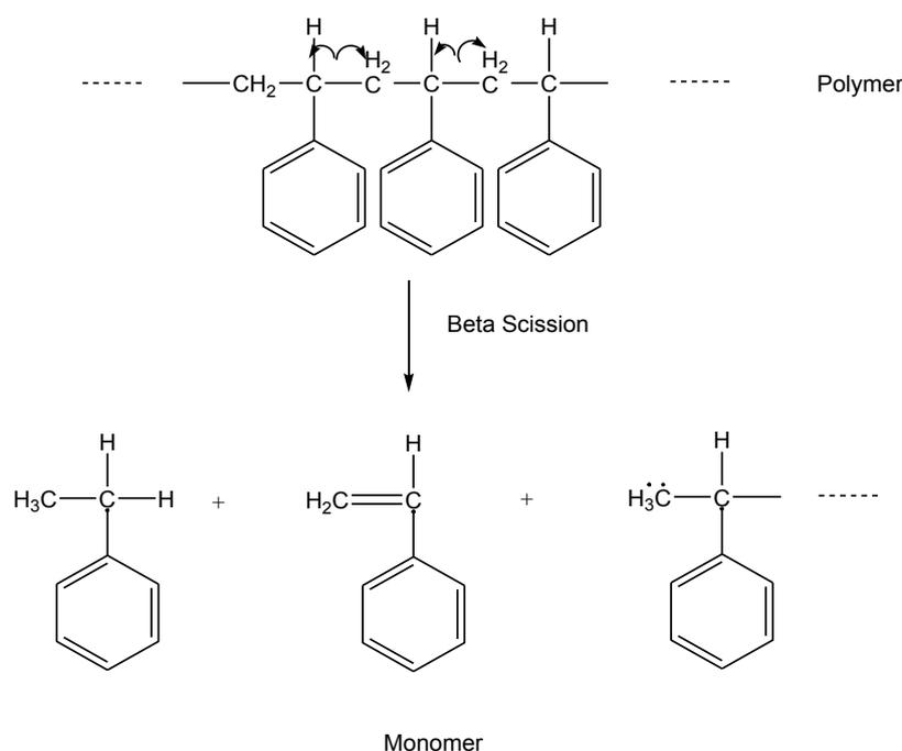
**Figure 1.12: Monomer Reversion of Polystyrene**
