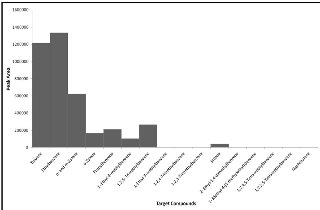
**Figure B1.4: Target Compound Chromatogram of Nylon (10cm x10cm swatch) burnt in a Can with Lid On**
