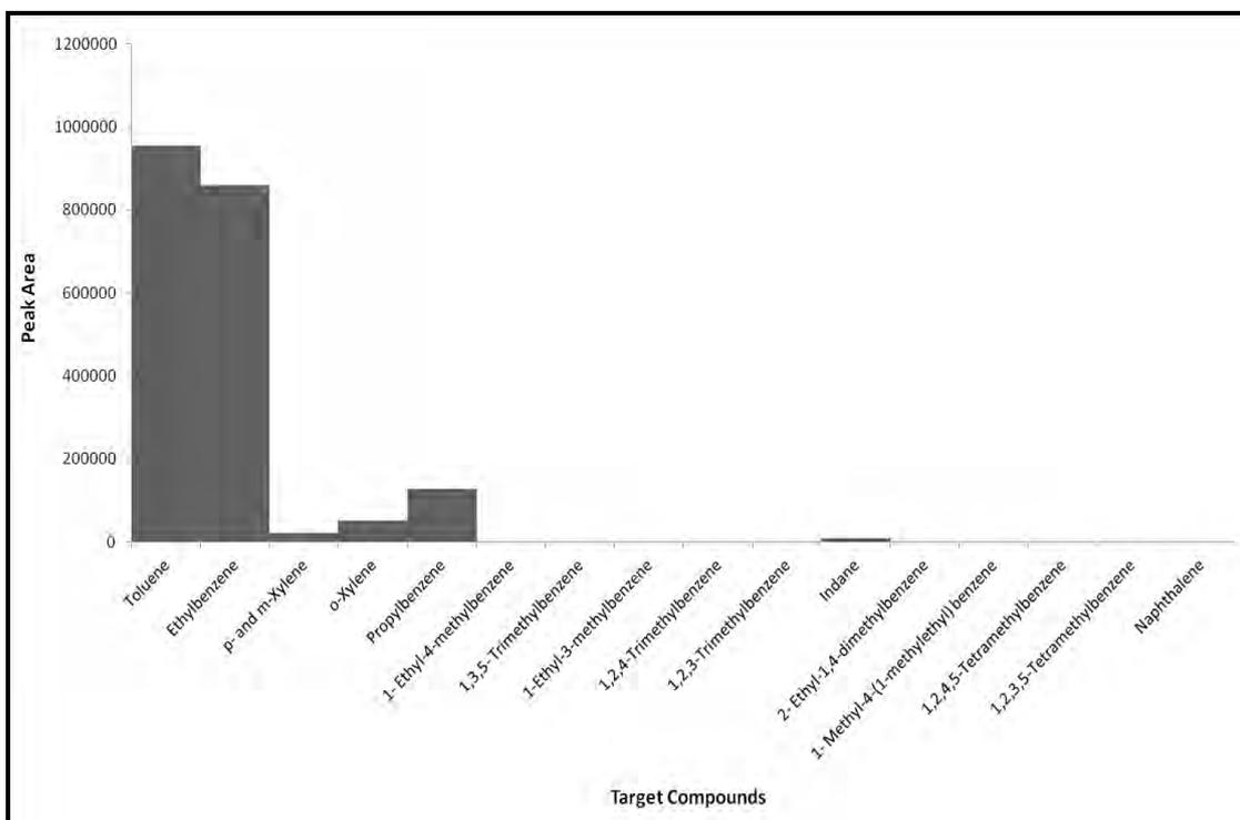
**Figure 4.43: Target Compound Chromatogram of a Nylon Carpet swatch burnt in a Can with Lid On for 2.5 minutes**
