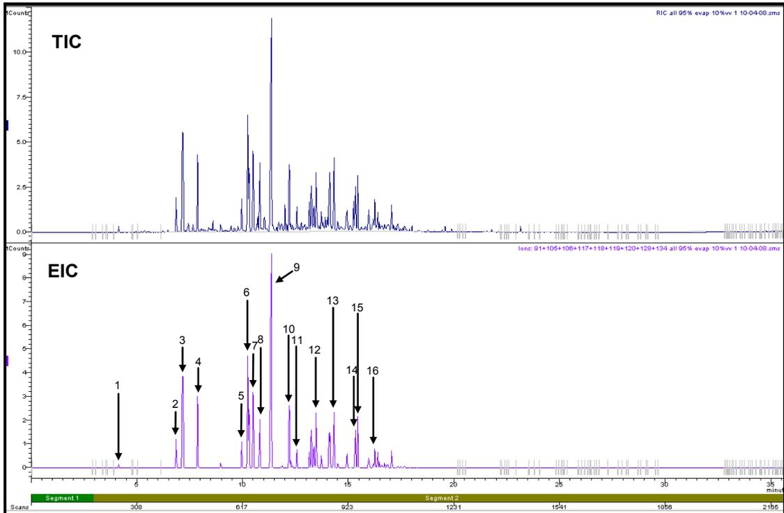
**Figure 3.8: Total Ion Chromatogram and Extracted Ion Chromatogram for 95% Evaporated Petrol Diluted to 10% (v/v) (Refer to Section 2.5.1 for GC/MS conditions)**
