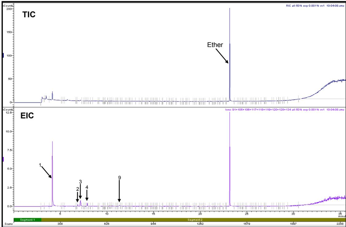
**Figure 3.30: Total Ion Chromatogram and Extracted Ion Chromatogram for 50% Evaporated Petrol Diluted to 0.001% (v/v) (Refer to Section 2.5.1 for GC/MS conditions)**
