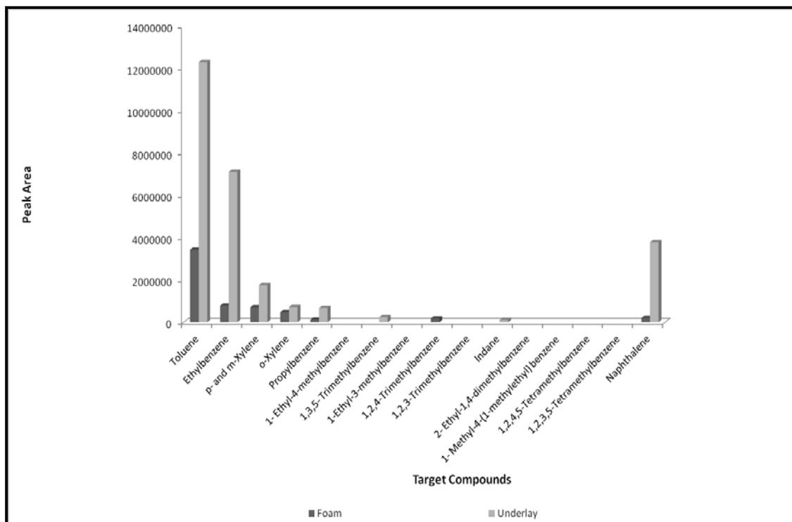
**Figures J1.19: Target Compound Chromatogram for Foam and Underlay pyrolysed at 750°C**
