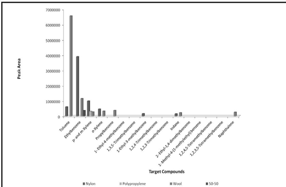
Figures J1.12: Target Compound Chromatogram for all Carpet Fibres pyrolysed at 600°C
