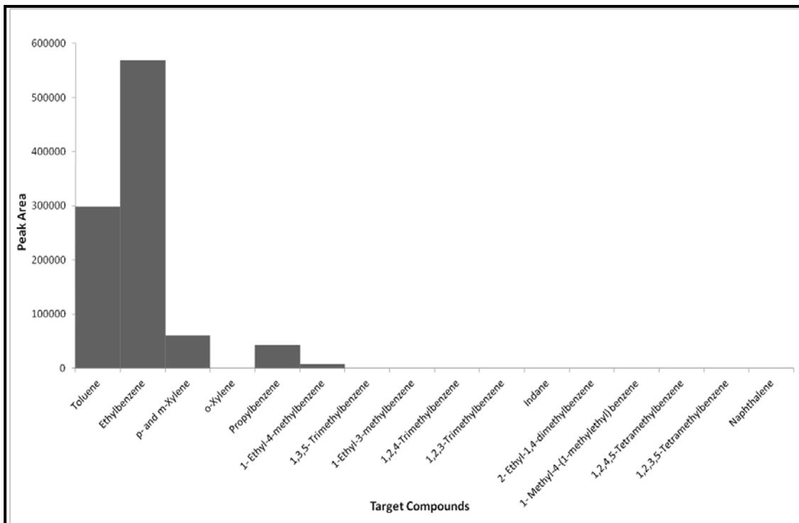
**Figure F2.3: Target Compound Chromatogram of Underlay Burnt in a Can with Lid On for 2.5 minutes**
