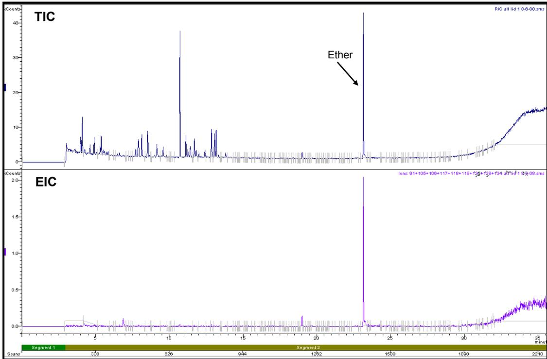
**Figure 4.37: Total Ion Chromatogram and Extracted Ion Chromatogram of the Lid (Refer to Section 2.5.1 for GC/MS conditions)**
