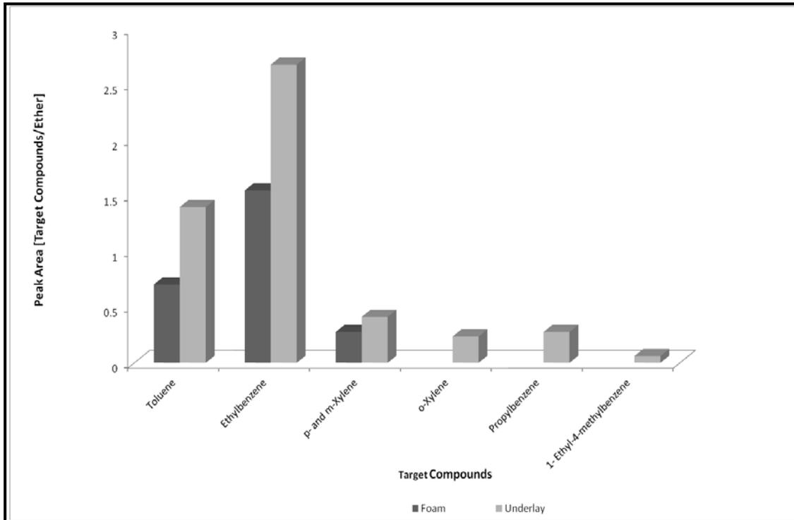
**Figure G1.2: Target Compound Chromatogram for Foam and Underlay when Burnt in the Small Can with Lid On for 5 minutes**
