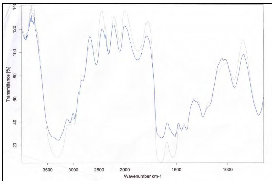
**Figure 3.60: FTIR Spectra of Wool Standard (grey) compared with Wool Carpet Fibres (blue)**
