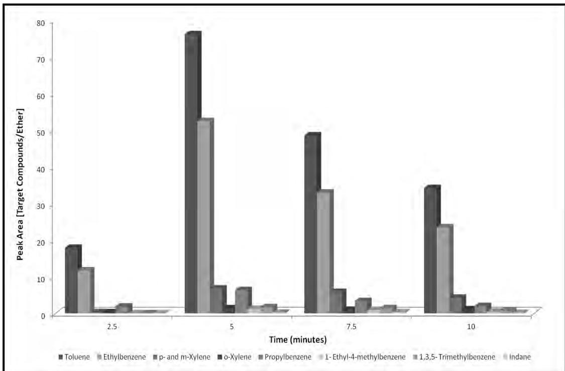
**Figure 4.52: Graph of Peak Area of Target Compounds with Butylated Hydroxytoluene vs. Burn Time for Wool Carpet**
