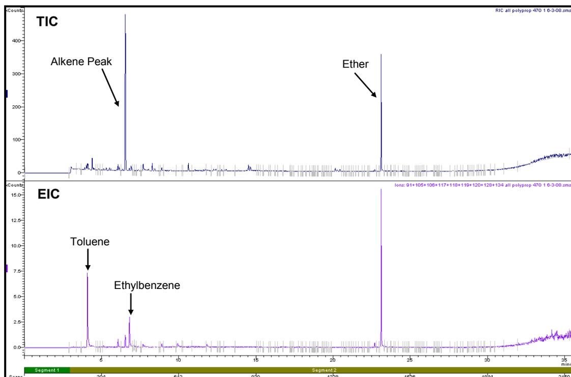
**Figure 4.22: Total Ion Chromatogram and Extracted Ion Chromatogram of the Polypropylene Carpet after Furnace Burn at 470°C (Refer to Section 2.5.1 for GC/MS conditions)**
