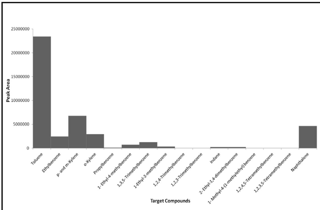
**Figure H3.2: Target Compound Chromatogram of Plastic Carpet Backing Pyrolysed at 900°C**
