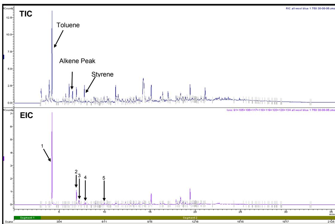
**Figure H6.3: Total Ion Chromatogram and Extracted Ion Chromatogram of Wool Fibres Pyrolysed at 750°C**
