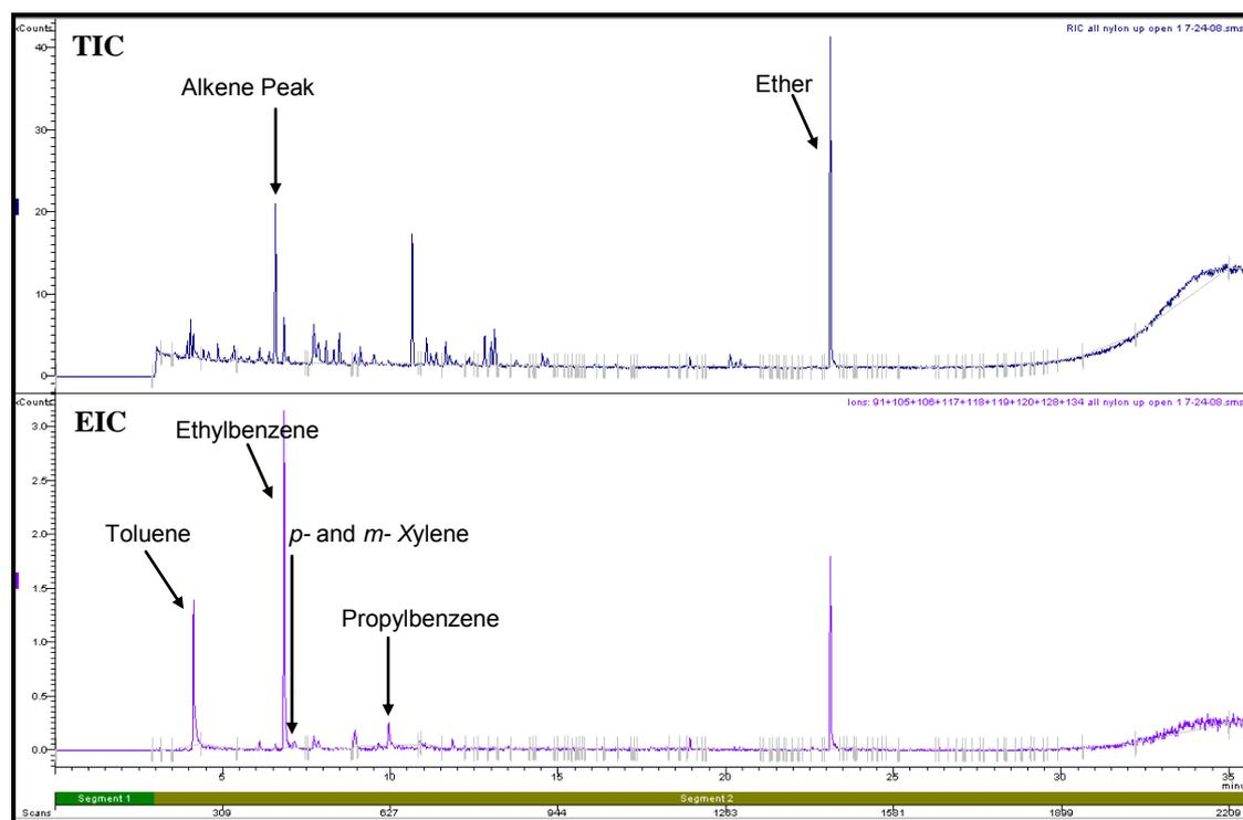
**Figure 4.32: Total Ion Chromatogram and Extracted Ion Chromatogram of Nylon Swatch burnt in a Small Can with Lid Off and Extinguished in a Bucket of Water (Refer to Section 2.5.1 for GC/MS conditions)**
