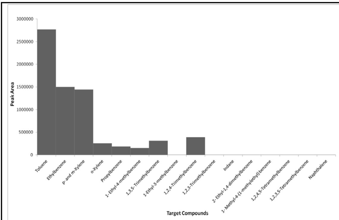
**Figure D3.12: Target Compound Chromatogram of a 50-50 Polypropylene-Wool Carpet Swatch burnt in a Can with Lid On for 10 minutes**
