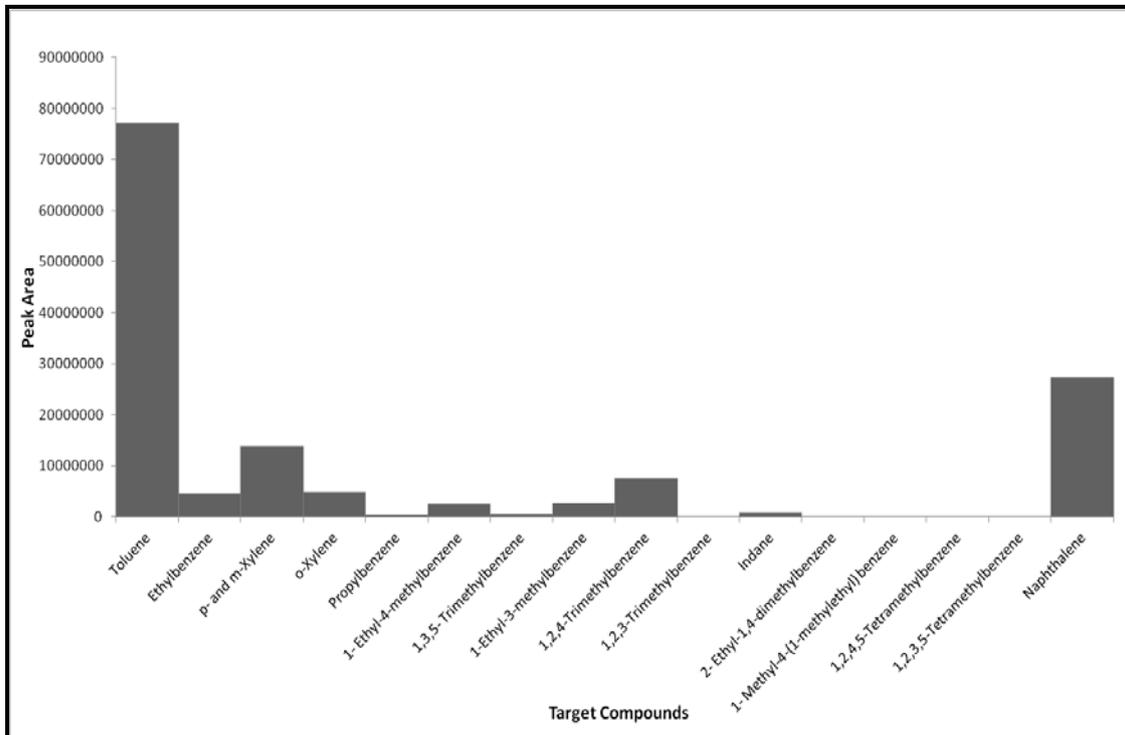
**Figure H5.2: Target Compound Chromatogram of Polypropylene Fibres Pyrolysed at 900°C**
