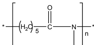
**Figure 3.54: Structure of Nylon 6**
