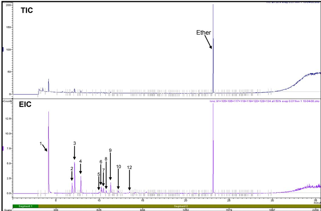
**Figure 3.24: Total Ion Chromatogram and Extracted Ion Chromatogram for 50% Evaporated Petrol Diluted to 0.01% (v/v) (Refer to Section 2.5.1 for GC/MS conditions)**
