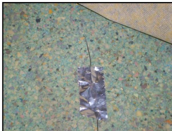
**Figure 3.70: Thermocouple placed between Underlay and Carpet**
