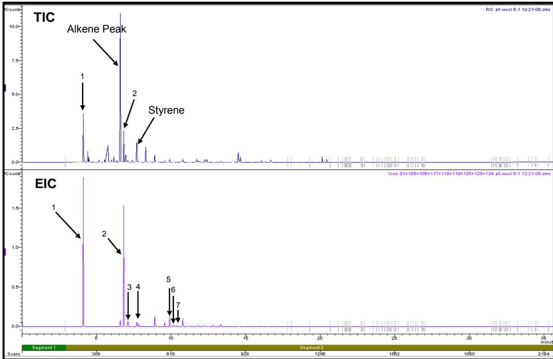
**Figure D2.5: Total Ion Chromatogram and Extracted Ion Chromatogram of a Wool Carpet Swatch burnt in a Can with Lid On for 5 minutes**
