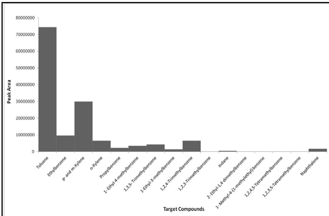
**Figure H7.4: Target Compound Chromatogram of 50-50 Polypropylene-Wool Fibres Pyrolysed at 750°C**
