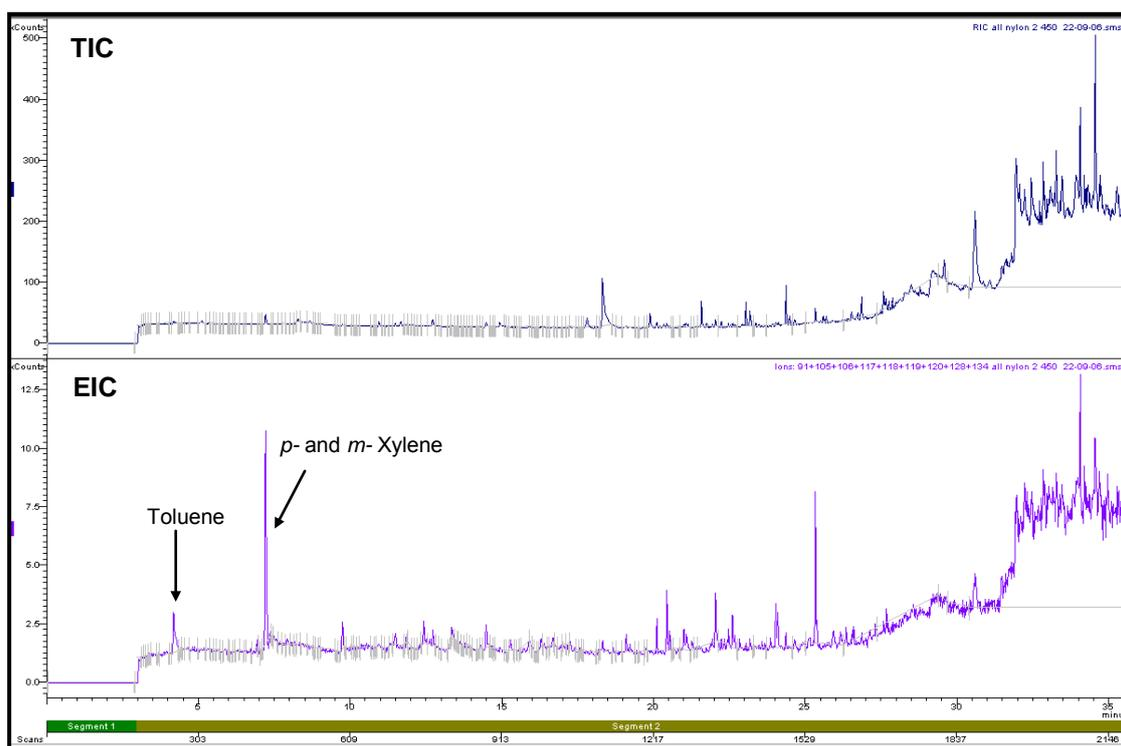
**Figure H1.7: Total Ion Chromatogram and Extracted Ion Chromatogram of Nylon Fibres Pyrolysed at 450°C**
