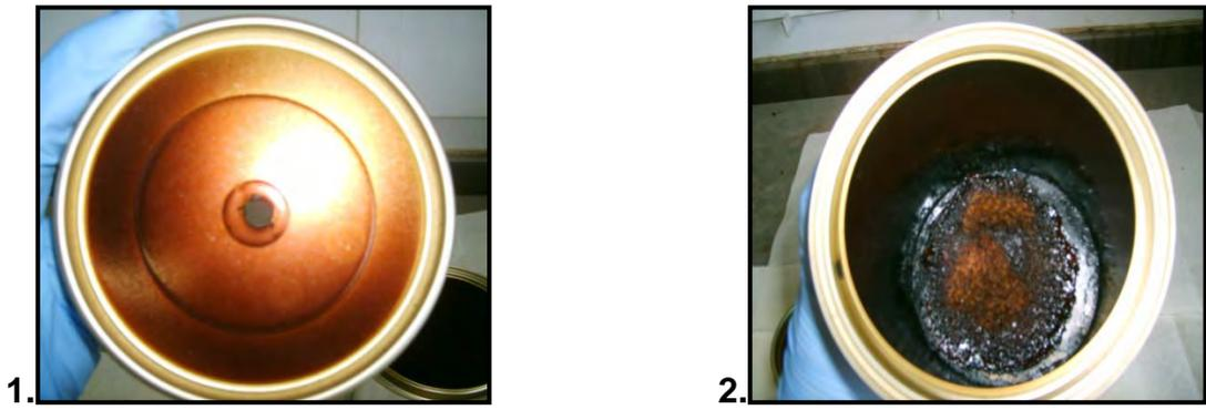
**Figure C1.7 (a): 1. Underside of Lid and 2. Sample in Bottom of Can after Burning**
