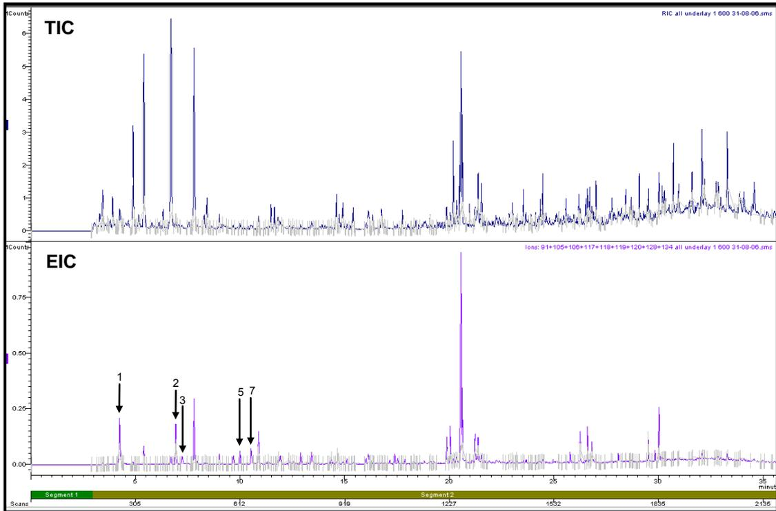
**Figure H9.5: Total Ion Chromatogram and Extracted Ion Chromatogram of Underlay Pyrolysed at 600°C**
