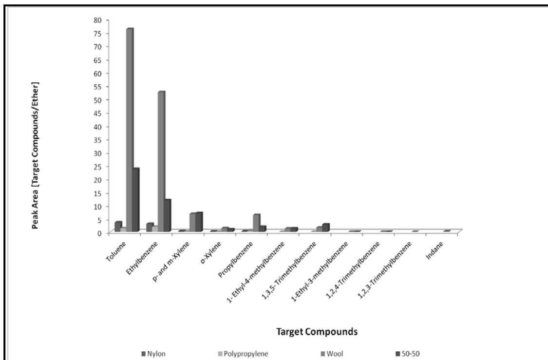
Figures E1.1: Target Compound Chromatogram for all Carpets when Burnt in the Small Can with Lid On for 5 minutes
