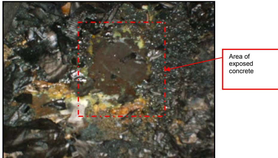
**Figure 3.85: Carpet and Underlay at Perimeter of Petrol Spill after the Fire (where group B Thermocouples were located)**
