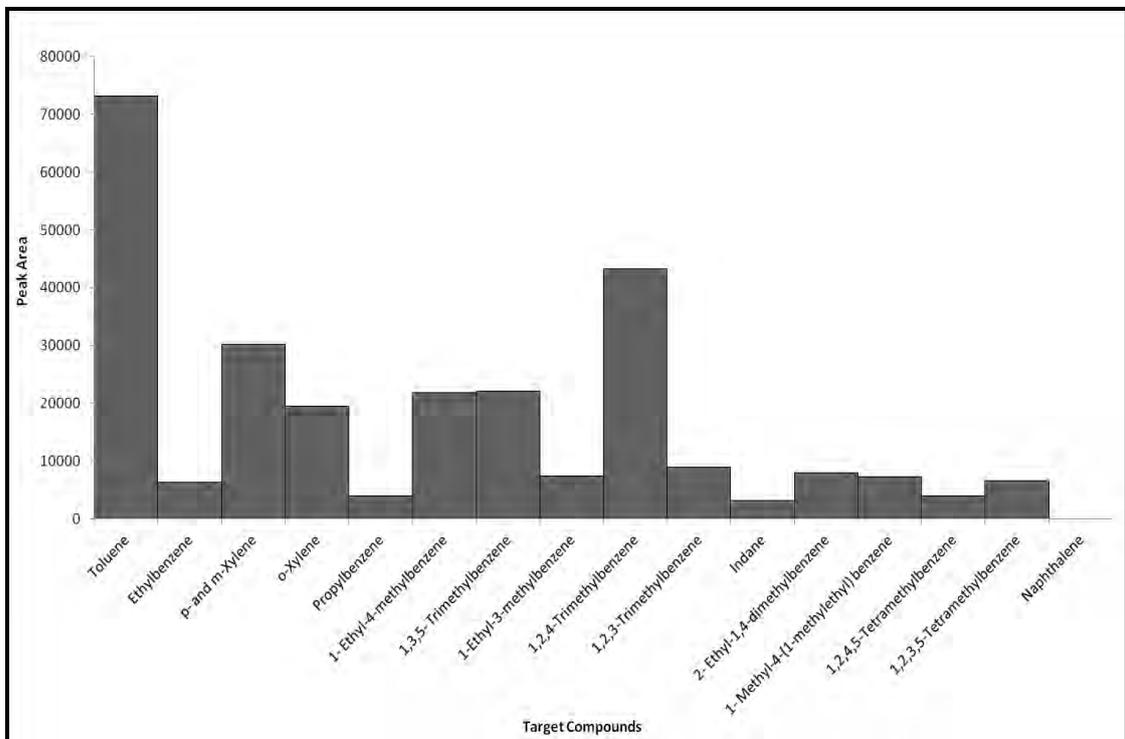
**Figure 3.27: Target Compound Chromatogram for 95% Evaporated Petrol Diluted to 0.01% (v/v)**
