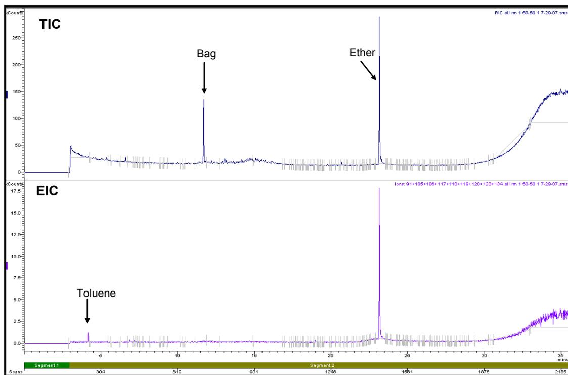
**Figure 4.11: Total Ion Chromatogram and Extracted Ion Chromatogram of 50-50 Polypropylene-Wool Carpet burnt in Room 1 (Refer to Section 2.5.1 for GC/MS conditions)**
