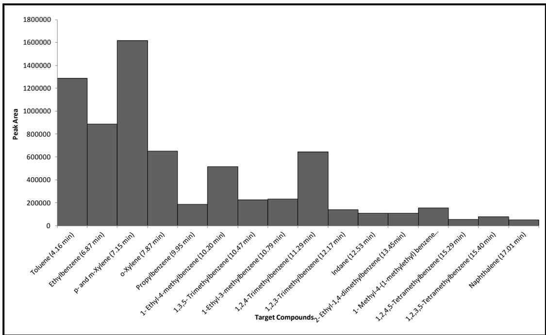
**Figure 1.8: Target Compound Chromatogram for Unleaded Petrol**
