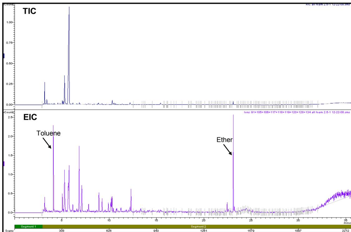
**Figure F1.2: Total Ion Chromatogram and Extracted Ion Chromatogram of Foam Burnt in a Can with Lid On for 2.5 minutes**
