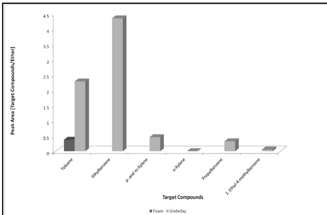
**Figure G1.1: Target Compound Chromatogram for Foam and Underlay when Burnt in the Small Can with Lid On for 2.5 minutes**
