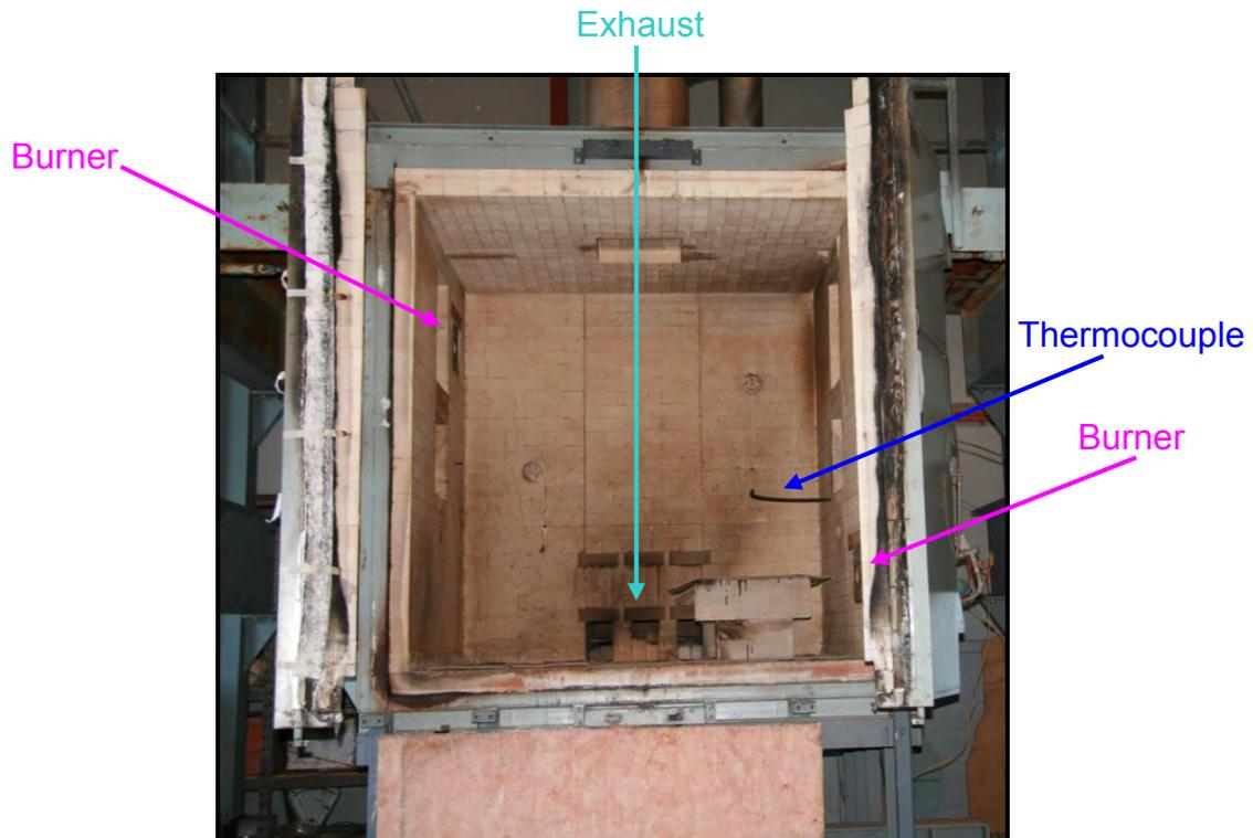
Figure 2.5: Interior of Furnace, showing Burners, Thermocouple and Exhaust
