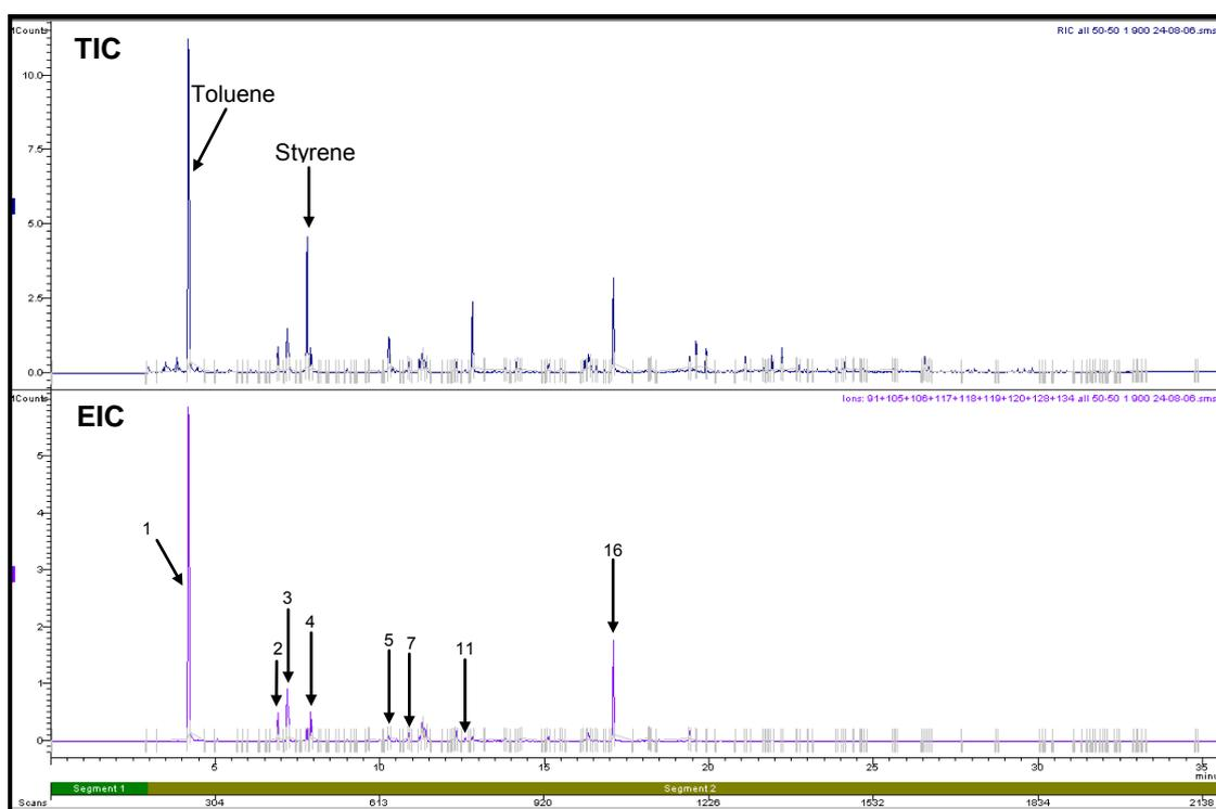
**Figure H7.1: Total Ion Chromatogram and Extracted Ion Chromatogram of 50-50 Polypropylene-Wool Fibres Pyrolysed at 900°C**
