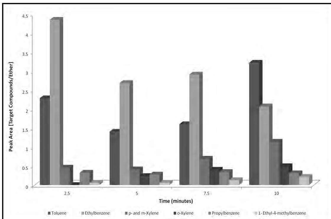
**Figure 4.56: Graph of Peak Area of Target Compounds with Butylated Hydroxytoluene vs. Burn Time for Underlay**
