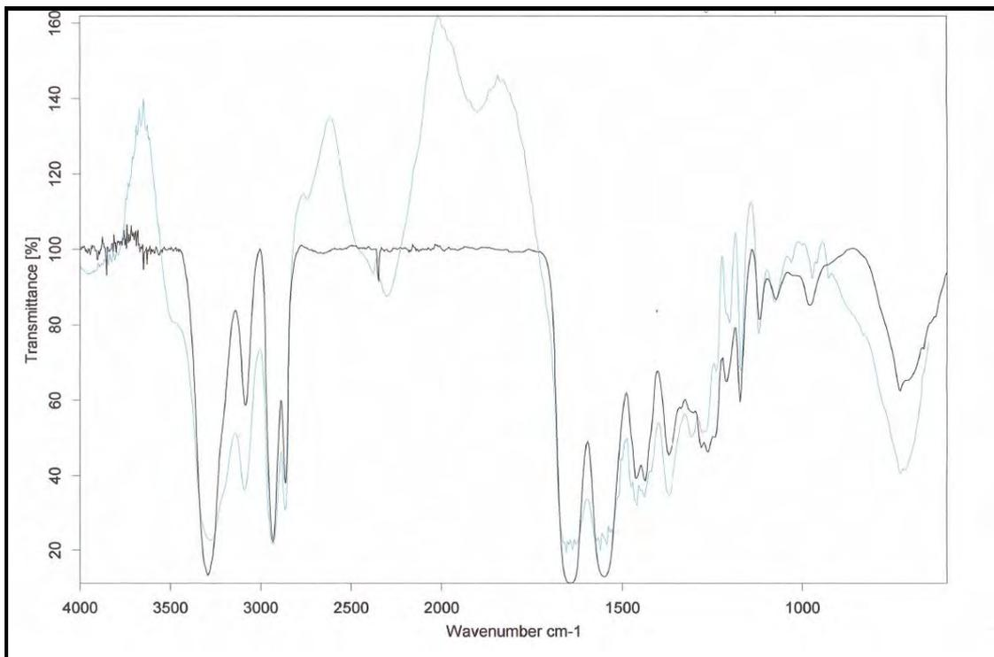
**Figure 3.59: FTIR Spectra of the 2 ply 100% Dyed Nylon Standard (light blue) compared with Library Spectra of Nylon (black)**
