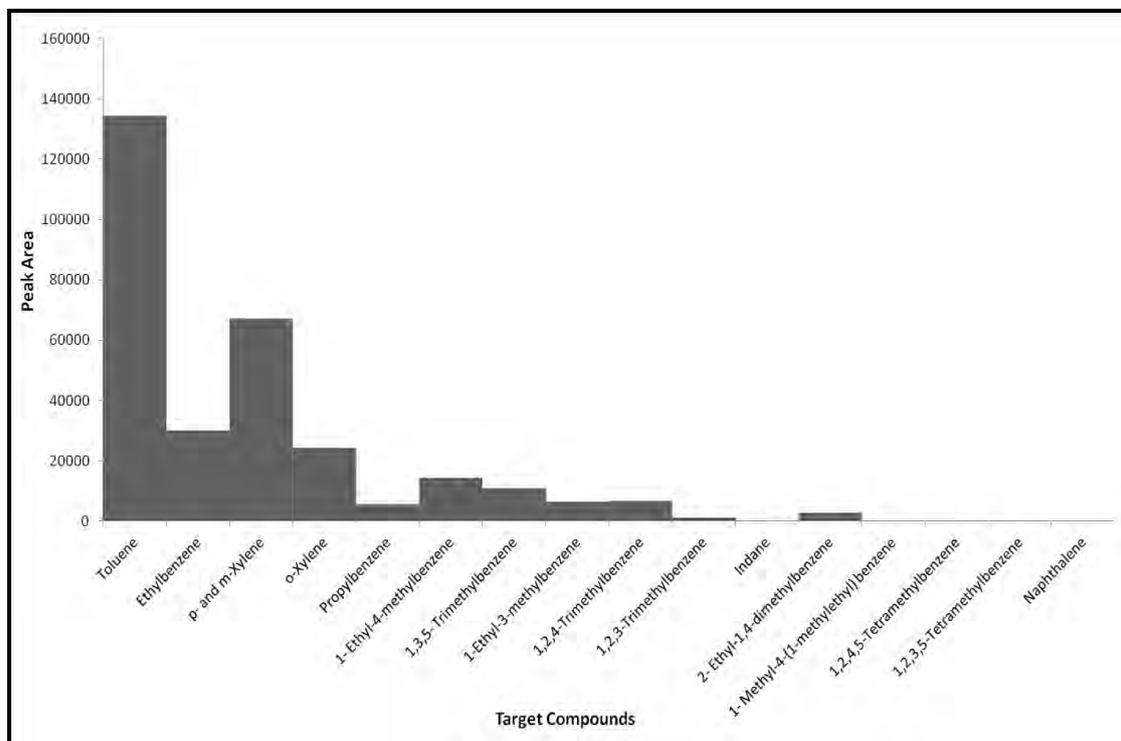
**Figure 3.43: Target Compound Chromatogram of KimWipe spiked with 10 $\mu$ L of Unevaporated Petrol**
