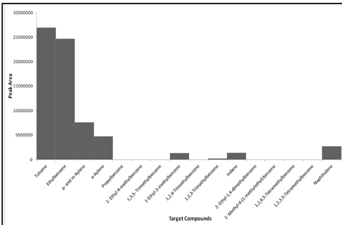
**Figure H1.4: Target Compound Chromatogram of Nylon Fibres Pyrolysed at 750°C**
