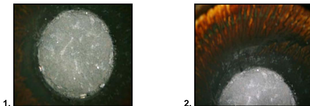
**Figure D2.7 (b): 1. Top of Sample and 2. Side of Can after Burning**
