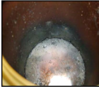
**Figure D1.1 (c): Inside of Can after Burning**
