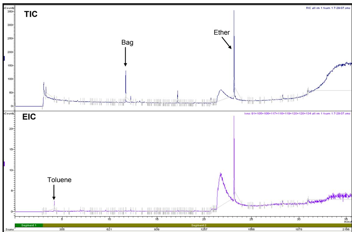
**Figure 4.12: Total Ion Chromatogram and Extracted Ion Chromatogram of Foam burnt in Room 1 (Refer to Section 2.5.1 for GC/MS conditions)**
