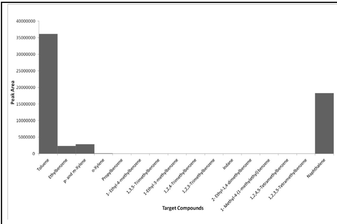
**Figure H6.2: Target Compound Chromatogram of Wool Fibres Pyrolysed at 900°C**
