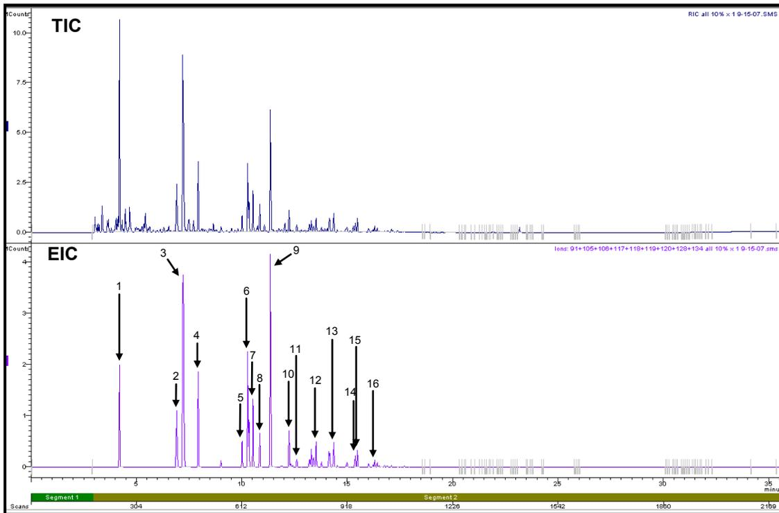
**Figure 3.4: Total Ion Chromatogram and Extracted Ion Chromatogram for Unevaporated Petrol Diluted to 10% (v/v) (Refer to Section 2.5.1 for GC/MS conditions)**
