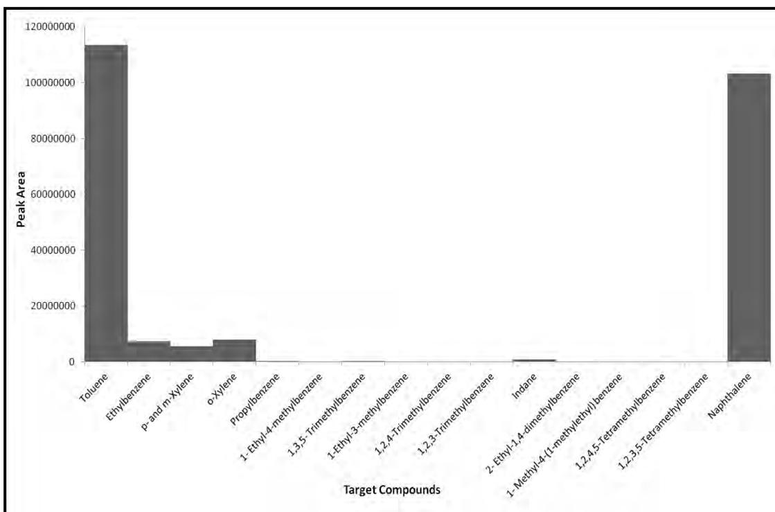
**Figure 4.62: Target Compound Chromatogram for Adhesive Pyrolysed at 900°C**
