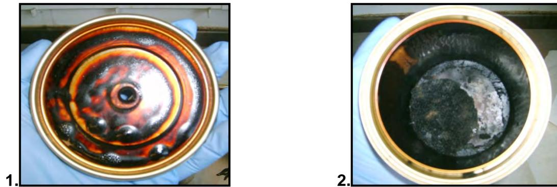
**Figure C1.20 (a): 1. Underside of Lid and 2. Sample in Bottom of Can after Burning**
