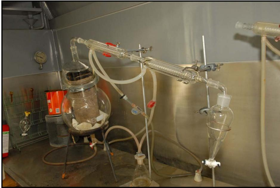
**Figure A1.1(b): Steam Distillation set up at VPFSC Laboratories with Sample of Burnt Nylon Carpet**
