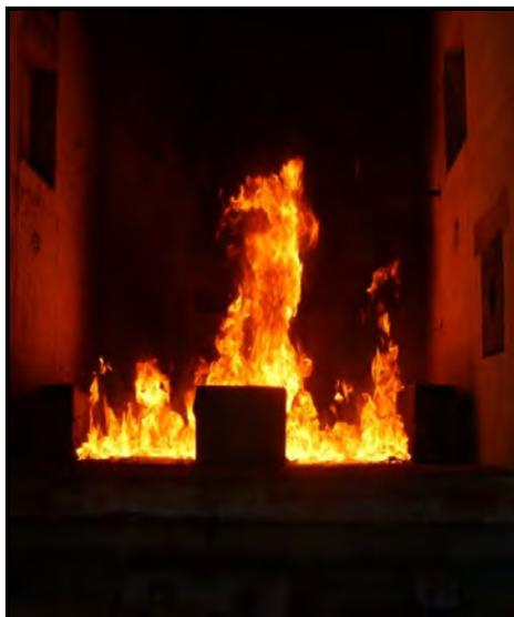
**Figure 4.20(a): Polypropylene Carpet when Doors were Opened after Furnace Burn at 470°C**
