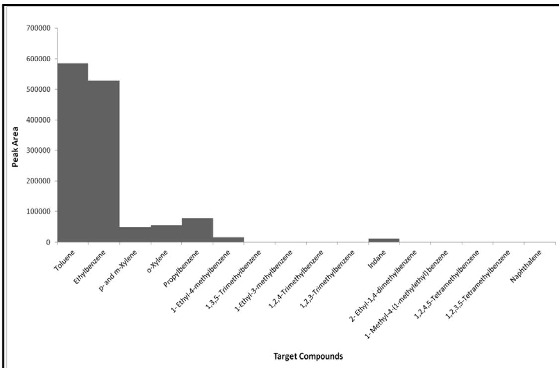
**Figure C1.13: Target Compound Chromatogram of a Nylon Carpet Swatch burnt in a Can with Lid On for 3 minutes**
