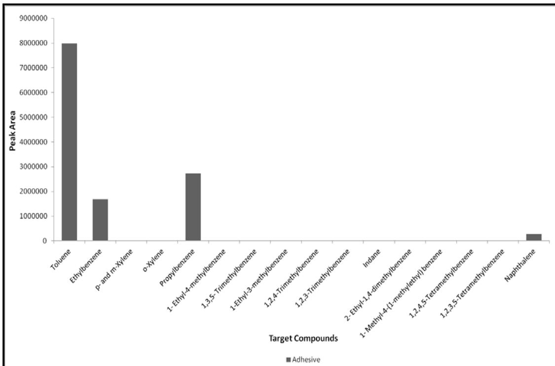
**Figures J1.17: Target Compound Chromatogram for Carpet Backing Components pyrolysed at 450°C**
