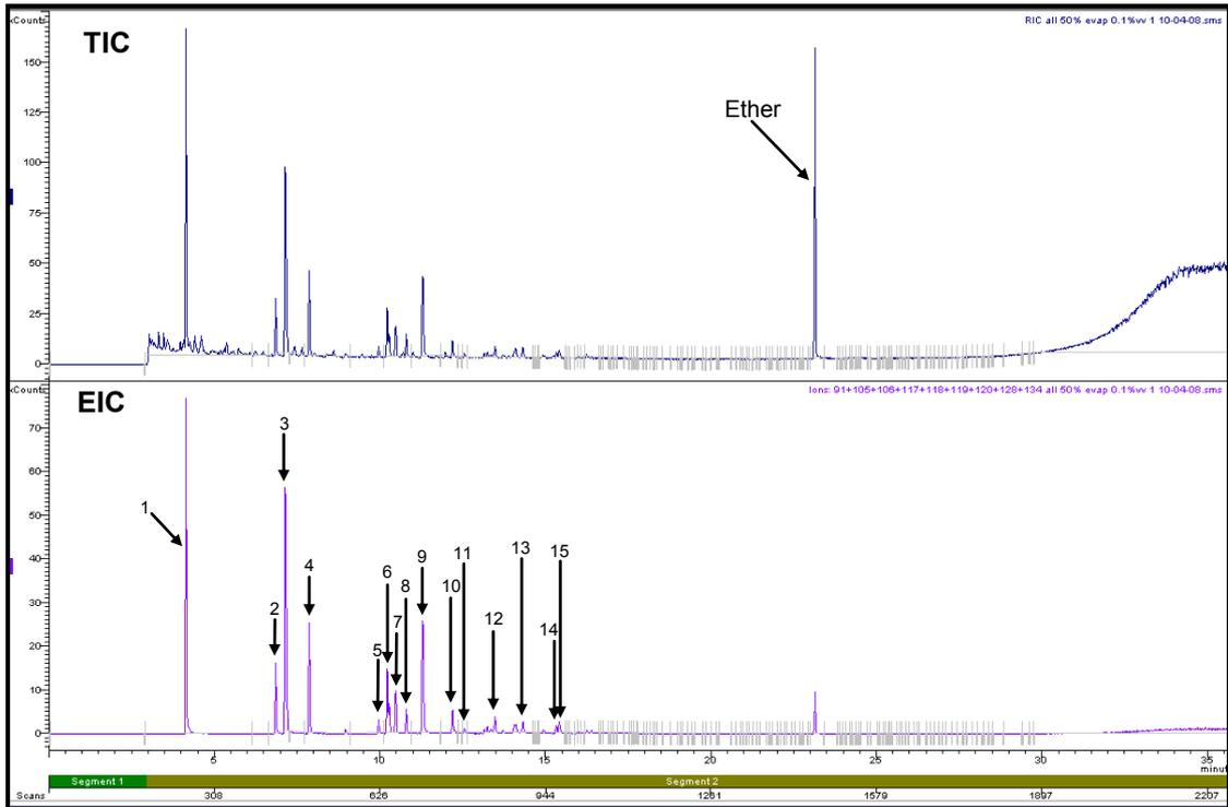
**Figure 3.18: Total Ion Chromatogram and Extracted Ion Chromatogram for 50% Evaporated Petrol Diluted to 0.1% (v/v) (Refer to Section 2.5.1 for GC/MS conditions)**
