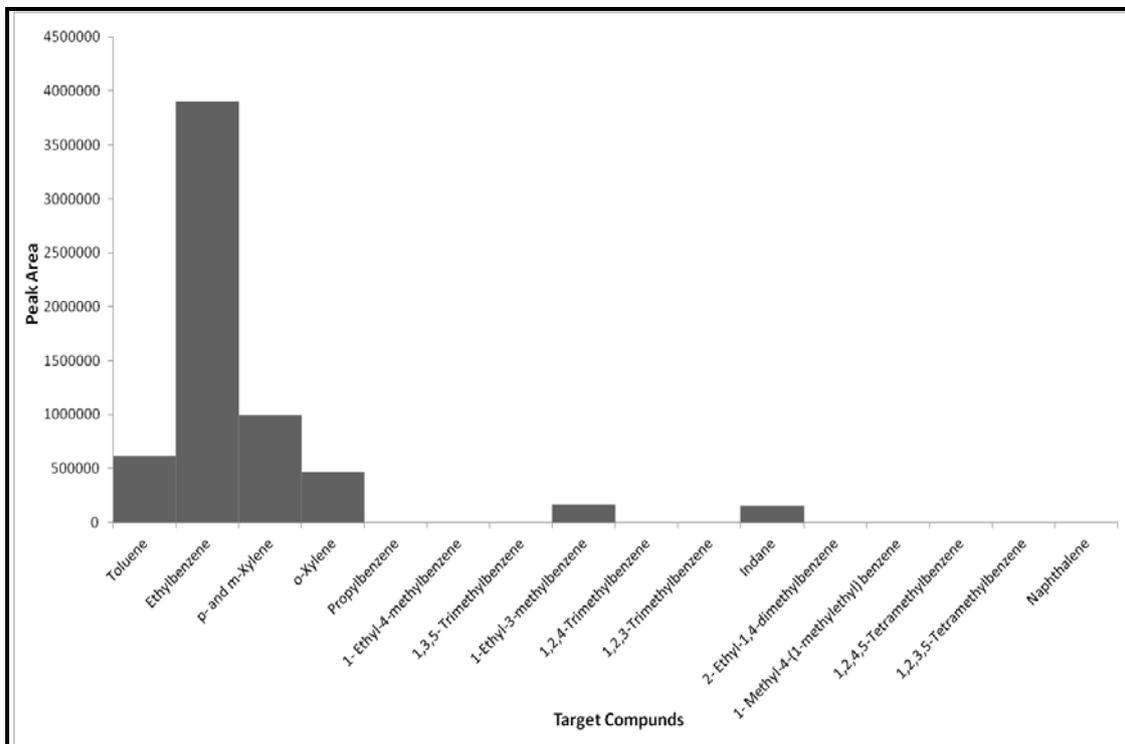
**Figure H1.6: Target Compound Chromatograms of Nylon Fibres Pyrolysed at 600°C**
