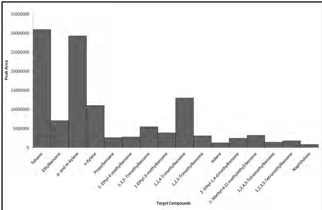
**Figure 3.7: Target Compound Chromatogram for 50% Evaporated Petrol Diluted to 10% (v/v)**
