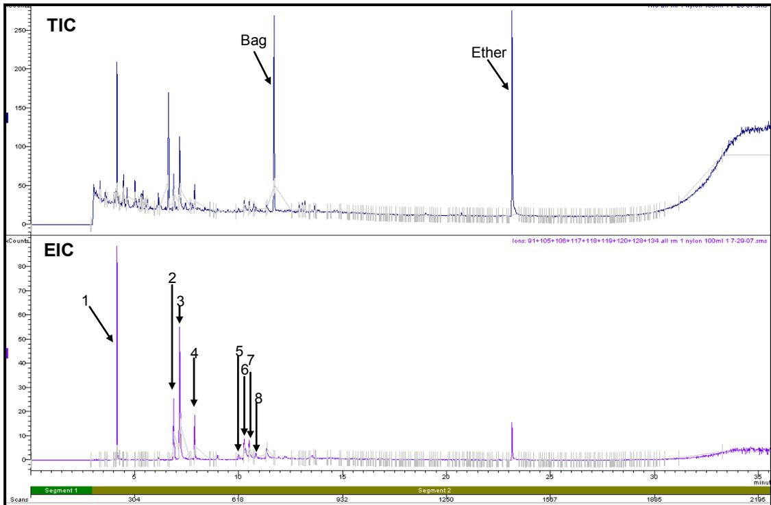
**Figure 4.7: Total Ion Chromatogram and Extracted Ion Chromatogram of Nylon Carpet spiked with 100mL Petrol burnt in Room 1 (Refer to Section 2.5.1 for GC/MS conditions)**
