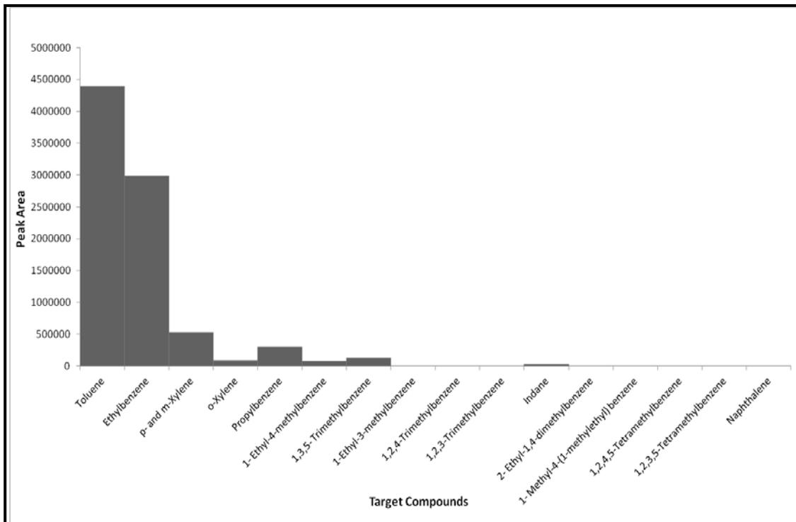
**Figure D2.9: Target Compound Chromatogram of a Wool Carpet Swatch burnt in a Can with Lid On for 7.5 minutes**
