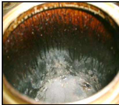
**Figure C1.29 (c): Inside of Can after Burning**
