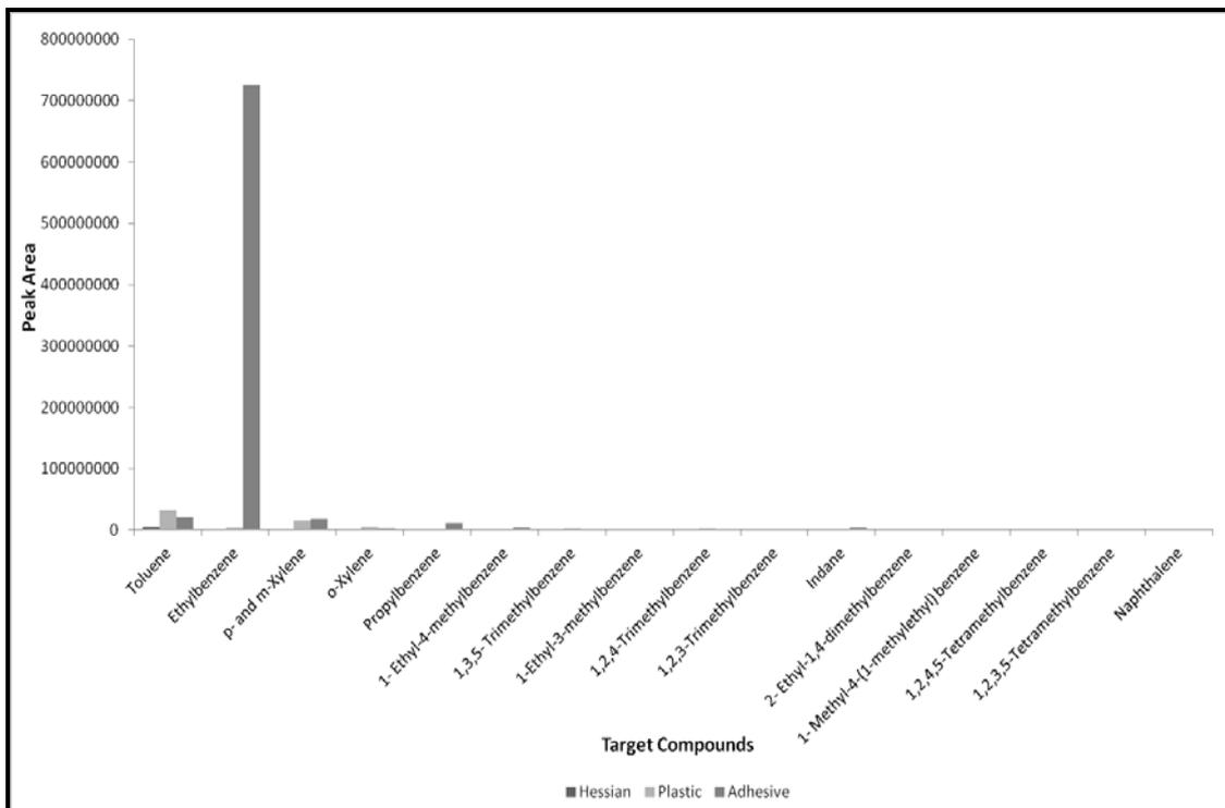
**Figures J1.15: Target Compound Chromatogram for Carpet Backing Components pyrolysed at 750°C**
