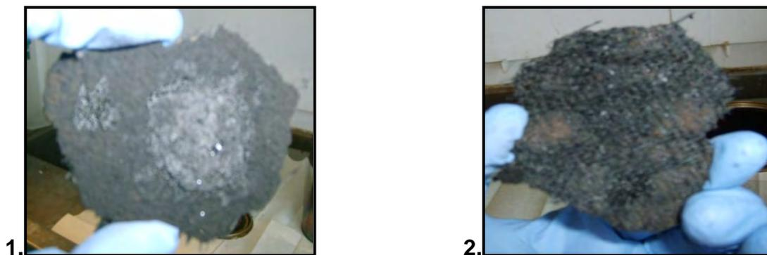
**Figure C1.23 (b): 1. Top and 2. Underside of Sample after Burning**
