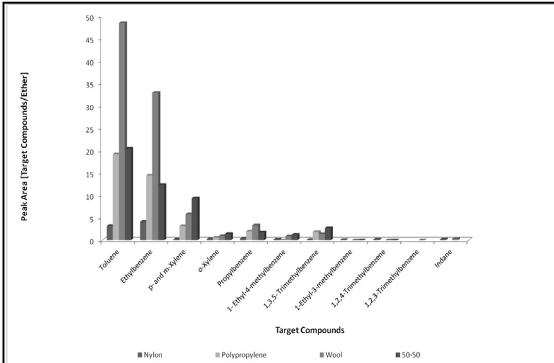
**Figures E1.2: Target Compound Chromatogram for all Carpets when Burnt in the Small Can with Lid On for 7.5 minutes**
