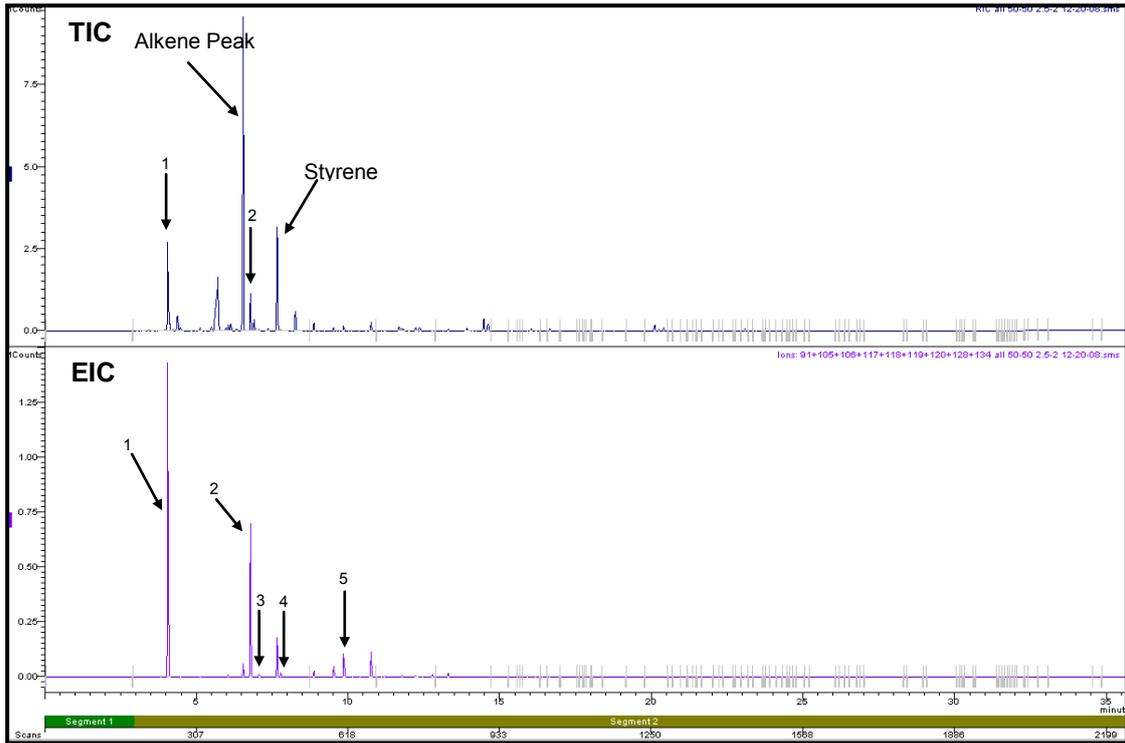
**Figure D3.2: Total Ion Chromatogram and Extracted Ion Chromatogram of a 50-50 Polypropylene-Wool Carpet Swatch burnt in a Can with Lid On for 2.5 minutes**
