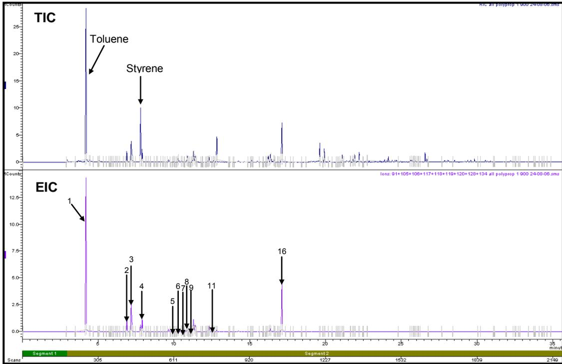
**Figure H5.1: Total Ion Chromatogram and Extracted Ion Chromatogram of Polypropylene Fibres Pyrolysed at 900°C**
