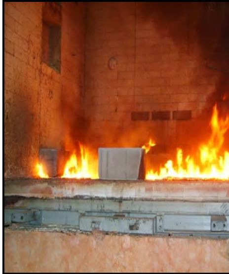
**Figure 4.19: Polypropylene Carpet when Doors were Opened after Furnace Burn at 570°C**
