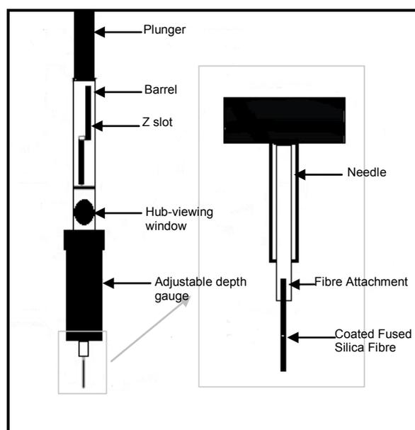
Figure 1.5: Schematic of the Solid Phase Micro Extraction Device
