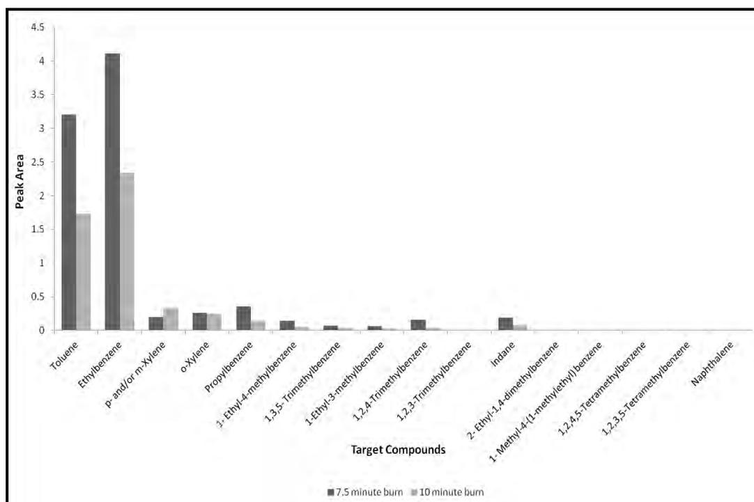
**Figure 4.41: Graph of peak area of Target Compounds recovered when burning Nylon Carpet for 7.5 and 10 minutes in a Small Can plotted as a Ratio with Butylated Hydroxytoluene**
