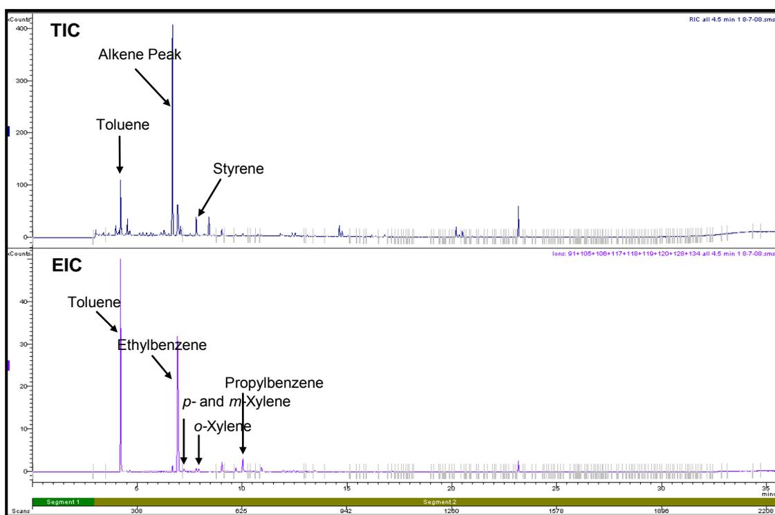
**Figure C1.21: Target Ion Chromatogram and Extracted Ion Chromatogram of a Nylon Carpet Swatch burnt in a Can with Lid On for 4.5 minutes**
