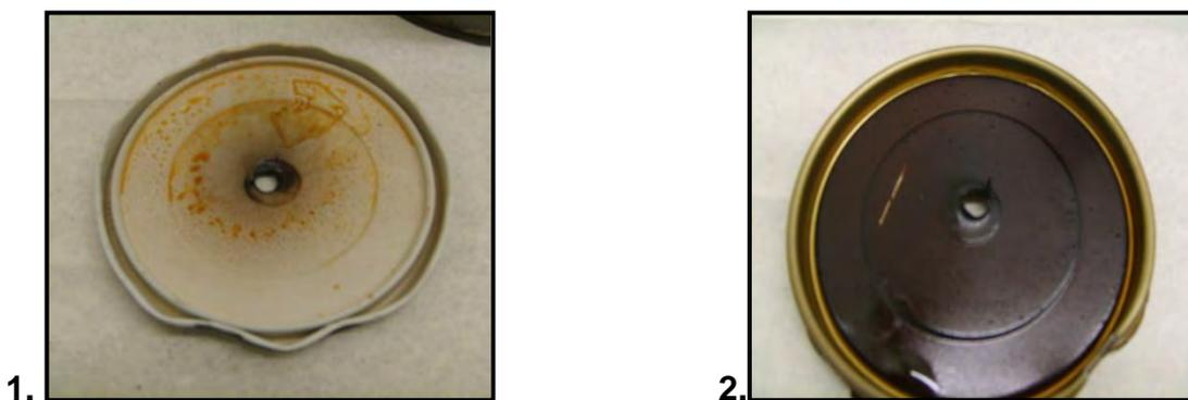
**Figure D1.10 (a): 1. Top of lid and 2. Underside of Lid after Burning**
