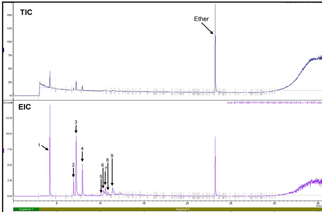
**Figure 3.22: Total Ion Chromatogram and Extracted Ion Chromatogram for Unevaporated Petrol Diluted to 0.01% (v/v) (Refer to Section 2.5.1 for GC/MS conditions)**
