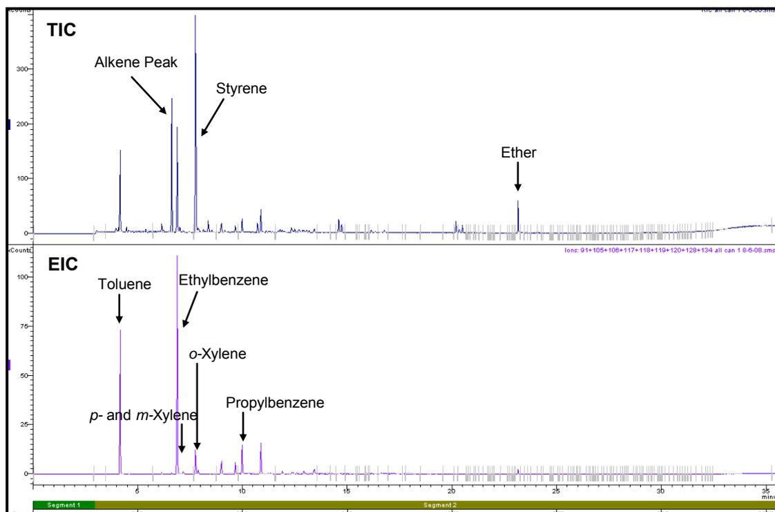
**Figure 4.39: Total Ion Chromatogram and Extracted Ion Chromatogram of Can (Refer to Section 2.5.1 for GC/MS conditions)**
