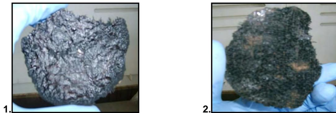
**Figure C1.20 (b): 1. Top and 2. Underside of Sample after Burning**
