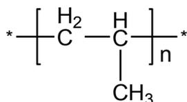
**Figure 3.61: Structure of Polypropylene**
