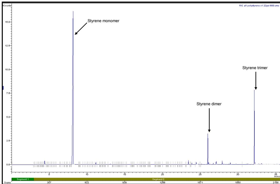
**Figure 3.68: Pyrogram of Polystyrene Pyrolysed at 600°C at 22psi (Refer to Section 2.5.1 for GC/MS conditions)**
