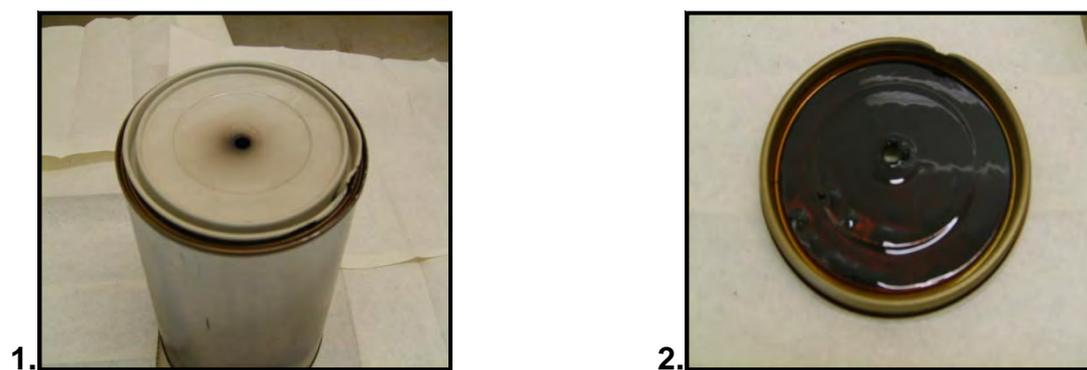
**Figure F1.6 (a): 1. Top and 2. Underside of Lid after Burning**
