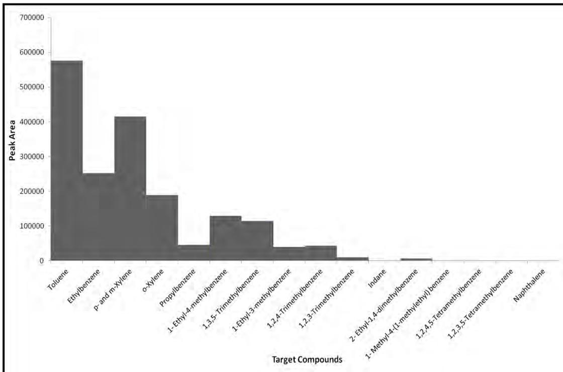
**Figure 4.8: Target Compound Chromatogram of Nylon Carpet spiked with 100mL Petrol burnt in Room 1**
