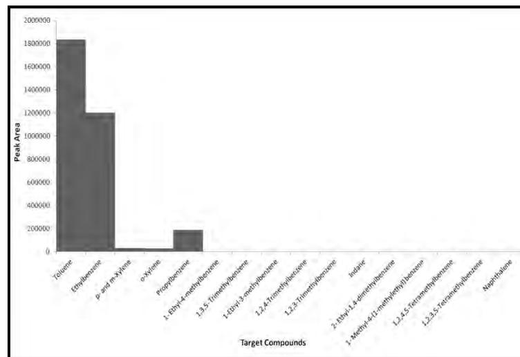
**Target Compound Chromatogram of a wool carpet swatch burnt for 2.5 minutes in a can**
