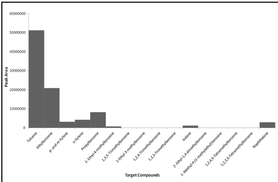
**Figure H4.6: Target Compound Chromatogram of Adhesive from Carpet Backing Pyrolysed at 600°C**
