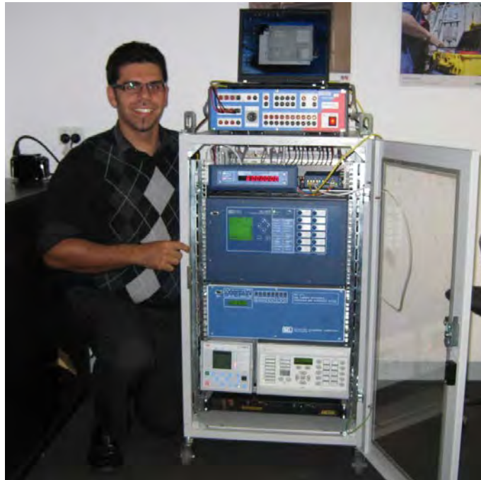
Figure A.39: Portable IEC61850 Testing Unit (Front View)
