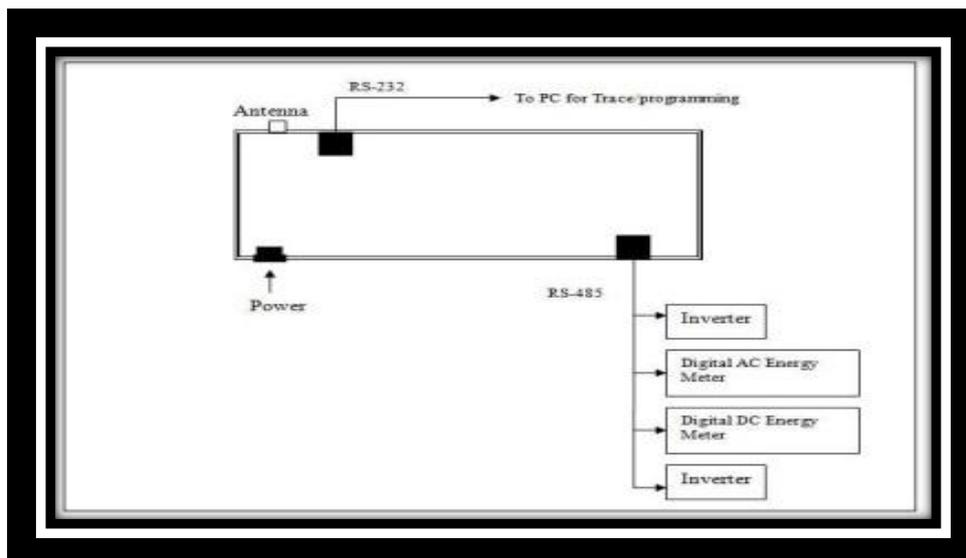
Figure 7.3: EWS Typical Layout showing RS-232 AND RS-485.
