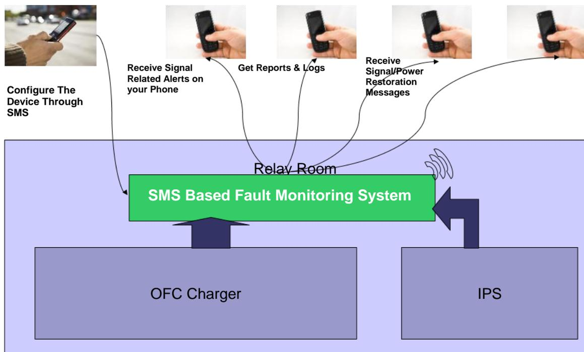
Figure 7.4: A solution to improve the reliability of Railway Signaling and Telecommunications. This system has been installed at a test site and working reliably
