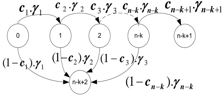
Figure 5.3: System failure process using non-homogeneous Markov chain.
