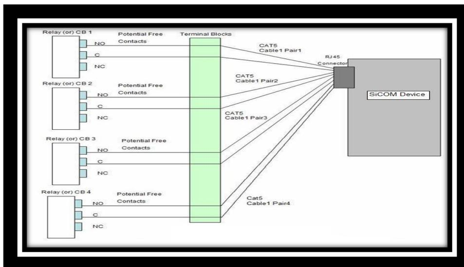
Figure 7.2: Wiring diagram for digital inputs
