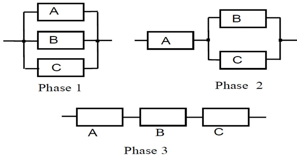
Figure 4.1: Phases: Phase1- during autumn and spring, when it has to ensure only the manger water, Phase 2- during winter then it has to ensure the heating process and manager water and phase 3-during the summer when it has to ensure the cooling process and the manager water [13].
