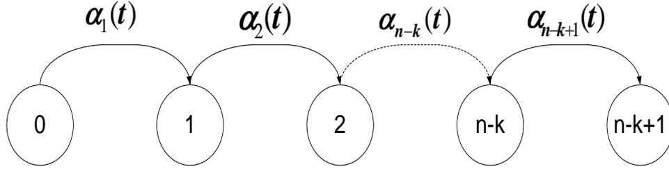
Figure 5.1: Non-homogeneous Markov process for identical components case.
