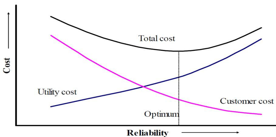
Figure 2.2 Components of Reliability and Cost
