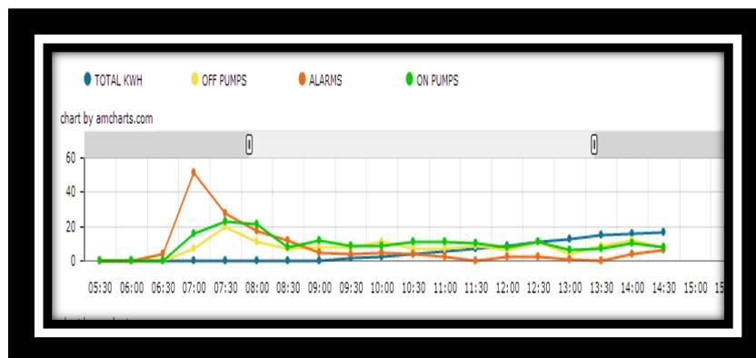
Figure 7.8: Total amount of energy produced, number of solar pumps in operation and number of alarm messages at particular time of the day.
