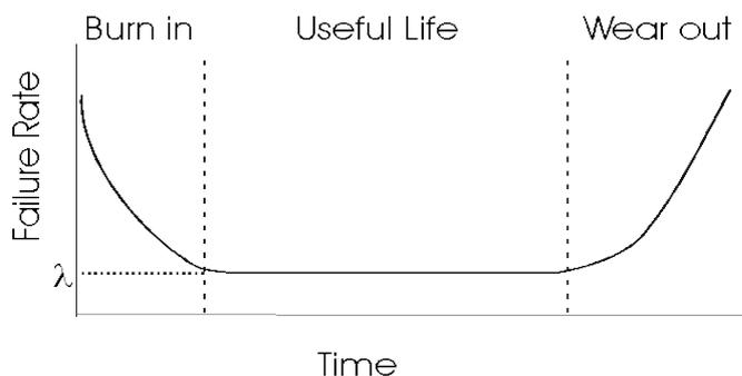
Figure 2.1: Bath tub shaped hazard rate function graph
