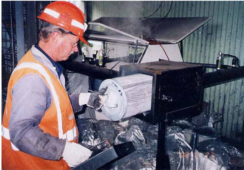
Figure 4.5 Changing Filter Element on Test Rig
