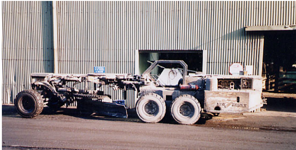
Figure 4.3 Photograph of Noyes Grader Used in Test Rig as Source of Particulate
