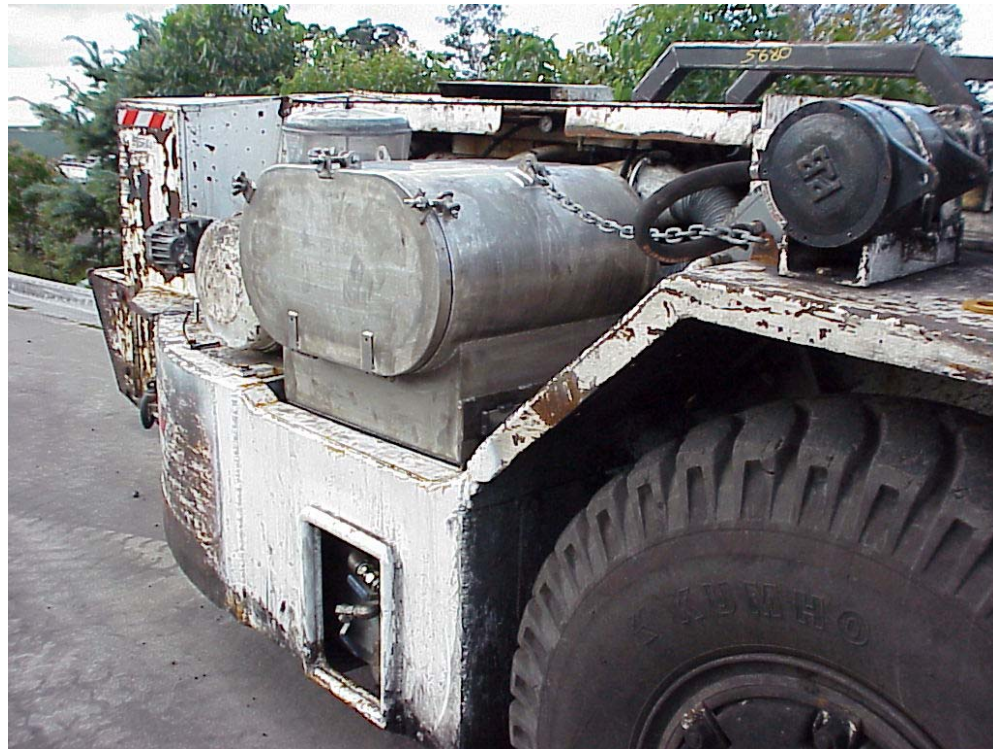
Figure 10 – Disposable filter assembly fitted to an underground mining machine (Source: Davies 2003)
