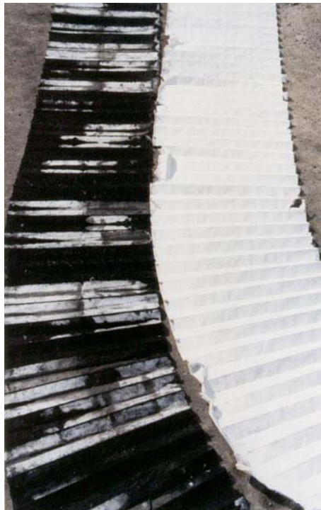
Figure 11 – Comparison of New (right) and Used (left) Filter Media
