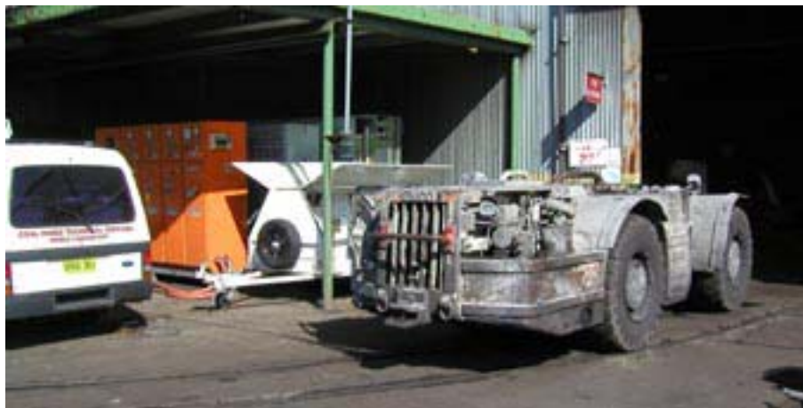
Figure 5.2 R&P Series 5100 Analyser and Mobile Gas Laboratory on-site during testing of an EIMCO LHD
