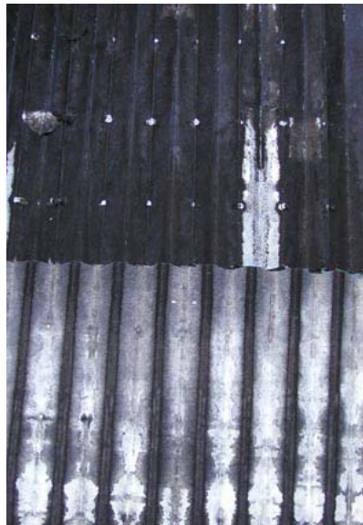
Figure 4.12 Filter Media After 44 Hours Use (160 Pleats) (Top – inlet side of filter; Bottom – outlet side of filter)
