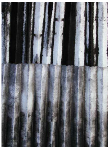
Figure 4.13 Filter Media After 31 Hours Use (200 Pleats) (Top – inlet side of filter; Bottom – outlet side of filter)
