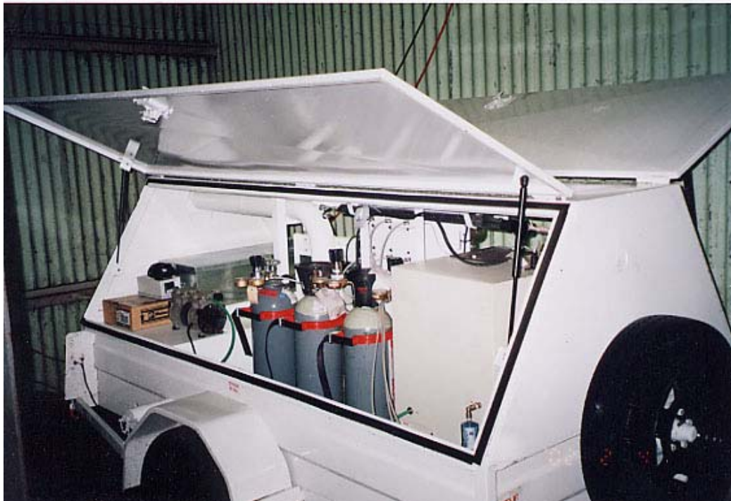
Figure 8 - Mobile Raw Exhaust Test Trailer fitted with modified Rupprecht & Patashnick Series 5100 Diesel Particulate Analyser
