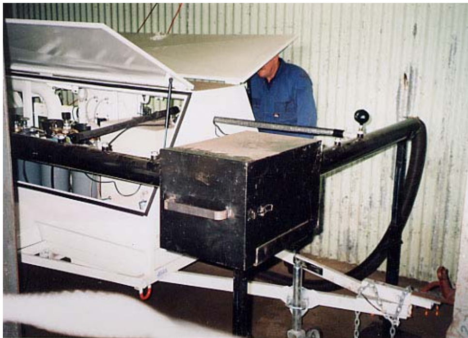
Figure 4.4 Filter Test Rig with Heater Pre and Post Filter Sampling Probes
