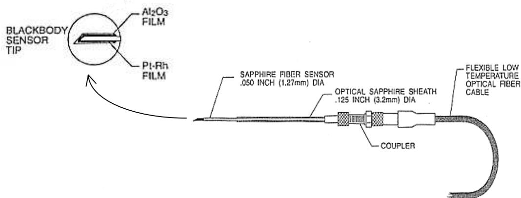
Figure 1.2.4 A black body radiation sensor [Accufiber Inc., 1988].
