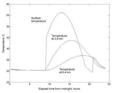
Figure 6. Temporal variations of the temperatures of wheat at the surface and at distances of 3.9cm and 8.4cm below the upper surface of the grain bulk before the passage of the cooling wave. All emissivities are assumed to be 0.9.
