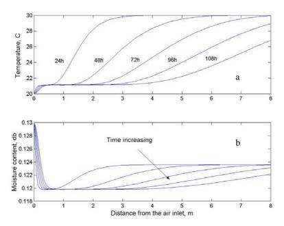
Figures 5a and 5b. The passage of temperature and moisture fronts through a bed of wheat 8 m high when the air flow rate is 0.08 kg dry air/(s.m<sup>2</sup>) when aerated with ambient air that has a dry bulb temperature of 20°C and a relative humidity of 50%. The initial moisture content and temperature of the wheat are 11% (wet basis) and 30°C respectively.
