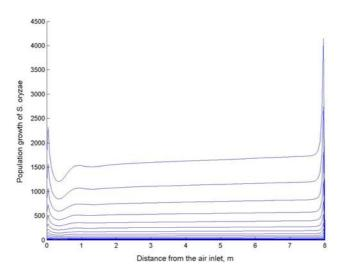
Figure 18. The population multiples of *S. oryzae* at intervals of five days for a total of 100 days in 11% moisture content grain, initially at 30°C, and aerated with ambient air.
