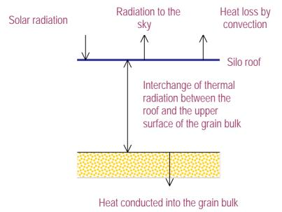
Figure 3. A representation of heat nows on a suo root and the upper surface of a bulk
