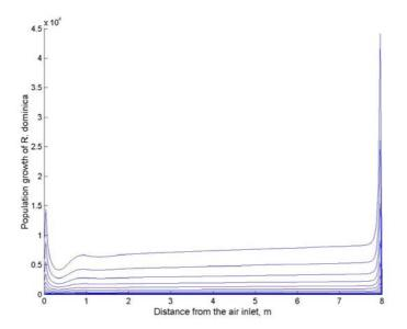
Figure 15. The population multiples of *R. dominica* at intervals of five days for a total of 100 days in 11% moisture content grain, initially at  $30^{\circ}$ C, and aerated with ambient air.
