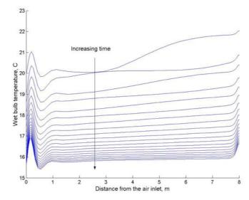
Figure 12. The wet bulb temperature profiles at intervals of five days in a bulk of wheat with an initial moisture content of 11% when the air leaving the upper surface of the grain is recirculated.
