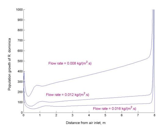
Figure 17. A comparison of the rates of population increase of R. dominica when 11% moisture content grain is recircaerated at flow rates equivalent to 1, 1.5 and 2 litres/(s.tonne).
