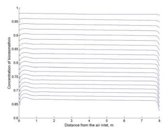
Figure 22. The rate of decay of the pesticide bioresmethrin on grain initially with a temperature of  $30^{\circ}$ C and with a moisture content of 11% (wet basis) when aerated with ambient air with an air flow rate of 0.008 kg/(s.m<sup>2</sup>).
