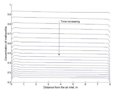
Figure 20. The rate of decay of the pesticide methacrifos on grain initially with a temperature of  $30^{\circ}$ C and with a moisture content of 11% (wet basis) when aerated with ambient air with an air flow rate of 0.008 kg/(s.m<sup>2</sup>).
