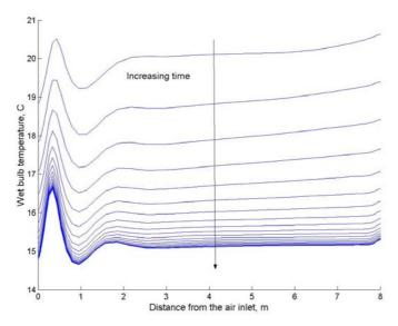
Figure 14. The development of profiles of the wet bulb temperature in beds of wheat recircaerated with an air flow rate of 2 litres per second per tonne of grain.
