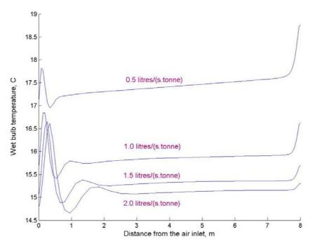
Figure 13. Profiles of wet bulb temperatures along the length of the grain bed after it has been recircaerated with nominal air flow rates of 0.5, 1.0, 1.5 and 2.0 litres per second per tonne of grain. The total elapsed time is 100 days.
