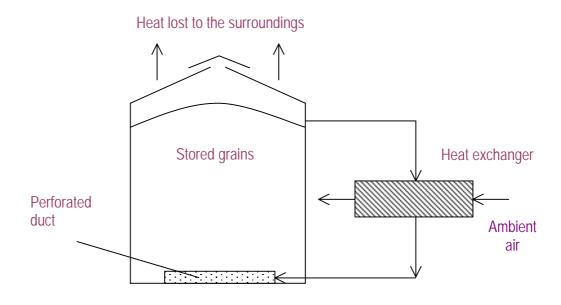
Figure 2. An arrangement of the components of a recircaeration system
