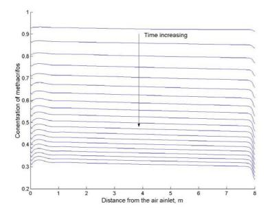
Figure 21. The rate of decay of the pesticide methacrifos on grain initially with a temperature of  $30^{\circ}$ C and with a moisture content of 11% (wet basis) when recircaerated with an air flow rate of 0.008 kg/(s.m<sup>2</sup>).
