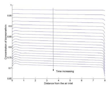
Figure 23. The rate of decay of the pesticide bioresmethrin on grain initially with a temperature of  $30^{\circ}$ C and with a moisture content of 11% (wet basis) when recircaerated with an air flow rate of 0.008 kg/(s.m<sup>2</sup>).
