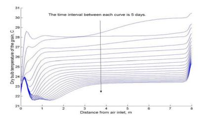
Figure 11. The dry bulb temperature profiles at intervals of five days in a bulk of wheat with an initial moisture content of 11% when the air leaving the upper surface of the grain is cooled and recirculated.
