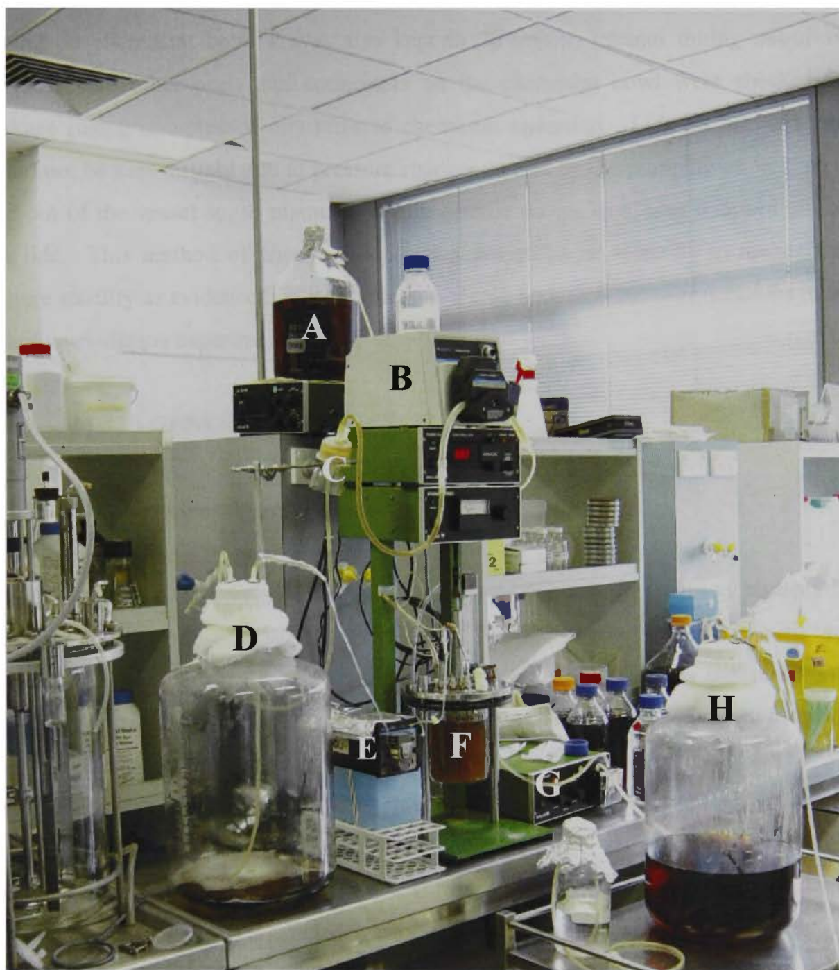
Figure 3.3: Chemostat and ancillary equipment used for adaptive evolution experiments. Labels show: Schott bottle with autoclaved medium (A), pump for sterile filtration (B), sterile filter (C), feed tank (D), feed pump (E), fermentor (F), waste pump (G) and waste tank (H).
