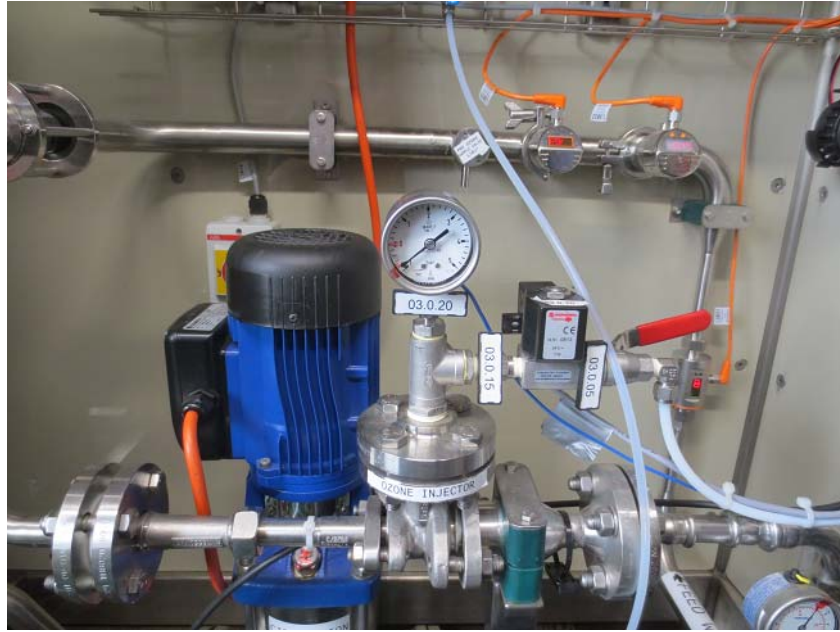
Figure x – Recirculation pump and ozone injection, ozone system, Section 1
