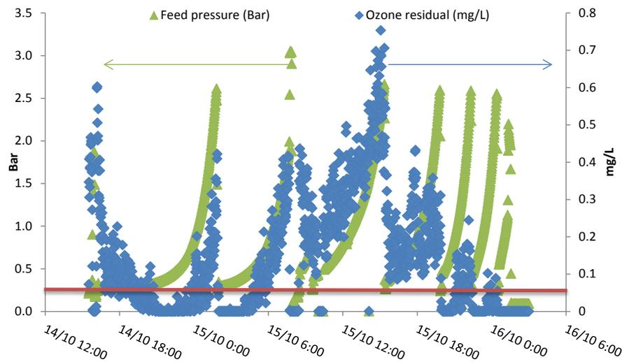
**Figure 5:** Relationship between the feed pressure and ozone residual.
