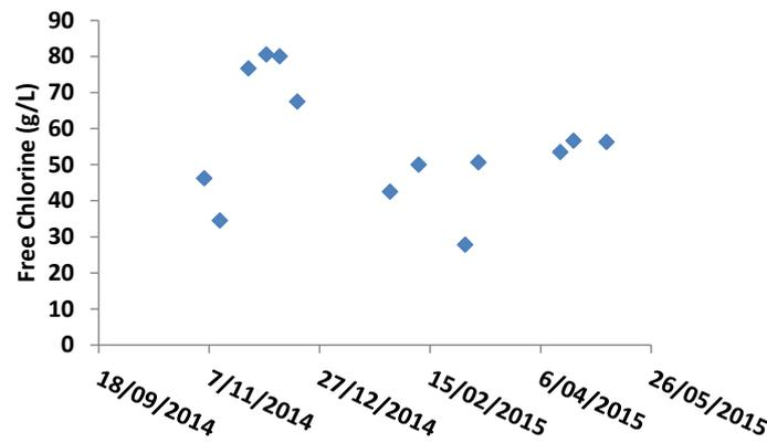
**Figure 26:** Free chlorine concentration in the sodium hypochlorite drum.
