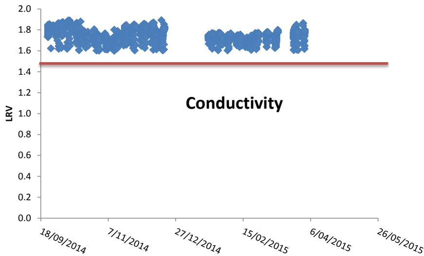
**Figure 19:** RO system LRV based on conductivity rejection.
