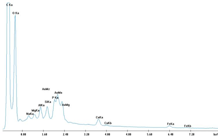
Figure D4. EDS for the element on fouled membrane surface
