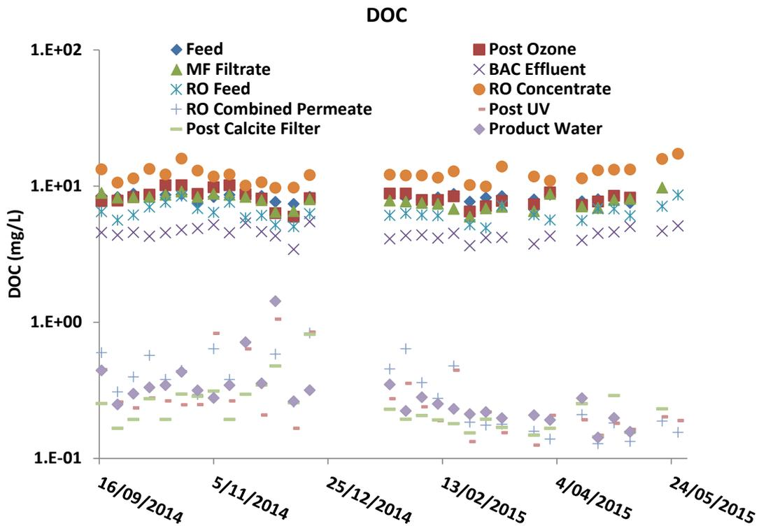
Figure B1a DOC concentrations in the feed and following each treatment unit (Log scale)
