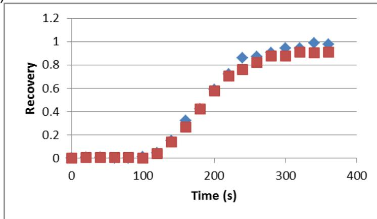
UV Hydraulic Retention Time Tests 1 & 2: Rhodamine WT, Flowrate = 12 L/min (design flowrate)
