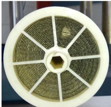
Figure D1. Side view of the RO element
