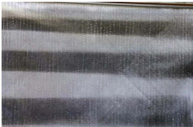
Figure D2. Patterns of foulant formed on the RO element surface
