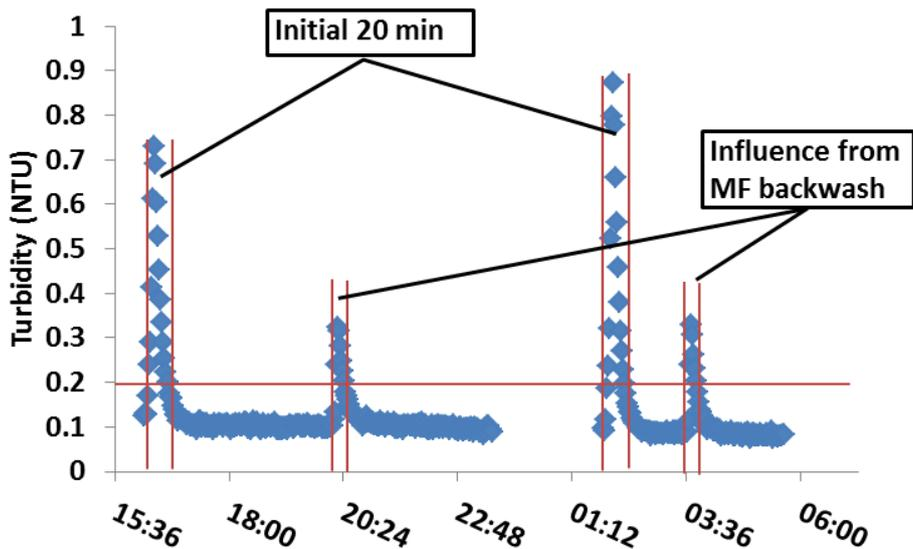
Figure 17: Typical turbidity values in the BAC filtrate.
