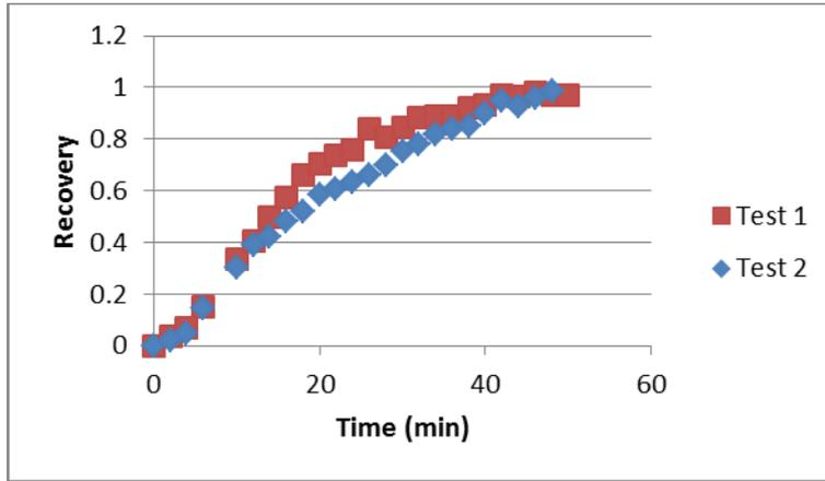
UV Hydraulic Retention Time Tests 1 & 2: Rhodamine WT, Flowrate = 14.4 L/min (design flowrate)
