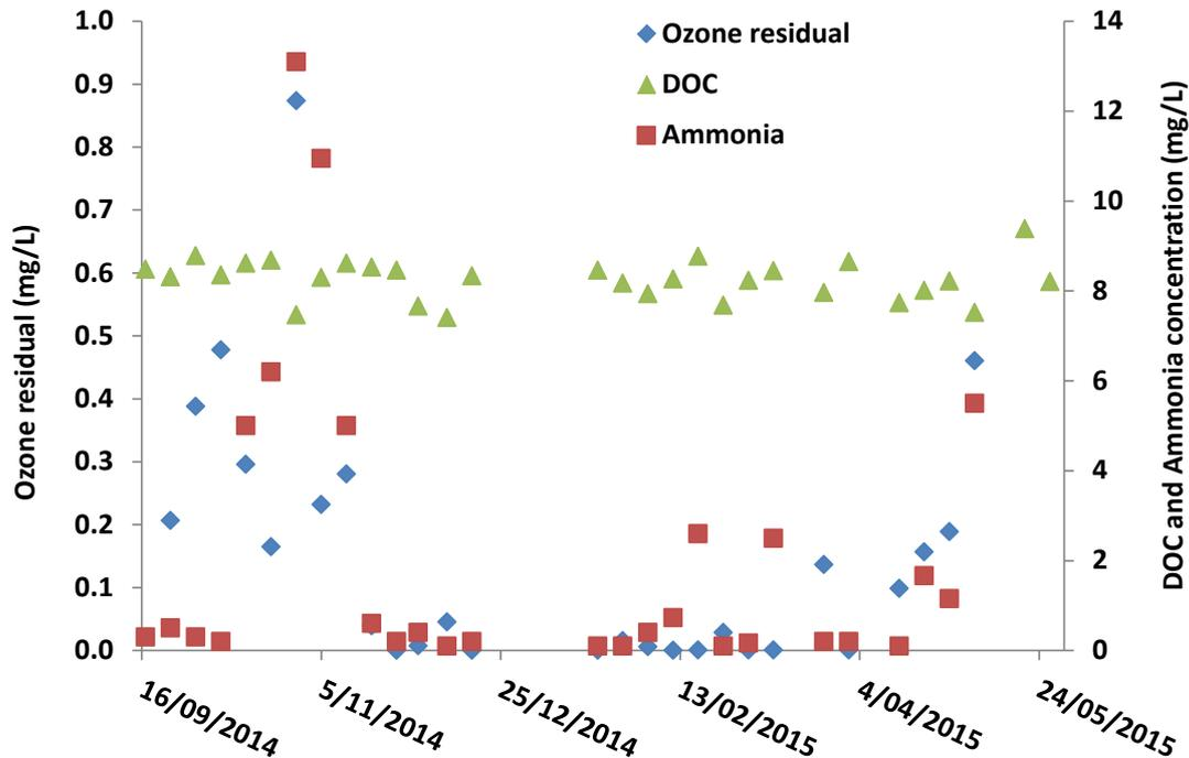
**Figure 6:** Ammonia and DOC concentrations in the feed water plotted with ozone residual.
