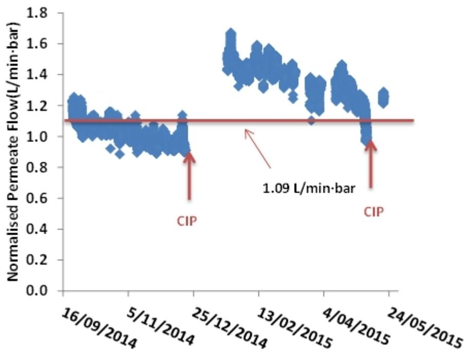
Figure D5. Normalised permeate flow during RO operation
