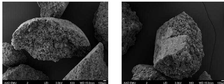
**Figure 15:** Scanning electron microscopy (SEM) images of BAC granules.
