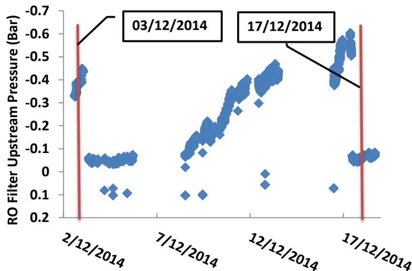
**Figure 20:** Pressure drop across the cartridge filter.
