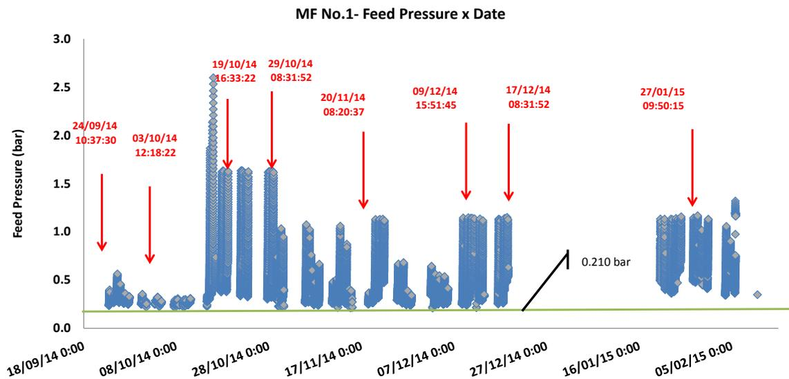
**Figure 13a:** No.1 membrane TMP changed with time.
