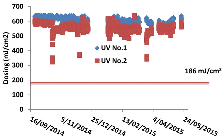
**Figure 24:** UV dose for the two Specktron 6 UV disinfection units.
