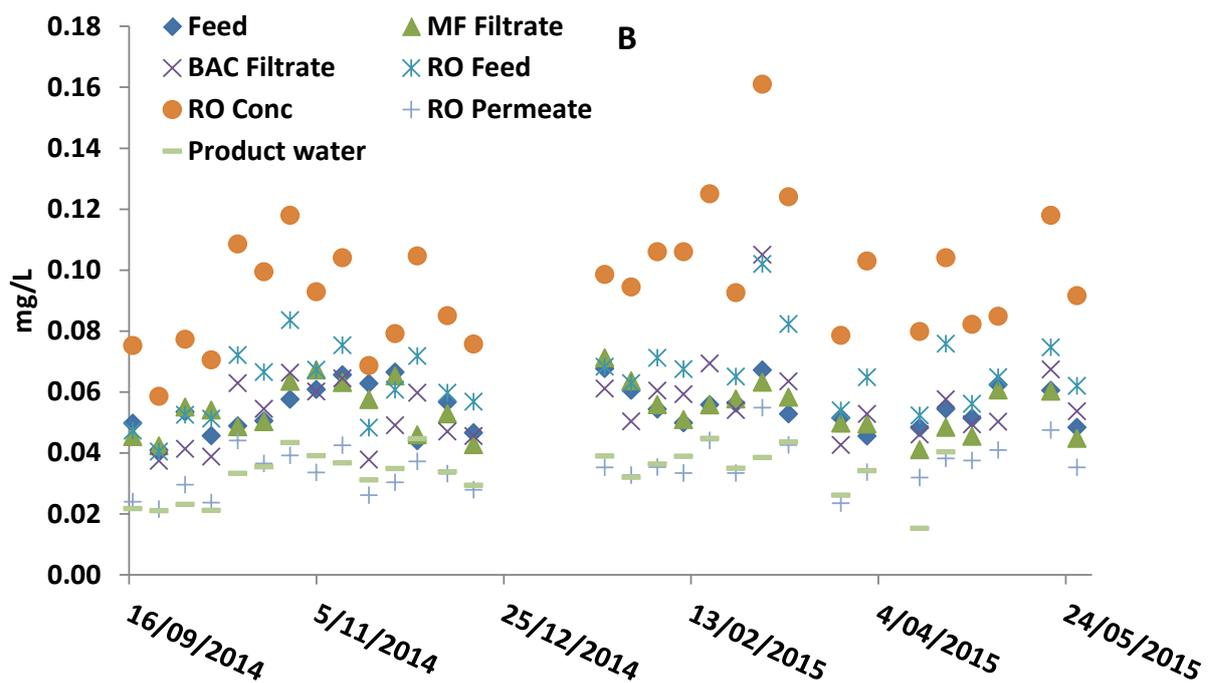
Figure B3 Boron concentrations in the feed and following each treatment unit
