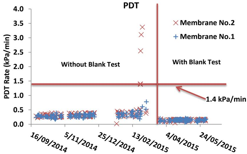
Figure 10: Pressure decay rate of the ceramic membranes.
