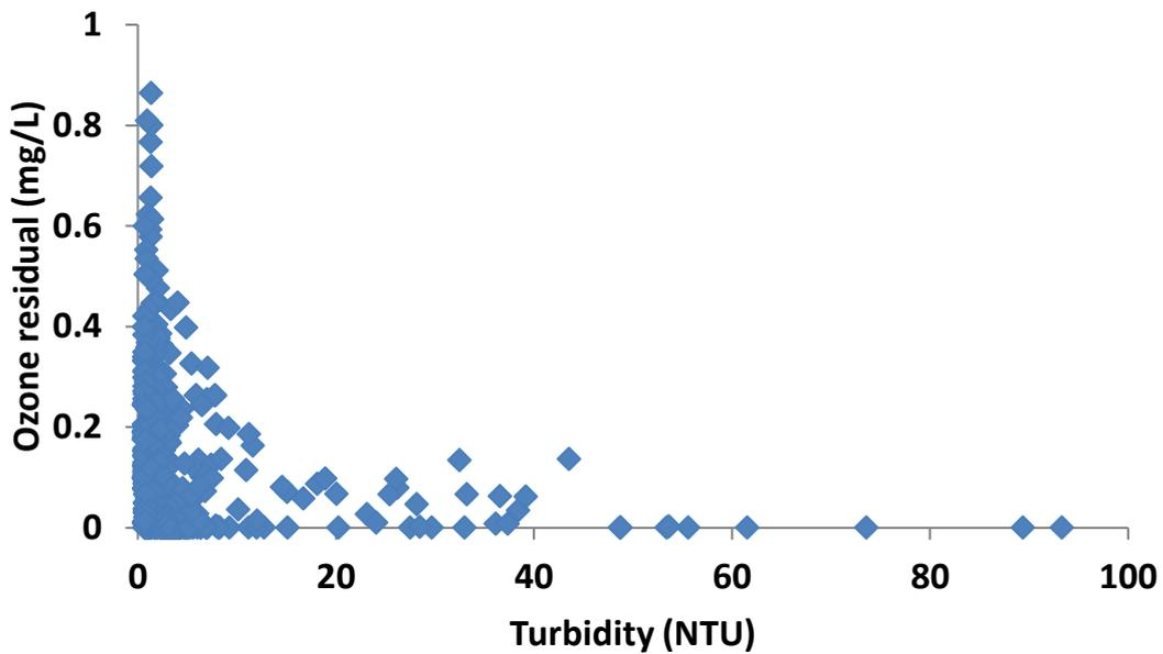
Figure 8: Turbidity in the feed water plotted against ozone residual.
