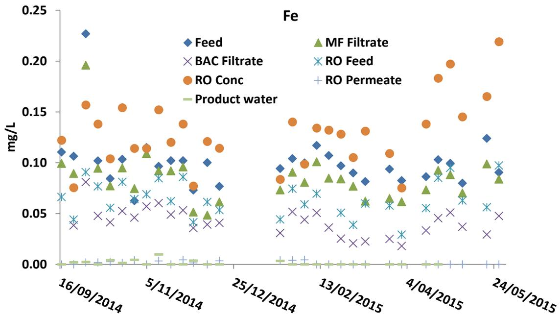
Figure B5 Iron concentrations in the feed and following each treatment unit
