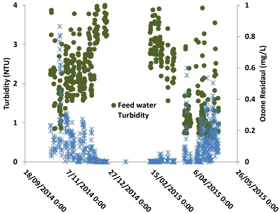
Figure 7: Turbidity in the feed water plotted with ozone residual.
