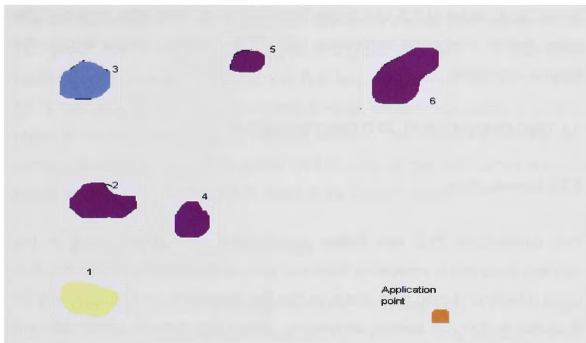
Figure 6.11. Diagrammatic representation of the separation of a bran flavonoid extract by two-dimensional TLC and their colours under UV light at 365 nm.
