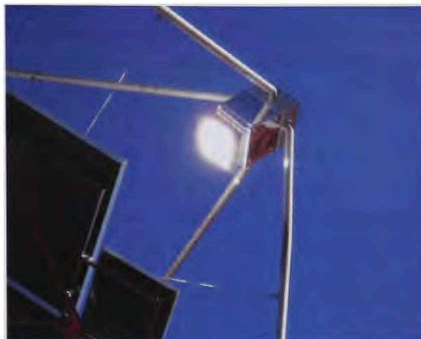
Figure 5-26: Multijunction 35-kWp CPV Receiver on sun with 102 kW of concentrated 'light power' entering the flux modifier
