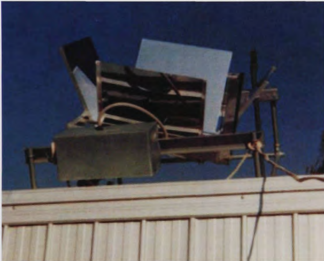
Figure 2-6: Photo of a 2 sun concentration built by the researcher. The system has 4 planar reflectors set at 30 degrees from the normal to the solar panel in the centre. Tracking was achieved by using a shadow band east-west with a seasonal tilt in the N-S direction.
