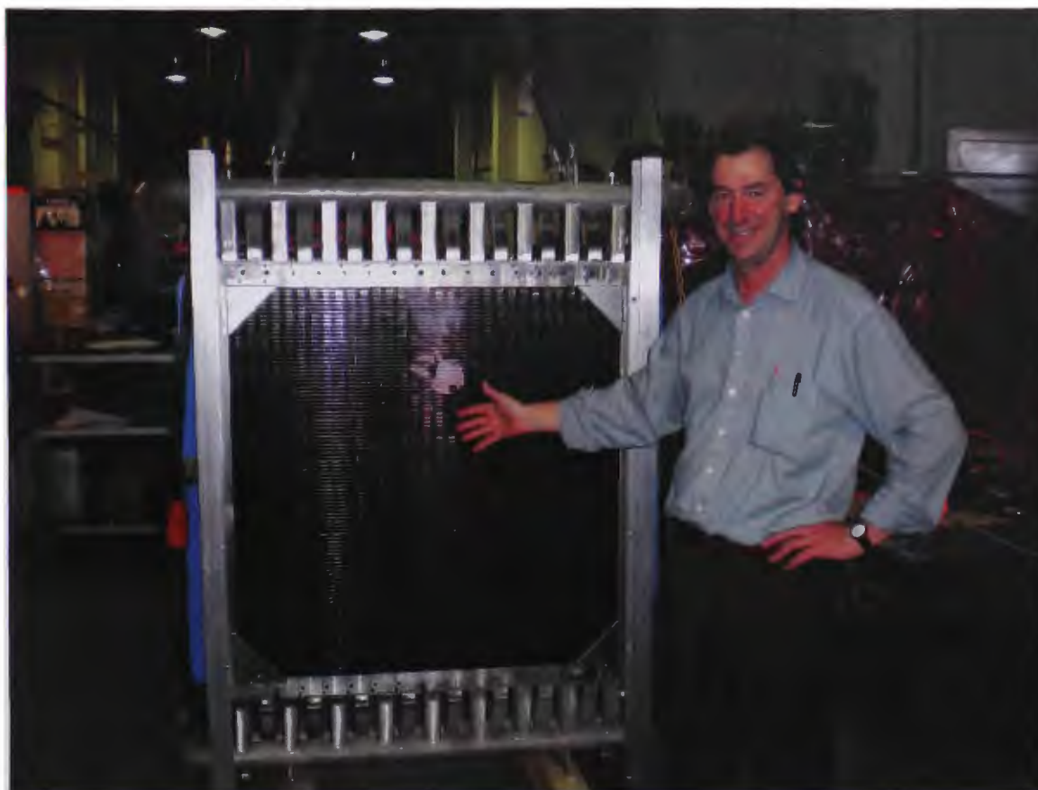
Figure 8-4: The researcher with the world's most powerful CPV array. The array has an area of slightly less than 1\text{m}^2 and a power rating of 140\text{kW} at 500 suns. The 140\text{kW}_{\text{DC STC}} system achieved specified performance with a peak DC efficiency of 25% including optical losses.
