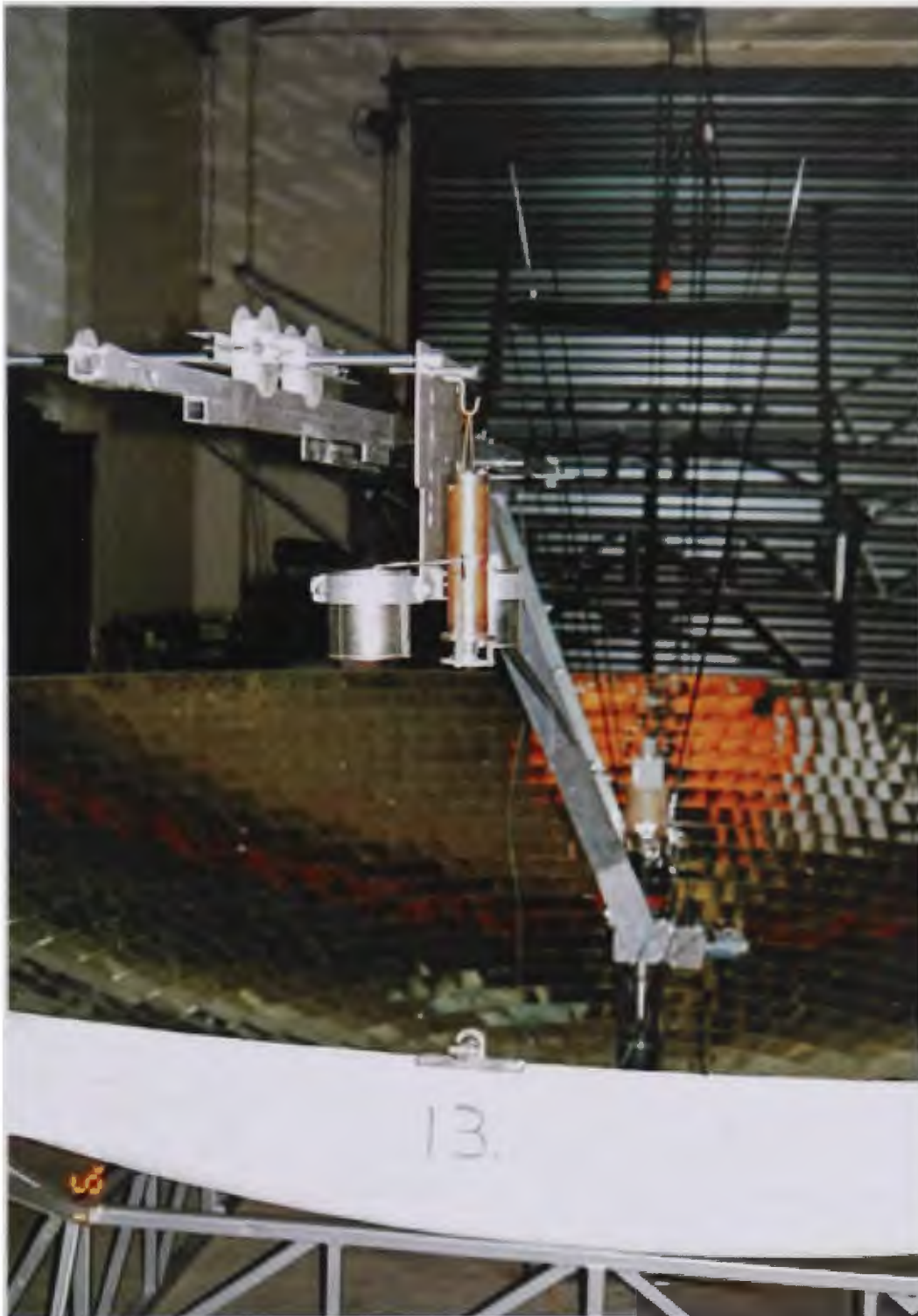
Figure 3-4: Robotic laser mapping alignment system to align mirrors for 20m 2 dish with 3127 faceted mirrors.
