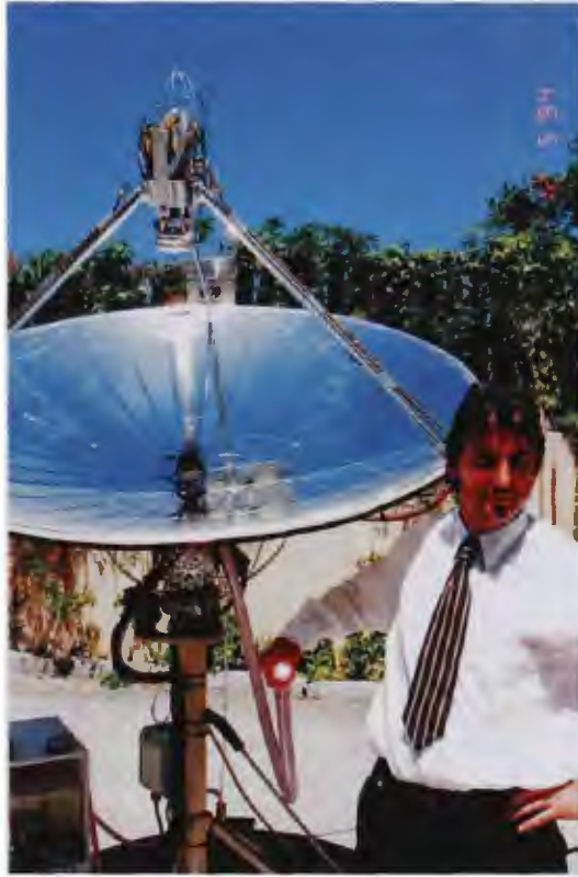
Figure 8-6: The researcher demonstrating a small CPV dish with a spectrum splitter invented by the researcher (Lasich, 1993). Piped light is produced at the same time CPV power is being produced.
