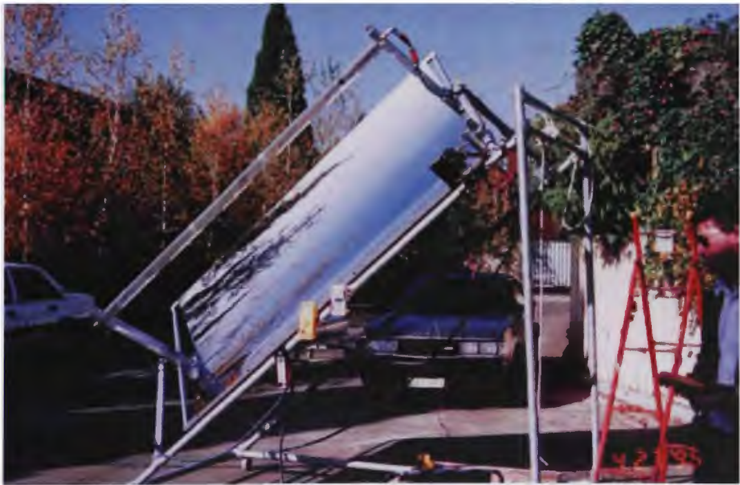
Figure 2-10: Second generation CPV trough built by the researcher using bright anodised aluminium reflectivity of 85% including silicon solar cells. The system is designed and built by the researcher and tested on his premises.
