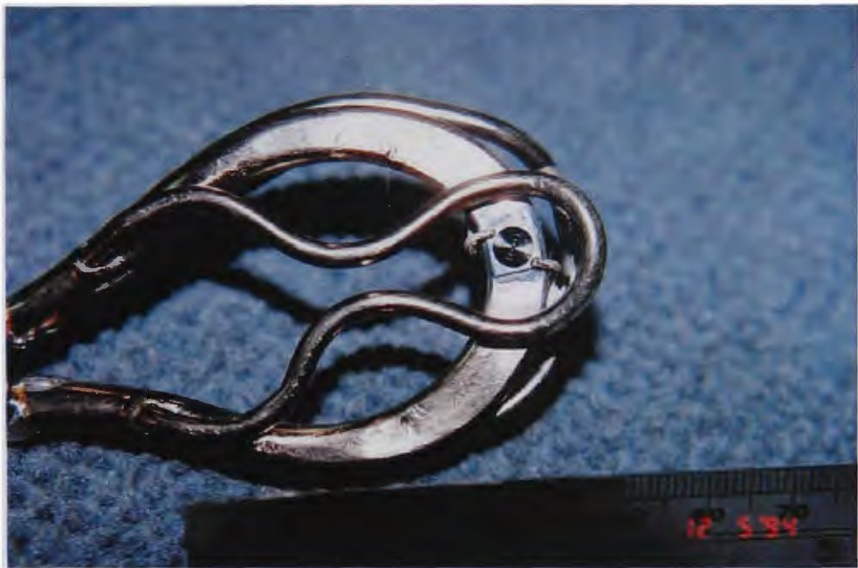
Figure 3-8: Solar Flux measurement ‘wand’ with variant GaAs concentration cell soldered to cooling tube (designed and constructed by the researcher)
