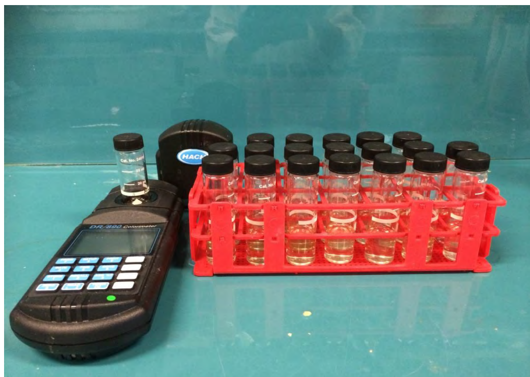
Figure 2 The nitrite nitrogen ( \text{NO}_2\text{-N} ) and the nitrate nitrogen ( \text{NO}_3\text{-N} ) test in wastewater (Influent and Effluents). The equipment used is DR890 colorimeter. Photo by Anusuya Joshi.
