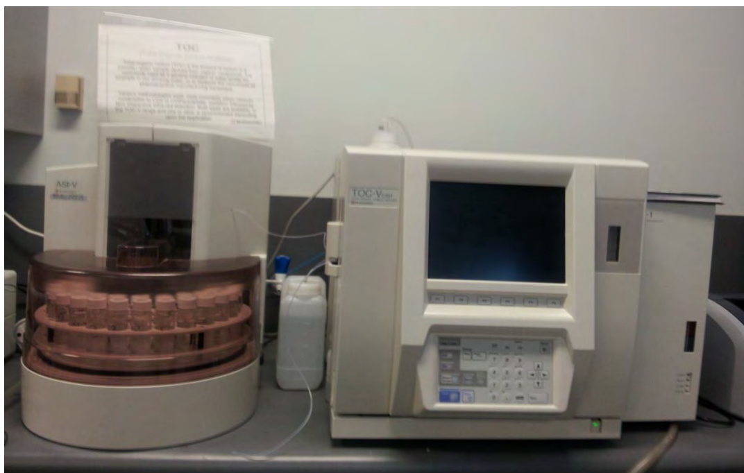
Figure 1 The total organic carbon (TOC) on analyser, used for the determination of the TOC and total nitrogen (TN). Photo by Anusuya Joshi.
