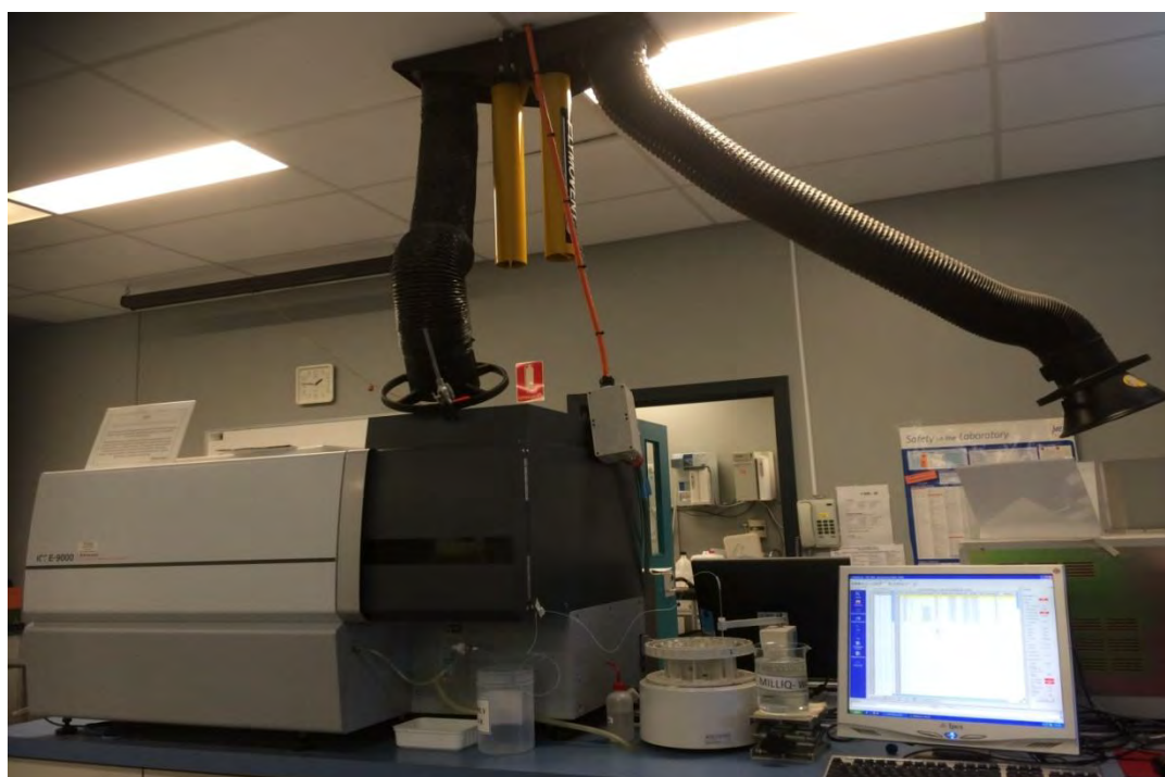
Figure 2 The inductively coupled plasma – optical emission spectrophotometer used for the determination of heavy metals, nutrients and macronutrients. Photo by Anusuya Joshi.
