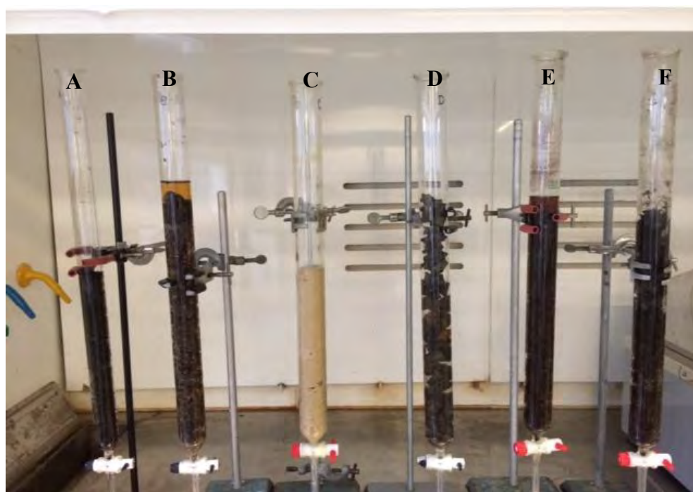
Figure 4.56 Laboratory-based nutrient removal experiments. Glass column containing (A) Soil (B) Soil & earthworms (C) Sand (D) Gravel (E) Mixture of soil, sand, straw, pine bark saw dust (4:1;1:1 v/v) and (F) Mixture of soil, sand, straw, pine bark saw dust (4:1;1:1 v/v) & earthworms.
