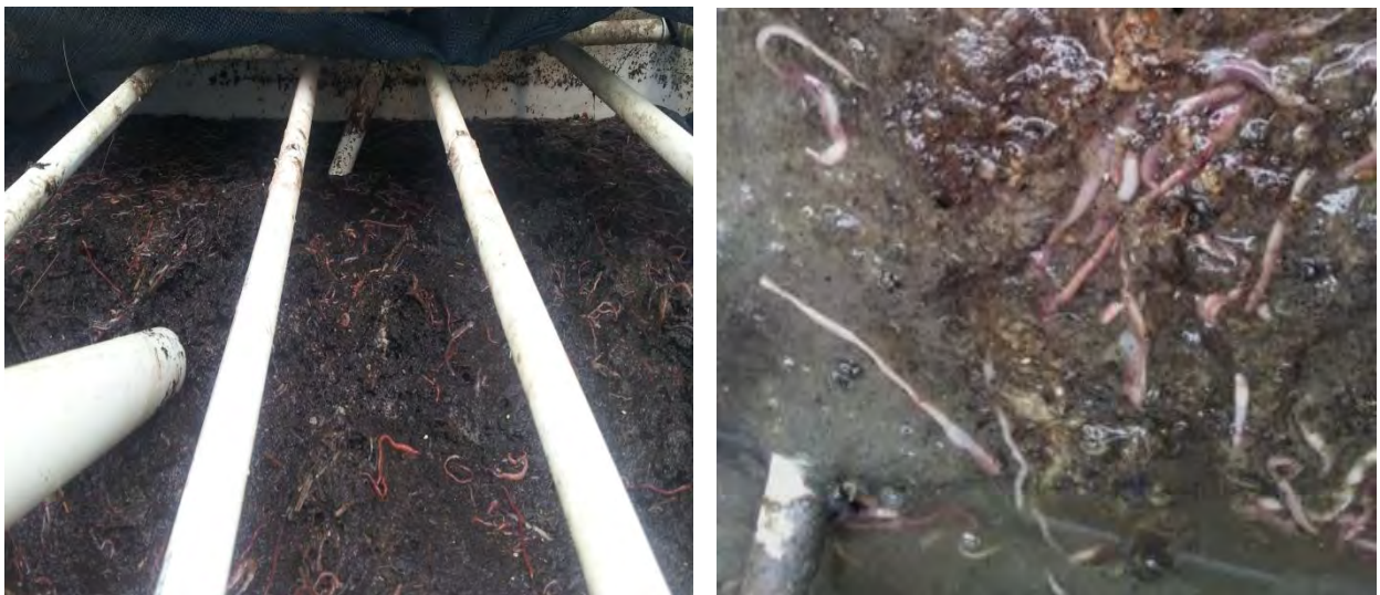
Figure 4.61 Dead worms on the soil layer due to pooling of influent. Worms were observed to come to the surface and tried to escape on the side of the unit. These pictures are from the few occasions when the timer failed and the VF unit received the IN in an uncontrolled way. Photos taken by Anusuya Joshi.
