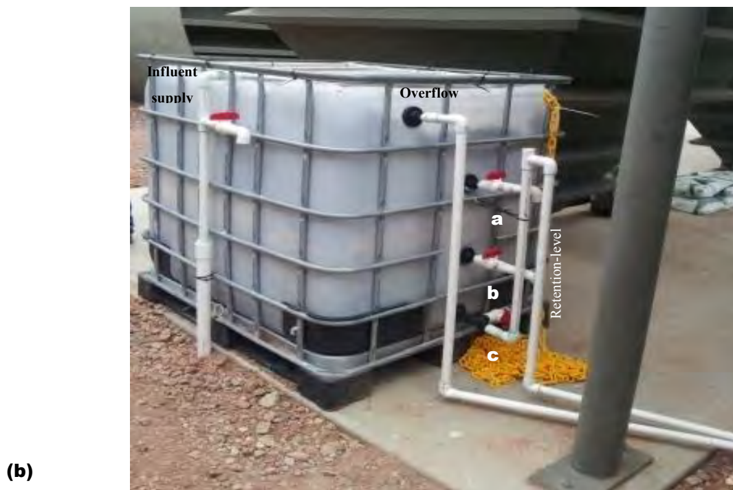
Figure 4.3 (a) Schematic diagram for the Vermifiltration unit (b) the Vermifiltration unit set-up at the SGCTP; a, b & c represents the outlets from Layer 1, Layer 2 & Layer 3 respectively. (S/P submersible pump)
