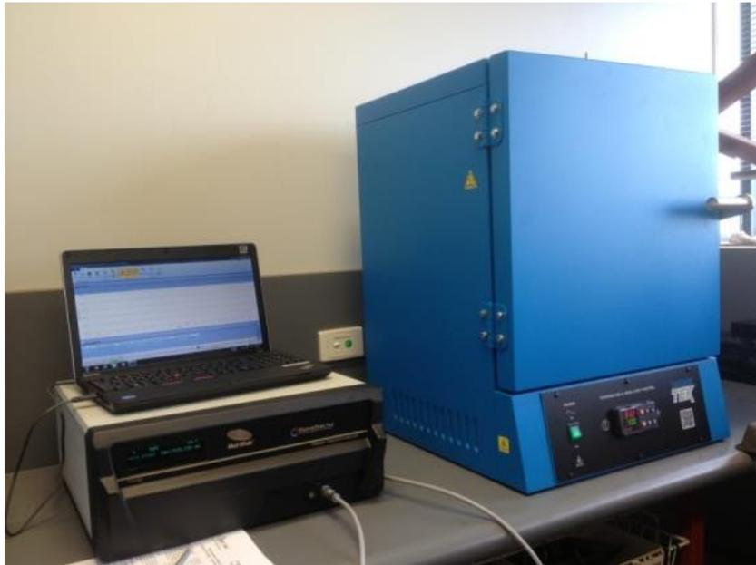
**Figure 2.4: Hot disk thermal constant analyser**
