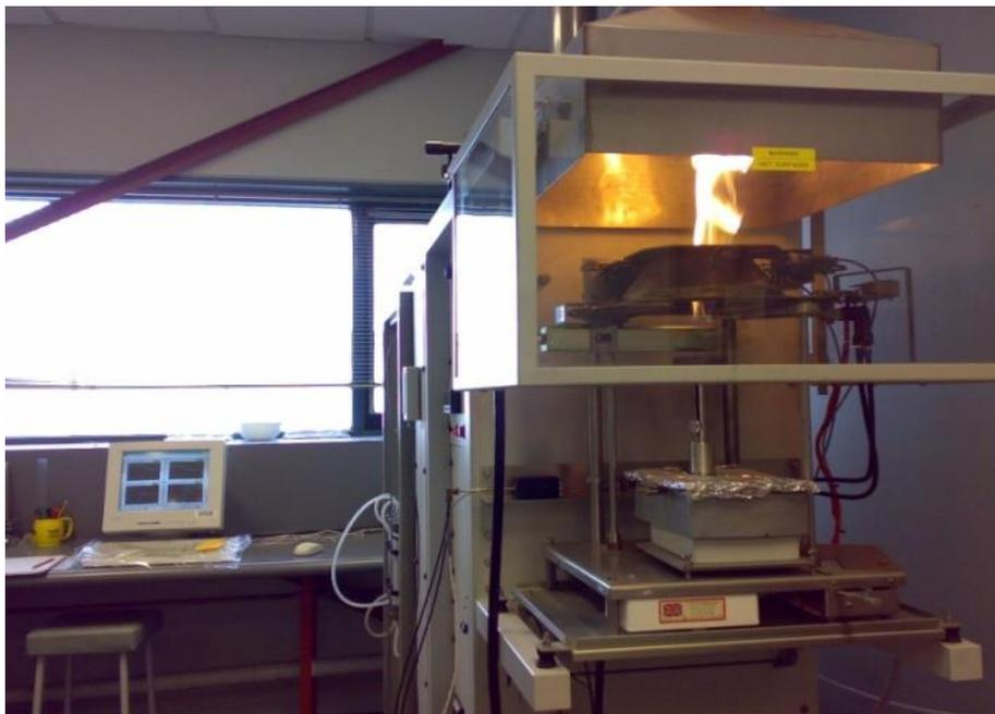
**Figure 2.2: Burning test sample material in the cone calorimeter**
